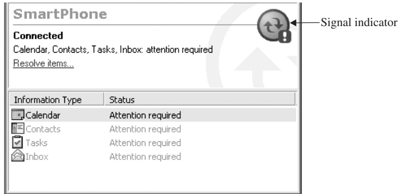
FIGURE 3-2 All Smartphones have a signal strength indicator in the upper-right corner of the screen. It's located next to the battery strength indicator.
