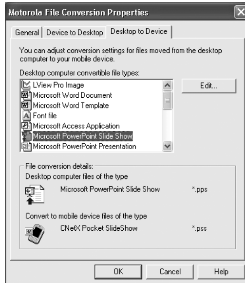
FIGURE 13-4 If you're using the ClearVue Presenter software on your Smartphone to view your PowerPoint files, you must first adjust the conversion settings in ActiveSync.
