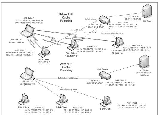
Figure 2.2 Arp Cache Poisoning for MITM Attacks
