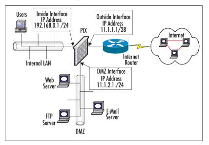
Figure 5.8 PIX Interface Configuration
