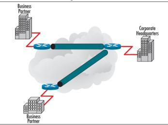
Figure 10.2 VPN Termination at Edge Routers
