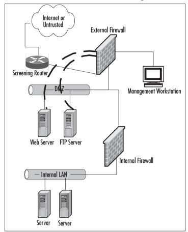
Figure 1.14 A Method to Provide Out-of-Band Management in the DMZ
