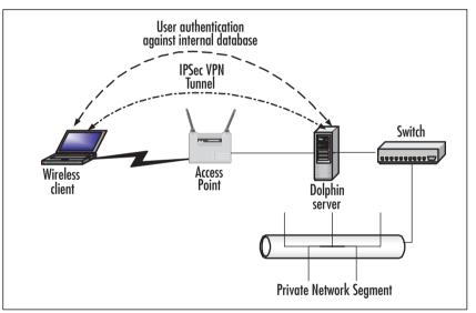
Figure 4.5 shows an overview of how you might implement an EWG on your network to provide security for the wireless segment. In this scenario, the wireless clients authenticate against a RADIUS server with the added benefit of a VPN tunnel being constructed by the EWG to further secure the traffic.
