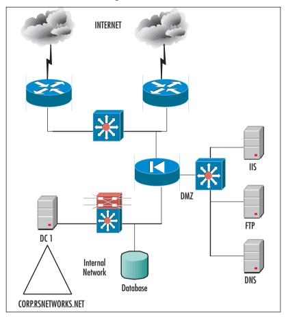
Figure 2.1 Fundamental DMZ Design
