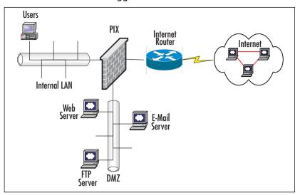
Figure 5.1 Traditional "Three-Legged" Firewall
