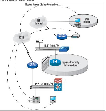
War dialing is your last check on the list for penetration testing. As you can see in the figure, it was pretty simple to get around the firewall. This is really the only way to get past your DMZ (if set up properly, as described in this book), and by probing analog lines, you can very easily and quickly break into a network undetected.
