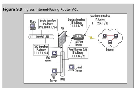
To only allow ICMP echo replies to enter the network from pings originated from the internal network, you must first permit the echo replies, then deny all other ICMP traffic so that pings initiated from the Internet will not be able to enter the network. This is an optional step but can be useful to prevent some DoS attacks.
