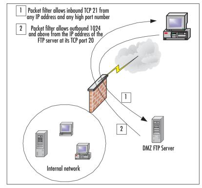
Figure 8.30 Creating Packet Filters to Support a PORT Mode FTP Server
