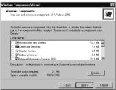
Notice that by default, IIS is selected for installation, but as you can see in the figure, it is deselected here. IIS in Windows 2000 is installed, by default, with virtually all services started, so as soon as a new system is started for the first time, it is immediately susceptible to IIS-based attacks. Rather than taking time out in the initial installation to configure IIS, it's almost always better to hold off on that step until we're ready to concentrate fully on that task.
