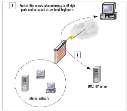
These are the parameters for the packet filter to support the PASV mode FTP in the DMZ:
