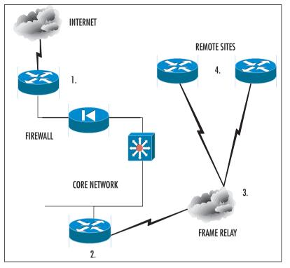
Figure 2.10 A WAN Connected to a Backbone with an Internet Connection
