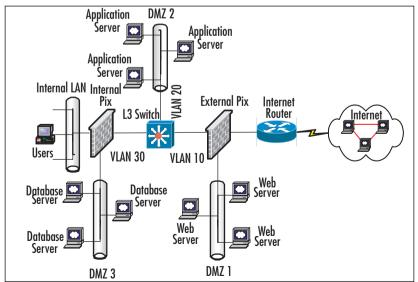
Figure 5.4 An Internal/External Firewall Sandwich
