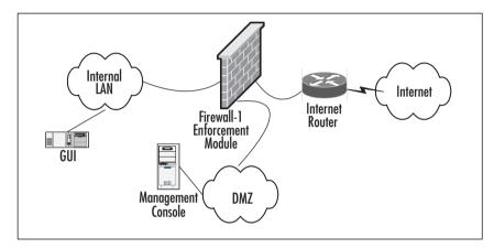
Figure 6.1 "Three-Legged" Firewall with Distributed Check Point Architecture
