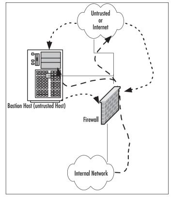
Figure 1.9 A Basic Firewall With Bastion Host Flow
