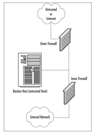
Figure 1.7 A Dual Firewall With a DMZ
