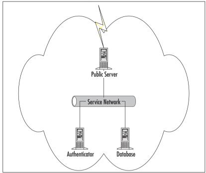
Although some administrators might opt for a firewall to separate the public servers from the private servers, doing so could be overkill. Since we are using a network that is both logically and physically separated, strong host security, including authenticated data communication paths (using IPSec, for example), is sufficient. Additionally, we can avoid the overhead and complexity of introducing a firewall.
