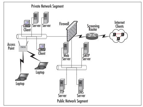
Figure 4.1 Most WLAN Implementations Place the WLAN Inside the Firewall
