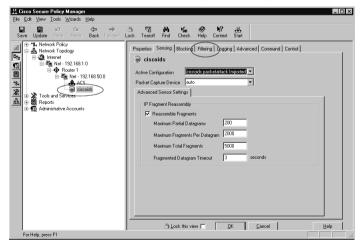
To make adjustments to the sensor to help reduce false positives, use the **Filtering** tab shown in Figure 15.16. This is where we tell the sensor to filter out certain signatures and IP addresses from the list of alarms.
