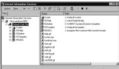
First, stop the Web site by either clicking the **Stop** button (which resembles the Stop button on a VCR) at the top of the MMC, or delete the **Default Web Site** by right-clicking it and selecting **Delete**. And yes, you're sure, so click **Yes** when asked.
