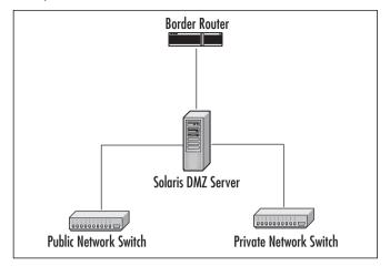
Figure 3.1 Basic Implementation of a Solaris DMZ Server in a Small Network
