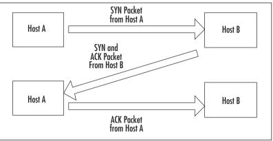
Figure 15.3 TCP/IP Three-Way Handshake
