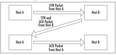
Figure 14.6 A TCP Three-Way Handshake for a Normal Connection
