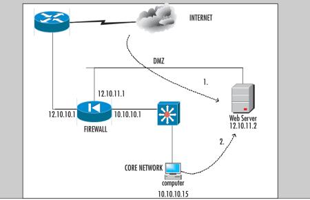
Figure 2.18 Traffic Directed to an IIS System on the DMZ
