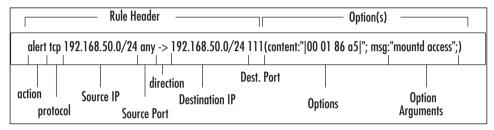
The text in the rule up to the first parenthesis is the *rule header*:
