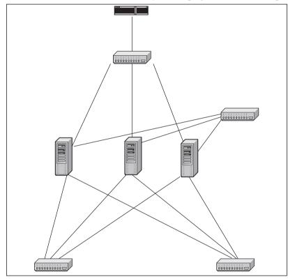
This figure contains many features similar to those in Figure 3.2. However, what is different is that rather than one DMZ system connected to the external network switch, three DMZs are connected to the external network switch. Additionally, there are several connections from these DMZ systems to the same public and private networks. We also see a connection between the DMZ systems.
