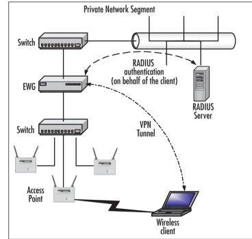
Figure 4.5 Using an Enterprise Wireless Gateway to Control Access
