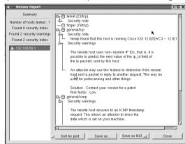
Figure 14.12 A Sample of a Nessus Report from Scanning a Cisco Router
