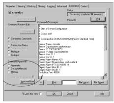
The default for CSPM is to have the approval as manual. This means that before the new configuration information is uploaded to the sensor, you must click the **Approve**
