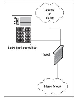
Figure 1.5 Basic Network, Single Firewall and Bastion Host (Untrusted Host)
