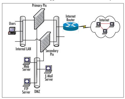
Figure 5.2 Traditional "Three-Legged" Firewall with Redundancy
