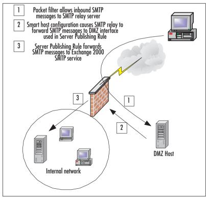
This configuration limits connections to the Exchange 2000 SMTP server publishing rule to the IP address of the ISA server's DMZ interface. In this case, you do not need to create a packet filter to allow the DMZ host access to the IP address of the ISA server's DMZ interface because the DMZ interface is local to the SMTP relay server. The server publishing rule should be configured to allow only the DMZ mail relay server access to the server publishing rule.
