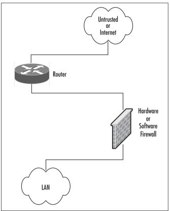
In Figure 1.4, we can see the basic configuration that would be used in a simple network situation in which there was no need to provide external services. This configuration would typically be used to begin to protect a small business or home network. It could also be used within an internal network to protect an inner network that
