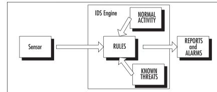
Figure 15.2 Block Diagram Describing the Way IDS Works
