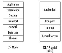
Figure 1.12 The OSI and TCP/IP Models
