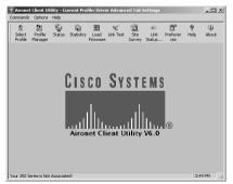
2. Click the **Profile Manager** button to create a new profile, as shown in Figure 11.32. Click the **Add** button to enter the new profile name, and then click the **OK** button to begin configuring the profile.
