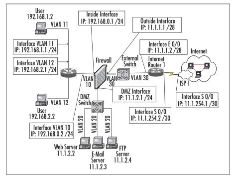
Figure 9.1 Router Placement in a Traditional DMZ Environment
