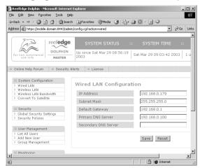
3. Click the **Wireless LAN** link to configure the wireless-side properties, as shown in Figure 11.11.You can change all these properties as you see fit. By
