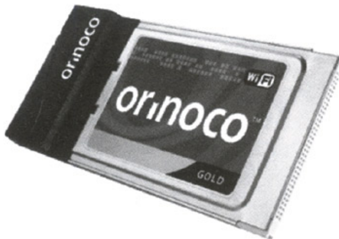
Figure 9.6: Agere Systems ORiNOCO PC Card. The following are some of the key features of ORiNOCO PC Card.
