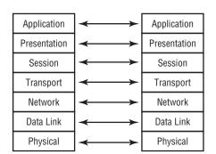
FIGURE 3.3 A representation of the OSI model peer layer logical channels
