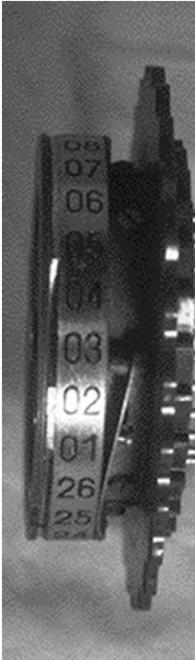
Figure 4.11: An Enigma rotor.
