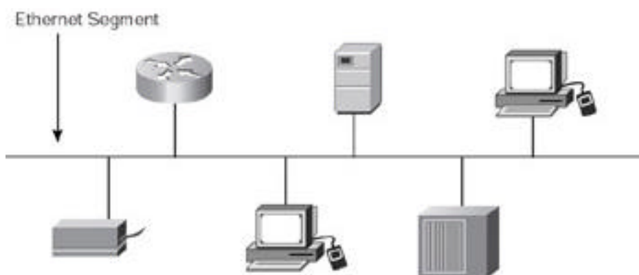
Figure 3.22: An Ethernet segment.
