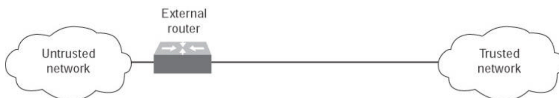
Figure 3.7: A packet-filtering boundary router.
