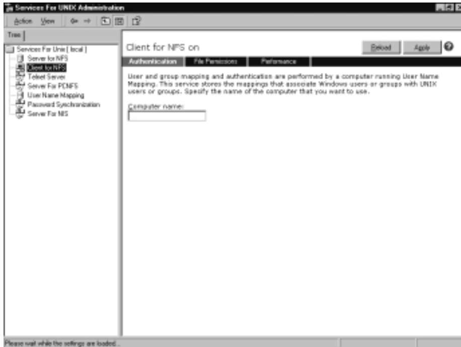
Figure 10.25 Managing the Client for NFS in the Services for UNIX Administration Tool
