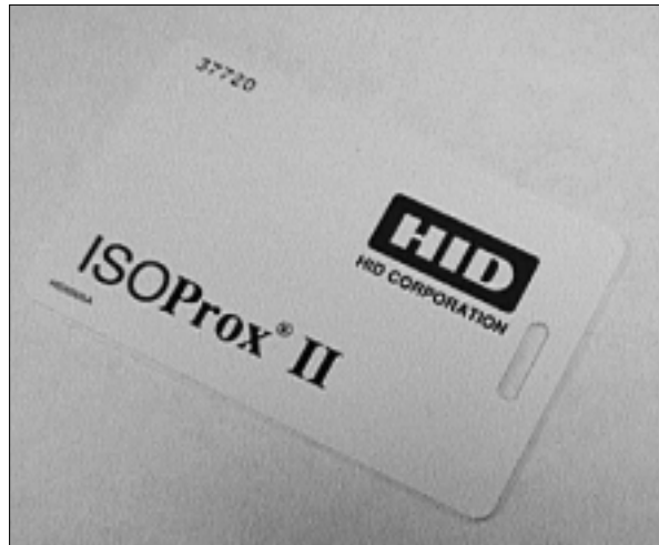
Figure 8.2 A Contactless Smart Card
