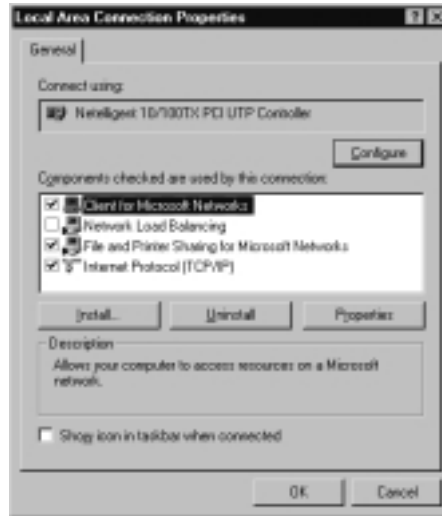
Figure 10.38 The Properties of the Local Area Connection
