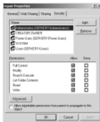
Figure 2.3 Security Permissions for the %Windir%\Repair Directory
