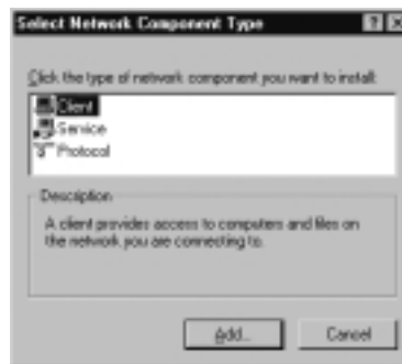
Figure 10.39 The Network Component Type Installation Options
