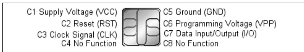
Figure 8.4 Sections of the Contact Pad for a Contact Smart Card Based on the ISO 7816-2 Standard
