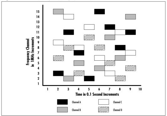
Figure 1.11 Frequency Hopping Spread Spectrum
