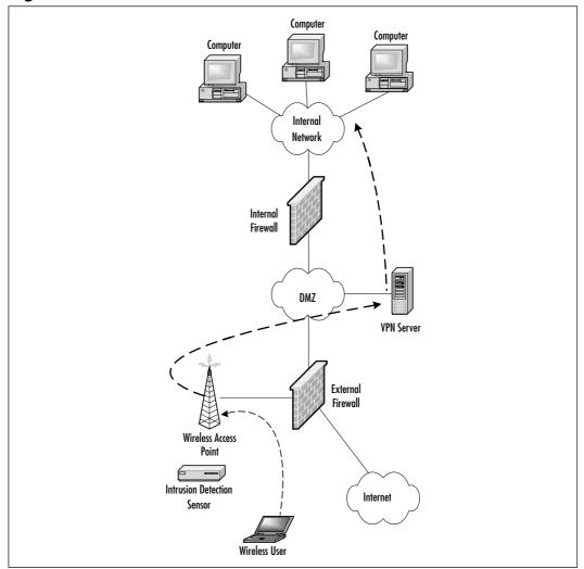
Figure 9.3 A More Secure, Dual-firewall Solution
