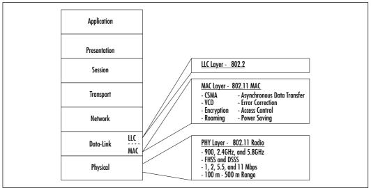
IEEE 802.11 wireless LAN networks are designed to provide wireless connectivity to a range of roughly 300 feet from the base. The lead application being shared over the wireless LAN is data. Provisions are being made to accommodate audio, video, and other forms of streaming multimedia.
