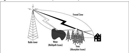
Figure 3.2 Fresnel Zone: Absorption and Multipath Issues
