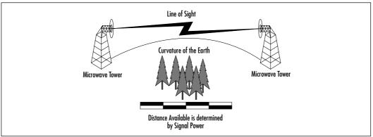
Figure 3.5 Point-to-Point Microwave
