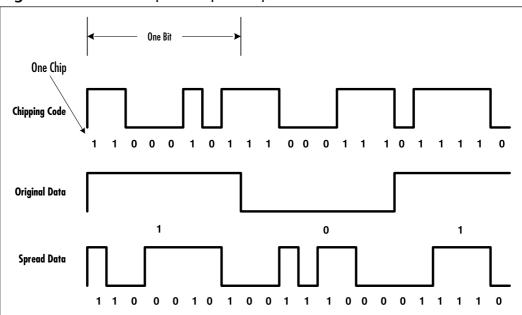
Figure 1.12 Direct Sequence Spread Spectrum
