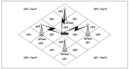
Figure 3.13 Basic Cell Architecture
