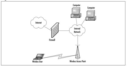
Figure 9.1 An Out-of-the-box Unsecure Wireless Network
