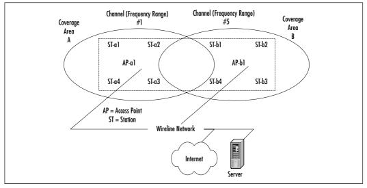
Since multiple Access Points exist in this model, the wireless devices no longer communicate in a peer-to-peer fashion. Instead, all traffic from one device destined for another device is relayed through the AP. Even though it would look like this would double the amount of traffic on the WLAN, this also provides for traffic buffering on the AP when a device is operating in a low-power mode.
