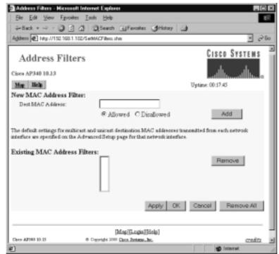
Figure 5.9 illustrates what the Cisco Aironet 340 AP interface looks like when MAC addresses have been entered into the configuration. As you can see, MAC address 00:02:2D:09:7E:C3 has been disallowed, while 00:02:2D:09:7E:C3 has been allowed. Note that the 00:02:2D points out the hardware manufacturer of the wireless card, while the remainder of the address is the globally unique identification number within that manufacturer's license.
