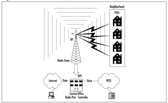
Figure 3.4 Wireless Local Loop Architecture
