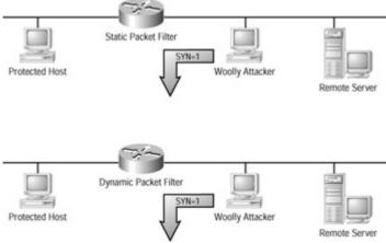
Figure 5.8: Both filtering methods can block a port scan.
