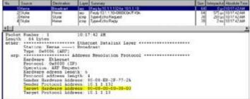
Figure 3.1: A transmitting system attempting to discover the destination system's node address
