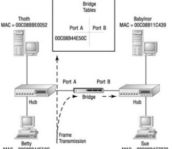
MAC = 00C08B44E50C MAC = 00C08B477B72 **Figure 4.9:** Betty transmits data to the server Thoth by putting Thoth's MAC address into the destination field of the frame.
