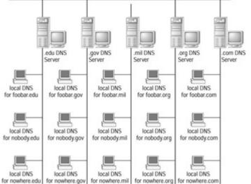
Figure 3.18: A visual representation of the hierarchical structure of DNS
