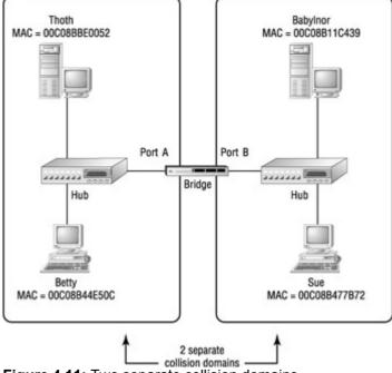
Figure 4.11: Two separate collision domains
