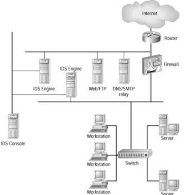
Figure 8.4: A potential deployment of two IDS sensors
