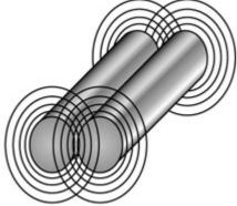
Copper wire conducting AC signal Figure 4.3: A conductor carrying an AC signal radiating EMI
