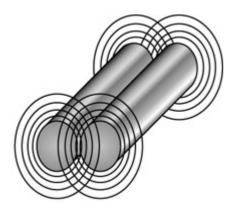
Copper wire conducting AC signal Figure 4.3: A conductor carrying an AC signal radiating EMI
