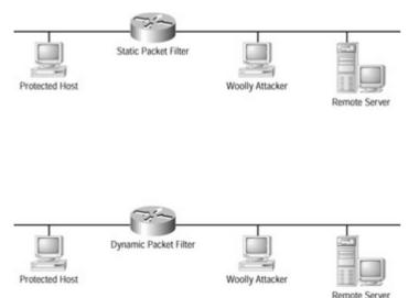
Figure 5.5: The differences between static and dynamic packet filtering
