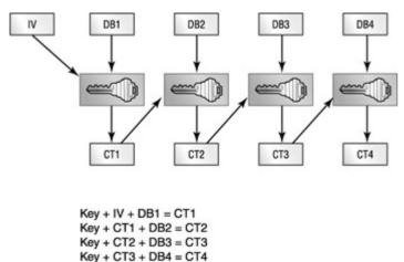
Figure 9.6: Block cipher encryption
