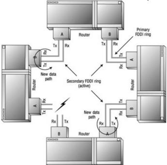
Figure 12.2: How FDDI stations recover from a cable failure
