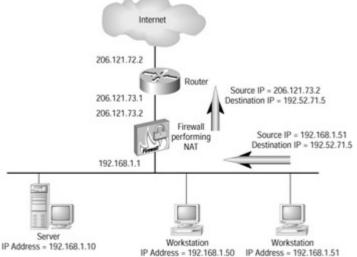
**Figure 6.1:** Our router does not need a route entry for the internal network because the firewall is performing NAT.
