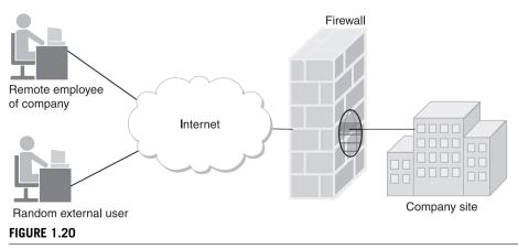
A firewall filters packets flowing between a site and the rest of the Internet.
