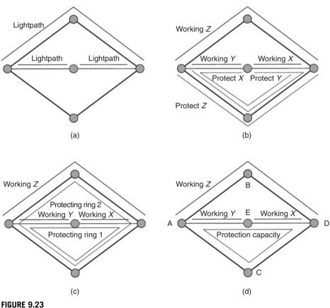
Example to illustrate the bandwidth efficiency of mesh protection relative to ring protection. (a) A mesh network with three lightpaths present. (b) Protecting the lightpaths using 1 + 1dedicated protection. (c) Protecting the lightpaths using OCh-SPRing protection. (d) Protecting the lightpaths using OCh-mesh protection.
