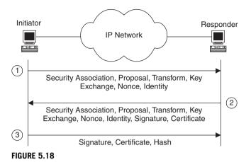
The number of messages exchanged to set up a security association can be kept down to just three using the Aggressive Exchange.
