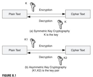
Symmetric cryptography and asymmetric cryptography.
