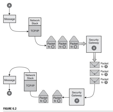
Using a secure tunnel.
