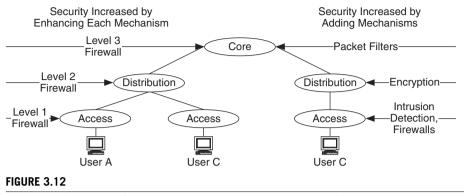
The Access/Distribution/Core architectural model as a starting point for security.
