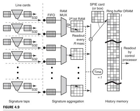
Hardware implementation of packet logging using Bloom filters. Note the use of two-level memory: SRAM for random read-modify-writes and DRAM for large row writes.
