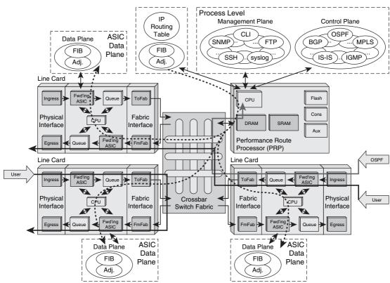
Figure 1-17 Distributed ASIC-Based Router Architecture
