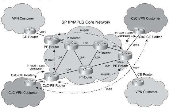
Figure 2-16 Carrier Supporting Carrier MPLS VPN Model
