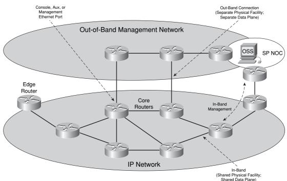
Figure 6-1 In-Band and Out-of-Band Management Architecture
