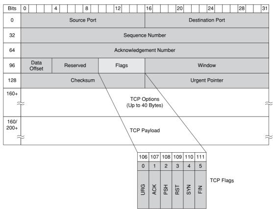
Figure B-2 TCP Header
