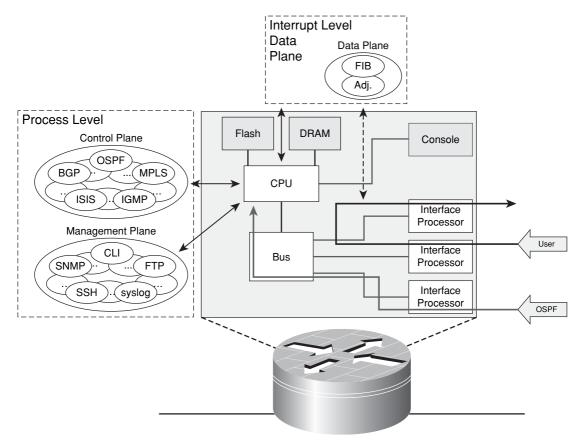
Figure 1-14 Centralized CPU-Based Router Architecture
