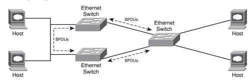
Figure 5-14 Spanning Tree Protocol BPDUs
