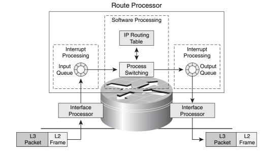
Figure 1-11 Illustration of Process Switching
