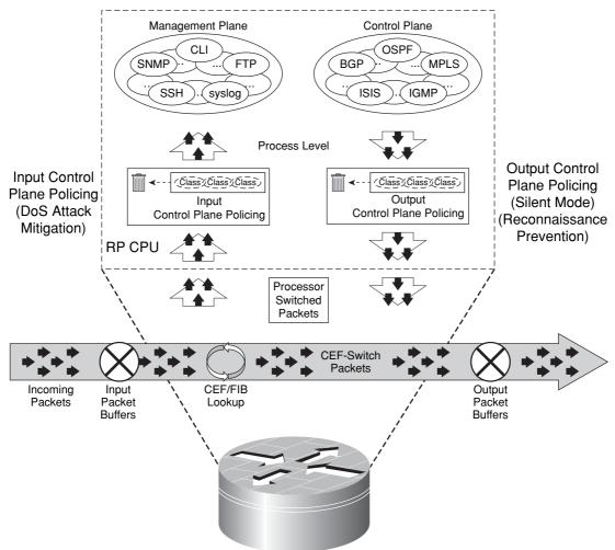
Figure 5-6 Control Plane Policing Conceptual View
