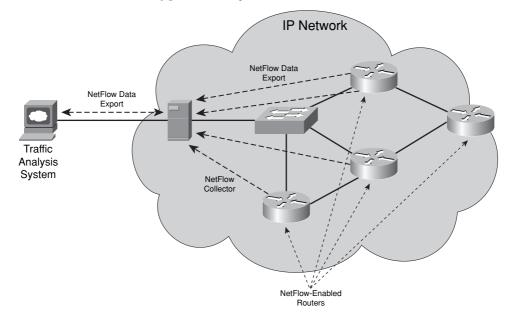
Figure 6-4 NetFlow Network Configuration Example
