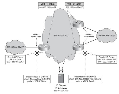
Figure 4-7 VRF Mode uRPF Source Address Verification Example
