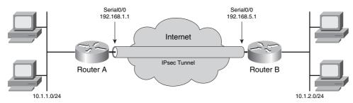
Figure 7-5 IPsec VPN Deployment Using ESP Tunnel Mode
