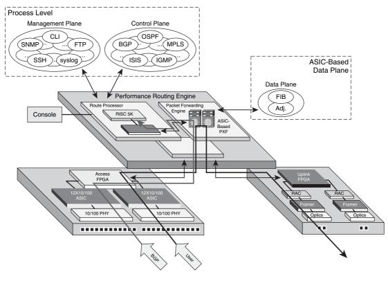
Figure 1-15 Centralized ASIC-Based Router Architecture
