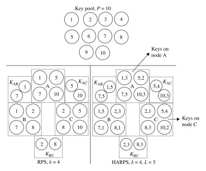
Figure 3.9. Illustrating the working of RPS and HARPs.
