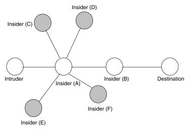
Figure 5.4. Use of redundancy to address node failures.
