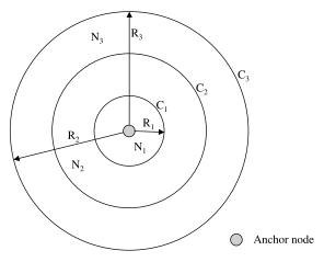
Figure 7.20. An anchor with three power levels.
