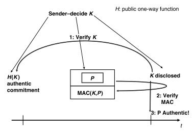
Figure 2.11. Basic operation of TESLA.
