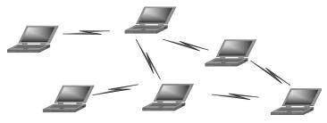
Figure 1.5. Ad hoc mode architecture using 802.11 technology.
