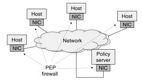
Figure 6.6. Distributed firewall architecture.
