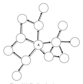
Figure 4.16. Flooding of routing messages.
