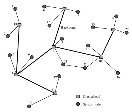
Figure 3.8. Secure communication structure imposed by backbone of clusterheads.
