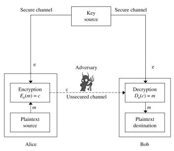
Figure 2.2. Model of a symmetric key encryption system.
