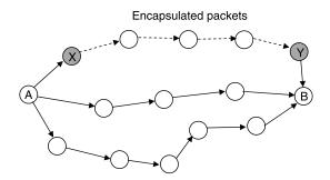
Figure 4.29. Wormhole attack (encapsulated packets).
