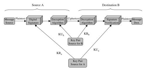
Figure 2.3. Operation of an asymmetric key system providing both confidentiality and authentication.
