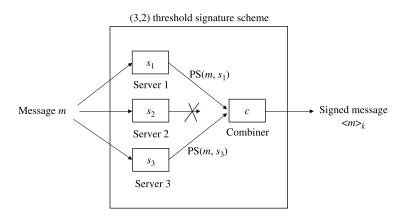
Figure 3.5. Example of signature generation with threshold cryptography.
