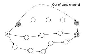
Figure 4.30. Wormhole attacks (out-of-band channel).
