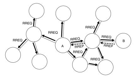
Figure 4.2. Illustration of the AODV routing protocol. In this case node A desires to find a route to node B.
