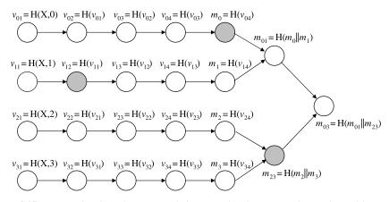
Figure 4.15. Tree-authenticated one-way chain (to authenticate a routing update with sequence number 1, metric 1, the shaded values have to be used).
