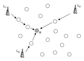
Figure 7.5. Hop count-based scheme. The shaded node determines the hop count from the three anchors and uses this to determine its location.
