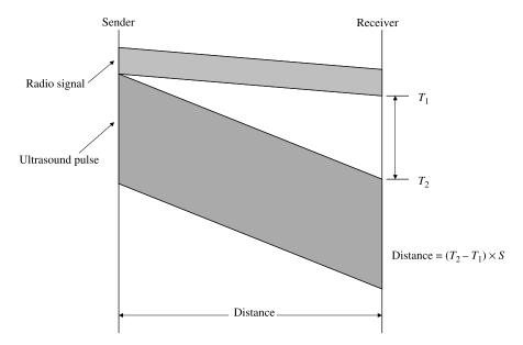
Figure 7.4. Distance estimation using time-of-flight measurements with both ultrasound and radio signals.
