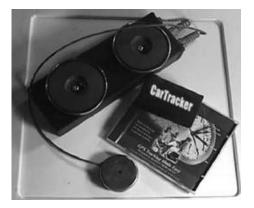
Figure 14.1 Commercially available covert vehicle tracker using GPS.
