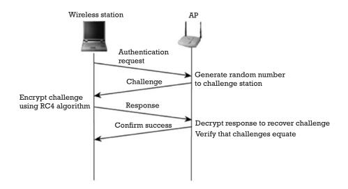
Figure 13.1 Handshaking protocol in Wi-Fi.
