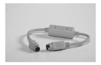
Figure 4.3 Keyghost keystroke-capturing device without adaptors.
