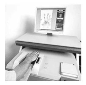
Figure 15.2 Palm-based biometric reader.
