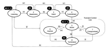
*Figure 4.* The local state model of the overall control system as coordination and interaction messages are passed between the controllers and their threads respectively. Each state is also labeled with its designated coordinator - AC: Access Controller; IC: Interaction Controller
