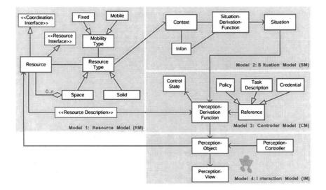
Figure 2. UML Diagram for Authorized Transient Control Management System, showing four component models and their interfaces
