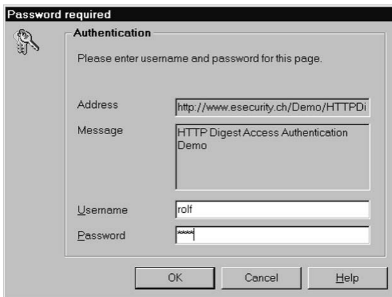
Figure 2.3 The Opera 6.0 'Password required' prompt using the HTTP digest access authentication scheme. (© 2002 Opera Software.)
