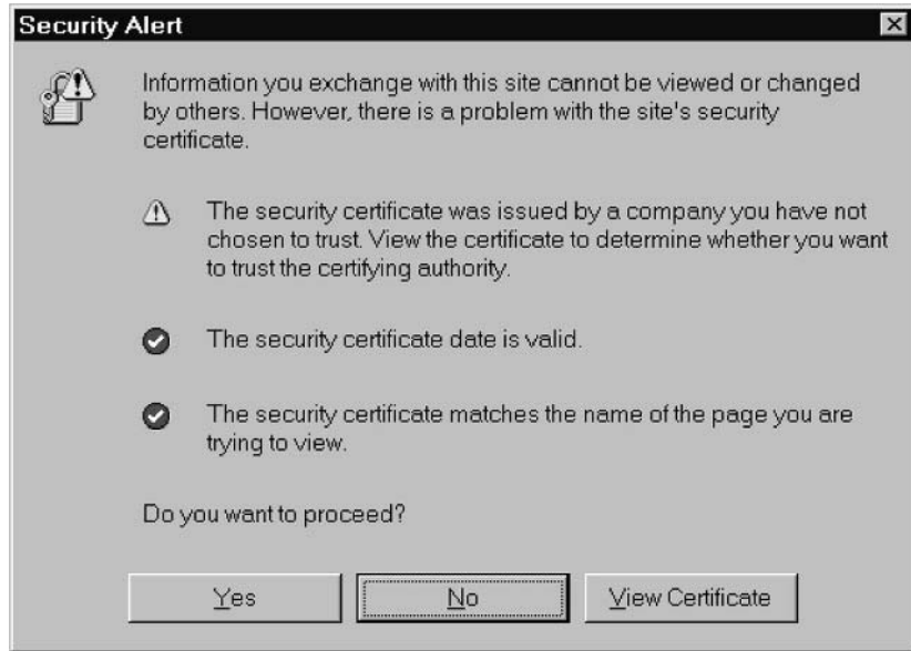
Figure 7.2 Microsoft Internet Explorer's Security Alert panel, which is displayed if the browser does not know or trust a server or site certificate. (© 2002 Microsoft Corporation.)
