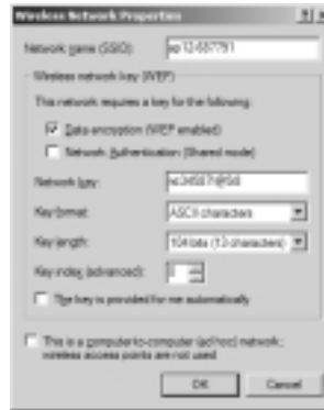
Figure 4.11 Configuring a Static WEP Key on Windows XP
