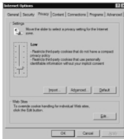
Figure 5.12 Cookie Options Can Be Set in IE via the Privacy Tab in Internet Options
