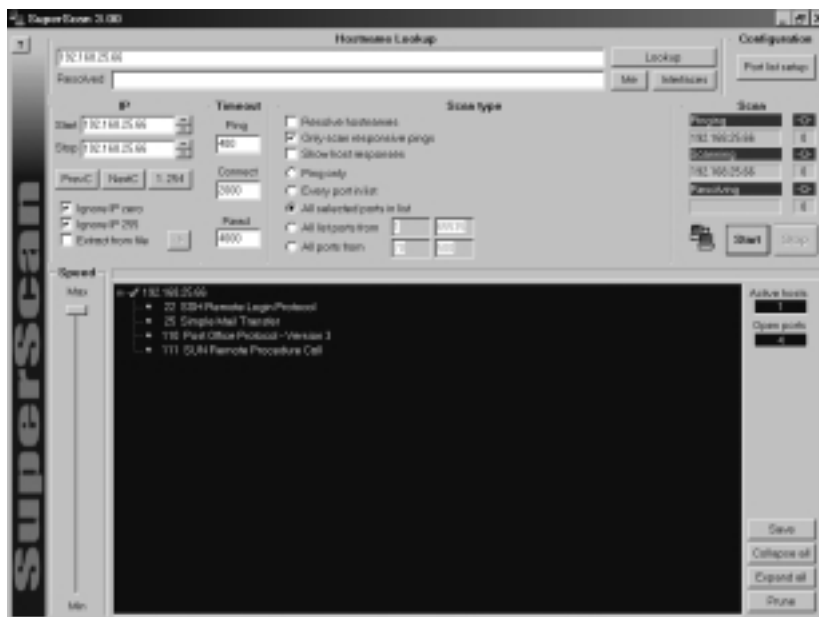
Figure 8.5 Displaying UNIX-based Open Ports After Scanning
