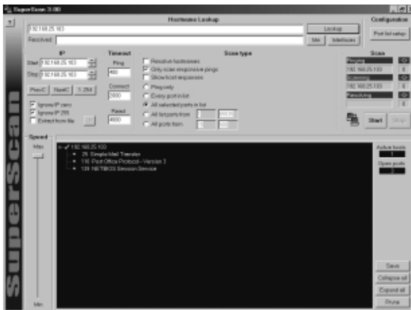
Figure 8.3 Displaying Open Ports on a Win9.x Machine After Scan
