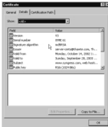
Figure 10.4 The “Details” Tab of a Certificate
