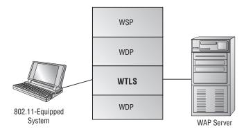
The Wireless Session Protocol (WSP) manages the session information and connection between the devices. The Wireless Transaction Protocol (WTP) provides services similar to TCP and UDP for WAP. The Wireless Datagram Protocol (WDP) provides the common interface between devices. Wireless Transport Layer Security (WTLS) is the security layer of the Wireless Application Protocol and is discussed in detail in Chapter 4.
