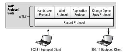
FIGURE 4.16 WTLS used between two WAP devices
