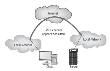
VPNs are becoming the connection of choice when establishing an extranet or intranet between two or more remote offices. The major security concern when using a VPN is encryption. PPTP offers some encryption capabilities, although they're weak. IPSec offers higher security, and it's becoming the encryption system used in many secure VPN environments.
