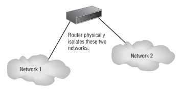
Routers are intelligent devices, and they store information about the networks to which they're connected. Most routers can be configured to operate as packet-filtering firewalls. Many of the newer routers also provide advanced firewall functions.
