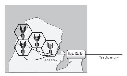
The individual cells have a high level of computer intelligence, and they hand off conversations to each other automatically. Cell phones in the United States operate in the 824MHz to 894MHz range. The Federal Communications Commission (FCC) requires police scanners to bypass these frequencies in the United States; most other countries don't require this frequency blocking in communications equipment.
