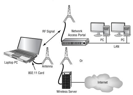
FIGURE 3.10 Wireless access point and workstation
