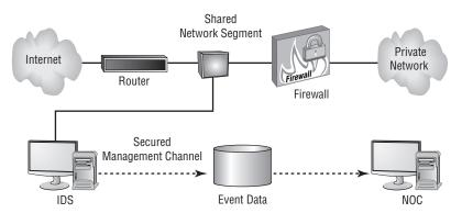
FIGURE 4.9 N-IDS placement in a network determines what data will be analyzed.
