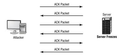
In this attack, the client continually sends and receives the ACK packets but doesn't open the session. The server holds these sessions open, awaiting the final packet in the sequence. This causes the server to fill up the available sessions and deny other clients the ability to access the resources.
