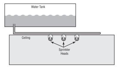
The one drawback to water-based systems is that they cause extreme damage to energized electrical equipment such as computers. These systems can be tied into relays that terminate power to computer systems before they release water into the building.
