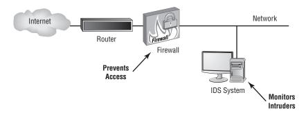
In the event the firewall is compromised or penetrated, the IDS can react by disabling systems, ending sessions, and even potentially shutting down your network. This arrangement provides a higher level of security than either device provides by itself.
