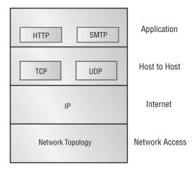
The four layers of TCP/IP have unique functions and methods for accomplishing work. Each layer talks to the layers that reside above and below it. Each layer also has its own rules and capabilities.
