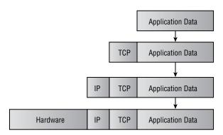
FIGURE 2.7 The encapsulation process of an e-mail message
