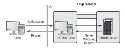
The major difficulty with a single-server RADIUS environment is that the entire network may refuse connections if the server malfunctions. Many RADIUS systems allow multiple servers to be used to increase reliability. All of these servers are critical components of the infrastructure, and they must be protected from attack.
