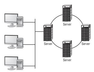
FIGURE 8.1 Server clustering in a networked environment
