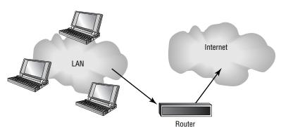
FIGURE 1.10 A typical LAN connection to the Internet
