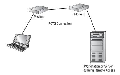
The RAS connection is accomplished via dial-up or network technologies such as VPNs, ISDN, DSL, and cable modems. RAS connections may be secure or in the clear, depending on the protocols that are used in the connection.
