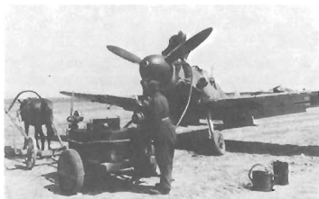
9. Local transport is pressed into use to tow an oil refuelling bowser. Note the retention of a single letter 'Q' under the port wing of the Bf109F, and the Bf108 in the background.
