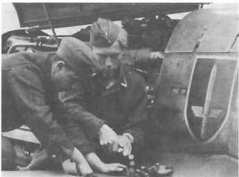
38. Armourers of JG 52 load 20mm shells for the underwing cannon of one of the unit's Bf109Gs.
