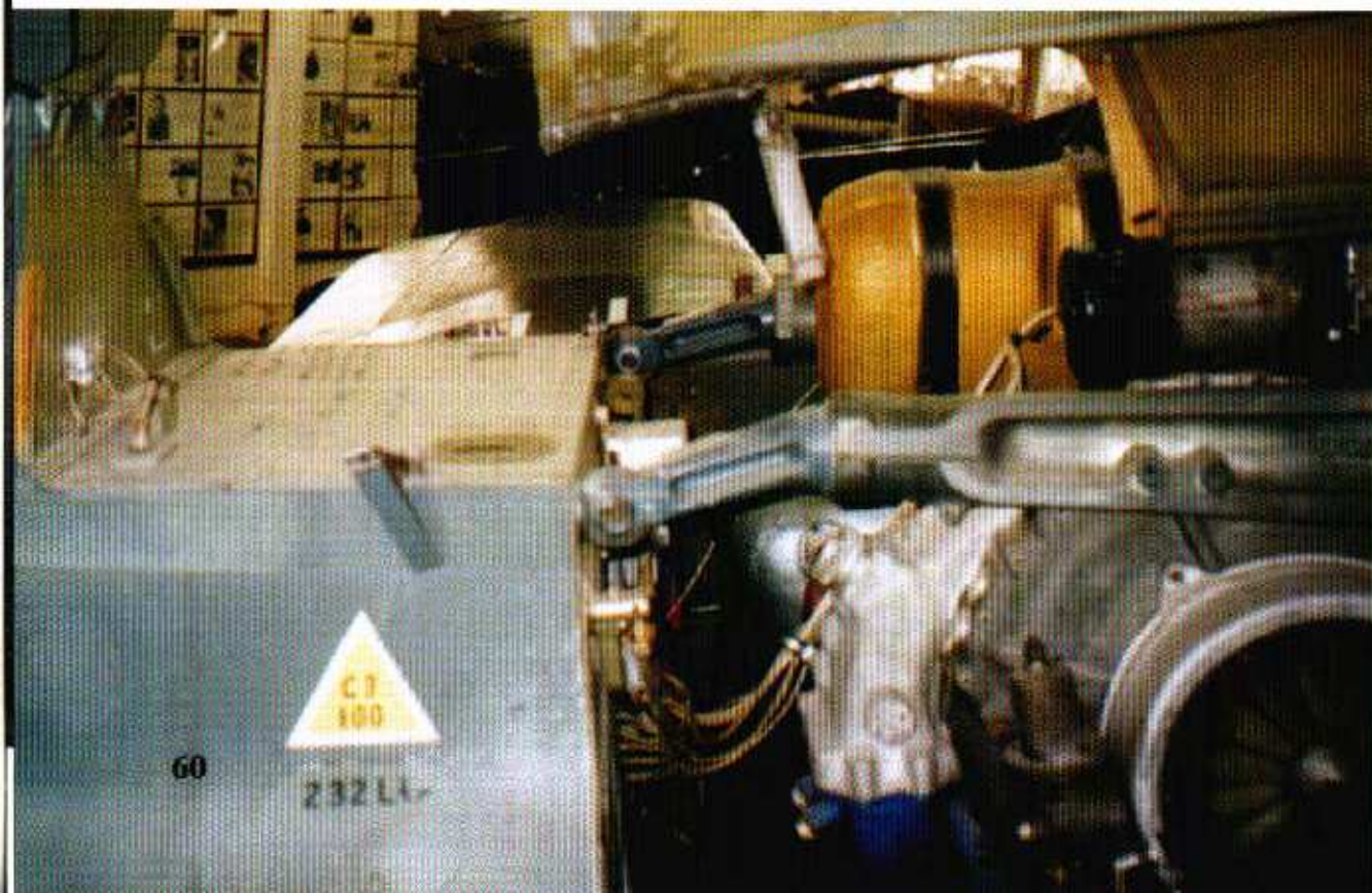
The engine compartment panels fold upward on each side, while the gun panel opens aft and lays flat against the armored windscreen. With no room to spare it is easy to see why the upper engine bearer links must bend downward to attach to the fuselage. (Author: Laing via Goss)
