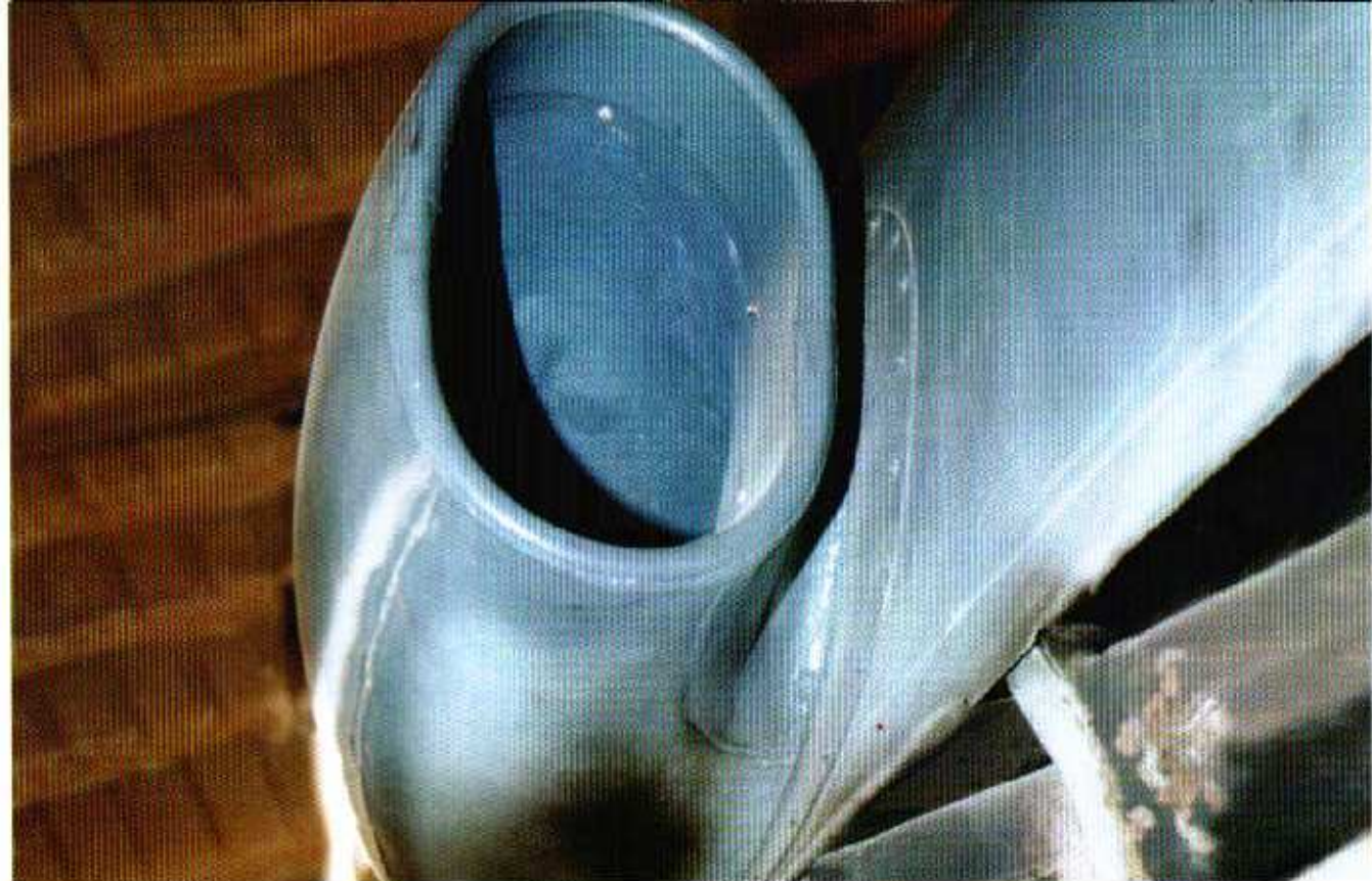
(Above and below) The size and shape of the later model intake found on the Fw 190D-11/12/13 and Ta 152 is much larger than the intake found on the earlier Fw 190D-9. The intake did not lie against the fuselage side and was made by welding together several component pieces. (Author: Ryle)
