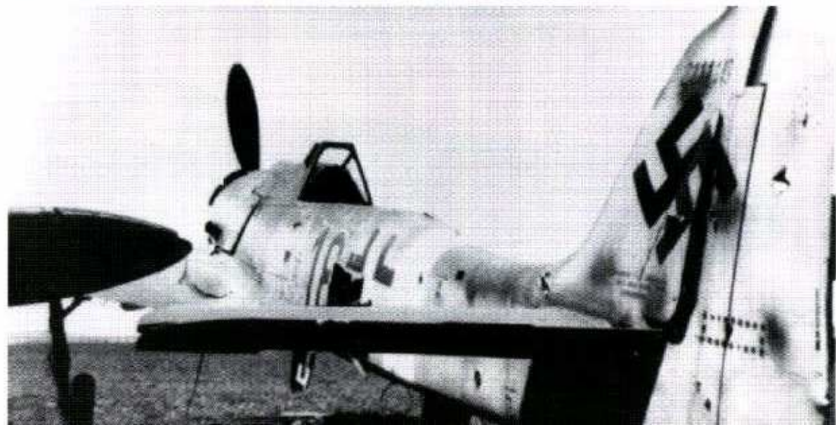
(Above and below) Black 18, an Fw 190D-9 (W.Nr. 211115) at Pilsen, Czechoslovakia in 1945, is believed to be an aircraft of JG 3. The machine has the port fuselage access panel removed as well as the radio access panel on the starboard side. Under the fuselage/wing center the 20mm ammo bay door is open and hanging down. (J. V. Crow)
