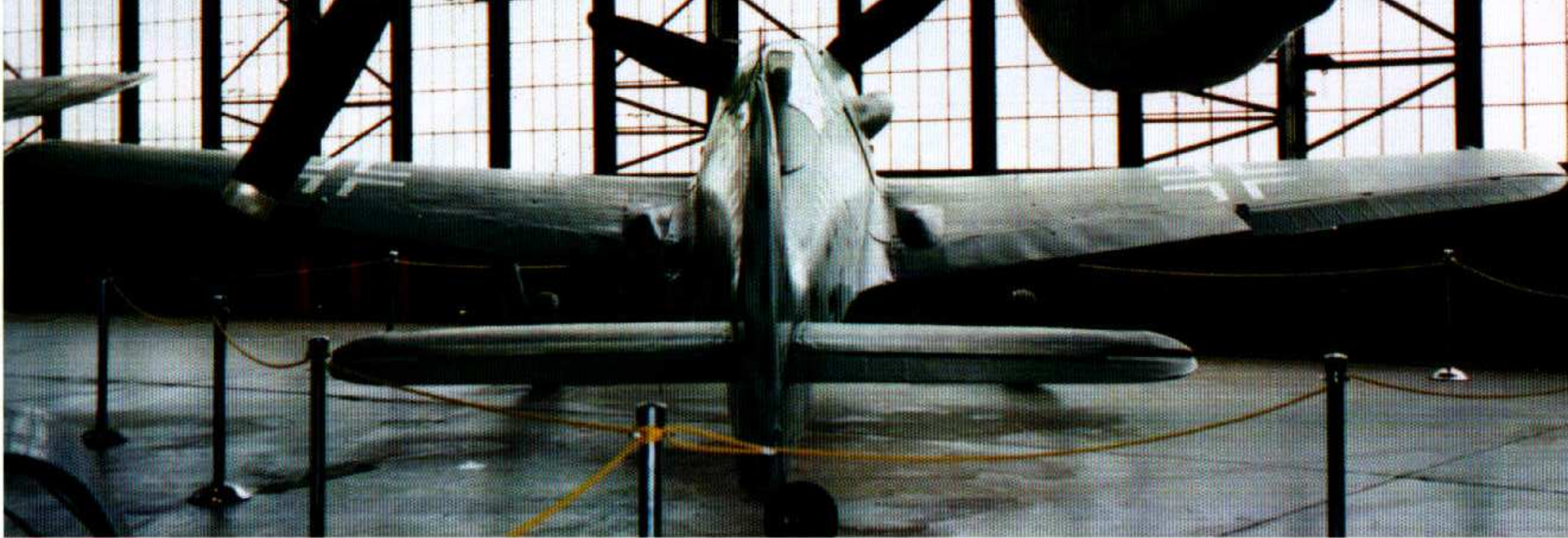
The Fw 190D-9 from the rear, the preferred view of Allied pilots. The taper from the thick forward fuselage to the thin tail assembly is evident. The tail wheel is turned 90 degrees to the right. (L & J Wahsum)
