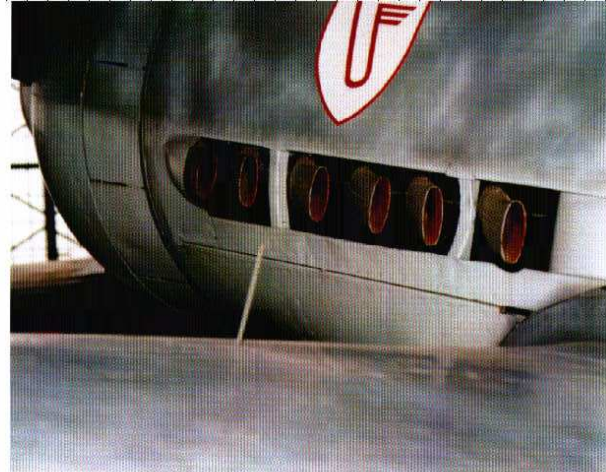
(Above) The oval shaped exhausts pipes have weld lines on both the front and back side of each exhaust. The rod extending upward from the wing top is the visual wheel position indicator rod. The top of the rod is usually painted red over a bottom of white. (J. Bishop)
