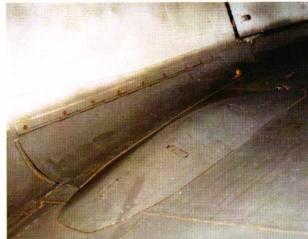
The access panel was bulged to accommodate the MG 151 20mm cannon. The access panel is attached to the fuselage with nine small screws, the "piano" hinge may be seen just below the screws. (J. Bishop)
