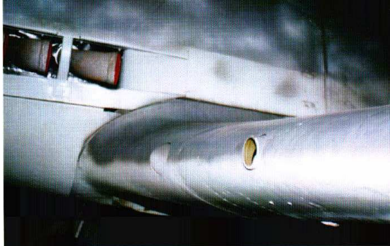
(Above and below) The port wing leading edge showing the empty wing root cannon port and the gun camera port. While the 20mm cannon port was produced as a part of the wing's leading edge panel, the camera port is a separate piece riveted into the leading edge of the wing panel. The glass cover on the camera port (missing) was exchangeable for a colored light filter. (D. Ryle)
