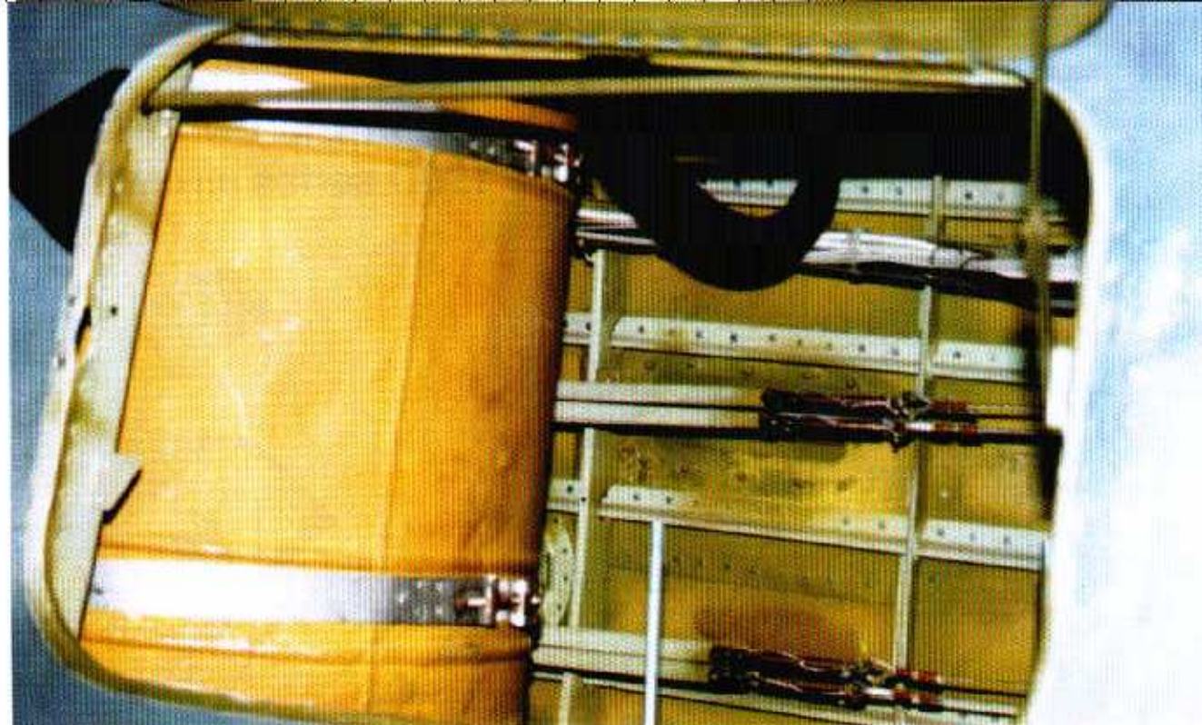
The Yellow 115 liter auxiliary fuel tank was used for either fuel or methanol for the MW 50 power booster. The elevator control cables run along the starboard side of the fuselage. (Author: Ryle)
