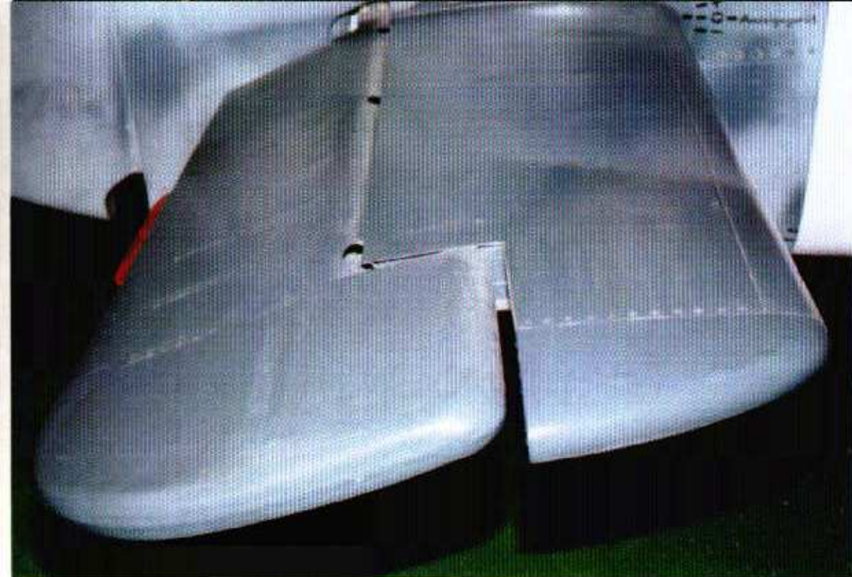
(Above and below) The replica horizontal stabilizer with the elevator in the full up and full down position. The horizontal stabilizer is all metal construction, while the elevator, like the rudder, is cloth over metal frame construction. The cloth is stitched to the elevator's frame, taped over, then the assembly is painted the same as the other parts of the aircraft. However, the difference in light reflection between the cloth covered parts and the metal parts almost made the fabric surfaces look like they were a different color. (Author: Ryle)
