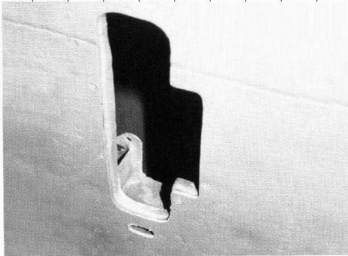
The disposal cartridge and link chute for the inboard wing mounted MG151 20mm cannon. The small hole aft of the chute opening was used to access the mounting screw for the internally fitted chute (which has been removed in this photo). (Author: Ryle)
