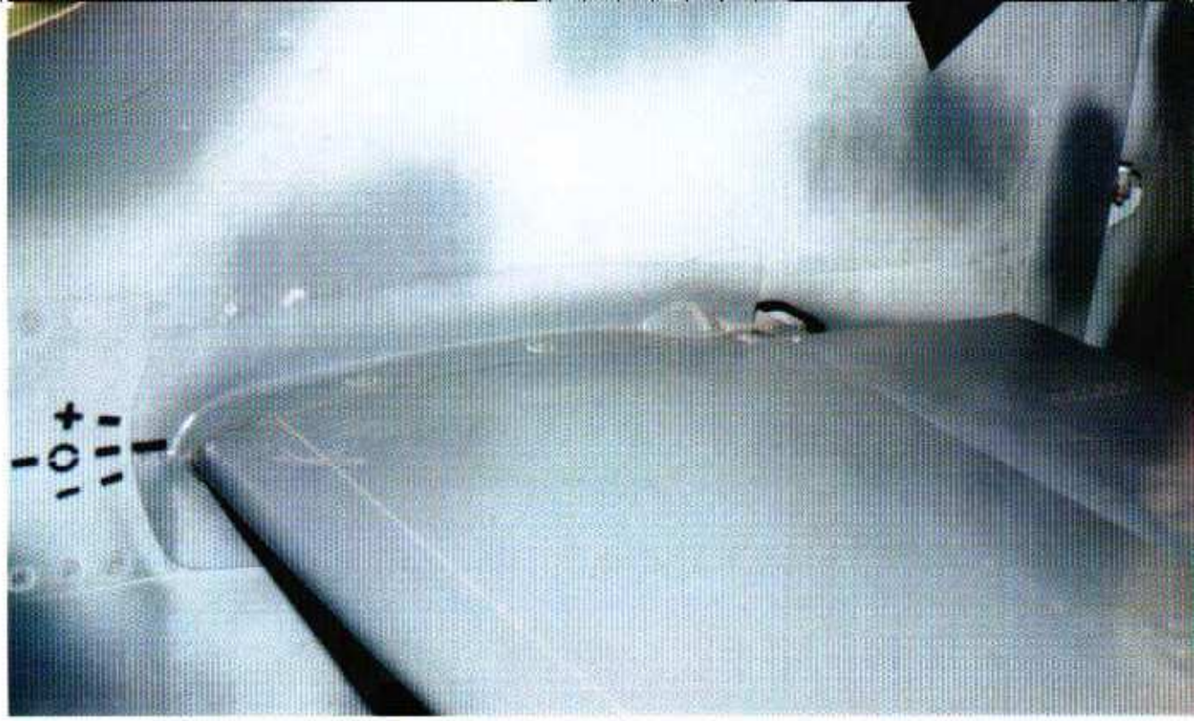
The + 0 - markings on the fuselage indicates the "horizontal stabilizer incidence" which could be adjusted by the pilot from +4 degrees to -1 degree, to compensate for changes in the aircraft's trim. A small electric motor in the tail actuated changes. The normal position is 0 (which is actually +2 degrees relative to the fuselage thrust line). (Author: Ryle)
