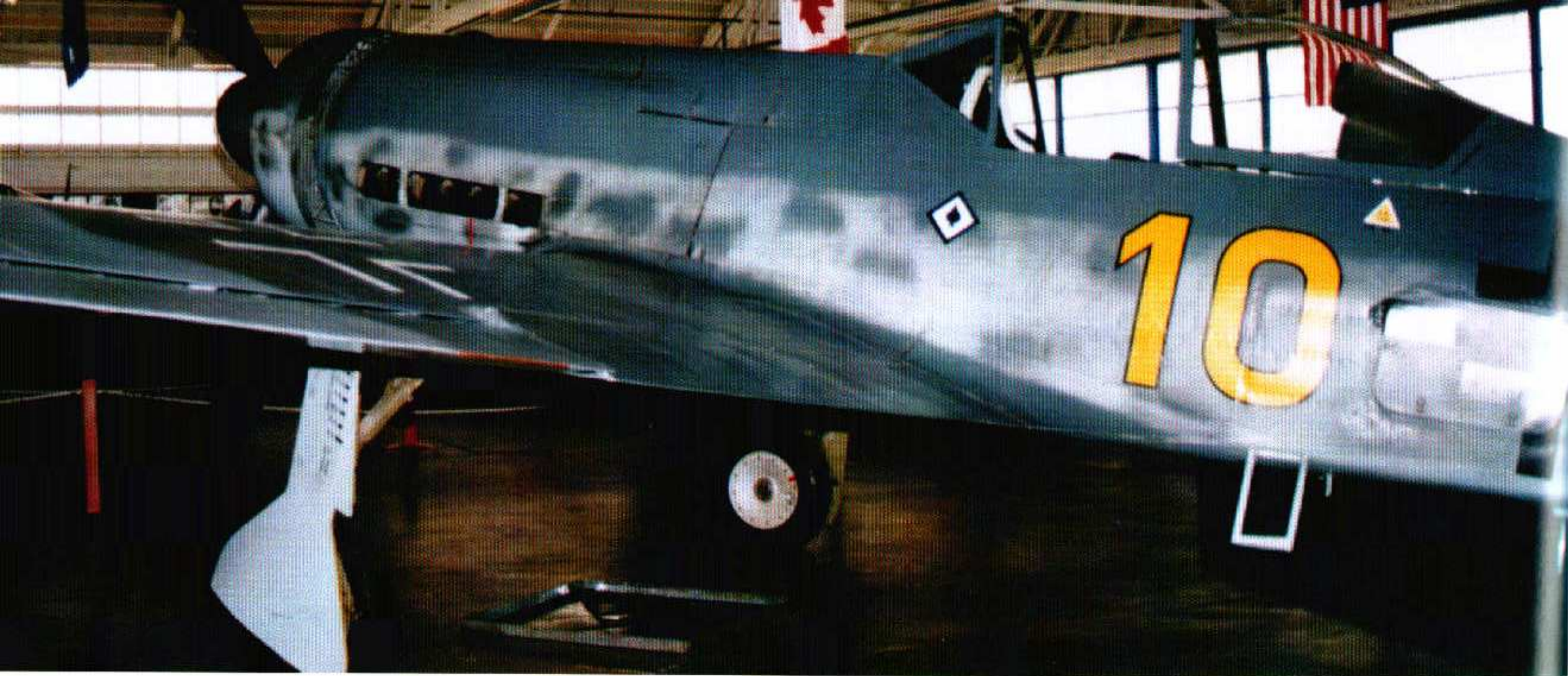
(Above) The port side of the Champlin Fighter Aces Museum Fw 190D-13. It is believed that this was the 17th Fw 190D-13 manufactured. Built by Roland in March of 1945, the fuselage for the Fw 190D-13 was rebuilt from an Fw 190A-8 airframe (174001) which had been produced at the Focke-Wulf plant at Cottbus in May of 1944. This rebuilding of usable airframes was a common practice with Fw 190 production. (Author: Ryle)
