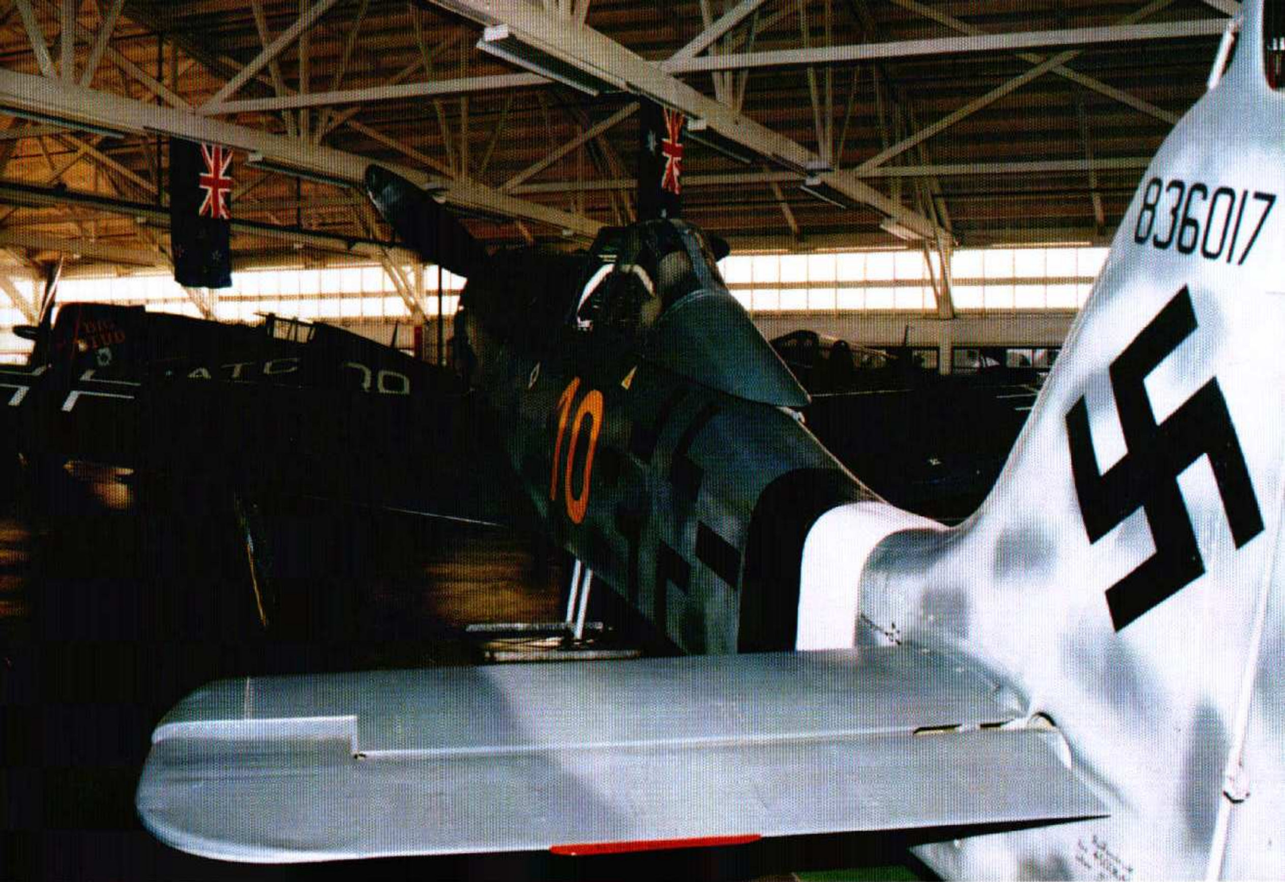
The trailing edge of the horizontal stabilizer along with its connection to the elevator. The aircraft's Work Number (836017) is at the top of the vertical fin. The placement of the Work Number in this location was a standard practice throughout the war. (Author: Ryle)
