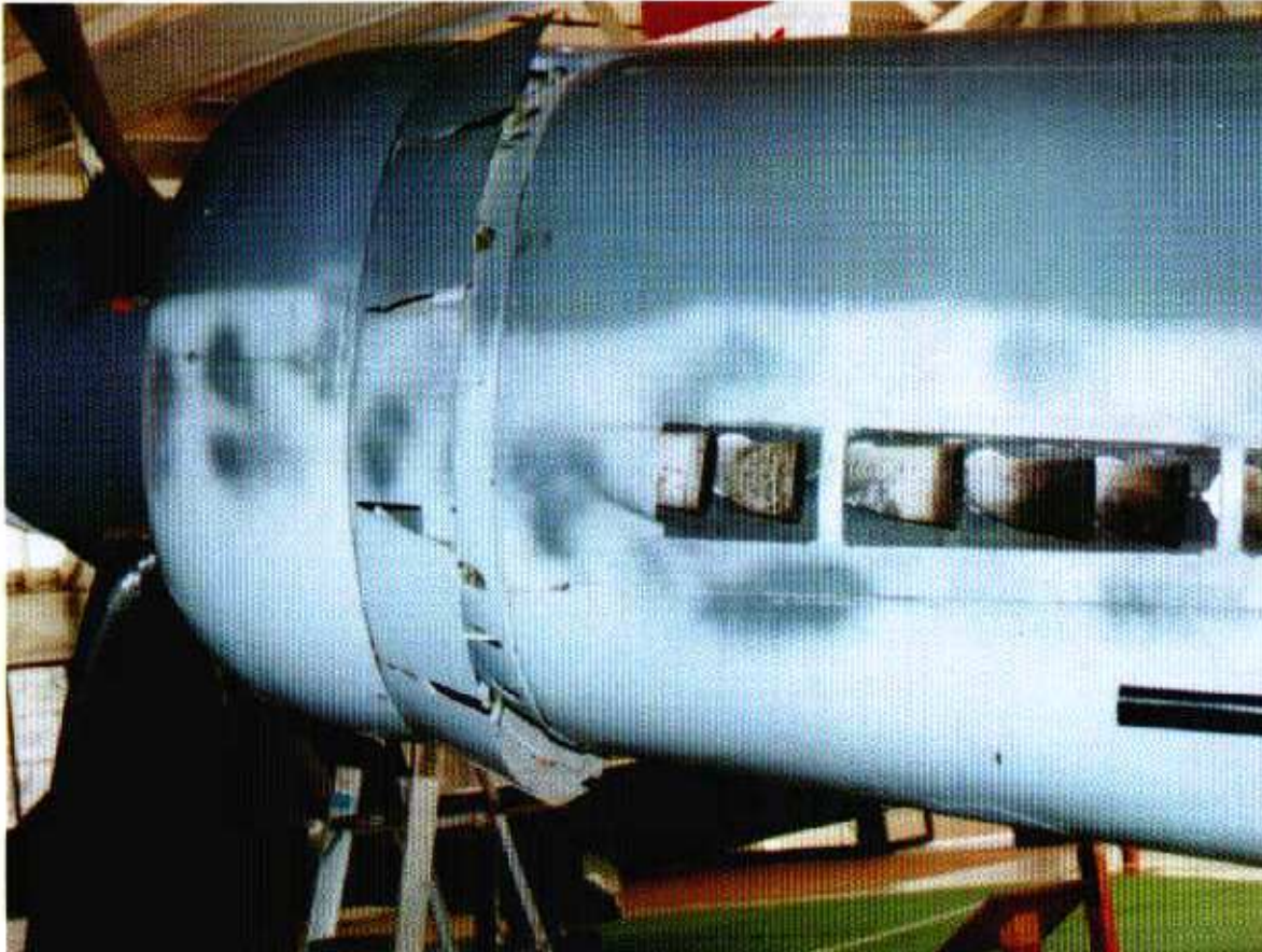
Just behind and under the cowl flaps, the fuselage can be seen to taper providing for air flow through the nose mounted radial radiator. (Author: Ryle)
