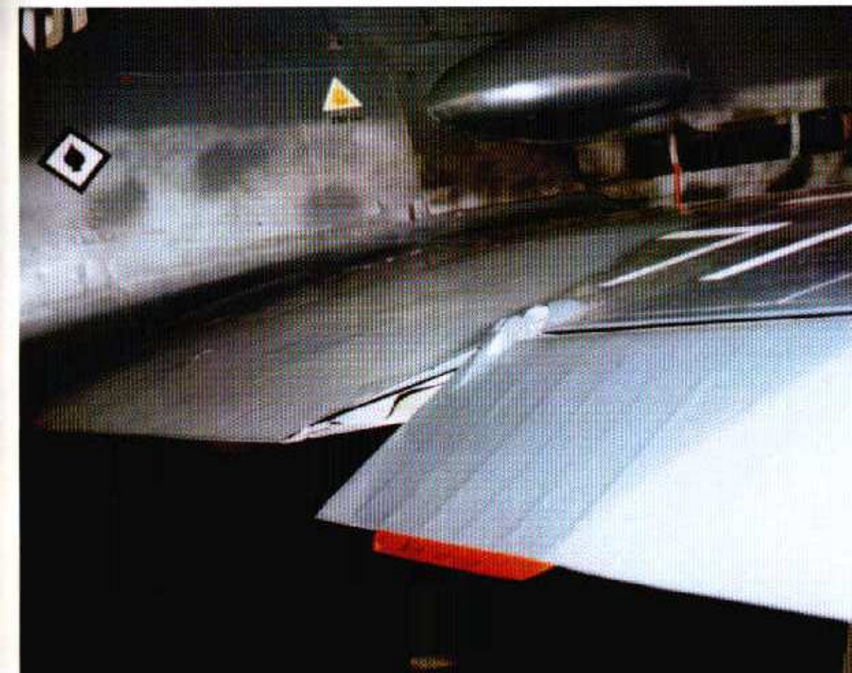
The starboard wing aileron in full up and in full down position. The aileron is cloth over a metal frame the same as the rudder and the elevators. Painted red, the metal trim tab is positioned quite close to the inboard edge of the aileron. (Author: Ryle)
