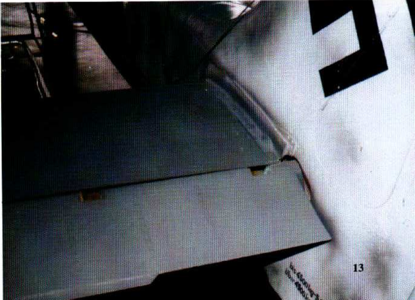
(Above)The lower starboard side of the fuselage looking aft. There are no external skin stiffeners on the tail prior to the tail wheel as are found on the later Fw 190D-13. (J. Bishop)
