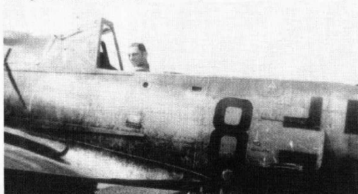
(Above and below) Black 8 (W.Nr. 500581) an Fw 190D-9 of II/JG 6 at Halle, Germany. The aft latch on cowling gun panel is open throwing a shadow onto the fuselage. Several of the cloth covers over the bolts on the port landing gear cover have not been installed, although some repair work or re-paint has been performed on the cover. (J. V. Crow)
