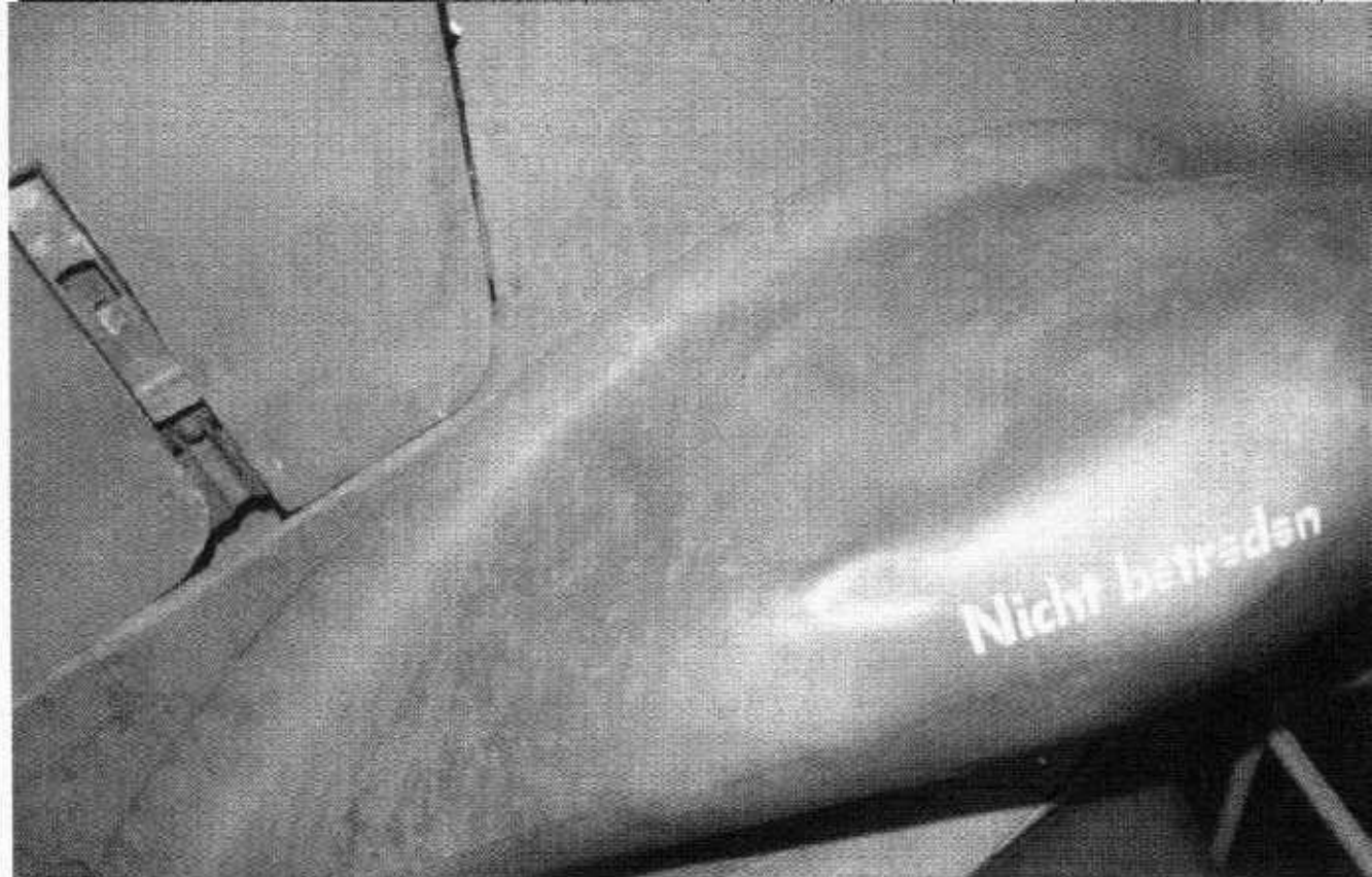
The weld line divides the supercharger intake into upper and lower halves. The words Nicht betreten translates as "No Step". (Author: Ryle)
