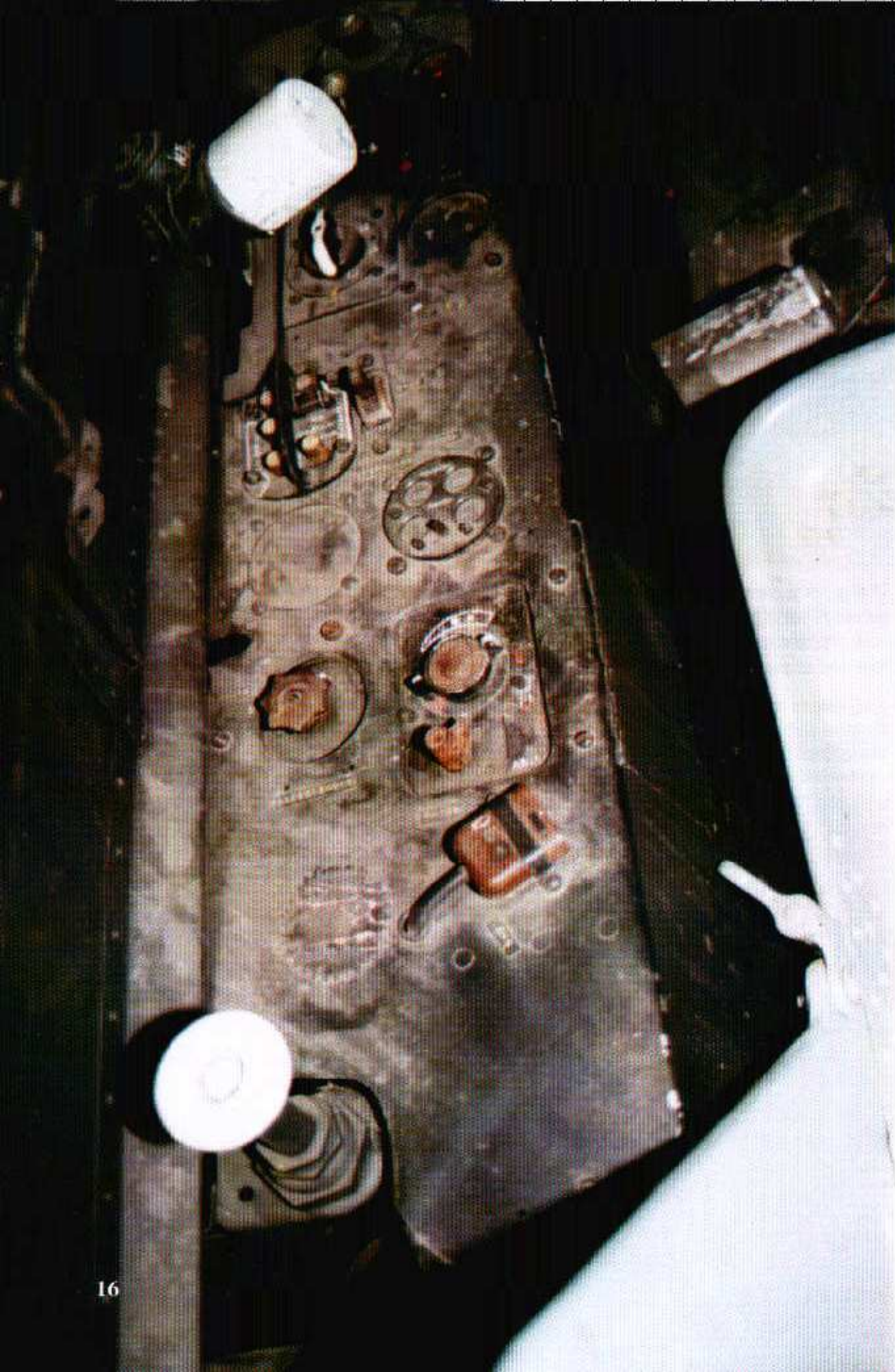
(Above) Forward of the throttle lever is the trim indicator, starter button, and the instrument light dimmer. On the lower instrument panel is the IFF panel, above that is the landing gear manual extension and the red knobbed handle is the manual fuel tank selector lever. (Author: Ryle)
