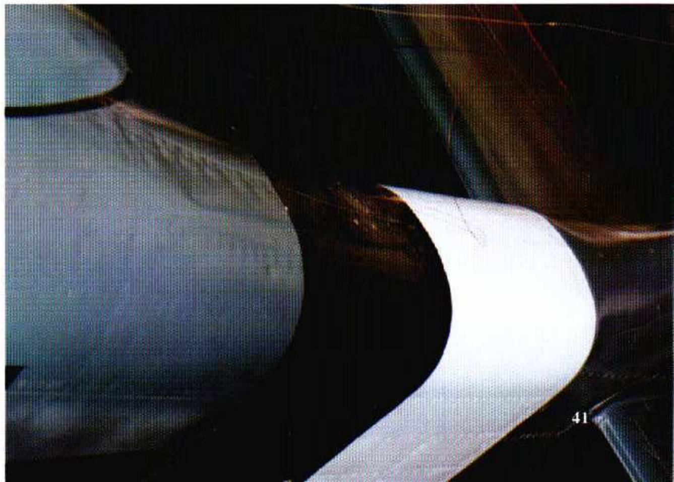
The fuselage extension plug is painted with a Black and White Defense of the Reich band. The entry point of the vertical antennawire can be seen in the Black band. (Author: Ryle)
