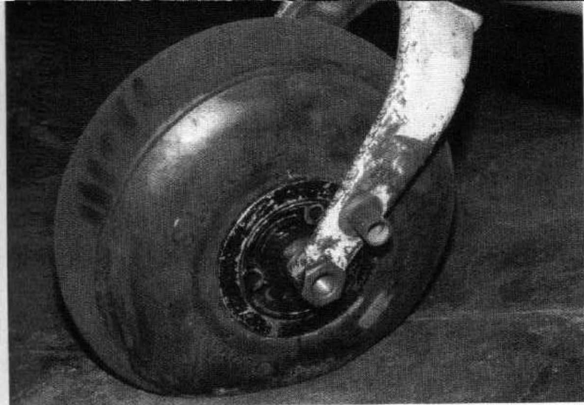
The tail wheel fork is a late war welded type with prominent rough weld lines. As the war got more desperate such things as deburring weld joints were ignored especially when they did not affect the functioning of the equipment. With no original available an American tail wheel and tire have been substituted. An unusual feature is the addition of a fairing around the tail wheel opening. (Author: Ryle)
