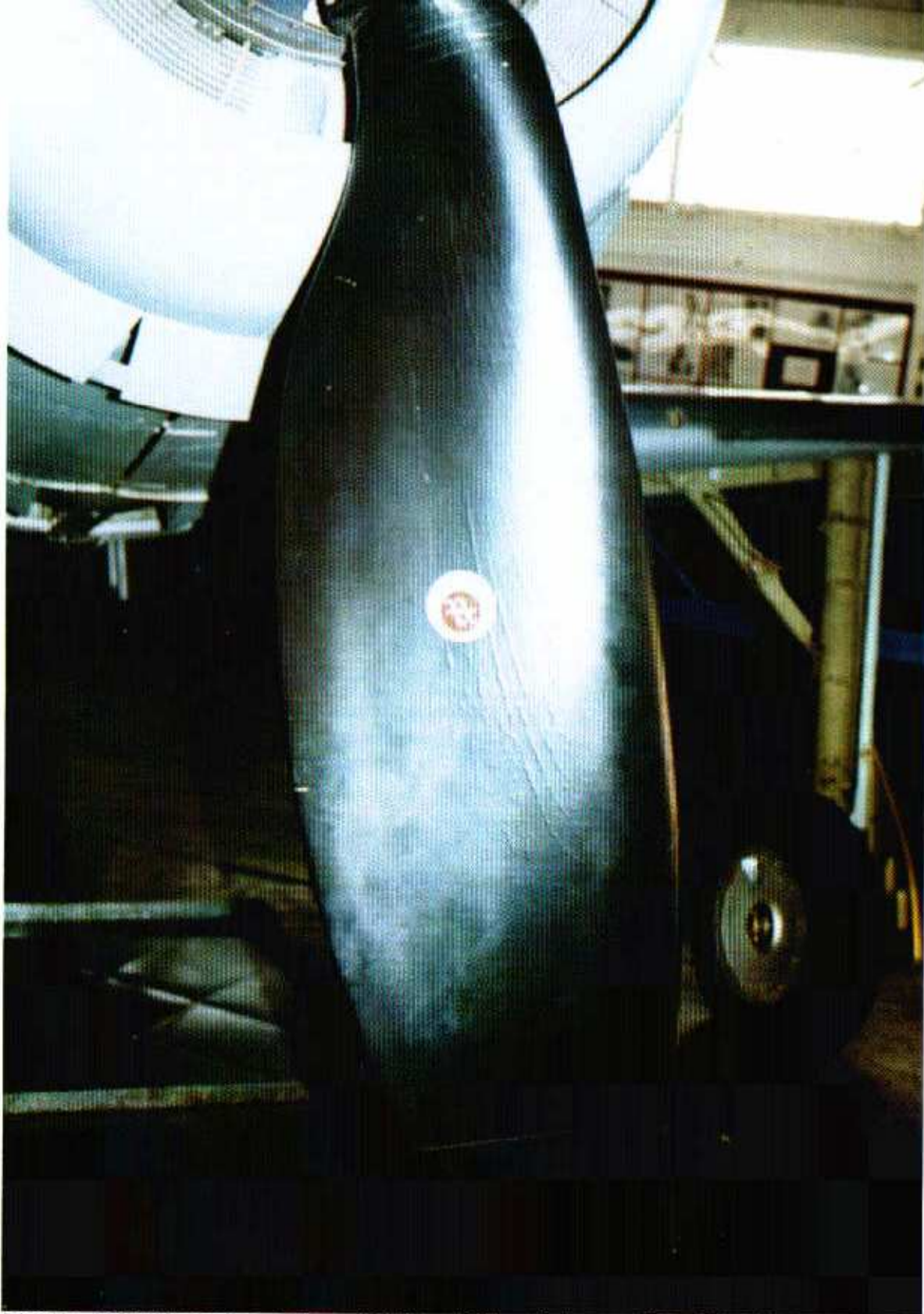
The Fw 190D-13 used a Junkers VS 10 variable pitch propeller. The blade seen here maybe original (but possibly not a VS 10), and if so, could have been made from one piece of hard wood with a metal leading edge and an exterior of painted cloth. The wrinkle lines on the blade are the result of the wooden blade shrinking inside its cloth cover. (Author: Ryle)
