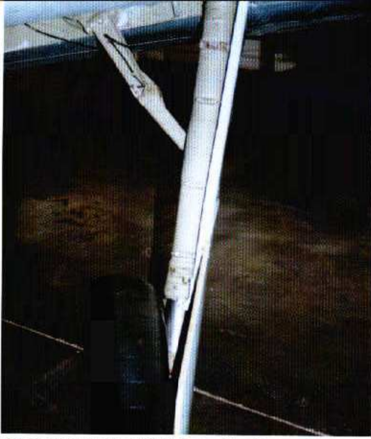
(Above and above right) The port landing gear from the front and from the rear. The landing gear of the Fw 190 did not extend straight down from the wing, but with a very pronounced inward angle. The landing gear extend/retract arms (upper and lower radius rods) are not over-centered but appear to have a slight bend. The landing gear like the wheel well is painted RLM 02. (Author: Ryle)
