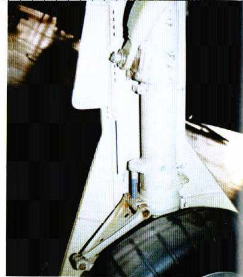
The extend/retract arm's attachment to the rear of the oleo shock strut on the port landing gear. The top of the scissors unit can be seen just above the wheel and immediately above that is the shock strut 'spur'. (Author: Ryle)
