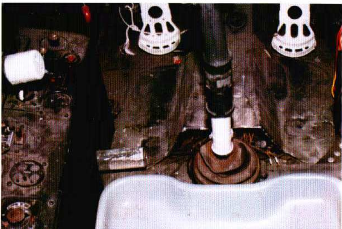
(Below) The throttle friction knob extends from the bottom of the left console. The control stick has a boot installed around its bottom just above the elevator control rod coming out of the boot to the right console. (Author: Ryle)
