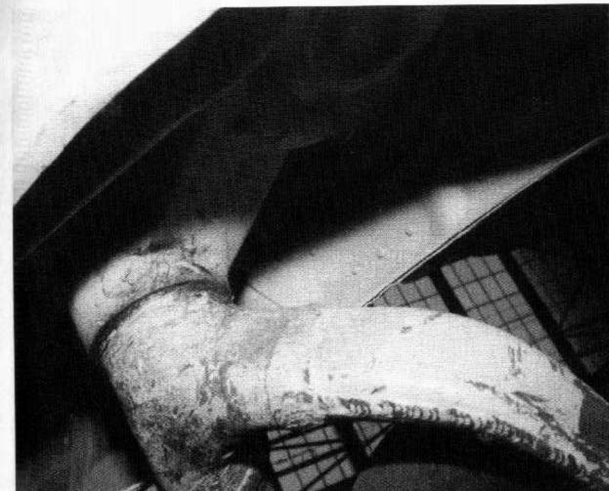
The tail wheel fork is a late war welded type with prominent rough weld lines. As the war got more desperate such things as deburring weld joints were ignored especially when they did not affect the functioning of the equipment. With no original available an American tail wheel and tire have been substituted. An unusual feature is the addition of a fairing around the tail wheel opening. (Author: Ryle)
