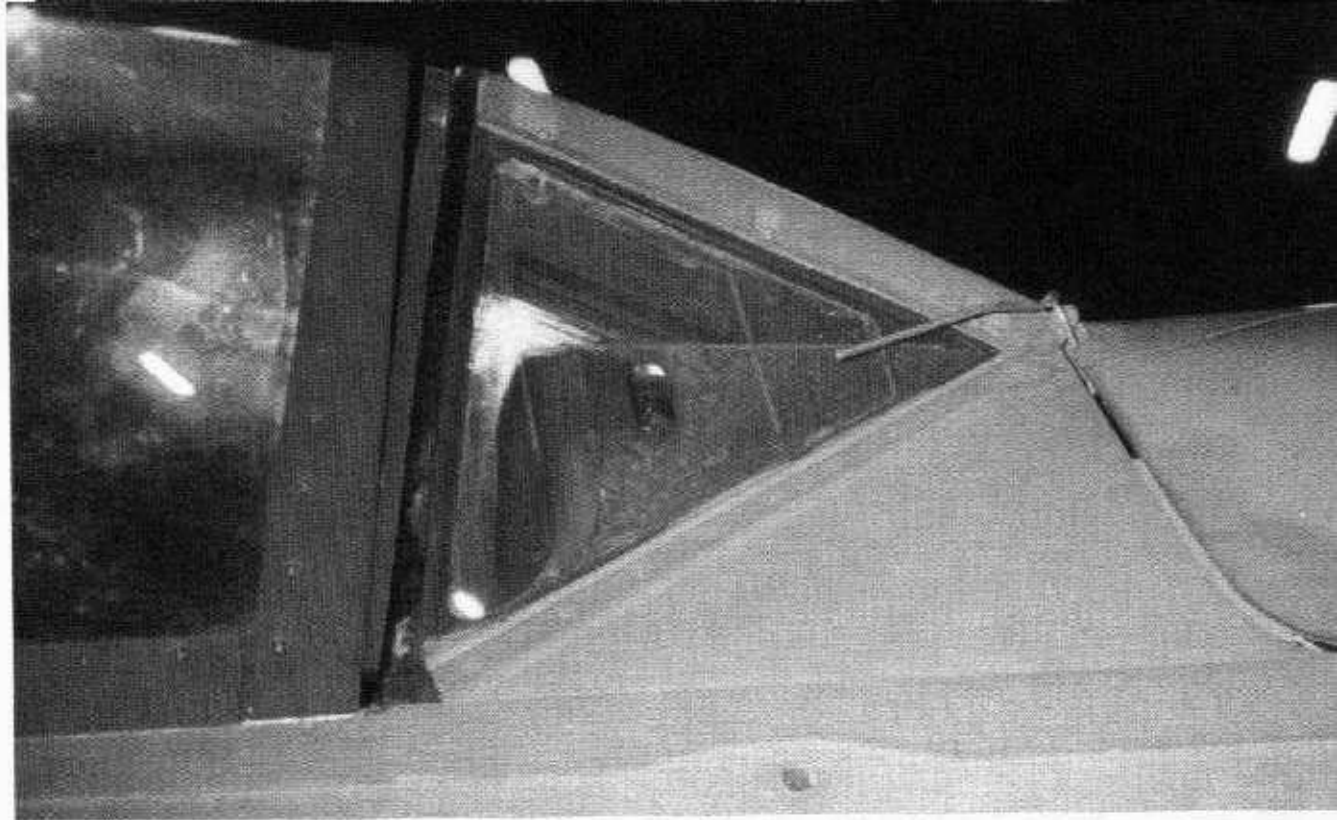
The replica canopy fits poorly to the armored windscreen. The small tube on the front of the windscreen is the windscreen (cleaning) spray tube which cleaned the windscreen with fuel from the fuel line running to the fuel pressure gauge in the cockpit. It has broken and slipped down, but its lower attachment can clearly be seen. (L & J Wahsum)
