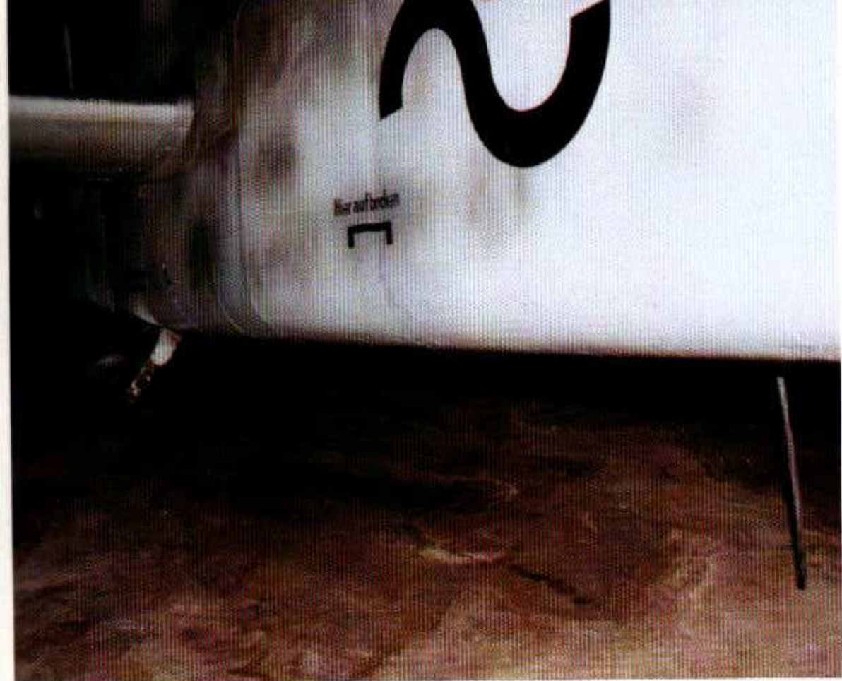
(Above)The lower starboard side of the fuselage looking aft. There are no external skin stiffeners on the tail prior to the tail wheel as are found on the later Fw 190D-13. (J. Bishop)
