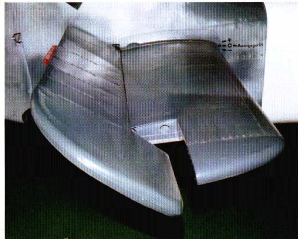
(Above and below) The replica horizontal stabilizer with the elevator in the full up and full down position. The horizontal stabilizer is all metal construction, while the elevator, like the rudder, is cloth over metal frame construction. The cloth is stitched to the elevator's frame, taped over, then the assembly is painted the same as the other parts of the aircraft. However, the difference in light reflection between the cloth covered parts and the metal parts almost made the fabric surfaces look like they were a different color. (Author: Ryle)
