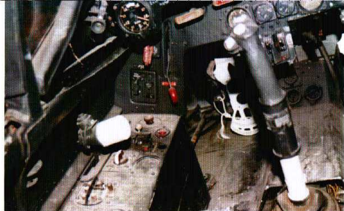
(Above) Forward of the throttle lever is the trim indicator, starter button, and the instrument light dimmer. On the lower instrument panel is the IFF panel, above that is the landing gear manual extension and the red knobbed handle is the manual fuel tank selector lever. (Author: Ryle)
