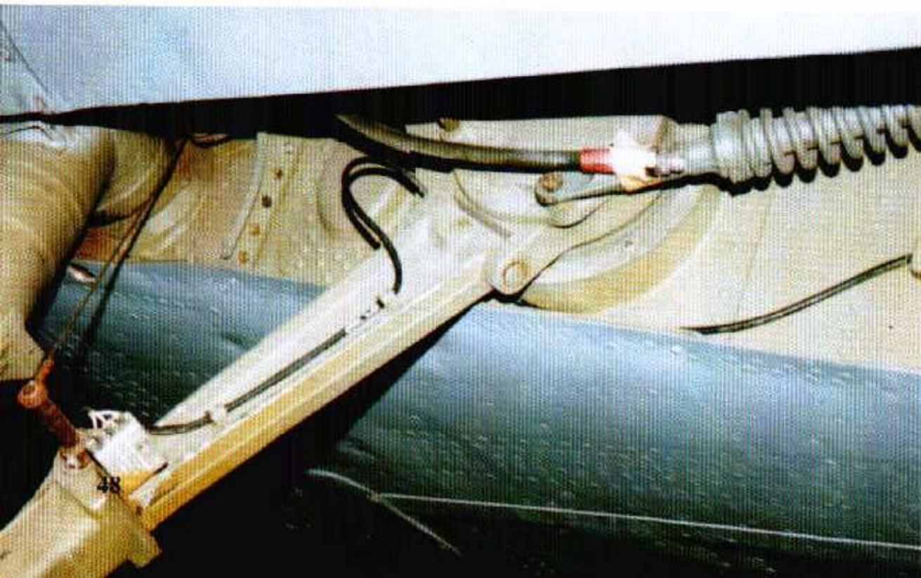
The starboard landing gear extend/retract arm. The wiring of the micro-switch may be seen as well as its plug-in on the rear wall of the wheel well. The tail wheel retract wire's attachment bolt is on the joint of the arm. (Author: Ryle)
