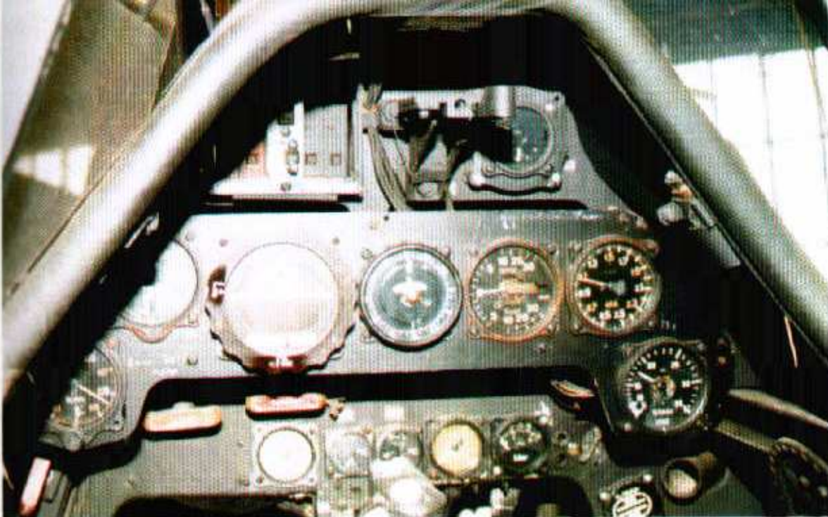
(Above) The upper and lower instrument panels are surrounded by a leather cushioned combing. On the upper left, just under the combing, are the ammunition counters (which are missing) and to the right of the counters is the Revi 16 gun sight (not installed) mount. To the right of the mount is the AFN 2 homing indicator used for instrument approaches. (Author: Ryle)
