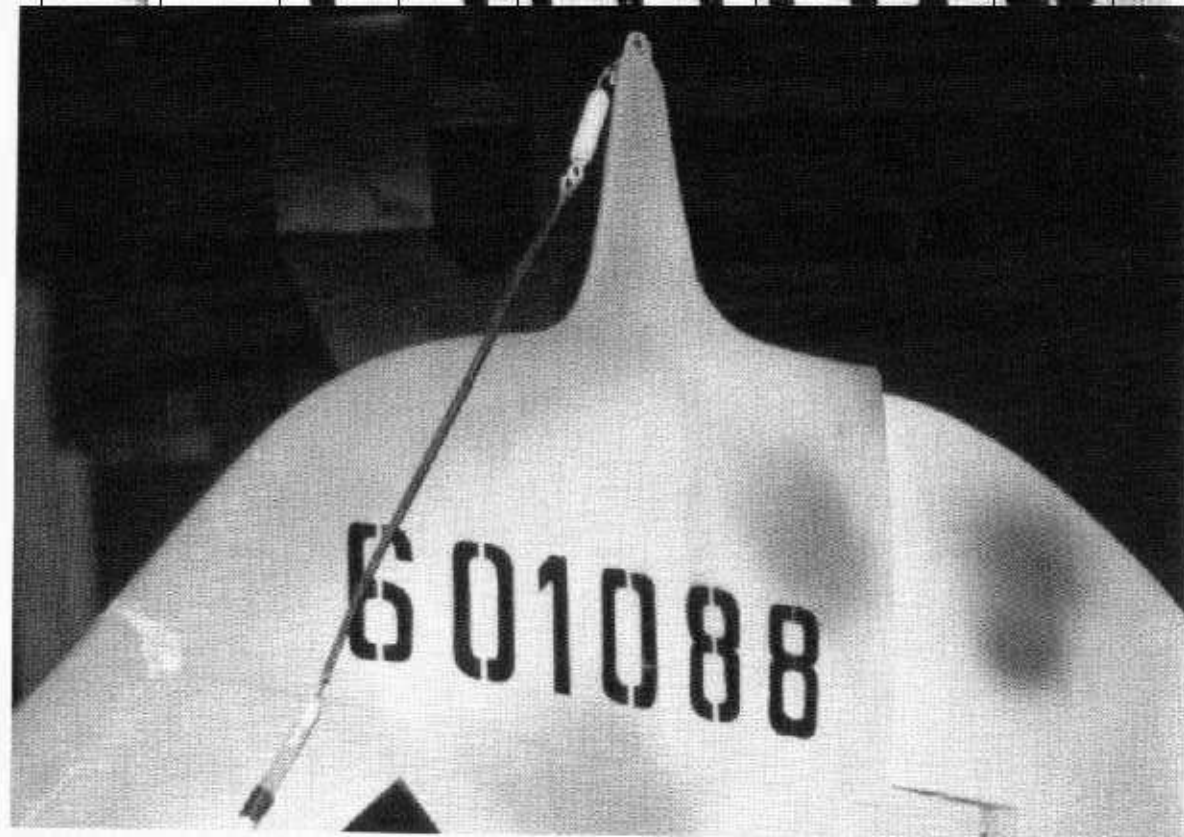
The canopy is open so the antenna wire drapes down slack. The aircraft's work number (601088) indicates it was built in a production batch of eighty aircraft that were some of the last Fw 190s to be produced before the end of the war. (Author: Ryle)
