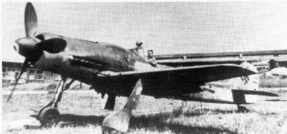
(Above and below) Black 8 (W.Nr. 500581) an Fw 190D-9 of II/JG 6 at Halle, Germany. The aft latch on cowling gun panel is open throwing a shadow onto the fuselage. Several of the cloth covers over the bolts on the port landing gear cover have not been installed, although some repair work or re-paint has been performed on the cover. (J. V. Crow)
