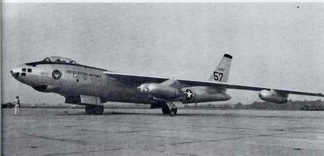
Original long bomb bay and rounded vertical fin is evident in this view of 49-1909. [Dave Menard]
