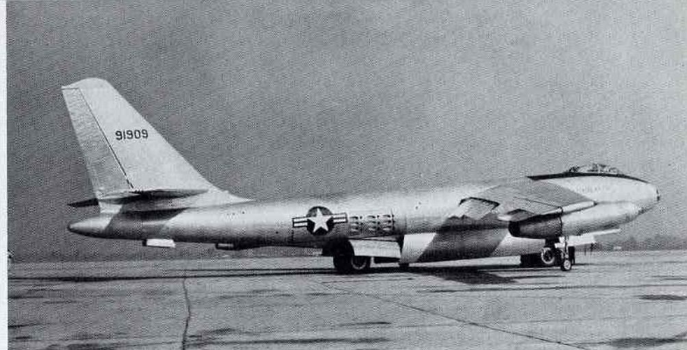
Original long bomb bay and rounded vertical fin is evident in this view of 49-1909. [Dave Menard]
