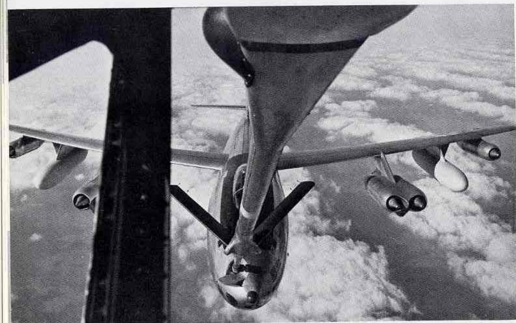
Early B-47E taking on fuel. Note that optical bombsight was not centered in the nose. [Boeing]
