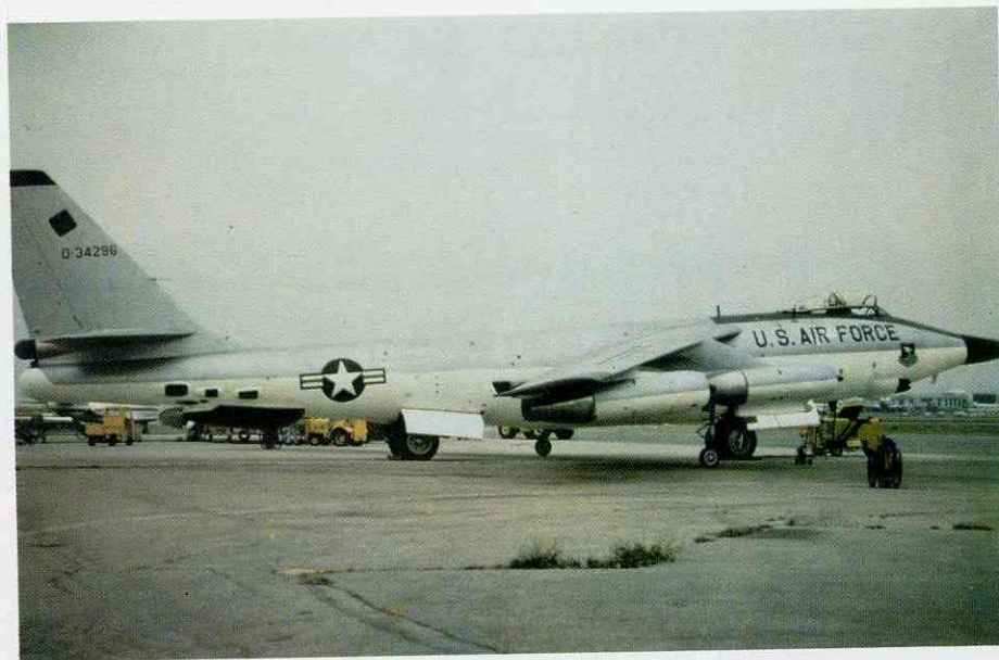
RB-47H was used as test bed for F-111A radar. It was fitted with the 111 nose. [N.E. Taylor]
