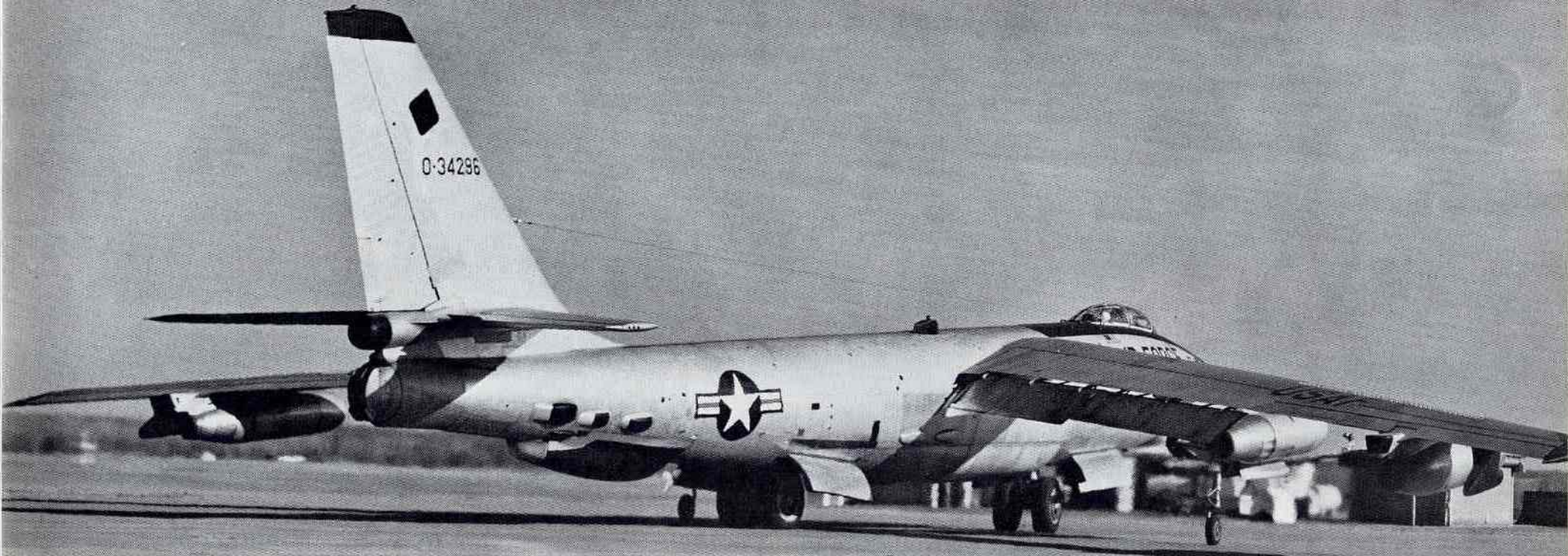
4296 taxis away from the ramp at Offutt. The aircraft carries a variety of antenna. Some that can be seen include extended wingtip, an underwing type outboard of engines number one and six, antenna located in the aft fairings of the number one and six engine mounts and a cluster of antennas on the aft fuselage. The guns have been removed from the aircraft. [USAF]
