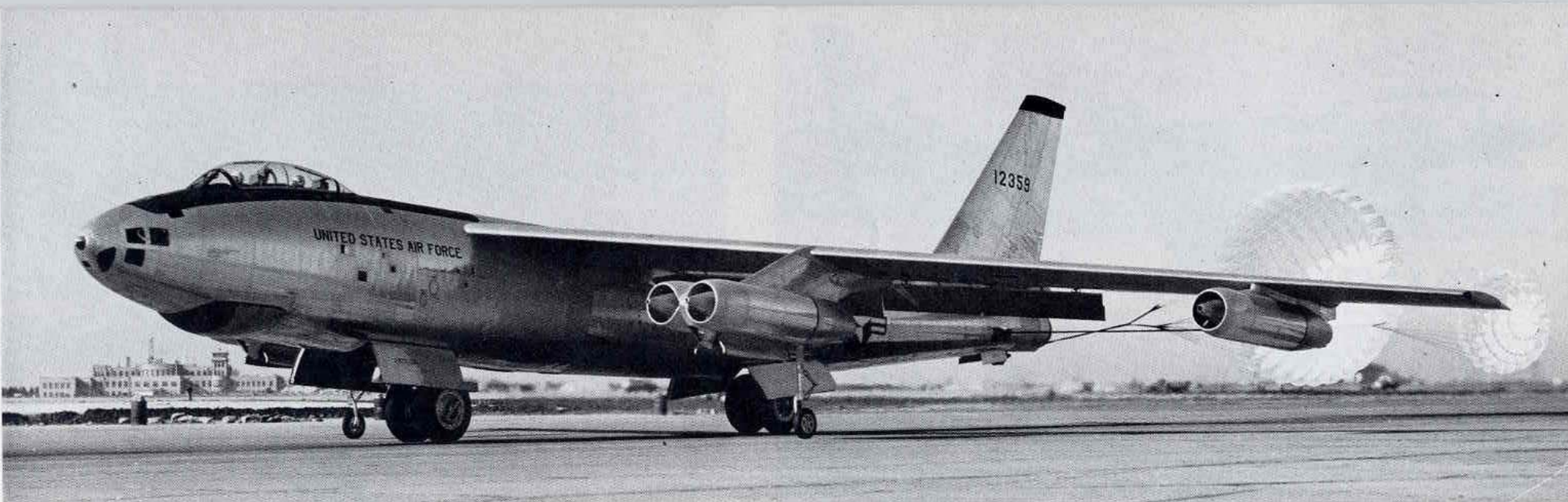
51-2359 taxis in with chutes billowing. The brake chute compartment is underneath the fuselage and the approach chute compartment is on the left side. The forward radar warning antenna has not yet been added above the periscopic bombsight. [Boeing]
