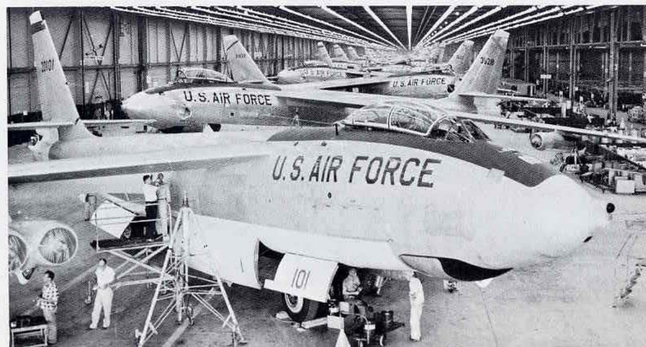
A group of B-47's going through the Milk Bottle structural modification at Tinker AFB.
