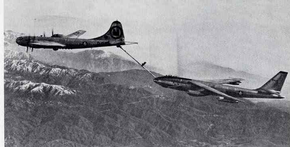
50-014, a B-47B-10-BW, refuels from a KB-29P during Phase IV Heavyweight Air Refueling Tests at Edwards in 1952. [USAF via Donald Bishop]
