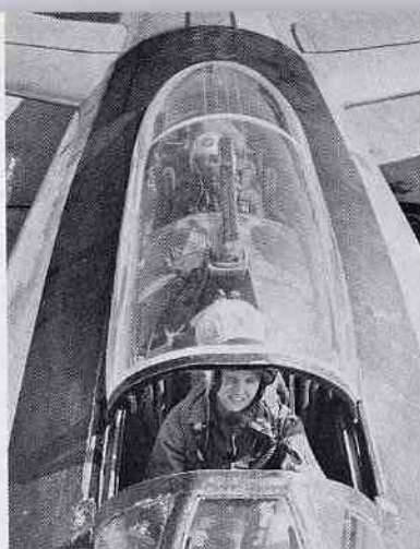
Looking aft down the spine of an early B-47. The canopy is the sliding type. The four cords in the canopy above the co-pilot comprise the radio compass sensing antenna. Radio compass loop antenna is just behind the pilot. [Boeing]
