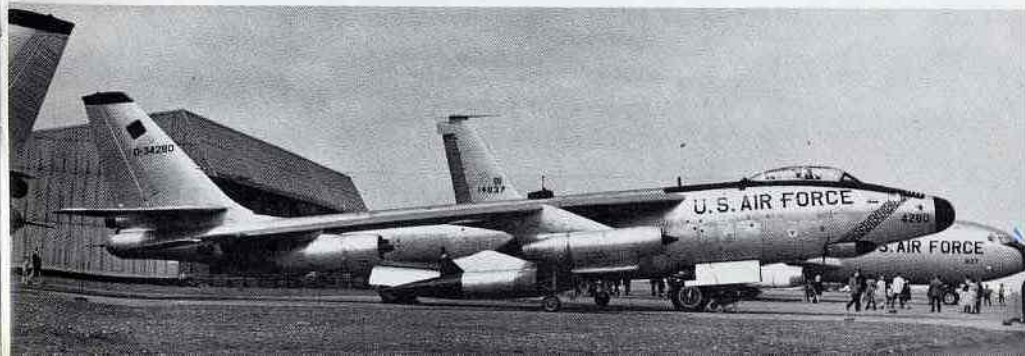
The 55th SRW's 53-4280 is shown on display at Upper Heyford on 13 May 1967. The large pod [which was carried only on the right side] carried additional reconnaissance gear and could be removed or attached as the situation required. The emblem on the nose was carried on both sides. [Bob Stynes via John Bowdler]
