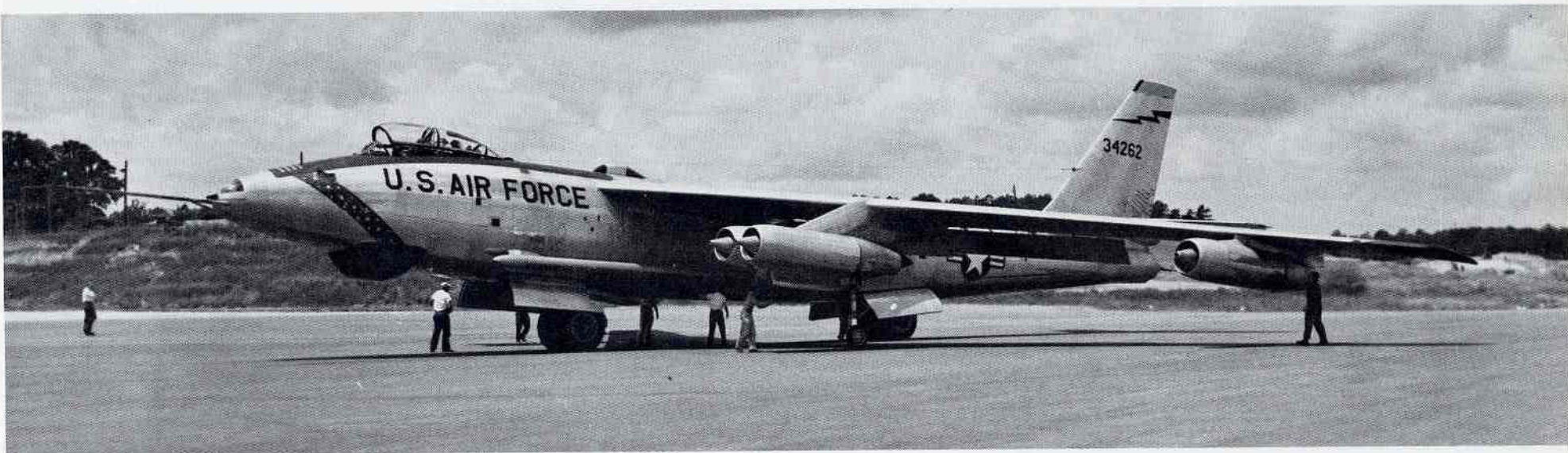
[Above] A "whatzit"...nominally an RB-47E, shows some interesting modifications. Notable is the deep bathtub-shaped radome, the nose probe, the antenna on the fuselage top, and the long cylinders on the fuselage side. What the aircraft was testing remains a mystery to the authors. [R.D. Neal]
