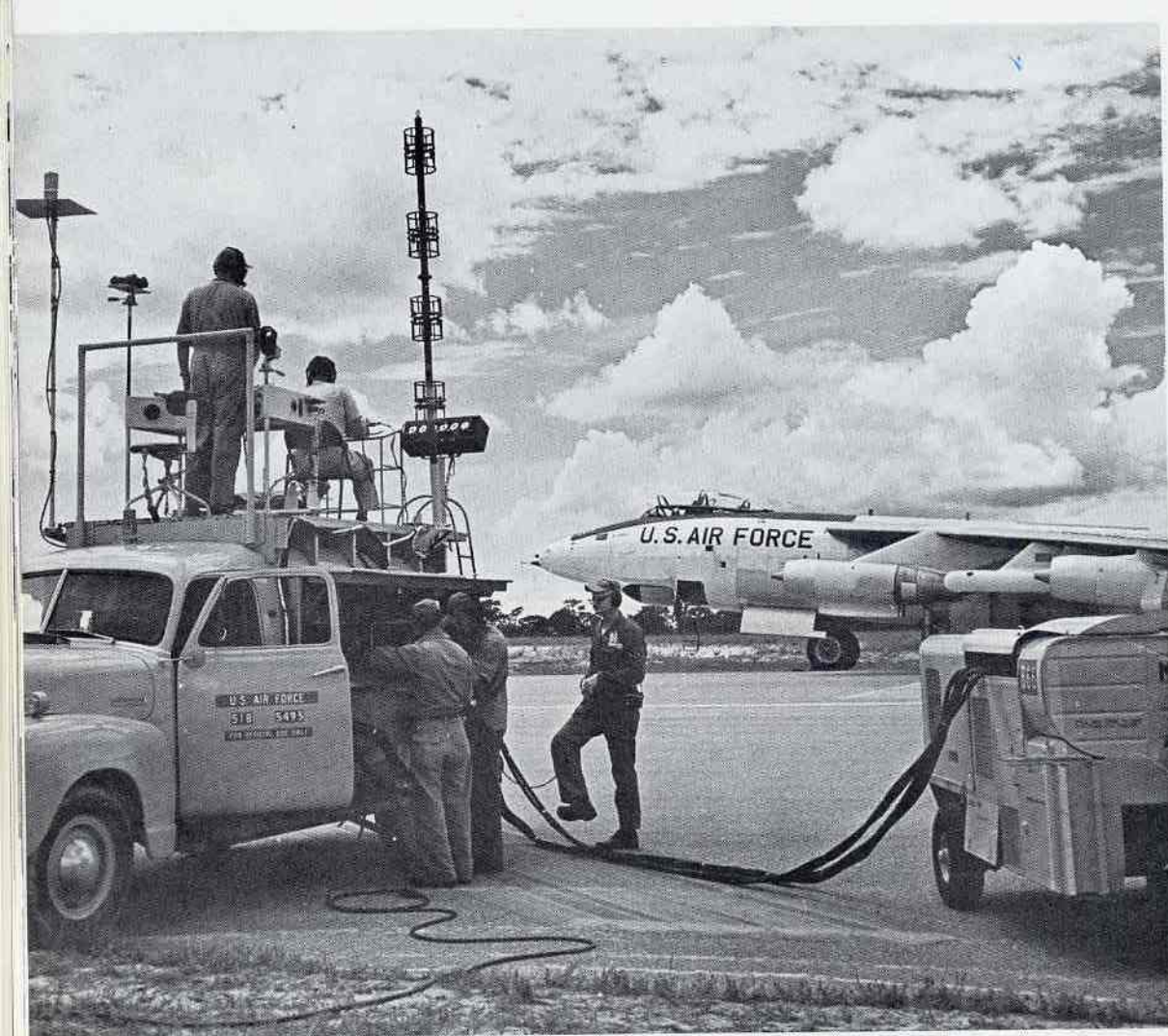
Taxi crew readies QB-47E for an unmanned [Nullo] flight. Ground controllers on top of MRW-5A vehicle handled the aircraft during takeoff and landing. [Boeing]
