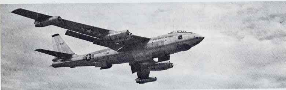
51-7080, a B-47E-75-BW of the 44th BW, takes off from Barksdale AFB on 23 February 1954. The aft gear doors are closing sooner than the forward doors. Obvious differences in the later E's from the B's and early E's are the solid nose and external ATO. [USAF]
