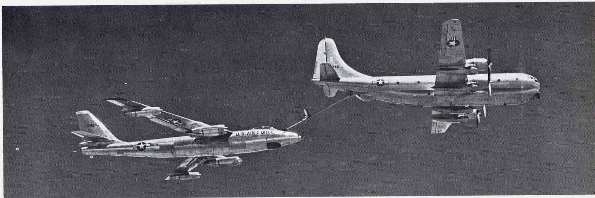
[Above] A "whatzit"...nominally an RB-47E, shows some interesting modifications. Notable is the deep bathtub-shaped radome, the nose probe, the antenna on the fuselage top, and the long cylinders on the fuselage side. What the aircraft was testing remains a mystery to the authors. [R.D. Neal]
