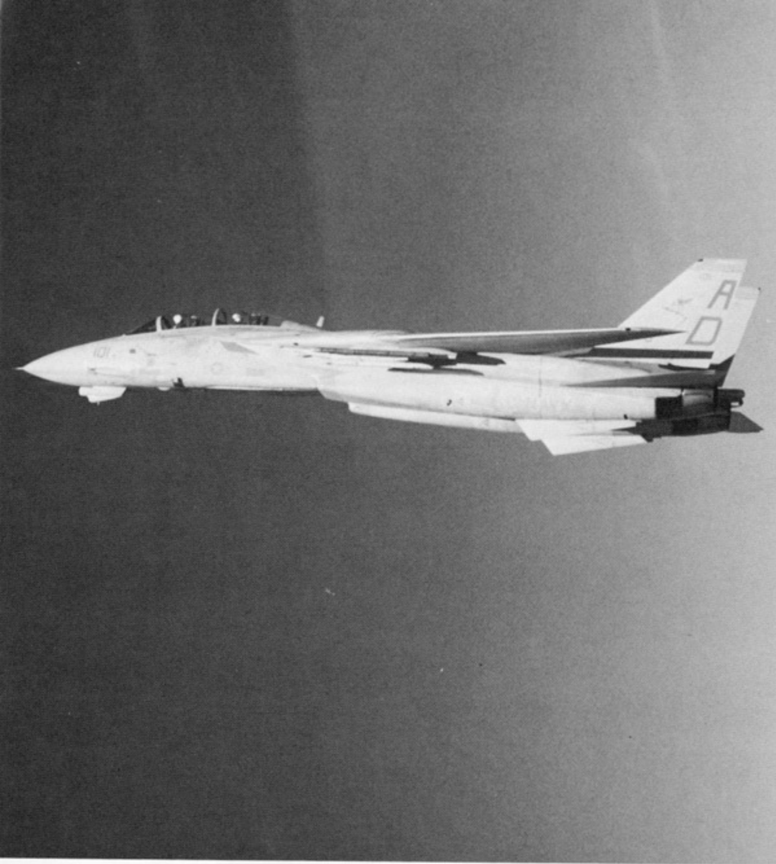
The F-14A (Plus) is the forerunner of the Super Tomcat F-14D. The F-14D will use the same engine/airframe of the F-14A (Plus) modified with upgraded electronics, radar, communications equipment and state-of-the-art cockpit displays. (Grumman)
