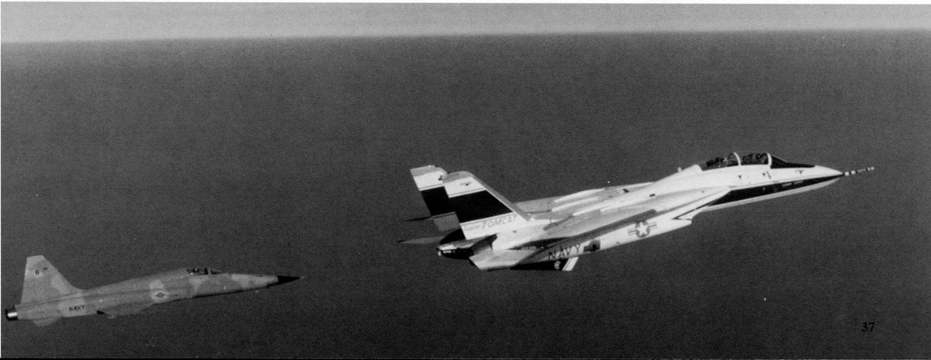
The F-14B prototype, in formation with a Northrop F-5 of VF-43, flies over the Atlantic during 1981. The General Electric F101 DFE engines provided the F-14B with considerably more thrust than the standard Pratt and Whitney TF-30-P412 engines. The GE F101 engine was originally designed for the Rockwell B-1 and was also tested in the General Dynamics F-16. (Grumman)
