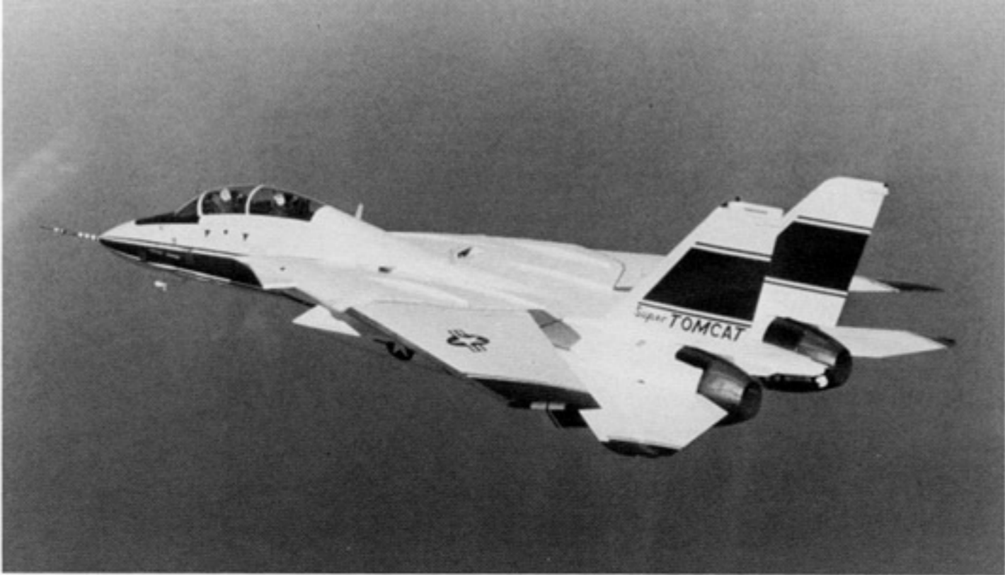
The F-14B (BuNo 157986) prototype with the General Electric Derivative Fighter Engines (DFE) made its first flight on 14 July 1981. The DFE engines were modular in design to ease production and maintenance. Because of these tests, GE engines were selected to power the F-14A (Plus) and the F-14D. (Grumman)
