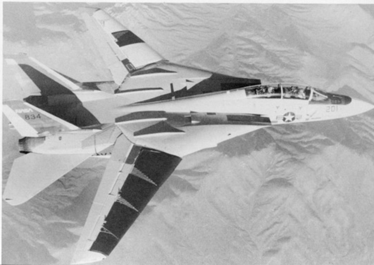
The wing gloves fitted to this F-14A (BuNo 159834) were made of fiberglass. The starboard wing glove smooths out the airflow and has sensors implanted in it. The port wing was unchanged to be used as a data base constant on the characteristics of a standard F-14 wing. (NASA)
