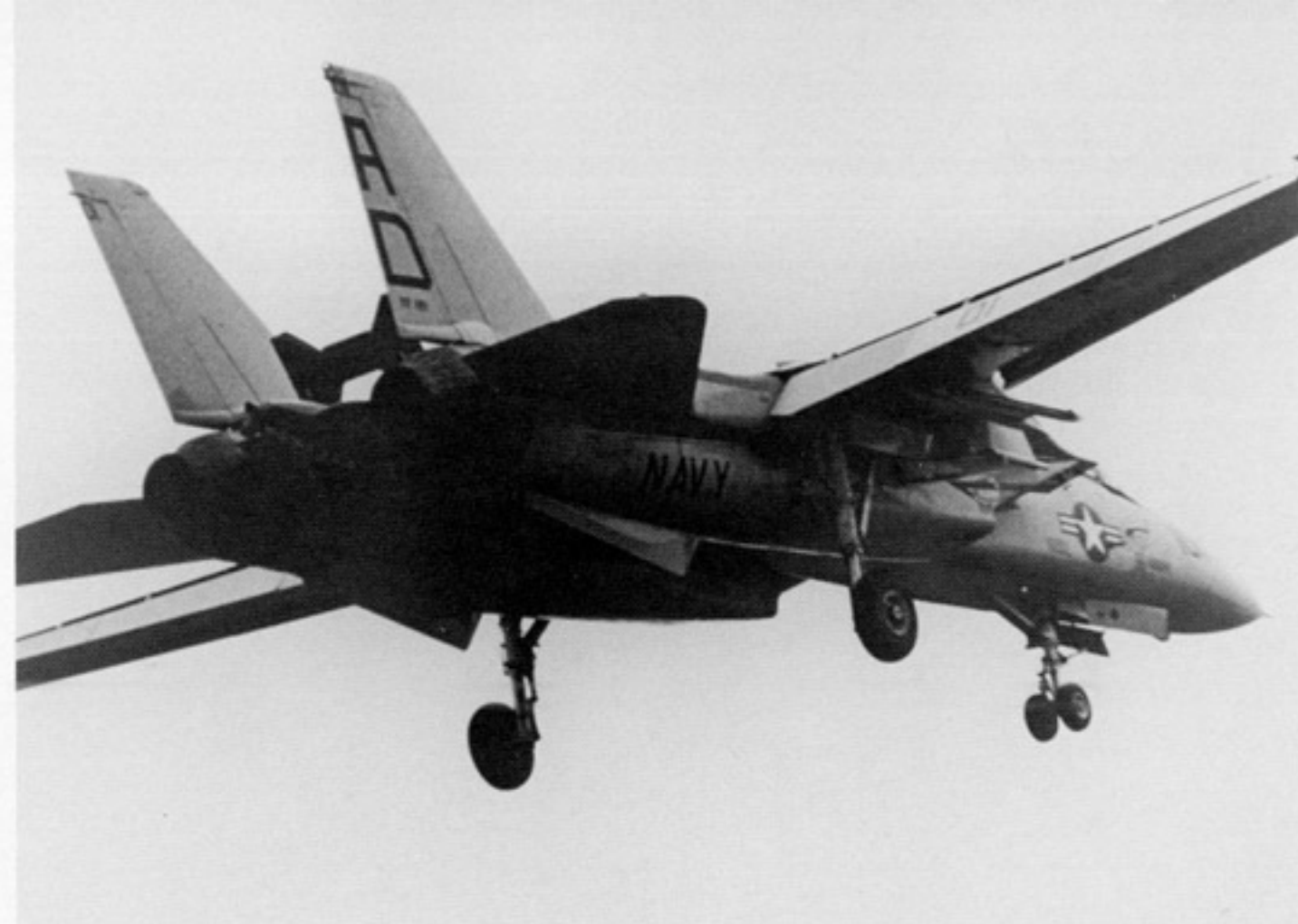
The speed brakes are fully deployed and the landing gear is extended; however, the tailhook is retracted as this F-14A of VF-101 Grim Reapers executes a go-around during a training mission. VF-101 is the Atlantic Fleet Replacement Air Group (RAG). (USN)
