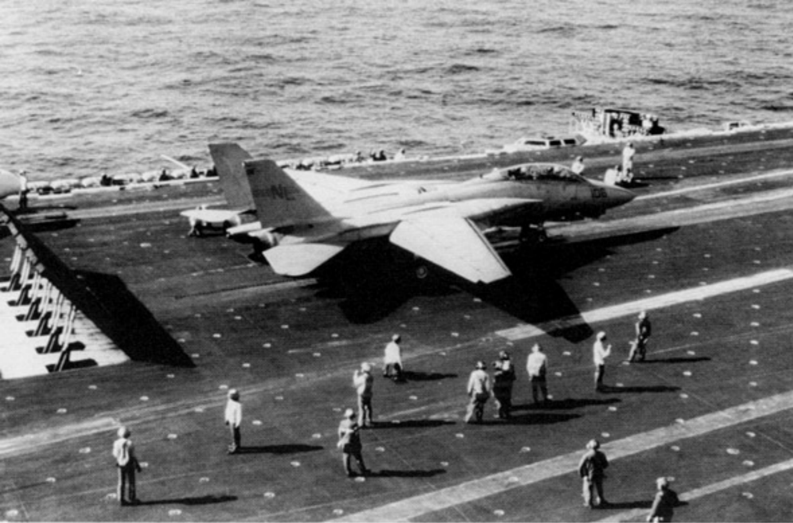
An F-14A of VF-51 positioned on the waist catapult of USS CARL VINSON in preparation for launch. Including catapult officers, it requires over thirty officers and deck crewmen to successfully launch an aircraft from the deck of an aircraft carrier. From plane handlers to ordnancemen, every job is important for safe operations. (USN by E. E. Cordero)
