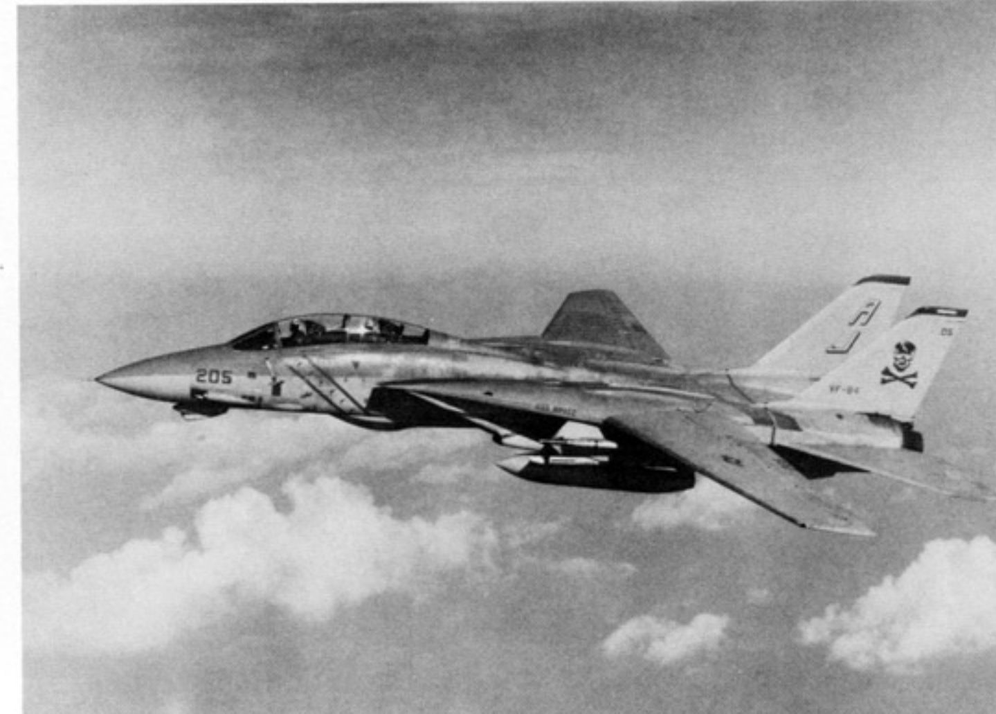
This F-14A of VF-84 Jolly Rogers is finished in three tone tactical camouflage consisting of Light Gull Gray vertical stabilizers, Medium Flat Gray fuselage uppersurfaces over Gull Gray undersurfaces. The Tomcat was stationed aboard USS NIMITZ (CVN-68) during 1986. (USN by R. Beno)
