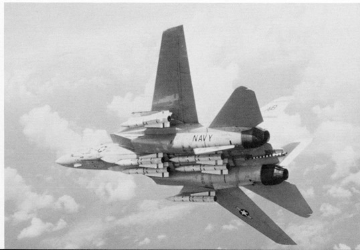
An AN/ALE-39 Chaff-Flare dispenser is fitted on the port side of the tail hook on this F-14A (BuNo 160919) of VF-32 Swordsmen. The dispensers have a capacity of thirty chaff, flare or jammer cartridges. Chaff cartridges are filled with thin strips of wire that are equal in length to the wavelength of the hostile radar emitters. (Grumman via Hughes)
