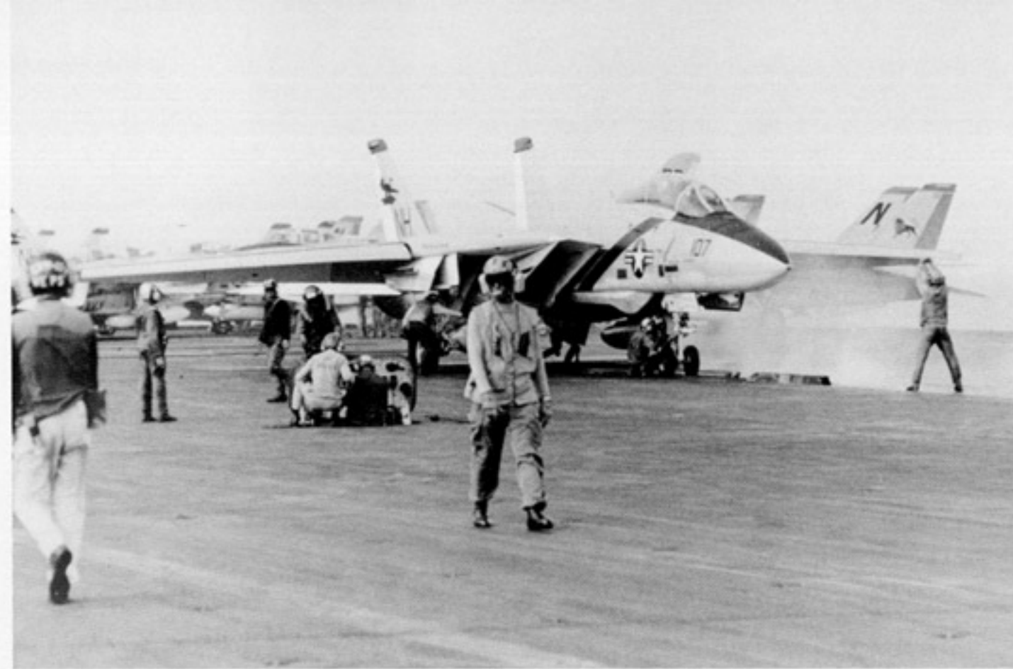
A Yellow shirted plane director signals an F-14A of VF-114 Aardvarks to hold as the catapult launch bar is positioned in the shuttle. VF-114 shared the deck with their sister squadron VF-213 Black Lions aboard USS KITTY HAWK (CV-63) operating in the Philippine Sea. (USN)
