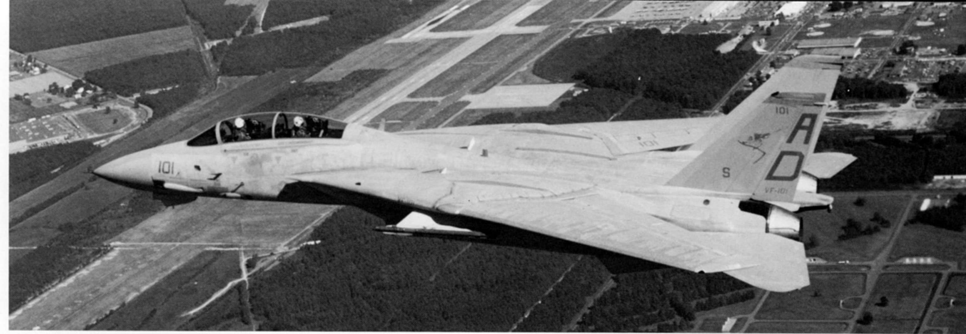
A VF-101 Grim Reapers F-14A (Plus) over the Virginia countryside near NAS Oceana during 1989. With the new General Electric engines, F-14A (Plus) can accelerate from 250 knots to 600 knots in just twenty seconds. (Grumman)
