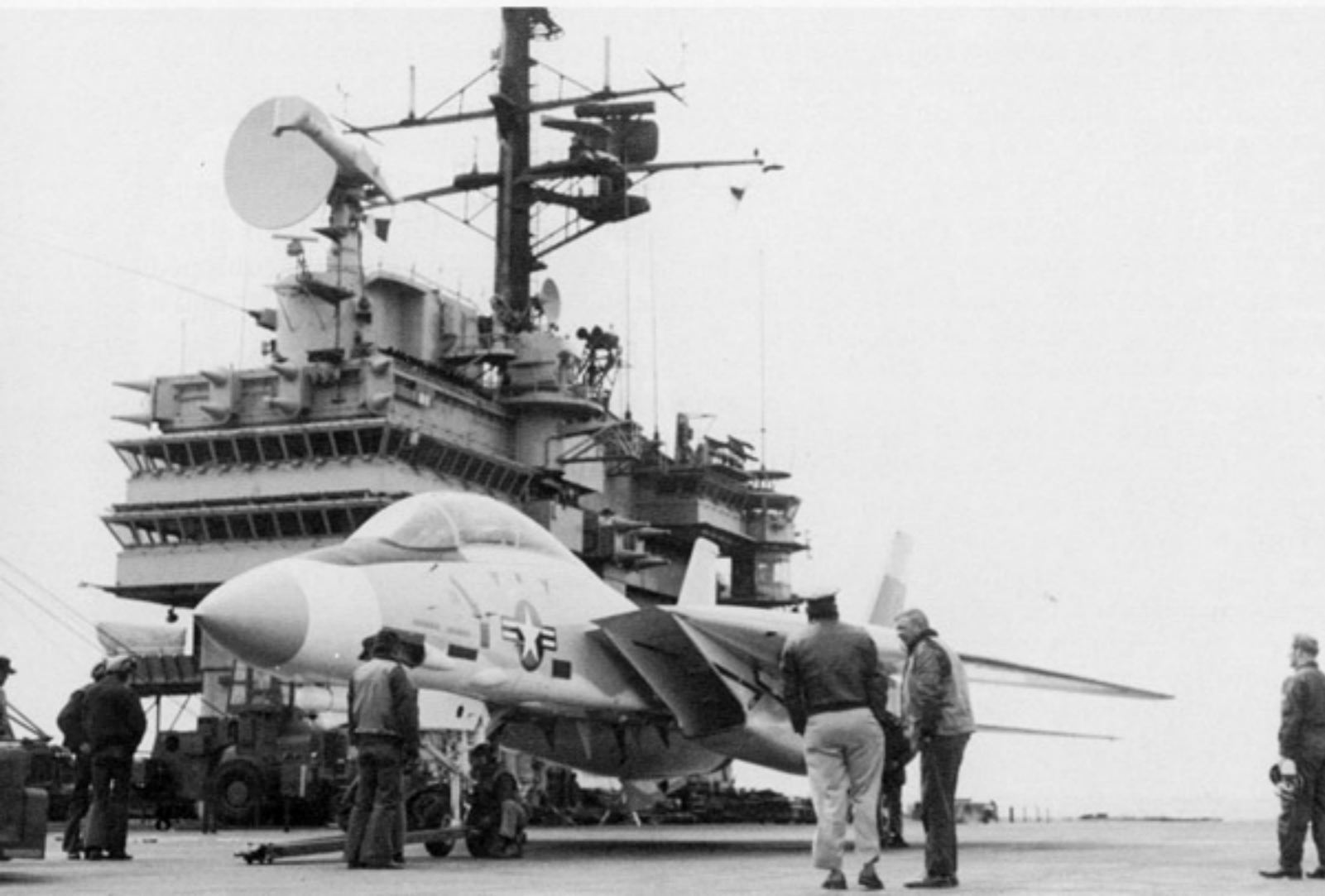
A deck crewman removes the nose wheel tow bar from aircraft number 11 during carrier suitability trials aboard USS INDEPENDENCE (CV-62) during March of 1972. The aircraft is carrying dummy Sparrow missiles in the underfuselage missile bays. (Grumman)
