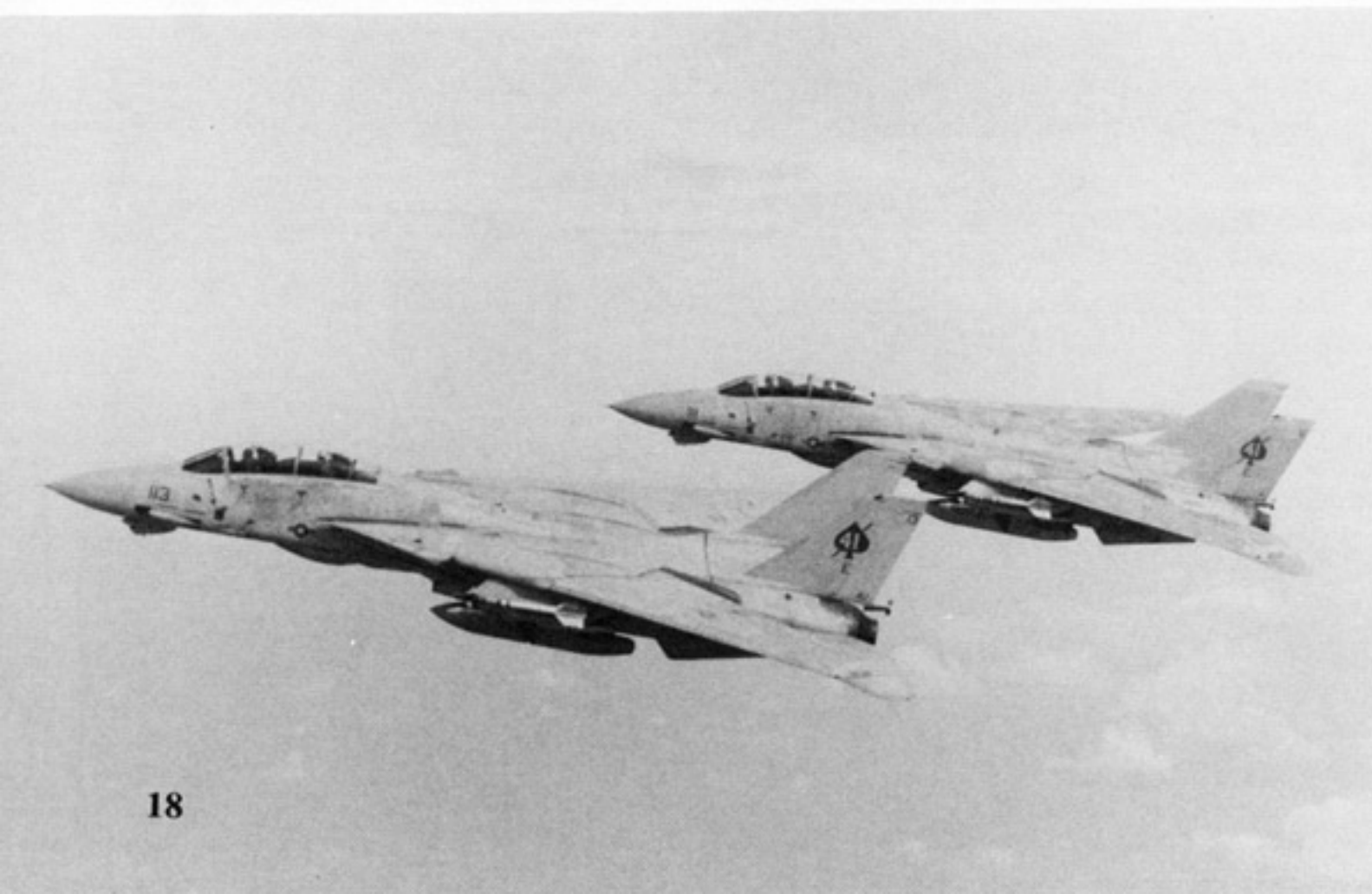
A pair of F-14A Tomcats of VF-41 Black Aces on combat air patrol over the Mediterranean Sea during 1986. AJ-111 and 113 are both armed with AIM-9 Sidewinder and AIM-7 Sparrow air-to-air missiles and are equipped with 270 gallon fuel tanks. The wing gloves are extended indicating that the aircraft are approaching Mach 1. (USN by R. Beno)
