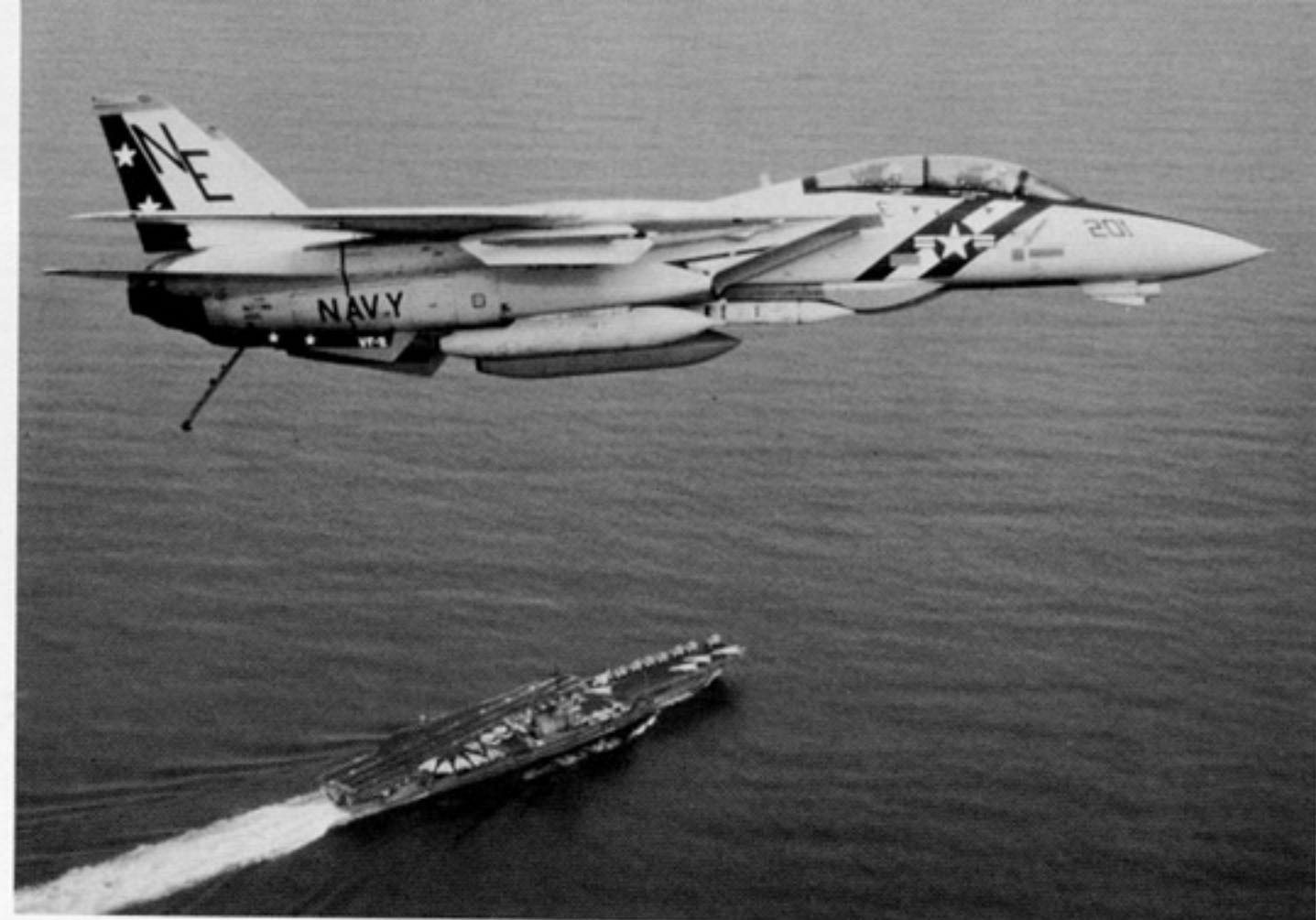
An F-14A of VF-2 Bounty Hunters over the USS RANGER (CV-61) during 1988. The aircraft is overall Light Gull Gray with Red, White and Blue fuselage stripes. The rudders and ventral fins are Blue with Yellow stars. The underfuselage fuel tanks have a capacity of 270 gallons and the aircraft is fitted with a TCS chin pod. (Hughes Aircraft)
