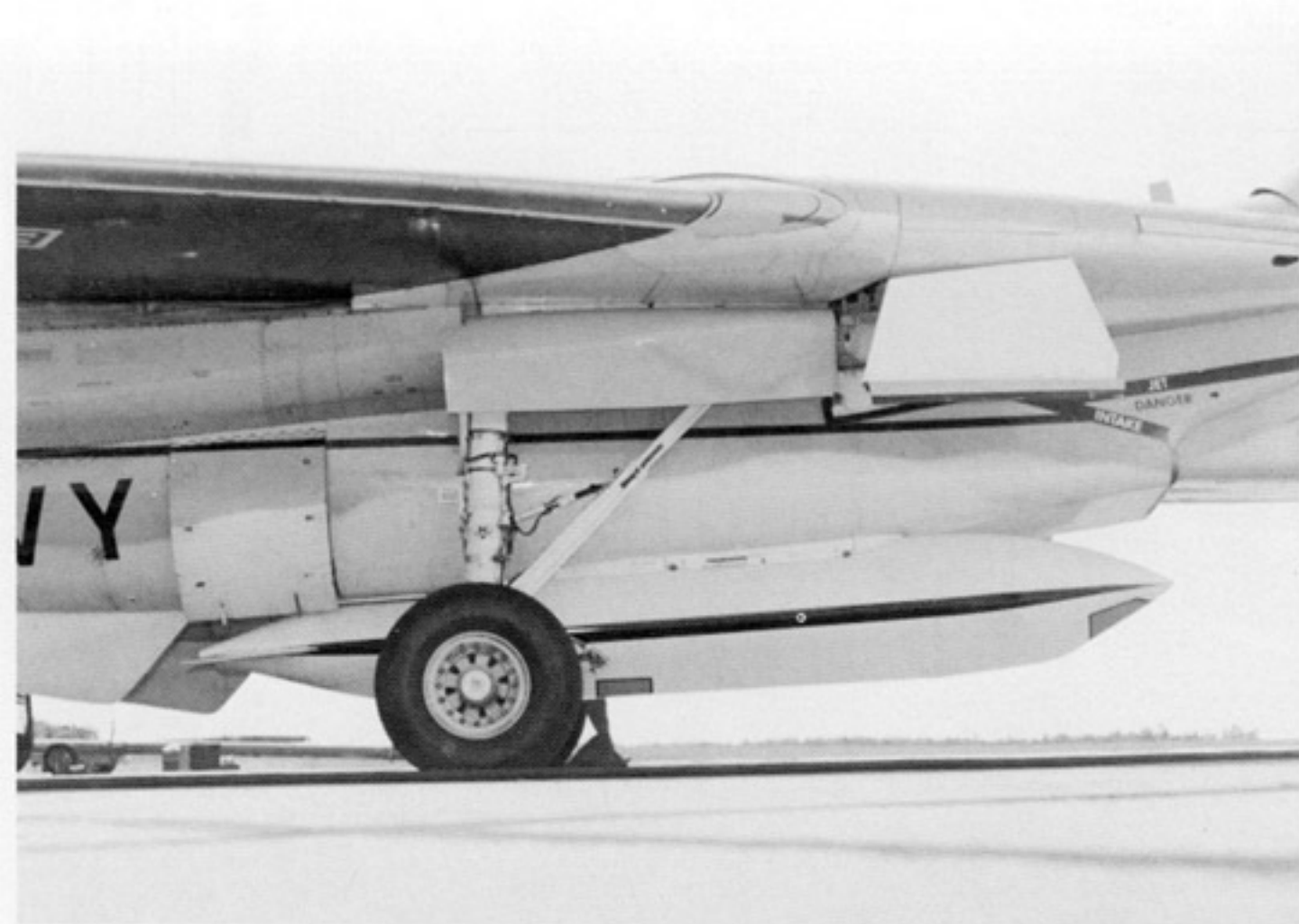
An early prototype of the Tactical Aerial Reconnaissance Pod System (TARPS) is mounted on the starboard engine nacelle during tests of the system held in 1973. This pod had horizontal fins at the rear of the pod and was mounted on the F-14's fuel tank hard point. (Grumman)
