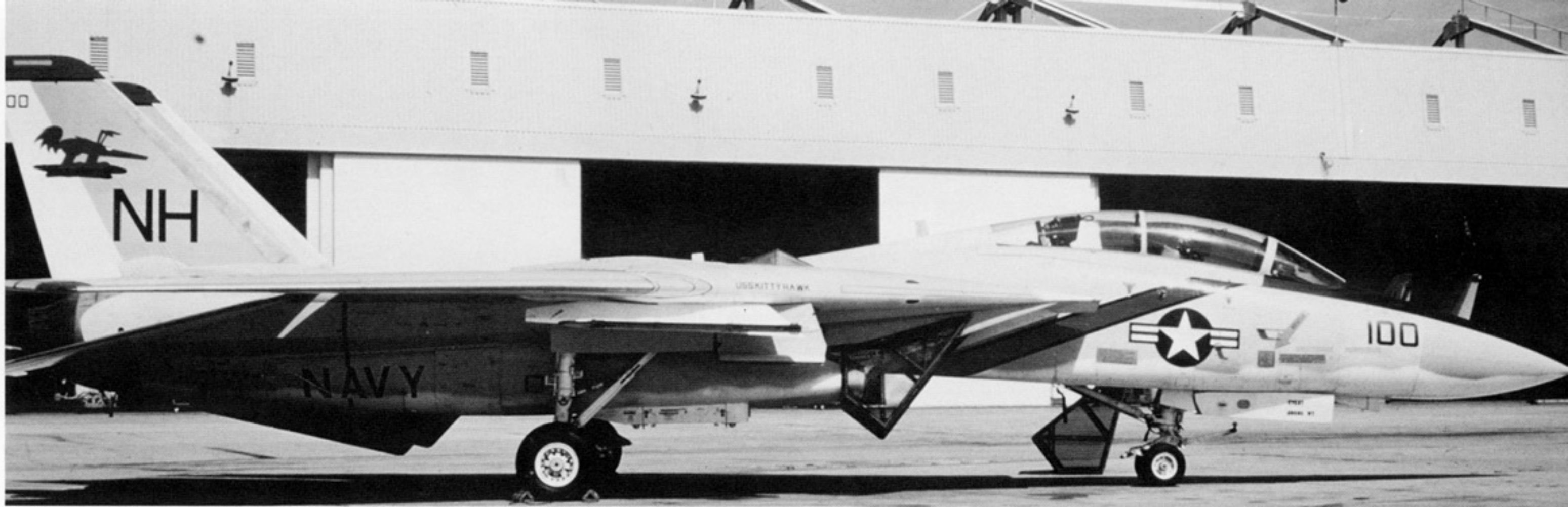
An F-14A (BuNo 159849) of VF-114 Aardvarks on the ramp at NAS Miramar, California, during late 1977. A Foreign Object Damage (FOD) screen is in place over the starboard intake while the port screen is visible just behind the nosewheel. The Aardvark, fuselage stripe, and tips of the vertical stabilizers are Orange. (INTERAIR)
