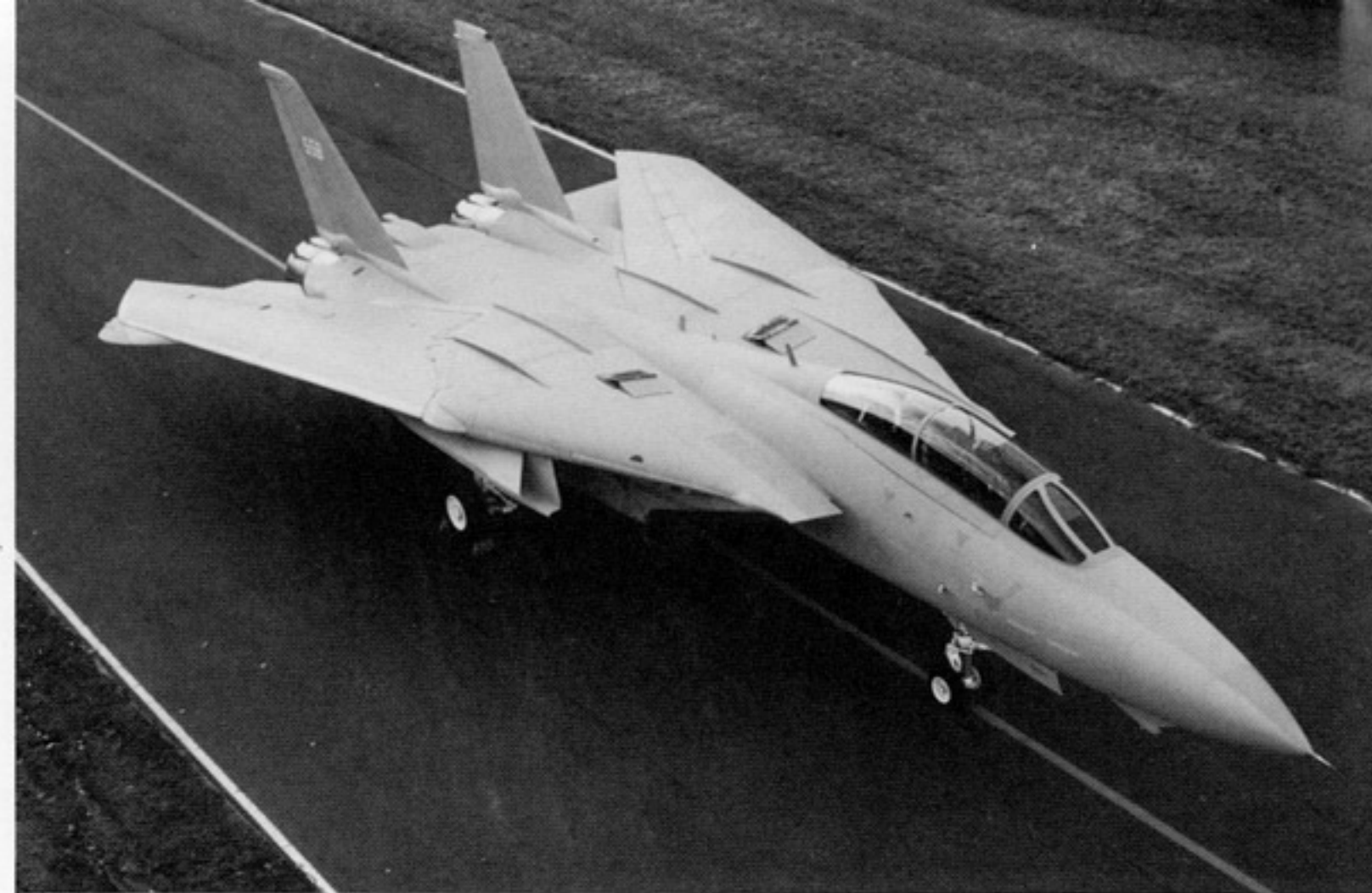
The first production F-14A (Plus) on the ramp at the Grumman facility. The aircraft was Fabrication Number 558 (BuNo 162910). The engine nozzles for the General Electric F110-GE-400 are larger than those of the TF-30s used on the standard F-14A. The aircraft was delivered to NATC, Patuxent River, Maryland during December of 1987 for acceptance tests by the Navy. (Grumman)
