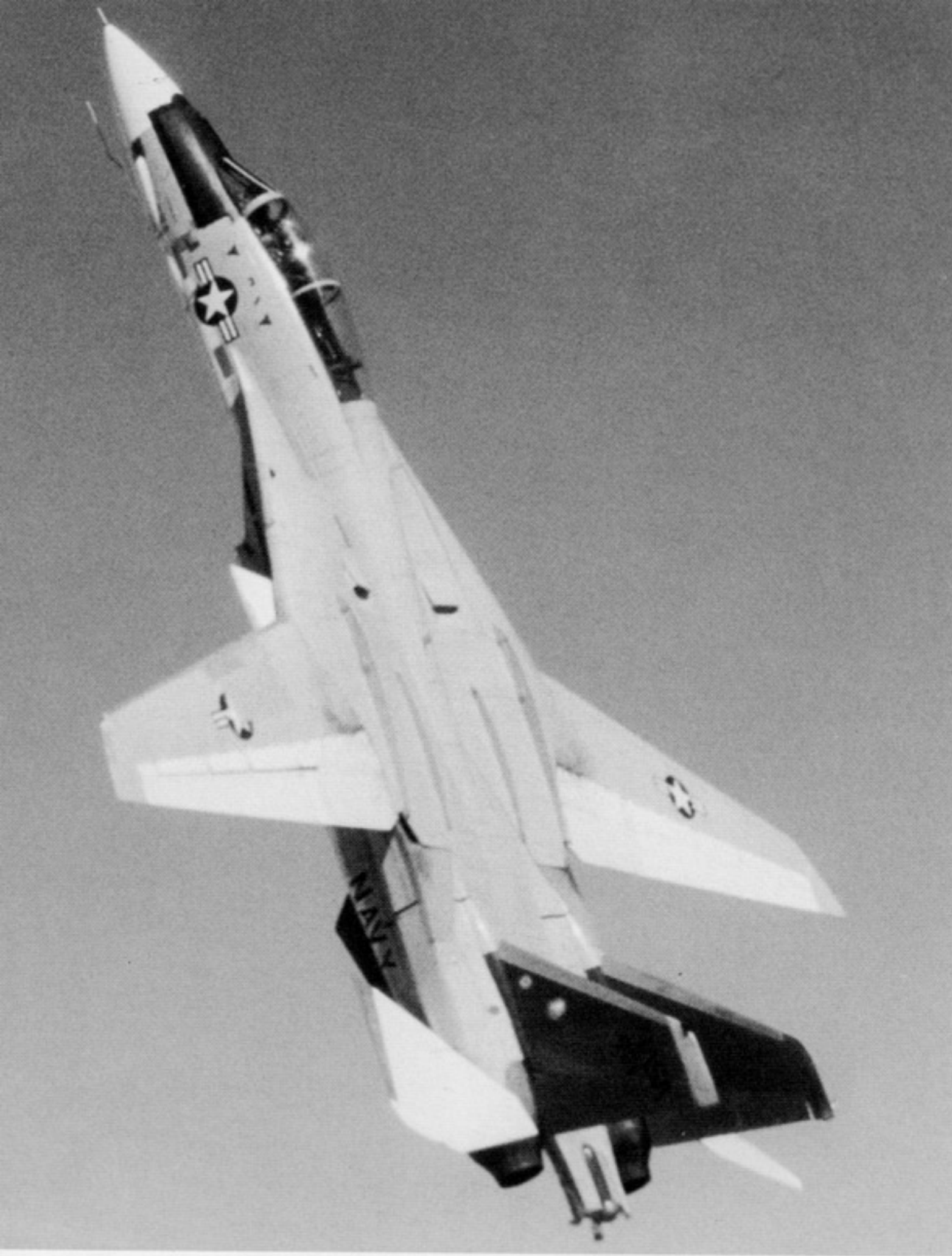
During testing, NASA and Navy pilots reported that angles approaching 70 degrees could be flown with the aircraft still flying forward, the only lift coming from the fuselage. Flight testing of the Alleron-Rudder Interconnect (ARI) commenced during June of 1985 and was completed by 9 August 1985. (NASA)
