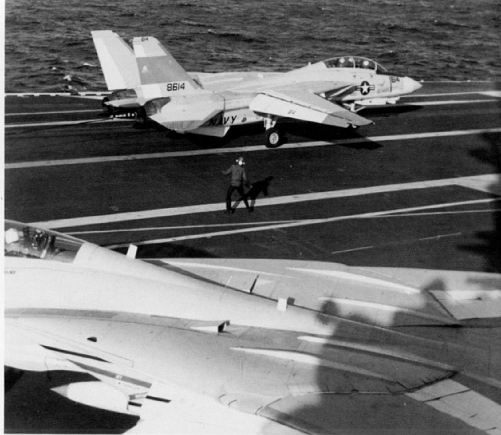
Tomcat 614 (BuNo 158614) comes to a halt after making an arrested landing aboard USS FORRESTAL (CV-59). After the deck crew disengaged the arresting cable, the F-14 taxied into position for another launch. F-14A (BuNo 158613), in the foreground, is carrying an inert AIM-54 Phoenix on the wing pylon. (Grumman)
