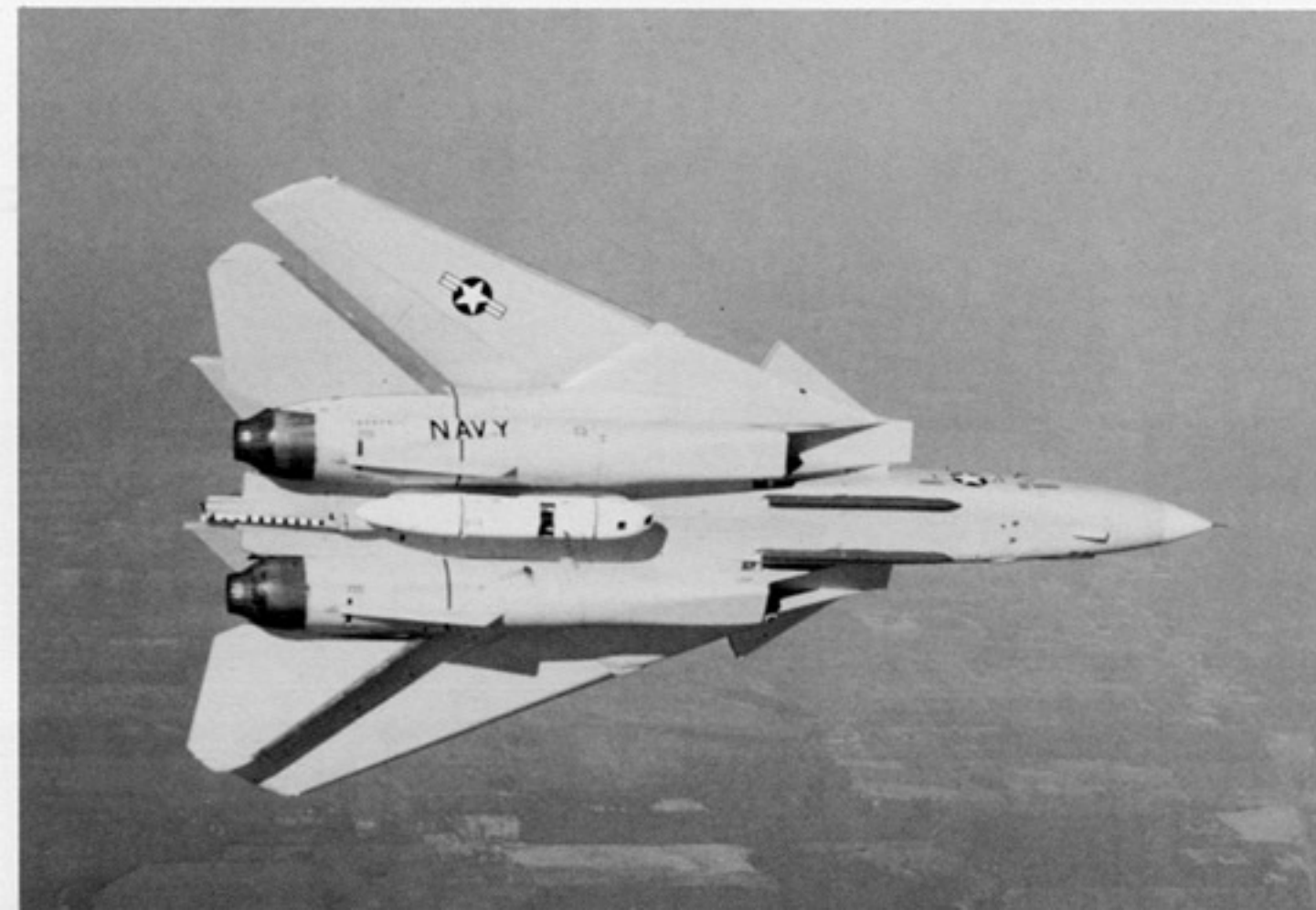
The first of forty-seven F-14As built as dedicated TARPS aircraft was BuNo 160696. The production variant of the TARPS pod is now carried on the number 5 weapons station, leaving the fuselage hard points clear for fuel tanks. The pod is seventeen feet long and contains two cameras and an infrared line scanner. (Grumman)
