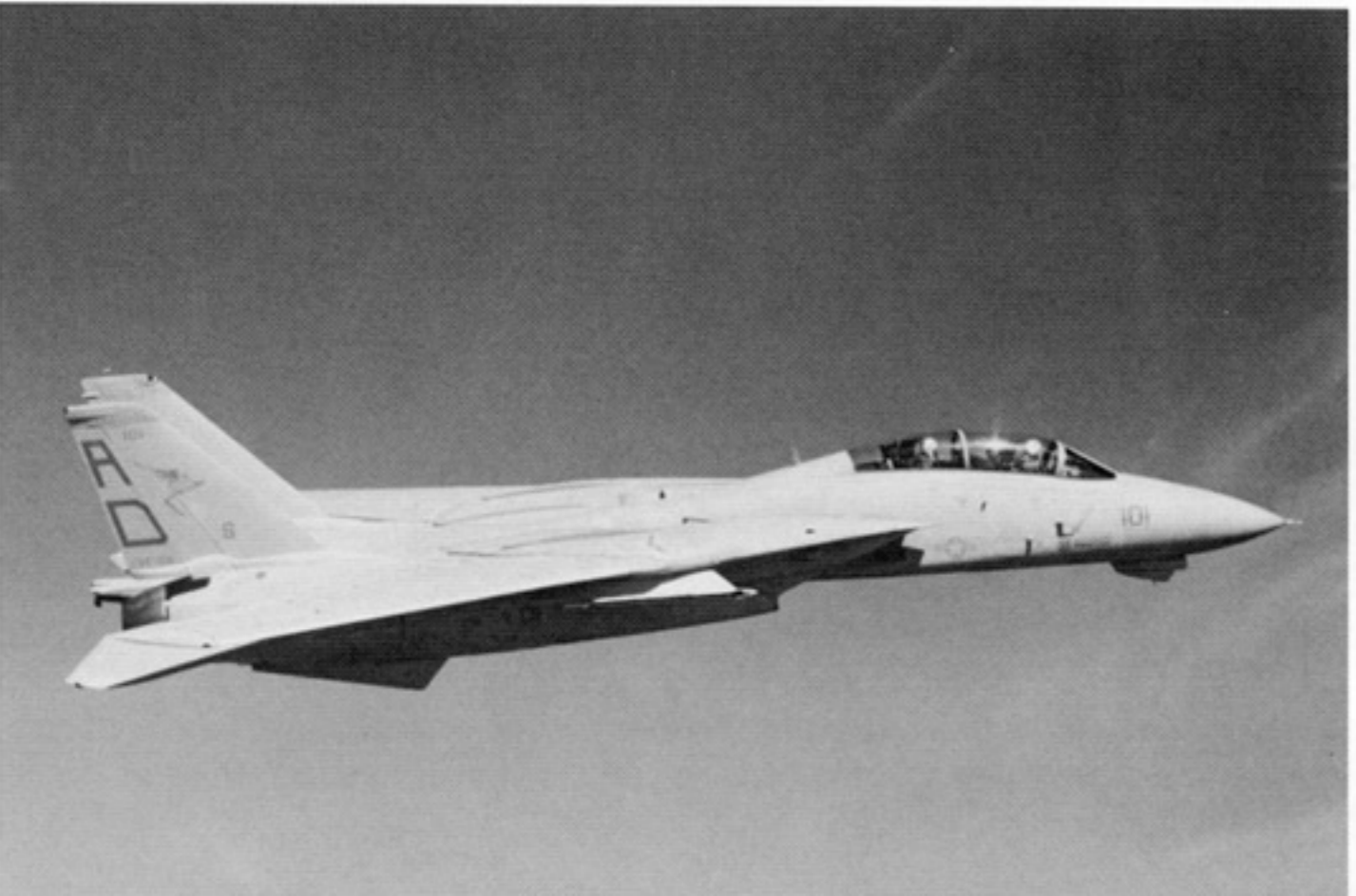
This F-14A (Plus) of VF-101 Grim Reapers is equipped with the Northrop developed Television Camera Set (TCS) pod under the nose. The aircraft is finished in overall Medium Gull Gray and carries an S (for Safety) on the vertical stabilizer. (USN via Bill Ennis)
