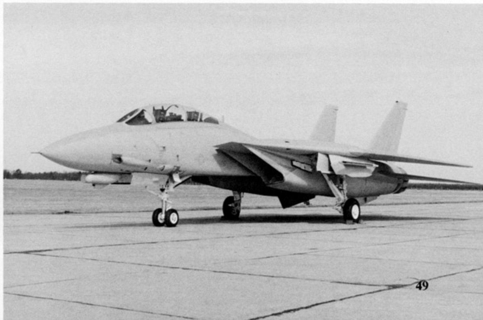
The TCS portion of the dual TCS/IRSTS chin pod has a cover in place over the lens to protect it. F-14D production is scheduled to run through 1995 and will involve both new production aircraft and the remanufacture of F-14As to F-14D standards. (Grumman)
