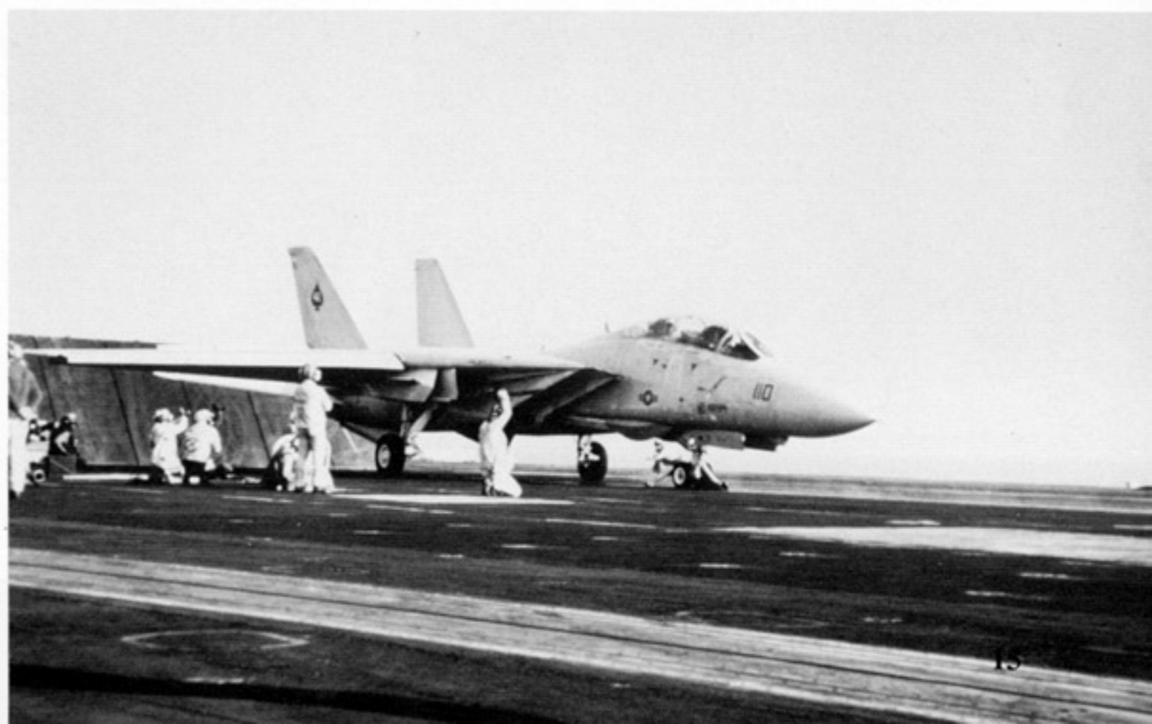
An F-14A of VF-41 Black Aces prepares for launch with the nose tow bar in the catapult shuttle and the hold back bar in place. The Black Aces made the first combat kill by an F-14 during 1981 when two VF-41 Tomcats shot down two Lybian Sukhoi Su-22 Fitters over the Gulf of Sidra. (USN by LT Bill Linder)
