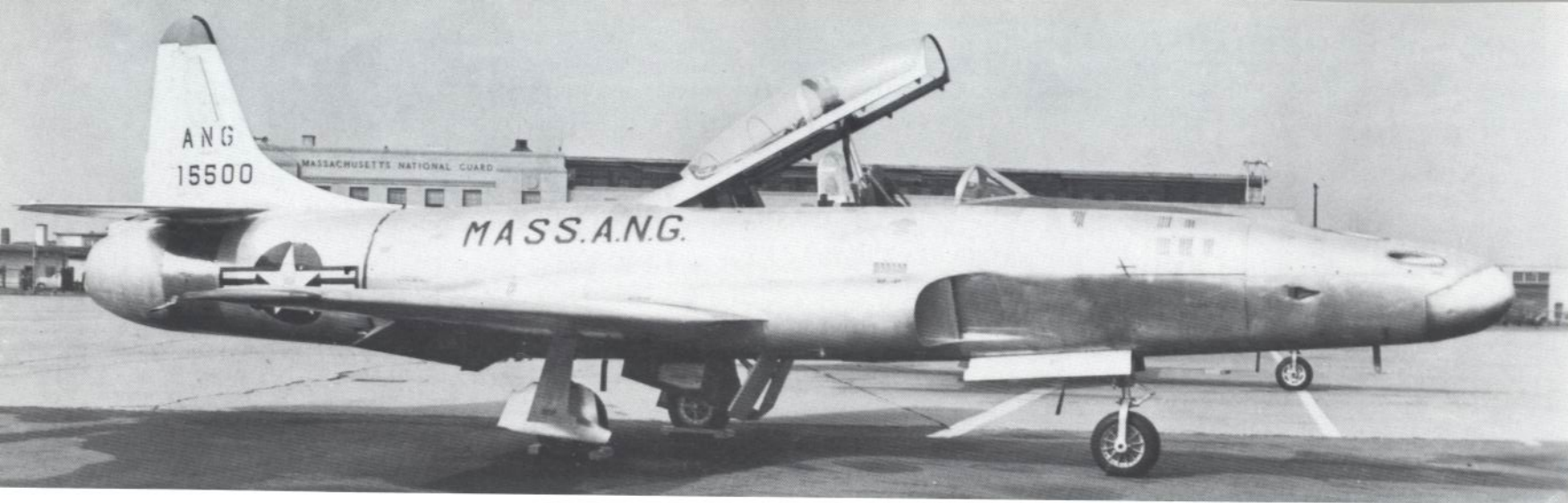
F-94C #51-5500 was fitted with a General Electric M-61 Vulcan rotary cannon, later used in the F-104 Starfighter. (USAF, Baker via Trump)
