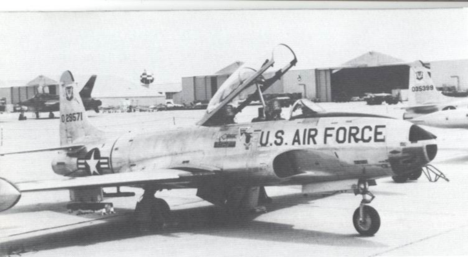
A TAC AT-33A at McClellan AFB. AT-33s had full armament capabilities including two .50 cal. guns, rockets and bombs. Most served with foreign air forces such as the Republic of Korea. (AFM)
