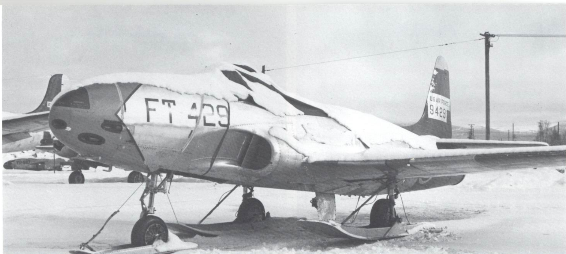
F-80C #49-429 was forced down in the Alaska tundra and had to be fitted with special skis so she could be flown out. (USAF)
