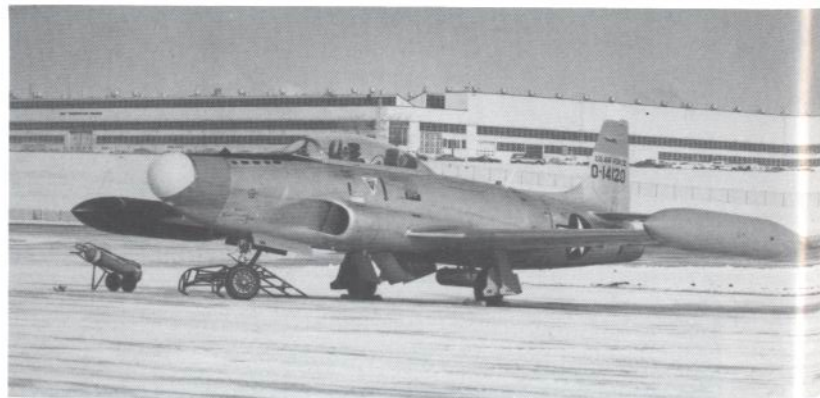
The F-94B may have passed from USAF's inventory, but its ghost lives on in the form of this T-33A seen at Offutt AFB, NB, 13 February 1980. The trainer has been fitted with an F-94B nose complete with blanked off gun troughs. (LTC George R. Cockle)
