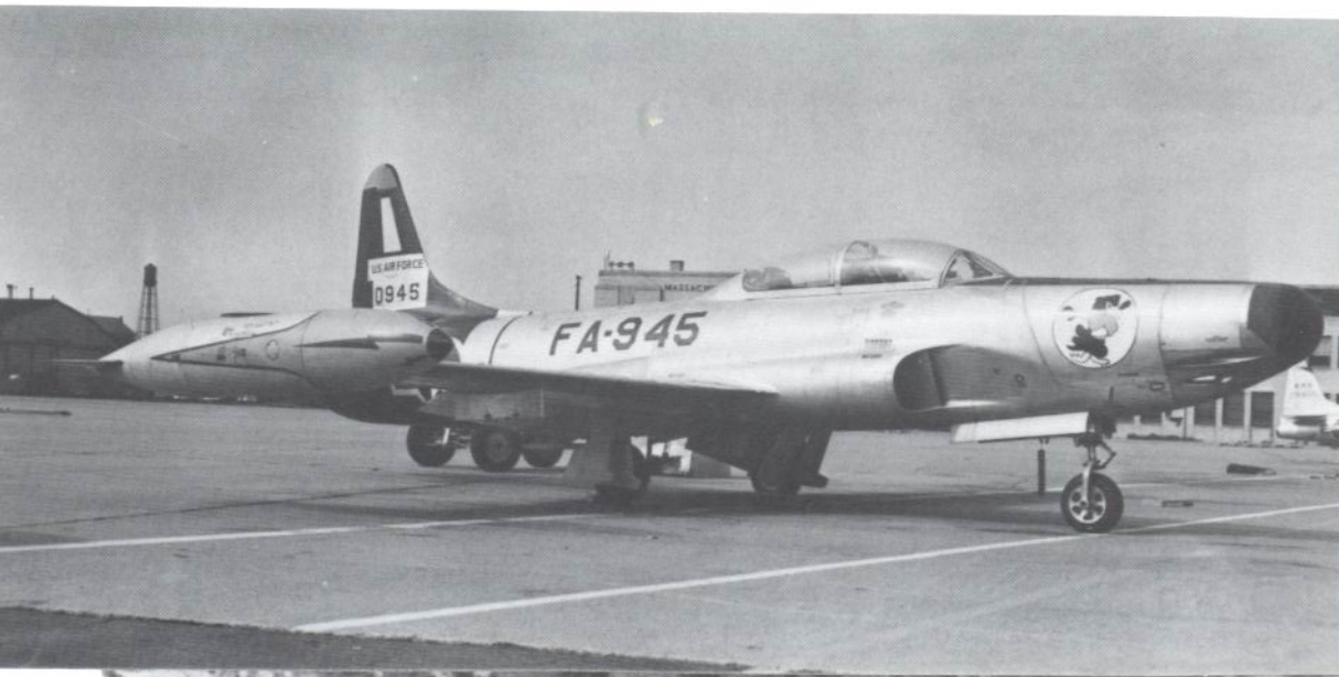
The F-94B may have passed from USAF's inventory, but its ghost lives on in the form of this T-33A seen at Offutt AFB, NB, 13 February 1980. The trainer has been fitted with an F-94B nose complete with blanked off gun troughs. (LTC George R. Cockle)
