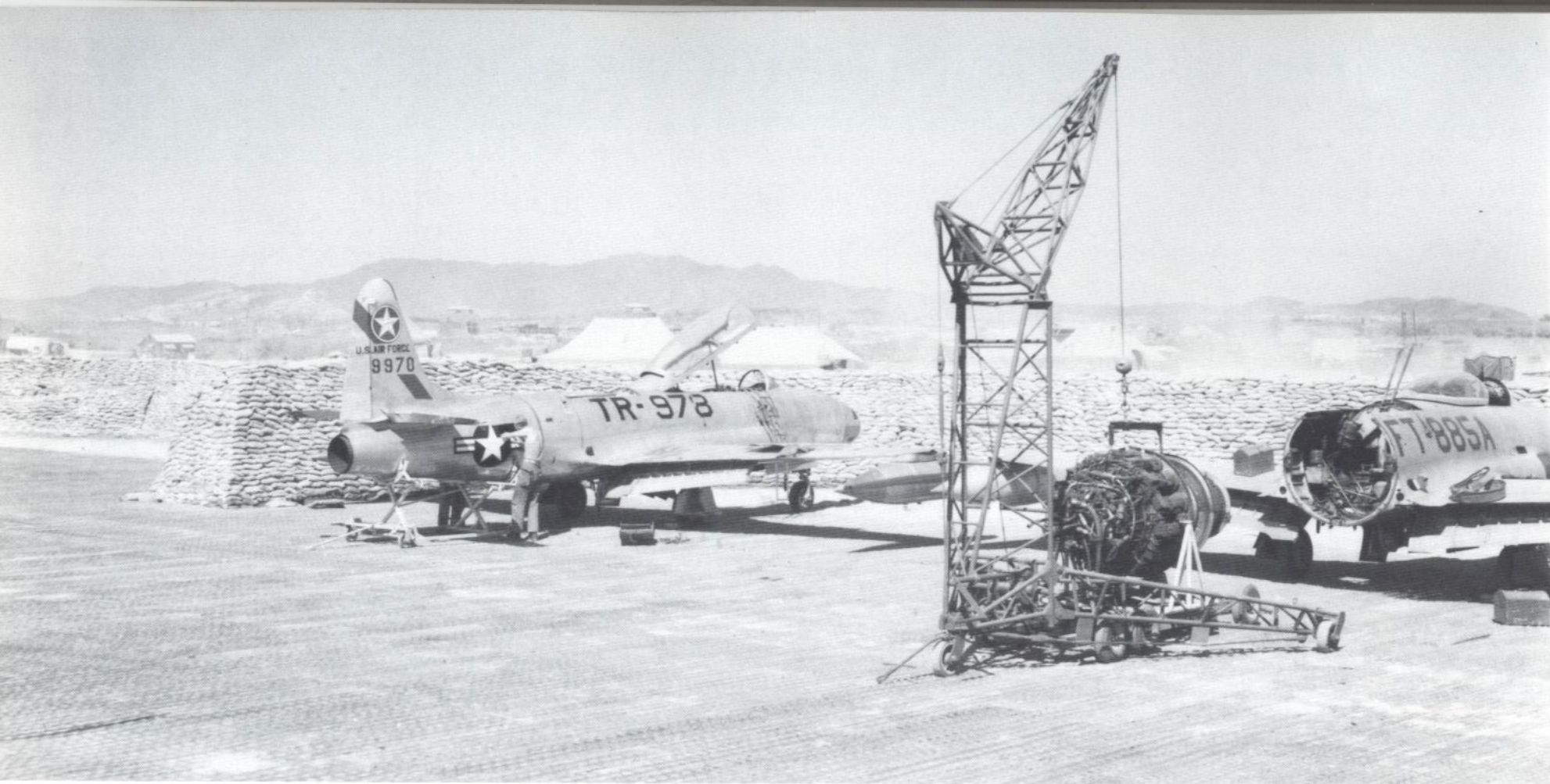
A T-33A from the 116th FBGp, an F-84 unit, undergoes an engine change at K-14. The 116th was a Texas ANG unit called into active service. (USAF)
