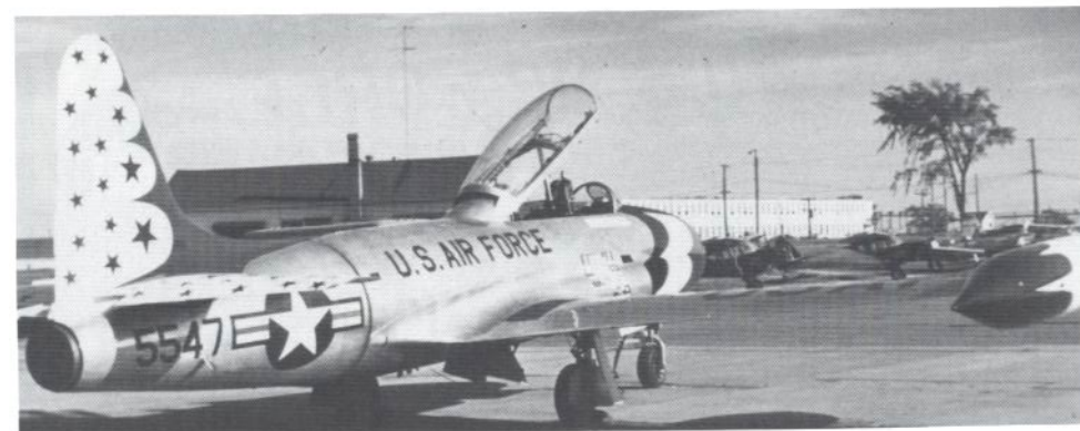
A TAC AT-33A at McClellan AFB. AT-33s had full armament capabilities including two .50 cal. guns, rockets and bombs. Most served with foreign air forces such as the Republic of Korea. (AFM)
