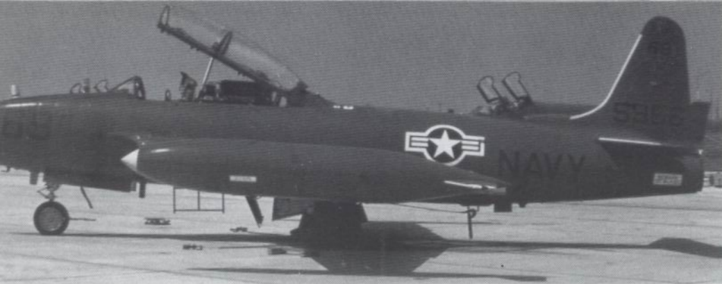
Many T-Birds have been converted to drone QT-33Bs. Note radio gear in place of second pilot. This QT's overall gloss orange. (Jem Slides)
