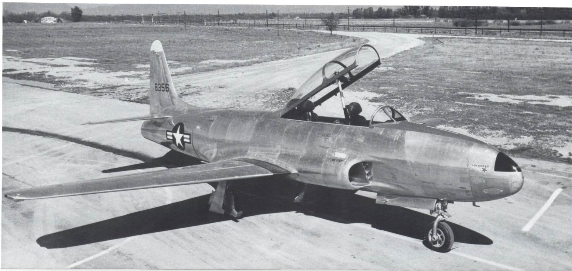
(Above) The first Air Force jet trainers were the 'Captivair' F-80As secured to the ground by steel frames around the wings. (Below) The first TF-80C (T-33A) was actually a converted P-80B. It was the first real U.S. jet trainer. (USAF and Lockheed)
