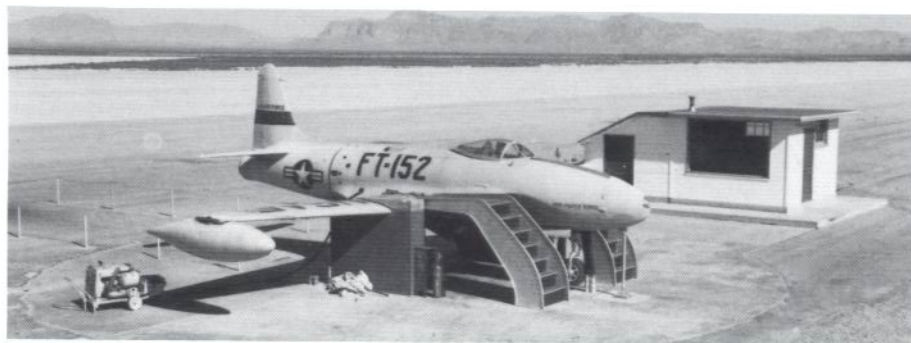
(Above) The first Air Force jet trainers were the 'Captivair' F-80As secured to the ground by steel frames around the wings. (Below) The first TF-80C (T-33A) was actually a converted P-80B. It was the first real U.S. jet trainer. (USAF and Lockheed)
