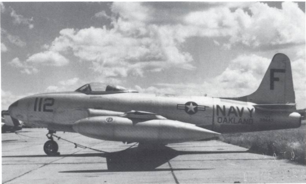
Seen in July 1956, this is one of the F-80Cs transferred to the Navy as TV-1s for use as jet familiarization trainers. These aircraft were essentially identical to standard USAF F-80Cs. (Menard)
