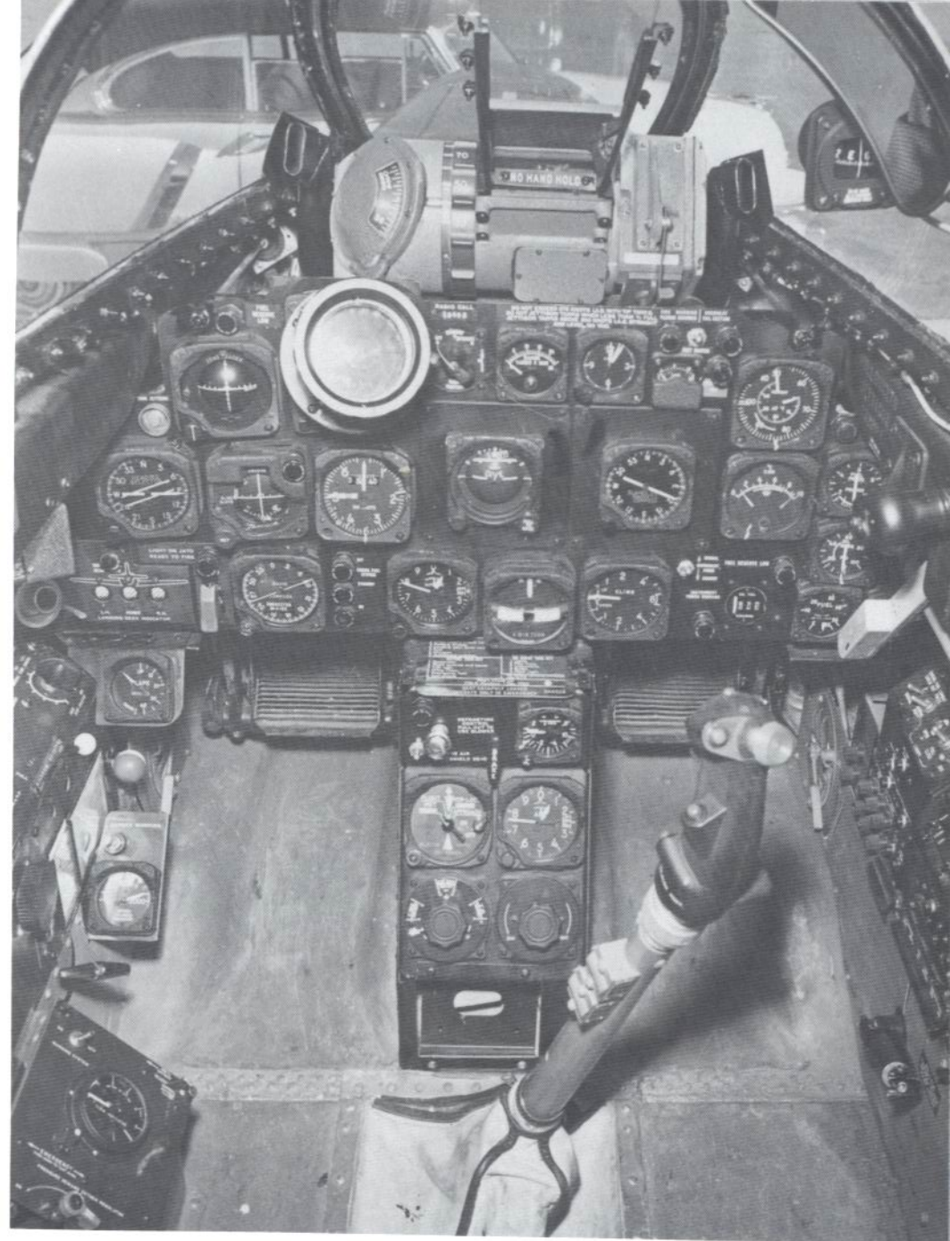
The F-94B front cockpit. Cockpit colors were chromate green floors and walls with black consoles. (AAHS)
