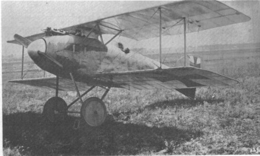
Albatros D.II prototype with upper wing in the lowered position caused by the new cabane system. Note non-standard windscreen. As on D.I prototype, no armament was carried.
