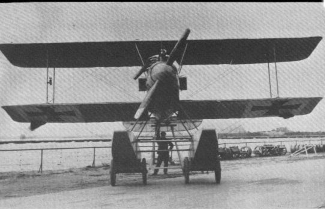
Albatros W.4 prototype, serial 747, ordered in June 1916 and completed three months later. It is seen in these three views being examined by German Naval personnel. Note the square-section floats, characteristic of early versions.
