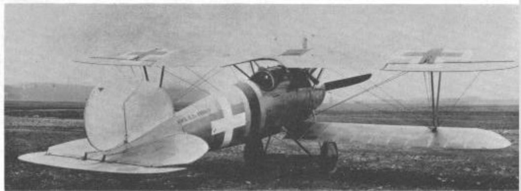
(Left & Below) O.A.W.-built D.Va, serial A.W.S. D.6988/17, possibly of Jasta 78b, was interned in Switzerland after the pilot became lost. The aircraft carries late-style German national markings, introduced in June 1918. The view below shows the aircraft after its rudder and fuselage crosses have been painted out, the latter seemingly replaced with a Swiss white cross. Initials A.W.S. in serial stood for Albatroswerke Schneidemuhl another name for Ostdeutsche Albatros Werke .
