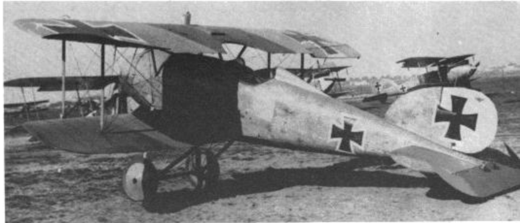
The only verified Albatros D.IV prototype. Note small headrest, square balance on rudder, larger chord of lower wing, parallel interplane struts and completely cowled engine. Of three examples ordered, this is probably the only one completed.
