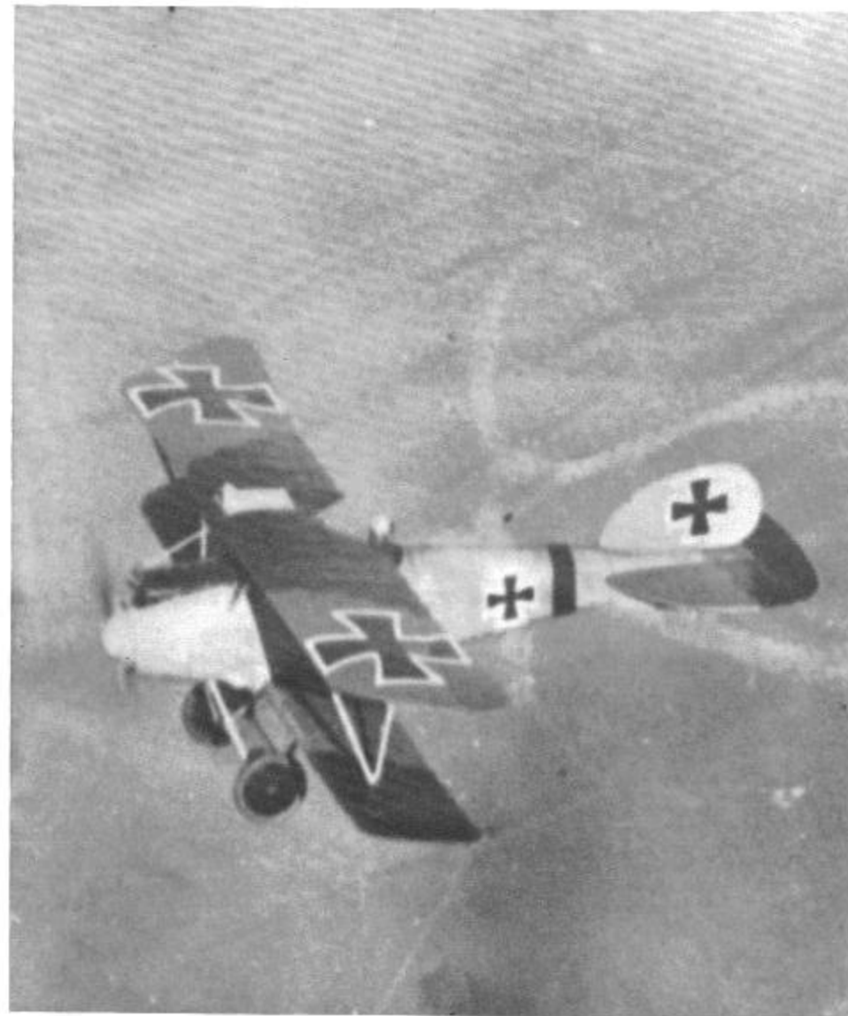
An O.A.W.-built D.III over the Russian Front. Dark green and mauve camouflage on upper wing is apparent, as is radiator located on starboard side of wing center section.
