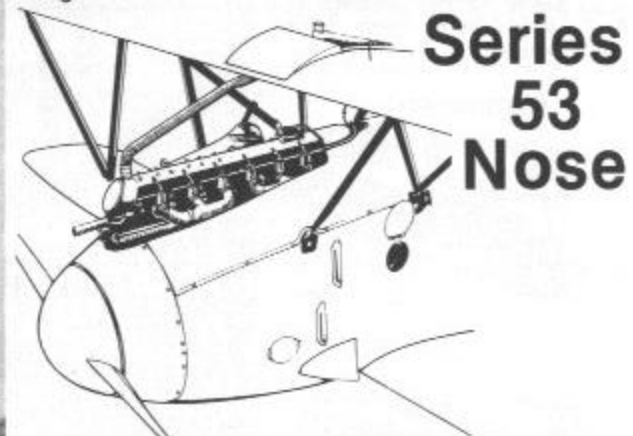
Oeffag-built D.III 53.24 was fifth D.III of the series (serials for D.III variants had begun with 53.20). Power plant was 185hp Austro-Daimler, which gave aircraft a top speed of about 110mph. Rate of climb was also slightly superior to German D.III.
