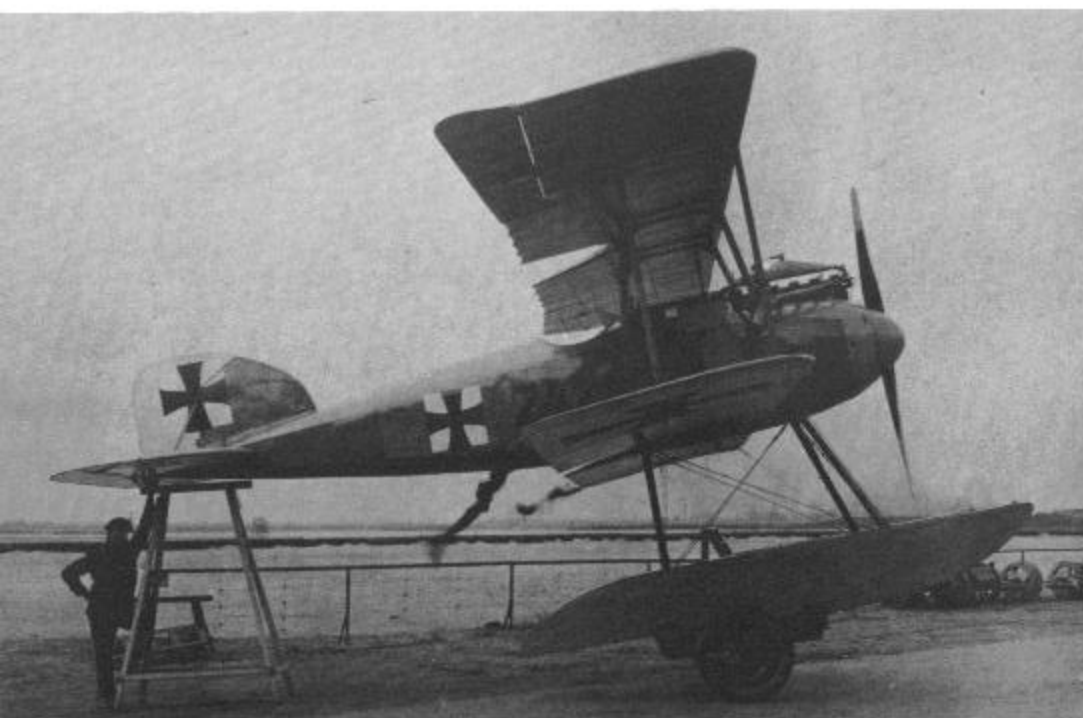
Albatros W.4 prototype, serial 747, ordered in June 1916 and completed three months later. It is seen in these three views being examined by German Naval personnel. Note the square-section floats, characteristic of early versions.
