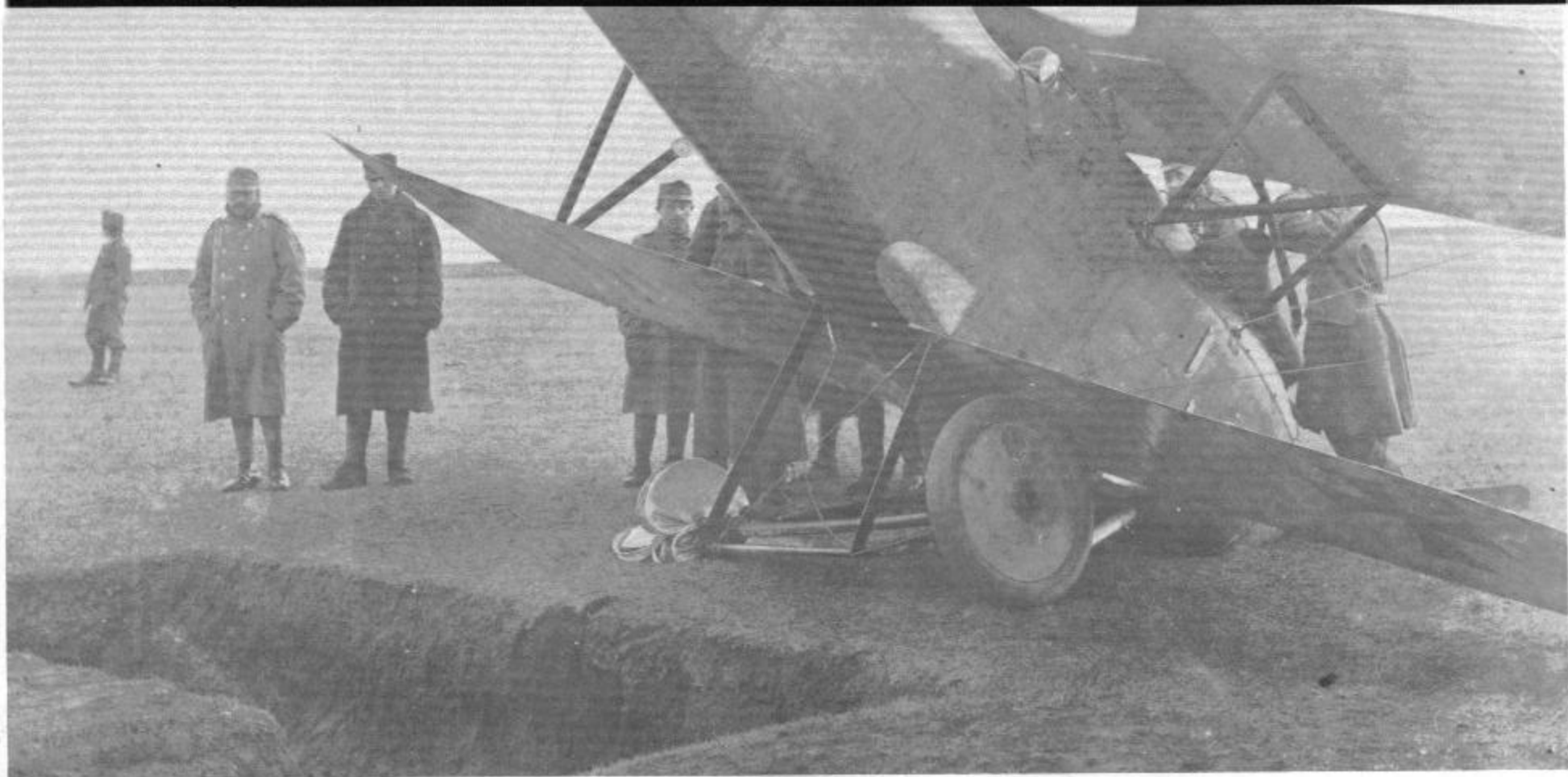
D.III, serial 53.40, flown by Oblt. Fischer cracked up during landing, having apparently hit the ditch shown. Blast tubes of buried Schwarzlose guns can be seen at sides of engine cylinder bank. Also note the shaped aluminum fairings which streamline the wing root into the contours of the lower fuselage.
