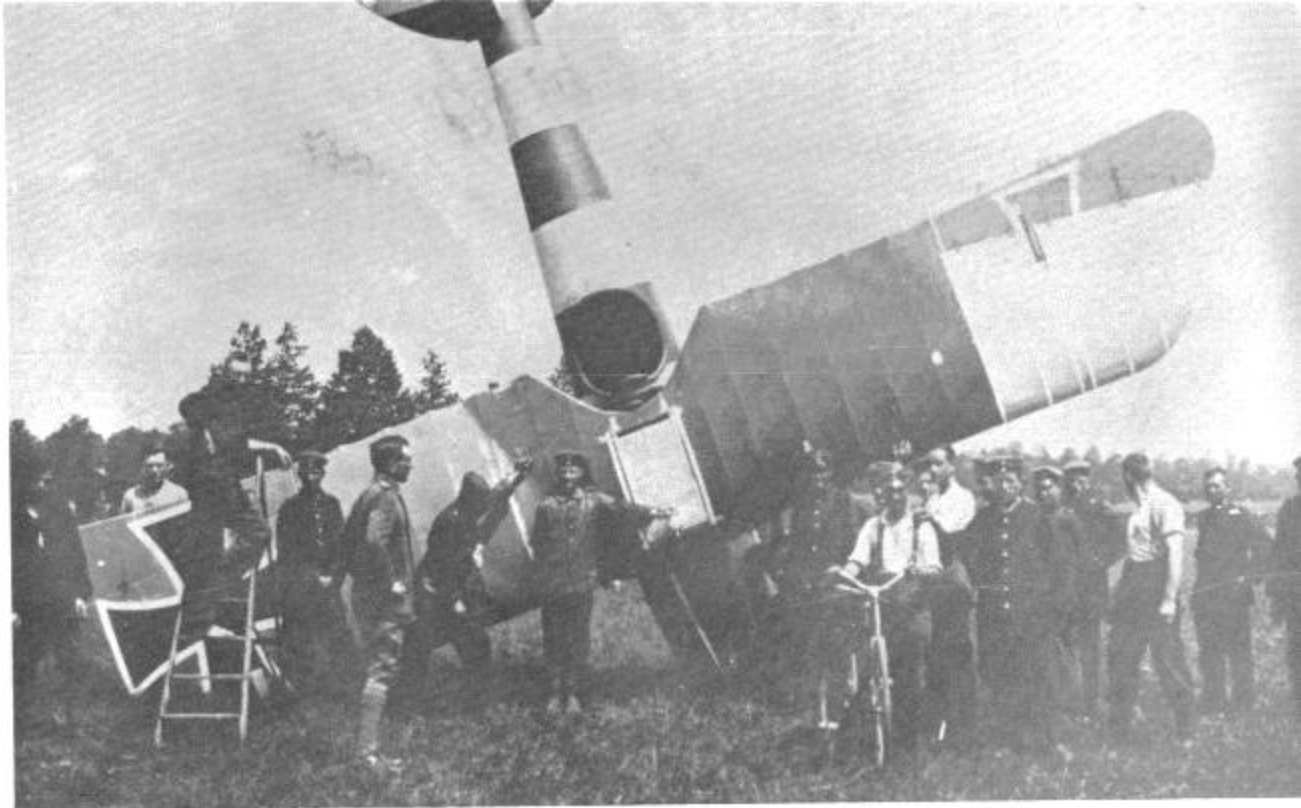
Pilots and mechanics of Jasta 26 discuss ways of righting Lt. Bruno Lörzer's black-and-white striped D.III. Note fabric repair patch on port upper wingtip, central location of wing radiator and green/brown upper wing camouflage pattern.
