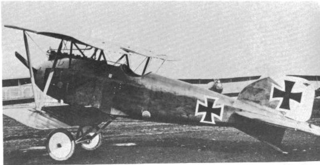
Albatros D.III prototype. Fuselage appears to be covered in a dark wood stain instead of clear varnish. Albatros trademark is apparent on clear-doped rudder. Note narrow-chord lower wing and 'V'-shaped interplane struts.
