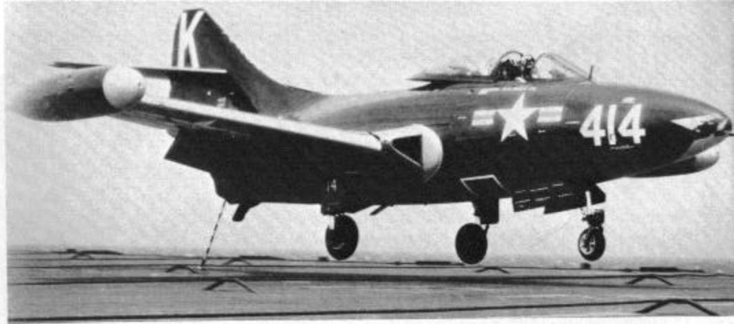
F9F-2 flown by Ens. Chew of VF-34 lands aboard the USS Leyte. Trim on this Panther is Yellow. Note the tailhook just about to engage the #3 wire. 6 August 1951. (National Archives)
