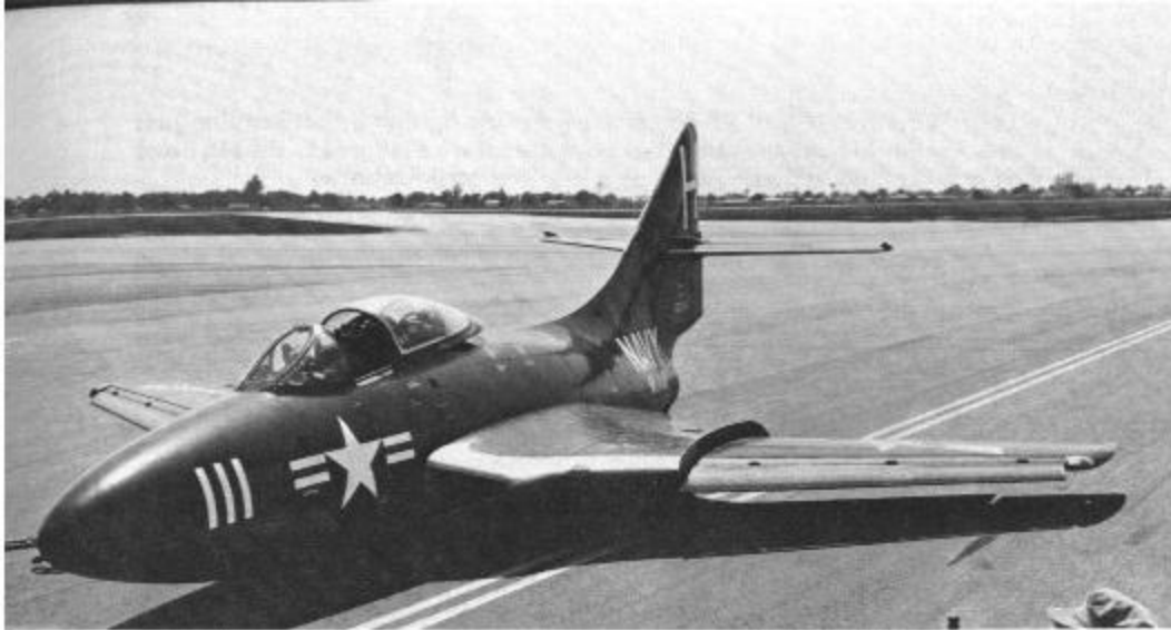
F9F-6 (127268) belonging to the Naval Air Training Unit at NAS Miami has made a wheels-up landing, stopping within a couple of feet of the runway centerline. May 1955. (Clay Jansson via Peter Mancus)
