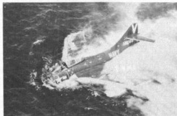
F9F-8 (141065) of VF-112 loses its nose section forward of the canopy on impact with the water. USS Essex off San Diego, CA. May 1956. (National Archives)
