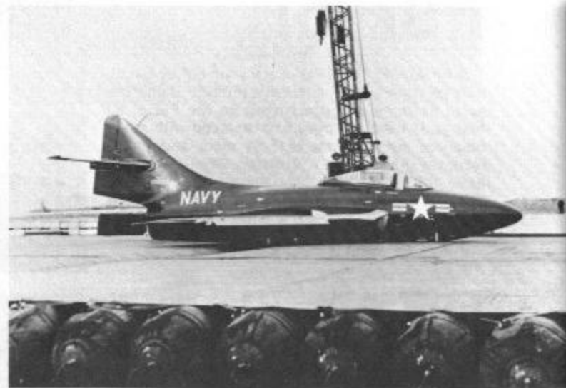
One of two Cougars modified to take part in an experiment called 'Flex Deck'. F9F-7 (130863) has landed on a rubberized fabric 'deck' which was secured to air bags. The 'deck' was 375FT long with arresting cables stretched across its 80FT width. The purpose of this Navy experiment was to determine the practicality of saving weight by eliminating the need for landing gear. NATC Patuxent River, MD. February 1955. (National Archives)
