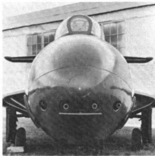
Business end of four 20mm cannon positioned in the nose of a F9F-2B at MCAS Quantico, VA. May 1978. (Jim Sullivan)
