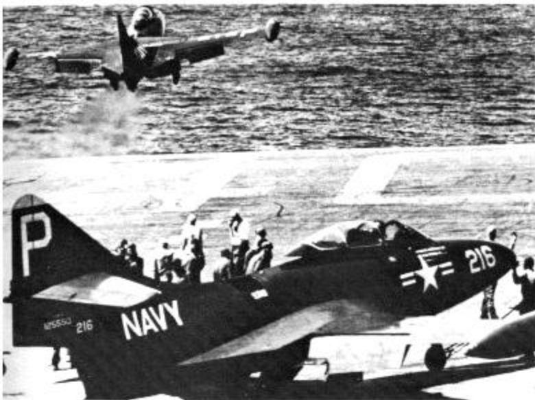
Both catapults having been fired, F9F-5 (125550) of VF-102 is guided on the starboard launch track aboard the USS Tarawa. The Panther just airborne is departing at approximately 110MPH. March 1954. (Walt Olrich)
