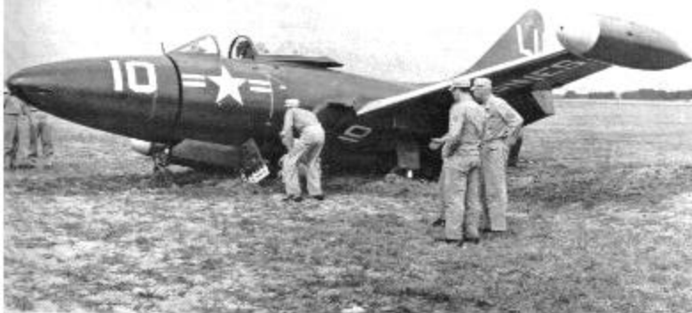
F9F-5 of MARS-37 has collapsed the starboard landing gear and dug up some Florida real estate after leaving the runway at NAS Miami, Fla. October 1953. (Clay Jansson)
