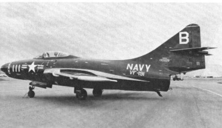
F9F-6 (130929) of VF-191 is trimmed in Red and White. Note the bulge under the nose that housed the IFF radar. San Francisco, CA. 8 August 1954. (Bill Larkins)
