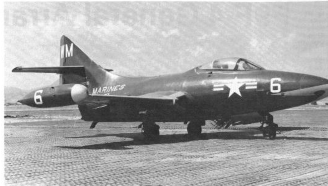
F9F-4 (125226) from MAG-33 is seen on the Marston mat steel strip at Pohang, Korea (K-3). Note the extended dive brakes, the natural aluminum strip on the fin and horizontal stabilizer leading edges. Trim color on the nose is Yellow. September 1953. (Clay Jansson)
