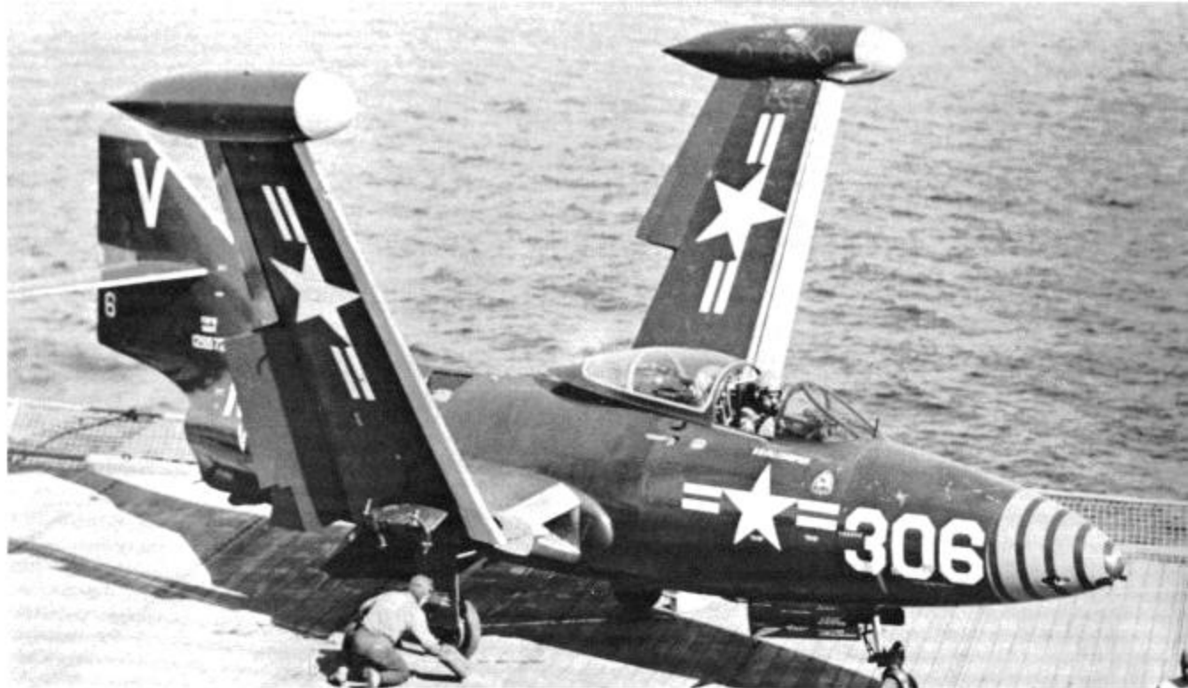
F9F-5 (125572) of VF-113 aboard the USS Boxer off San Diego, CA. The wing folding mechanism was designed with strength capable to operate the wing with full tip tanks and six 500lb bombs in a 32 knot wind across the deck. Nose and tail trim on this Panther is Medium Blue. 25 February 1953. (National Archives)
