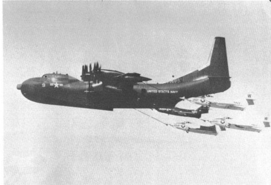
A flight of four F9F-8s of VF-123 demonstrate multiple in-flight refueling while attached to a R3Y-1 flying boat. 31 August 1956. (National Archives)
