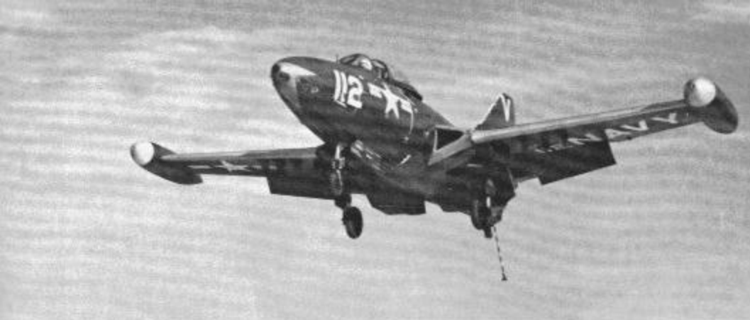
F9F-2 of VF-111 just moments away from landing aboard the USS Philippine Sea. Aircraft is trimmed in Red. Note the six inch downward deflection of the "droop-snoop" wing leading edge slats. November 1950. (Ronald Gerdes)
