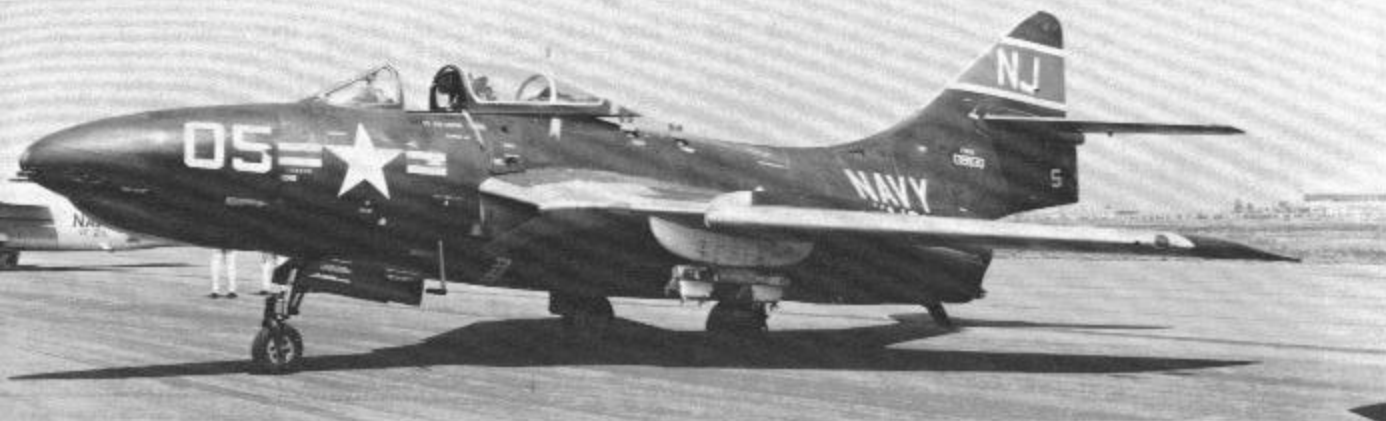
F9F-8 (138830) of VA-126 carries a single multiple-launch rack beneath each wing. The rudder trim colors are Dark Green and White. NAS Miramar, CA. 10 August 1957. (Bill Larkins)
