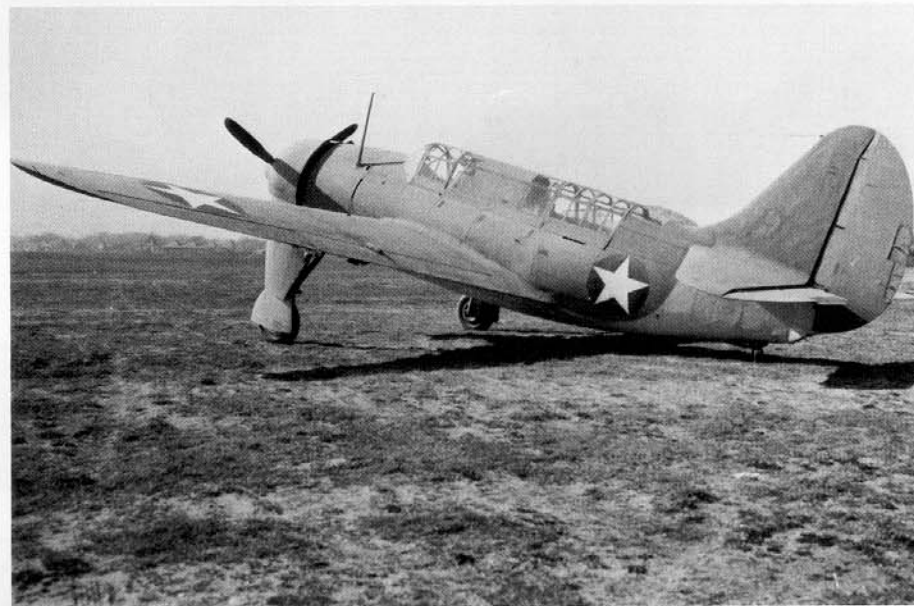
The Shrike prototype, still in Navy camouflage and carrying BuNo 00006 on its tail, is seen at Wright-Patterson Army Air Field, 27 October 1942. The prototype had the extended exhaust and smaller fixed tailwheel of production A-25As but retained such very early Helldiver features as the DF loop and lack of a flexible gun. (WPAFB/NARS)
