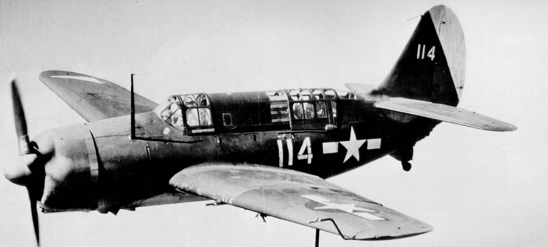
A recently delivered SB2C-4 in the now standardized markings of Yorktown's VB-3, February 1945. Note that the aircraft number has been repeated on the wing leading edge, and the canopy center section window appears to have been damaged and repaired. (USN via Jim Sullivan)
