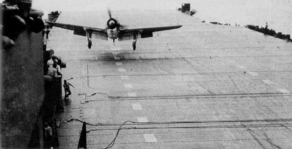
As with all units that transitioned into early Helldivers, VB-17 had its share of problems taming the Beast. It was involved in numerous barrier crashes or worse, as is the case with '35', a Mod III SB2C-1, caught in the process of turning itself into scrap on Bunker Hill, 11 September 1943. Note the red-rimmed national insignia. (USN/NARS)
