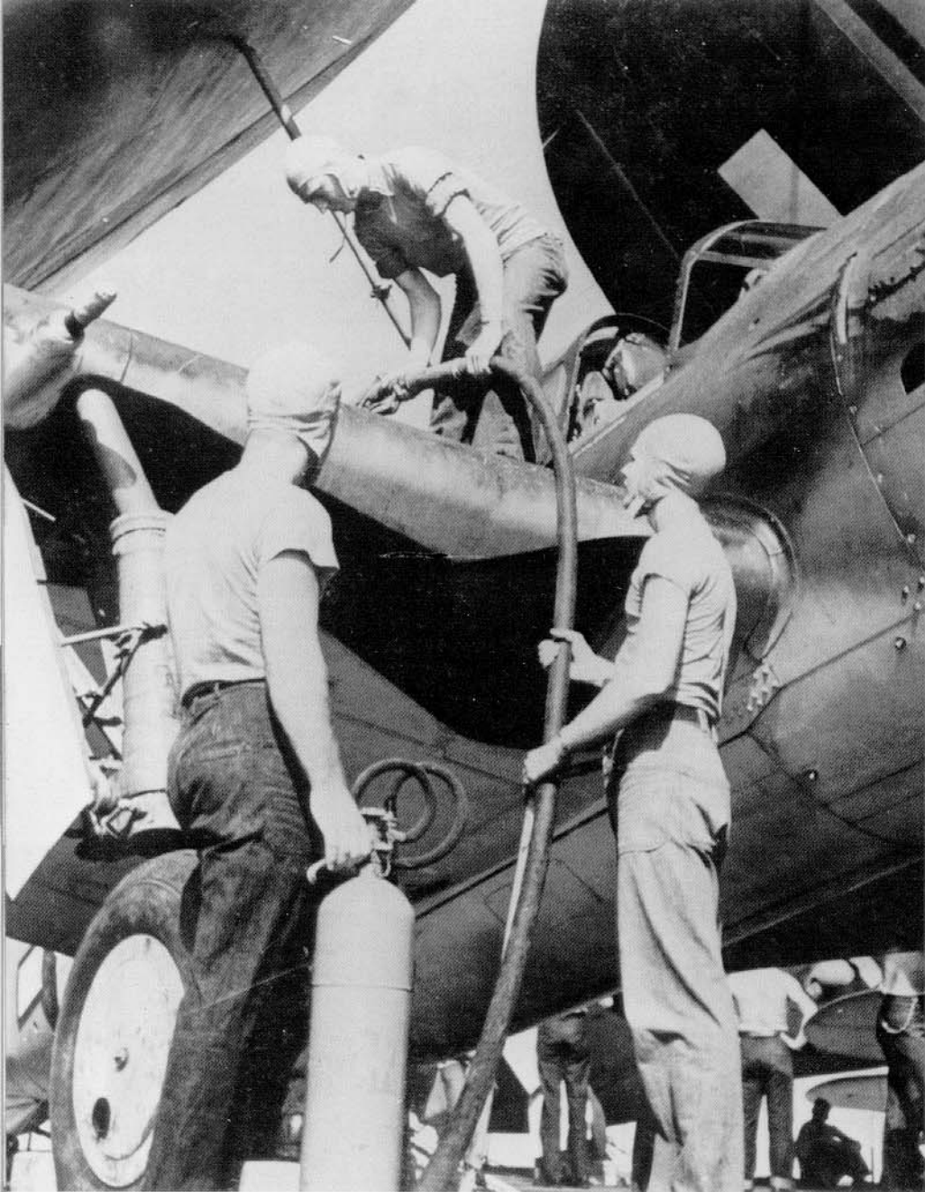
Arming and fueling aircraft and positioning ready aircraft on deck were practiced repeatedly during the slack days between raids. The ability of US deckcrews to handle aircraft rapidly in action was a major factor in more than one battle. With fire extinguisher at the ready, a crewman watches one of VB-15's Beasts being tanked up, 10 May 1944. (USN/NARS)
