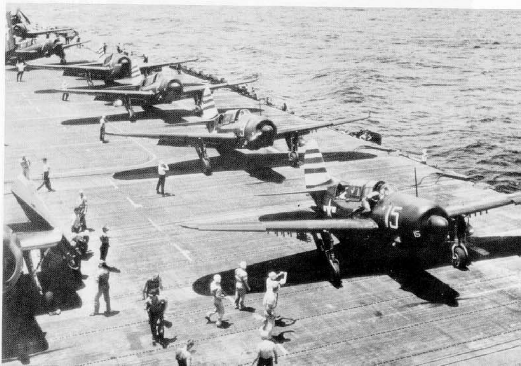
Five of Randolph's 'dash-4s' line up for takeoff, July 1945. These VB-16 Beasts, like most aircraft repainted Glossy Sea Blue after having originally been three-tone, retained a strip of Non-Specular Sea Blue in front of the cockpit which acted as an anti-glare panel. (USN via Dick Hill)
