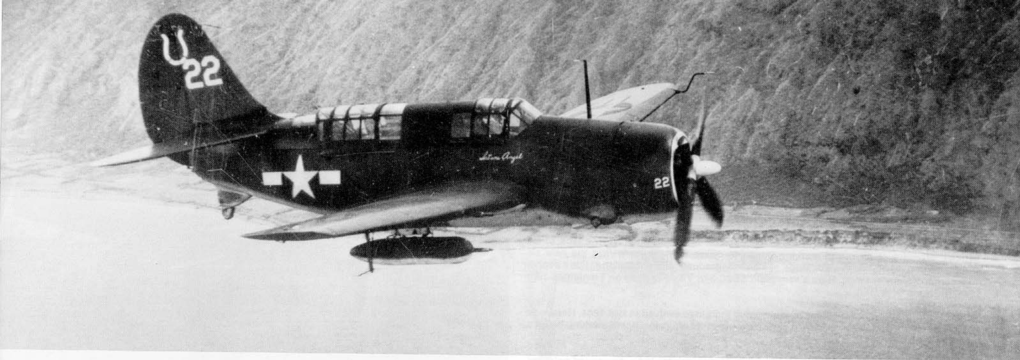
One-by-one the new air groups adopted markings. Satan's Angel, an SB2C-3 off Hancock (VB-7), displays that carrier's 'Omega' insignia, 13 October 1944. The pod under the right wing contains a pair of machine guns for added forward firepower. (USN/NARS)
