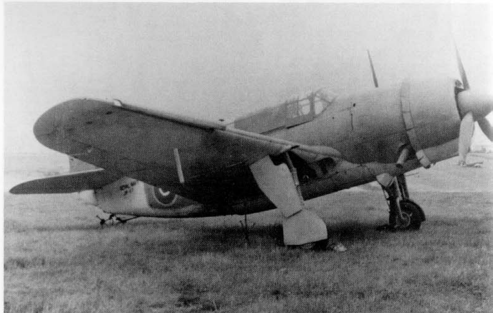
Another endearing quality of early Helldivers was frequent main gear collapse. Here, '13' plants its left wing on landing, Essex, 20 May 1944. (USN/NARS)
