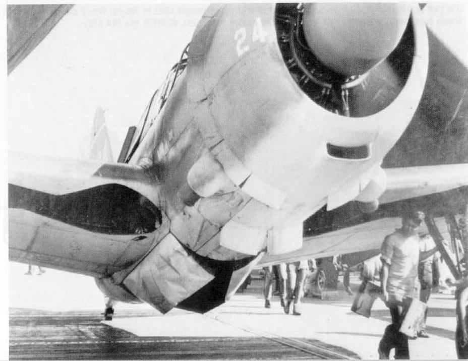
Some of the Beast's failings couldn't be blamed on the pilot. This SB2C-1C lost its bomb through its bomb-bay doors - while landing back on Essex, 20 May 1944. (USN/NARS)
