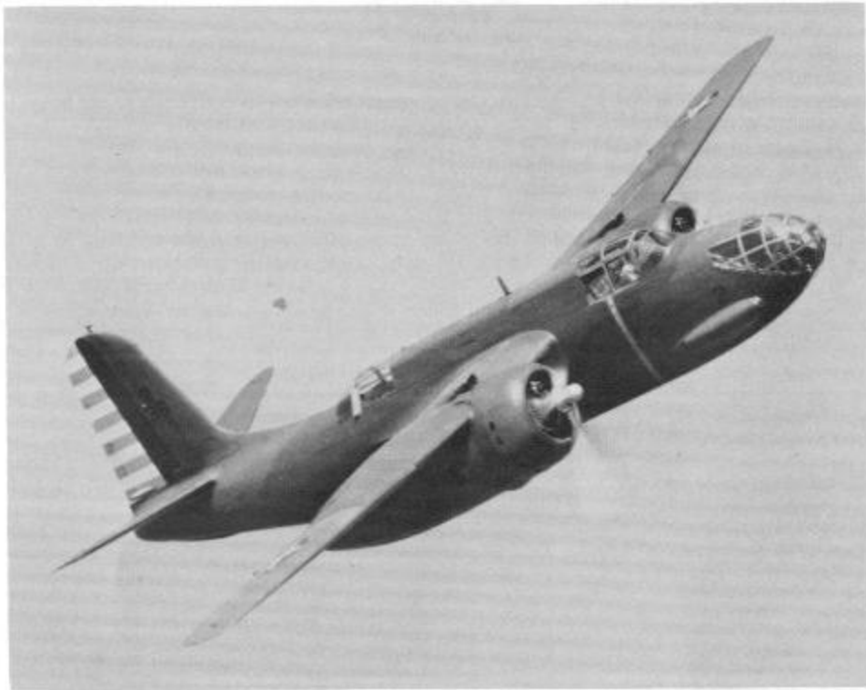
An A-20A from the 3rd Bomb Group camouflaged in Olive Drab 41 and Medium Green 42 with Neutral Gray undersurfaces. The vents on the cowling sides were an identification point of the early A model. These were later deleted from future production runs. (USAF)
