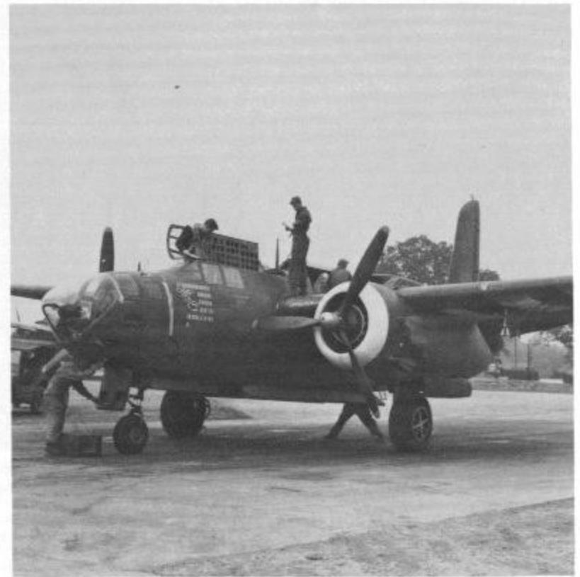
This A-20J-10 is being prepared for a mission by a ground crew from the 410th Bomb Group. At this time in her career Eva Mae had completed forty three missions. Notice how the leading edge of the wing by the fuselage has been worn down to bare metal from constantly being slid over by the crew and ground personnel. (USAF)
