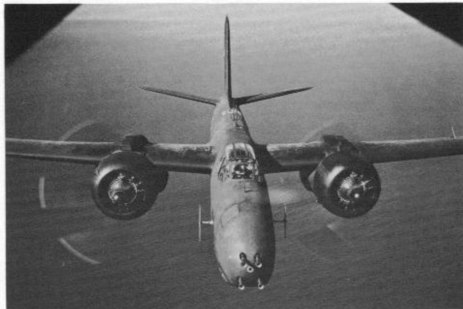
Head-on view of a P-70 over the Pacific as it approaches another P-70. The guns have flash suppressors attached so as not to blind the pilot when the guns are fired. The radar antennas are the two objects protruding from the fuselage just aft the nose. The color scheme is Olive Drab on top and Dull Black below. (USAF)
