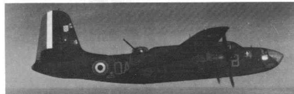
A Boston IV of No. 342 Lorraine Squadron on its way to a target in France after "D-Day". Insignia below the cockpit is the crest of the Free French forces. (Scutts)
