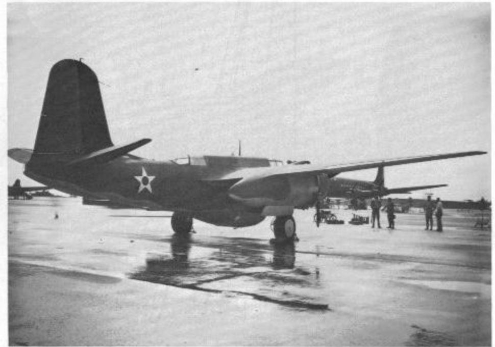
An A-20C with a long range fuel tank fitted under the fuselage. When these types of tankers were fitted, no bomb load could be carried in the bay. (USAF)
