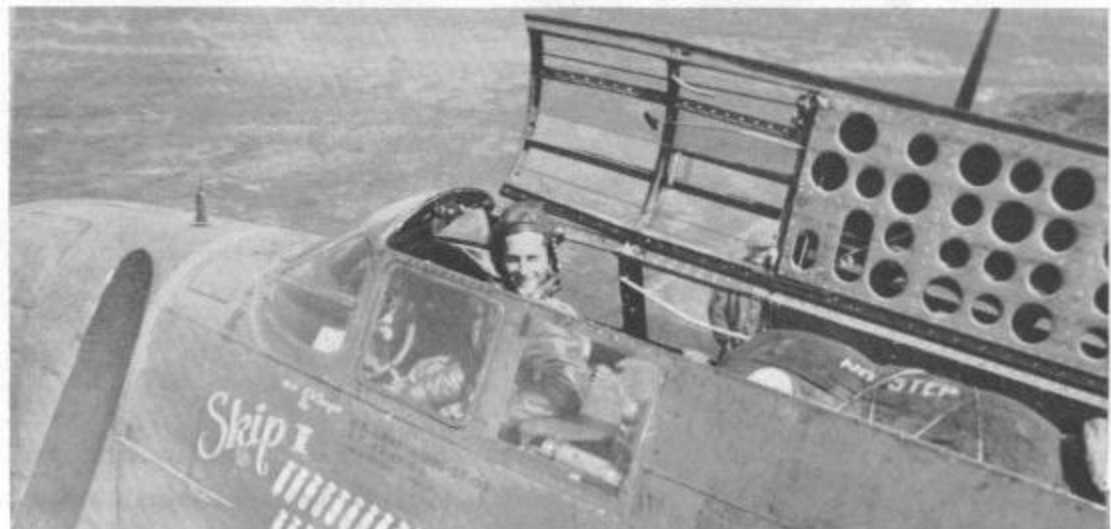
Good view of the pilot's entry hatch on an A-20G-35 from the 668th Bomb Squadron. Item behind cockpit marked with No Step is a life raft. (Morrow via 668th B.S./ Martin)
