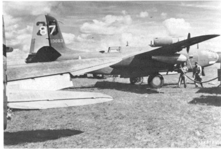
This A-20B from the 47th Bomb Group was pressed into service as a fuel carrier. It would fly to a base where all fuel except for the amount needed to return to its base was siphoned off. Using this technique aircraft could begin operating out of captured bases as soon as the runway was repaired and ground personnel flown in. (USAF)
