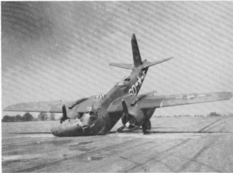
The nose wheel of this A-20G buckled upon landing which caused the nose to literally cave in. This was quite common if the gear gave way while the plane was landing. (USAF)
