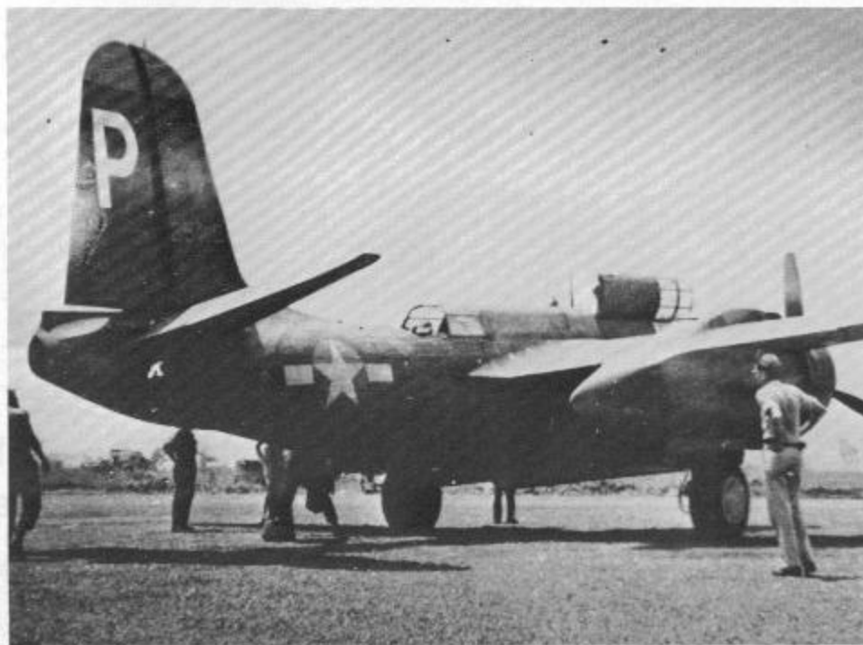
This A-20G-10 carries the tailmarkings of the 3rd Bomb Group. The -10 production block did not carry the power operated turret which was introduced on the later G series. (Swain)
