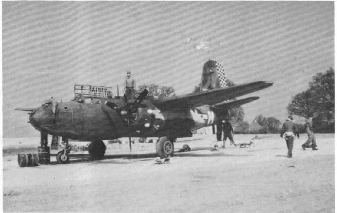
The nose wheel of this A-20G buckled upon landing which caused the nose to literally cave in. This was quite common if the gear gave way while the plane was landing. (USAF)
