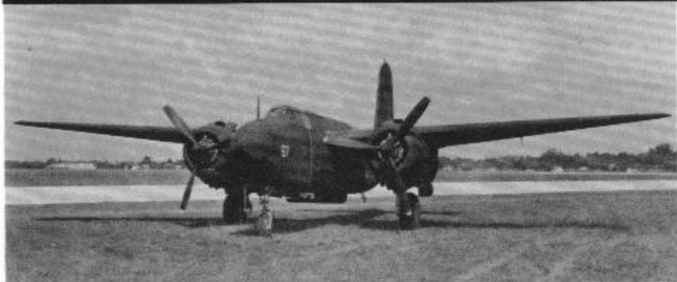
(Above) The first P-70 sits at Wright Field in a color scheme of Dull Black. The radar was mounted in the nose and the glass nose was painted Black. The object under the fuselage is a ventral pack containing four 20mm cannons. (USAF)
