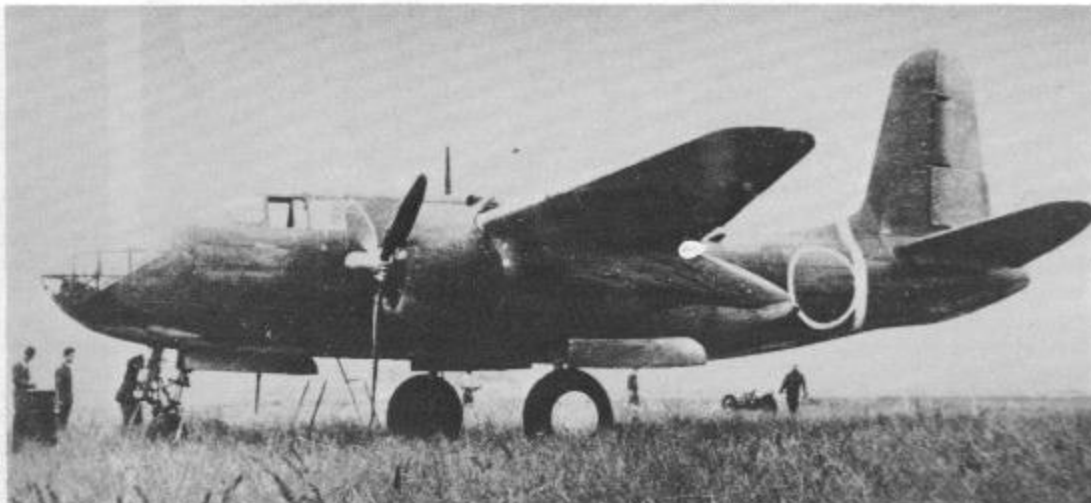
One of the few A-20s sent to the Dutch on the island of Java in the early part of 1942. It was assembled by the Japanese following their capture of the island and flown back to Japan for evaluation. (USAF)
