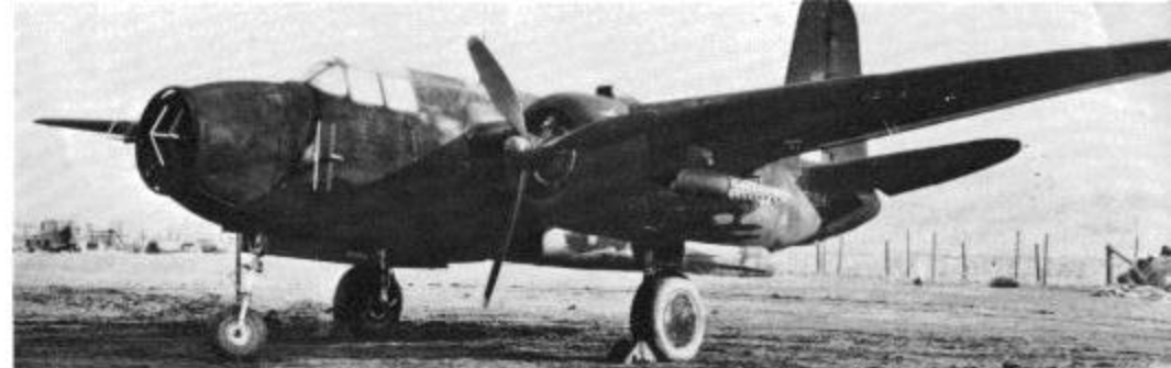
A Havoc Turbinlite from No. 532 Squadron. The unusual exhausts greatly cut down on the telltale flame from the day bomber version. This aircraft's serial number is Z2184. (Scutts)
