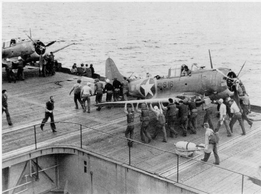
Mechanics work on the Wright R-1820-52 of this SBD-3 on the deck of the Ranger in November of 1942. The composite spinners were removed on all of VS-41's Dauntlesses, exposing the the hub and operating mechanism of the adjustable pitch prop. (USN/NARS)
