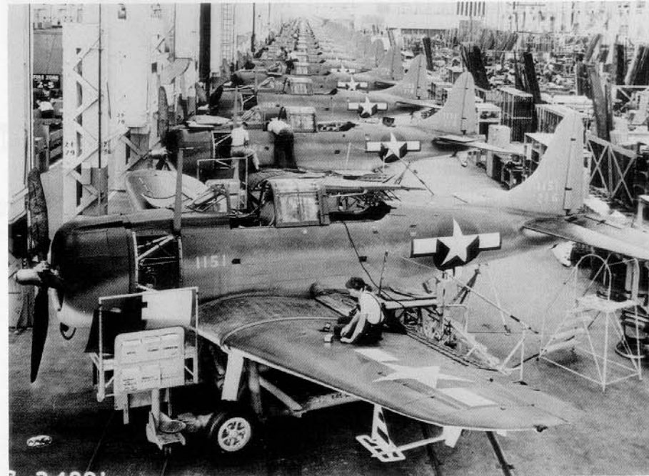
Dauntlesses almost as far as the eye can see; SBD-5s on the assembly line at El Segundo. (NASM)
