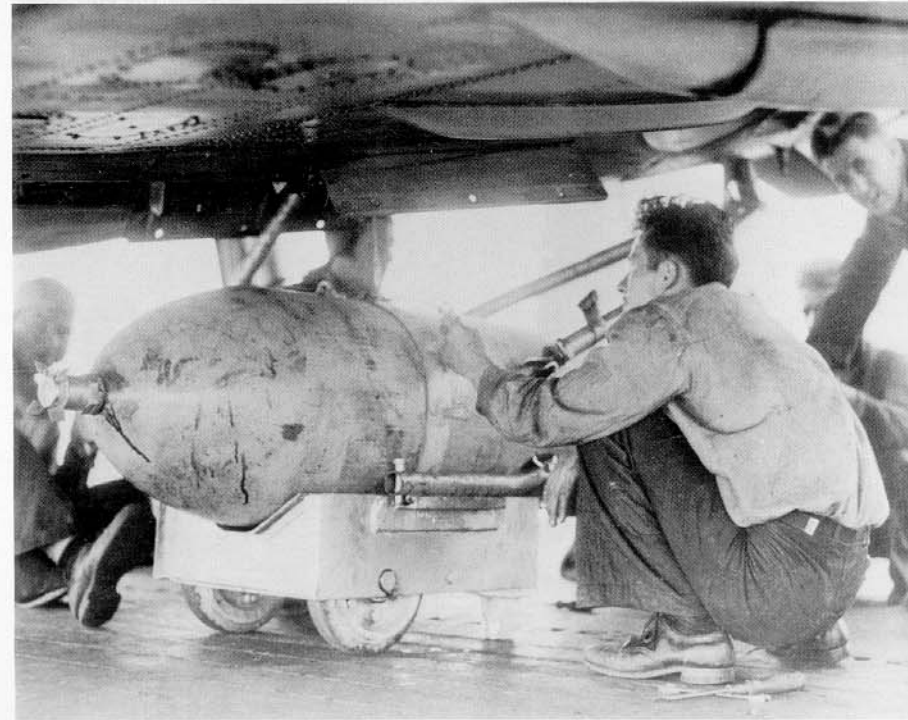
Deck crewmen on Enterprise (above) and Ranger (below) rig 1000 lb GP bombs on SBD-3s. Once the bomb is positioned, the armorers set the fuse and the bomb is hoisted with a handwinch (USN/NHC and USN/NARS)
