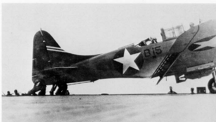
This SBD-3 of VB-6 has just trapped on board Enterprise, 15 May 1942. The painting out of the Red markings on this aircraft preceded the official order to do so, which was not ordered until 20 May. By the Battle of Midway the SBD-3 had almost completely replaced the SBD-2 on the carrier decks. (USN/NARS)
