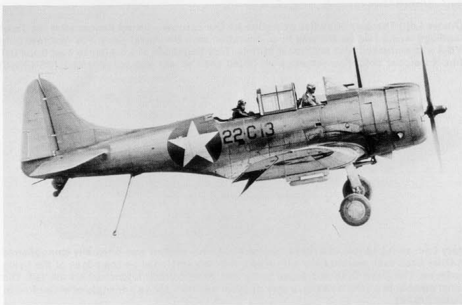
22-C-13 with its hook down, approaches the Independence. The Sea Blue has been incorrectly applied. It should be painted down the sides of the fuselage between the leading and trailing edge of the wing joining the Sea Blue of the wing. (USN/NARS)
