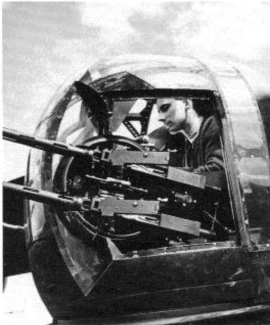
The Halifax tail turret remained much the same throughout its service life. Apart from a small number of new turrets introduced toward the end of the war, tail defense was provided by the Boulton Paul Type E turret, seen here with the gun breech covers open. (IWM)
