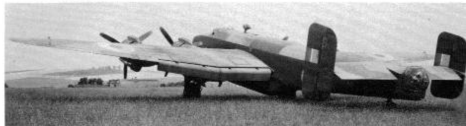
This B Mk III conversion (LV838) served as the prototype C Mk VI, and is fitted with an 8,000lb capacity freight pannier.
