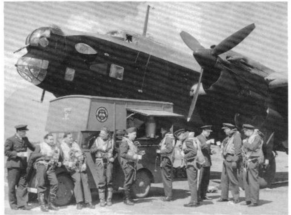
Aid from the USA to Britain in the early war years wasn't always in the form of weapons. Cash donations bought this YMCA tea car for an RCAF Halifax base. One of the six per wing cable cutters can be seen in the juncture of the engine nacelle and the leading edge of the wing. (Aeroplane)
