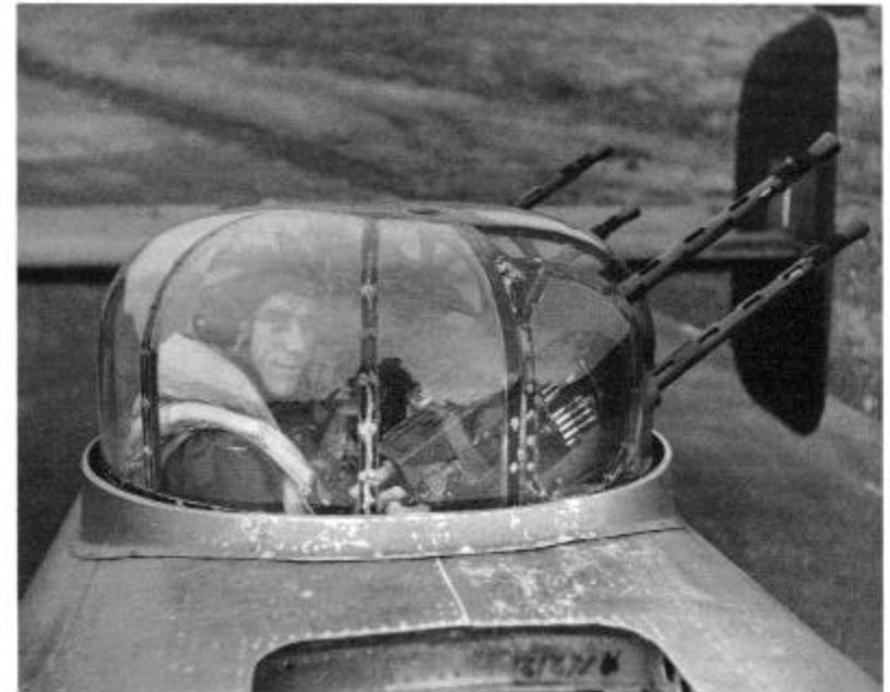
Flight Sergeant Jack 'Junior' Cumbers in the Boulton Paul Type A mid upper turret of a Halifax B III of No 424 (Tiger) Squadron RCAF. The compact turret greatly improved the Halifax's chance of survival when attacked by night fighters. (RCAF)
