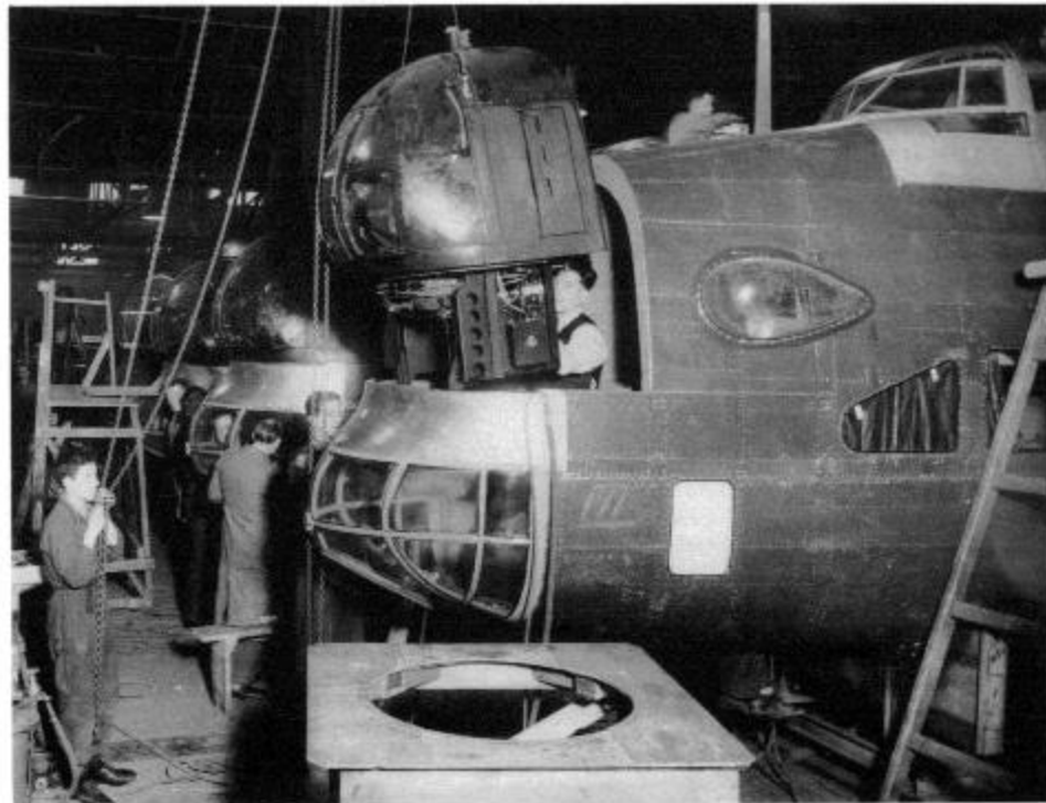
Halifax front fuselages on the production line. Apart from guns and ammunition boxes, the Boulton Paul C type nose turret went in complete.
