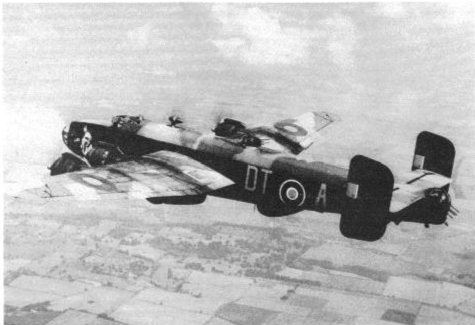
Halifax B Mk III of No 192 (Special Duties) Squadron configured for a dual bombing and electronic intelligence gathering role. Operating a variety of aircraft, No 192 only employed Halifaxes for this double task from January of 1945. Part of the ECM task was to drop 'Window' as a contribution to the Special Window Force of No 100 Group. (M. Wright)
