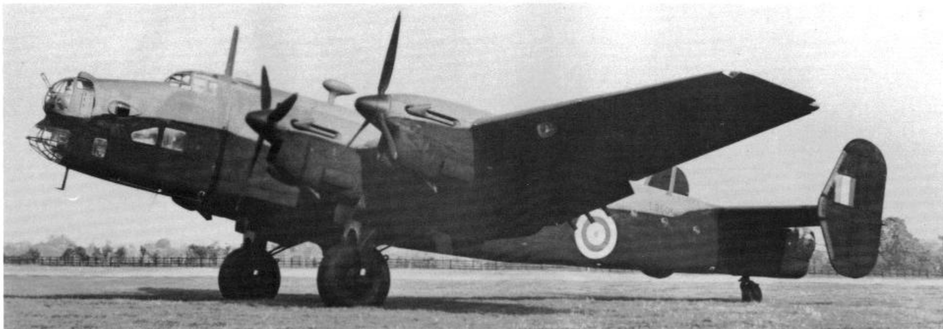
The nine B Mk I Series 3s introduced features carried over to the Mk II, including the deeper oil cooler lip on the engine nacelle undersides. The second machine of the production batch, L9601, served with No 76 and No 78 Squadrons. (Flight International)
