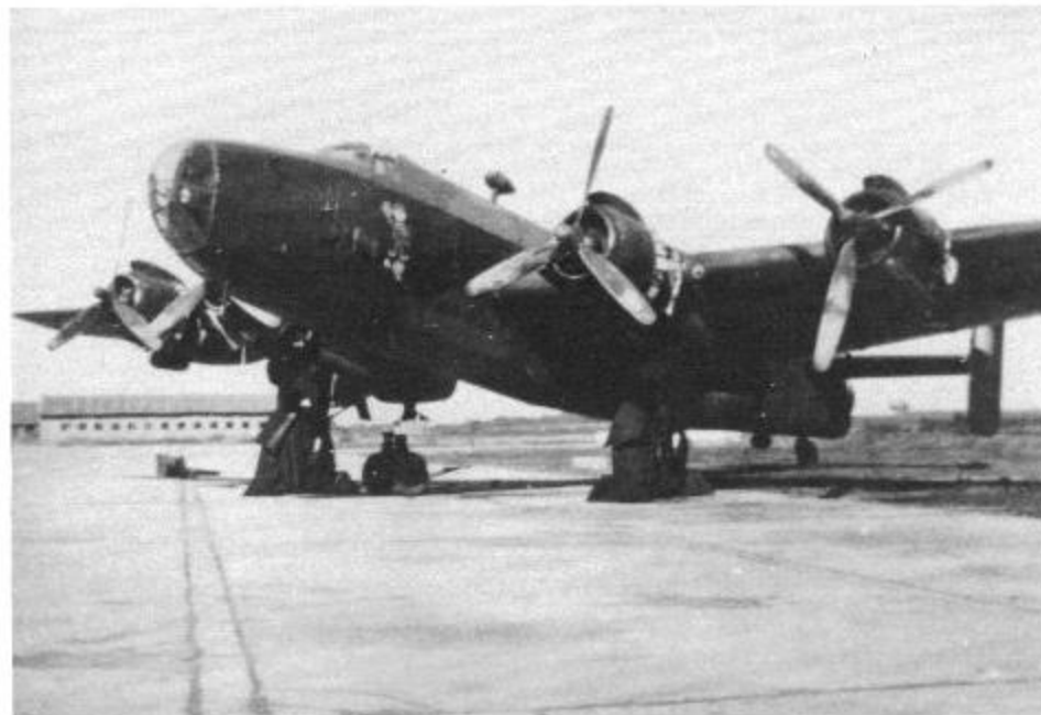
A 1341 Flight B Mk III used for ELINT sorties against Japanese radars just before the end of the war. As well as SEAC markings, these aircraft carried an extra DF loop forward of the tailwheel. (R. L. Ward)
