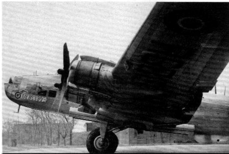
The Empire Radio School at Debden, Essex, had two B Mk VIs, 'Mercury' (RG815) being the second delivered, in July of 1946. Configured as a 'flying classroom', this aircraft had a special navigation radar fit and a modified nose. It made a number of long range flights before being struck off charge in October of 1948. (Aeroplane)
