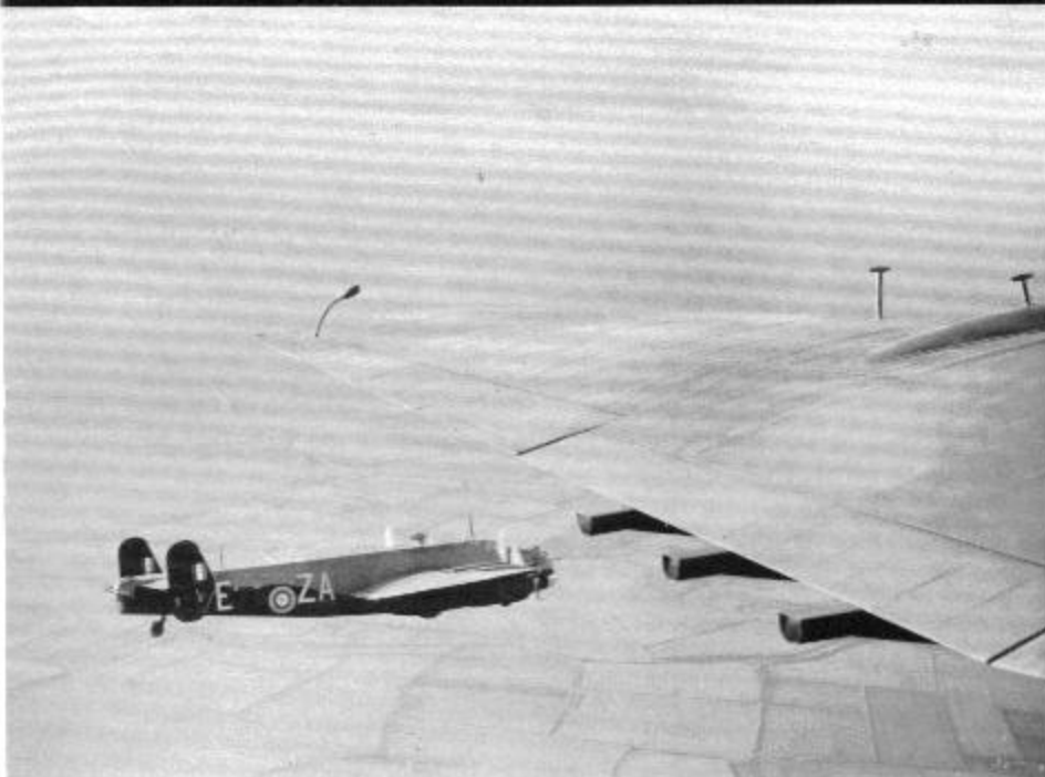
(Above) No. 10 Squadron Halifax IIs in flight. The sister aircraft of BB194 shows to advantage the aileron mass balance, the fuel jettison pipes on the bottom of the flap, and the breather/filler pipes for the outboard wing tanks. There were six breather/filler pipes on the early marks of Halifax. BB194 is an early Mk II without the bulbous Boulton Paul C mid upper turret. (IWM)
