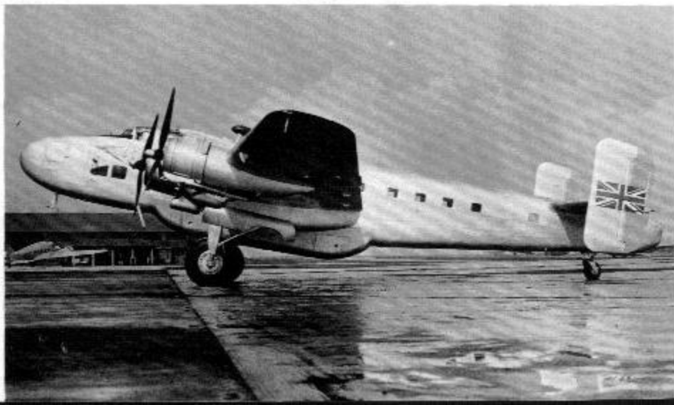
One of BOAC's Haltons at Short Brothers' Belfast works in Northern Ireland. Clearly visible are the larger fuselage windows and the port side baggage loading hatch in the nose. (Shorts)
