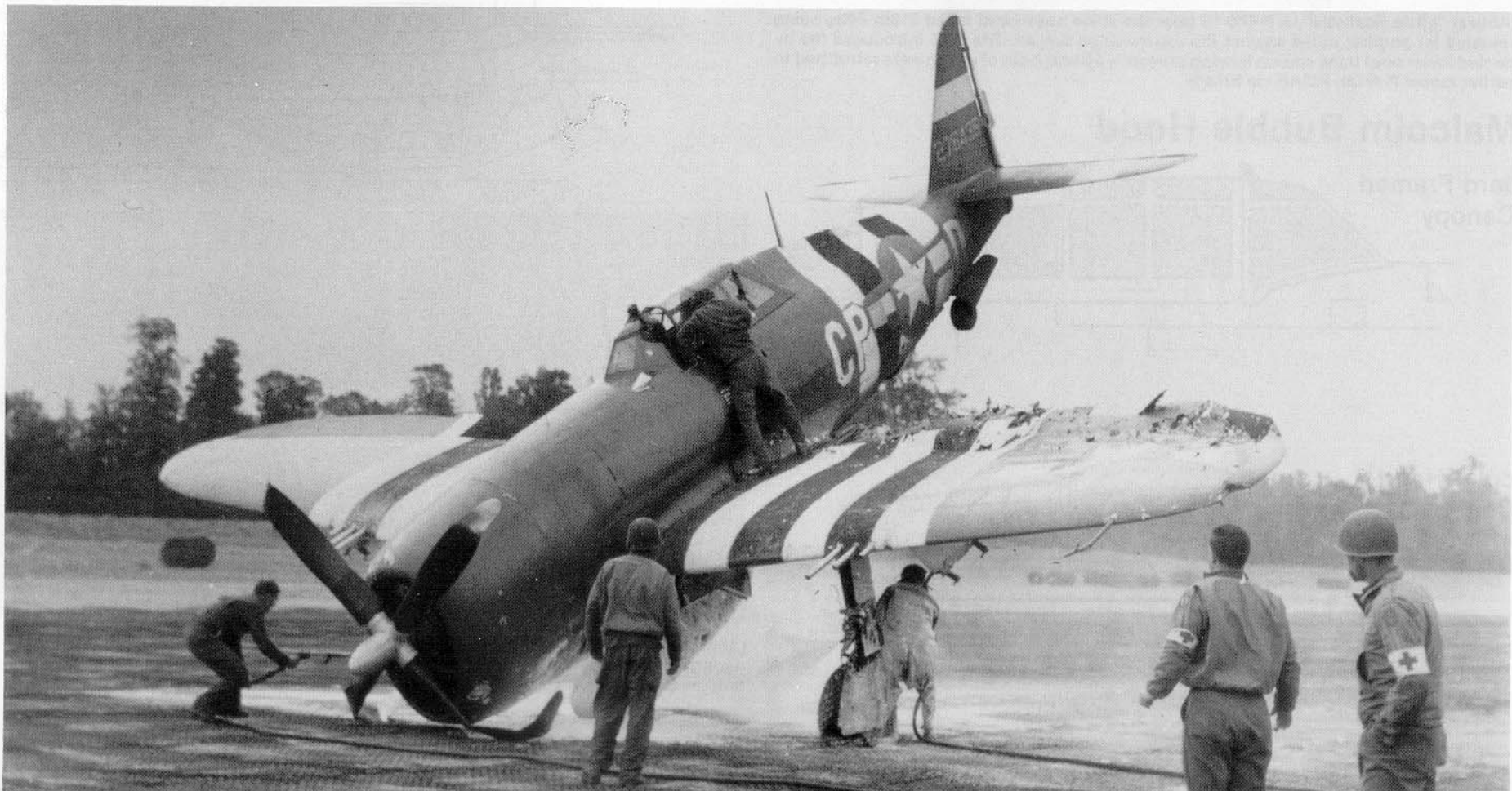
(Below) The pilot of this 367th FSq, 358th FGp P-47D-20 brought the aircraft home with extensive damage to the port wing during one of the many D-Day strikes carried out by Thunderbolt crews. The full D-Day striping is well illustrated. (Olmsted)
