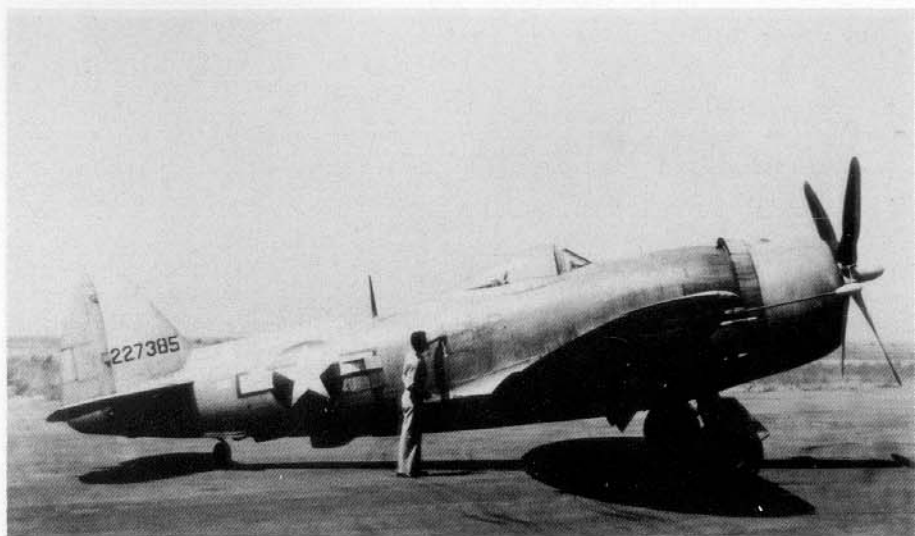
(Above) The YP-47M was basically a D-30 airframe fitted with the R-2800 C rated at 2800 horsepower with water injection. The YP-47M was the fastest production Thunderbolt with a 473 mph top speed. (AFM)
