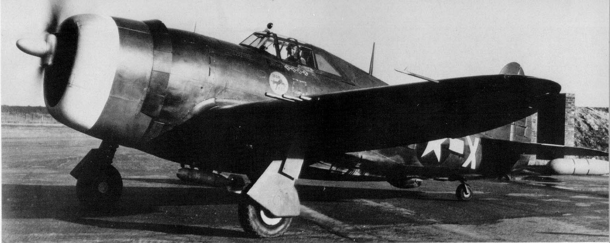
(Above) "Iron Ass", another P-47D-5 from the 56th FGp, is armed with a 250lb bomb on the centerline station and no underwing fuel tanks. Thus armed, the aircraft is probably taxiing out for a practice bombing mission since Thunderbolt pilots rarely ventured over the Continent without wing tanks. (AFM)
