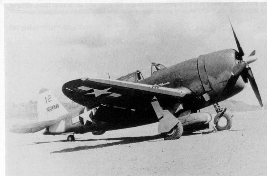
(Above) A P-47D-2 from the 348th FGp on New Guinea. Note the white leading edges on the wing, an attempt to help pilots quickly identify friendly P-47s from the Mitsubishi Zero. Note the flat 200 gallon belly tank. (AFM)
