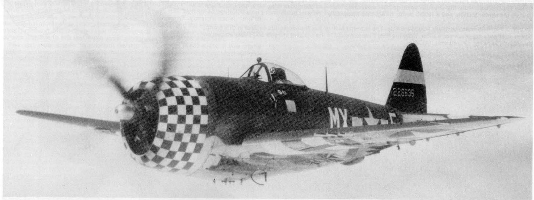
(Below) A P-47D-25 from the 82nd FSq, 78th FGp returning to Duxford after a bomber escort mission during the summer of 1944. The 78th FGp camouflaged some of their aircraft with Medium Green (34092) upper surfaces over Sky (34424) undersides. (AFM)
