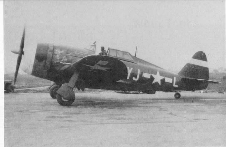
(Above) "Chief Wahoo", a P-47D-1 from the 351st FSq/353rd FGp, exhibits many mission and kill marks. Since the P-47 had a similar profile to the German Focke Wulfe FW 190A, Eighth Fighter Command had white bands applied to the nose and tail to help pilots quickly identify a friendly aircraft during a fight. (AFM)
