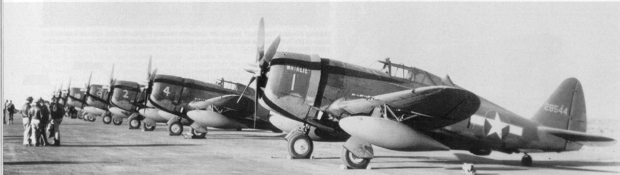
(Below) A ramp full of P-47D-5s at the Republic plant awaiting ferry pilots for the long trans-Atlantic flight to combat units in England. Note the 150 gallon long range underwing fuel tanks that were adapted from Lockheed P-38 tanks. (USAF via Ethell)
