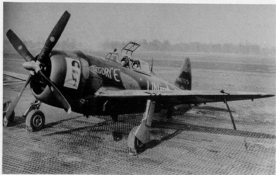
(Below) Although only two P-47G-15s were factory-built as two-seated aircraft, many 'DoubleBolts' were built by combat units in the field. "Category E" had a second cockpit added behind the first on a War Weary P-47D-11. "Category E" was assigned to the 63rd FSq, 56th FGp. (AFM)
