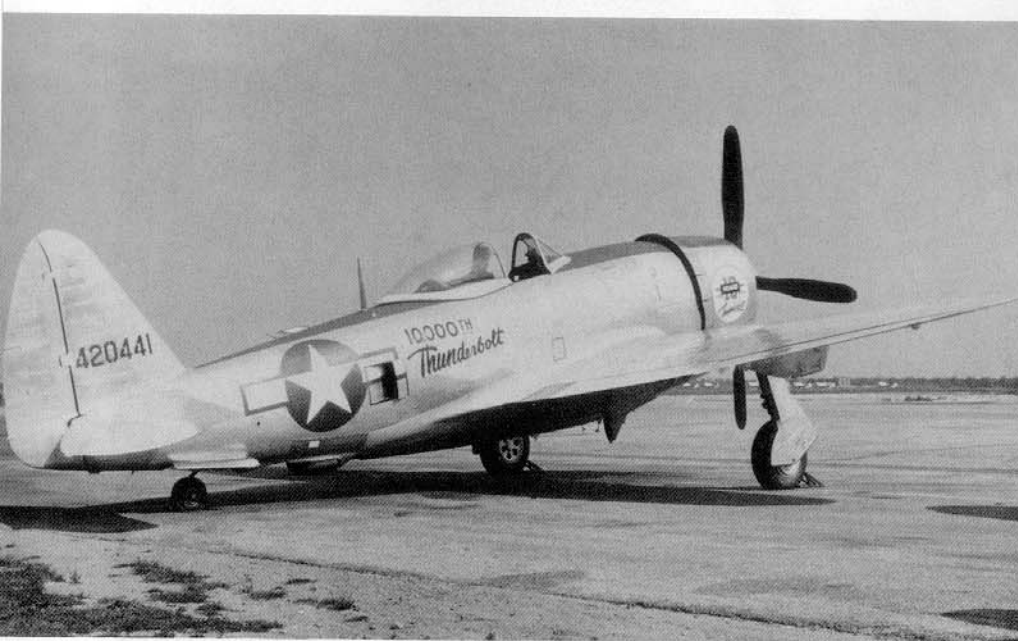
(Above) The 10,000th Thunderbolt built was a D-30 from Republic-Farmingdale. The D-30 was the first Thunderbolt to have the underwing dive flaps and permanent underwing pylons. (AFM)
