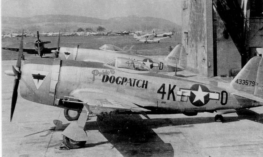
(Above) The "Pride 'O Dogpatch" is a D-30 from the 506th FSq/404th FGp at Fritzlar Air-drome, Germany. The D-30 also introduced a rear vision mirror inside the canopy, as well as electrically operated external stores releases. (Ethell)
