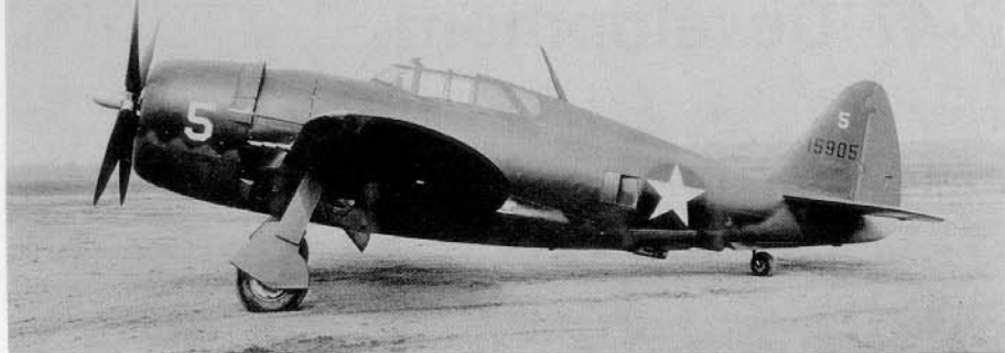
(Above) The No 5 production P-47B with a combination canopy area -- XP-47B razorback area with side windows, but also having a sliding canopy from the P-47B. The forward rake of the radio antenna mast was another characteristic of production P-47Bs. (AFM)
