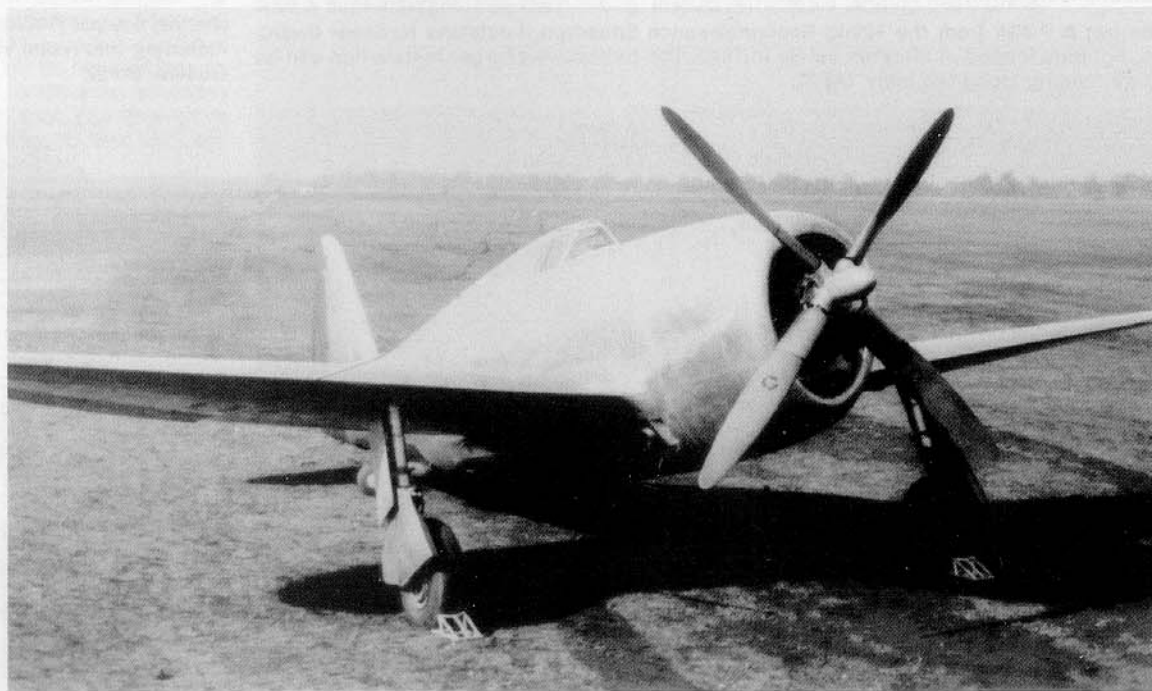
(Above) The XP-47B at Farmingdale. Note the car door style canopy entrance, which was done away with on production model P-47Bs. (AFM)
