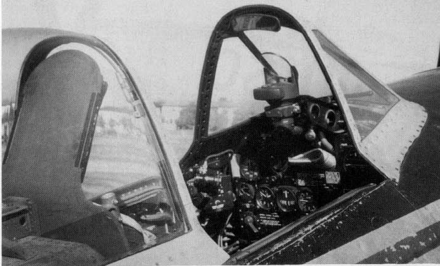
(Above) The F-47D cockpit. The cockpit colors were Interior Green floor and console walls, with Black consoles, instrument panel, and upper side walls. (Olmsted)
