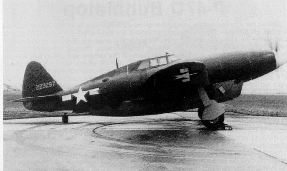
(Above) The XP-47H was a modification of a standard P-47D-15 airframe to accept a 2500 hp, liquid-cooled Chrysler XI-2220 sixteen cylinder, inverted-Vee engine. Despite the added streamlining and horsepower, the XP-47H could only achieve 414 mph and did not fly until July, 1945. (AFM)
