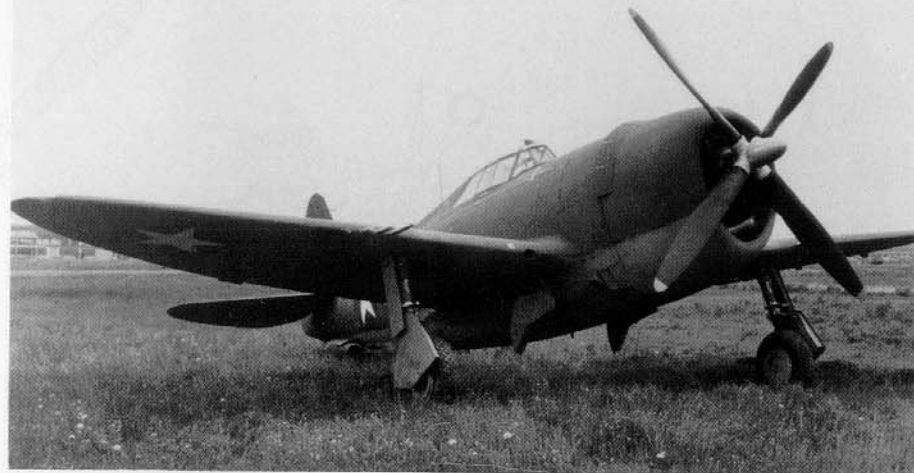
(Above) The P-47G series were various razorback Thunderbolts that were manufactured by the Curtiss Aircraft Corporation. Two P-47G-15s were factory-built as two-seat Thunderbolt trainers, the only "factory-built" two-seated Thunderbolts. (AFM)
