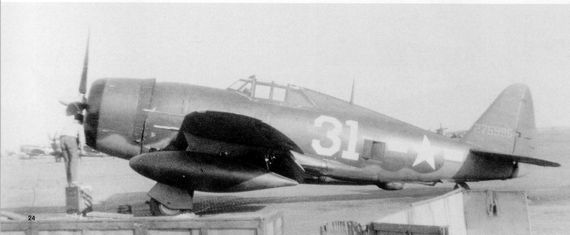
(Below) A brand new P-47D-16 on the ramp at Solimon, Tunisia, in 1943. P-47s arrived by ship without props, wingtips, or accessories. The aircraft were assembled at Solimon and flown to their combat units, in this case the 325th FGp at Foggia. (Brown via Ethell)
