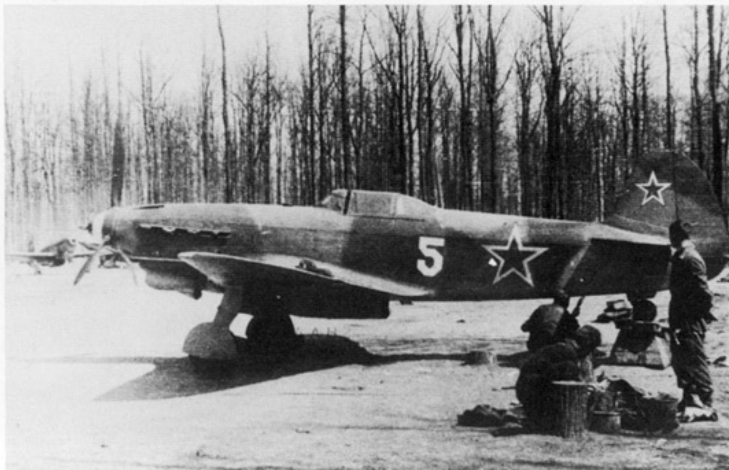
(Below) White 5, a Yak 9T-37 equipped with the efficient NS-37mm cannon. The weapon was capable of penetrating armor up to 48mm thickness. The standard tailwheel doors are carried. (SHAA)
