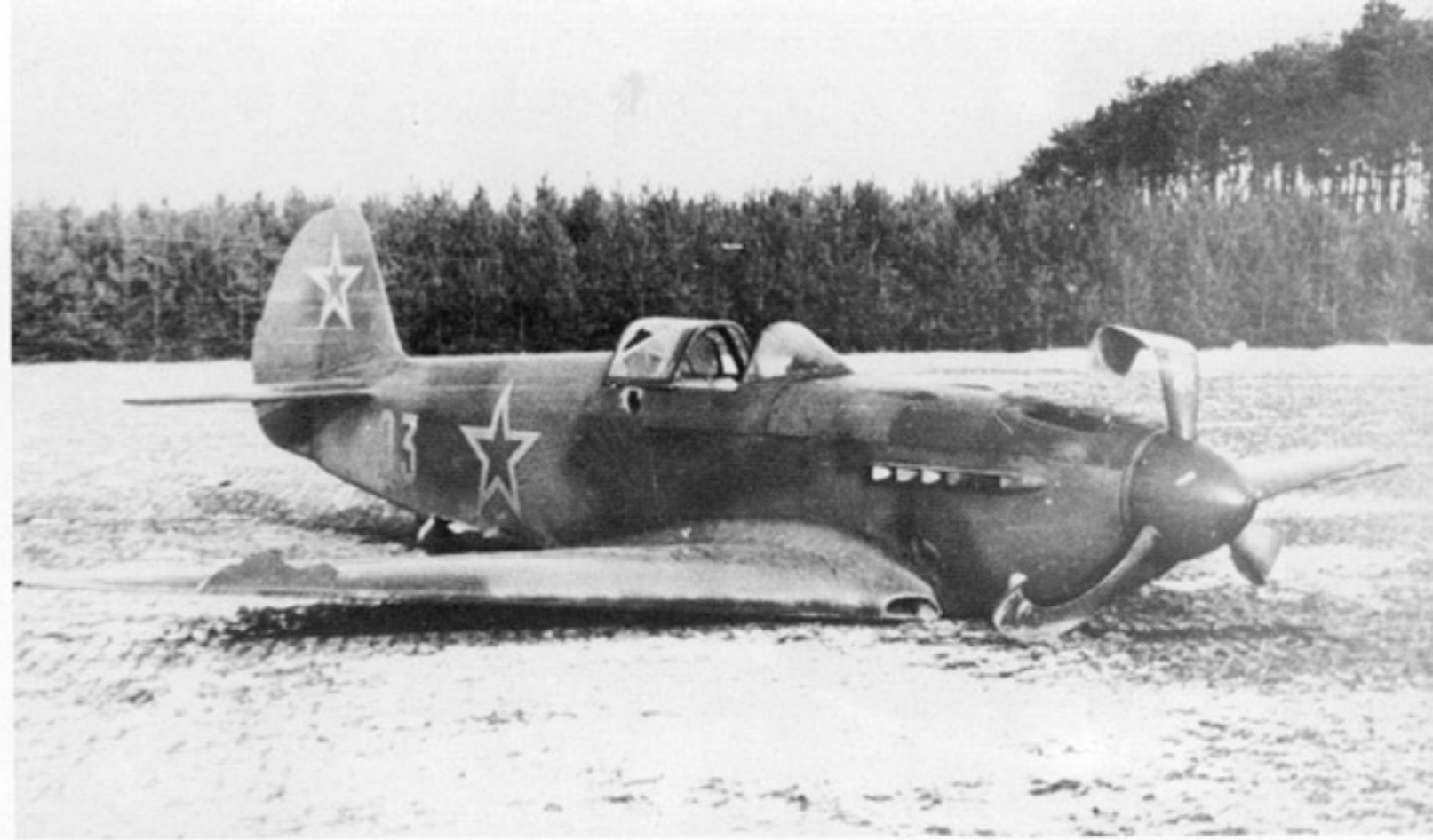
(Above Right) German Flak (Abbreviation of Fliegerabwehrkanone - anti-aircraft gun) brought this Yak 3 down near Warsaw in January of 1945, with the pilot managing to escape to friendly lines. A large hole has been shot in the sliding plexiglass canopy. The bent propeller blades indicates that the engine was running when the plane bellied in. The tactical Marking '03' and the outline on the fuselage star is in Yellow, while the rudder star is outlined in White, and spinner is Red. (Andrzej Morgala)
