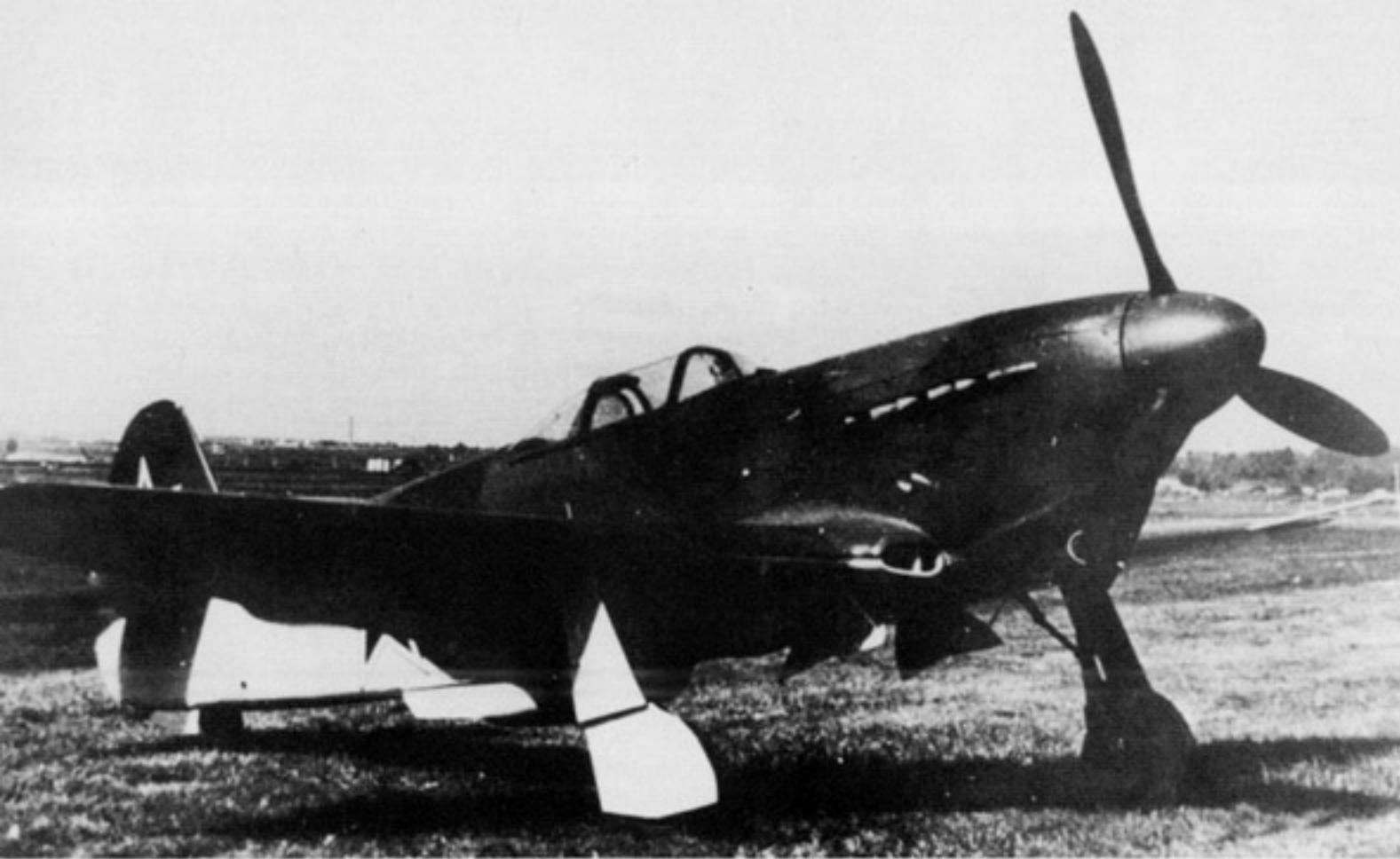
(Above Left) The very early Yak 3 variant carried the original Yak 1M armament of an engine mounted 20mm cannon and a single Berezin UB 12.7mm machine gun on the port side. The frameless windscreen along with the all-around vision rear canopy provided the Yak 3 with unparalleled visibility for the pilot. (Jan Horn)
