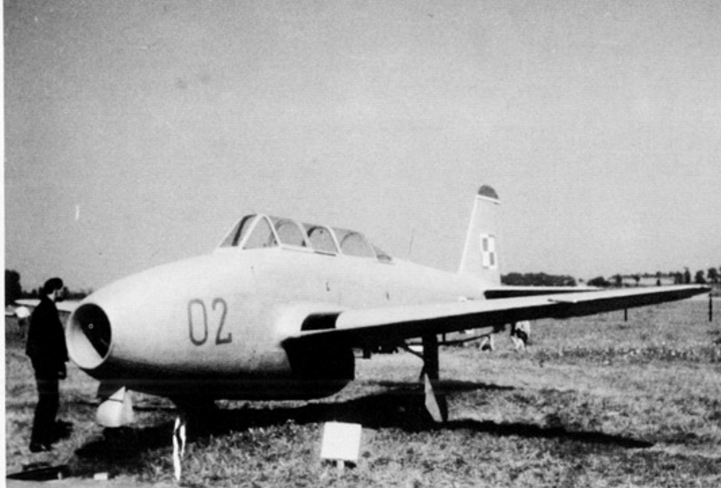
(Above) Red 02, a Polish Yak 17V Trainer during the summer of 1964. The two-seat trainer became the World's first jet trainer equipped with a full set of dual controls. It flew for the first time in May of 1947. The trainer variant of the Yak 17V usually did not carry armament. (Andrzej Morgala)
