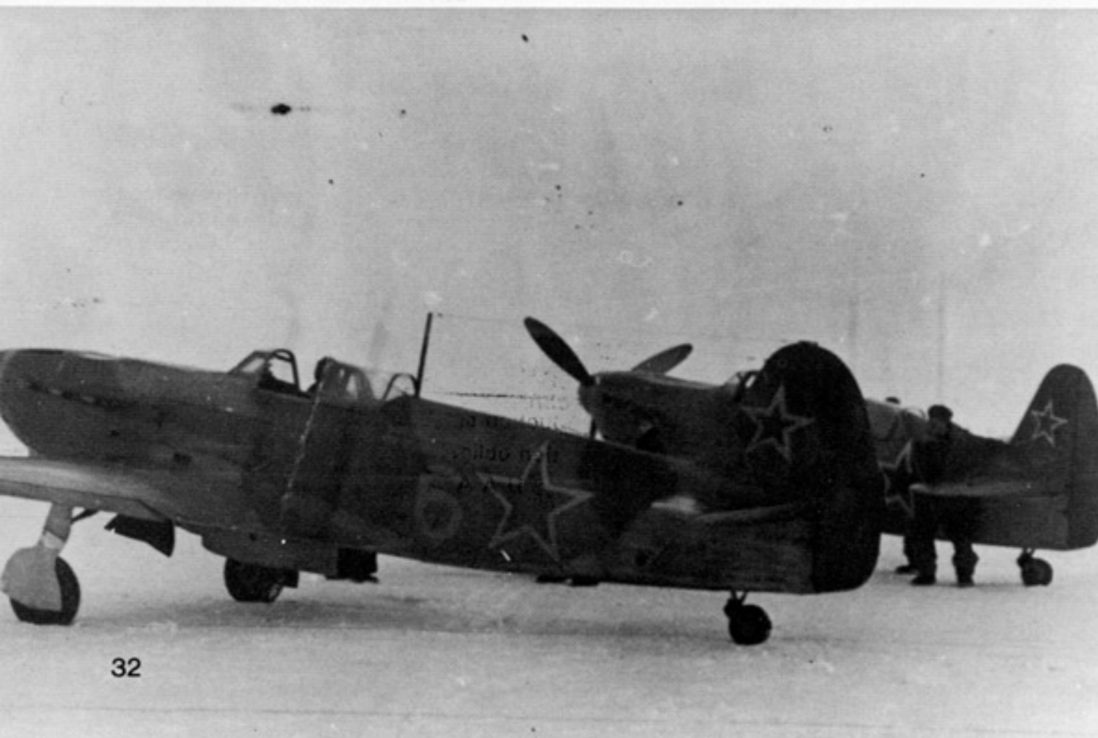
(Below Left) Warm up of a Yak 9 at Toula Airfield in late 1943. During the cold snowy Russian winter, ground crews often removed the tailwheel doors. The Aircraft in the background is a two seat Yak 7V trainer. (SHAA)
