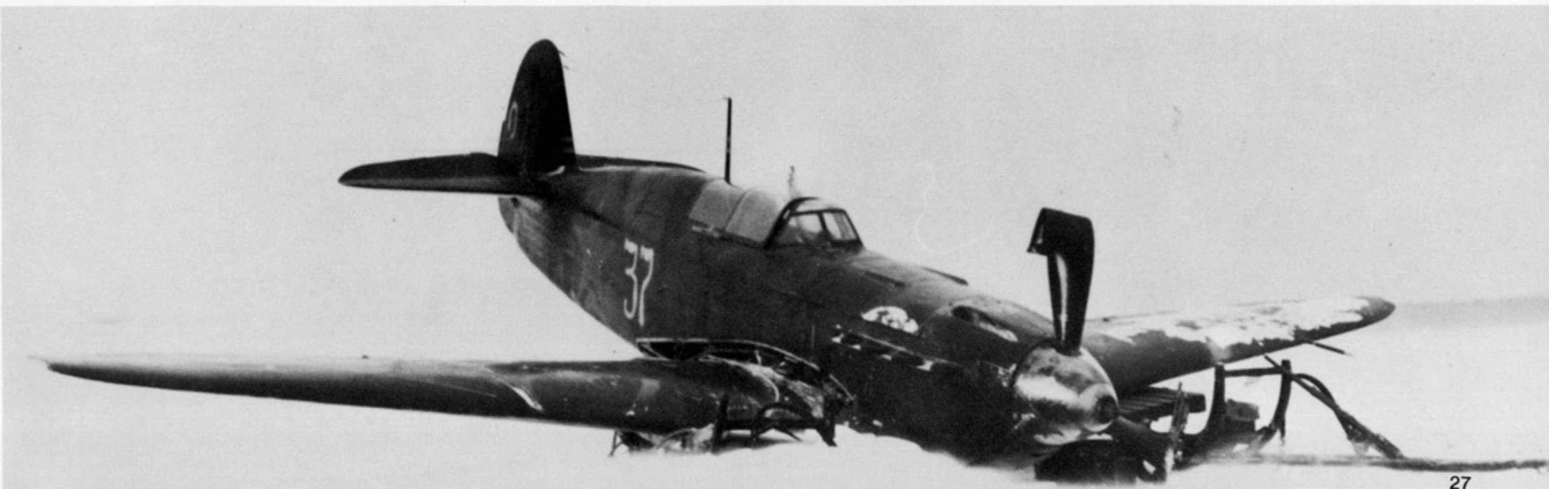
(Below) Lt. Martshenko ran out of fuel and bellied in this Yak 7B, serial number 34-37 at Ice Lake of Onega in Finland on 8 February 1943. This late production Yak 7B had Yak 9 styled exhaust stubs and trim tab on rudder. The landing light was eliminated on late production batch Yak 7Bs during the Autumn of 1942. (Hanan Valtonen)
