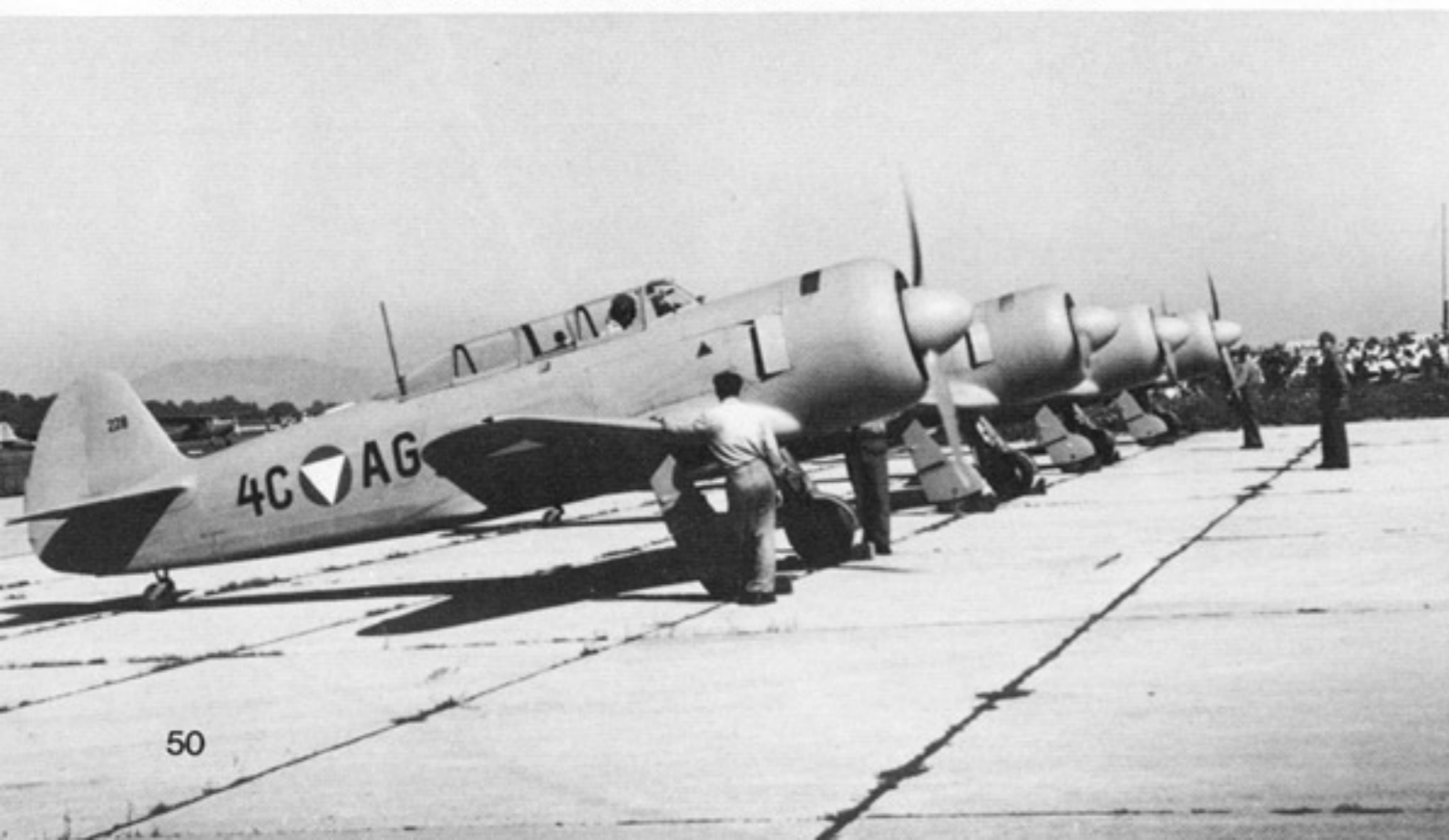
(Below) A line up of all four Austrian Yak 11s at Langenlebarn-Tulln Airfield during 1955, shortly after the trainers were passed to the Austrian Air Force. The airplanes arrived in crates as a present from the Soviet Union and were re-assembled with neither help nor technical information from the manufacturer. One aircraft, 4C-AF is now on exhibit at the Heeresgeschichtliches Museum in Vienna. (Heeresgeschichtliches Museum Wien)
