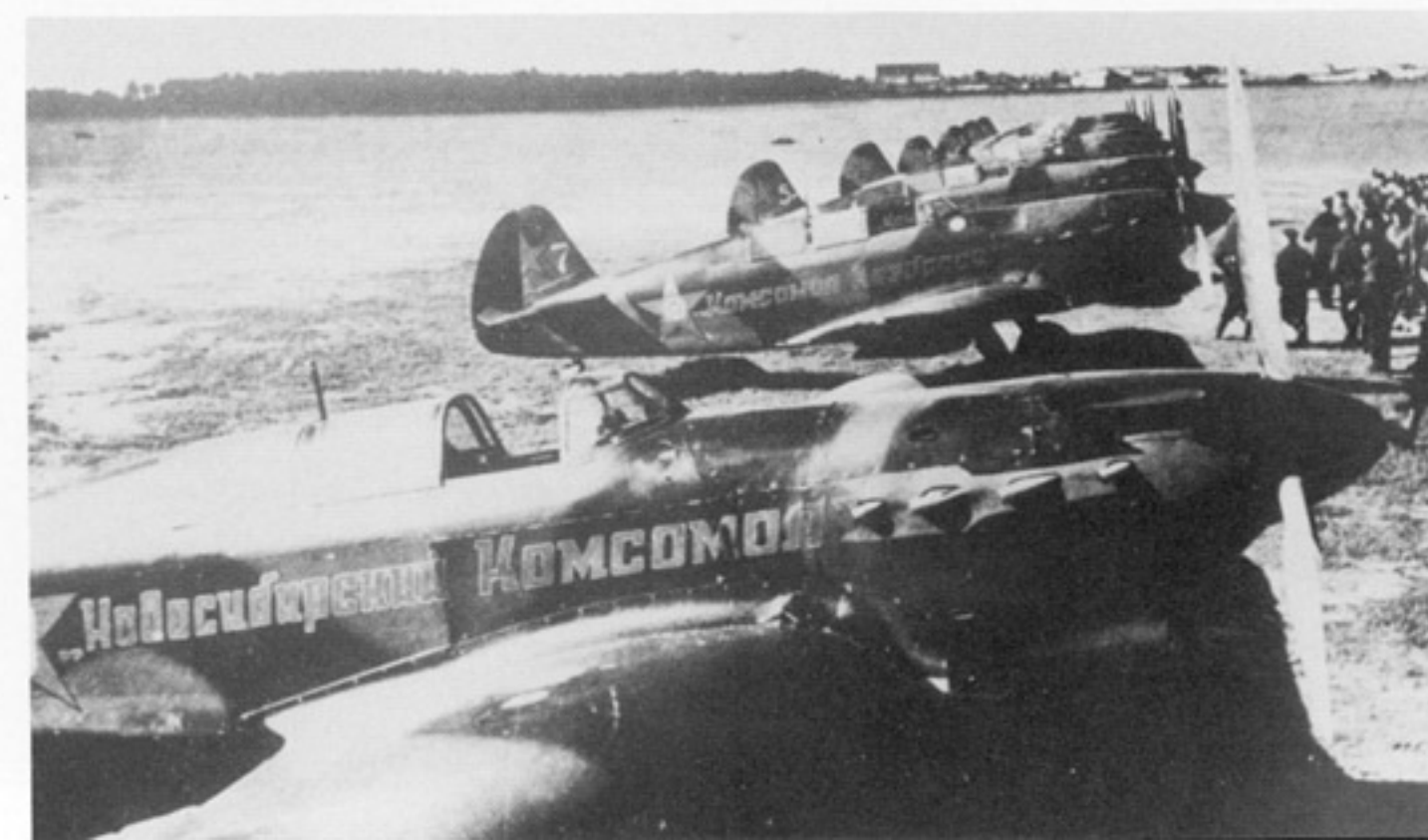
(Below) A Line up of early Yak 7Bs donated by the Communist Youth International Organization Komsomol during early 1942. The Komsomol insignia has been applied to the center of the fuselage star on each of the aircraft. Early Yak 7Bs lacked the gun cocking mechanism fairing and tailwheel doors. This version also had non-standard wing root carburetor intakes and a small aerial mast. The inscription on the first aircraft reads Novosibirsk Komsomol and on White 7 the inscription reads Kuzbas Komsomol . White 7 also carries a replacement rudder. The Novosibirsk Komsomol aircraft carries a Red arrow on the nose surrounding the exhaust stacks. (Don Henry)
