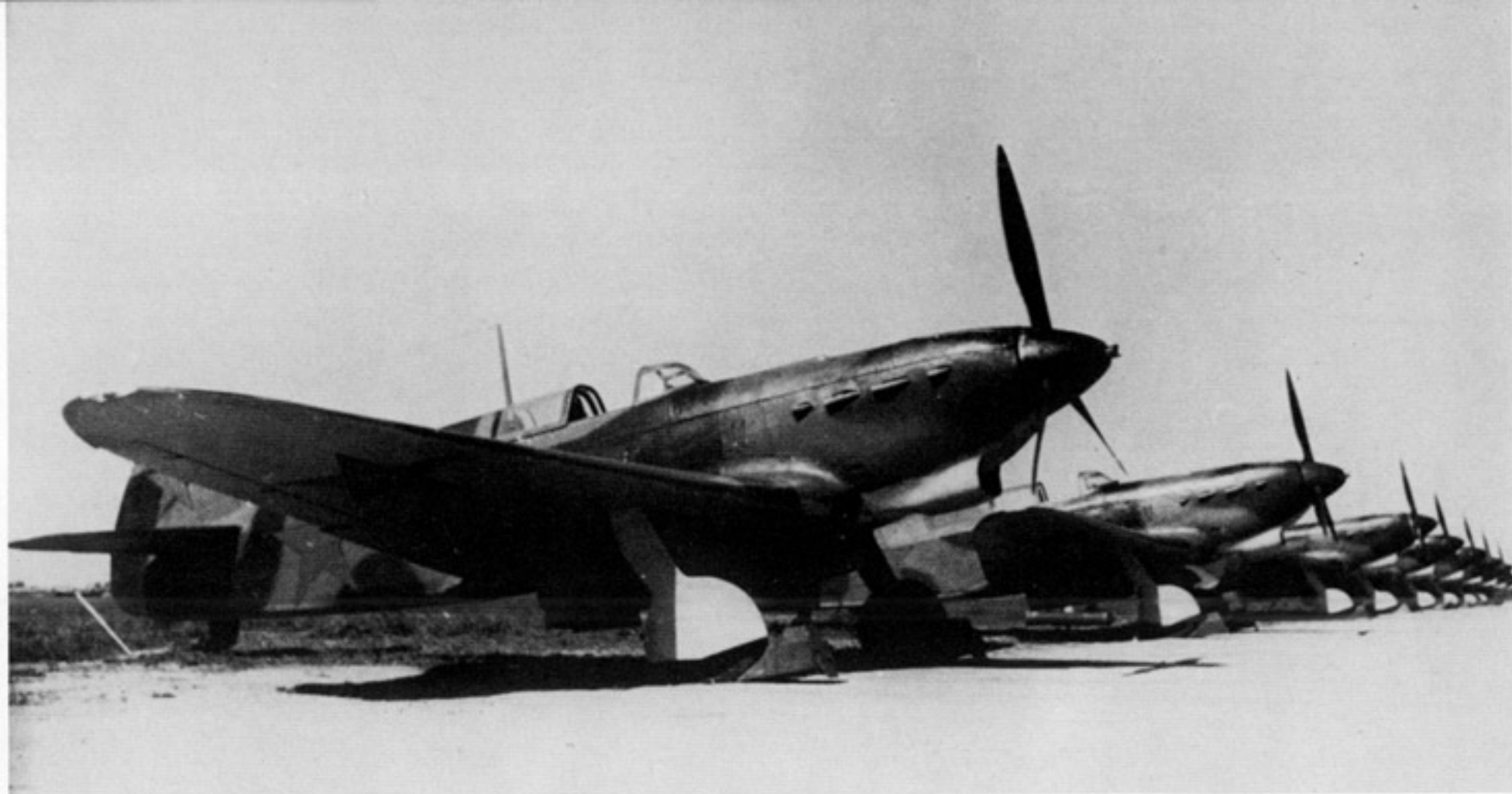
(Above) Originally intended as the two seat trainer version of the Yak 1, the war situation quickly turned the Yak 7 variant into a fighter which had both better endurance and firepower than the Yak 1 fighter. The Yak 7 became the 'heavy' fighter, a multi-purpose plane within the Soviet Air Force. (Tomasz Kowalski)
