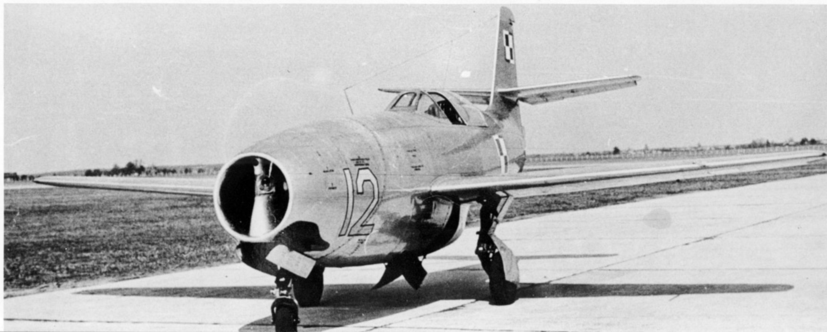
(Below) A Polish Yak 23 without the usual wingtip drop tanks on. Yellow 12 is in the natural aluminum finish. A landing light is mounted in the nose. The sturdy undercarriage allowed take-offs and landings from grass landing fields. (Andrzej Morgala)
