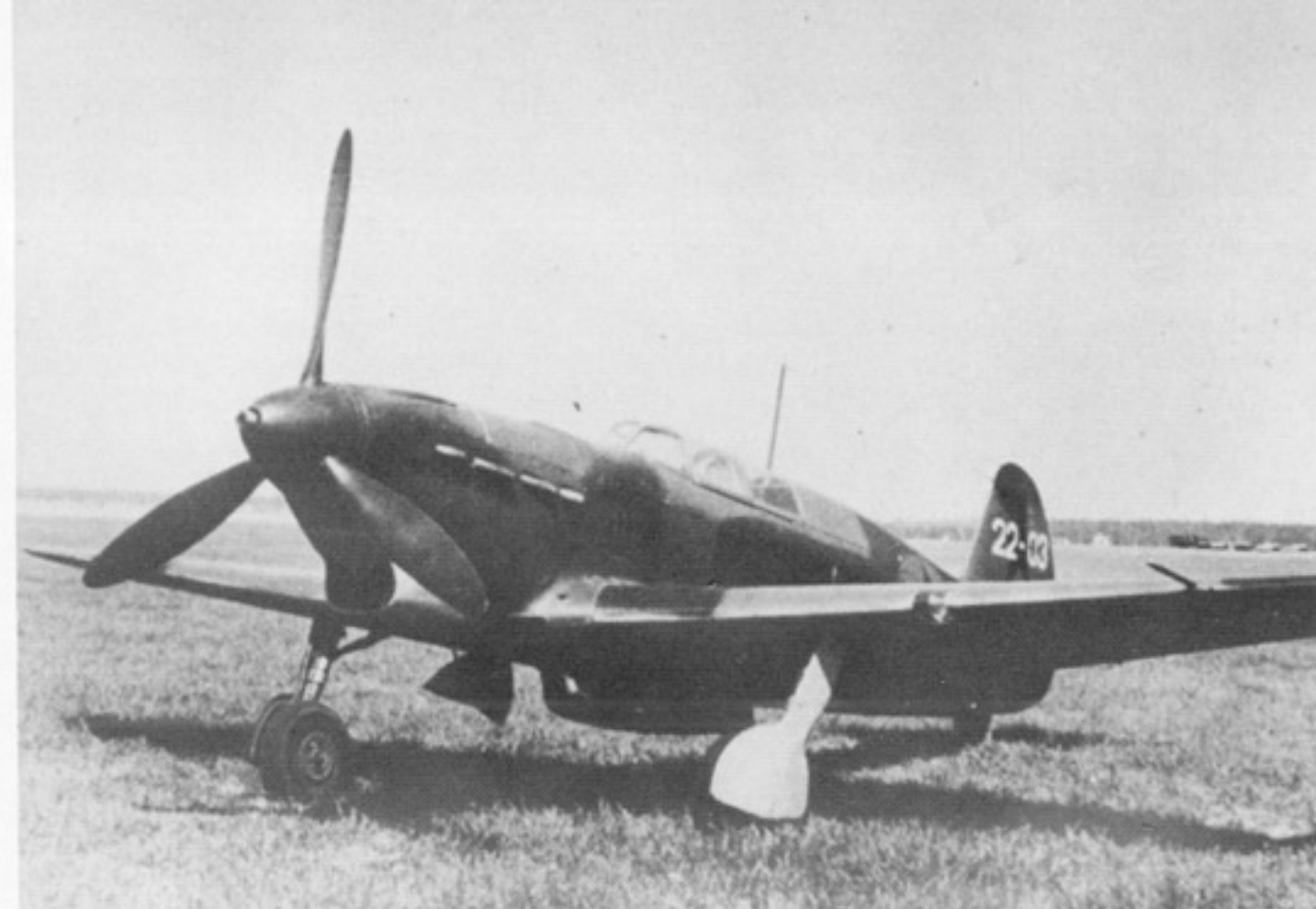
(Above) This standard Yak 7B, serial number 22-03 was completed at Zavod 153 at Novosibirsk during the summer of 1942. The serial number painted in White on the tail indicates the third aircraft built in Batch Number twenty-two. The number of aircraft built varied from batch to batch. Only State Aircraft Factory 153 used this system of serial numbers, all other plants applied the serial number in very small letters on the tail. The large Zavod 153 serial numbers were usually overpainted as soon as the fighter reached a front line unit. (Robert J. Ruffle)
