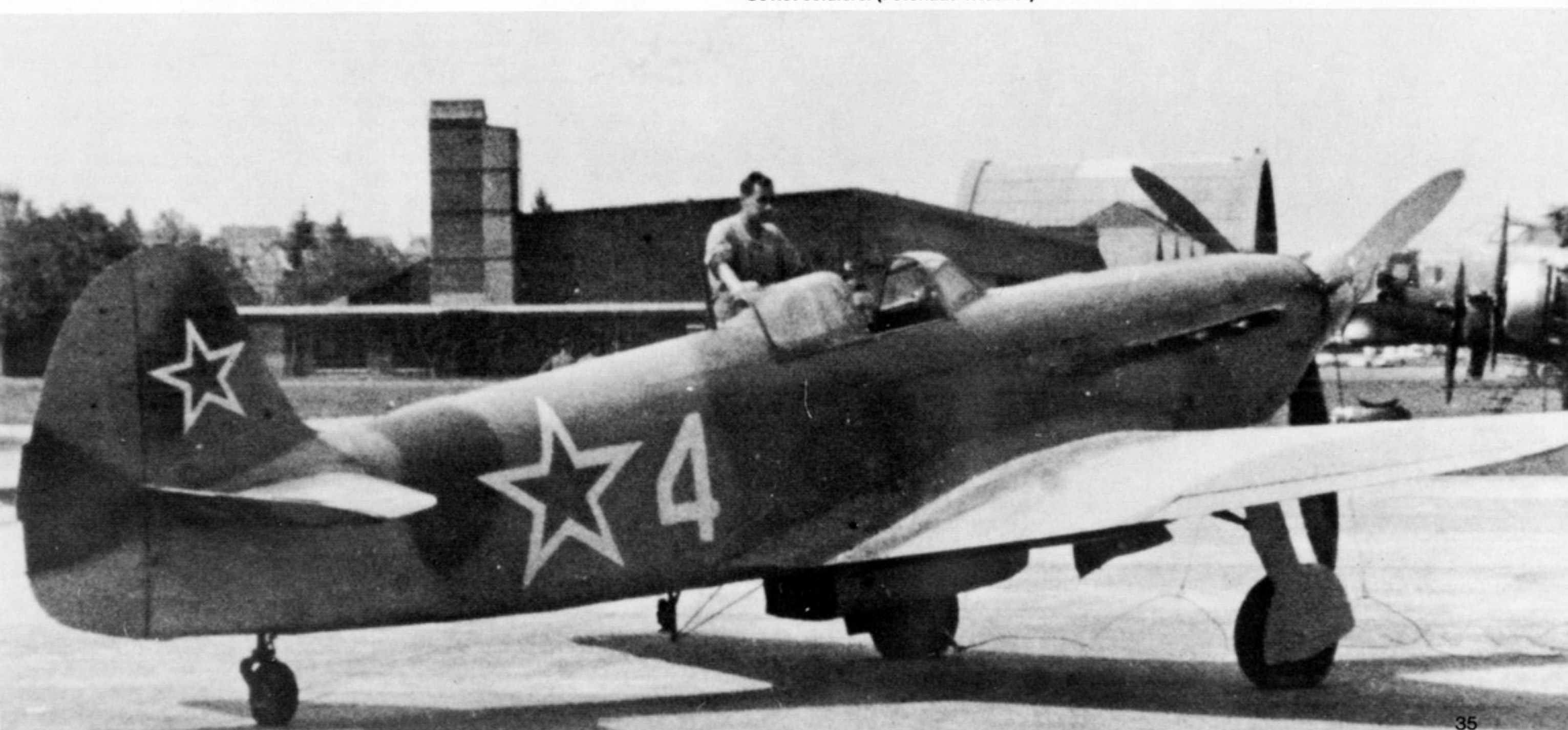
(Below) Lt. Kotchetov's Yak 9 at Dübendorf Airfield with a Swiss Mechanic, who turned the propeller every two days to avoid corrosion of engine parts. The aircraft in the background is a Boeing B-17G-55-B0 (42-102651) belonging to the 447th Bomb Group. Lt. Herbert Altman landed PICADILLY ANN II in neutral Switzerland on the plane's tenth mission. Seventy-six Flying Fortresses and eighty-two Liberators were interned in Switzerland, along with 10,000 Soviet soldiers. (Fotohaus Wiesner)
