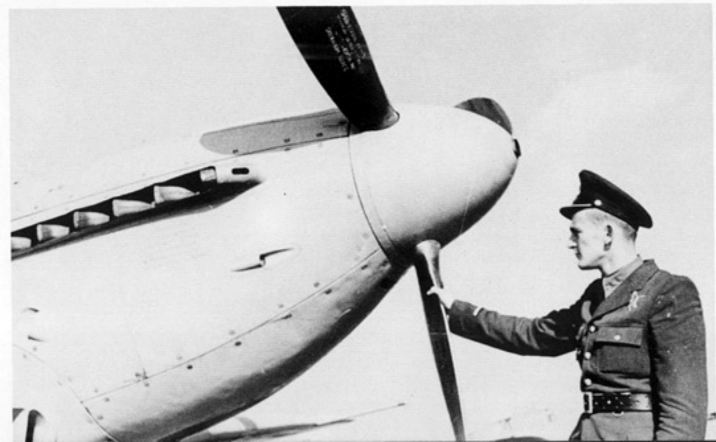
(Below Left) An overall Light Gray Yak 9P in Polish service. A Russian inscription in white can be seen on the propeller blade. All Yak 9Ps were powered by a 1,600 hp Klimov M-107 A engine and carried an armament of a single ShVAK 20mm cannon with 100 rounds, and two 12.7mm machine guns each with 250 rounds. Some examples of the Yak 9P were also armed with a 23mm cannon. (Andrzej Ec)
