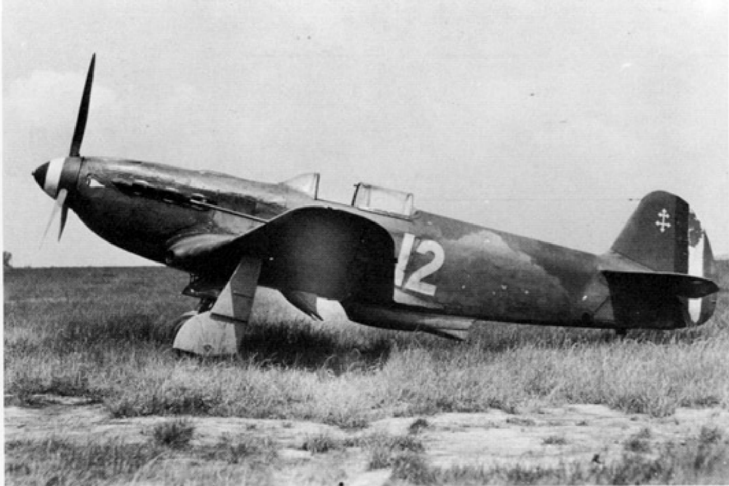
(Above Left) The performance of the robust Yak 3 presented a real problem for the Luftwaffe . This nimble fighter was superior to its German opponents and Soviet pilots loved its low altitude handling qualities. The removal of the oil cooler intake from the nose provided quite a different silhouette from previous Yak variants. (SHAA)
