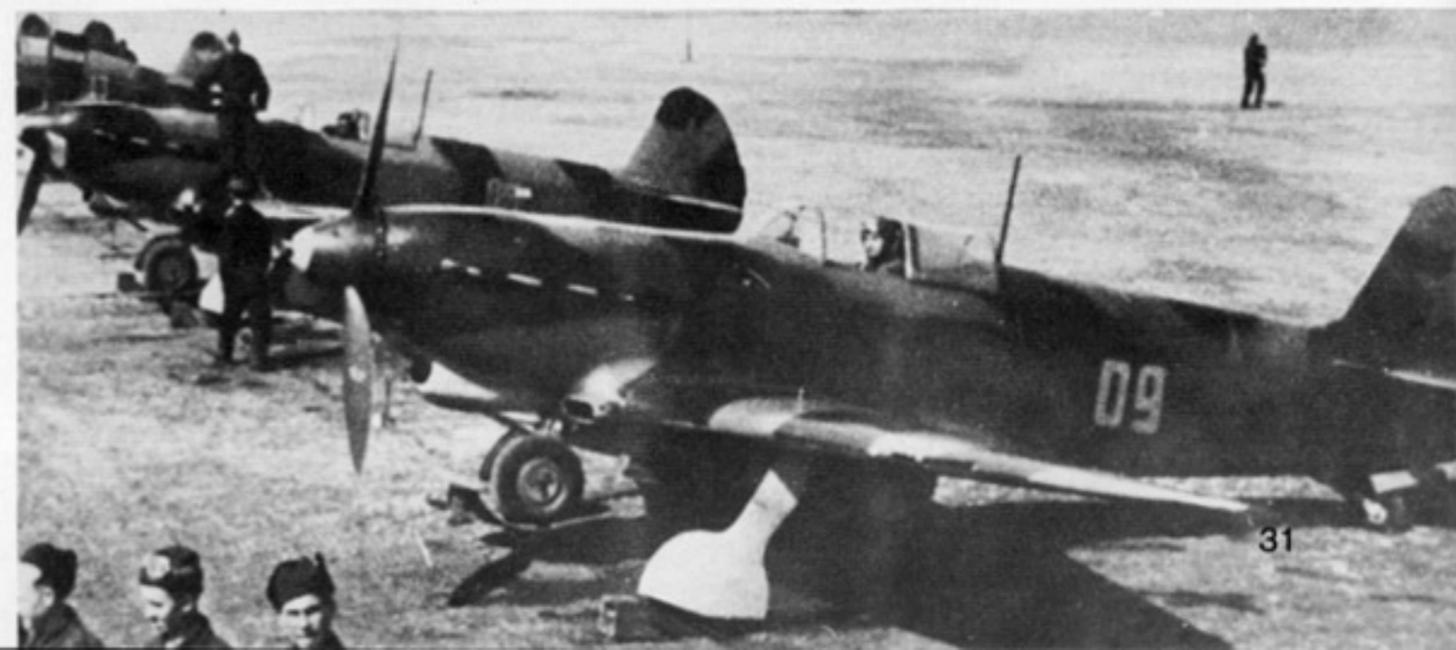
(Below) The Yak 9 saw action for the first time in late November of 1942. The aircraft in the foreground is an early Yak 9 with the earlier Yak 7 wing and armor plate. Later Yak 9 variants produced in early 1943 would feature a new spinner and aerodynamically refined wing root carburetor intakes. The numerals 76 in White is painted on the rudder. (Andrzej Morgala)
