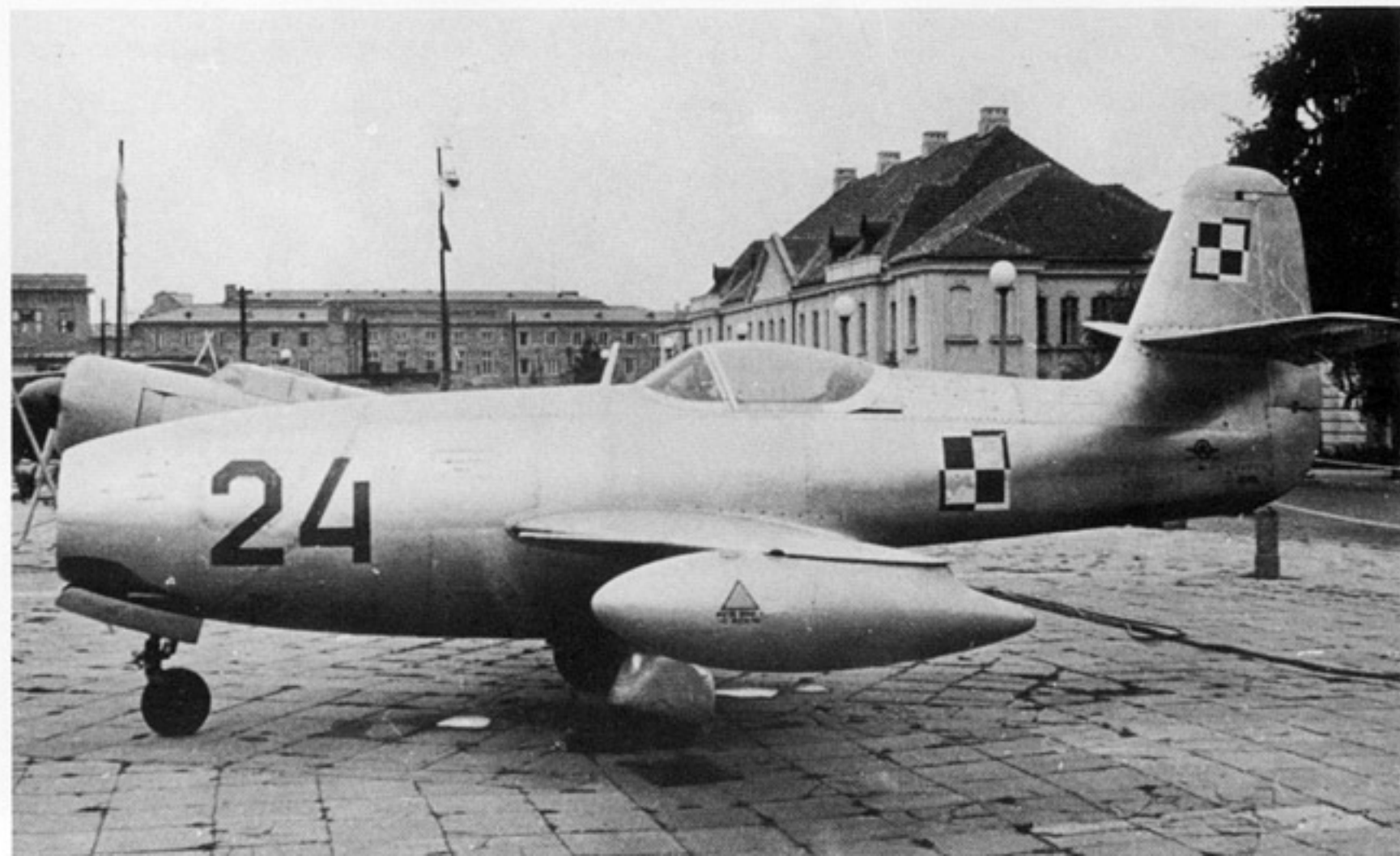
(Below) The Yak 23 entered service with the Polish Air Force in 1950, mainly serving with 1. PLM (Fighter Group). The Yak 23 was powered by the Soviet RD-500 engine, a Soviet copy of the Rolls-Royce Derwent V powerplant. Projects to build the Yak 23 under license were dropped in favor of the more advanced MiG 15. (Andrzej Morgala)
