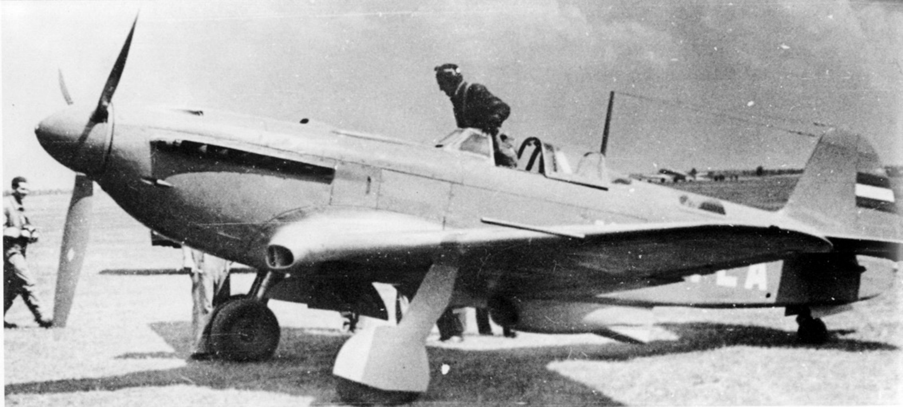
(Below Left) An overall Light Gray Yak 9P in Polish service. A Russian inscription in white can be seen on the propeller blade. All Yak 9Ps were powered by a 1,600 hp Klimov M-107 A engine and carried an armament of a single ShVAK 20mm cannon with 100 rounds, and two 12.7mm machine guns each with 250 rounds. Some examples of the Yak 9P were also armed with a 23mm cannon. (Andrzej Ec)
