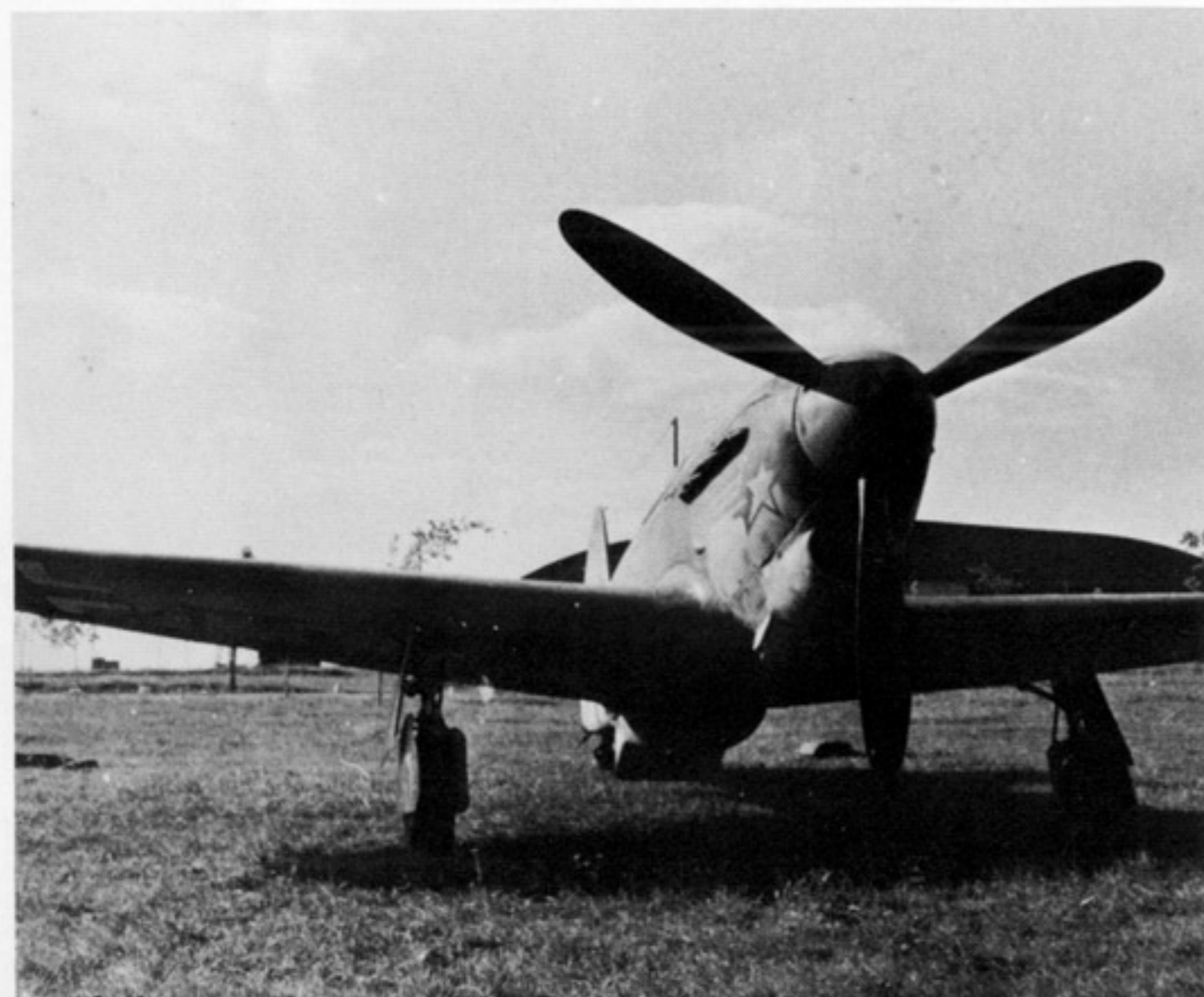
(Left) This Yak 1M was captured by the Wehrmacht at Uman in 1943. A freshly applied Balkenkreuz can be seen under the wings. The original Russian 'Winged Star' marking on the side of the nose and a Red spinner with a White star are still on the aircraft. This particular aircraft did not carry a wing root oil cooler intake. (Willy Radinger)
