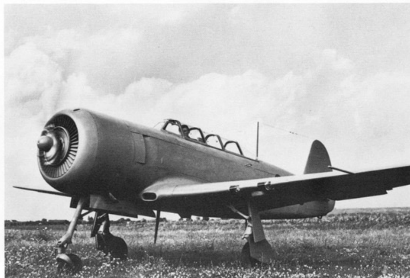
(Below) The sole C-11U built at the Uherské Hradiste LET factory at Kunovice. The type was developed to facilitate pilot conversion to jet fighters equipped with tricycle landing gear. Two landing lights are mounted in the port wing. (Hans-Joachim Mau)
