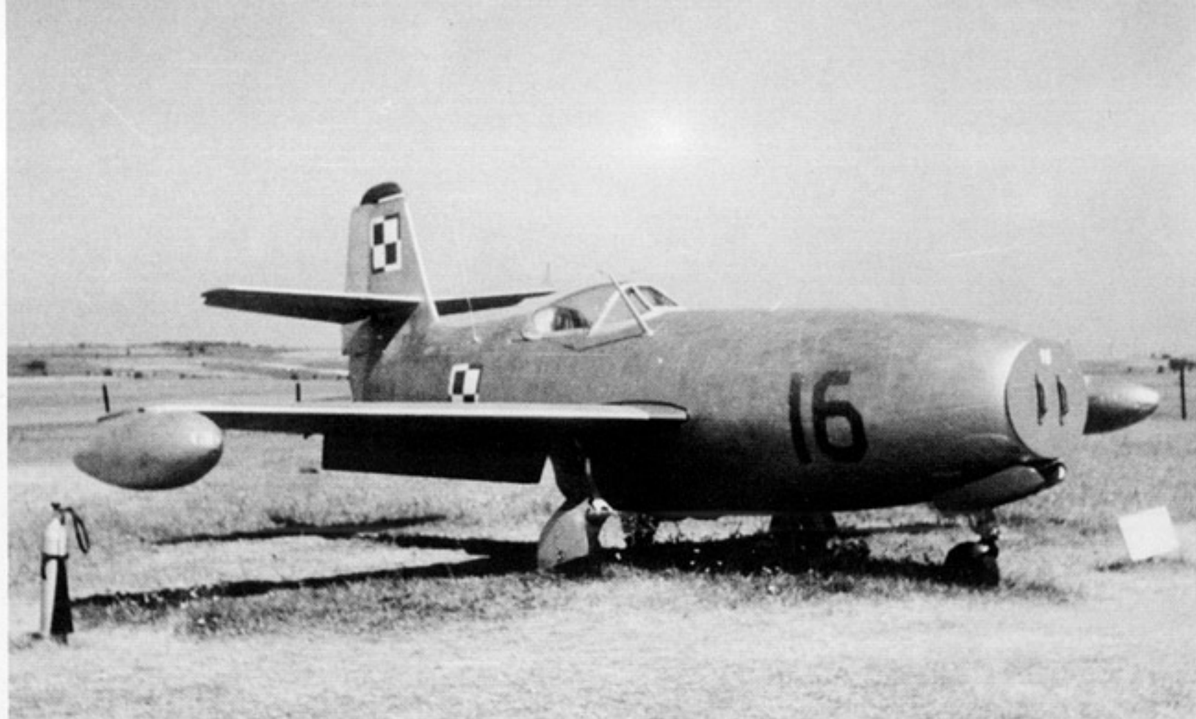
(Above) 230 Yak 23s were built between March of 1948 and 1950. The Yak 23 replaced the Yak 9P in front line fighter units, and also saw service in Czechoslovakia, Poland, Bulgaria and Rumania. Most Yak 23s carried a bubble tank on the wing tips. (Andrzej Morgala)
