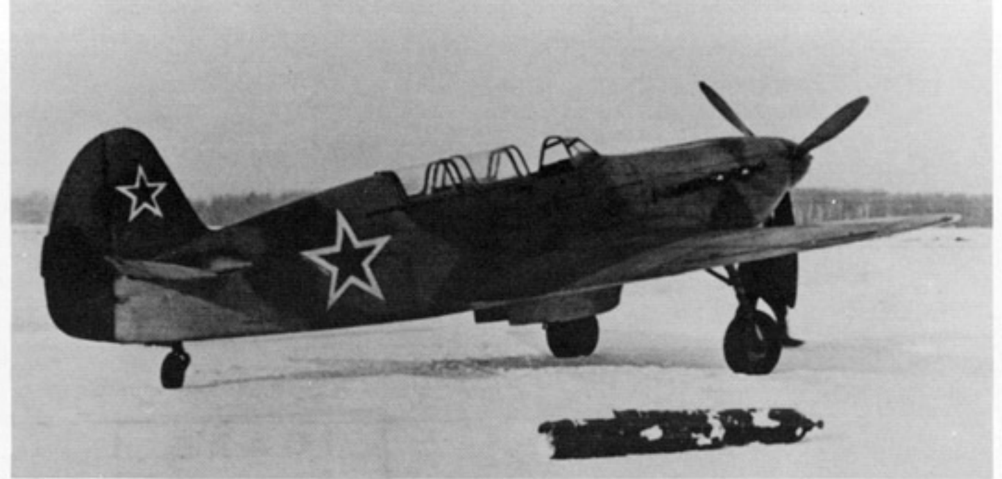
(Above) A Yak 7V trainer with a fixed undercarriage. Trainers and fighters were structurally identical. A trim tab was applied only to late Yak 7s. The camouflage is Gray and Dark Gray, colors not often used on Trainers. (SHAA)
