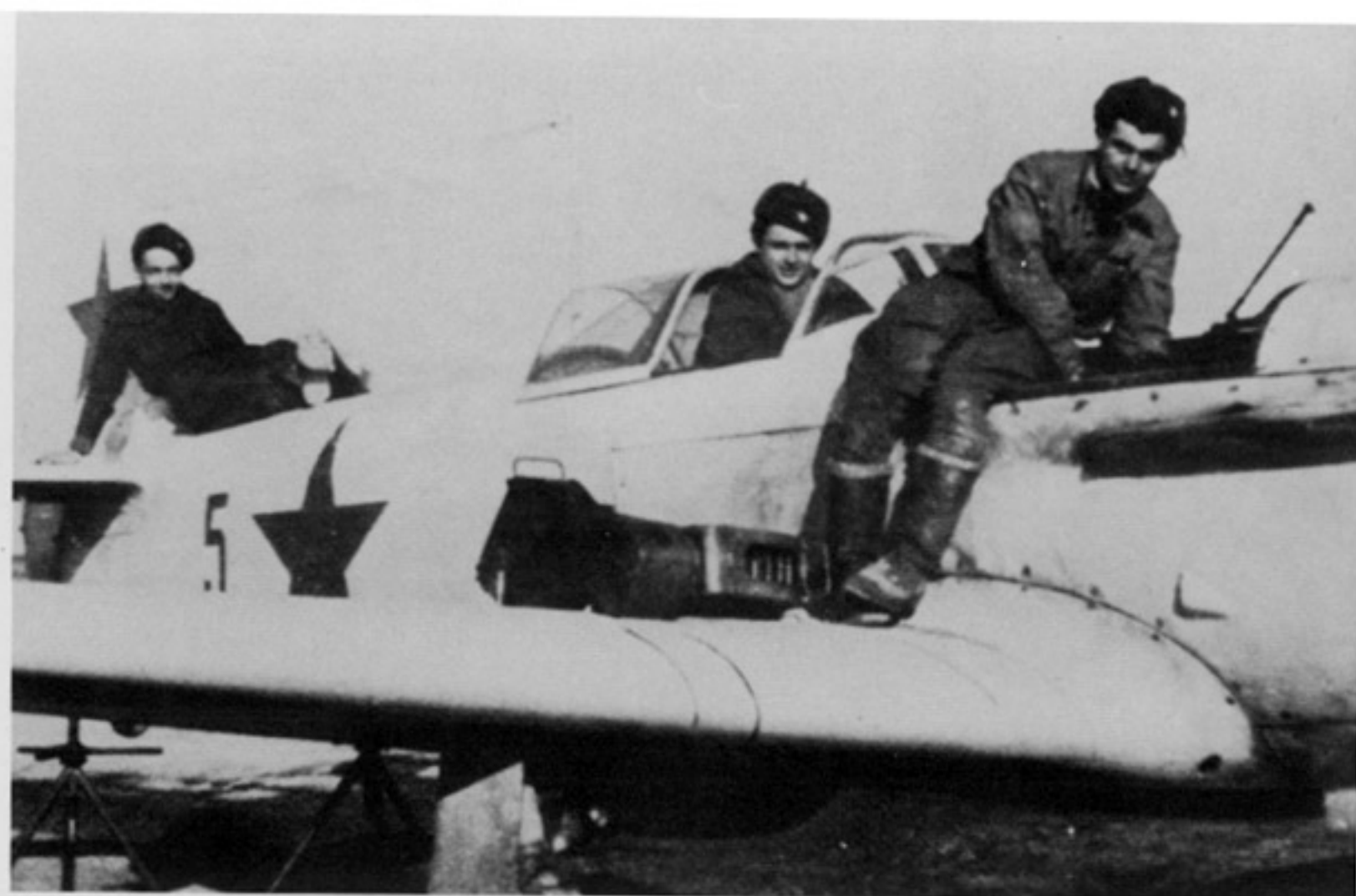
(Above Right) Ground personnel overhaul Red 5, a winter camouflaged Yak 1M at Ivanovo in late 1942. The large wing root intake is not on this aircraft, but it has the small non-standard inlet. Five mechanics could change a complete Klimov engine including adjusting the Cannons within six hours, even under the poorest of conditions. (Karl Hänggi)
