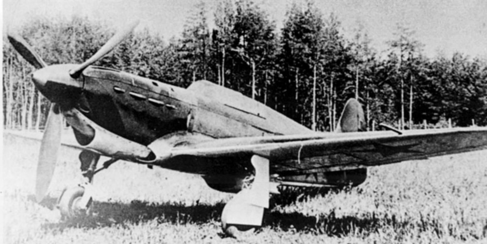
(Above) A very early I-26 (Yak 1) built at Zavod (Factory 115) near Moscow. Pre-war production fighters carried an armament of a single 20mm ShVAK cannon and two 7.62mm ShKAS machine guns mounted in the upper deck of the nose, but this rather inadequate firepower was rather unpopular with front line pilots. Most early I-26s had no radio equipment. (Hannu Valtonen)
