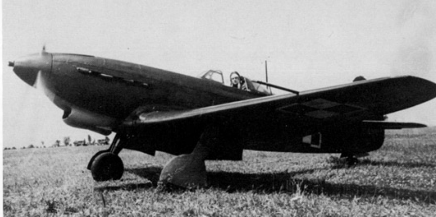
(Above) The Yak 9T-37 received a 37mm cannon developed by A. Nudelman and A. Suranov. To accommodate the breech of the large cannon within the fuselage the cockpit was move aft 15.75 inches. This modification became standard on all late Yak 9Ds. Poland received twelve Yak 9T-37. (Andrzej Morgala)
