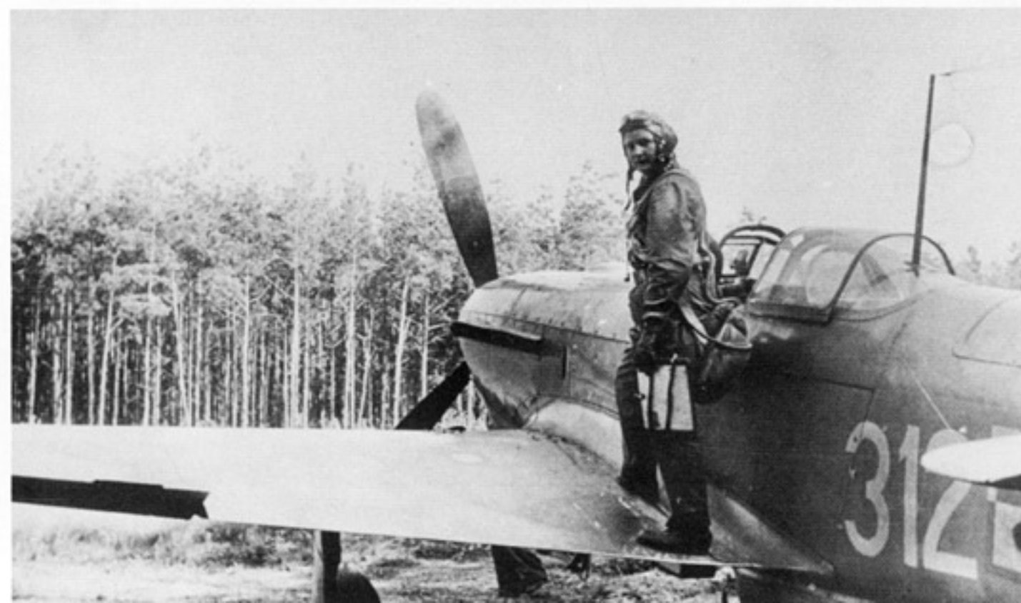
(Below) One of the ninety Yak 9Ps used by the Polish Air Force during the post war period. These aircraft were camouflaged in Light Gray, Olive Drab and Medium Gray uppersurfaces over Light Blue undersurfaces, such as carried on White 312. The Yak 9P could be distinguished from the earlier Yak 9D by the aerial mast coming through the rear canopy and redesigned exhaust stubs. Cockpit equipment of a Yak 9P included a RSI-4 Radio and a RPKO-10 radio compass. The circle on the wing is a fuel gauge indicator. (Andrzej Morgala)
