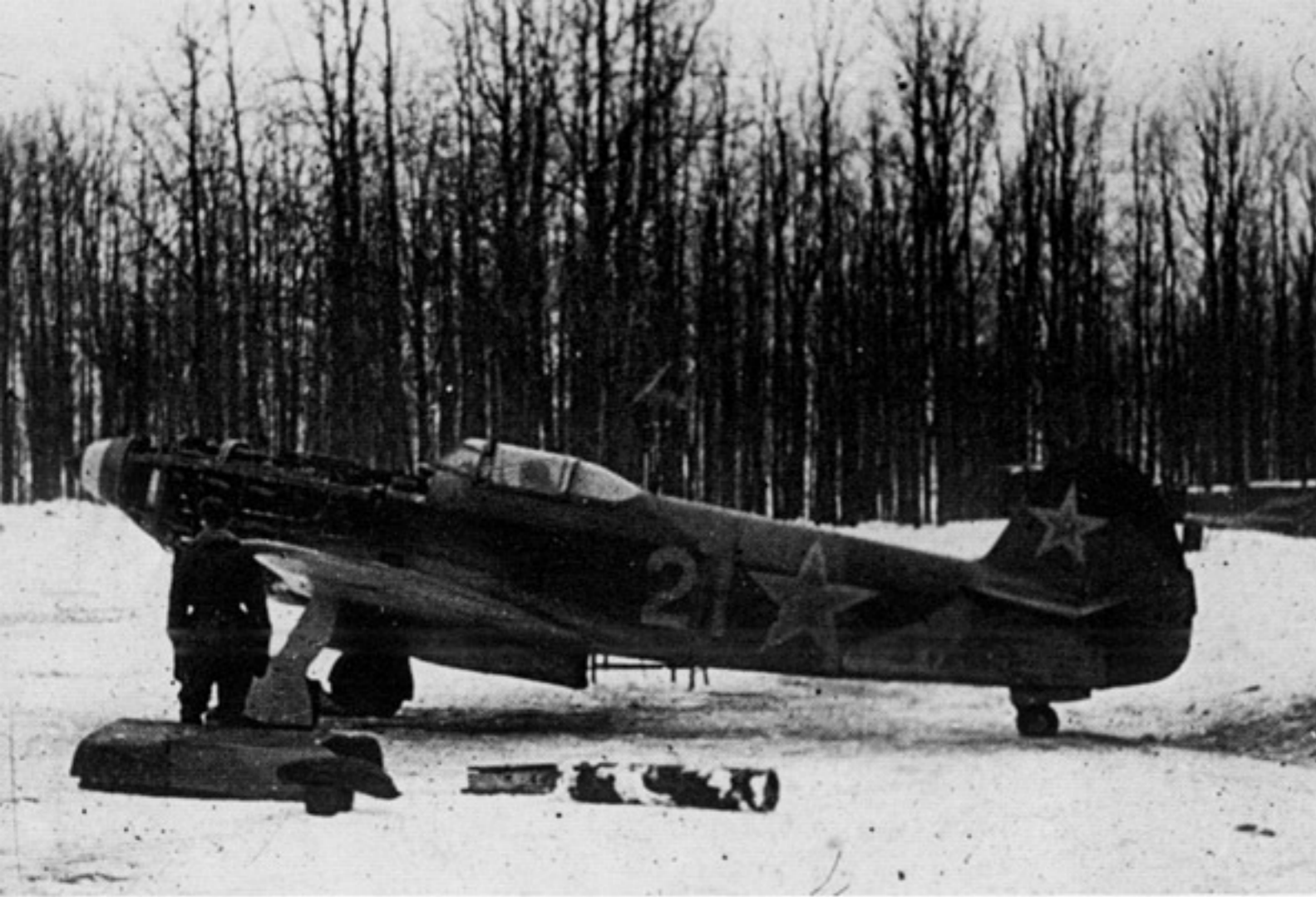
(Above Left) Russian Mechanics check out an engine after an overhaul at Toula in late 1943. The Soviet Klimov M-105 PF powerplants proved very reliable even in the coldest periods. Inexperienced pilots often tended to bring the engine to full start-performance before sufficient warm-up. The Klimov engine was usually forgiving of such brutal treatment, but not so the more fragile engines in the American and British lend-lease fighters! (SHAA)
