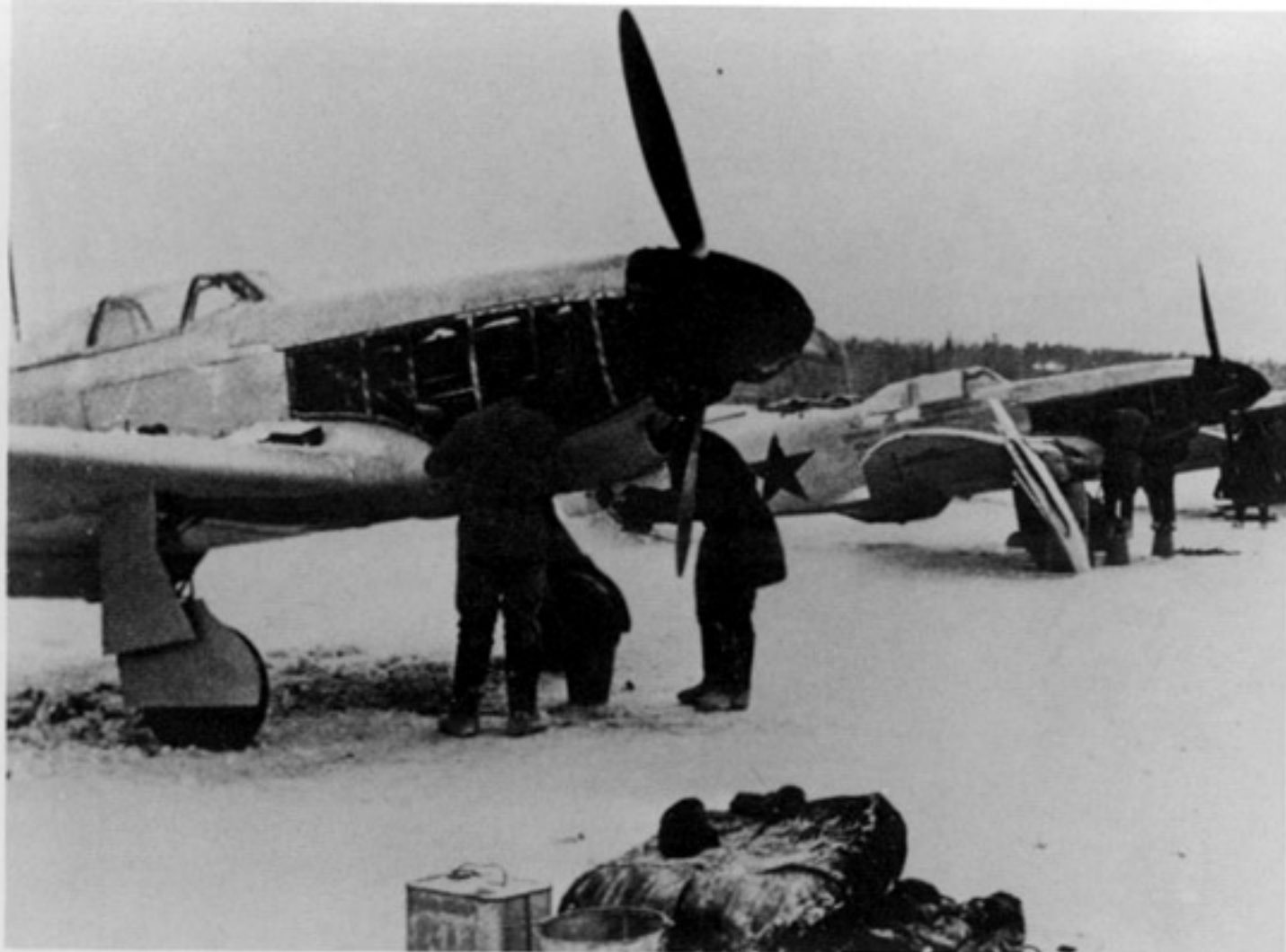
(Above Left) Line-up of Yak 1Ms at Ivanovo during early 1943. The Klimov M-105 PF engine demanded 92 octane fuel. Ground crews liked the aircraft, which was very reliable and easy to maintain, with refueling and re-arming seldom taking more than twenty minutes. During the very cold winter months standard lubricant Type MSZ was replaced by the low temperature lubricant type MZSZ. (SHAA)
