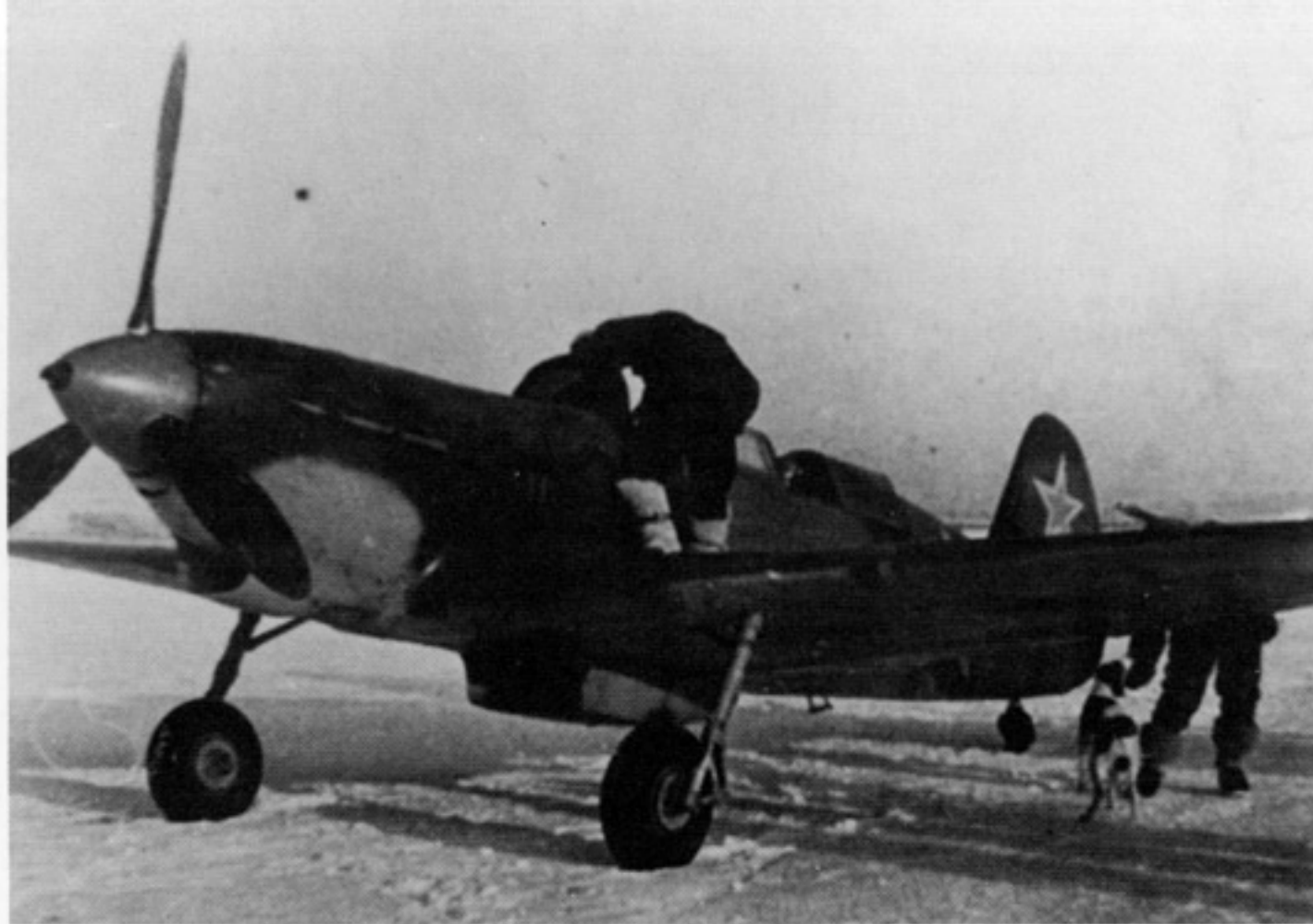
(Above) The initial two seat Yak 7V trainer had a fixed undercarriage and no radio, and was armed with a single 20mm cannon. Besides the trainer role, the Yak 7V saw exhaustive use as a courier aircraft. This machine is painted in Gray and Dark Gray over Light Blue under surfaces, with a Red spinner. The line between the Gray and Light Blue on the nose is unusually high. (SHAA)
