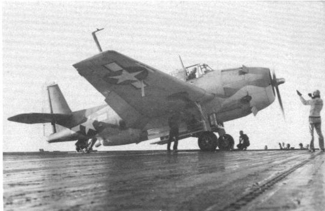
This TBM-1 was one of six USS MISSION BAY (CVE-59) Avengers modified to carry the Cal-Tech retro-bomb and Magnetic Anomaly Detector (MAD) equipment (mounted in the 'stinger' position). The retro-bomb had a small rocket motor which stopped the bomb's forward movement and allowed it to drop vertically. (USN via David Lucabaugh)
