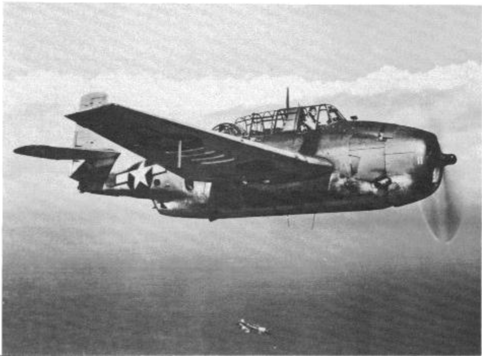
A very weathered, war-weary Avenger on patrol over the Pacific from USS TICONDEROGA (CV-14) on 30 June 1944. This TBM-1C of VT-80 carries four Mk 4 rocket rails, ASB radar antennas on the outer wing panels, and a gun camera mounted just in front of the windscreen. (USN via Jim Sullivan)
