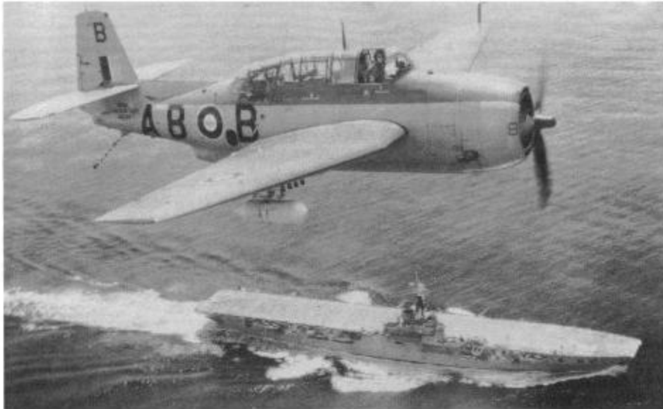
125 Avengers served with three Royal Canadian Navy squadrons from 1950 to 1957. This TBM-3S of No. 825 Squadron passes over the Canadian carrier HMCS MAGNIFICENT during 1951. Canadian Avengers carried a Dark Sea Grey over Light Sea Grey camouflage scheme and a Red and White striped tailhook. (National Museums of Canada)
