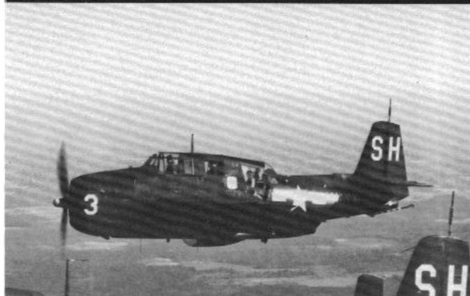
A number of TBM-3E airframes were modified for the anti-submarine strike role under the designation TBM-3S. This TBM-3S carries a search light mounted under the port wing and a data link antenna mounted on the top of the rudder. The white rectangle on the center fuselage is the hatch for the life raft stowage compartment. (Grumman)
