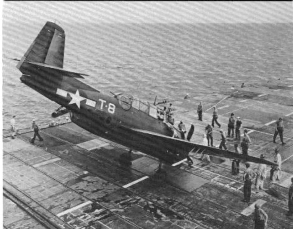
The US Navy operated two side paddle wheel aircraft carriers on Lake Michigan during the Second World War. Both USS WOLVERINE and USS SABLE were training carriers converted from Great Lakes cruise ships. ENS W.D. Henderson nosed over this overall Glossy Sea Blue TBF-1 during Carrier Qualifications (CARQUALS) aboard USS SABLE on 2 August 1945. (Smithsonian via F.C. Durant)
