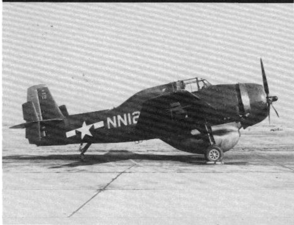
The original 'Project Cadillac' XTBM-3W prototype, an extensively modified TBM-3 equipped with an APS-20 radar mounted in the bomb bay. To improve lateral stability auxiliary tail fins were installed on the horizontal stabilizers. (Grumman)
