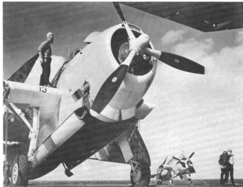
A TMB-1C of an Atlantic CVE is equipped with flame damping exhausts for night operations. The propeller hub and a portion of each propeller blade were painted in Non-Specular Insignia White in keeping with the aircraft camouflage. (Grumman)
