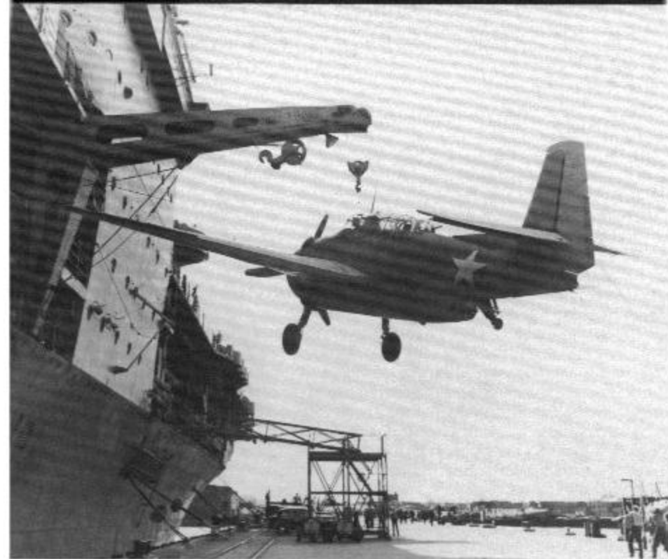
A ship's crane lifts a TBF-1 from the dock to the hangar deck of a Pacific carrier during 1942. When level with the deck edge, the Avenger will be swung tail first through the open hangar bay hatch. The crewman riding in the cockpit is the aircraft's plane captain who will control the brakes as the aircraft is moved into position within the hangar deck. (USN via MAJ J.M. Elliott, USMC-Ret.)
