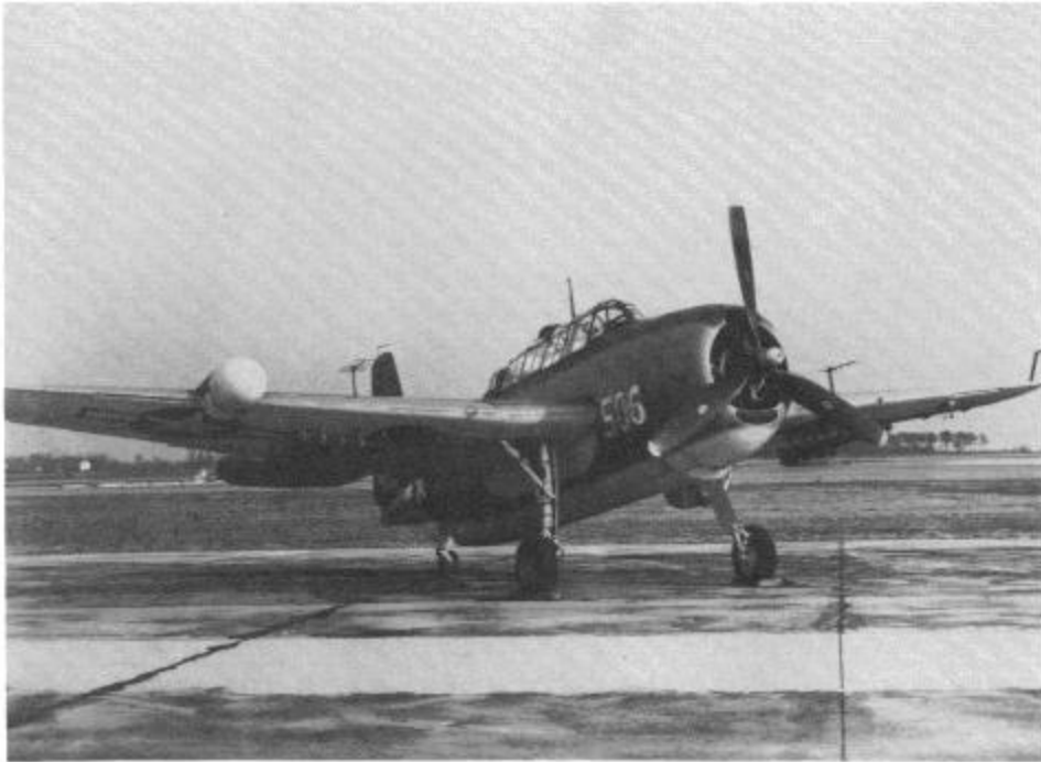
This TBM-3D carries 5 inch HVAR rockets, an ASD radar in the radome mounted on the starboard wing leading edge, a search light mounted under the port wing, and ASB radar yagi antennas on top of the wings. (USN via MAJ John Elliott, USMC)
