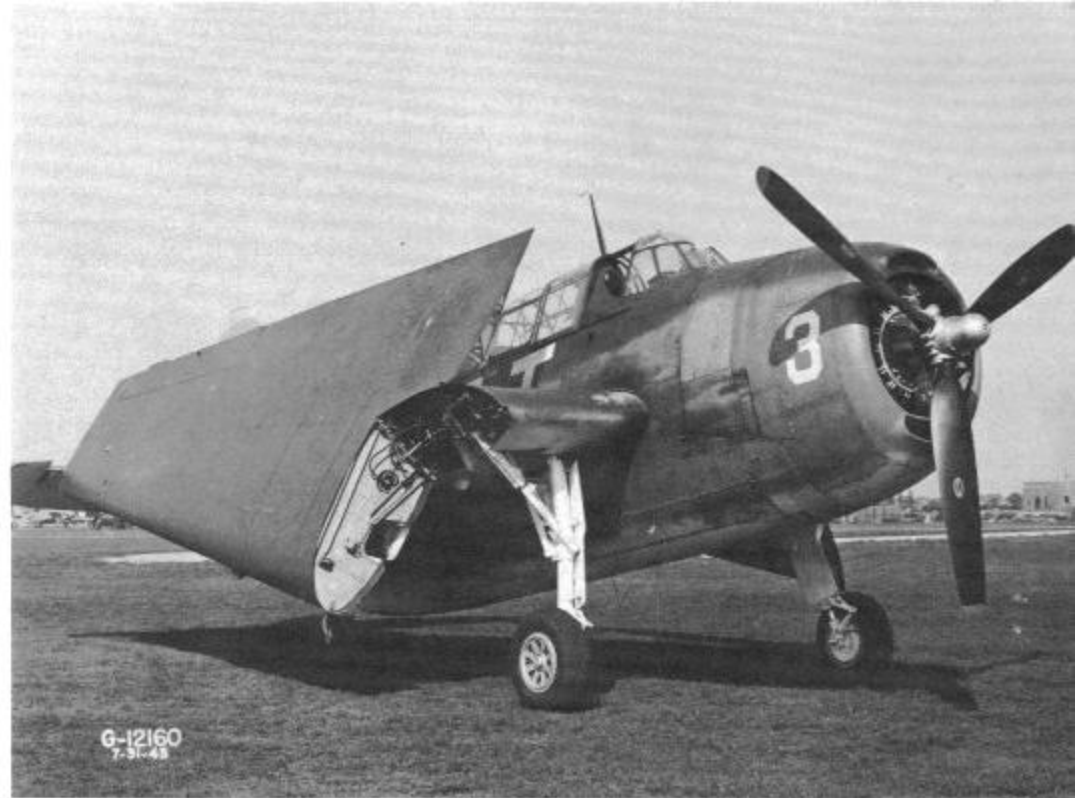
The Grumman XTBF-3 prototype parked on the grass at Bethpage during October of 1943. The TBM-3 featured a reconfigured cowling for the 1,900 hp Wright R-2800-20 engine, with four cowl flaps on each side and an oil cooler intake added to the lower cowl lip. (Grumman)
