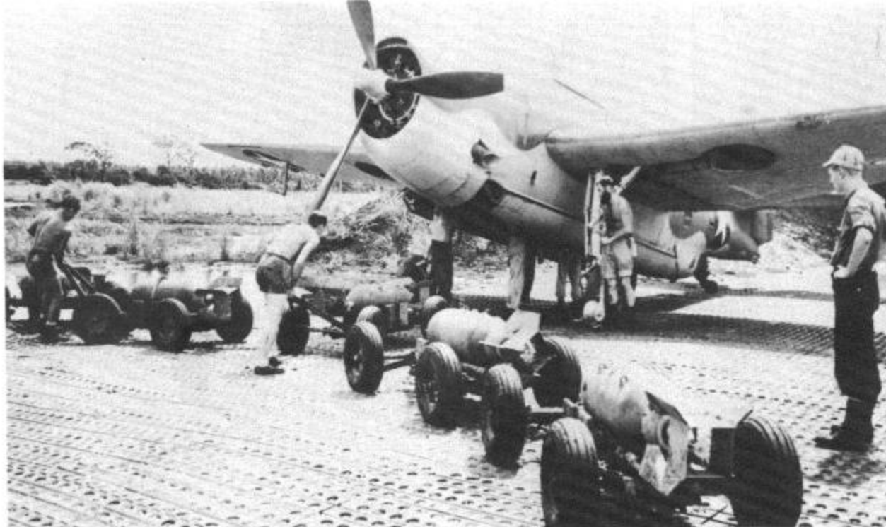
Groundcrews on Guadalcanal prepare to load a train of 500 pound GP bombs on an Avenger during 1942. The bombs are fully armed with both nose and tail fuses in place. Navy and Marine Avengers on Guadalcanal were used as glide bombers against Japanese shipping attempting to land reinforcements on the island. (Grumman)
