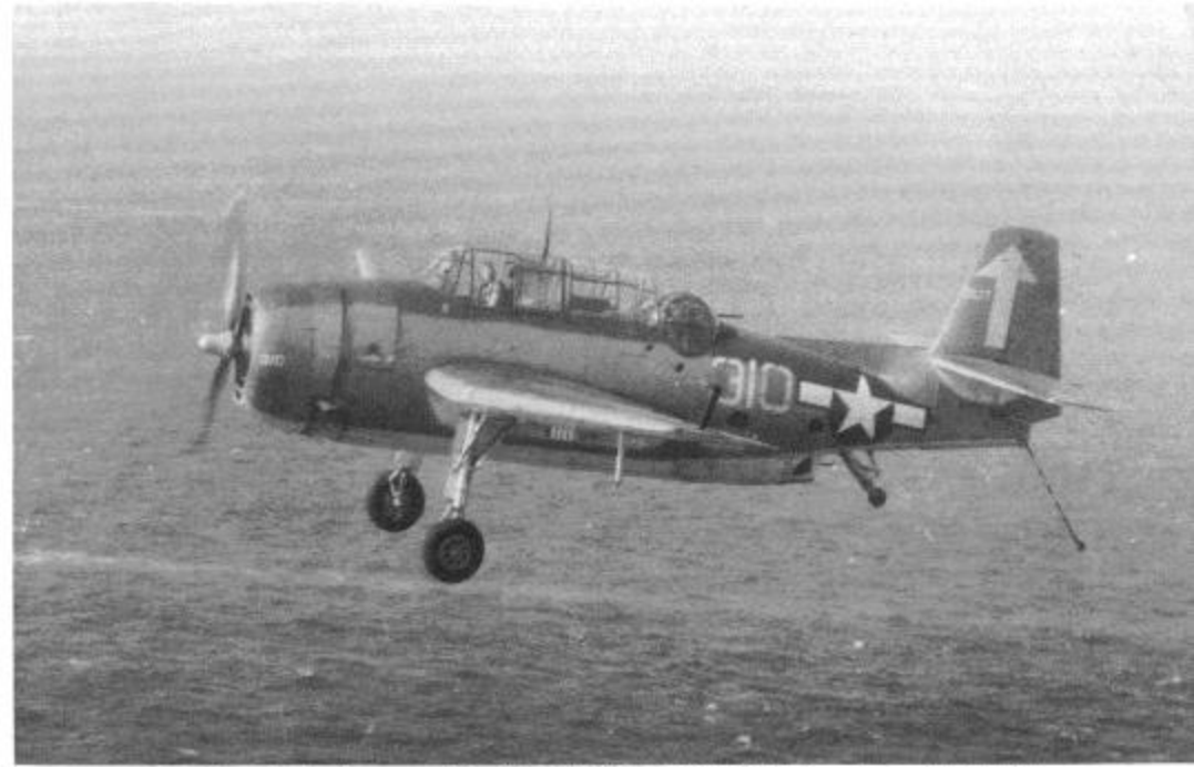
A TBM-3 of VT-84 on its final approach to USS BUNKER HILL (CV-17) on 5 April 1945. The Avenger's retractable tail hook is down and ready to catch an arresting wire on the carrier's deck. The White arrow on the fin is the identification marking carried by BUNKER HILL aircraft. (USN via David Lucabaugh)
