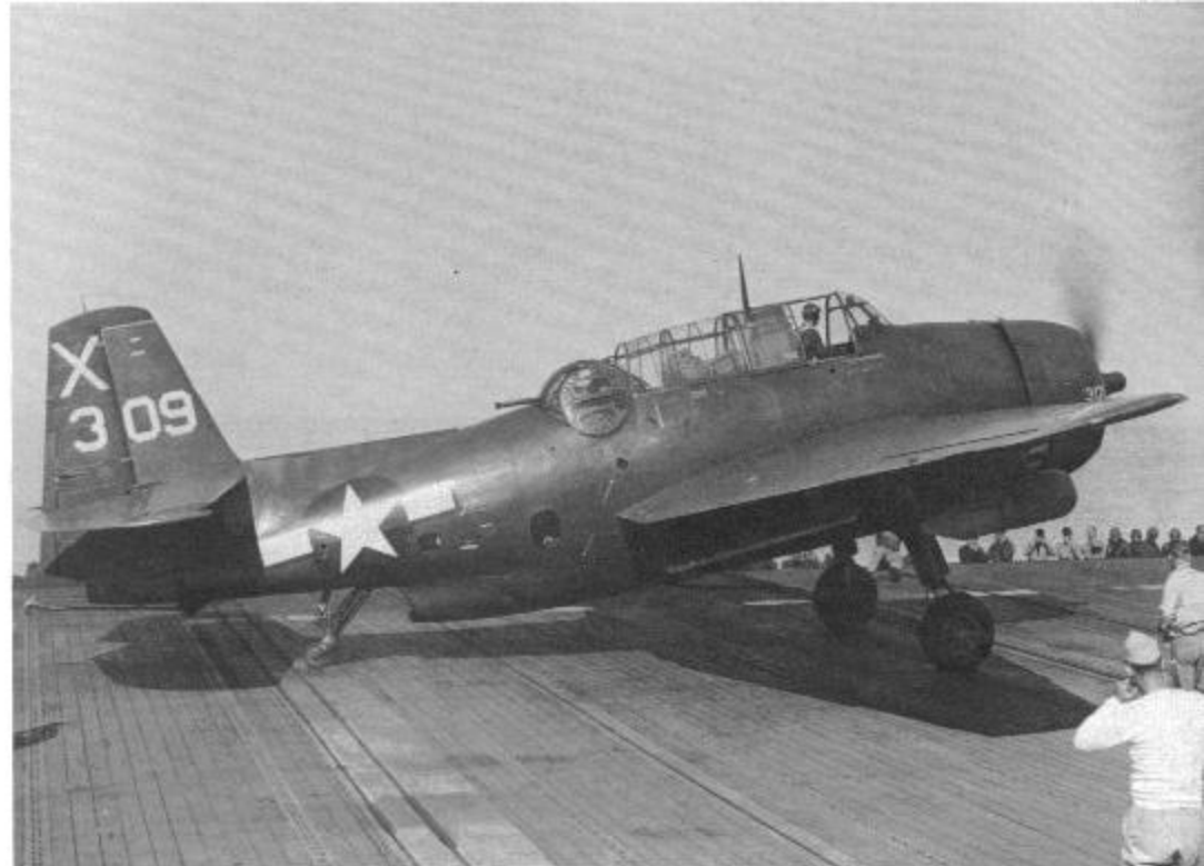
A TBM-3E of VT-86 prepares for takeoff from USS WASP (CV-18) during October of 1945. The radioman's 'stinger' gun position was deleted on the light weight TBM-3E and the earlier retractable tail hook was replaced by an externally mounted non-retractable hook. (USN via David Lucabaugh)
