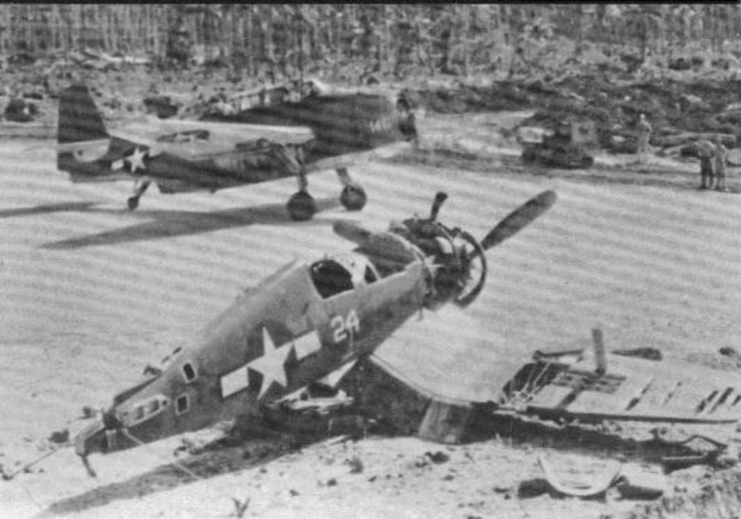
A Marine Corps TBM-3 taxis past an abandoned F4U-1 Corsair which has been cannibalized for spare parts on a Pacific island during 1944. The hard rubber tail wheel tire has been replaced by a larger pneumatic tire for operations on land. (USN via Jim Sullivan)
