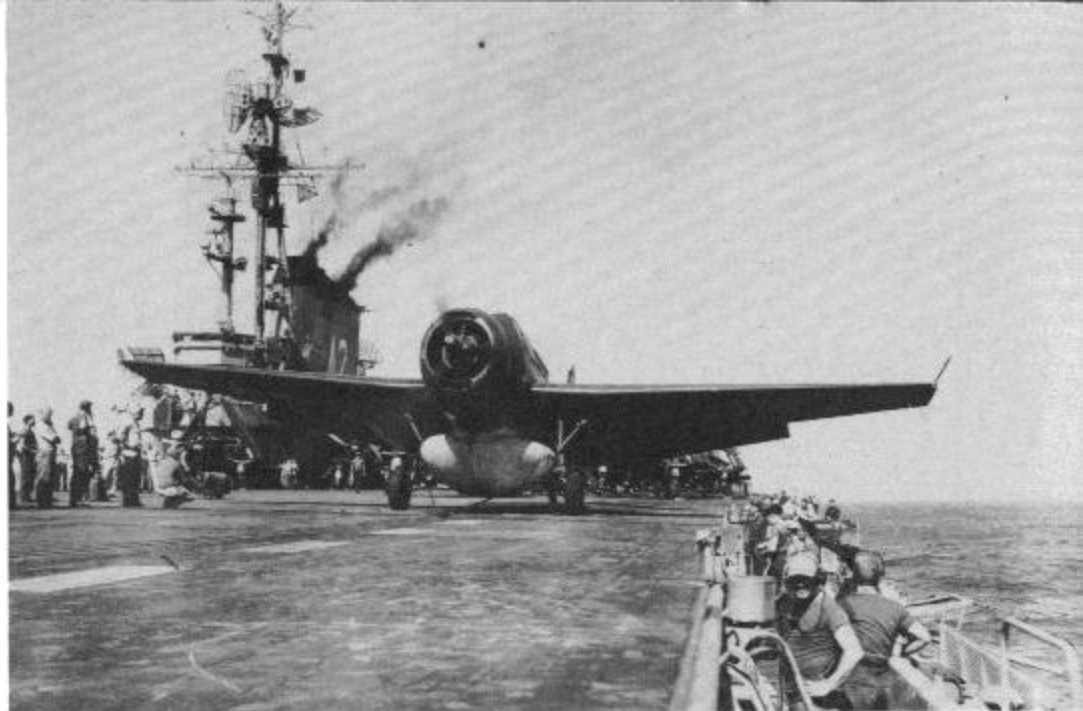
A TBM-3W of VA-4B on USS FRANKLIN D.ROOSEVELT's (CVA-42) port catapult is just seconds away from launch. TBM-3Ws usually operated at some distance from the carrier on standing radar patrols, or teamed with TBM-3S strike aircraft in anti-submarine operations ahead of the carrier. (Grumman)
