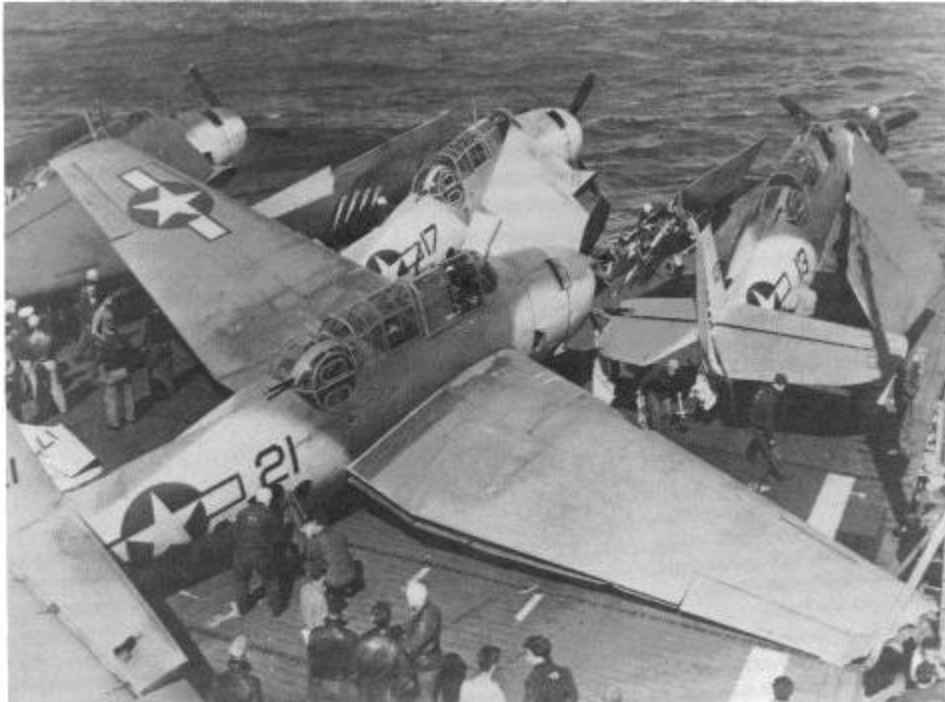
On 18 September 1944, this VC-42 TBM-1C has gone over the barrier on USS BOGUE (CVE-9) and crashed into other Avengers parked forward on the flight deck. For destroying three TBMs, the pilot was awarded a mock Iron Cross by his squadron mates. (USN via David Lucabaugh)
