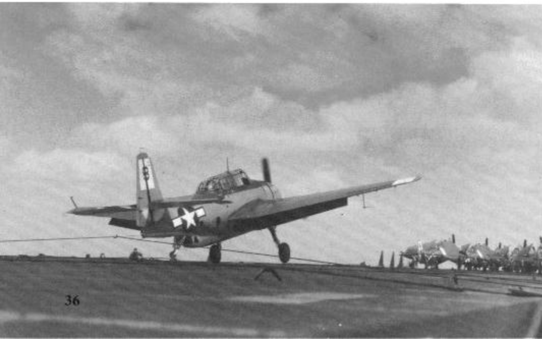
A TBM-3 of VT-45 'traps' (catches an arresting cable) aboard USS SAN JACINTO (CVL-30) on 21 March 1945. The cables running across the deck just behind the parked Avengers are the crash barrier, designed to stop any landing aircraft that failed to engage an arresting cable. (USN via David Lucabaugh)
