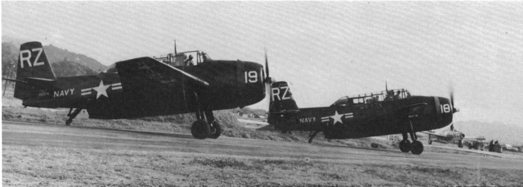
(Above) A pair of TBM-3Rs of VR-21 go through final engine checks before take off from Itazuke, Japan during 1951. These TBM-3Rs have a glass panel fairing instead of a metal fairing over the turret position. (Grumman)
