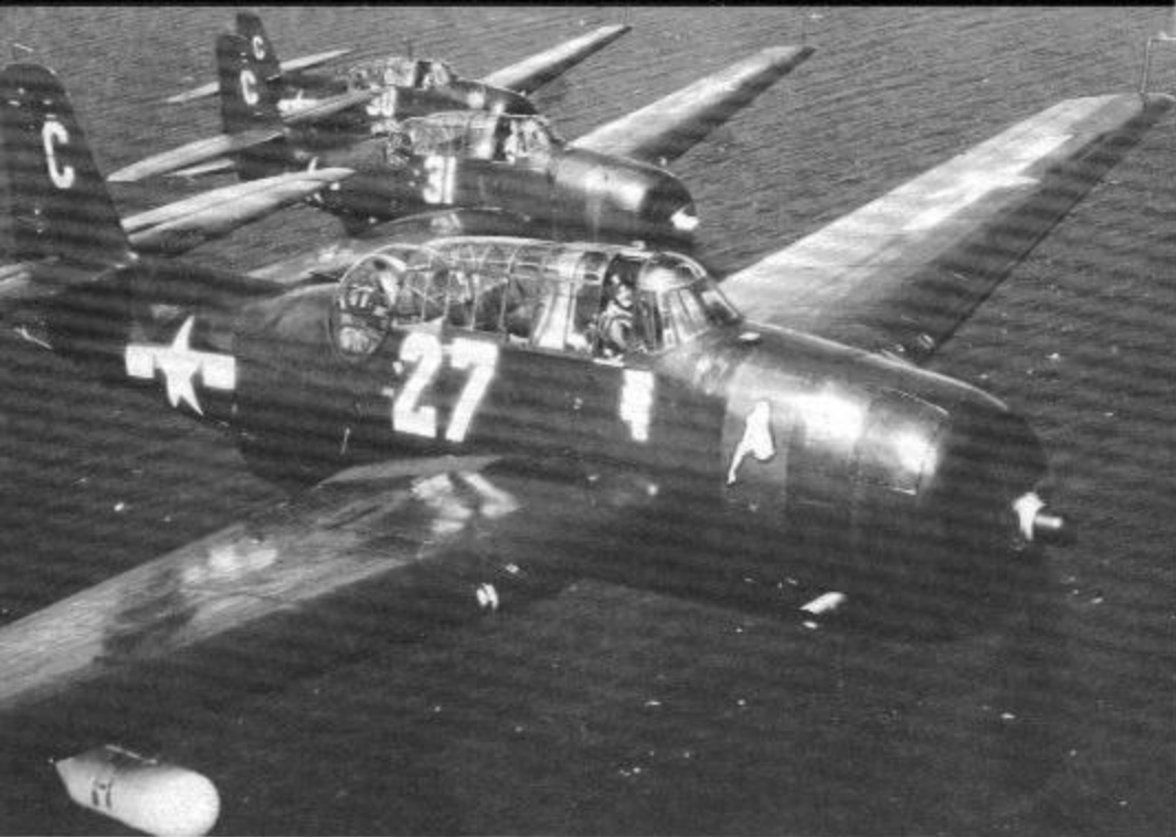
A flight of TBM-3Es of VT-34 return to USS MONTEREY (CVL-26) on 29 Aug 1945. The demarcation line between the upper surfaces of Glossy Sea Blue and Non-Specular Sea Blue lower surfaces is easily seen. Markings such as the White mission marks just below the cockpit and the shapely pin up girl on the fuselage are extremely rare on a Navy aircraft. The white pod under the starboard wing is an AN/APS-4 radar pod. (USN via Nick Waters)
