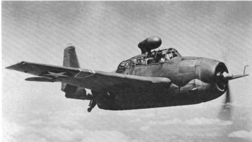
An Avenger of the Naval Experimental Station, Philadelphia, Pennsylvania carries an experimental ASD-1 radar installation on the canopy. This installation proved impractical and the radome was moved back to the leading edge of the starboard wing on the TBF/TBM-1D. (USN via Jim Sullivan)
