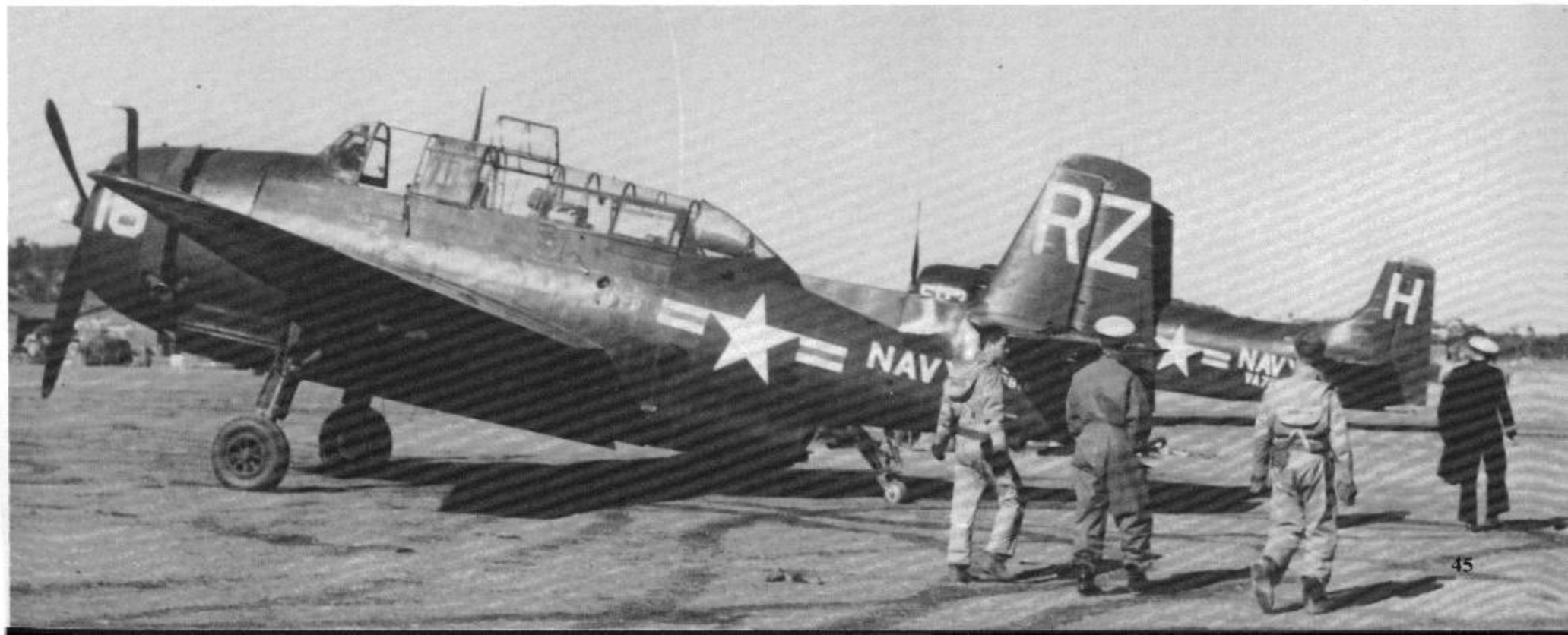
(Above) A pair of TBM-3Rs of VR-21 go through final engine checks before take off from Itazuke, Japan during 1951. These TBM-3Rs have a glass panel fairing instead of a metal fairing over the turret position. (Grumman)
