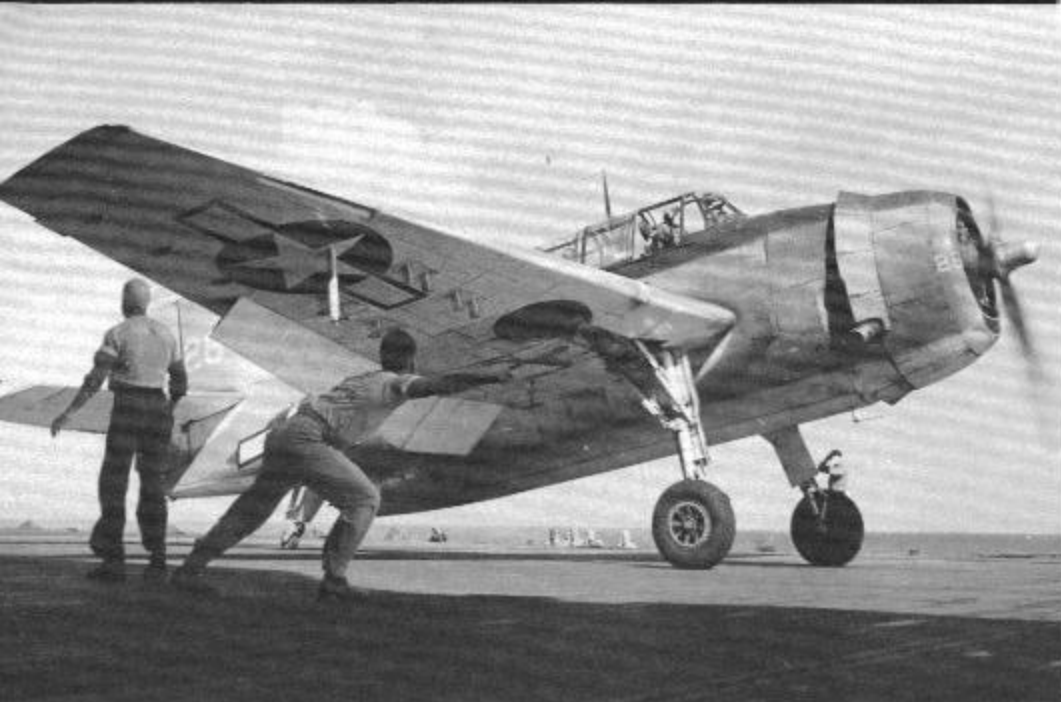
A TBM-3 receives the launch signal from the flight deck officer and begins its takeoff roll from USS FRANKLIN (CV-13) during March of 1944. The Avenger is fitted with ASB radar antennas and Mk 5 rocket launchers on the outer wing panels. (USN via David Lucabaugh)
