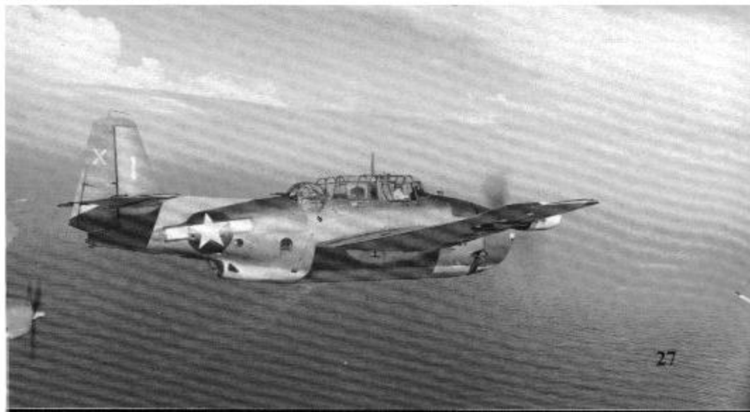
A TBM-1D of VT-51 flying from USS SAN JACINTO (CVL-30) on anti-submarine patrol during July of 1944. The TBM-1D carried ASD-1 radar in a streamlined radome mounted on the starboard wing leading edge. The ASD-1 range varied considerably, the author was able to get an 80 mile range, and large land masses could be picked up at distances up to 100 miles. (USN via David Lucabaugh)
