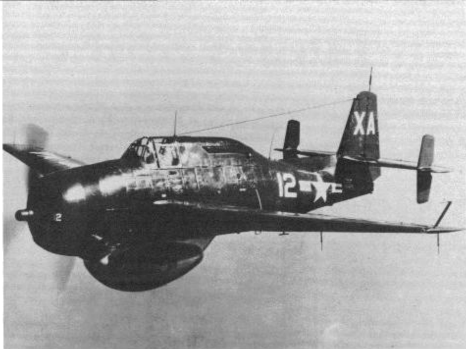
A TBM-3W of VX-1 in flight near Naval Air Station Boca Chica, in the Florida Keys during January of 1950. The TBM-3W carried numerous whip antennas, for communications, IFF, and data link transmitters and receivers. The 'turtle-back' fairing was hinged to allow easy access to the electronics behind the pilot's cockpit. (Grumman)
