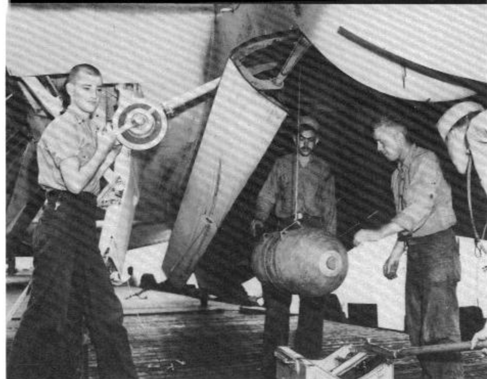
Ordnancemen load 500 pound GP bombs into the bomb bay of an Avenger with a Mk 7 Bomb Hoist. After the bombs are shackled in place, fuses and arming wires will be installed and the bomb bay doors closed. A normal bomb load for the Avenger was four 500 pound bombs. (Grumman)
