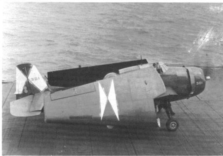
TBM-3 of VT-83 taxis forward on USS ESSEX (CV-9) 19 April 1945. The White 'double triangle' is the geometric recognition marking assigned to all ESSEX aircraft. Avengers during WWII have often been mistakenly identified as carrying overall Glossy Sea Blue paint. In fact Avengers carried Glossy Sea Blue on the upper surfaces only, with Non-Specular Sea Blue on the lower fuselage sides and under-surfaces. (USN via David Lucabaugh)
