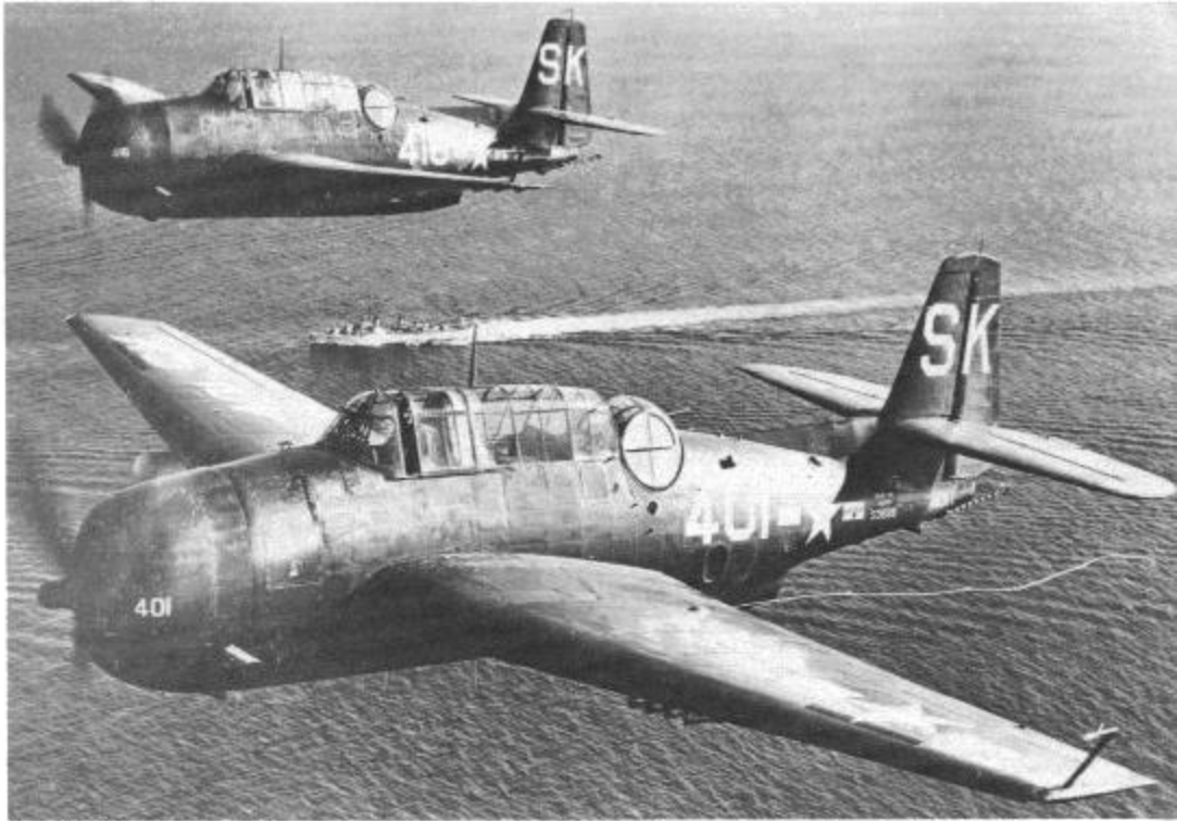
A pair of TBM-3Es during a postwar anti-submarine training exercise. The Trailing Radio Antenna under the port wing was used for aircraft to ship radio communications with the destroyer, USS GURKE (DD 783), and would (hopefully) be reeled-in before landing. (Grumman)
