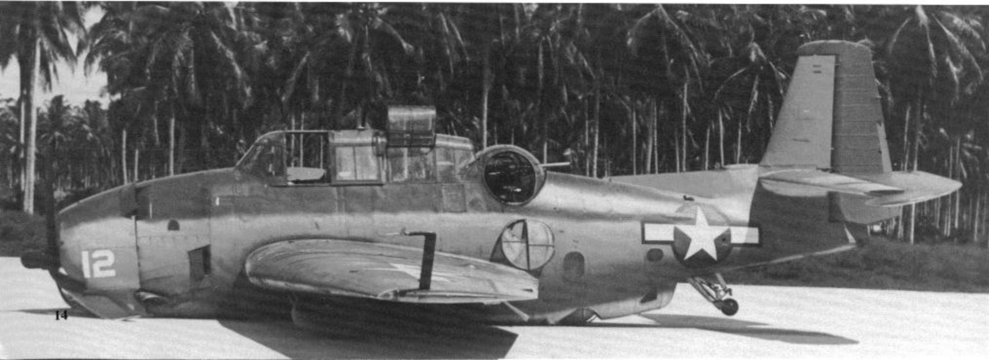
This TBM-1 nosed over during night carrier qualifications aboard USS BATAAN (CVL-29) on 3 February 1944 damaging the starboard wing. Light carriers normally operated a squadron of fighters and a squadron of Avengers. Later in the war Avengers flying from USS BATAAN would score four torpedo hits on the Japanese battleship YAMOTO, the worlds most heavily armed warship. (USN via David Lucabaugh)
