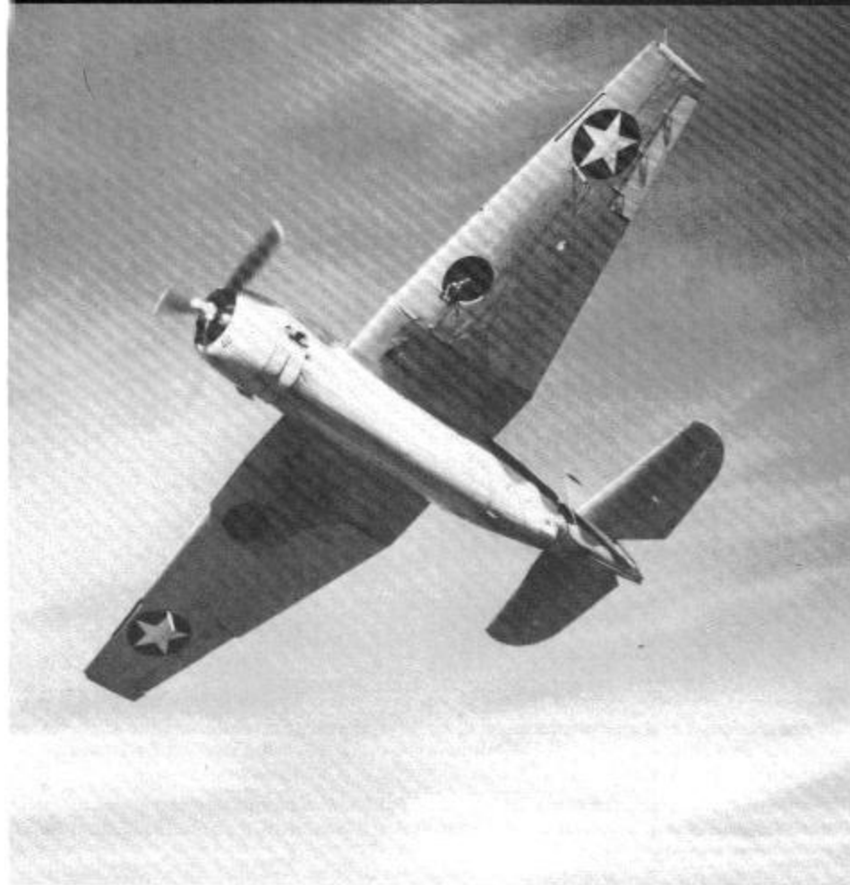
The two antennas mounted on the inboard edge of the national insignia are yagi antennas for the ASB radar. The TBF main landing gear wheel wells deliberately lacked covers, because Grumman engineers thought wheel well doors were unnecessary weight and would further increase maintenance difficulties. (Grumman)
