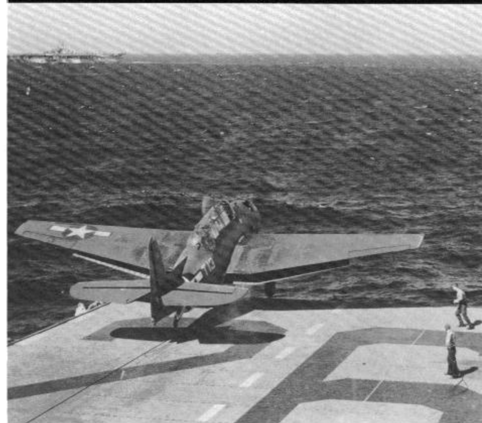
A TBM-1C of VC-30 is catapulted from the deck of USS MONTEREY (CVL-26) during 1943. Heavily loaded Avengers usually settled after leaving the deck until they built up enough airspeed to begin their climb to altitude. (Hank Weimer Collection via Jim Sullivan)
