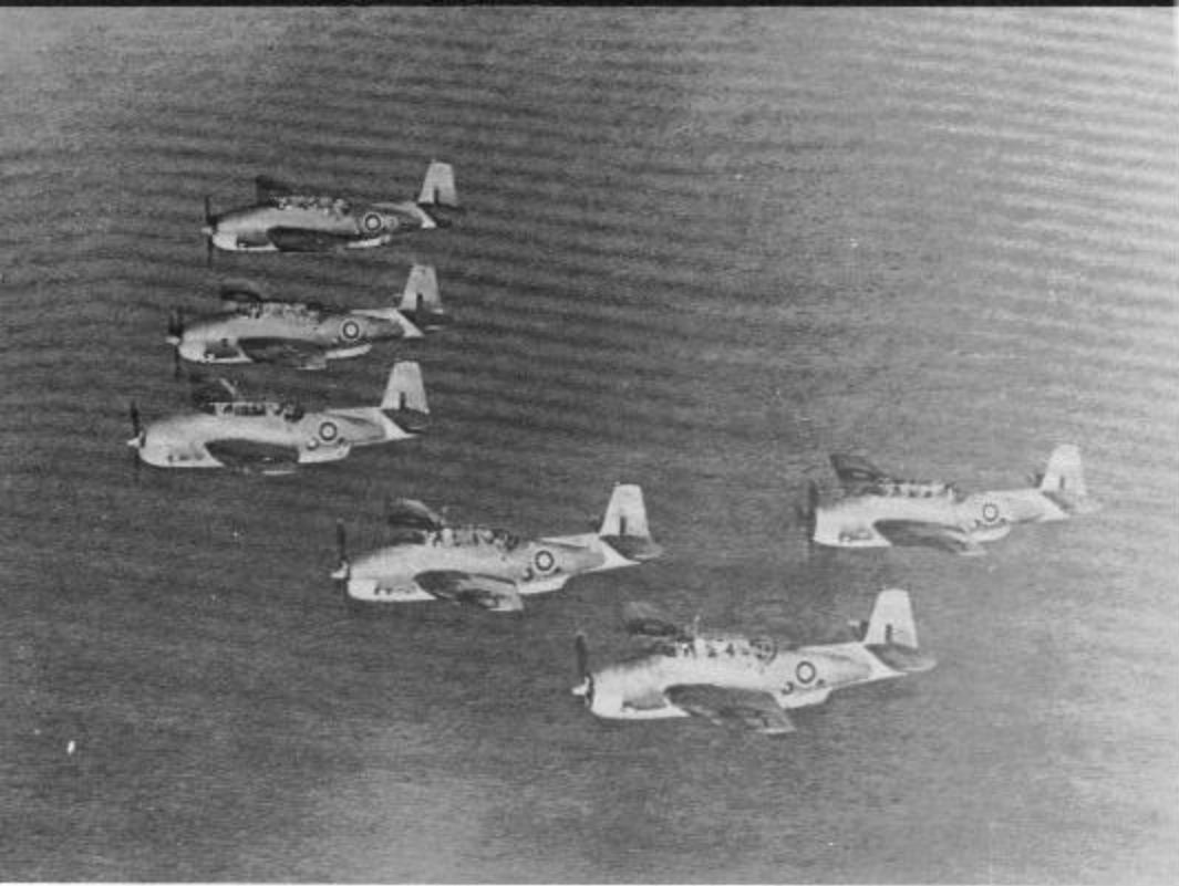
Six Fleet Air Arm Tarpon Mk IIs on patrol over the Atlantic. The bulged dome windows on the fuselage sides were the Tarpon's distinctive external feature. (Grumman)
