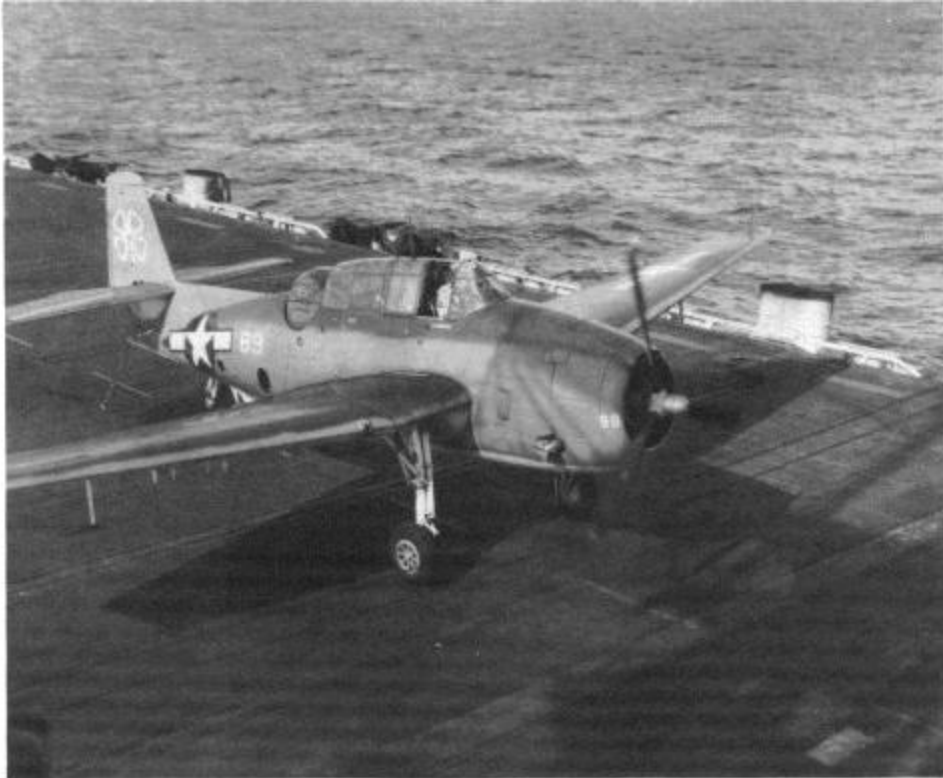
A TBM-1C of Composite Squadron Seventy-Six (VC-76) taxis clear of the arresting gear aboard USS PETROF BAY (CVE-80) on 30 January 1945. The .50 caliber wing gun blast tubes were usually sealed over with tape to keep out moisture, when the guns were fired the tape was torn away. (USN via David Lucabaugh)
