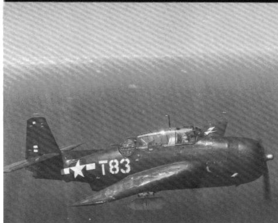
This early production TBM-3E of VMTB-234 from USS VELA GULF (CVE-111) still has the retractable tailhook. The ASP-4 surface search radar pod was found to be more practical than the earlier fixed radomes mounted on the wing of the TBM-3D and became a standard feature on TBM-3Es. (USN via David Lucabaugh)
