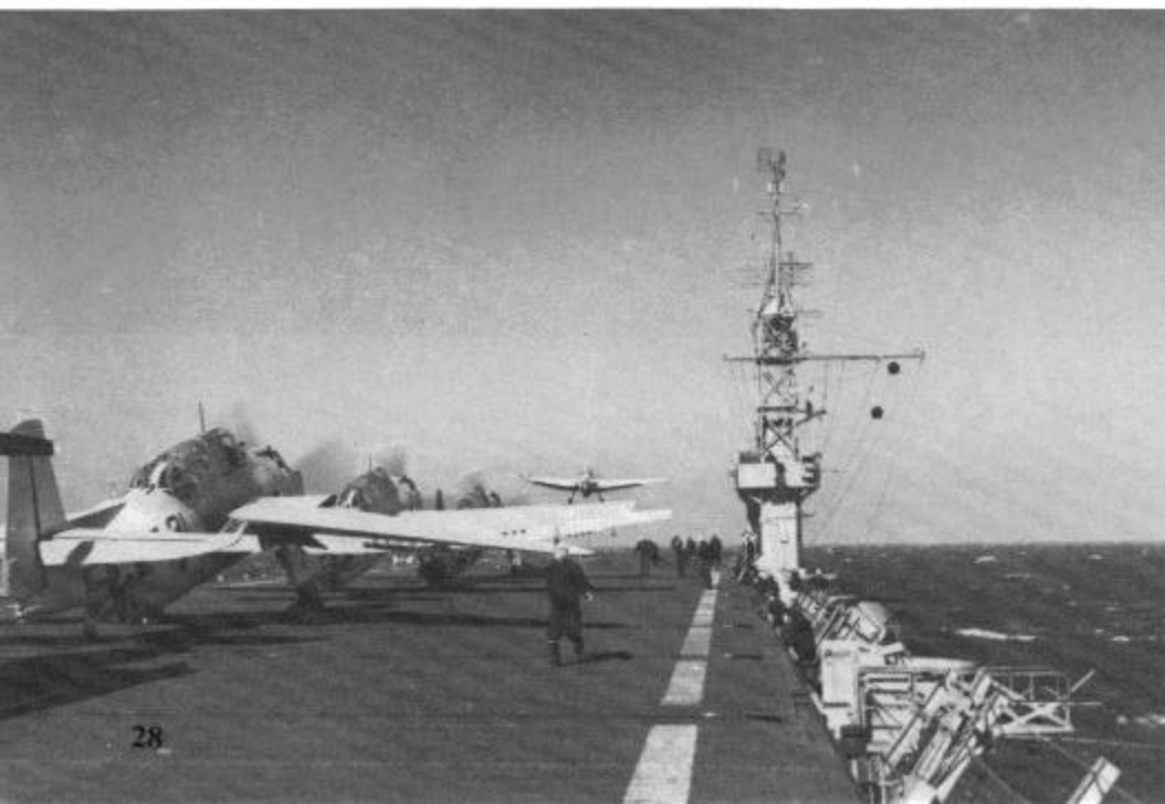
A TBF-1C unfolds its wings while waiting to take off from USS GUADALCANAL (CVE-60) during April of 1944. Anti-submarine Avengers were normally armed with Mk 54 depth bombs and rockets. The drag of the early Mk 4 rocket rails reduced the Avengers airspeed by 17 knots. (NAH-00173)
