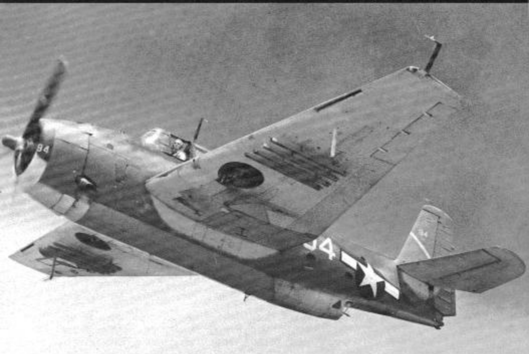
A TBM-1C of VT-10 flying from USS YORKTOWN (CV-10) carries four 70 inch British style Mk 4 rocket rails under each wing. The small 'T' shaped antenna under the inner port wing is a radio altimeter antenna. (USN via David Lucabaugh)
