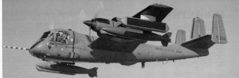
(Above) This OV-10B (60-15932) of the Army Flight Test Center was a developmental test aircraft used for the testing of the Aik/ALG-147 infrared suppression system (Hot Brick) during 1977. The Hot Brick system required an extra air intake which is visible just above the engine. (Grumman)
