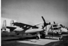
This National Guard OV-10 (87-1897) is now at the Greiner facility at Stuart, Florida for modernization and upgrading. The two teardrop shaped fairings on the lower forward fuselage are the attachment points for the SLAR pod. (Author)
