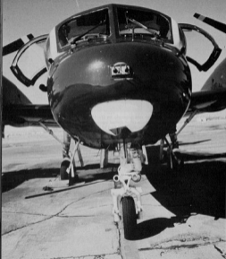
The FLIR turret installed on Customs Service Mohawks is made by Texas Instruments and has proven to be very effective in tracking low flying aircraft. The FLIR installation is similar to the installation used on the Navy's Grumman A-6E Intruder attack aircraft. (Vernon Skewer)
