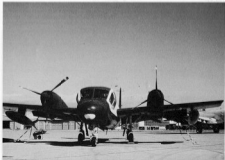
This OV-1 of the U.S. Customs Service is painted in Gloss Navy Blue and White. The white pod under the nose is a Forward Looking Infrared (FLIR) sensor turret used to track low flying aircraft. (Vernon Skewer)
