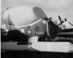
A number of early OV-10 Mohawks, such as these OV-10Bs, are in storage at Davis-Monthan Air Force Base and are available for future rebuild programs. These aircraft have all openings sealed with a plastic coating to protect them from dust and moisture. (Tom Garcia via Wayne Muzza)
