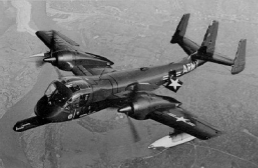
The first production OV-1B (59-2621) on a test flight from the Grumman test facility deploys its fuselage-mounted speed brakes. These speed brakes were later deleted as a weight saving measure on late production OV-1Bs. (Grumman)
