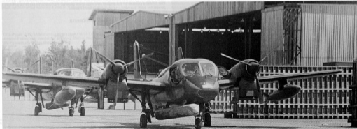
A crew chief cleans the windshield of an OV-10A that has been retrofitted with a nose camera and ILS antenna. The nine small Redhearts painted on the nose wheel door indicate that this OV-10 has taken nine hits from enemy ground fire. (Scott Rubke)
