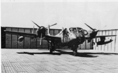
Spud 23, an OV-10C of the 131st SAC sits in its retirement at Phu Bai, Vietnam during 1970. While on the ground, the propellers were feathered and the side windows were normally left open to offset the heat in the cockpit generated by the canopy. (Scott Rubick)
