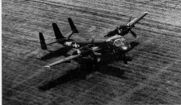
An OV-1B (62-5874) lands on a grass field during 1964. The OV-1B's outer wing panels were extended nearly three feet, increasing the wing span to 47 feet 10 1/2 inches. (Grumman)
