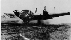
An OV-1C takes off from a dirt strip while on an Army field exercise during 1965. The Mohawk has excellent short field capabilities thanks to the large flaps mounted inboard of the engines and auxiliary flaps located between the main flaps and the ailerons. (U.S. Army Military History Institute)
