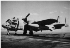
This OV-10 parked on the ramp at El Paso, Texas on 26 February 1963, is assigned to the 124th Military Intelligence Battalion. The propellers are feathered, a standard practice for Mohawks when parked, to prevent them from windmilling. (T M J. Kusiba)
