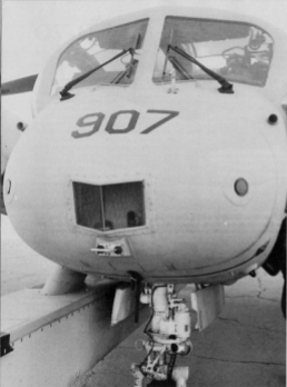
The flat glass panels on the nose of this OV-1D are the camera windows for the KA-60C panoramic camera. The loop antenna under the glass panels is for the AN/ARN-58 glide slope receiver, while the two round sensors on each side of the nose are antennas for the AN/APR-25 Radar Homing and Warning (RHAW) receiver. (Dick Divold via Cobra Company)
