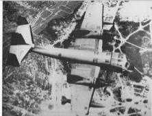
An OV-1 of the 131st Surveillance Aviation Company on patrol over Vietnam during 1971/72. The forward portion of the engine cowlings were painted Flat Black to serve as anti-glass panels for both the pilot and observer. (Scott Rutke)
