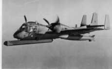
This OV-1D (87-18896) of the 73rd Combat Intelligence Company (CIC) during 1969 is carrying a pair of the rarely used 300 gallon ferry drop tanks in place of the 150 gallon drop tanks normally carried on the Mohawk. (Grunman)
