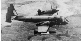
An armed OV-10A of the 131st SAC, Nighthawks, on patrol over the Vietnamese country side. The White bar down the fuselage spine was a recognition marking to make spotting the Mohawk easier for higher flying fighter aircraft. (Scott Rubke)
