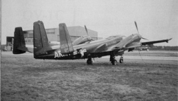
(Above) This OV-1C (61-2686) at Fort Eustis, Virginia during March of 1966 carries photo flare dispensers on the wing trailing edge next to the fuselage. The dispenser can be carried singly or in pairs with each flare dispenser carrying fifty-four photo flash flares. (Author)
