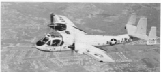
The first YAO-1AF Mohawk (57-6462) on a test flight over Long Island, New York during the Summer of 1958, had the fuselage covered with yarn tufts to reveal the air flow over the fuselage. The eyebrow windows and small rear cockpit windows were deleted on production Mohawks. (Grumman)
