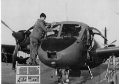
A crew chief cleans the windshield of an OV-10A that has been retrofitted with a nose camera and ILS antenna. The nine small Redhearts painted on the nose wheel door indicate that this OV-10 has taken nine hits from enemy ground fire. (Scott Rubke)
