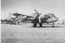
This RV-1D (68-15964) carries a Quick Look I ECM pod on the outboard wing pylon suspended from an Aero 15C stores rack. The Quick Look I system featured a monitor in the cockpit which permitted real time readout of intercepted signals. (Grumman)
