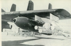
This JOV-1A Mohawk is configured for night armed reconnaissance with an SUU-12 .50 caliber machine gun pod on the center pylon and multiple ejector racks, each armed with nine Mk 24 flares, on the inboard and outboard pylons. (Army Aviation Museum)
