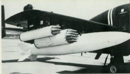
Mohawks in Vietnam were usually armed with seven-shot XM-157 rocket pods and nineteen-shot XM-150 rocket pods, both of which carried 2.75 inch rockets. The underwing weapons pylons on the Mohawk were a carry-over from the original Marine specification which had called for a close air support capability. (Army Aviation Museum)
