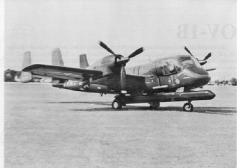
This Mohawk (59-2621) was the first OV-1B to roll off the production line. The OV-1B Mohawk had no provisions for dual flight controls or underwing armament, carrying only 150-gallon drop tanks on the underwing pylons. The SLAR (side looking airborne radar) unit carried on the OV-1B was the Motorola AN/AP5-9A. (Grumman)
