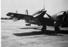
When armed with a pair of seven-shot and a pair of nineteen-shot rocket pods on the wing stations, a total of fifty-two 2.75 inch FFAR rockets could be carried by the Mohawk. This JOV-1A Mohawk is assigned to the 73rd SAC based at Yung Tau, Vietnam during October of 1966. (Author)
