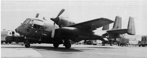
[Above] The large blade antenna just behind the cockpit of this OV-10 of the 73rd OIC is for the UHF/FM radios. The small flat antenna on the fuselage spine is an Automatic Direction Finder loop antenna. These are just part of the extensive onboard communications equipment fitted to the OV-10. (Grummer)
