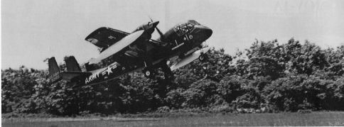
An OV-10A takes off from a grass airstrip during demonstrations of the Mohawk's Short Take Off and Landing (STOL) capabilities. The aircraft is in the early Gloss Olive Drab scheme with high visibility markings used prior to the Vietnam war. The 150 gallon drop tanks are in Gloss White. (Grunner)
