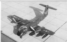
This wooden mockup of the Mohawk, built during the Summer of 1957, has the original T tail configuration, snow skis, 156 gallon drop tank, and proposed armament pylons. (Grumman)
