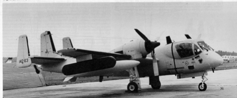
(Above) This OV-10B (60-15932) of the Army Flight Test Center was a developmental test aircraft used for the testing of the Aik/ALG-147 infrared suppression system (Hot Brick) during 1977. The Hot Brick system required an extra air intake which is visible just above the engine. (Grumman)
