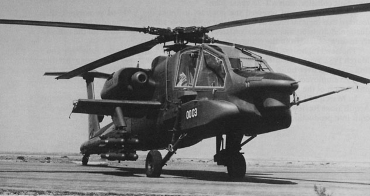
The third YAH-64 prototype, AV-03 (Air Vehicle 03, 77-23256) was configured with Hellfire anti-tank missiles on modular launchers. The early prototypes featured a T-tail horizontal stabilizer configuration and flat sided canopies. (U.S. Army)
