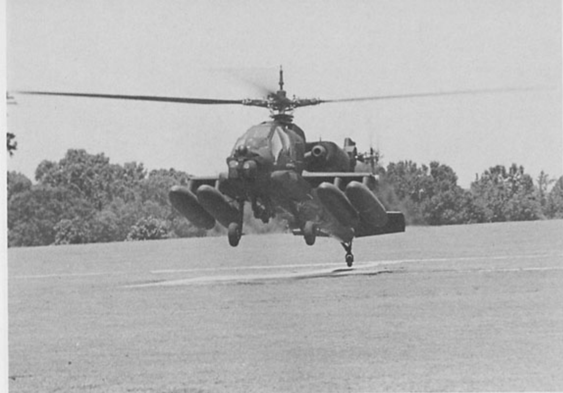
The test AH-64A touches down at Fort Rucker, Alabama at the end of the long range validation flight from Mesa, Arizona. The flight was made with only one stop, thanks to the added range afforded by the four 230 gallon long range tanks. For extended range search and destroy missions, two tanks and Hellfire or other missile systems could be fitted. (U.S. Army)
