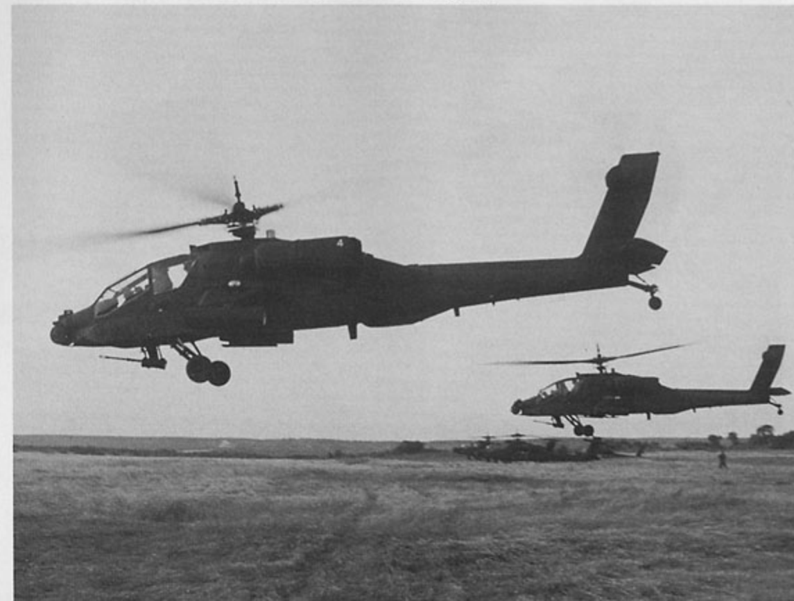
A pair of fully armed Apaches take off from a grass field on an early morning training mission near Fort Hood, Texas. Both aircraft are equipped with the Disco Light infrared (IR) jammer unit behind the main rotor masts. (McDonnell Douglas)
