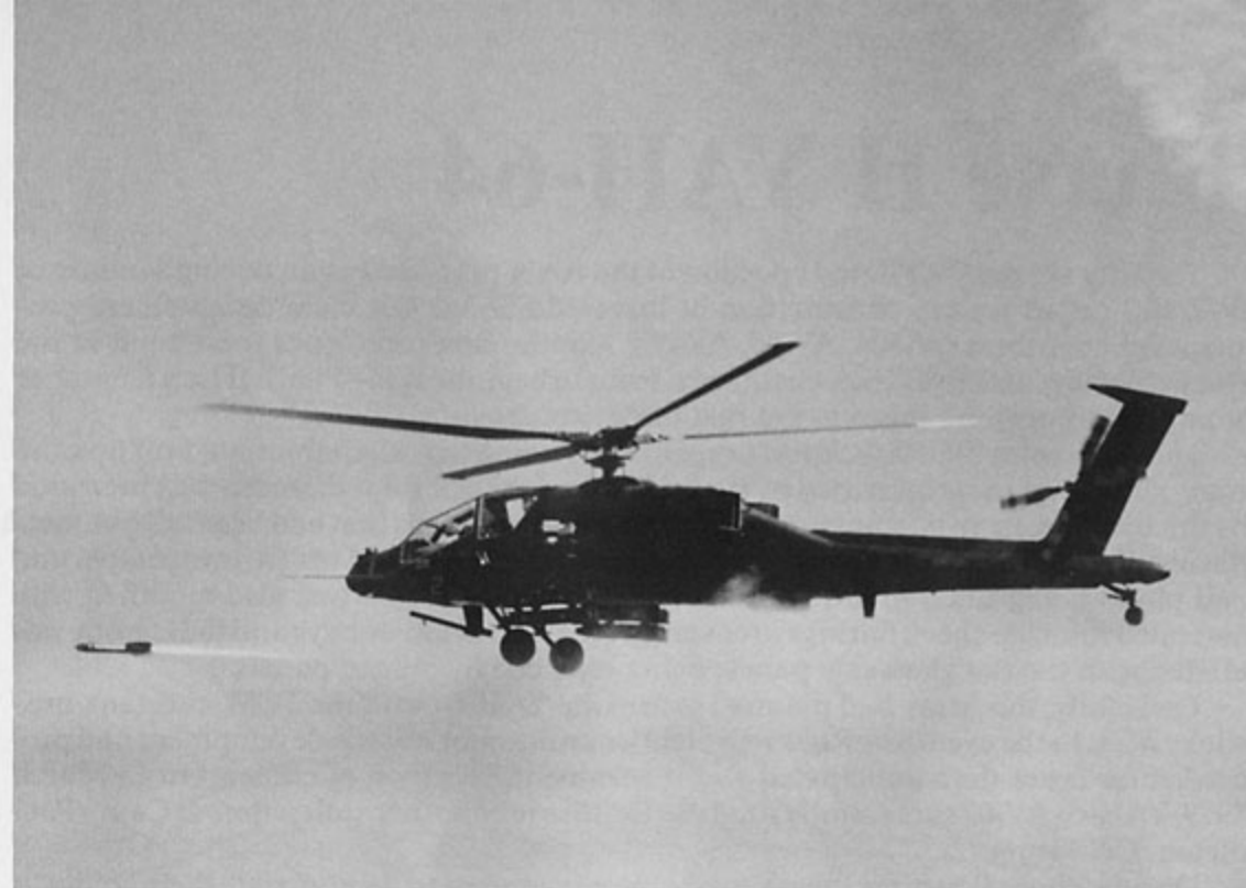
The second YAH-64 prototype (AV-02 73-22249) was the first to actually fire a Hellfire missile. The first launch took place during missile firing trials held at Camp Pendleton, California. The 30mm cannon under the fuselage was a dummy installation. (McDonnell Douglas)
