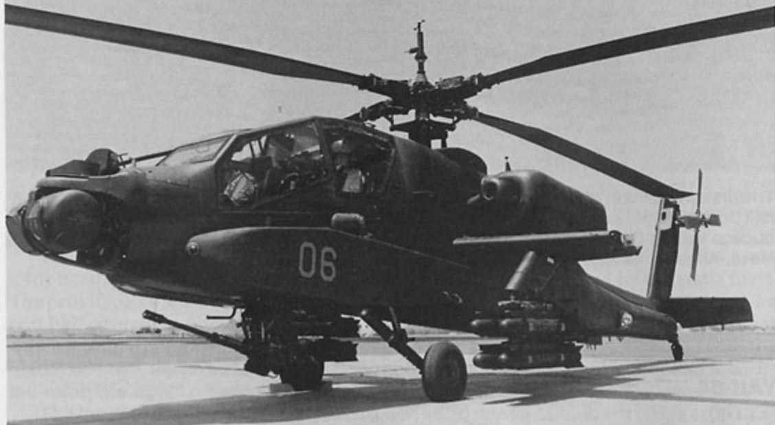
The sixth YAH-64 prototype (AV-06 77-23259) was the first to be fitted with the low mounted stabilator. AV-06 was also fitted with a production TADS/PNVS nose turret, an Air Data Sensor (ADS) probe on the rotor mast above the blades, and extended side sponsons. (Rockwell)
