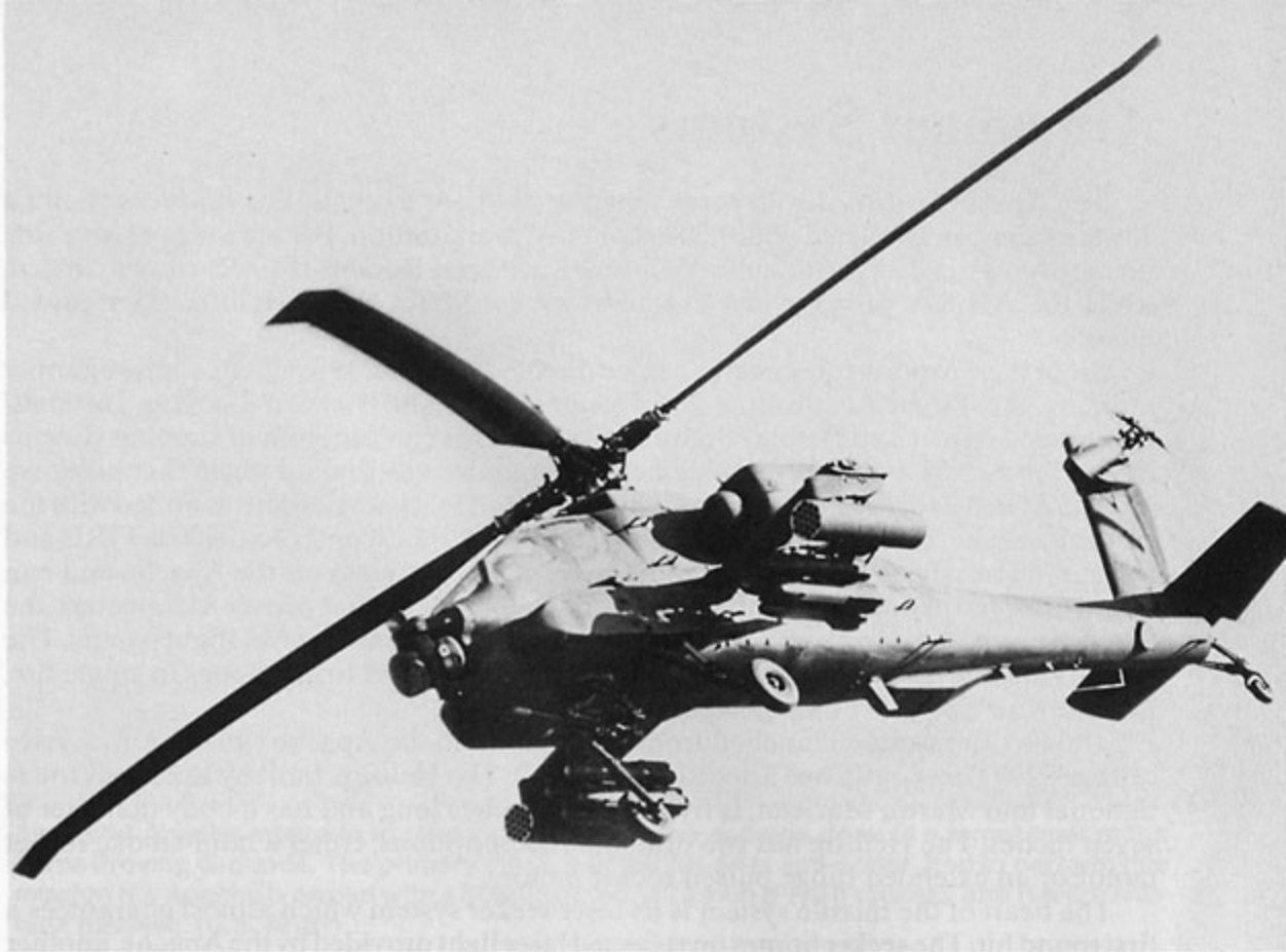
This Apache is attached to the 145th Aviation Brigade at Fort Rucker, Alabama and is armed with eight Hellfire missiles, two 2.75 inch rocket pods and a 30 mm cannon. The nose sensor turret has been rotated to port and depressed to track a target below and left of the Apache. (U.S. Army by Frank Sullivan)
