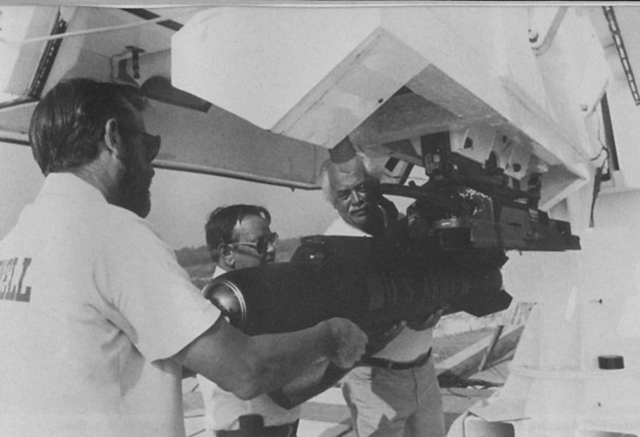
Rockwell employees install a production Hellfire onto a modular launcher rail on a test hardstand at Eglin Air Force Base, Florida, where initial test firings of the Hellfire took place. The test hardstands are designed to handle the wide variety of missile types tested at Eglin. (Rockwell)
