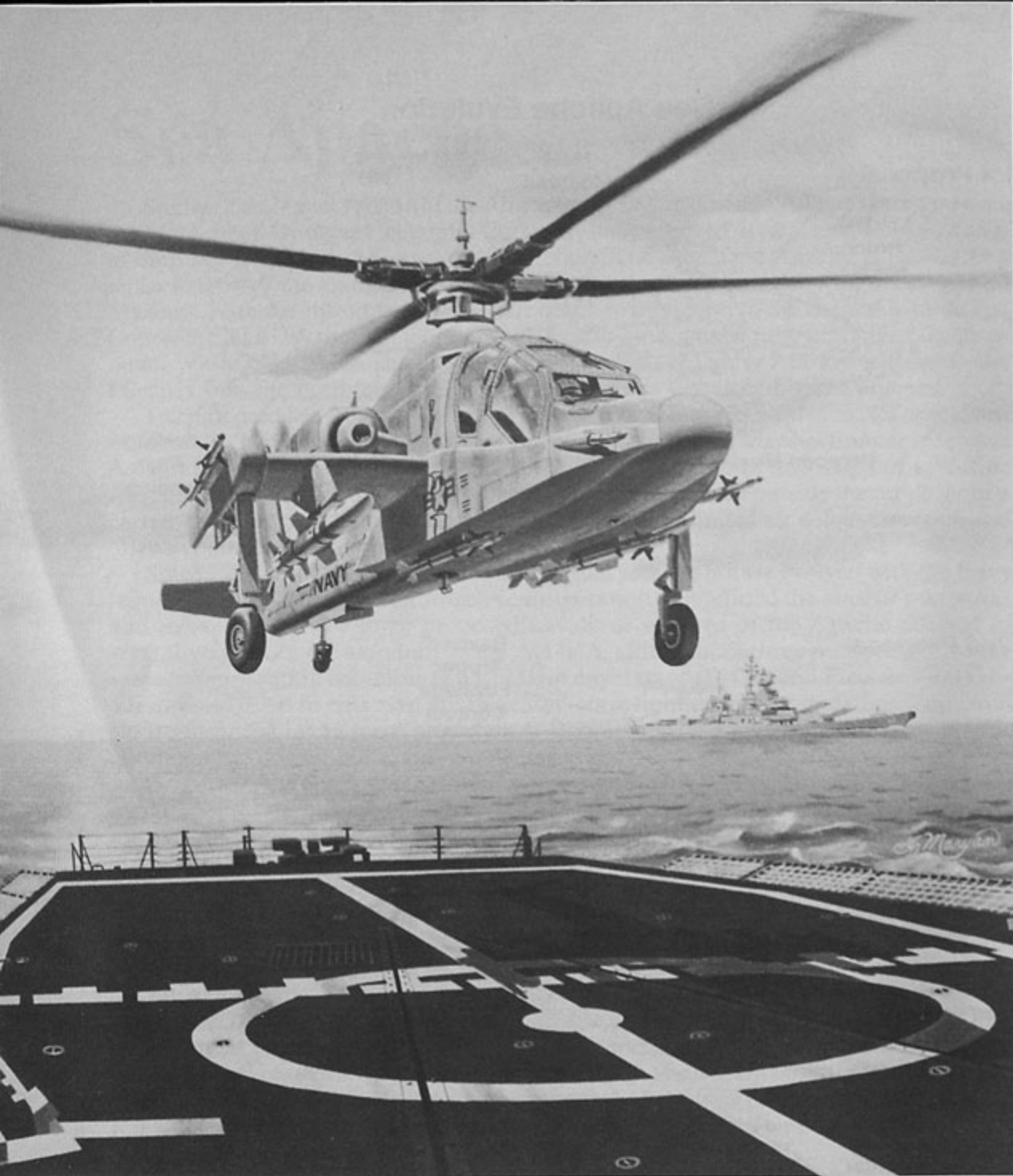
In response to Navy requirements, McDonnell Douglas modified the Sea Apache proposal with a new nose area housing upgraded electronics, relocated landing gear, and the cannon deleted. The Sea Apache has also been nicknamed Gray Thunder because of its overall Light Gray camouflage scheme. (McDonnell Douglas)
