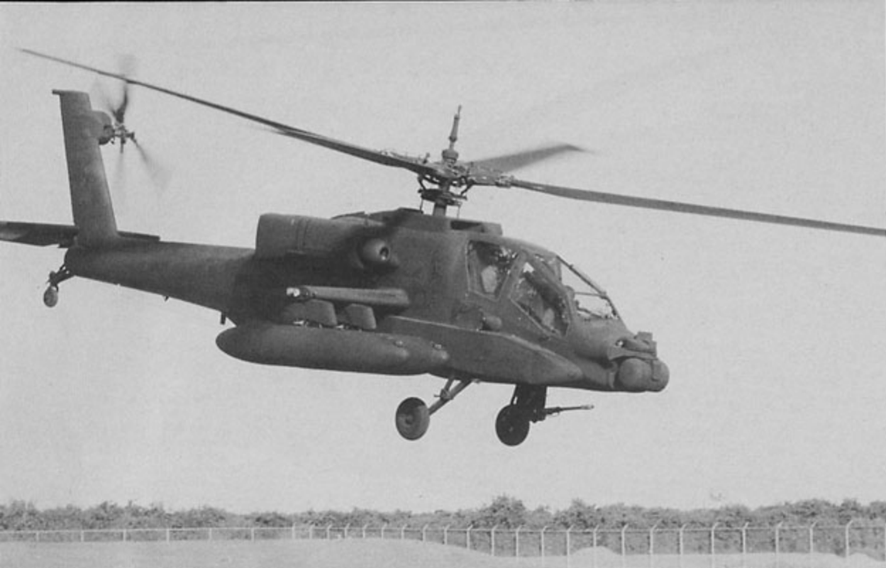
An AH-64A (85-23789) takes off on a practice long-range flight fitted with four 230 gallon underwing fuel tanks. The 230 gallon tanks are made of Kevlar, the same lightweight armor material that is used to protect the crew and other vulnerable areas of the AH-64. (McDonnell Douglas)
