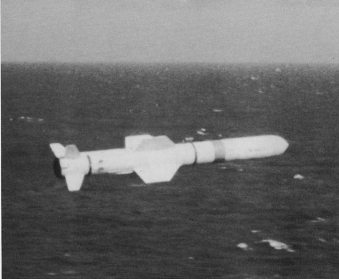
The Harpoon is an air breathing, turbo-jet engine powered, all weather, over-the-horizon anti-ship missile. The Harpoon, like the French Exocet (AM.39), is a low level cruise type missile that employs active radar guidance and a high explosive warhead. (McDonnell Douglas)
