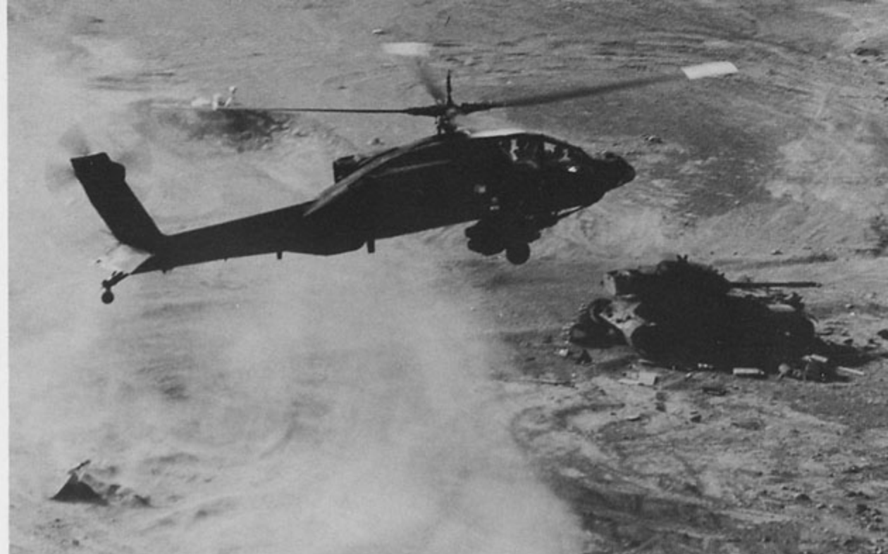
An AH-64 Apache moves in to take a close look at the damage done to a target tank at the Yuma Proving Grounds. The primary mission of the AH-64 is anti-armor, and to perform this mission the Apache is armed with a 30mm cannon, 2.75 inch (FFAR) rockets, and Hellfire anti-tank missiles. (U.S. Army)
