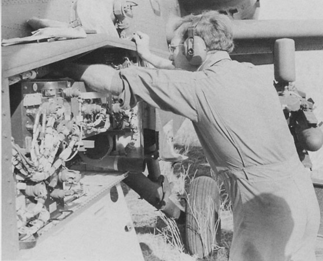
Most minor maintenance can be accomplished in the field from ground level. This crewman is working in the forward avionics/electronics bay which contains components of the fire control system. The Apache has miles of wiring connecting the various electronic systems and sub-systems. (U.S. Army)
