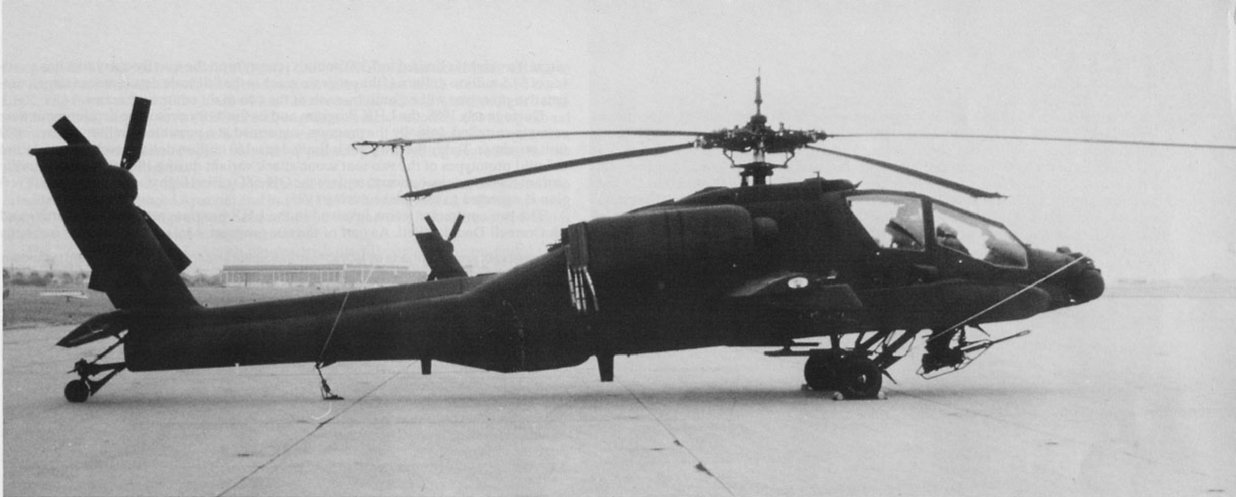
This late production Apache (86-9002) is also equipped with the Wire Strike Protection System. The WSPS uses deflectors and cutters to protect the Apache from damage caused by one of the major dangers to low-flying helicopters, — telephone and electrical power lines. (China Clipper Photo)
