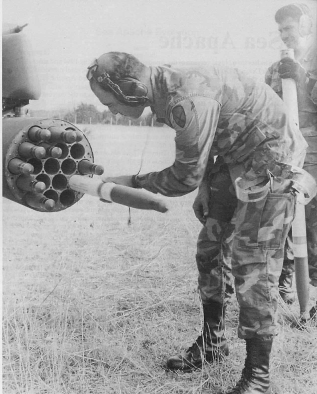
(Above) Ground crewmen load 2.75 inch FFAR rockets into the port rocket launcher of an AH-64A. The crewmen wear radio headsets to communicate with the aircrew and for noise protection. These rockets have Blue warheads to signify that they are practice rounds. (U.S. Army)
