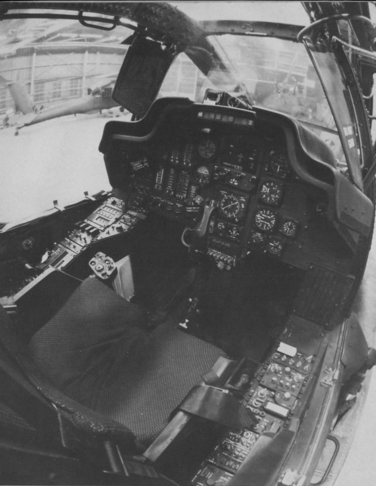
The pilot's instrument panel of the AH-64A is equipped with a full range of analog and digital instruments along with a video display unit (VDU) in the panel center. The VDU displays altitude, speed, attitude, and weapons control and status information. A transparent blast shield is between the pilot and copilot/gunner to protect them from shell fragments. (McDonnell Douglas)
