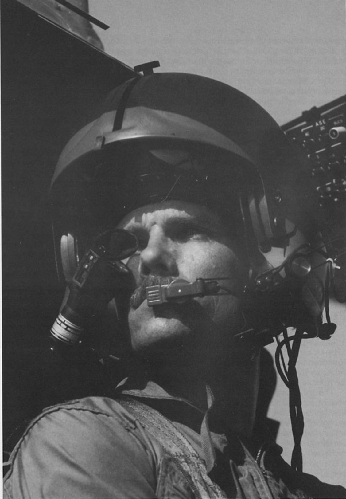
Both pilot and copilot/gunner are provided with Helmet Display Units (HDU) that, when placed in front of the right eye, display selected video and/or symbology to each crew member. The HDU consists of a one inch cathode ray tube mounted in a high impact plastic barrel. (Martin Marietta)
