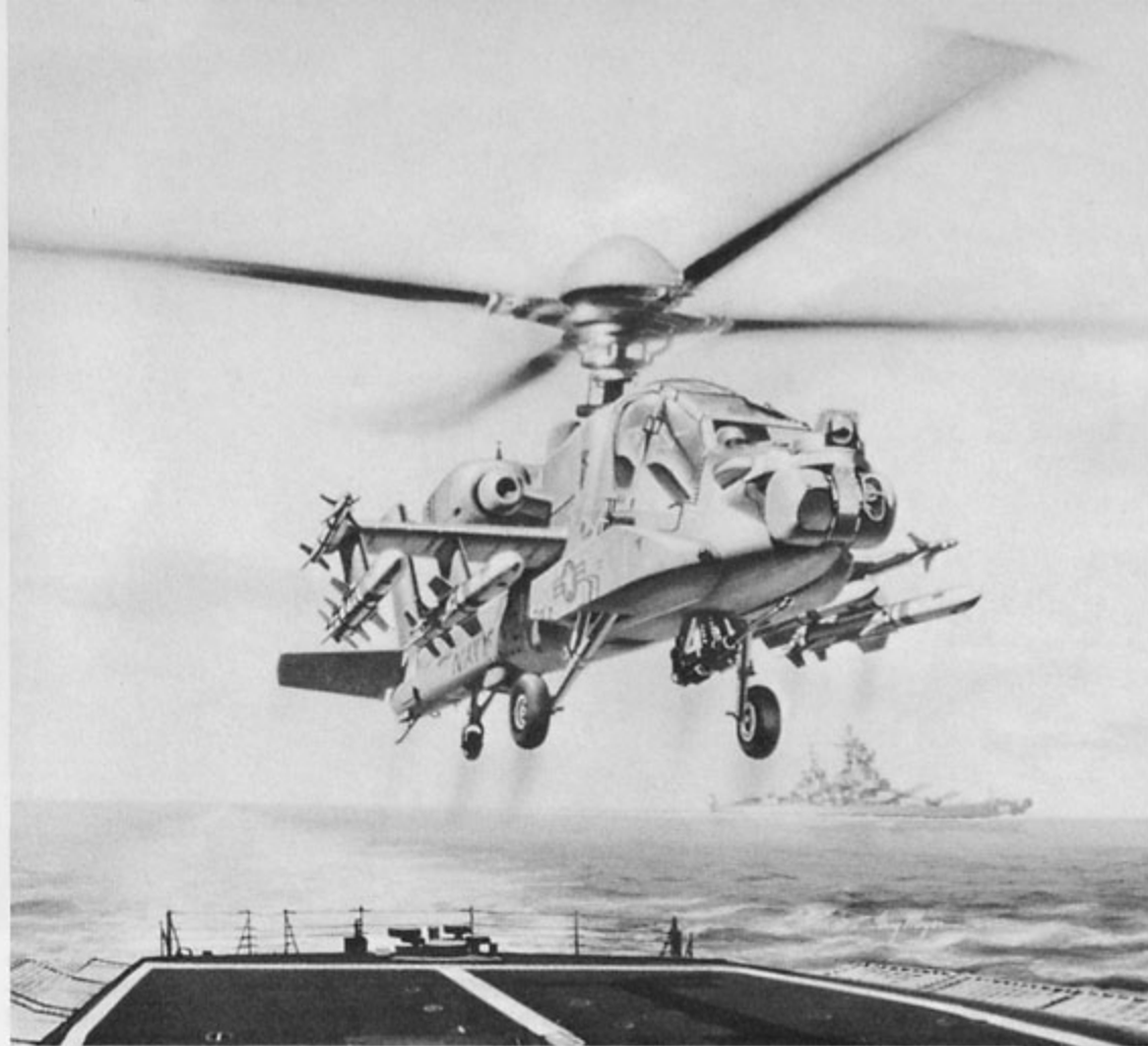
The U.S. Navy has shown an interest in acquiring the AH-64A in a navalized form to replace the AH-1 Sea Cobra. McDonnell Douglas' initial design study was a modified AH-64A equipped for duty aboard ship and armed with Sidewinders on each wing tip and four Harpoon anti-ship missiles. (McDonnell Douglas)
