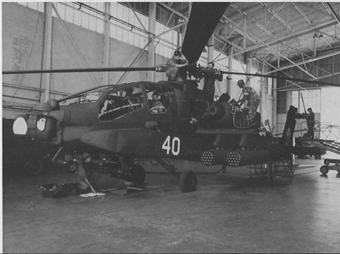
Ground maintenance personnel inspect the engines, rotor system, instruments and armament systems on this AH-64A (buzz number 40) inside one of the maintenance hangars at Fort Rucker. Later the buzz number will have a letter code added to it. (U.S. Army)
