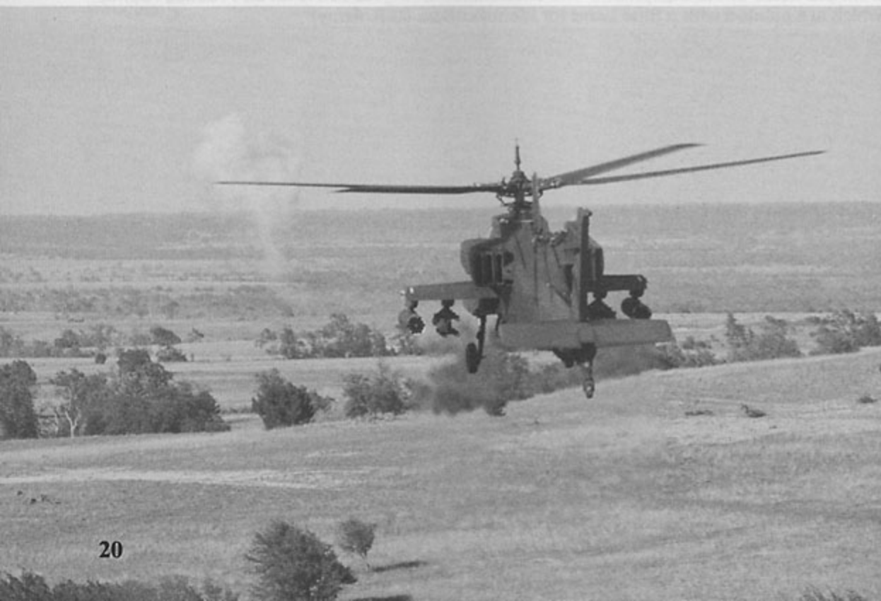
This AH-64A is firing rockets from a hover. Crews report that the Apache is a very effective and steady platform for launching rockets. The smoke cloud ahead of the Apache is from one of the rockets. (McDonnell Douglas)
