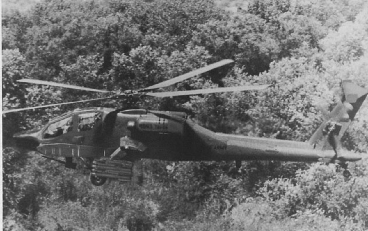
In an attempt to reduce dynamic vibrations in the tail area, the horizontal stabilizer was given a reverse taper and fitted with end plates. This modification did not produce the desired improvement and the tail was later completely redesigned. (U.S. Army)
