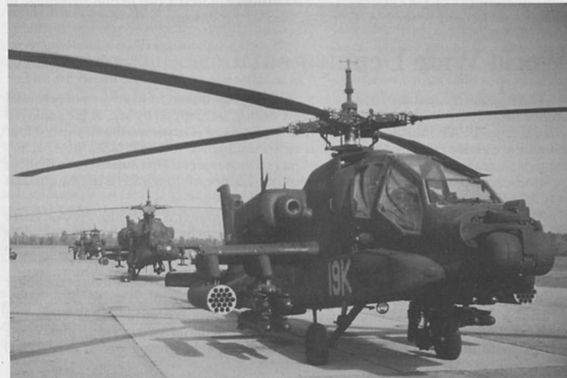
Eck Army Airfield is used as a stage field for AH-64 training. The field is used primarily for practice landings and takeoffs, instrument approaches and other flight training associated with the Apache program. The TADS/PNVIS turret on the Apache in the foreground has been rotated to the stowed position. (Author's Collection)
