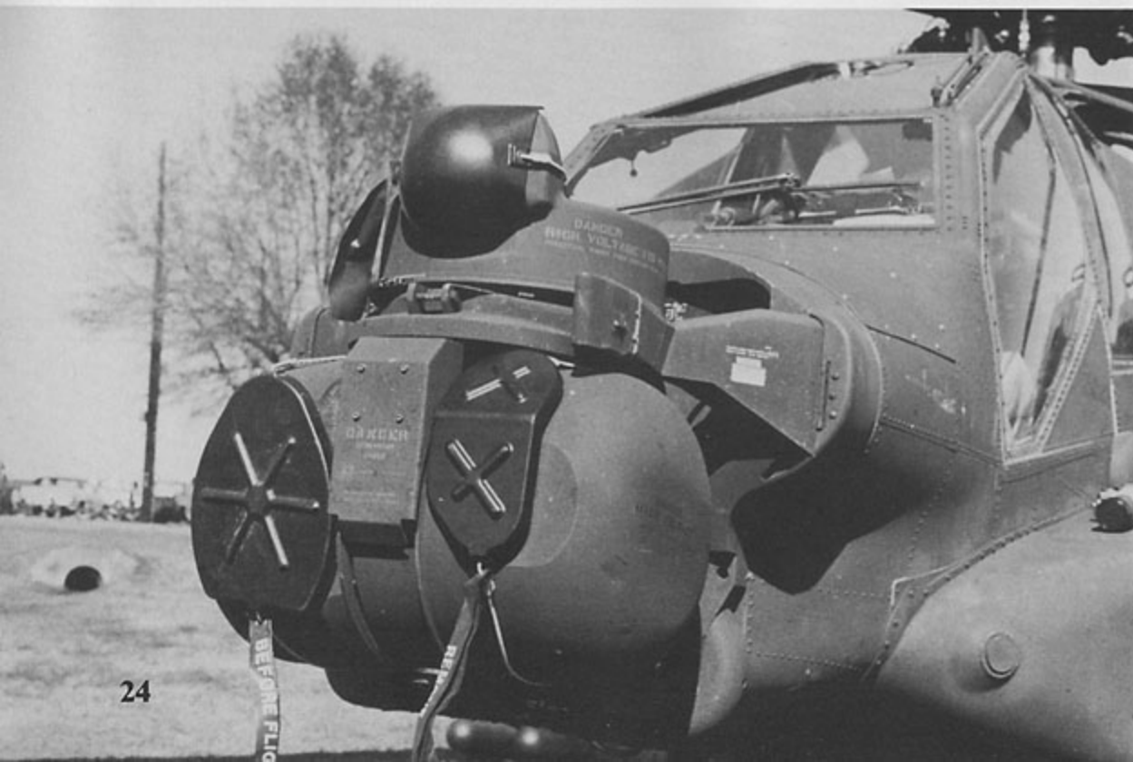
The nose of the AH-64A houses the TADS/PNVS turret. TADS is an acronym for Target Acquisition Designator System, while PNVS stands for Pilot's Night Vision Sensor. The TADS occupies the lower section of the turret while the PNVS is mounted above it. (Martin Marietta)
