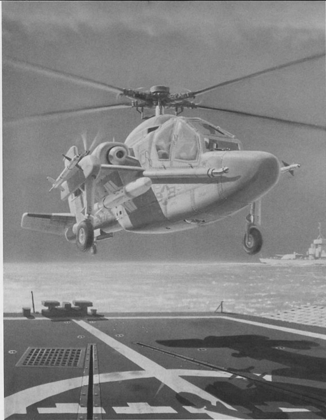
The final proposal for the Sea Apache calls for a deepened fuselage, a further modification to the nose section to incorporate a radar from an F/A-18 Hornet, and an inflight refueling probe. The projected missions for the Sea Apache include; anti-shiping, anti-air, combat search and rescue escort, naval gunfire spotting and forward air control. (McDonnell Douglas)
