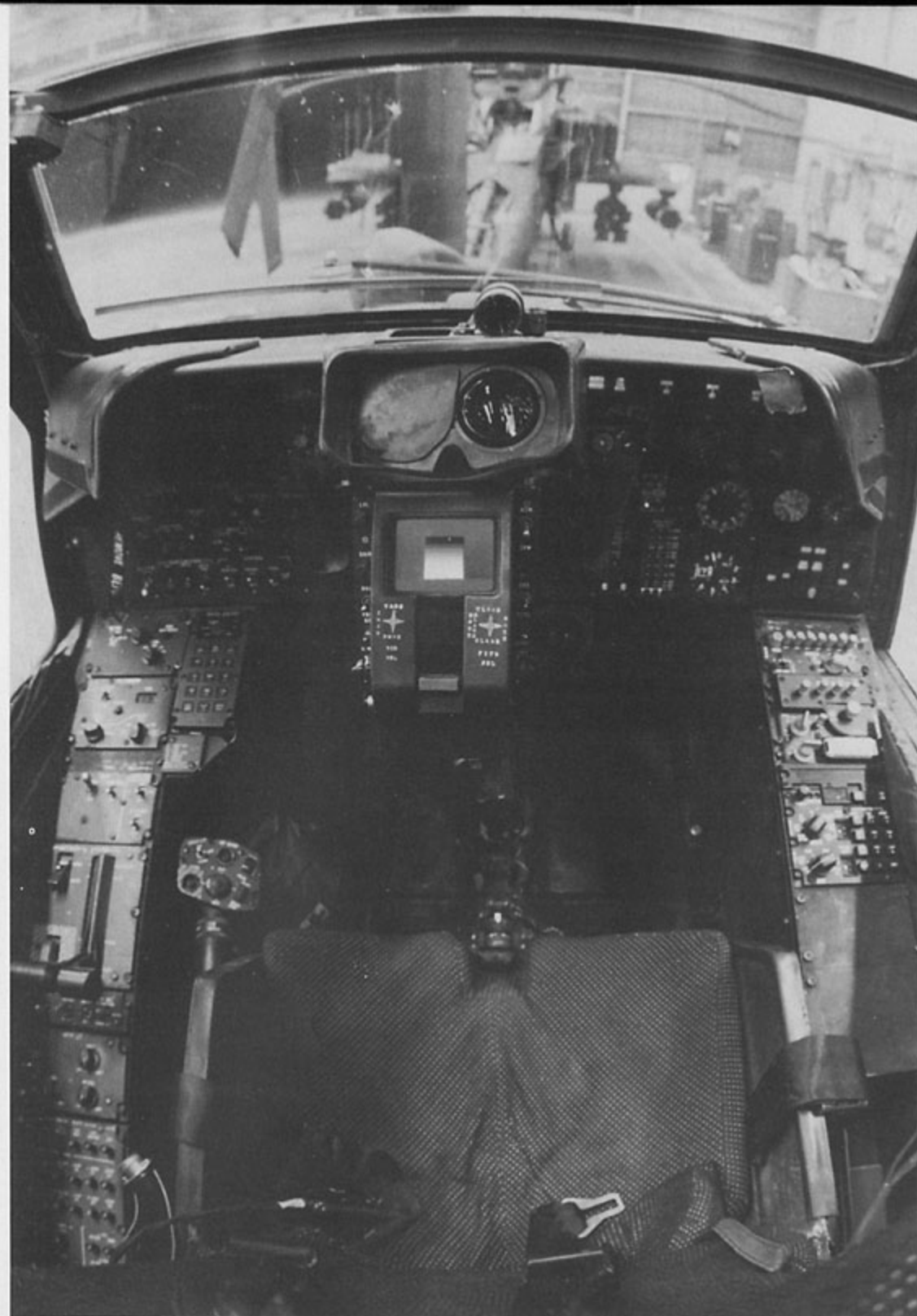
The copilot/gunner's cockpit of the AH-64 is dominated by the multi-purpose sight system in the center of the instrument panel. The sight system contains an optical relay tube and handgrips with small circular "coolie hat" switches. The copilot/gunner can operate the complete weapons system with this sight. (McDonnell Douglas)
