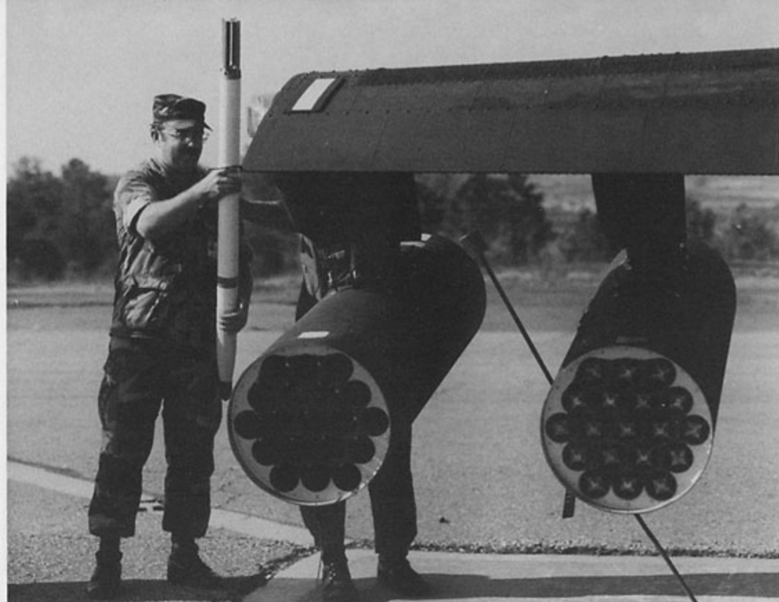
Army armorers load the port outer rocket pod of an Apache with 2.75 inch folding fin rockets. The AH-64A can carry up to seventy-six of these rockets in four nineteen shot underwing pods. The rockets have an effective range of 6,000 meters and can be fitted with a variety of warheads. (U.S. Army)
