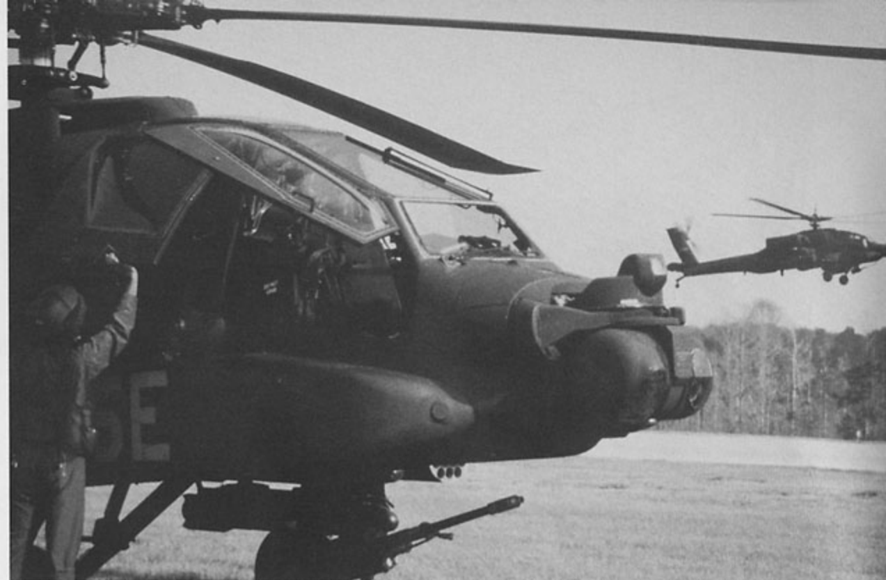
An Army aviator prepares to man his AH-64A at Eck Army Air Field, Alabama. Both pilot and copilot/gunner enter the aircraft through the opening canopy panels on the starboard side. During Apache training, flight time is interspersed with time in the Combat Mission Simulator (CMS). (Author's Collection)
