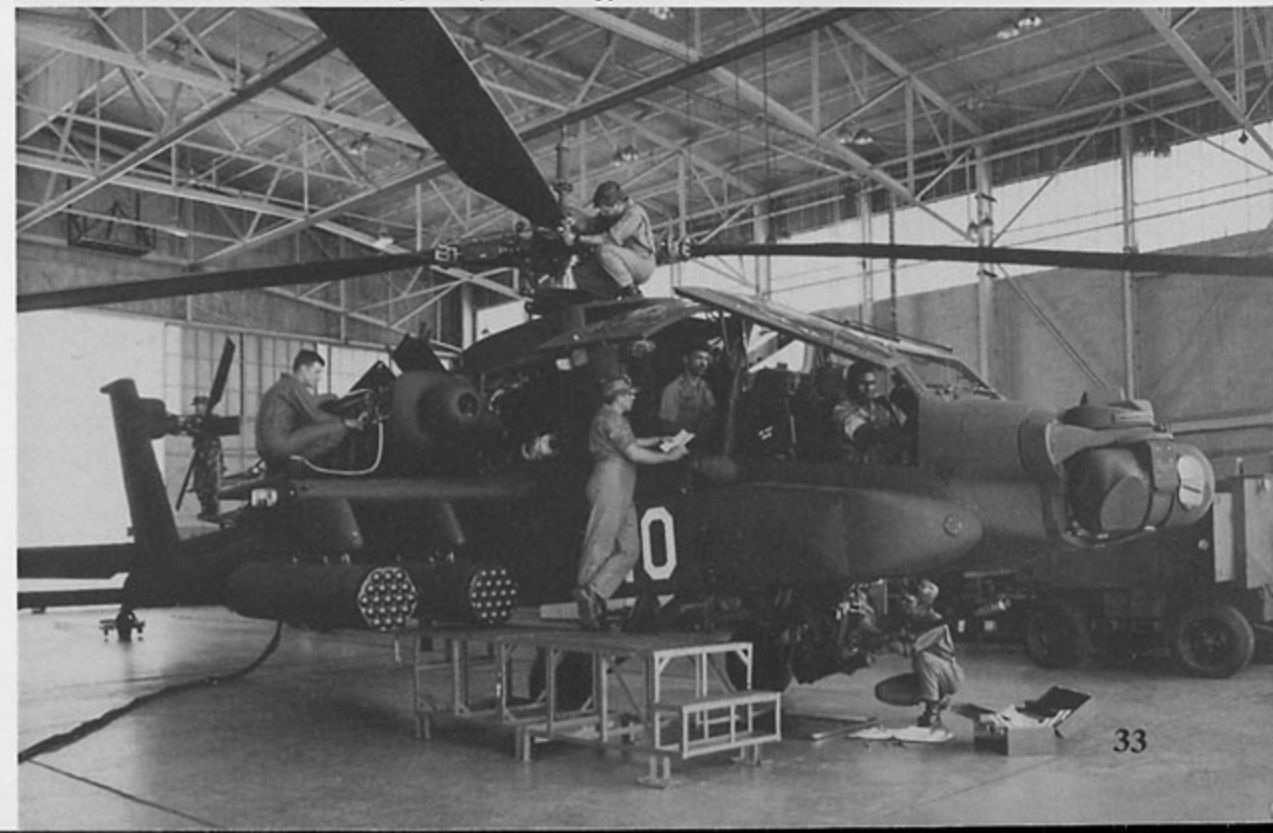
This AH-64A (40) is undergoing periodic maintenance inspection in one of the hangars at Fort Rucker. The Apache was designed to operate with the troops in the field, and most major mechanical and electronic components are modular to ease maintenance and reduce the time the aircraft is down for repairs. (U.S. Army)
