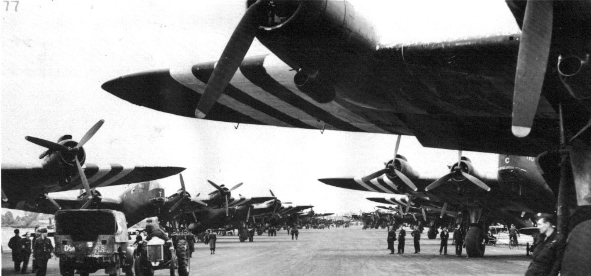
Stirling Mk IVs of an unidentified squadron line up on the taxiway of a British airfield just prior to commencing D-Day operations. The Black and White Invasion markings were carried by all Allied aircraft involved with D-Day except four-engined strategic bombers.
