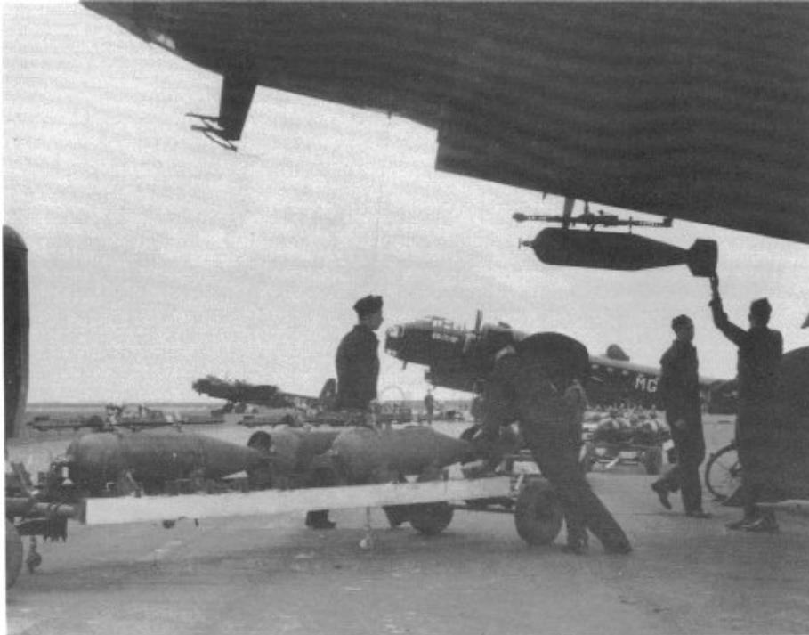
Ground crewmen hoist 500 pound bombs, fitted with extended nose fuzes, into a Stirling Mk I of No 7 Squadron. The pitot tube mast covers are still in place. A number of aircraft were lost due to failure to remove these covers before take off. With the covers in place, the pilot had no way of knowing his airspeed.
