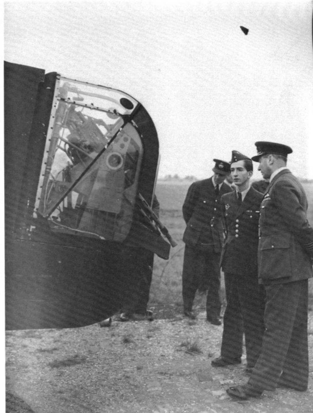
King Peter of Yugoslavia (middle) inspects the tail turret of a Stirling Mk I. The Frazer Nash FN20A rear turret was unique to the Stirling. In their fully depressed position, the barrels of the four .303 machine guns barely protrude beyond the cartridge ejection chutes on the bottom of the turret.
