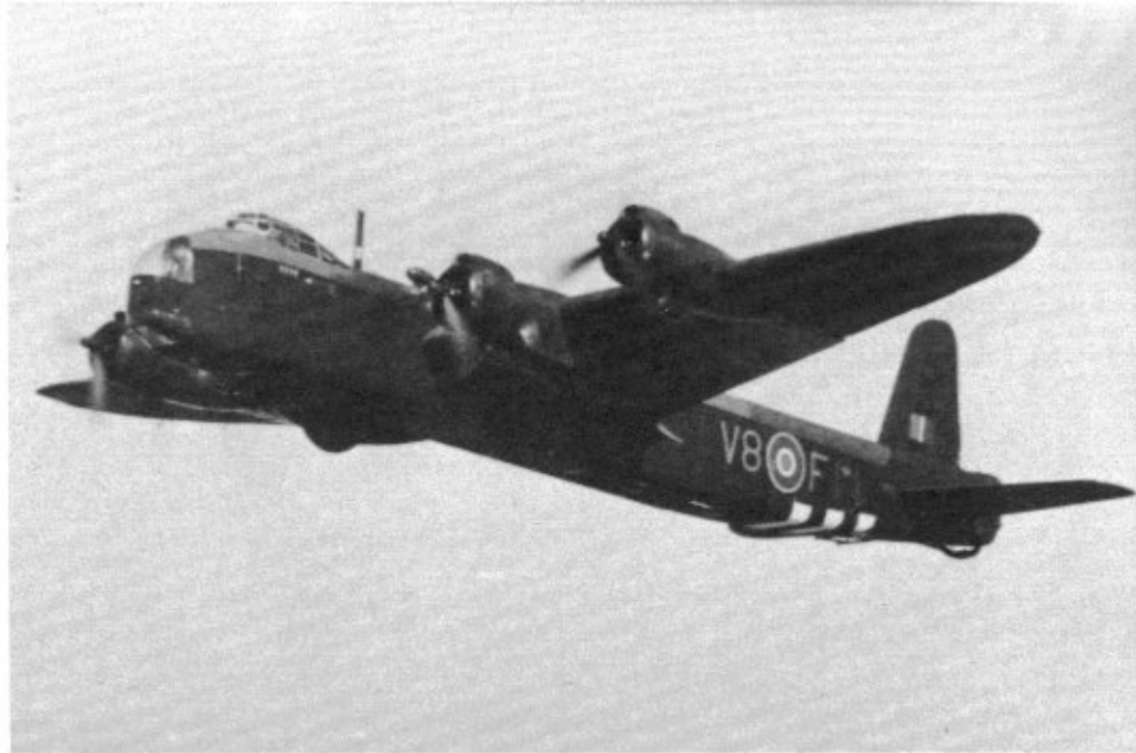
This Stirling MK IV of No 570 Squadron has the early Perspex nose cap and carries under-fuselage D-Day Black and White invasion stripes. The fuselage side code has a rounded style 8 which was later changed.
