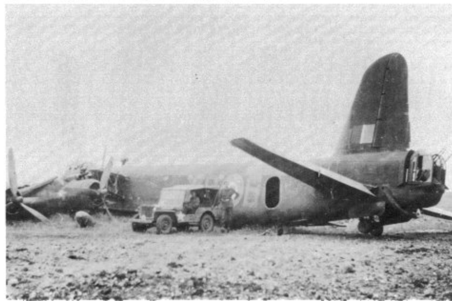
This Mk IV of No 190 Squadron was one of the casualties of the Arnhem operations on 21 September 1944. The aircraft lost its port wing in the crash landing and the side canopy of the rear turret appears to have been damaged by enemy fire.
