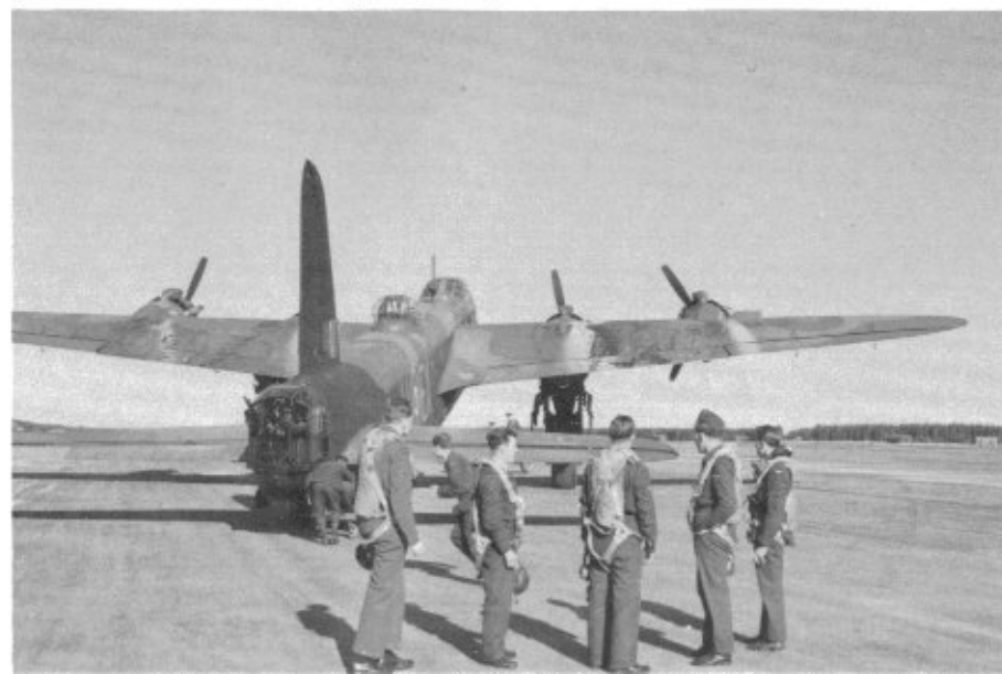
An aircrew prepares to board a Stirling Mk III of No 199 Squadron at Lakenheath during 1944. The wing surfaces are streaked with oil thrown back by the engines and the light areas on the wing upper surface are engine exhaust strains. The absence of heavy flight clothing suggests that this is to be a non-operational flight.
