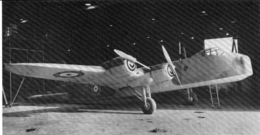
The S31/M4 was a half scale Stirling prototype used to test the aircraft's aerodynamics. The single stage undercarriage fitted to the S31 was later replaced with a two stage undercarriage that was adapted for the second prototype and all production Stirlings.
