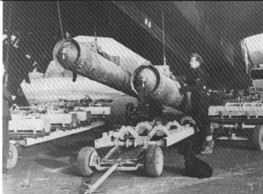
A pair of 2,000 pound light case bombs are hoisted into the narrow bomb bay of a Stirling Mk I of No 7 Squadron. The narrow width of the bomb bays limited the carriage of high explosive bombs to those of no more than 2,000 pounds, since larger weapons were too wide to fit in the bay. The cases on the bomb trolleys contain incendiary clusters.
