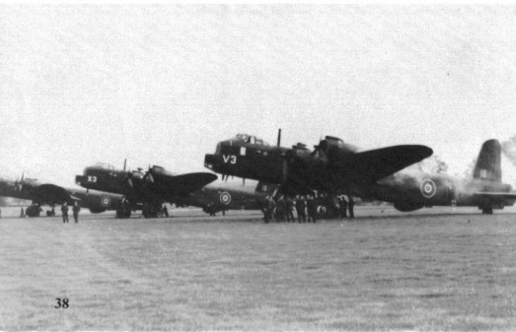
A trio of Stirling Mk IVs of the Central Navigation School (Summerside) start their engines on a Canadian airfield during June of 1944. The fairing under the rear fuselage houses the H2S radar antenna. The Stirling in the foreground is believed to be LK589 which returned to Britain and served with Nos 295 and 570 Squadrons at Rivenhall.
