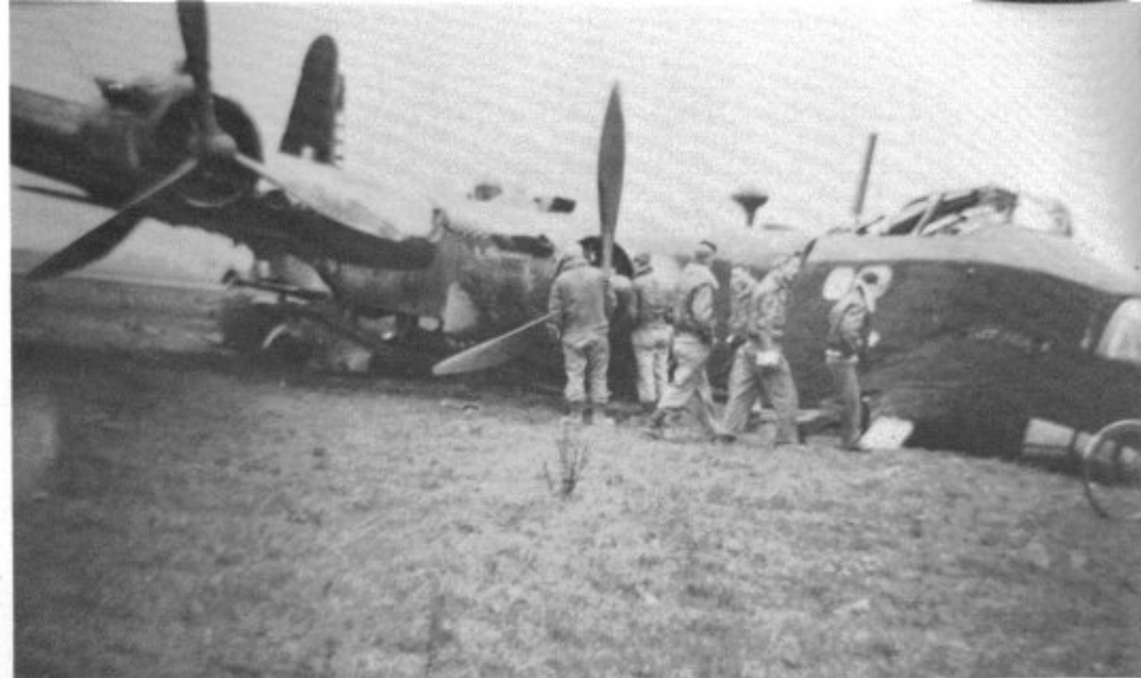
This Stirling Mk I (BK601) was one more victim of the Stirling's weak undercarriage. The aircraft had been on active service with Nos 214 and 149 Squadrons, before being assigned to No 1657 HCU. The aircraft was on a visit to the USAAF 94th Bomb Group base at Rougham on 28 January 1944, when the accident occurred.
