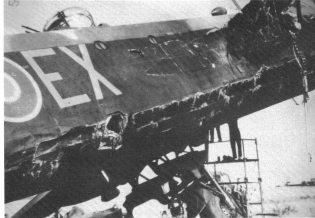
This Stirling Mk III (LJ569) of No 199 Squadron crashed during takeoff from North Creake on 15 September 1944. The starboard wing was torn off inboard of the engine and is visible just under the fuselage. Not surprisingly, C - Charlie was declared fit only for the scrap heap.
