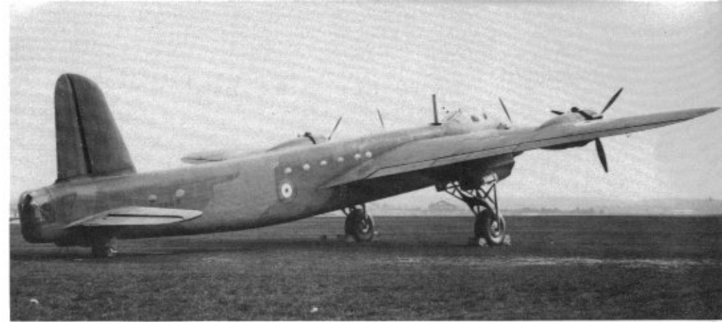
The Stirling prototype (L7600) reveals the high landing gear that became hallmark of the Stirling. National markings carried by the prototype were confined to Type A wing and fuselage roundels. On 14 May 1939, the aircraft made its maiden flight and suffered an undercarriage failure on landing, ending its career.
