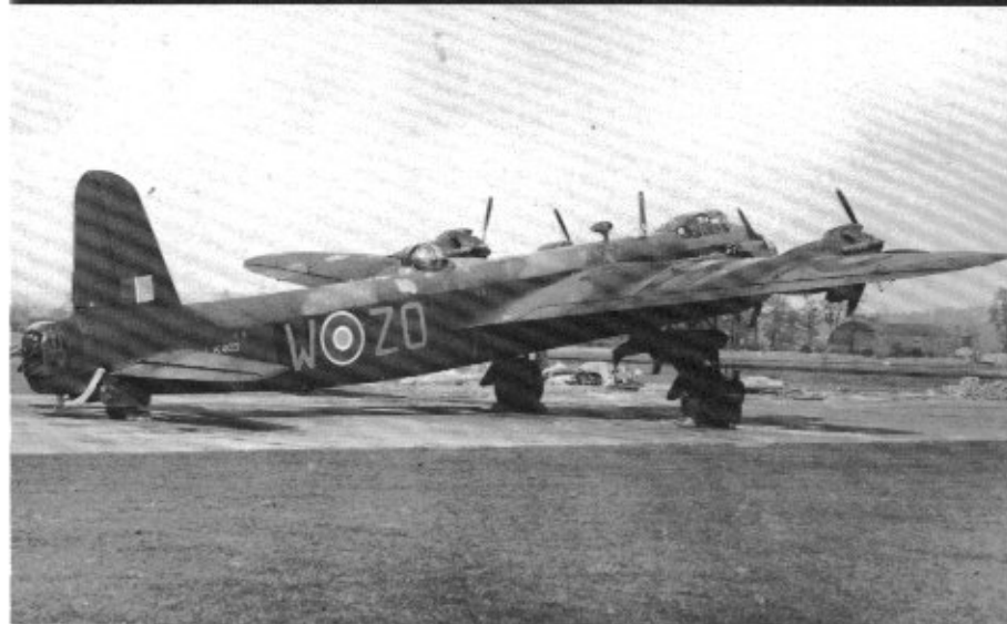
This Mk III (LK403) of No 196 Squadron is fitted with a glider towing yoke installed under the rear turret as part of the tests conducted to determine if the Stirling could tow large gliders. The tests were successful and led to the Stirling Mk IV. This Stirling later ended its career at No 1665 HCU where it was written off after it crashed when the undercarriage failed.
