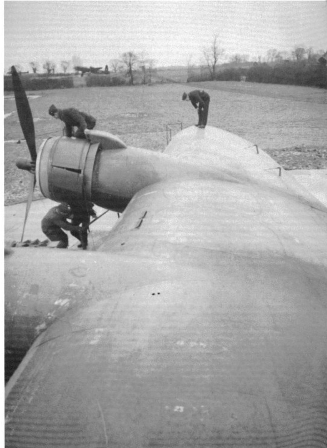
Ground crews perform maintenance on a Stirling Mk I engine. The oval panels on the wing upper surface are the fuel tank covers which were a carry over from the Sunderland flying boat. The two angled posts near the wing trailing edge are the twin alleron control link cables and rods.
