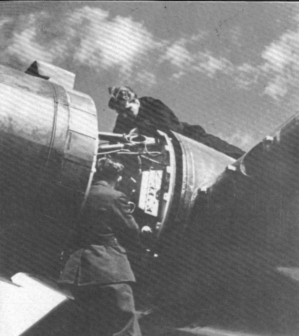
Ground crewmen perform maintenance on a the starboard outboard engine of a Stirling Mk I. The three square protruding shapes on the wing leading edge are barrage balloon cable cutters, while the circular intake in the wing leading edge is the oil cooler intake.
