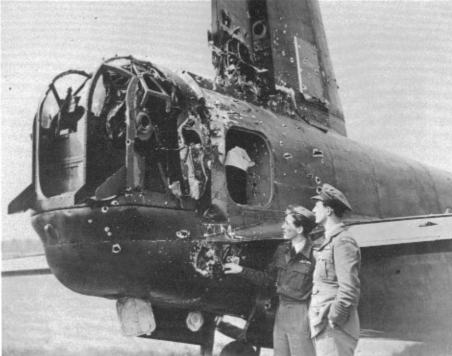
Pilot Officer Peter Buck (Royal New Zealand Air Force, left) inspects the damage to the tail turret and rudder of his Stirling Mk III of No 75 (New Zealand) Squadron. The perspex turret center section was completely shot away by enemy fire over Essen and the escape hatch cover just forward of the turret was jettisoned.
