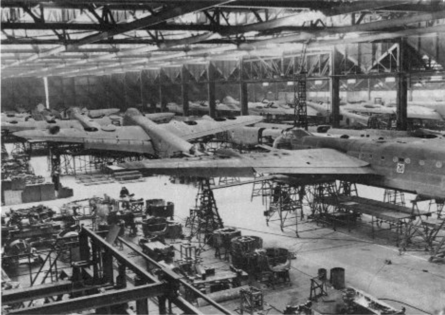
The lack of a dorsal turret indicates that these Stirling Mk Is on the Rochester production line are part of the Series I production batch. The panels on the wing of the second Stirling reveals the location of the wing fuel tanks. The wing trailing edge curves forward at the wing/fuselage joint, producing a bent look when the flaps are lowered.
