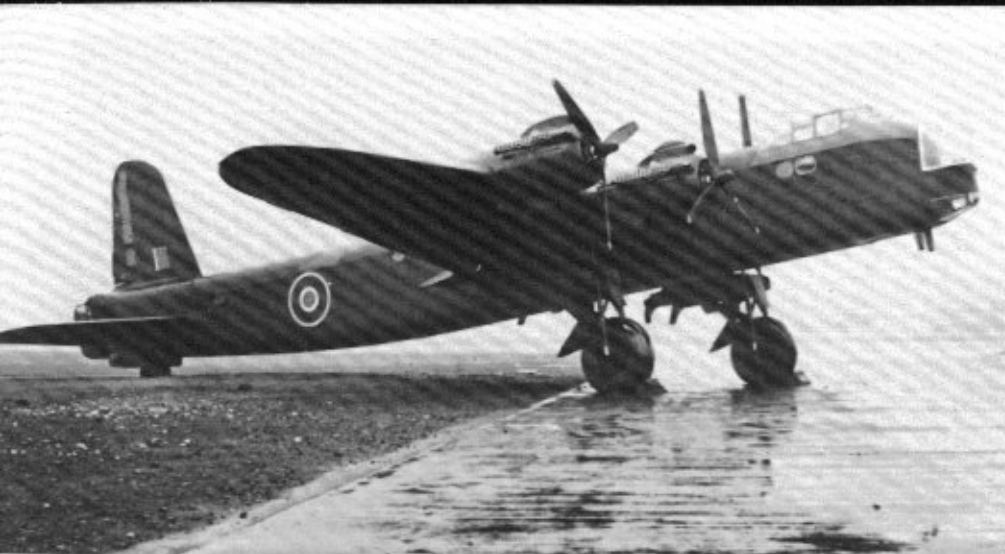
This Stirling Mk IV (EF317) was the first of a production batch produced during December of 1943. These aircraft never saw front line squadron service and were finally SOC between 1945 and 1947. This aircraft is unusual in that it still carries twin pitot tube masts under the nose.
