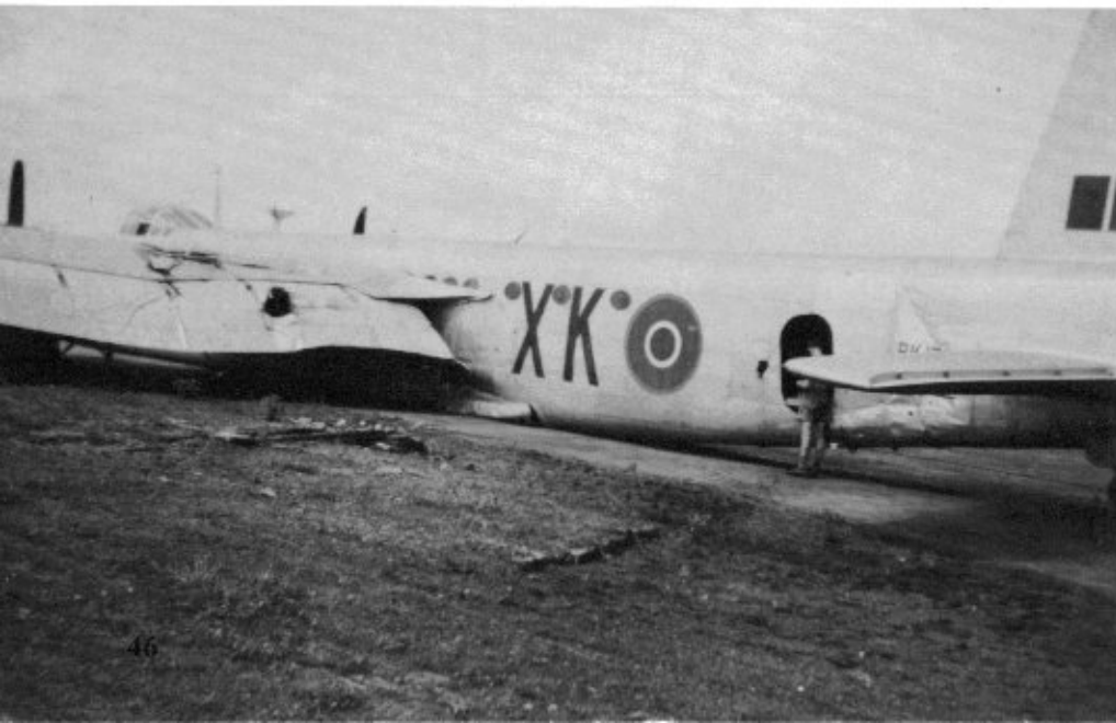
(Below) This Stirling Mk V of No 46 Squadron (PK173) crashed on takeoff from St. Thomas Mount, India on 13 November 1945. The collapse of the undercarriage has caused the propellers to be bent over and the flaps to be dented and holed.
