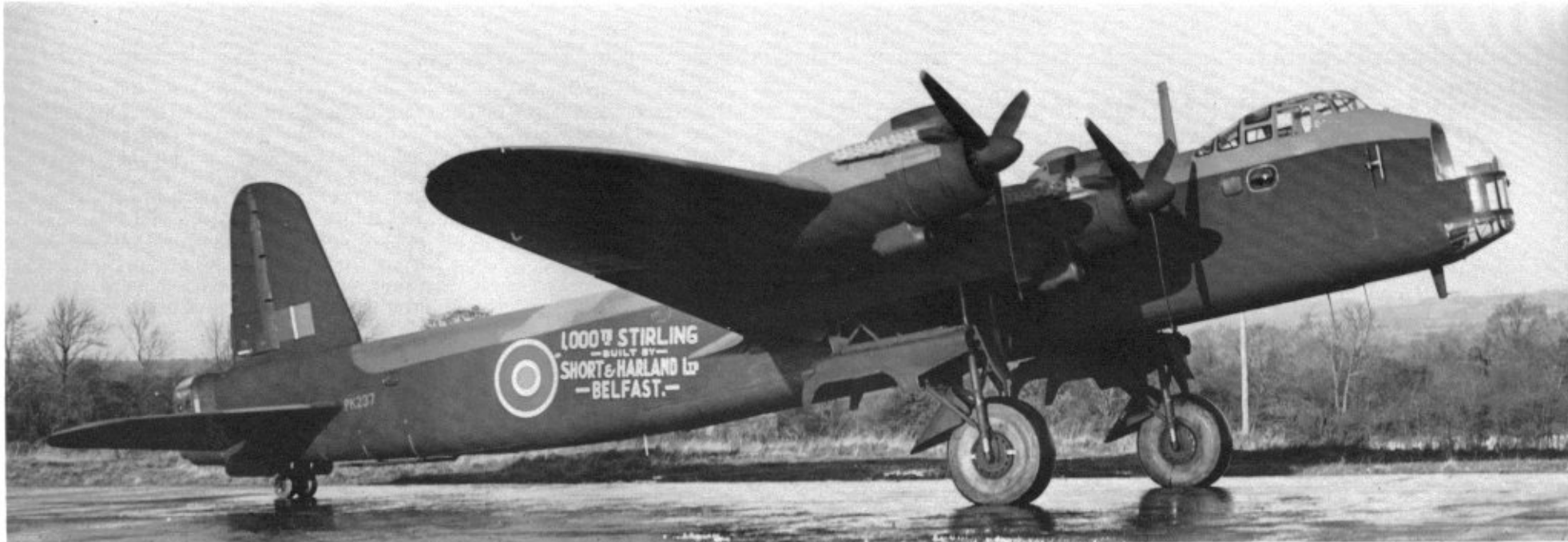
This Stirling Mk IV carries an inscription on the fuselage in White identifying it as the 1,000th airframe manufactured by Short's Belfast plant. This aircraft has not had the glider towing yoke installed on the rear fuselage, but has had the stop guard mounted on the fuselage underside in front of the tail wheel.
