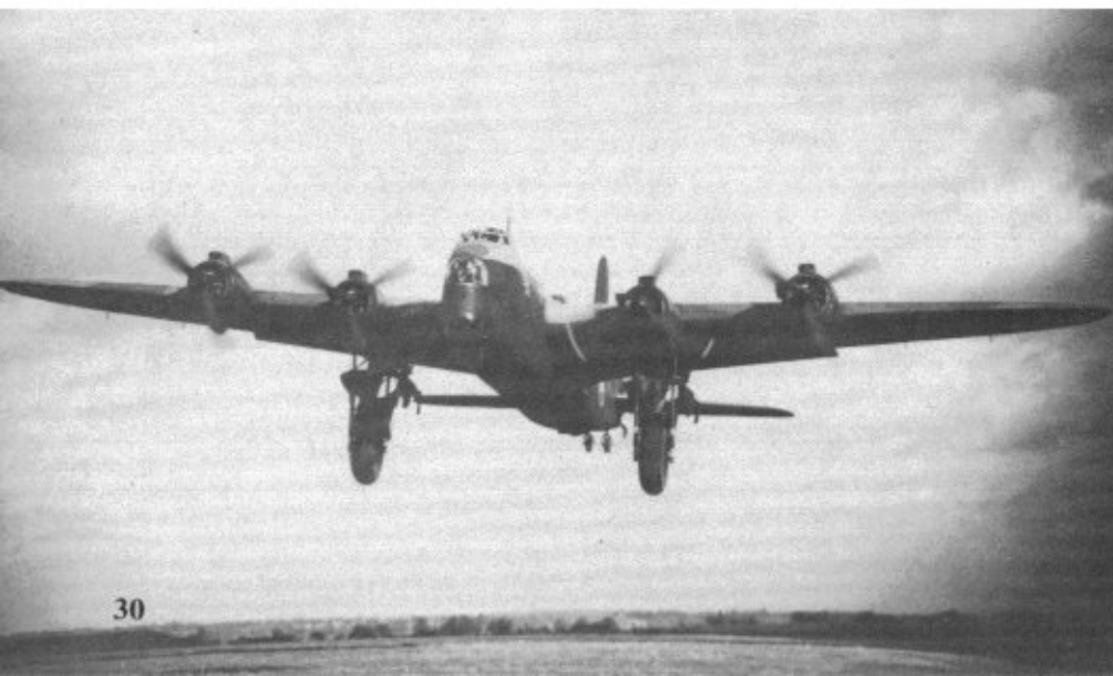
A Stirling Mk III of an unknown squadron on final approach, moments before touch down. The enlarged upper cowling air intakes are visible as are the twin tail wheels.
