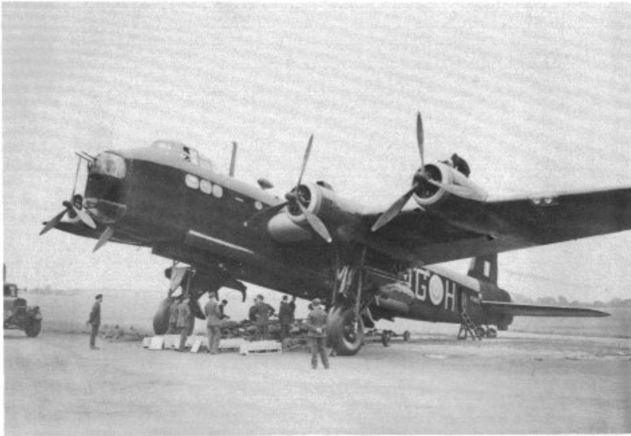
This Stirling Mk I of No 7 Squadron is being loaded with a mixed load of explosive and incendiary bombs. The aircraft is unusual in that it carries standard size code letters on the fuselage side. It was No 7 Squadron's normal practice to use small code letters for the squadron code and a large letter for the individual aircraft code.
