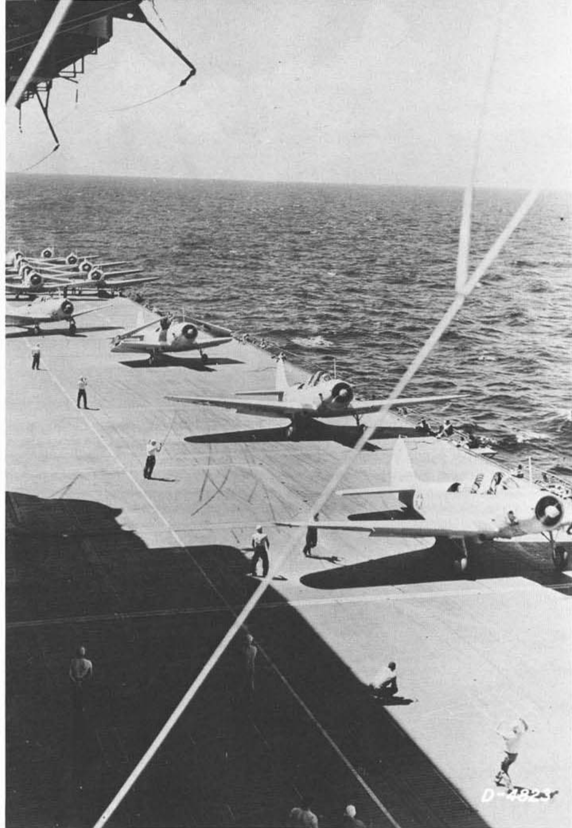
TBD-1s of VT-3 line up for takeoff from the USS SARATOGA during early 1941. The aircraft carry the overall Non-specular Light Gray camouflage adopted by the Navy in December of 1940. In addition to the new camouflage, the TBDs now carry a small national insignia on the fuselage side. (United Technologies Archives)
