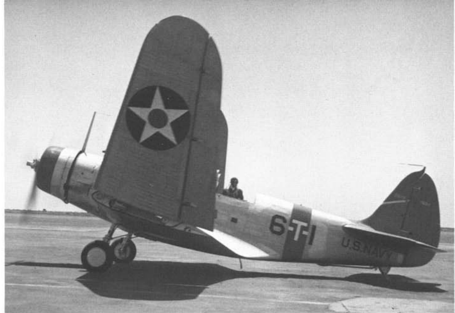
This TBD-1 (BuNo 0324) of VT-6 spreads its wings on the ramp before taxiing out for takeoff. After his aircraft crashed during 1939, the commander of VT-6 took over BuNo 0324 as his aircraft and had it renumbered 6-T-1 with the original number being painted out with Aluminum paint. (William T. Larkins)
