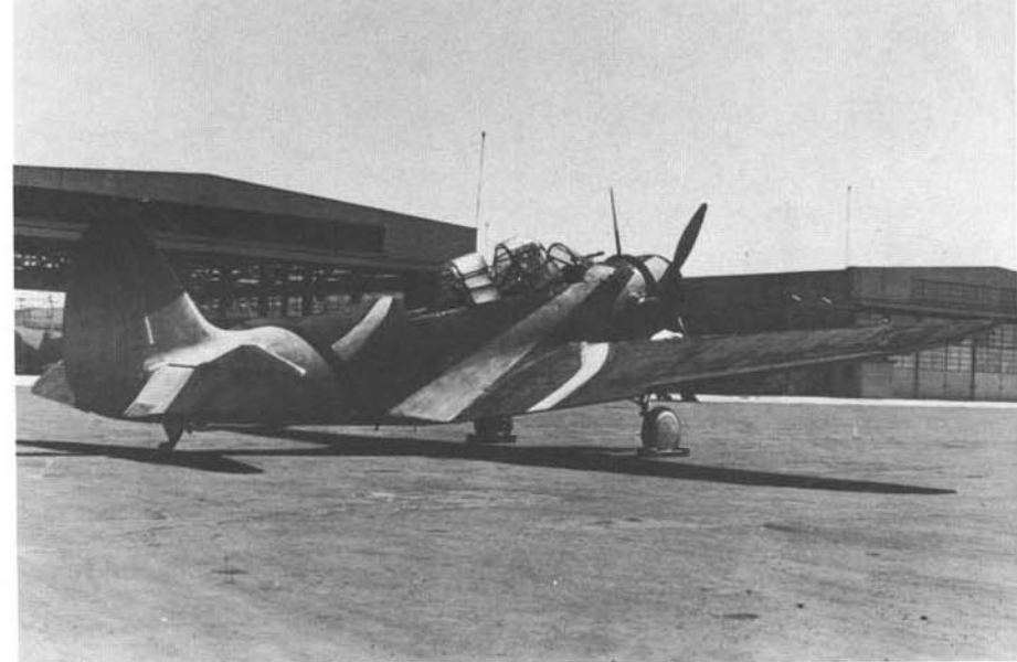
This TBD-1 (BuNo 0320) of VT-2 was painted in the experimental Barclay Design 7 camouflage scheme which was designed to confuse enemy gunners at extreme range. The aircraft was later lost in combat during the Battle of the Coral Sea. (USN/ B. Cressman via Jim Mesko)
