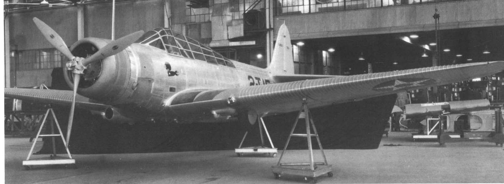
(Above) This TBD-1 (BuNo 0308) is undergoing landing gear drop tests at the Douglas factory. The aircraft will be delivered to VT-2 aboard USS LEXINGTON and carries the squadron insignia on the fuselage below the cockpit, along with the squadron code, 2-T-15, in Black on the rear fuselage sides. (McDonnell Douglas Aircraft)
