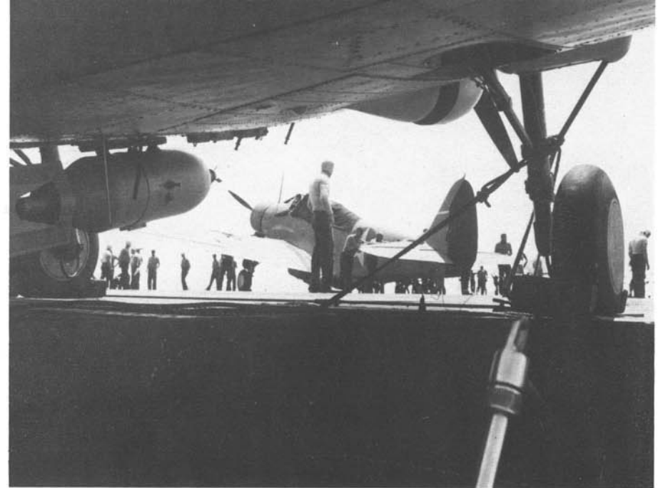
Plane handlers move a TBD-1 on the deck of USS ENTERPRISE prior to the Wake Island raid. The bomb in the foreground is a 500 pound bomb mounted on the port centerline rack of another TBD. The canopy and rudder stripes of the TBD in the background are covered to reduce the possibility that they might be spotted. (National Archives)
