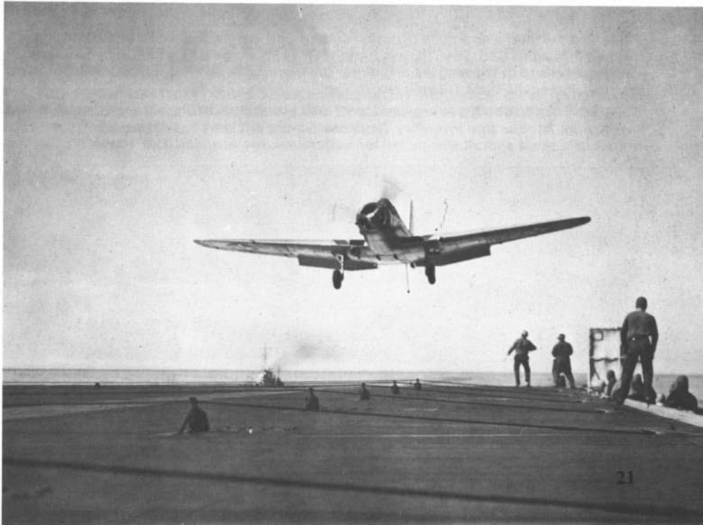
A TBD-1 of VT-3 comes in for a landing aboard USS SARATOGA (CV-3). The landing signal officer (LSO) has just given the pilot the cut signal for him to chop his throttle. The TBD-1 had a landing speed of 63 mph, thanks to its light wing loading and large flaps. (National Archives)
