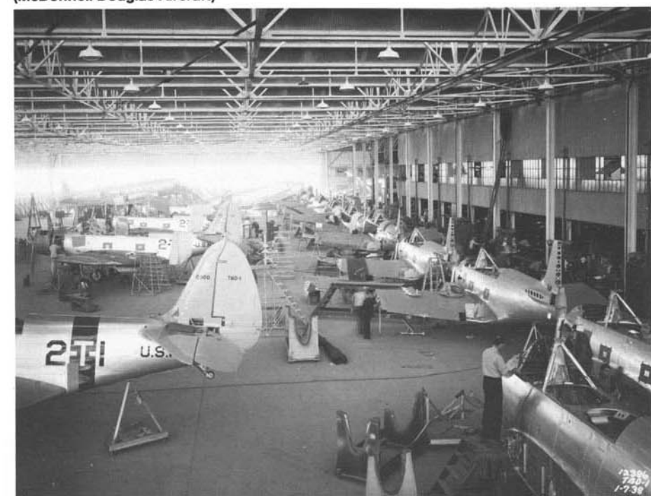
(Below) The TBD-1 production line at Santa Monica during January of 1938 shows fourteen TBD-1s in various stages of construction. Aircraft that were scheduled to be delivered to various fleet squadrons were marked with the proper codes and colors before leaving the factory. The aircraft in the left foreground are destined for VT-2 aboard USS LEXINGTON. (McDonnell Douglas Aircraft)
