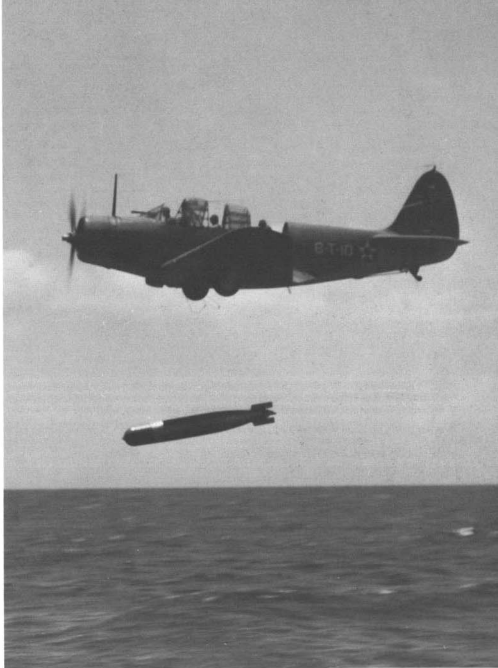
A TBD-1 of VT-6 makes a practice torpedo drop. VT-6 was one of the first squadrons to repaint their aircraft in the Non-specular Blue Gray over Non-specular Light Gray camouflage authorized in October of 1941. (National Archives)
