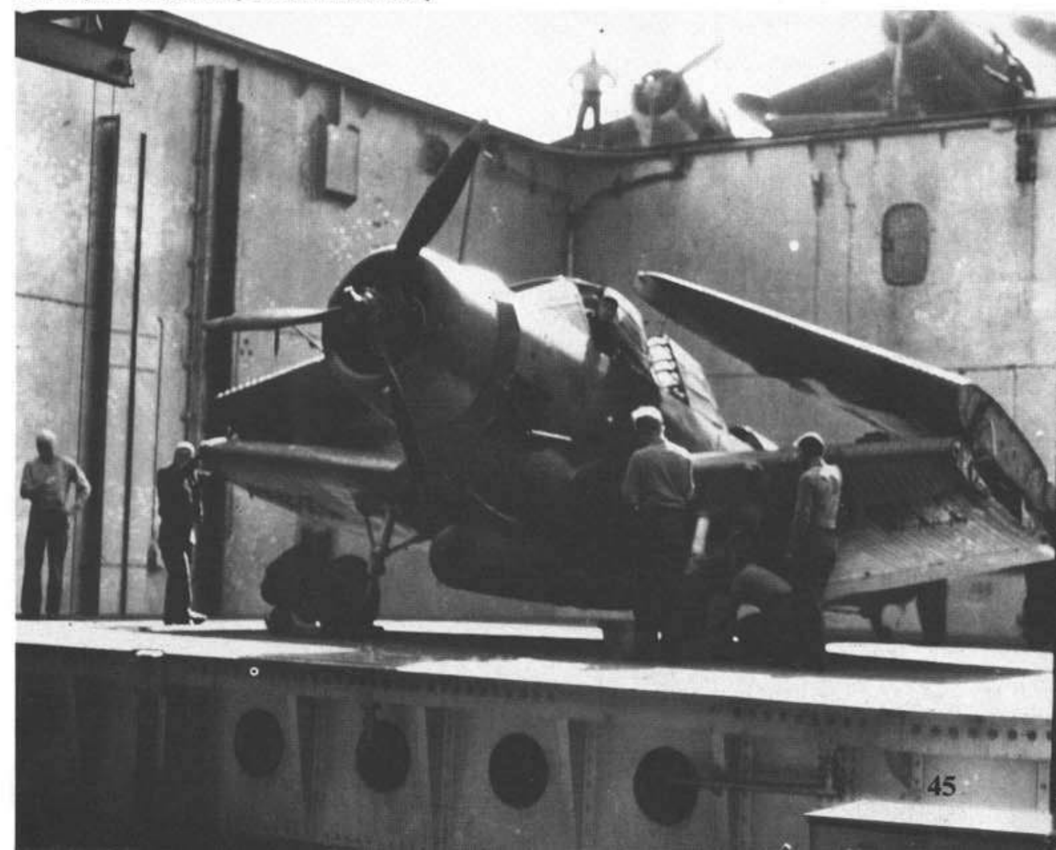
Deck handlers position and chock a torpedo armed TBD of VT-6 on the aft aircraft elevator aboard USS ENTERPRISE (CV-6). The wing insignia has been covered over to lessen its visibility from above. (National Archives)
