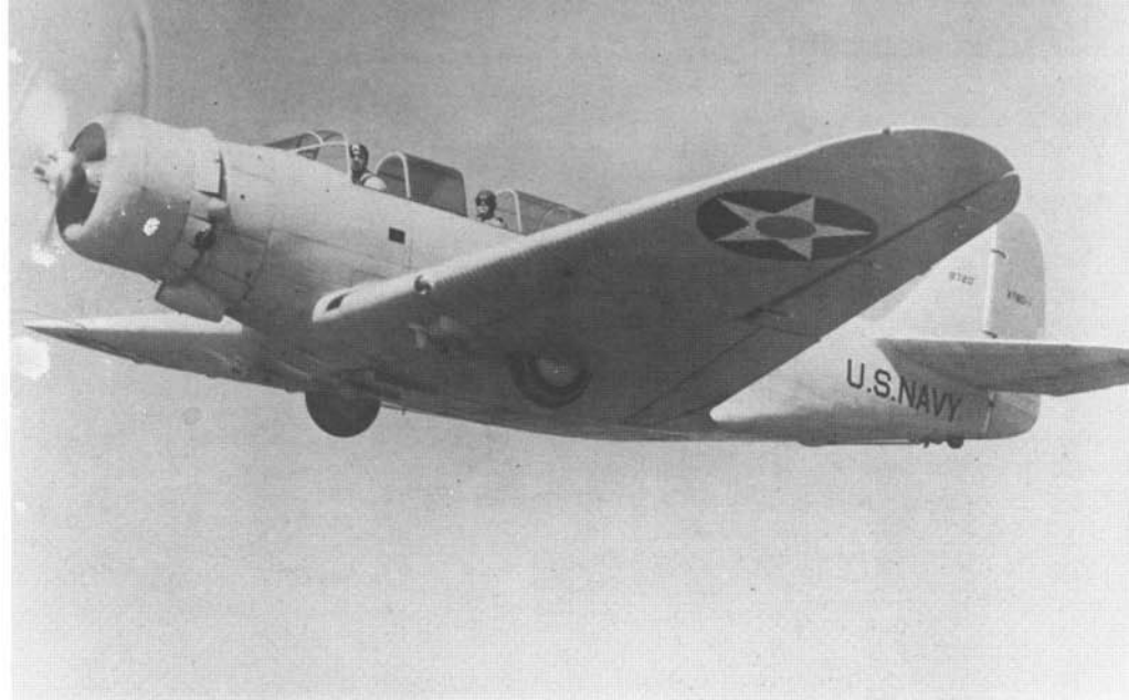
The XTBD-1 (BuNo 9720) prototype on a test flight during 1935. The XTBD-1 was the first all metal, low-wing monoplane to be accepted by the Navy for service aboard aircraft carriers. The main wheels were partially exposed when retracted to protect the fuselage underside in case of an emergency wheels up landing. (U.S. Navy)
