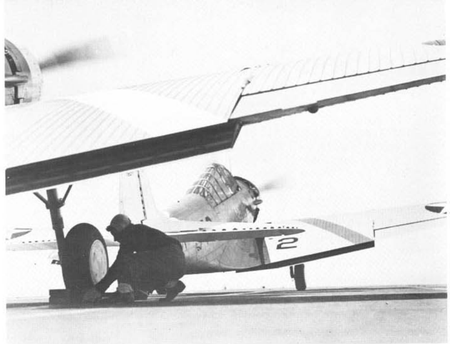
A deck crewman prepares to remove the wheel chocks from a TBD-1 of VT-3 aboard USS SARATOGA as the aircraft ahead of it (3-T-2) goes to full power for a deck launch. Deck crews had to be alert at all times to avoid being blown off the deck by the prop wash of maneuvering aircraft. (National Archives)
