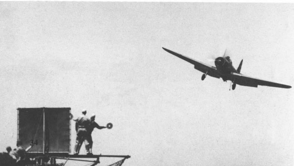
The Landing Signal Officer aboard ENTERPRISE guides a TBD-1 of VT-6 back aboard after the raid against Kwajalein on 1 February 1942. The aircraft still carries one 500 pound bomb on the port centerline bomb rack. (National Archives)
