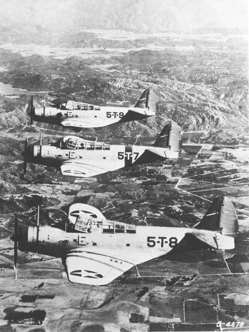
TBDs of the third section of Torpedo Squadron Five (VT-5) fly formation over California during 1940. 5-T-7 has the twenty inch wide True Blue fuselage band indicating it as the section leader's aircraft. VT-5 was stationed aboard the USS YORKTOWN (CV-5). (United Technologies)
