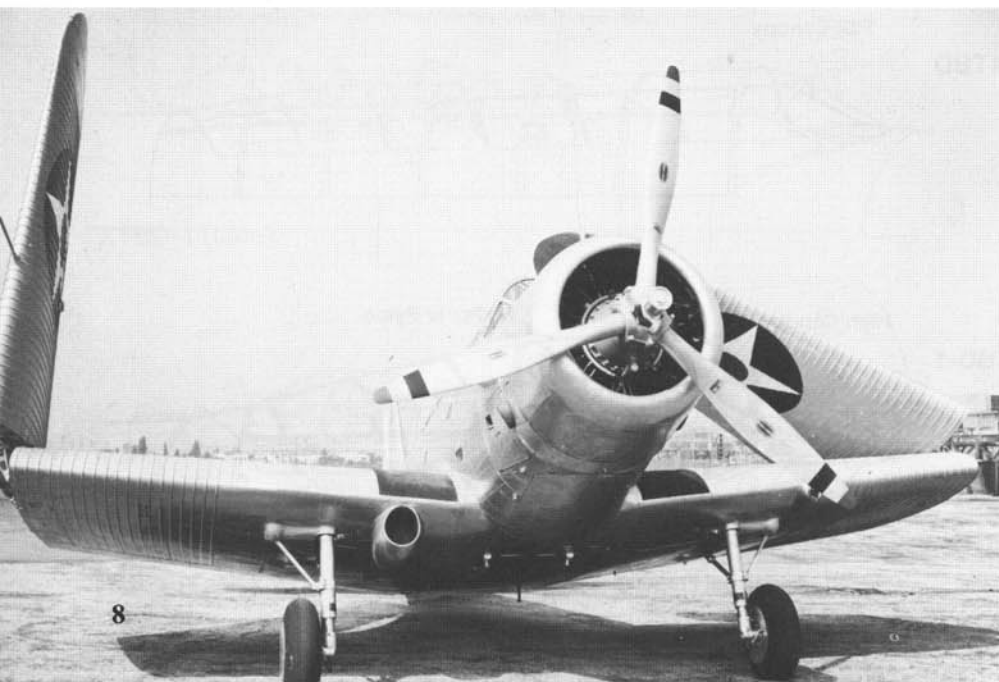
(Below) The TBD-1 was the first Navy aircraft to feature hydraulic folding wings. The outer thirteen feet of each wing folded up over the cockpit. The wings could be folded from inside the aircraft by either the pilot or assistant pilot/torpedoman. (U.S. Navy)
