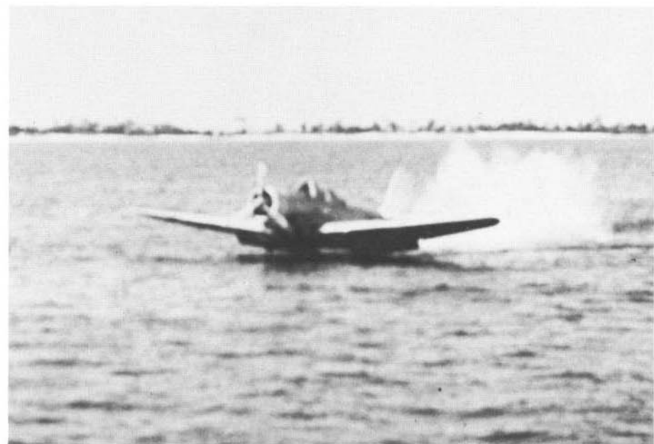
(Below) This TBD-1 (BuNo 0358) suffered a hydraulic failure and made a water landing in Pensacola Bay on 15 August 1938. The flotation bags worked, and the aircraft was salvaged, repaired and later served with Torpedo Squadron Five (VT-5) in the Atlantic. (U.S. Navy)
