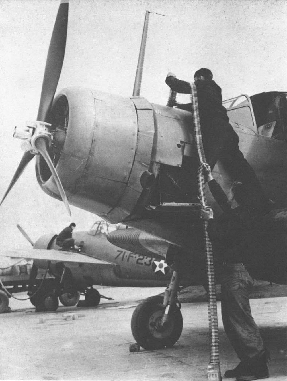
Armorers load Blue tipped .30 caliber ammunition into the nose gun of a TBD to ready it for a practice gunnery mission, while other crewmen fuel an F4F Wildcat at Scapa Flow, Scotland during March of 1942. The Blue painted tips of the ammunition left a blue mark on the target, indicating which aircraft hit it. (National Archives)
