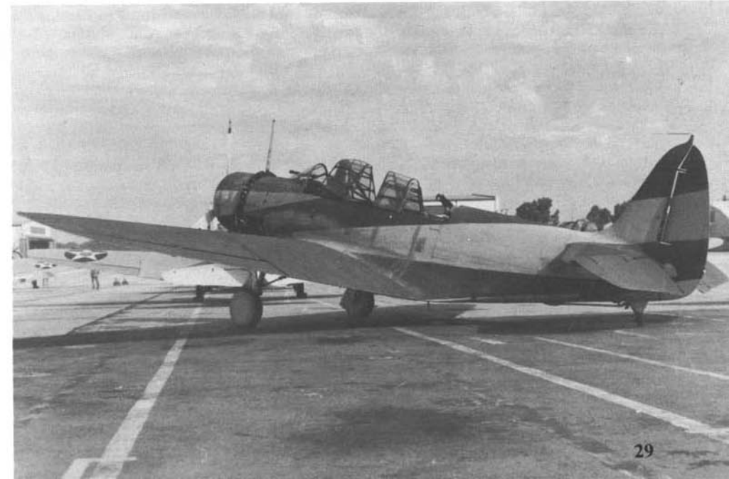
After the fleet trials were completed, 0339 had the paint stripped off and was returned to its original finish. The Barclay camouflage was found to be ineffective and the tests were terminated in the late Fall of 1940. 0339 was later transferred to VT-2 and was lost in the Coral Sea during May of 1942. (USN/B. Cressman via Jim Mesko)
