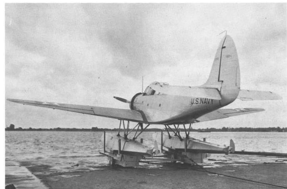
The TBD-1A on its beaching gear on the seaplane ramp of the Naval Torpedo Station at NAF Gould Island, during late 1939. The aircraft was a one of a kind prototype and was used for various test programs. The float installation reduced the aircraft's top speed by 20 mph. (CAPT W.E. Scarborough)
