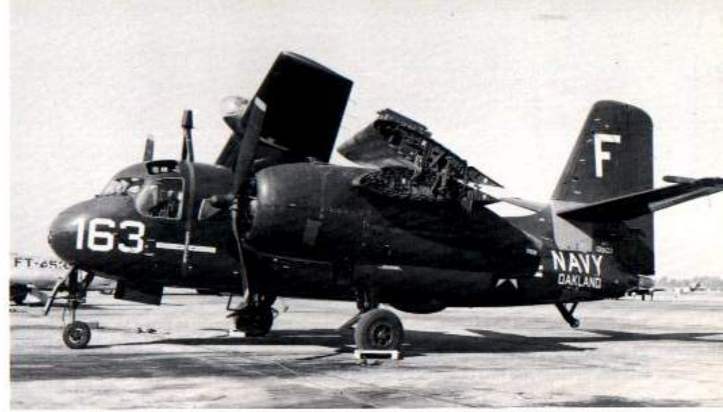
This S2F-1 (BuNo 133103) on the ramp at NAS Oakland, California, on 16 September 1956, carries an International Orange fuselage band indicating that it was assigned to the Naval Reserves. The pilot's escape hatch on top of the fuselage is in the open position. (Bill Larkins)
