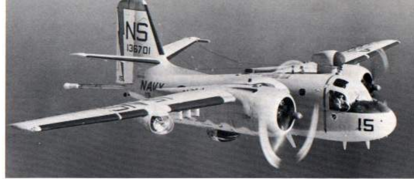
An S-2A (S2F-1/BuNo 136701) of VS-21 flies an ASW search mission with the belly radome and MAD boom deployed. NS-15 was operating off the coast of San Diego, California, on 18 December 1963 and carried a Red lighting bolt, outlined in Black, on the rudder and a Red fin tip. (U.S. Navy)
