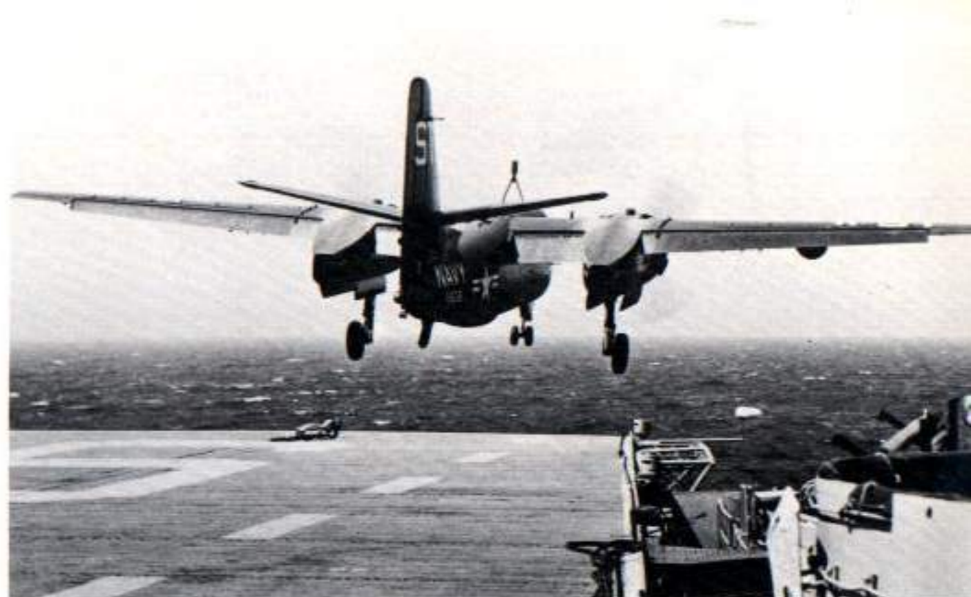
An S2F-2 (BuNo 133349) of VS-38 is launched from the starboard catapult of the escort carrier USS BADOENG STRAIT (CVE-116) on 23 September 1954. (U.S. Navy via Hal Andrews)
