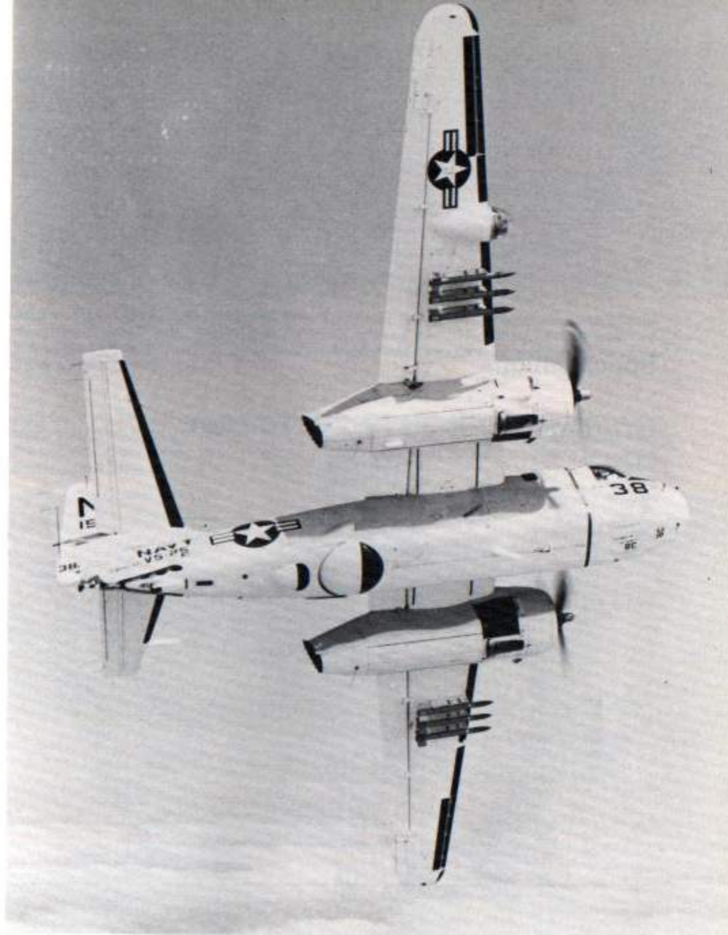
This S-2E (BuNo 151640) of VS-25 is armed with six 5 inch HVAR rockets on the underwing pylons. The small second radome on the fuselage underside behind the belly radome identifies this STOOF as an S-2E. (U.S. Navy via Peter Mersky Collection)
