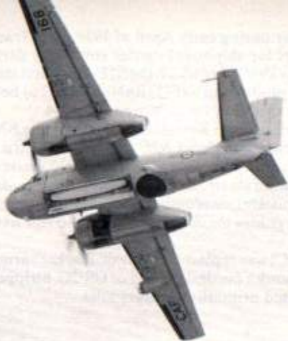
A CS2F-3 (12168) of MR-880 with the weapons bay open reveals the weapons bay auxiliary fuel tank installation used to extend the range of the Tracker for maritime reconnaissance missions. (Terry Panopalis)
