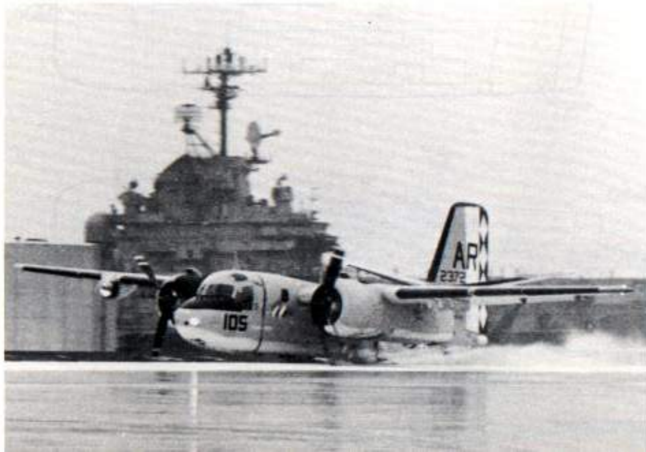
An S-2E (BuNo 152372) of VS-30 makes a belly landing on the foamed runway of NAS Quonset Point, RI during 1971. Hydraulic failure caused the No. 2 engine to be shut down and the propeller was feathered. When the landing gear failed to extend, the pilot elected to perform a belly landing. (U.S. Navy)
