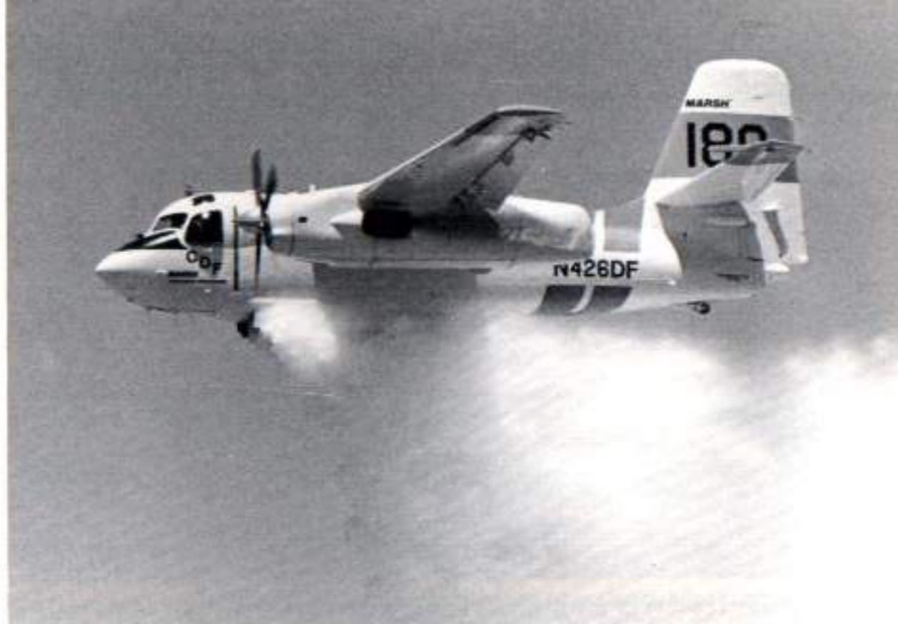
S2F-1 (S-2A/BuNo 136613/N426DF) has been modified with a turboprop engine by Marsh Aviation of Mesa, AZ. Powered by a Garrett TPE331-14 turboprop driving a five blade Hartzell propeller, this Turbo-Tracker is configured as a firefighter for the California Division of Forestry (CDF) during 1988. (Marsh Aviation Co.)
