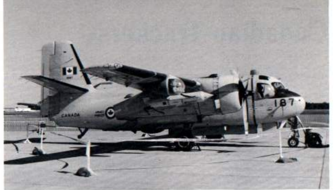
This CS2F-3 (12187) of Maritime Reconnaissance Squadron 880 (MR-880) is roped off for a display on 29 June 1986. The aircraft carries a streamlined, day/night photographic pod on the outboard starboard wing pylon. The aircraft is used primarily for maritime reconnaissance, flying from CFB Shearwater, Nova Scotia. (Terry Panopalis)
