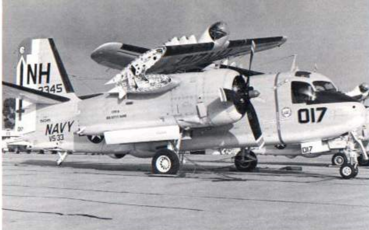
An S-2G (BuNo 152345) of VS-33 on the ramp at NAS North Island on 22 September 1973. VS-33 was assigned to Carrier Air Wing 11 (CVW-11) on board USS KITTY HAWK (CV-63). NH-017 has not yet been fitted with the smoke marker retro-ejector installation on the engine nacelle. (Peter Mancus)
