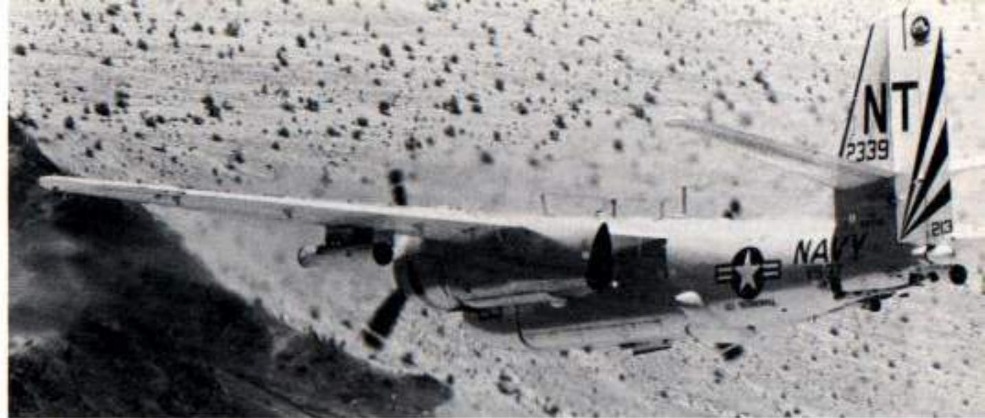
An S-2E (BuNo 152339) of VS-37 unleashes Zuni rockets over the Chocolate Mountain Aerial Weapons Testing Range located near Yuma, AZ, on 24 June 1978. The rockets were carried in four shot LAU-10A launcher pods and the S-2E could carry six such pods. (U.S. Navy via Peter Mersky Collection)
