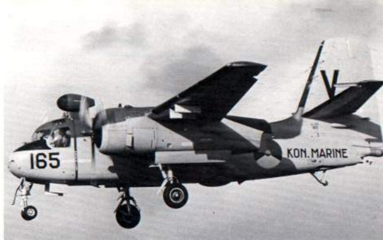
Dutch Navy S-2Ns (modified S-2As) carried a two tone Gray camouflage scheme. The S-2N was a version of the S2F-1 (S-2A) modified for use by the Netherlands Navy by Fairley of Canada. This Tracker was landing at Ypenberg, Holland during 1970. (M. Herben)
