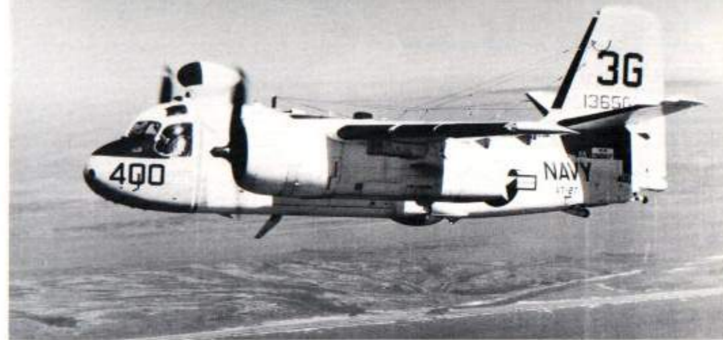
A student pilot and his instructor fly a TS-2A (S2F-1T/BuNo 136507) of VT-27 off the coast of Southwest Texas, on 20 June 1968. Trackers were used by the Training Command as advanced trainers to provide qualified multi-engine pilots for the fleet. (U.S. Navy via Hal Andrews)
