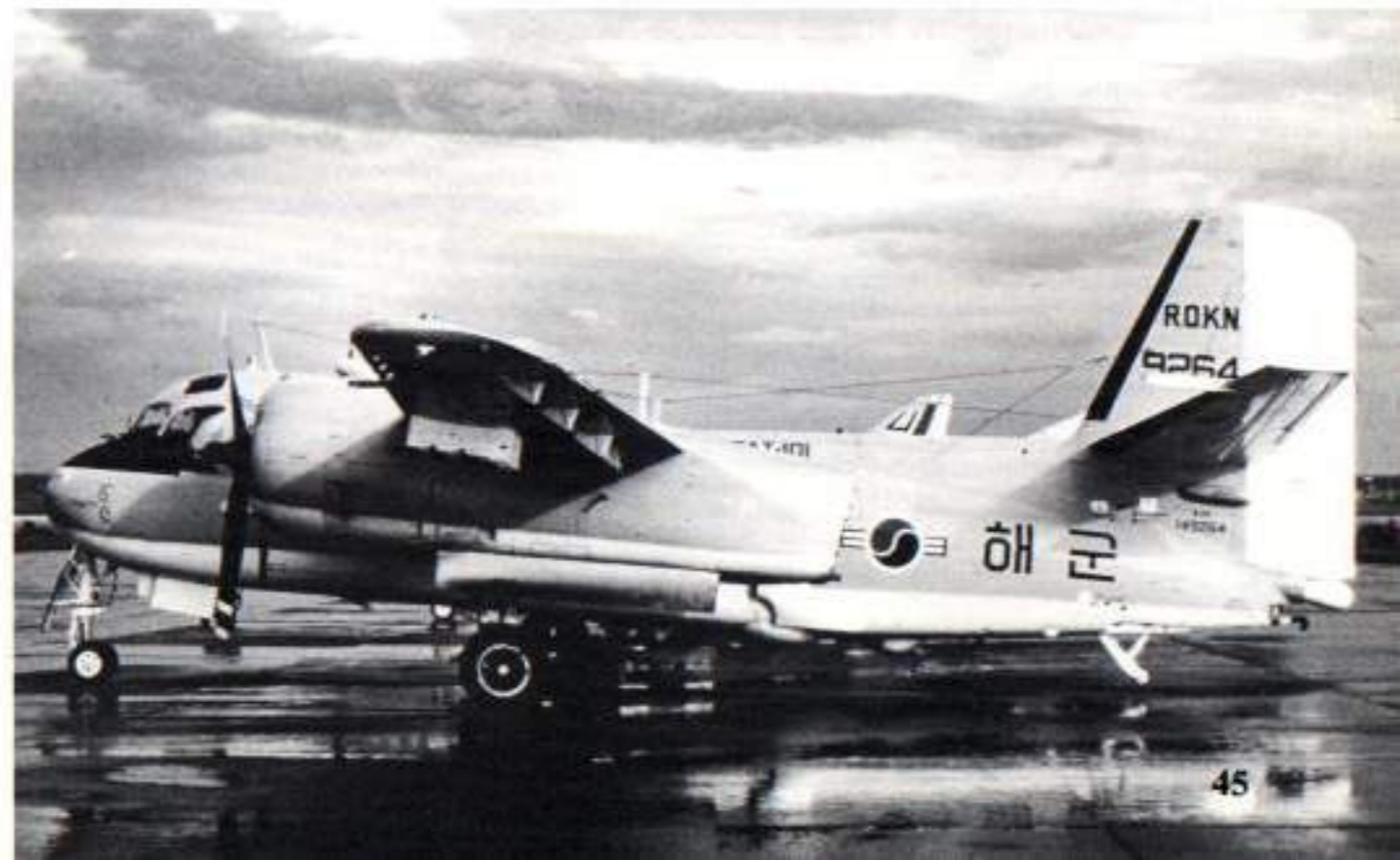
The S-2 was used by both the Korean Air Force and Navy. This S-2E (BuNo 149264), at NAS Dallas, Tx, during July of 1976, belonged to the Korean Navy and was one of twenty-three aircraft provided for ASW and coastal patrol work. The Tracker carried the standard Gull Gray over White paint scheme. (D. Barnes via JEM Aviation Slides)
