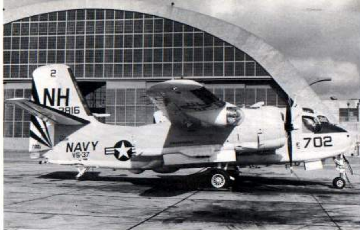
This S-2G (BuNo 152816) of VS-37 on the ramp at NAS North Island on 27 March 1976, has a smoke marker retro-ejector pod installed on the starboard side of the engine nacelle. The pod carried three marine smoke markers. The S-2G was the last S-2 variant to serve with the U.S. Navy. (Clay Jansson)
