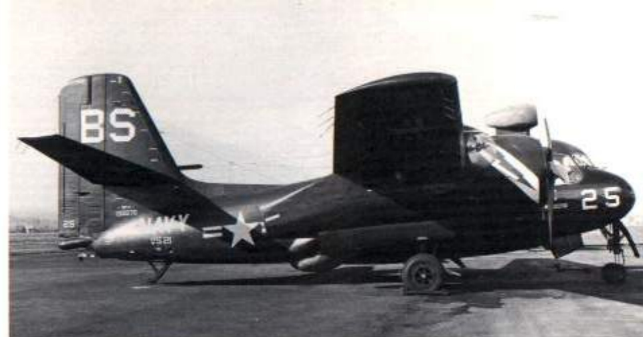
This S2F-2 (BuNo 133370) of VS-21 is sitting on all five wheels, with the tail bumper resting on the ramp. The standard Glossy Sea Blue paint scheme was carried on U.S. Naval aircraft from late 1944 until 1957. (Pete Bowers Collection)
