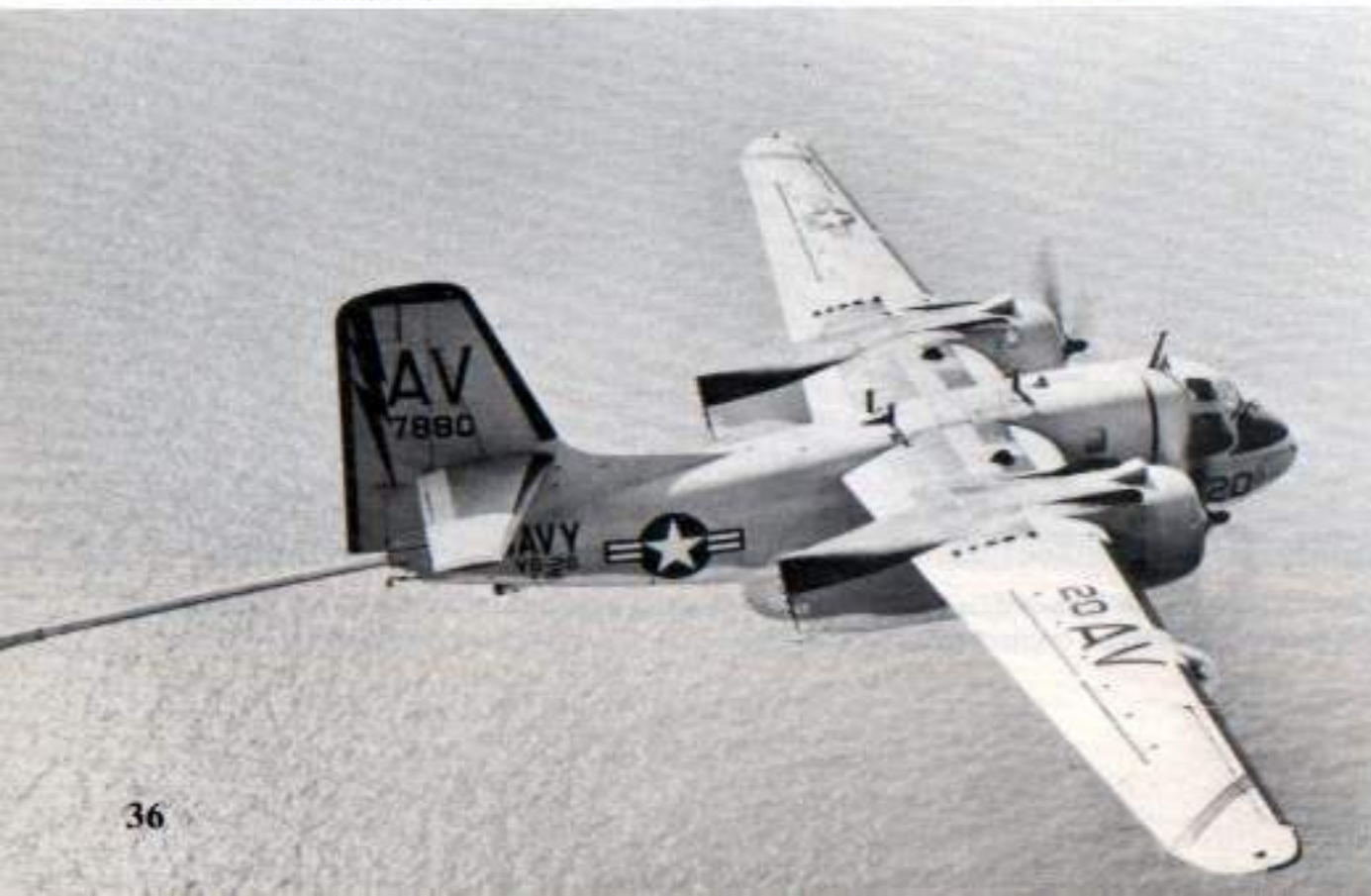
An S-2D (BuNo 147880) of VS-26 flies an ASW patrol during 1965 with the fuselage underside radome and MAD boom extended. ASW patrols were generally flown at an altitude of 1,500 feet and an airspeed of 130 knots. (Grumman via Terry Panopolis)
