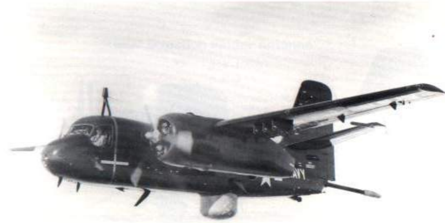
This S2F-1 (BuNo 133237) has its Radome and Magnetic Anomaly Detector (MAD) boom fully extended as it would be during an ASW mission. The forward-raked mast on the fuselage underside and just forward of the weapons bay, is the barricade guard. (Grumman via Pete Bowers)
