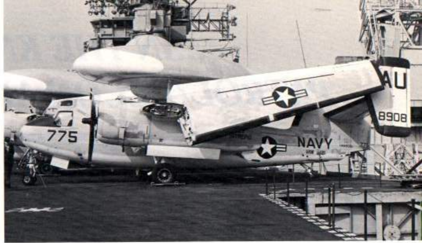
This E-1B (BuNo 148908) of VAW-121 was assigned to USS INTREPID during her visit to Portsmouth, England, on 11 September 1971. E-1Bs served as AEW (Airborne Early Warning) aircraft providing the fleet with information on incoming enemy aircraft. (Peter Russell-Smith)
