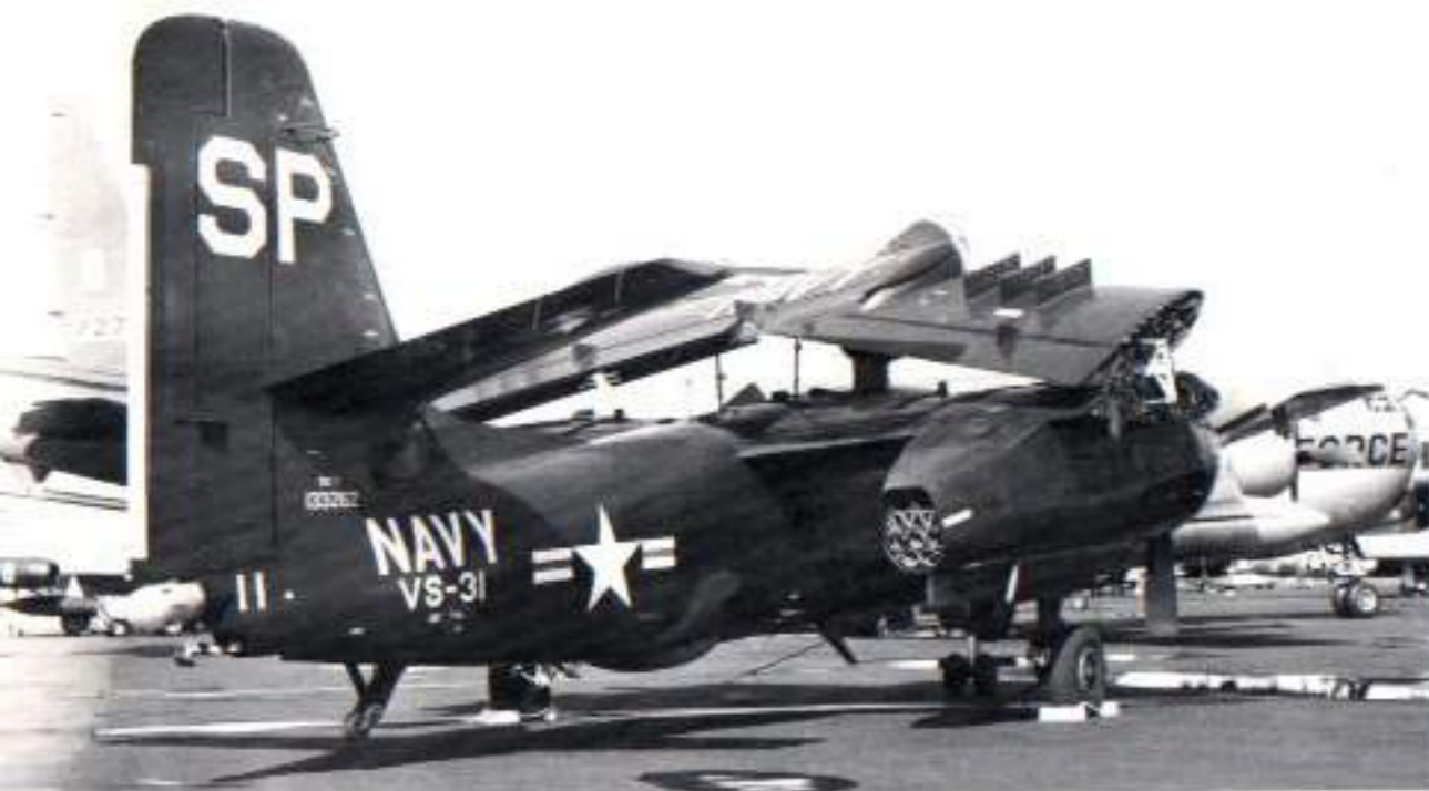
An S2F-1 (BuNo 133262) of VS-31 shares the ramp with a KC-97, F-89 and F-94C at New York during 1958. The S2F is Glossy Sea Blue with White codes and markings and was delivered with the APA-69 radome in place of the earlier bi-pole antenna installation. (F.G. Freeman via Bill Larkins)
