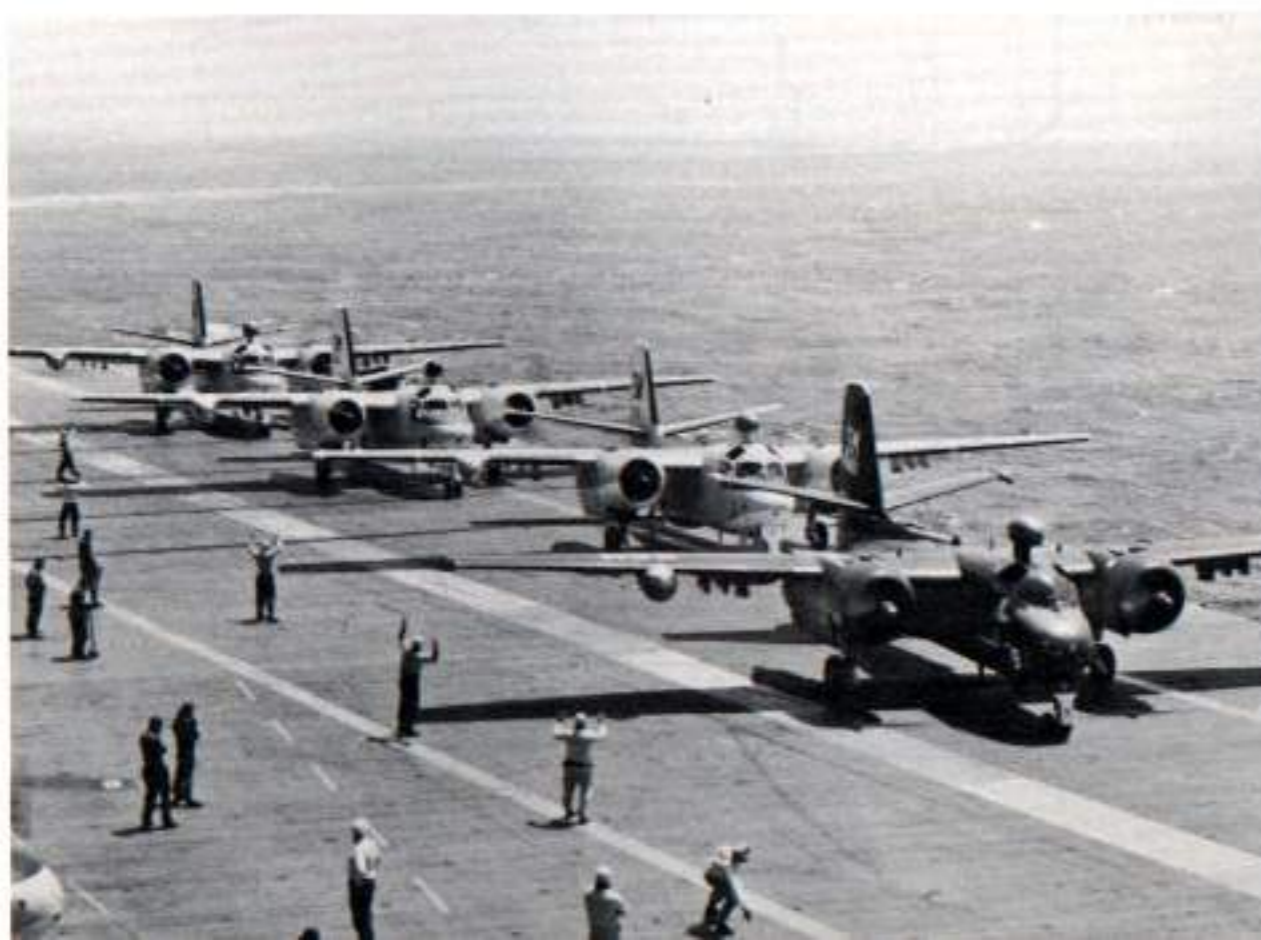
S2F-1s of VS-27 line up for deck launch aboard USS WASP as she steams off the Virginia coast. During 1957 the Navy changed the tactical paint scheme carried on carrier aircraft and it was not uncommon to see aircraft within the same squadron in both the Glossy Sea Blue finish and the new Gull Gray over White scheme. (U.S. Navy via Hal Andrews)
