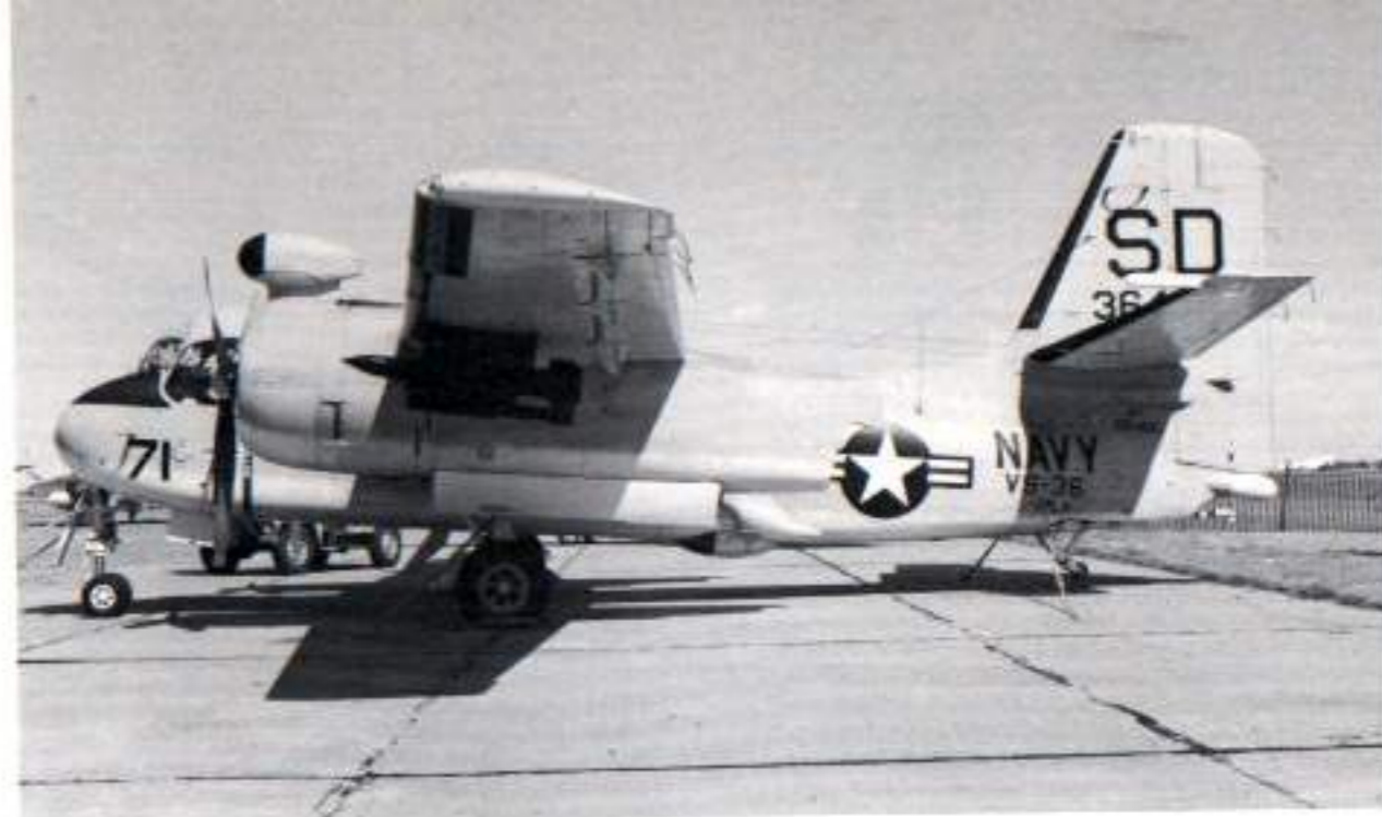
This S2F-1 (BuNo 136482) of VS-36 is loaded with inert 5-inch HVAR rockets and depth charges on the underwing pylons for a display during 1960. The lines coming off the trailing edges of the wing and horizontal stabilizer are static electricity dischargers. (Pete Bowers Collection)
