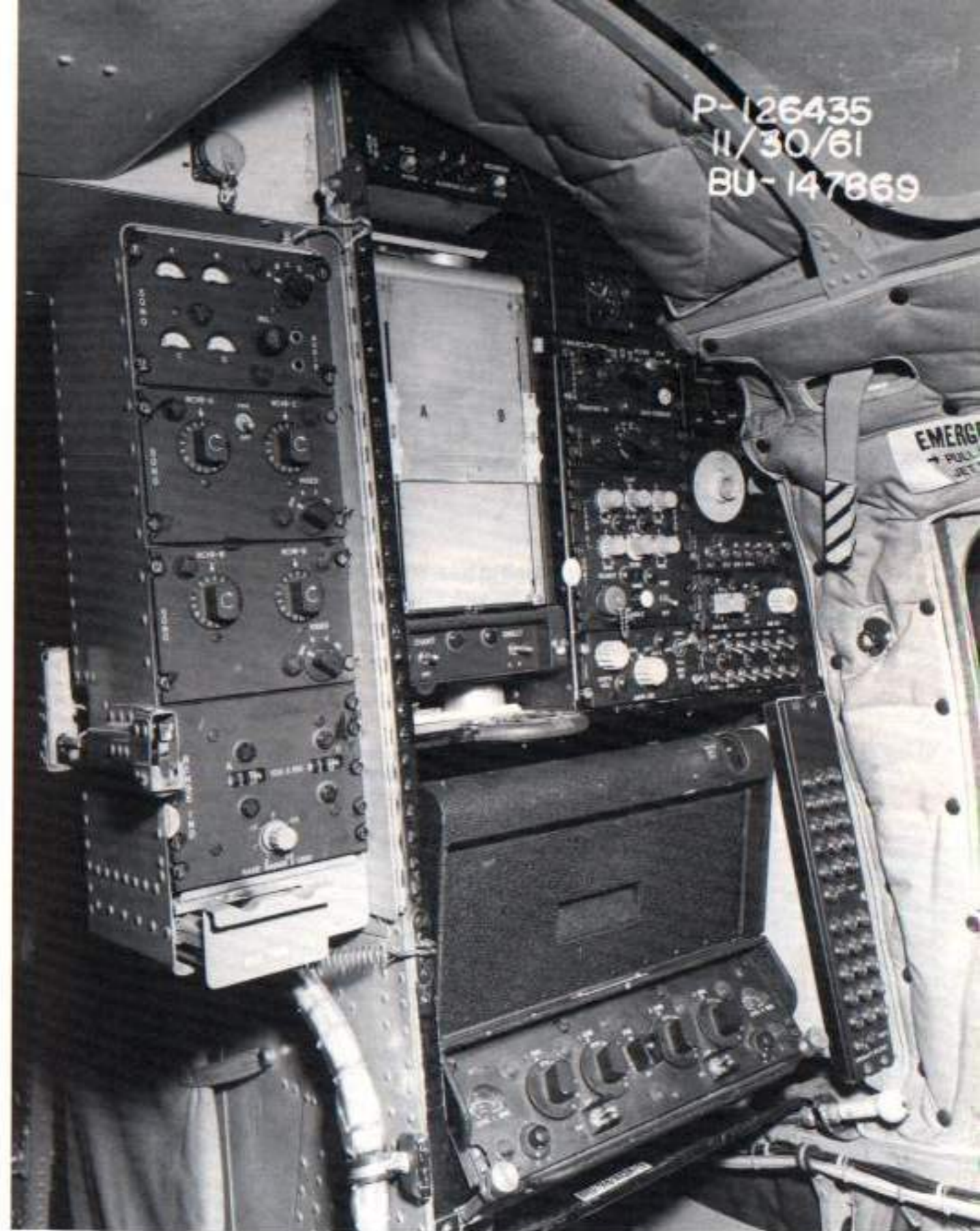
The starboard ASW Operator's Station had the plotting tape printer for the MAD system and the sonobuoy release control panel (far right).
