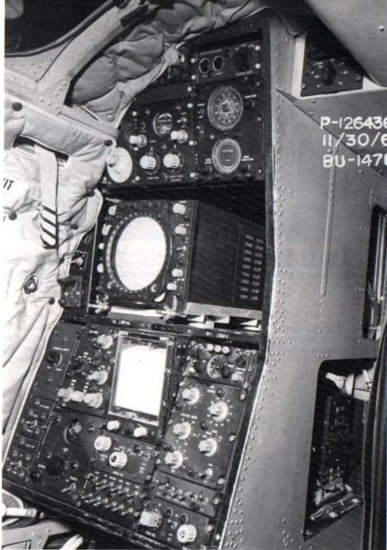
The port ASW Operator's Station contained the main search radar screen and other sensor equipment.
