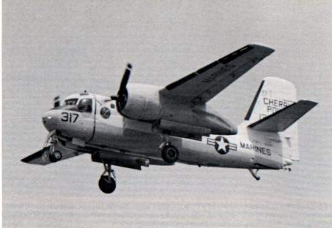
On final approach to the duty runway, a US-2A (BuNo 133317) from MCAF New River, North Carolina, lands at Shaw AFB, South Carolina, on 18 June 1970. The US-2A had all ASW equipment deleted and target tow capability added. (Jim Sullivan)
