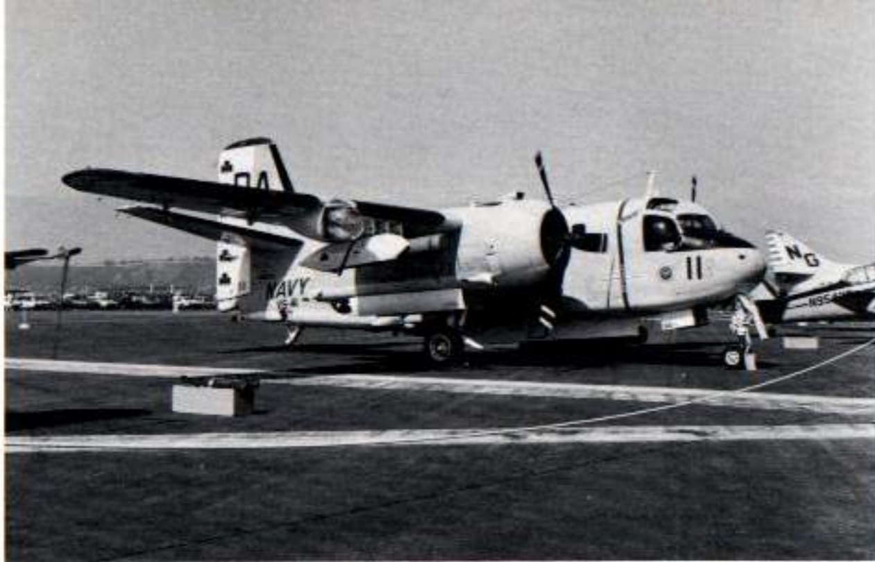
This S-2E (BuNo 149263) of VS-41 on the ramp at NAS North Island during May of 1967, had a combination camera pod/flare launcher on the outboard pylon and a Mk 46 practice torpedo on the inboard pylon. The squadron markings are Green shamrocks on a White rudder. (Author's Collection)
