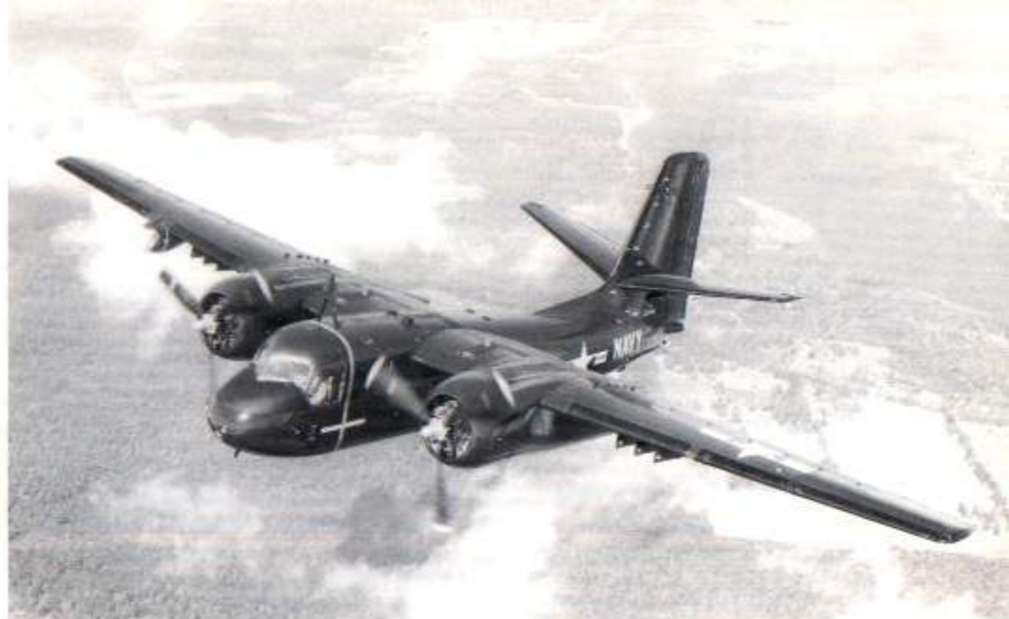
The 13th production S2F-1 (BuNo 129151) Tracker during its acceptance flight over Long Island, near Grumman's Bethpage factory. The bi-pole ECM direction finder antenna is mounted over and just to the rear of the cockpit. The overall Glossy Sea Blue paint scheme remained the standard factory applied finish until 1957. (Grumman via Pete Bowers)
