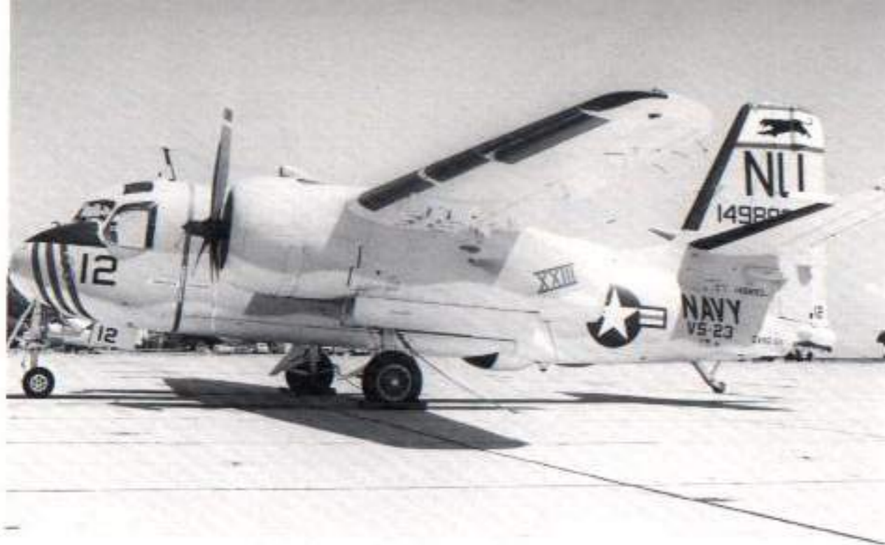
This S-2E (BuNo 149892) of VS-23 on the ramp at NAS North Island on 2 May 1964, carries the special markings used during UNITAS-23, a large-scale military exercise held with South American countries. The nose stripes, XXIII on the nacelle and the outline above and below the Black Panther on the fin tip are RED. (Clay Jansson)
