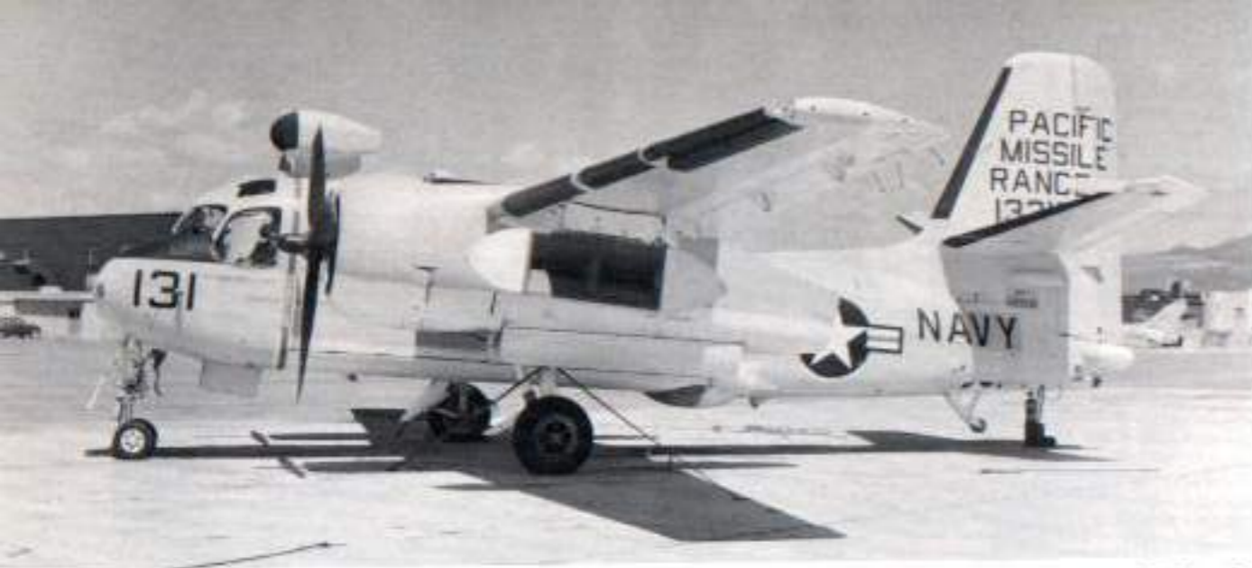
This S2F-1 (BuNo 133131) assigned to the Pacific Missile Range at Point Mugu, California, carries a streamlined loudspeaker pod on the port outer wing pylon on 22 April 1961. The pod consisted of four large speakers, with a nose and tail fairing. The pod was used to warn boaters to clear the test range prior to a missile launch. (Clay Jansson)
