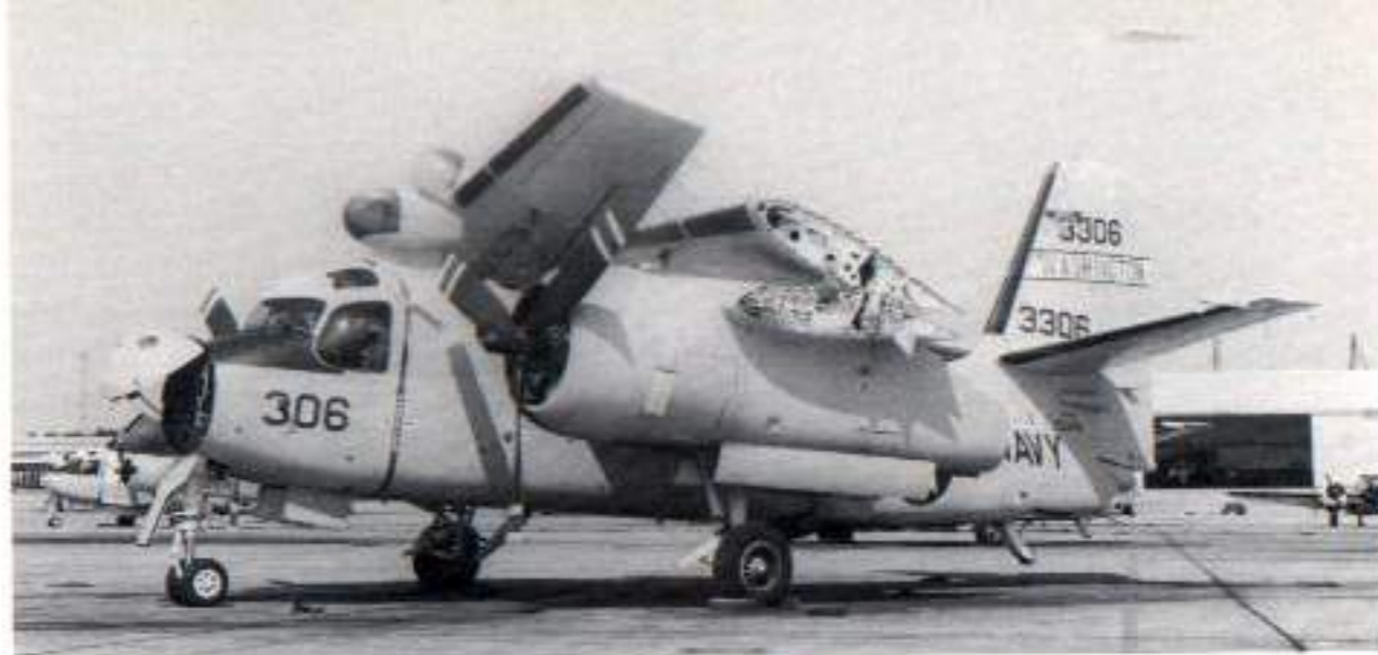
The nose cap on this US-2B (BuNo 133306), at NAF Washington, on 2 June 1967, is open and held in position by a brace on the starboard side. This particular Tracker retained its ASW gear, but carried the US-2B designation under the horizontal stabilizer. (Clay Jansson)
