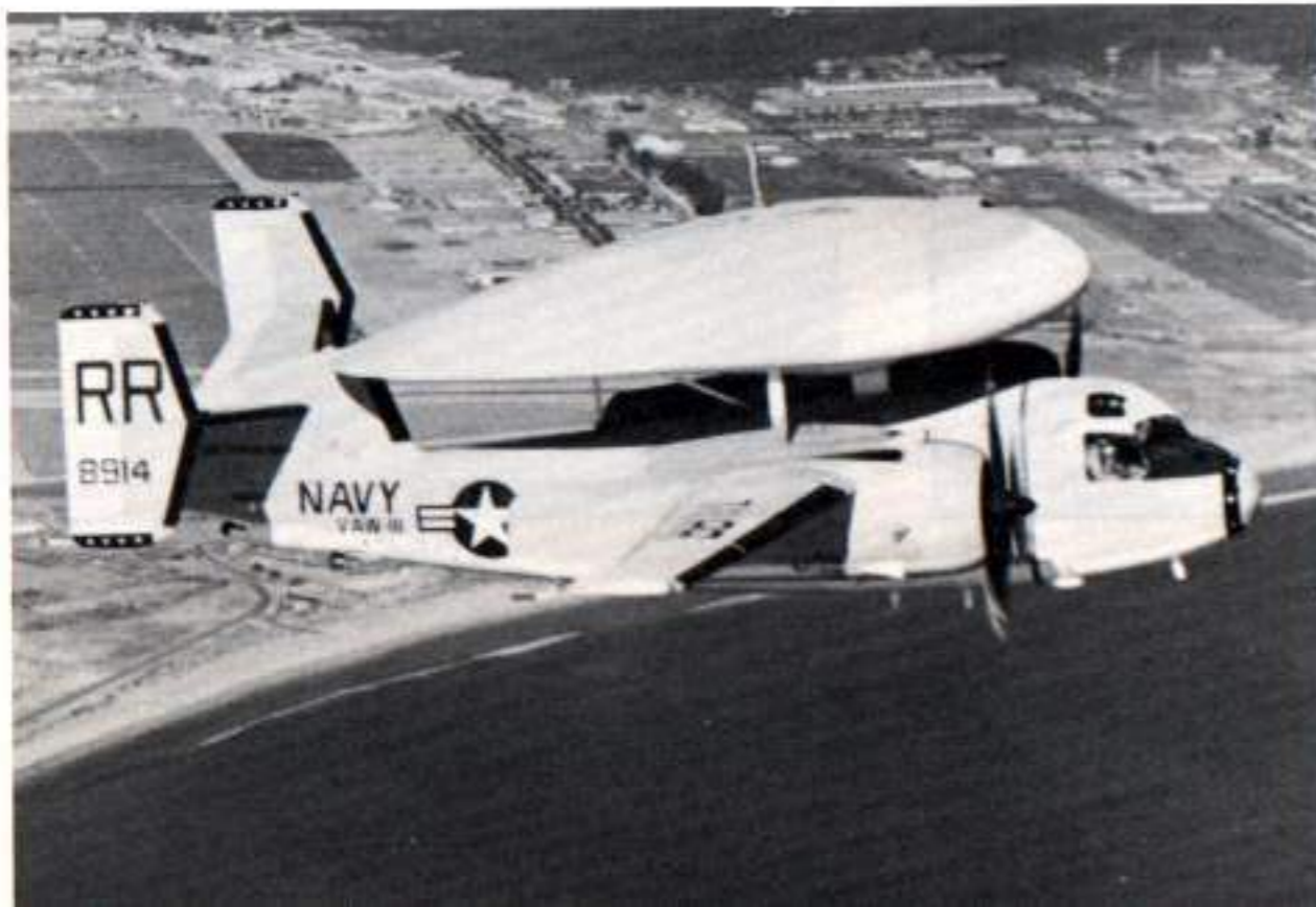
An E-1B (BuNo 148914) of VAW-111 over the sea near NAS North Island during 1972. The large dish mounted on top of the Tracer housed the APS-82 search radar antenna and actually contributed to the aircraft's lift. (U.S. Navy via Bill Curry)
