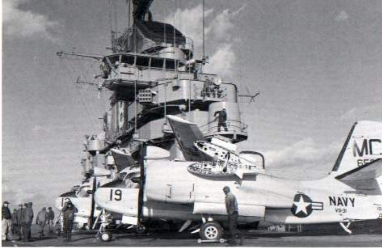
A pair of S2F-1 Trackers of VS-31 are parked on the deck of USS WASP during the Winter of 1959. The Tracker had an unusual wing fold system; the starboard wing folded in front of the port wing. (Grumman)
