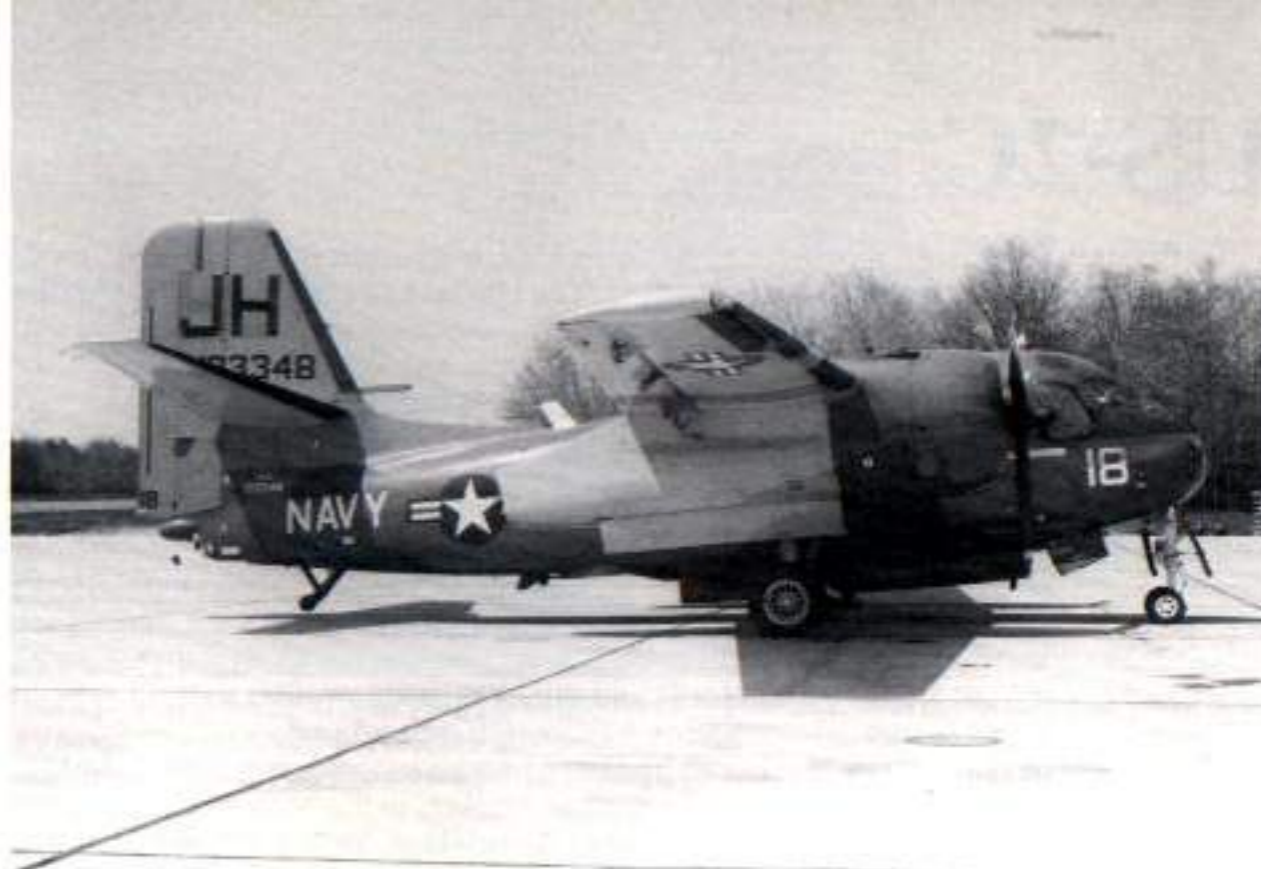
A US-2C (BuNo 133348) of VU-10 parked on the transient ramp at NAF Washington, DC, during 1972. The US-2C was a modification of the S-2C (S2F-2) with the searchlight, belly radome and internal ASW equipment removed. (Bob Esposito via Clay Jansson)
