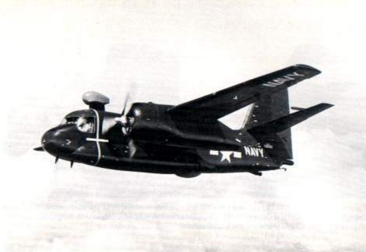
An early production S2F-2 (BuNo 133330) during factory acceptance flights. The horizontal stabilizer of the S2F-2 was nearly five feet longer than the earlier S2F-1 and the weapons bay was enlarged to accommodate larger ordnance loads. (Grumman)
