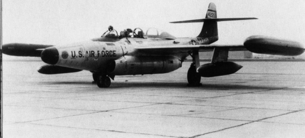
This F-89D of the 57th Fighter Interceptor Squadron was unusual in that it carried 600 gallon wing tip fuel tanks in place of the standard rocket/fuel tanks. The extra fuel was needed for the long flight to Iceland. The aircraft carries the Military Air Transport System (MATS) insignia on the nose since the 57th FIS was the only fighter unit ever assigned to MATS. (David Menard)
