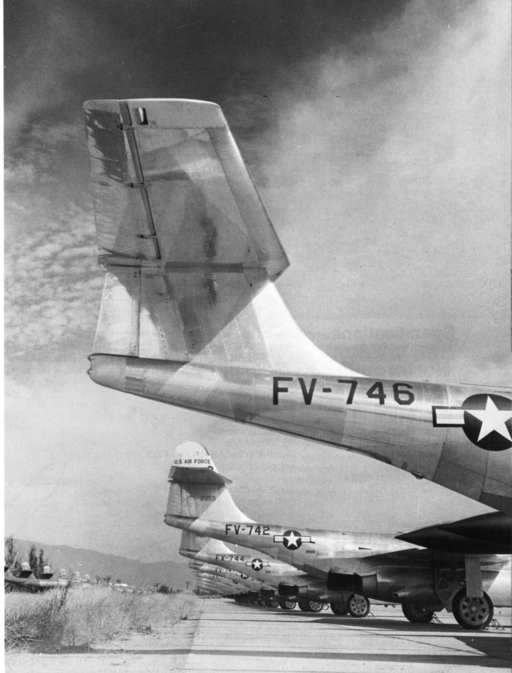
The F-89C differed from the F-89A/B in that it had an internally balanced stabilizer/elevator assembly, a redesigned jet wake fairing and a fuel system purge generator on the starboard engine nacelle. These modifications ended the F-89's tail flutter problem and made the Scorpion one of the safest aircraft in the Air Force. (Northrop)
