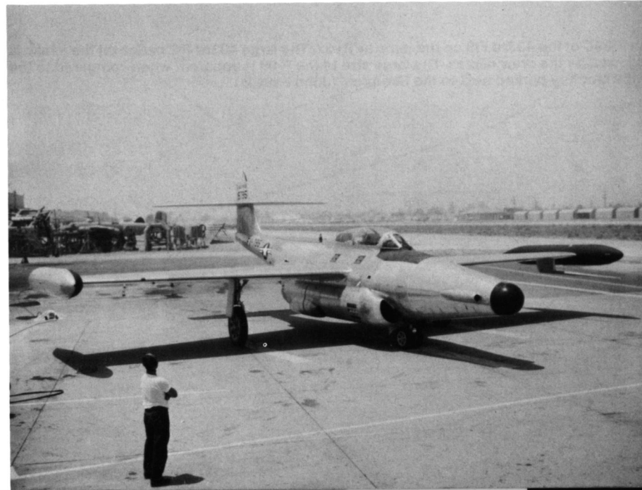
One of the armament experiments conducted with the F-89 was the use of two T-110 rocket guns mounted in the nose. The T-110 used a 2.75 inch spin stabilized rocket projectile which was fired through a rifled barrel. Once clear of the aircraft the rocket ignited, giving the projectile a range of 2,000 yards. (Northrop)
