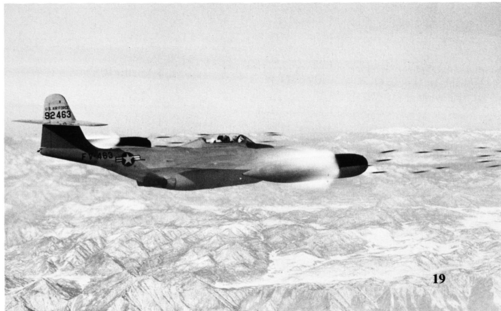
The YF-89D fires a salvo of the 2.75 inch FFARs on a test flight. All 104 rockets could be fired at once, or the pilot had the option to fire the rockets in volleys called ripples. The fire control system allowed for either two or three ripples to be selected. (Northrop)
