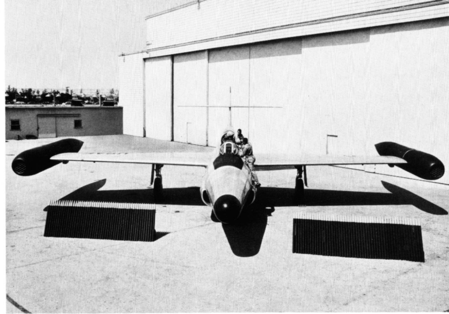
An early production F-89D was posed on the ramp with its full load of rockets lined up in front of it. One hit from a 2.75 inch FFAR was capable of bringing down any Soviet bomber then in service. (Northrop)
