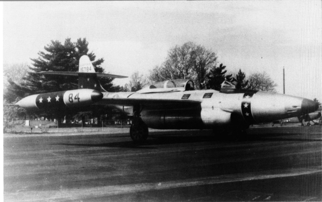
An F-89C of the 57th Fighter Interceptor Squadron (based at Presque Isle AFB) on the ramp at Ethan Allen AFB for an Open House during 1953. The bands on the nose, tail and tip tanks are Black with White stars and outline. The main landing gear doors are Black with a Yellow crescent Moon and stars. There is a Black flight leader's stripe on the rear fuselage. (via Marty Isham)
