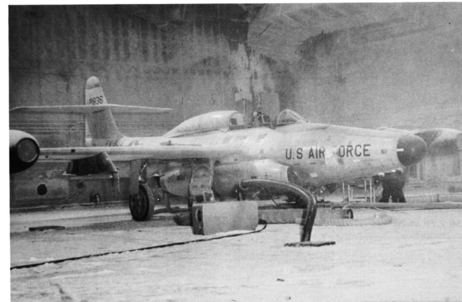
Every time the aircraft was changed during development, whether it was in electronics, engines or armament, cold weather tests were performed on the aircraft in the climatic hangar at Eglin AFB. Here the temperature could be dropped to -65 degrees, simulating the Winter weather in Iceland or Alaska. (Northrop)
