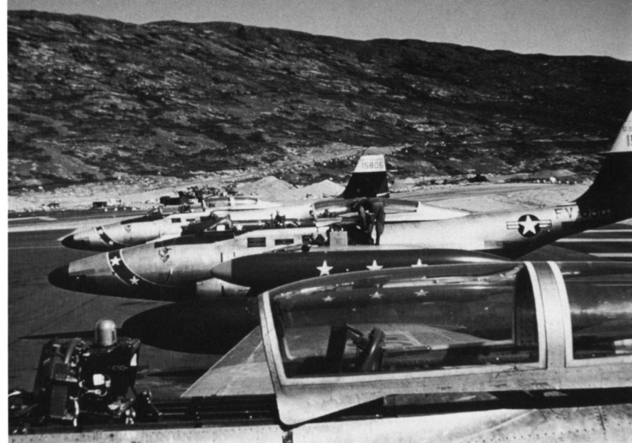
Three F-89Cs of the 74th FIS on the ramp at Thule, Greenland, during 1954. The 74th moved to Thule on 20 August 1954 from Presque Isle, Maine. The Arctic markings (Insignia Red FS12197) were required on all Air Force aircraft flown over snow covered areas as an aid in locating aircraft that might be forced down. (James Ford)
