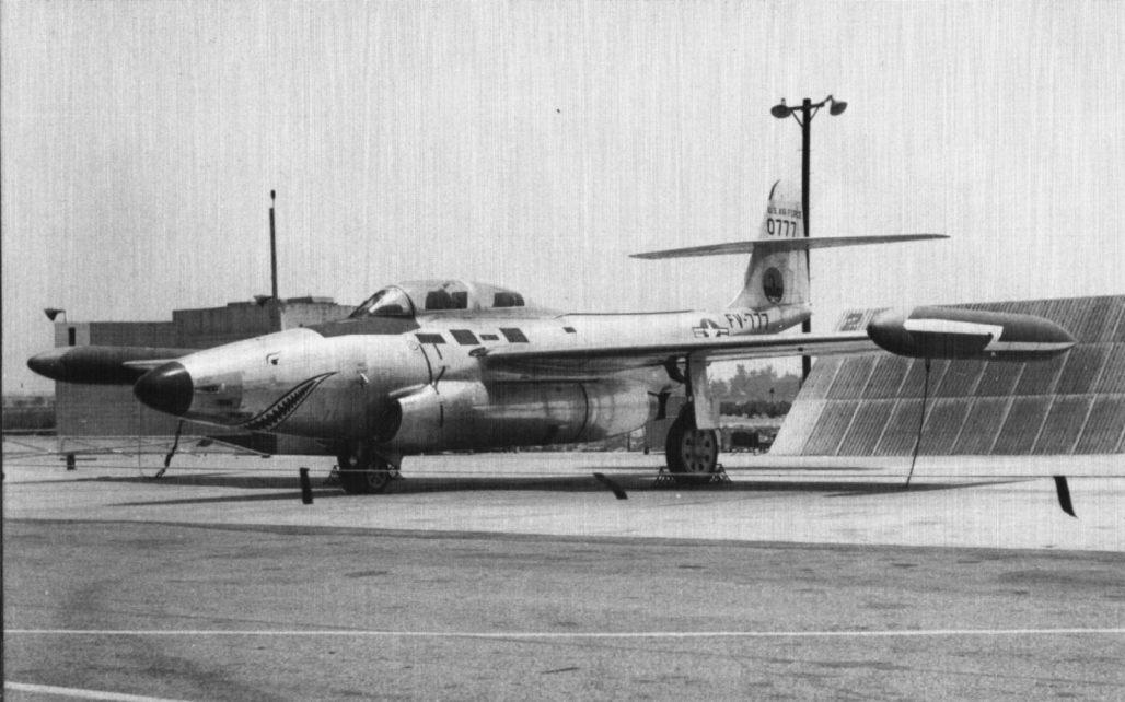
A shark mouthed F-89C-15 of the 433rd Fighter Interceptor Squadron at Truax AFB, Wisconsin. The first forty F-89Cs off the Northrop production line had the external mass balances on the horizontal tail. These aircraft (like this F-89C) were retrofitted with the internally balanced tail as soon as they were available. (William J. Balogh)
