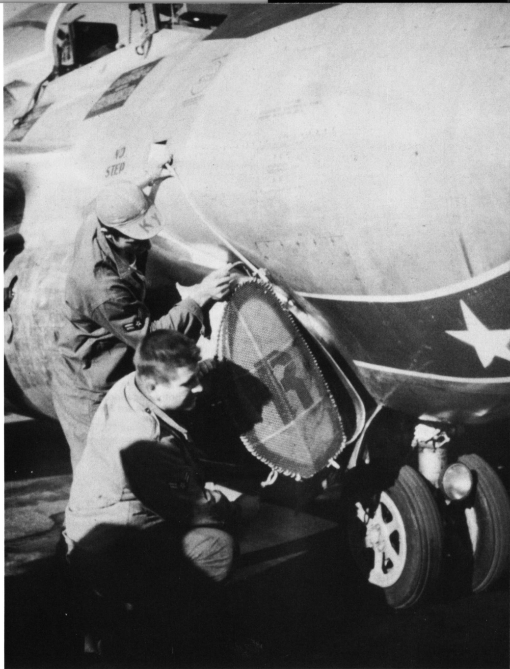
Ground crews attach external intake screens to an F-89C of the 74th FIS at Thule. Although the F-89C had electrically operated internal engine screens, these external screens were used to keep foreign objects out of the intakes of alert aircraft (which were exposed to the elements for longer periods). (USAF)
