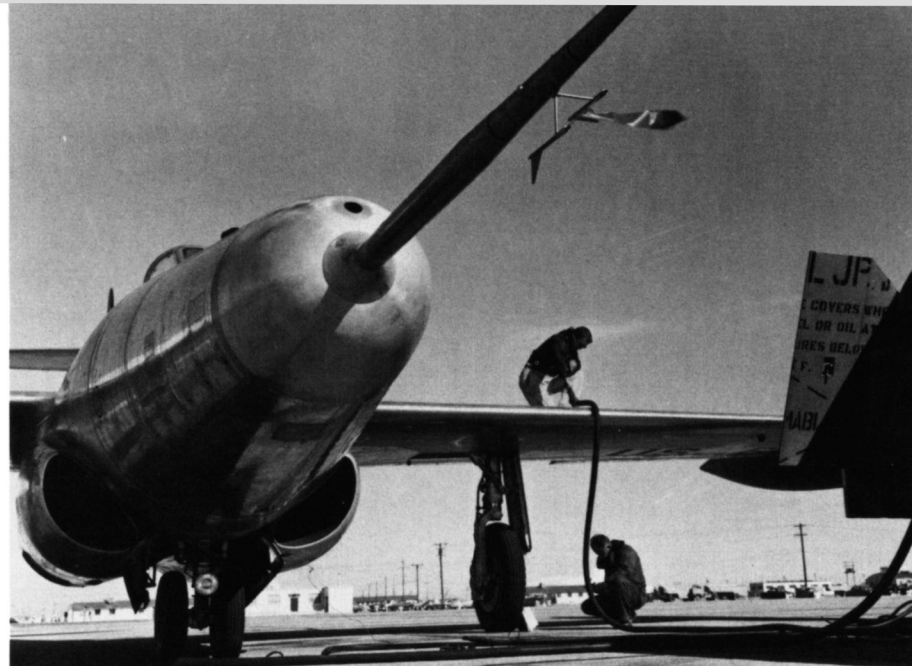
An F-89B (49-2463) was pulled off the production line and converted to the YF-89D prototype. The nose was recontoured to house the Hughes E-6 Fire Control System with its larger, flatter radome and a 260 gallon fuel tank was installed in the area formerly used for the guns. (Northrop)
