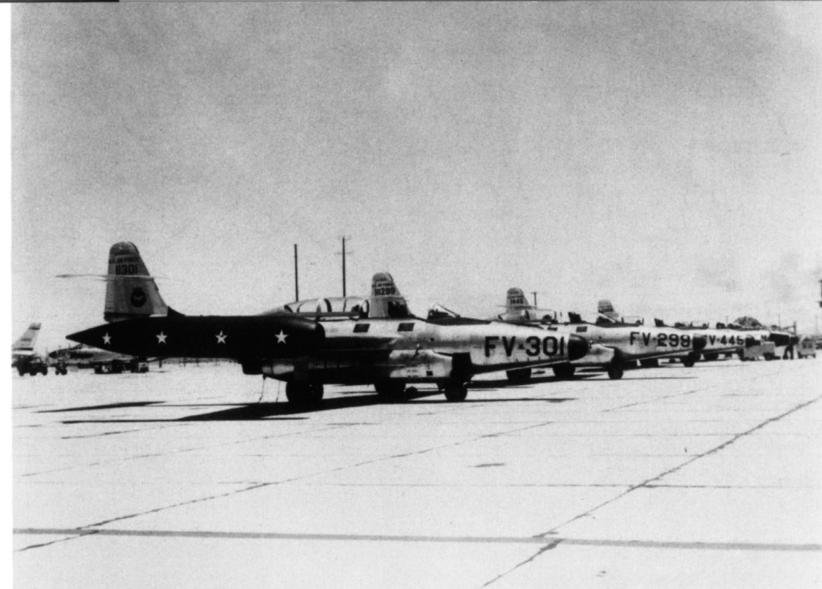
A lineup of F-89D-15s of the 3550th Combat Crew Training Wing (Interceptor) at Moody AFB during March of 1957. The 3550th was responsible for training of both air and ground crews for F-89 operational units. The placement of the buzz number on the nose is unusual. (via Marty Isham)
