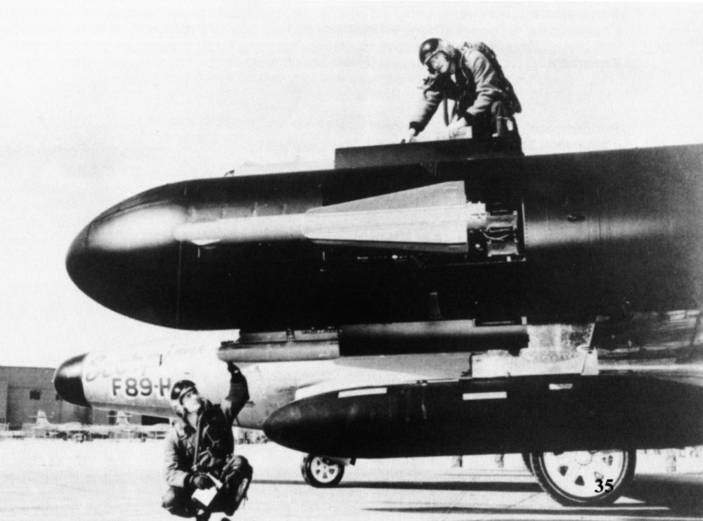
The Falcon missile bay had two fairing doors and a three rail launcher for the missile. These GAR-1 missiles are inert test airframes and are painted overall Light Blue. (AFM)
