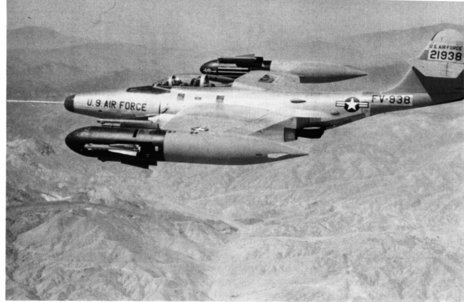
One of three F-89Ds that were converted to test the wingtip weapons/fuel pods that were configured to carry the Hughes Falcon air-to-air missiles, which would be the primary armament for the F-89H. The Falcons were carried inside the pods until ready for firing. (Barry Miller)
