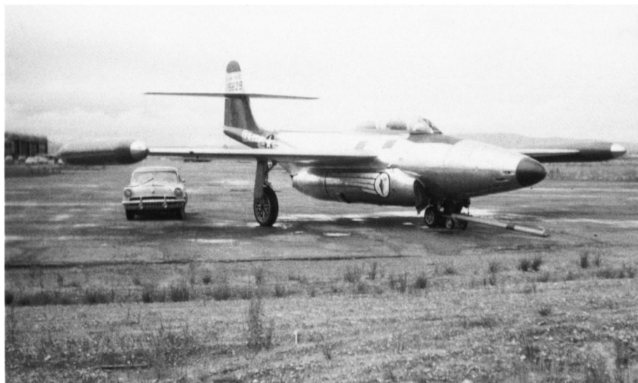
An F-89C of the 433rd FIS on the ramp at Truax. The large 433rd FIS badge on the intake is followed by the crew names. The large size of the F-89 is apparent when compared to the 1952 Mercury parked next to the Scorpion. (John Finiello)
