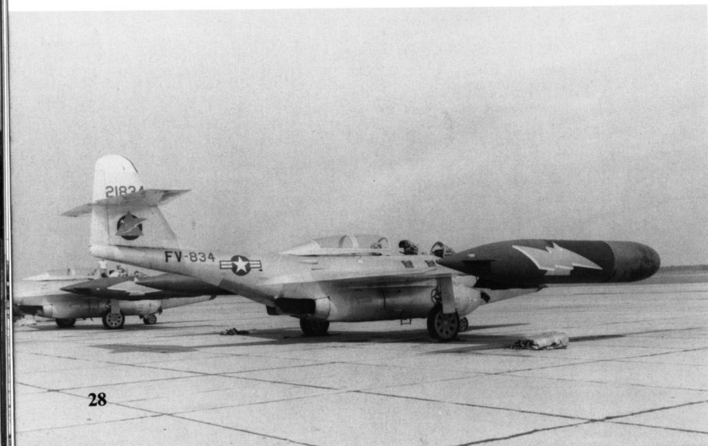
This F-89D is assigned to the 4750th Test Group at Tyndall AFB, Florida. The 4750th was responsible for tactics training in the F-89 and training crews in changes in the aircraft's systems and equipment. The small hole in the rear of the tip tank is the fuel dump pipe. (David Menard)
