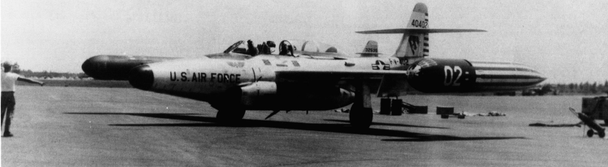
An F-89H of the 76th Fighter Interceptor Squadron at Pinecastle AFB, Florida. The 76th FIS moved from Presque Isle, Maine, to Florida during November of 1957. The stripes on the tip tanks and rudder are Red and White. The angled object under the fuselage is the barrier hook used to engage the crash barrier in an emergency. (Marty Isham)
