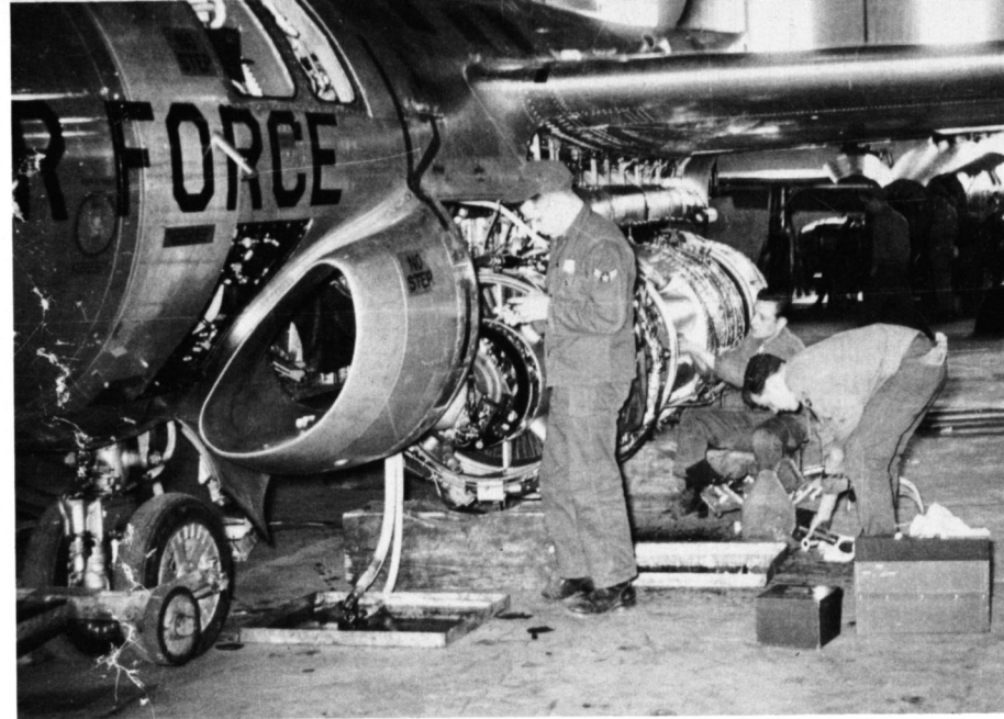
This J35-A-35 engine has been lowered using the internal hydraulic system of this 433rd FIS F-89D at Ladd AFB. During the early days of F-89 operations, crew chiefs and mechanics had to lower the engines onto mattresses when doing engine changes since dollies were in short supply. (John Finiello)
