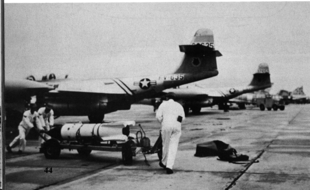
Armament crews at Ladd AFB, Alaska prepare to load a Douglas MB-1 Genie rocket onto the wing pylon of an F-89J of the 449th FIS. This unit retained the FFAR/fuel pods of the F-89D in preference to the standard 600 gallon fuel tanks normally carried by F-89Js. (Northrop)
