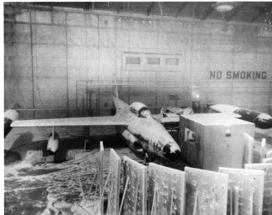
An F-89H parked in the climatic hanger at Eglin AFB, Florida, at -65 degrees Fahrenheit (similar to an Alaskan winter day). After sixteen hours, the doors were opened and a test crew scrambled the aircraft on a simulated mission. Fog, resulting from the cold air meeting the hot, humid Florida air, was so heavy that the propeller wash from a Beech C-45 was used to keep the entrance clear. (David Menard)
