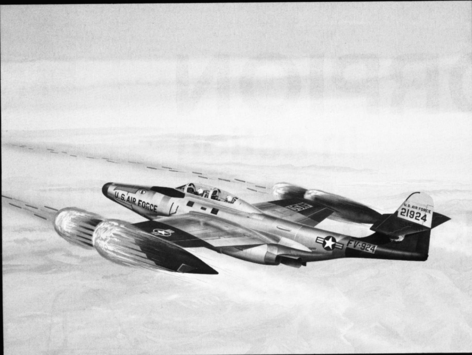
An F-89D Scorpion of the 449th FIS, fires a ripple of 2.75 inch Folding Fin Aircraft Rockets (FFARs) during an exercise at the Yuma firing range. The F-89D carried a total of 104 FFARs and when fired at the same time, the rockets covered an area the size of a football field.
