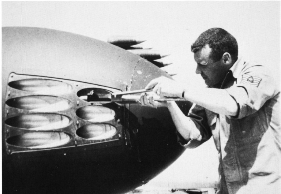
MSGT Dick Rosenthal, an armament specialist, loads 2.75 inch Folding Fin Aircraft Rockets (FFARs) into the seven shot rocket compartment of the Falcon/FFAR weapons/fuel pod on an F-89H during 1960.
