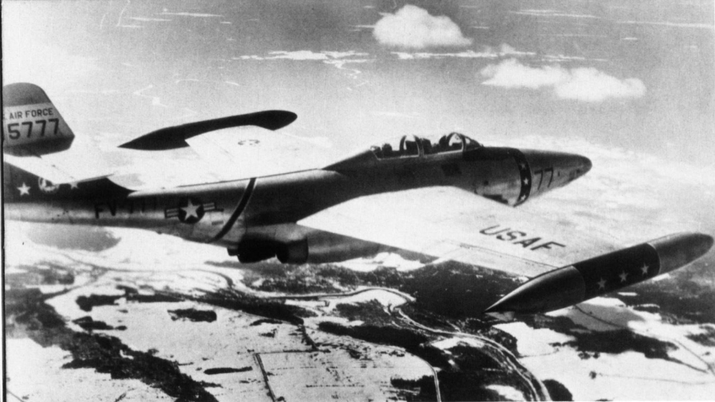
This F-89C of the 57th FIS at Presque Isle, Maine, is a flight leader's aircraft as identified by the band on the rear fuselage. The markings are identical to those of the 74th FIS with the exception of the Black Knight badge on the tail. The small fins on the wing tip tanks countered aero-elasticity, which twisted the wingtip and could cause a wing failure. (Bob Dorr via Marty Isham).
