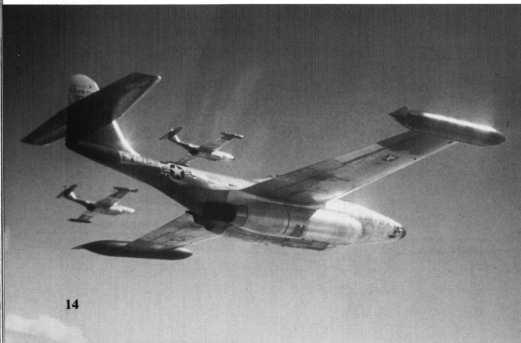
A flight of F-89Cs of the 57th FIS over Iceland during 1954. The 57th FIS moved from Presque Isle to Keflavik, Iceland, on 12 November 1954. The leading edges of the fin and horizontal stabilizers were left natural metal since the Red paint of the Arctic markings peeled easily at high speed. (Erroll Williams)
