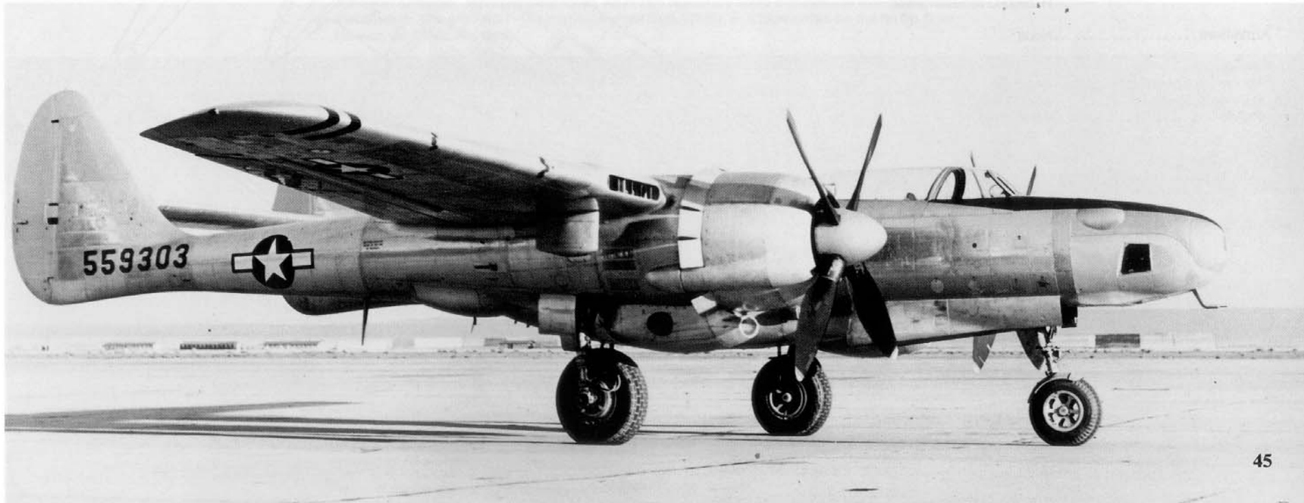
The F-15A-1 production aircraft was externally identical to the second XF-15 test aircraft, with the exception of P-61C engines, a slightly modified camera nose and a sliding canopy. (AFM)
