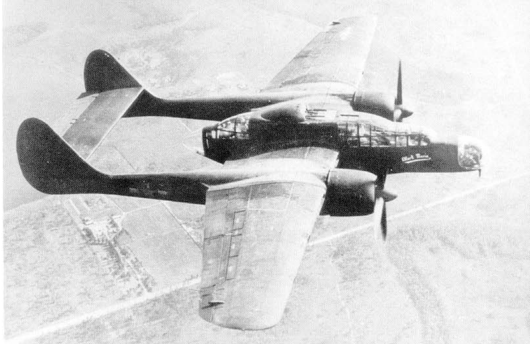
This YP-61 of the 481st NFOTG at Orlando, carried the name Black Maria on the fuselage side in White. The modified two gun dorsal turret was an attempt to alleviate the tail buffet problem. This YP-61 also had an opaque Plexiglas radome. (Jeff Ethell)
