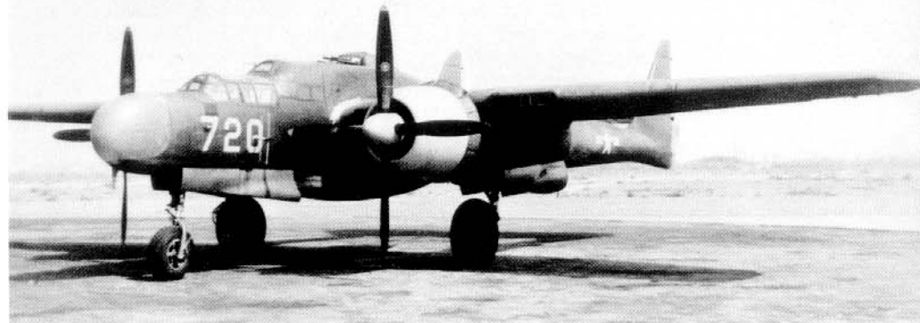
This P-61A-1 (42-5488) on the ramp at Northrop Field in Hawthorne, California, was the third production Black Widow. The aircraft carried Yellow spinners and cowlings indicating it was a Northrop test aircraft. The P-61A differed from both the XP and YP-61 in the canopy shape and camouflage. Early production P-61As were delivered in Olive Drab over Neutral Gray undersides. (AFM)
