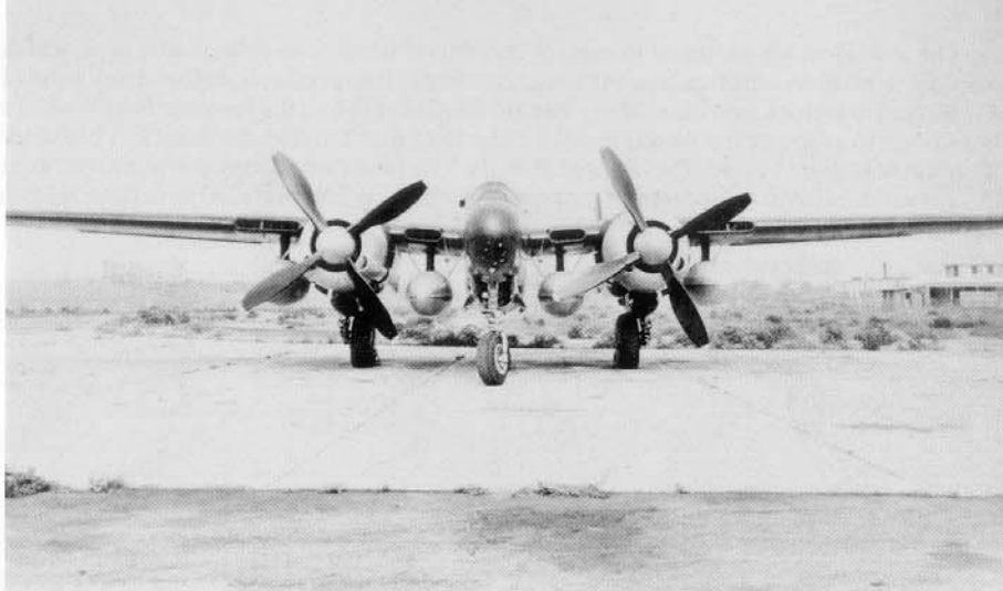
The second production P-61C reveals the distinctive shape of the cheek air intakes on the engine cowlings for the carburetors. The P-61C also had two additional underwing pylons mounted between the boom and fuselage allowing it to carry four 300 gallon underwing drop tanks. (AFM)
