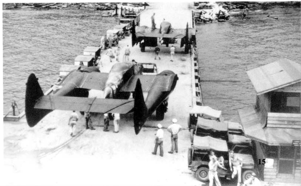
Most P-61s were delivered to the combat zones by ship, with their wings removed to make room on deck. This pair of P-61As of the 419th NFS were off loaded at Guadalcanal and towed up the causeway to Henderson Field where they were reassembled and made ready for combat. (AFM)
