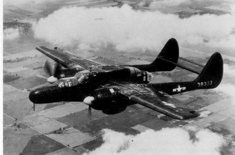
This P-61C was assigned to Hammer Field, California as a night-fighter trainer, preparing pilots for the F-82 Twin Mustang program. The de-icer boots have been removed from the leading edges of all the flying surfaces and the dorsal turret has been deleted and the opening faired over. (USAF)
