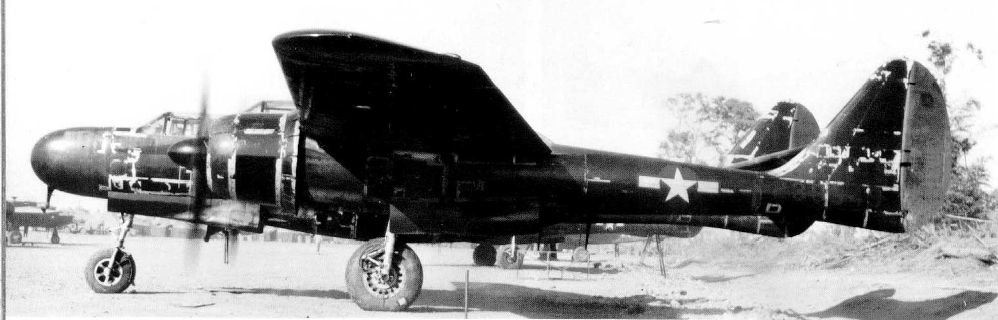
This P-61A-10 (42-39349) was assigned to the 427th NFS at Myitkyina, Burma, during January of 1945. The aircraft had a very patchy appearance because of the way the paint weathered and peeled along every panel line joint. (Ken Summney via Jeff Ethell)
