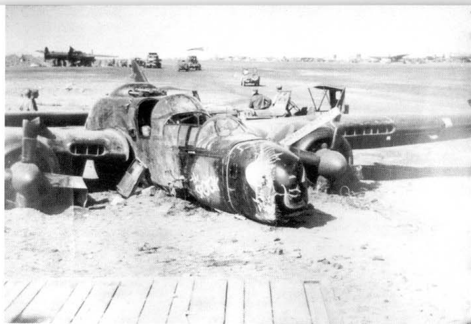
LT Mel Bode tried to land The SPOOK in a rare heavy fog on Iwo Jima. The left wingtip struck the ground, the Black Widow hit another P-61 and finally came to a halt 150 feet later. The impact of the crash set off all four cannons, which kept firing until they finally ripped completely out of the aircraft. (Northrop)
