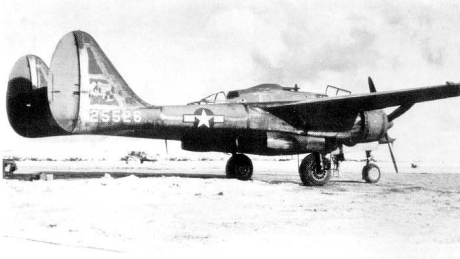
NIGHTIE MISSION was a P-61A-1 (42-5526) of the 6th NFS based at East Field, Saipan, during July of 1944. Although this aircraft was the 42nd P-61A built (the fifth aircraft after the dorsal turret was deleted), it retained the turret. Most 6th NFS aircraft were equipped with the turret. (Ernie McDowell)
