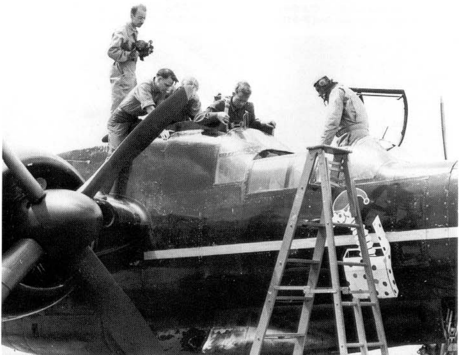
The General Electric Type A-4 remote control dorsal turret was armed with four Browning M2 .50 caliber machine guns. The guns are at maximum elevation and the flexible ammunition feeds are fully loaded. (Northrop)
