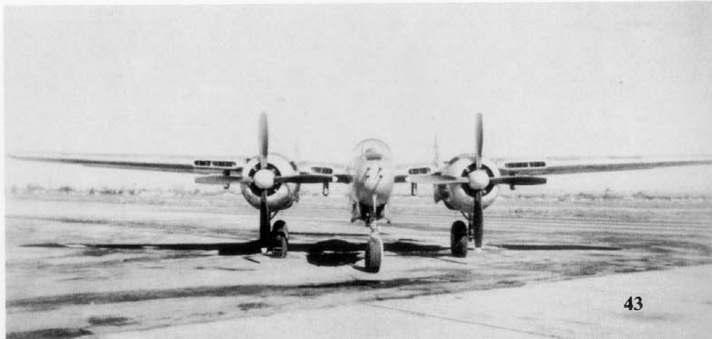
The first prototype on the ramp at Hawthorne. The four .50 caliber machine guns were arranged above and below each other, with the bottom two guns slightly further apart than the top guns. (Northrup)
