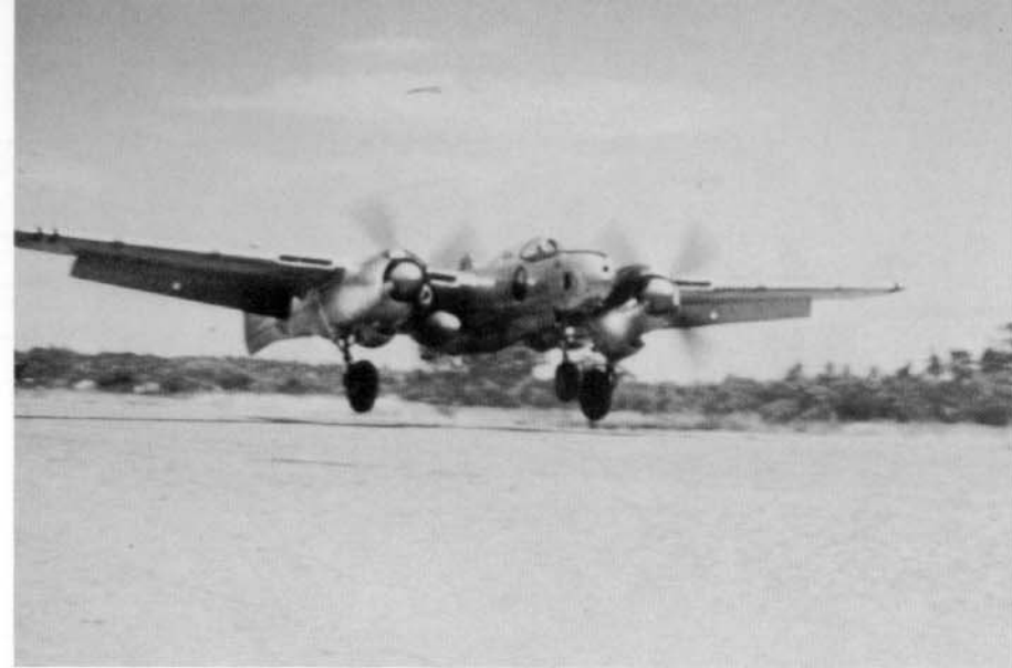
An F-15A Reporter of the 8th PRS takes off from its home base of Johnson Air Base, Japan. The dark hole in the center of the nose is the camera window for the forward looking oblique camera. (Linkiewicz via David Menard)
