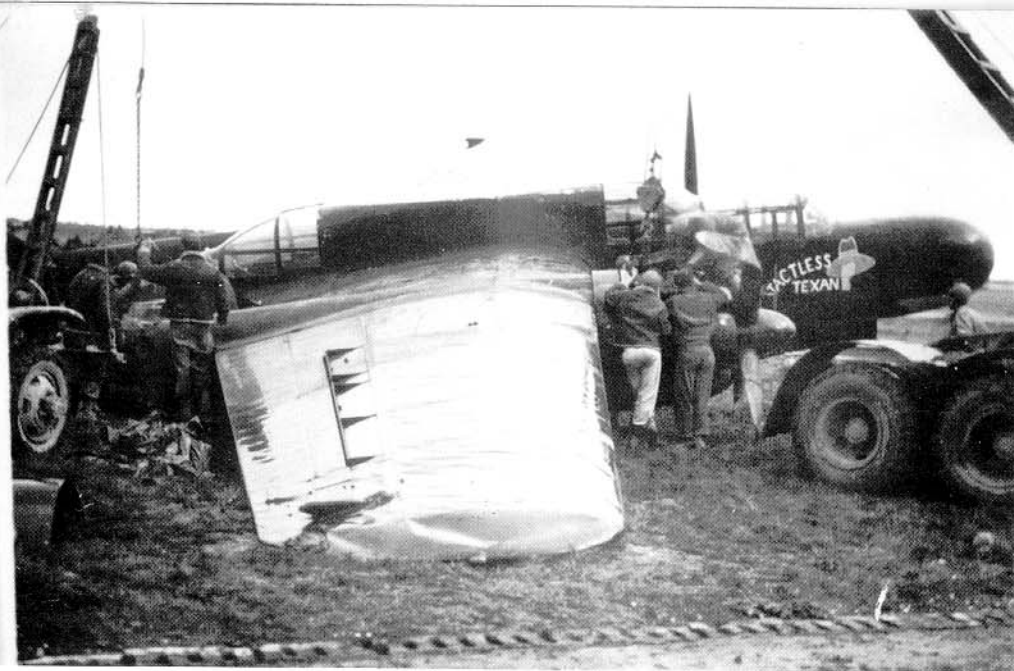
The TACTLESS TEXAN was a P-61A (42-5577) of the 422nd NFS. The Black Widow had the right wing tip and propeller damaged after the main landing gear collapsed on landing at Maupertus, France. The retractable ailerons are partially extended. (G. Stafford)
