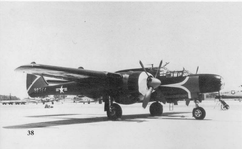
This P-61C was one of the black Widows used during Project THUNDERSTORM. The aircraft were assigned to Air Material Command and were flown into and through violent weather to determine the effects on aircraft. The nose flash is Red and Yellow as are the wingtip and tail markings, while the cowl ring was Yellow and the spinners were Red. (David Menard)
