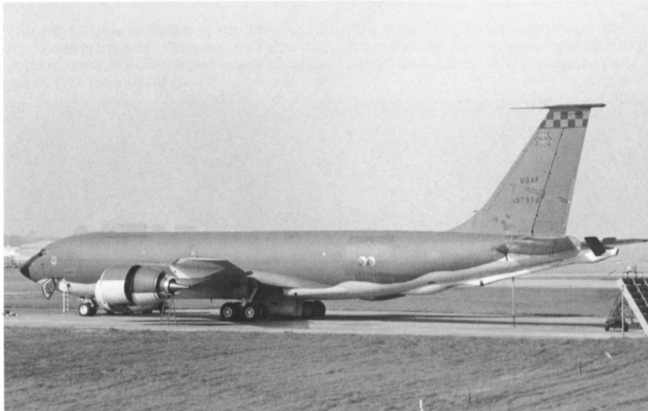
The two round ports on the fuselage side of this KC-135R (63-7978) of the 70th ARS, 305th ARW are exhaust ports for the auxiliary power unit. The tail band consists of Black squares against the aircraft's camouflage (originally the band was Black and White squares). (Simon Edwards)
