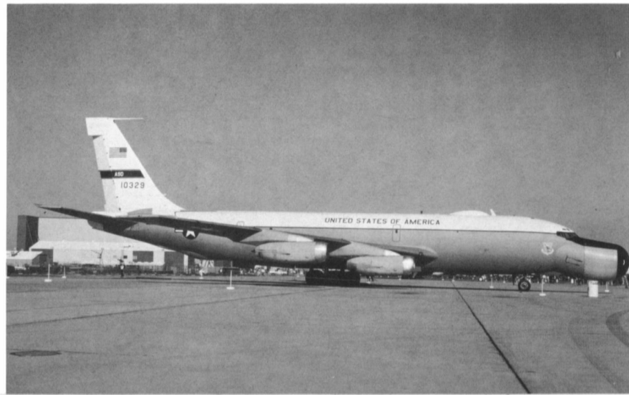
The nose radome on the EC-135N houses an eighty-five inch steerable antenna. These aircraft were first used to support the Apollo program but have since been modified as Advanced Range Instrumentation Aircraft (ARIA). (via Terry Love)
