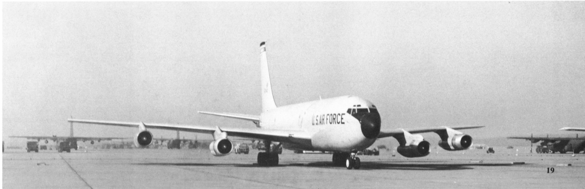
A KC-135E of the Arkansas Air National Guard on the ramp at Little Rock AFB. The KC-135E was basically a KC-135A with new TF-33 turbofan engines and enlarged horizontal stabilizers. (189th TAG)
