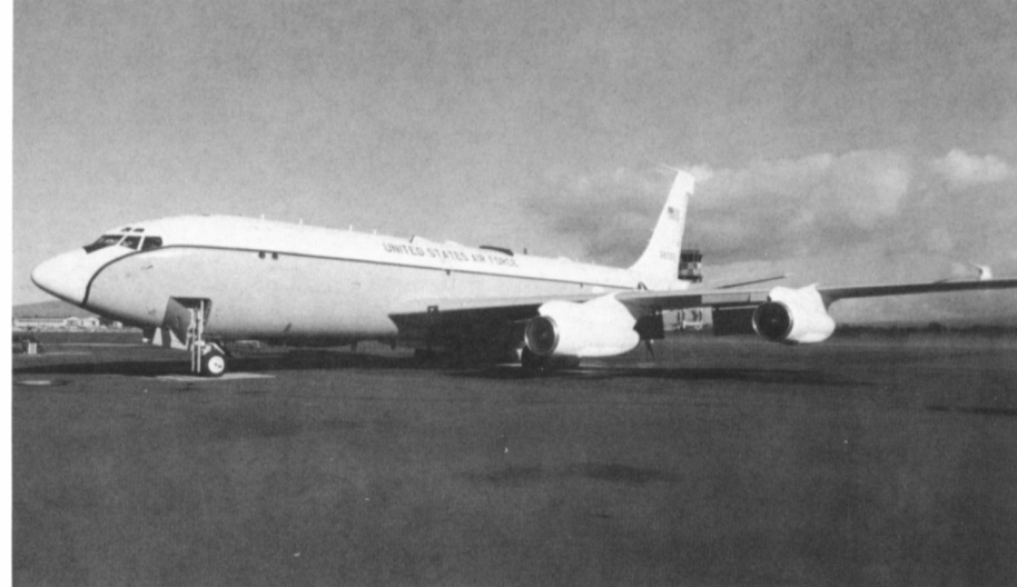
An EC-135J (63-8055) on the ramp at Hickam AFB, Hawaii. Externally the EC-135J is very similar to the earlier EC-135C, except for the three blisters on the upper fuselage for the new navigation system. (15th ABW)
