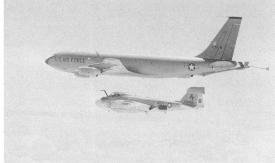
A KC-135A equipped with a drogue adapter on the Flying Boom flies formation with a Navy EA-6A Intruder. Through the use of the drogue adapter, KC-135s can refuel Navy aircraft as well as certain Air Force aircraft (such as the A-37) which use the probe and drogue method of refueling. (Larry Davis)
