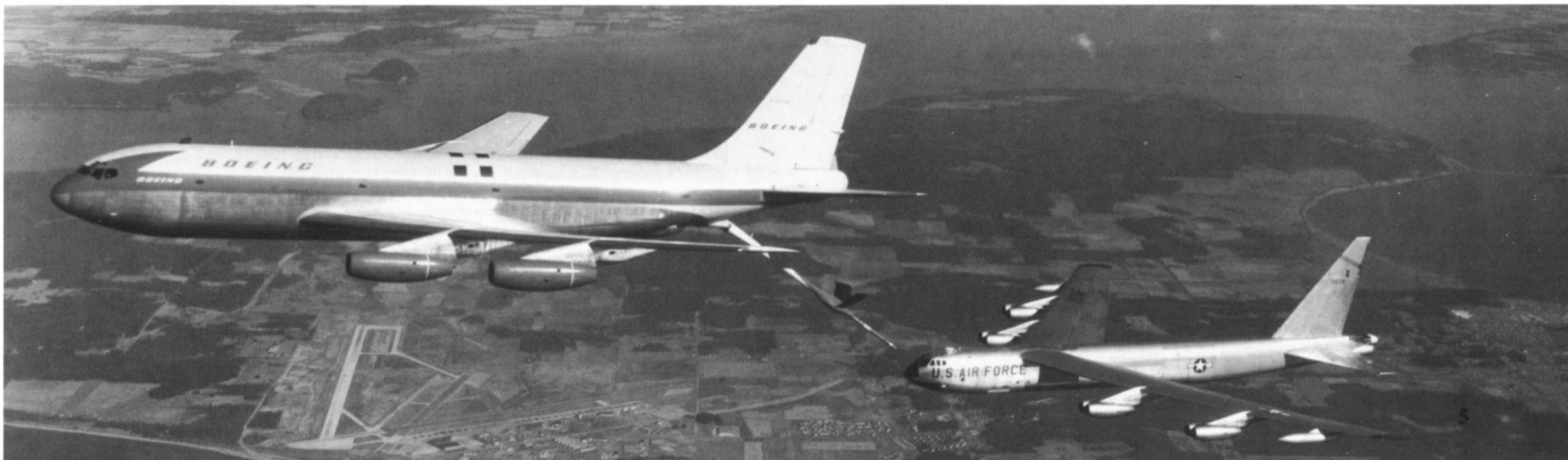
The Boeing 367-80 "Dash Eighty" prototype conducts a refueling test with an early B-52 Stratofortress. The prototype was outfitted with a dummy flying boom for simulated refueling tests to determine approach and positioning data. (Boeing)
