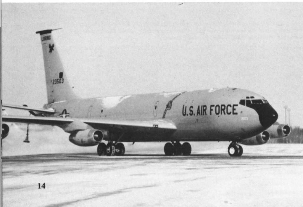
This KC-135 of the 42nd BMW has a drogue adapter attached to the Flying Boom. When the adapter is in place, the aircraft can only refuel aircraft that use the probe and drogue refueling method. (42nd BMW)
