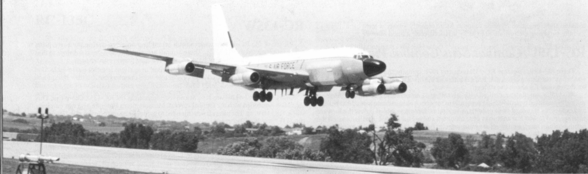
An RC-135V (64-14845) of the 55th SRW on final approach to landing. The RC-135V has numerous blade antennas mounted under the fuselage. As with most other RC-135 variants, the RC-135V began life as an RC-135B. (Via Terry Love)
