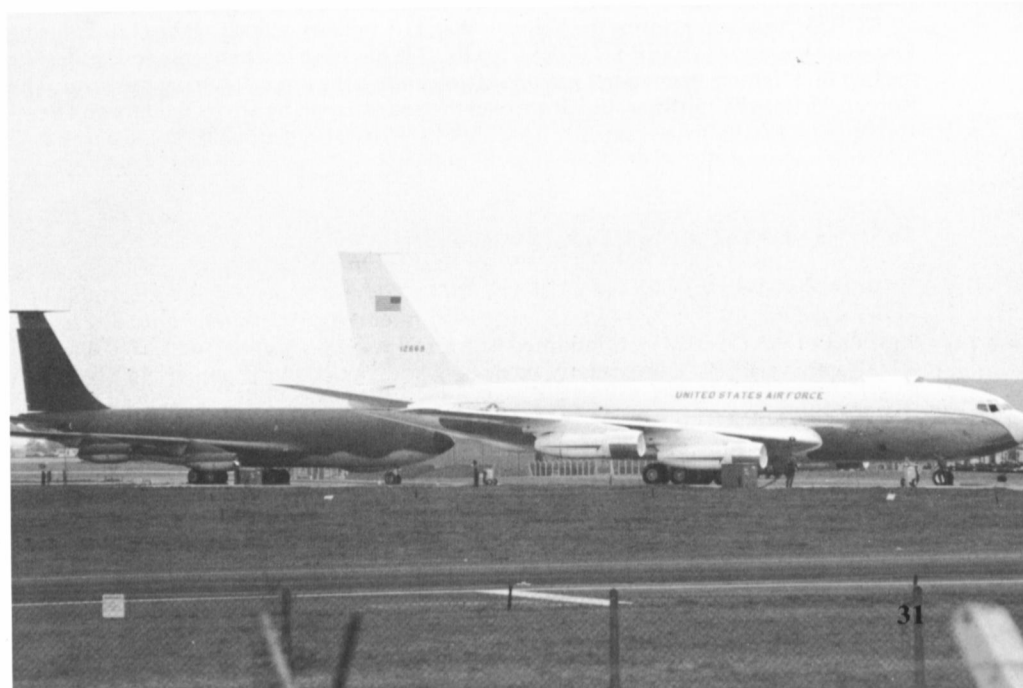
A C-135C staff transport shares the ramp at RAF Fairford, England with a camouflaged KC-135A during April of 1988. C-135Cs are used to ferry high-level Air Force and government officials. (Simon Edwards)
