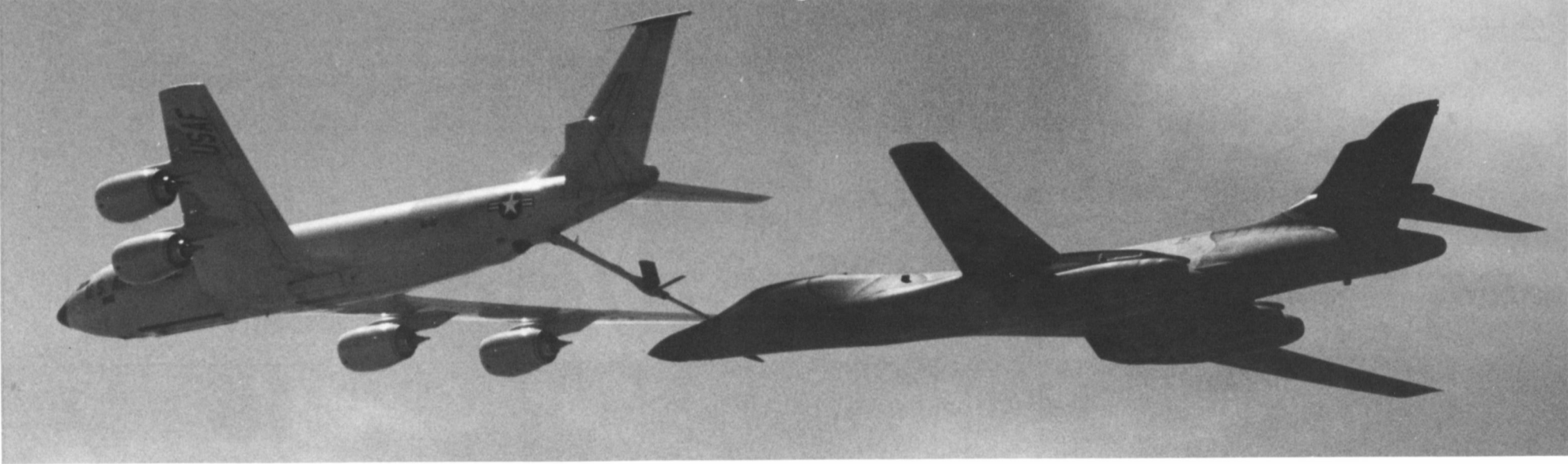
A KC-135R refuels a Rockwell International B-1B strategic bomber. Unlike most aircraft, the B-1B has the refueling receptacle mounted forward of the cockpit making it easier for the pilot to position his aircraft for refueling. (USAF)
