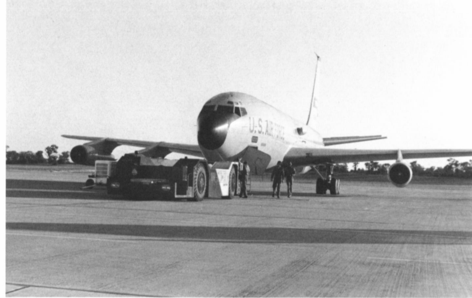
WC-135Bs are all conversions of C-135B transports. They have air sampling intakes mounted on each side of the fuselage and are powered by TF33 turbofan engines. (55th WRS)
