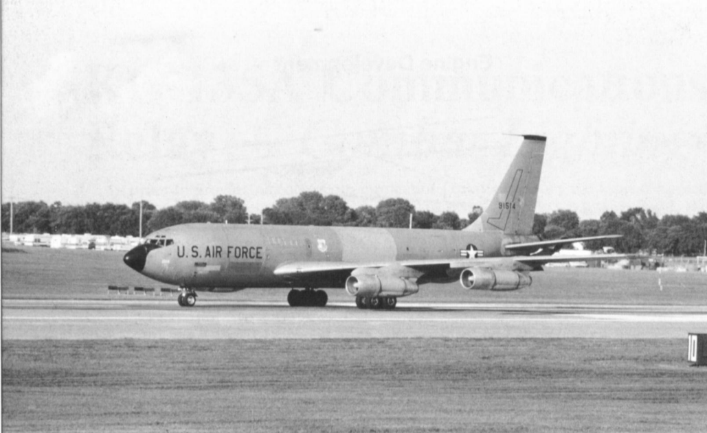
This KC-135E has the last four digits of the serial repeated on the nose in White. The aircraft also lacks the refueling area floodlight at the tip of the vertical stabilizer. (Via Terry Love)
