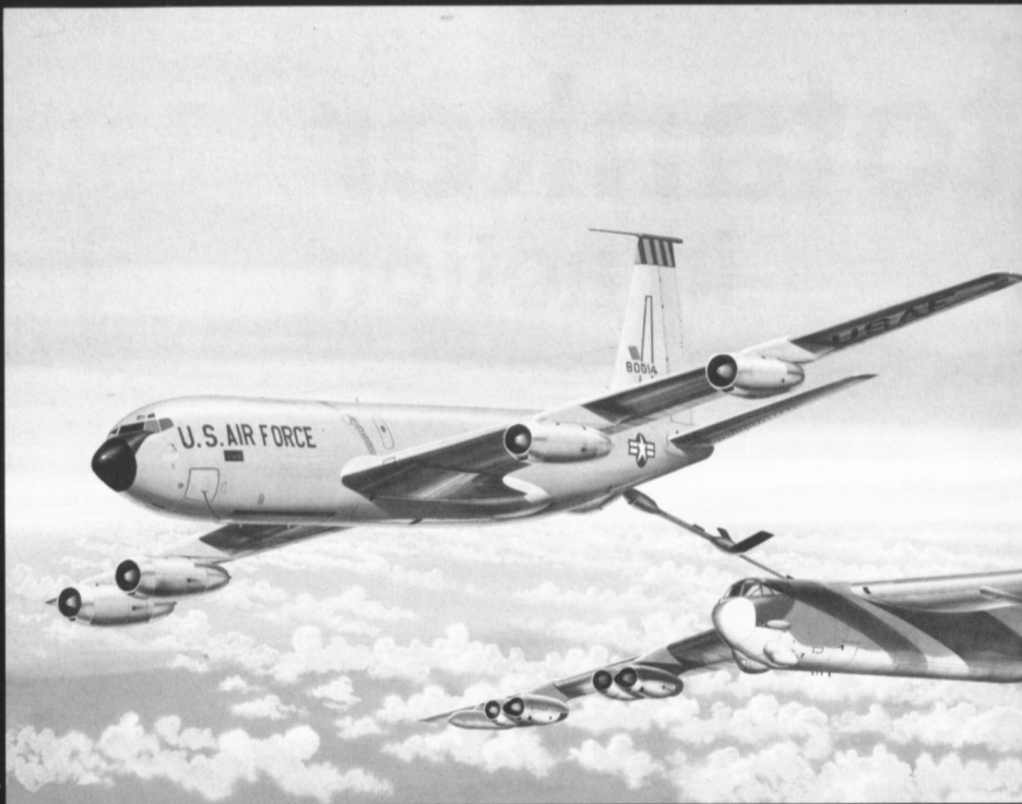
A KC-135A Stratotanker of the 379th Bomb Wing based at Wurtsmith AFB, Michigan, refuels a Boeing B-52 Stratofortress bomber. The primary mission of the Stratotankers in SAC is to support the B-52/B-1 bomber fleets.
