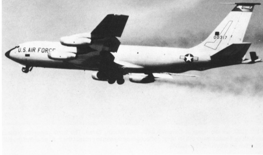
The smoke trail behind this KC-135A Stratotanker (60-0317) lifting off from Wurtsmith AFB, Michigan, was a characteristic of the J57 turbojet. This aircraft is painted overall ADC Gray with a Black radome and anti-glare panel. (379th BMW)
