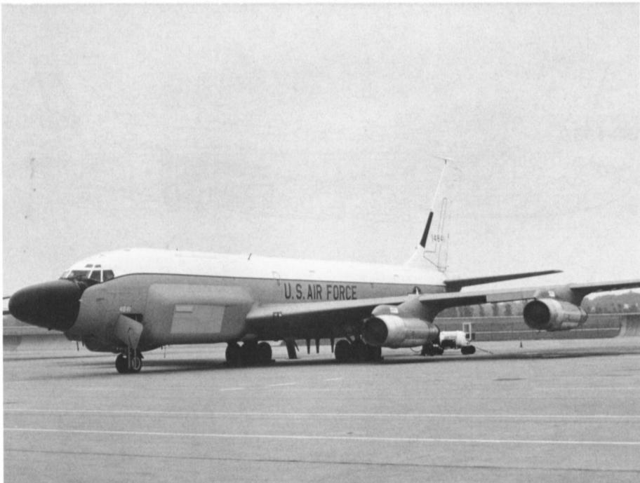
An RC-135W (64-14841) of the 55th Strategic Reconnaissance Wing. The engine pylons have small air intakes in the front of each pylon that supply air to the air conditioners needed to keep the electronics cool. (Via Terry Love)
