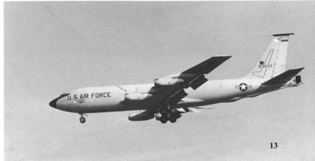
A KC-135A (56-3632) Stratotanker on final approach for RAF Fairford during 1988. This aircraft was one of the few early KC-135As that was not converted to either an NKC-135A test aircraft or rebuilt as a KC-135E. (Simon Edwards)
