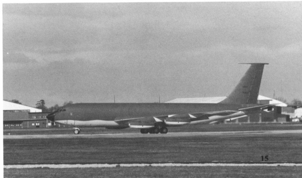
This KC-135A has been camouflaged in Dark Gray uppersurfaces over Light Gray undersurfaces. The aircraft has all codes, serials and national markings in Black while emergency markings and exit markings are in Red. (Simon Edwards)
