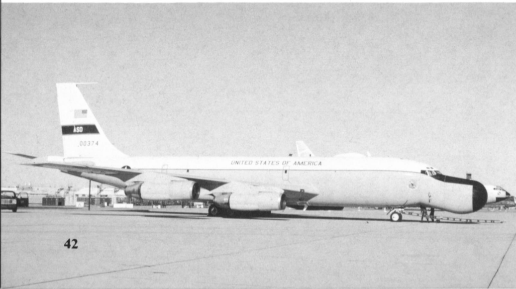
An EC-135N of the Aeronautical Systems Division, 4950th Test Wing, Air Force Systems Command. These aircraft carry special antennas to track space vehicles. (Via Terry Love)
