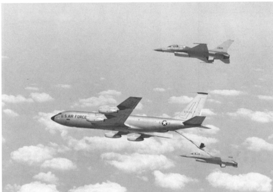
AKC-135A (55-3130) refuels a General Dynamics F-16A while a two-seat F-16B flies the wing position waiting his turn to move into the refueling position. (General Dynamics)
