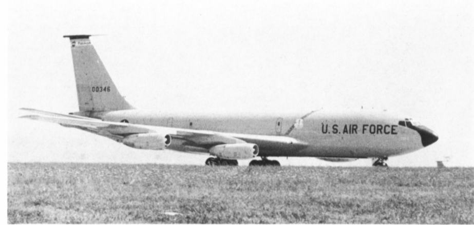
A KC-135Q (60-0346) on the taxiway at Plattsburgh AFB. The KC-135Q was externally identical to the KC-1325A although internally it was specially reconfigured to carry JP-7, the primary fuel for the SR-71 Blackbird strategic reconnaissance aircraft. (380th BMW)
