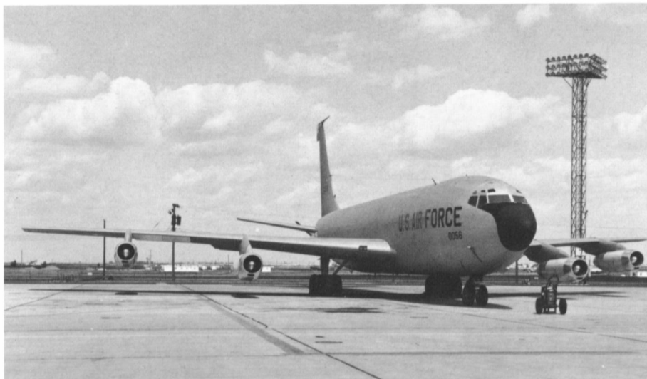
The small openings beneath the main air intakes on the J57 turbojet engine pods of this KC-135A are cooling air inlets for the oil radiators. The small rectangular opening on the wing leading edge near the fuselage is the housing for a pair of landing/taxi lights. (57th AD)
