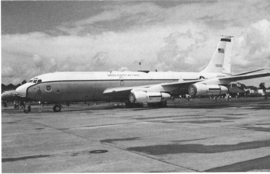
An EC-135H Silk Purse based at RAF Mildenhall, England. Four EC-135Hs are assigned to Mildenhall as Airborne Command Posts for the U.S. Commander in Chief Europe (CINCEUR). They have been updated with TF33 turbofan engines. The blisters in front of and behind the saddle antenna are part of a satellite navigation system. (Simon Edwards)
