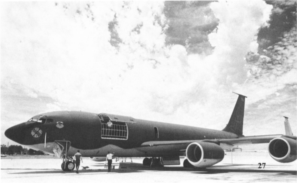
The large cargo door in the fuselage side of the KC-135R gives the aircraft a cargo capacity, although the KC-135R is not primarily an airlift aircraft. (443rd MAW)
