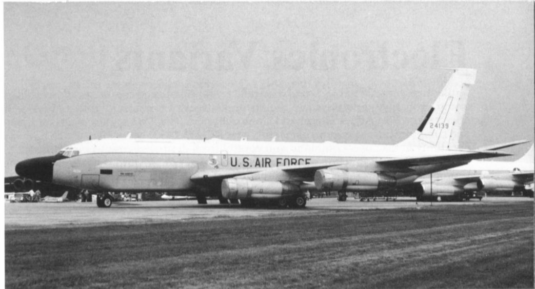
An RC-135V (62-4139) on the ramp at SAC Headquarters, Offutt Air Force Base. The RC-135V has numerous large blade antennas on the fuselage underside. (Via Terry Love)
