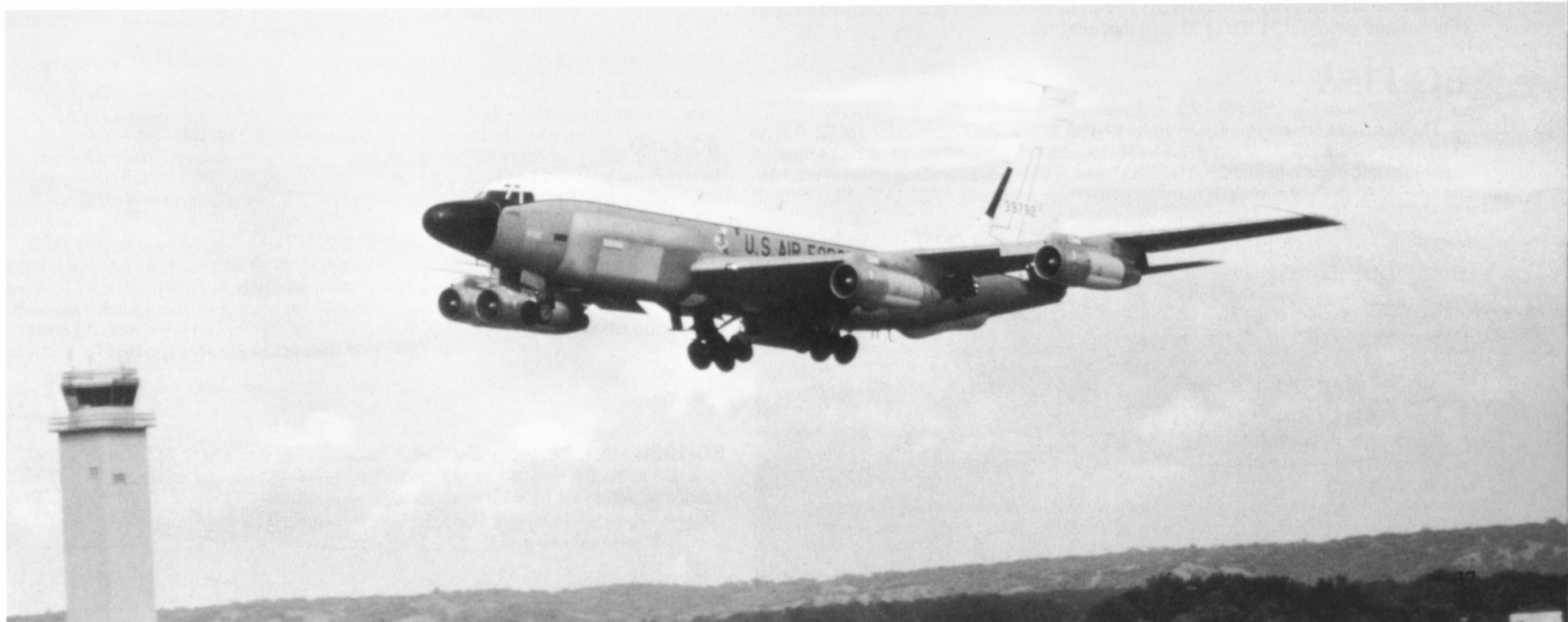
An RC-135W (64-14841) of the 55th Strategic Reconnaissance Wing. The engine pylons have small air intakes in the front of each pylon that supply air to the air conditioners needed to keep the electronics cool. (Via Terry Love)
