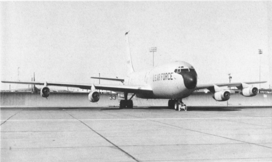
A KC-135A on the ramp at Carswell AFB, Fort Worth, Texas. The large concrete objects behind the Stratotanker are jet blast deflectors designed to protect the B-52s behind the KC-135 from jet exhaust. (7th BMW)
