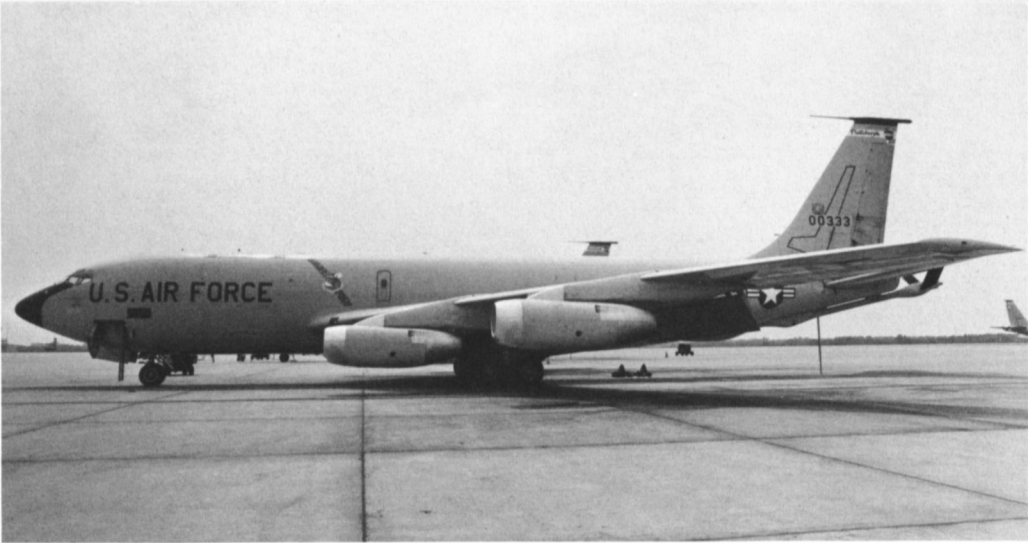
This KC-135A (60-0333) was part of the 380th Bombardment Wing and had been modified with the refueling area floodlight on the tin tip. The 380th operated a mixed force of KC-135As and KC-135Qs. (380th BMW)
