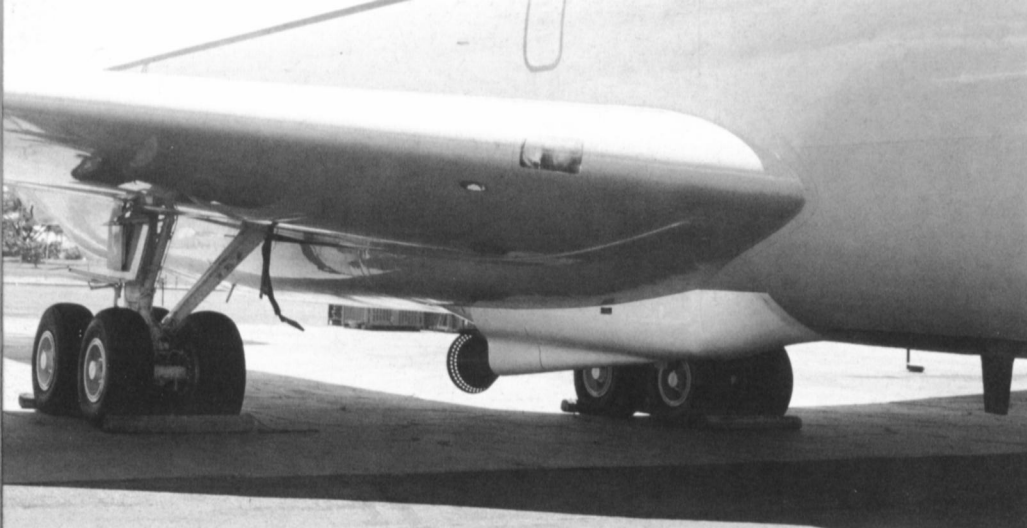
The Very Low Frequency (VLF) Trailing Antenna is carried in a housing faired into the fuselage underside. The basket on the end of the antenna helps keep the wire stretched out when deployed. (Via Terry Love)
