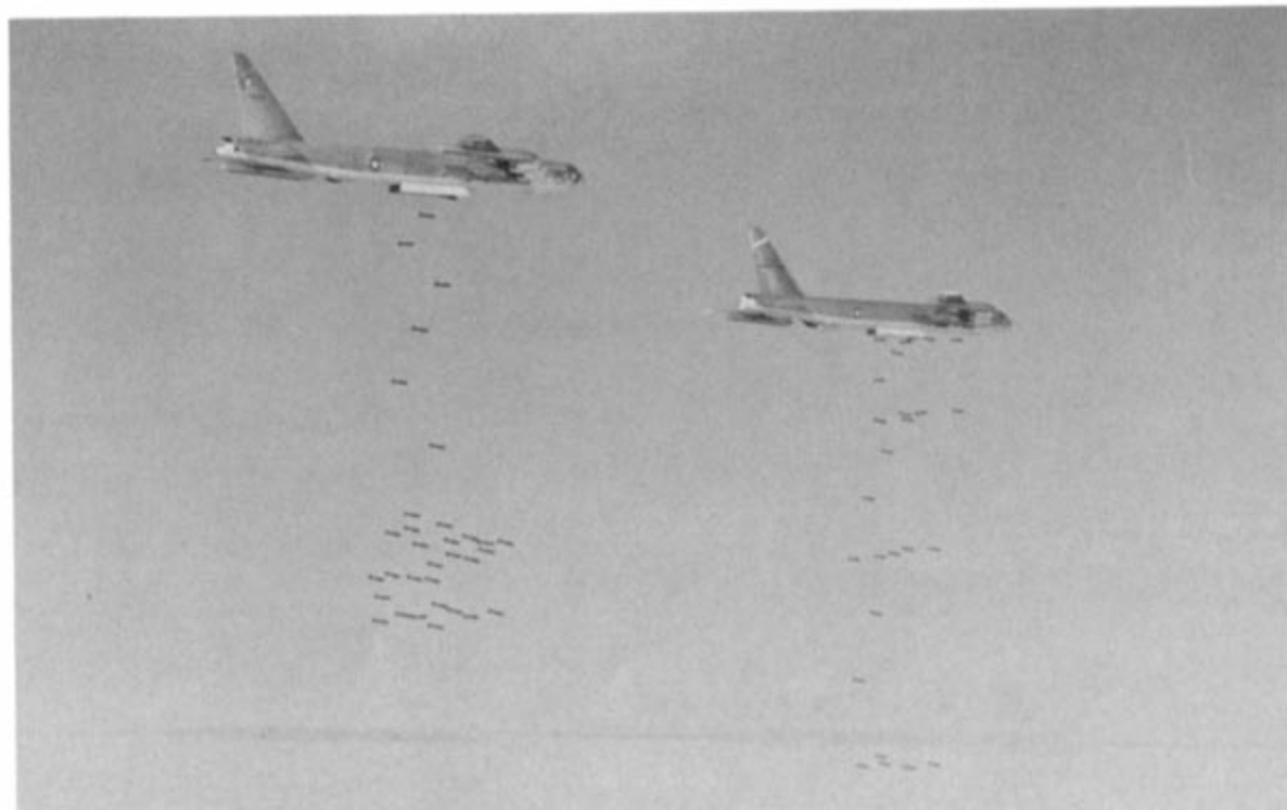
A pair of B-52Fs of the 454th Bomb Wing unloading their bomb loads on Viet Cong targets in South Vietnam during 1965. Each B-52F could carry a maximum of fifty-one bombs. B-52F operations were conducted under the code name ARC LIGHT. (Joe Bruch)
