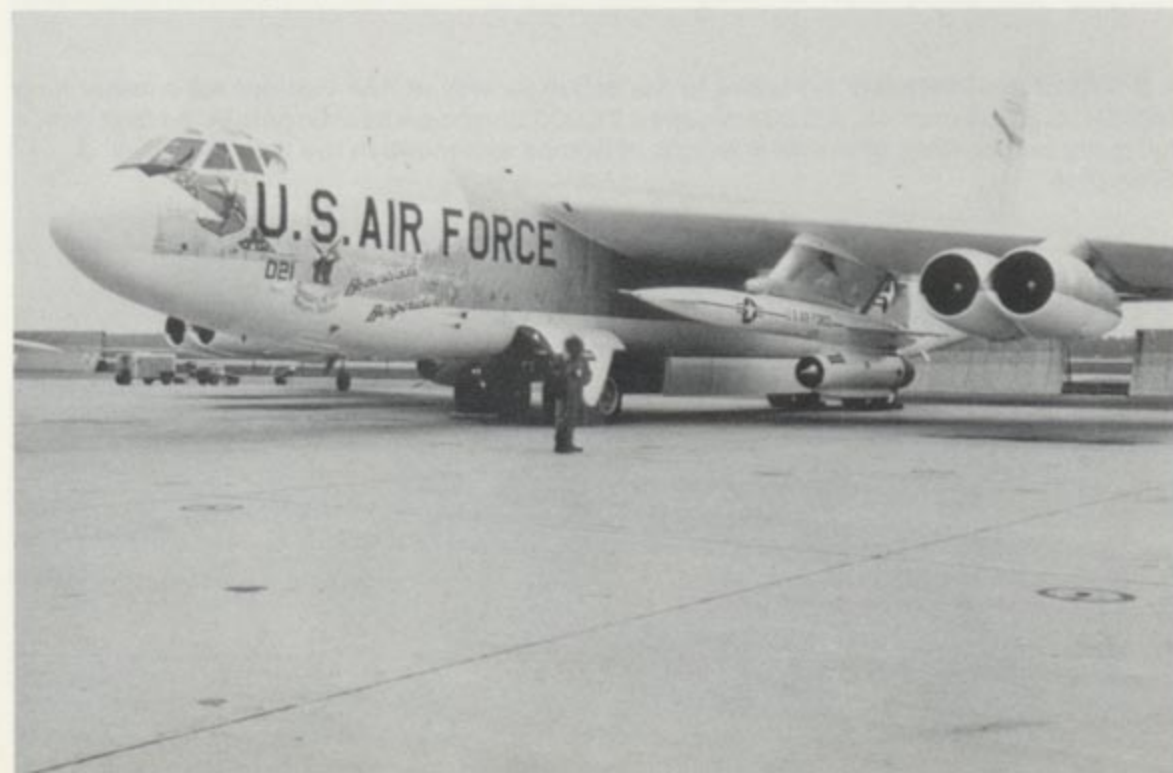
Homestead's Hesperides/Guardian Of The Golden Peace was a B-52H of the 19th BW based at Wurtsmith AFB during the Cuban Missile Crisis. The B-52H was powered by eight 17,000 lbst Pratt & Whitney TF-33 turbofan engines. (Joe Bruch)
