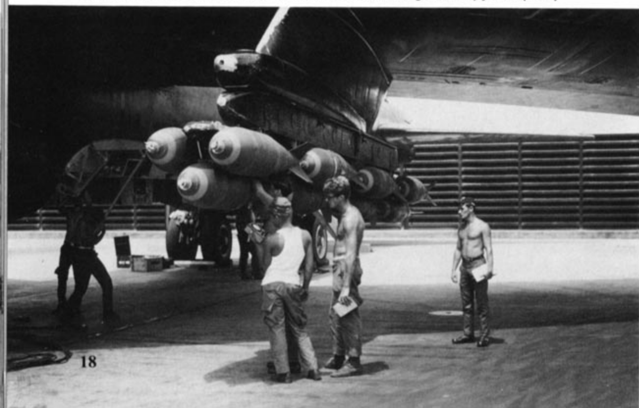
Armament specialists check the electrical circuits controlling the drop sequence of the Multiple Ejector Racks (MERs). The MERs are attached to Heavy Stores Adapter Beams (HSABs) which are, in turn, mounted to the AGM-28 Hound Dog missile pylons. (AFM)
