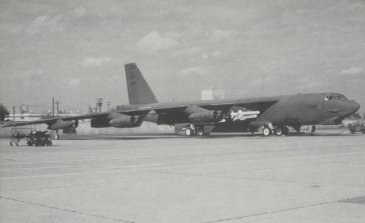
A B-52G of the 320th BW on ramp alert at Mather AFB, California in November of 1987 armed with twelve AGM-84 Harpoon missiles for a maritime patrol mission. The AGM-84 is powered by a small 660 pound thrust Teledyne jet engine. (Brian Rogers)
