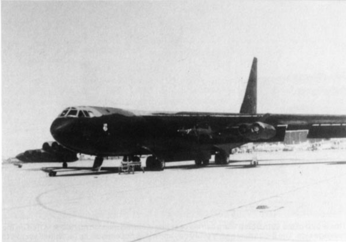
In the late 1970s many B-52Ds were modified to carry and launch the GBU-15 electro-optically guided bomb. This B-52D (55-676) carries a pair of GBU-15s on each MER and carries one NVAF MIG kill marking under the SAC badge. (AFM)
