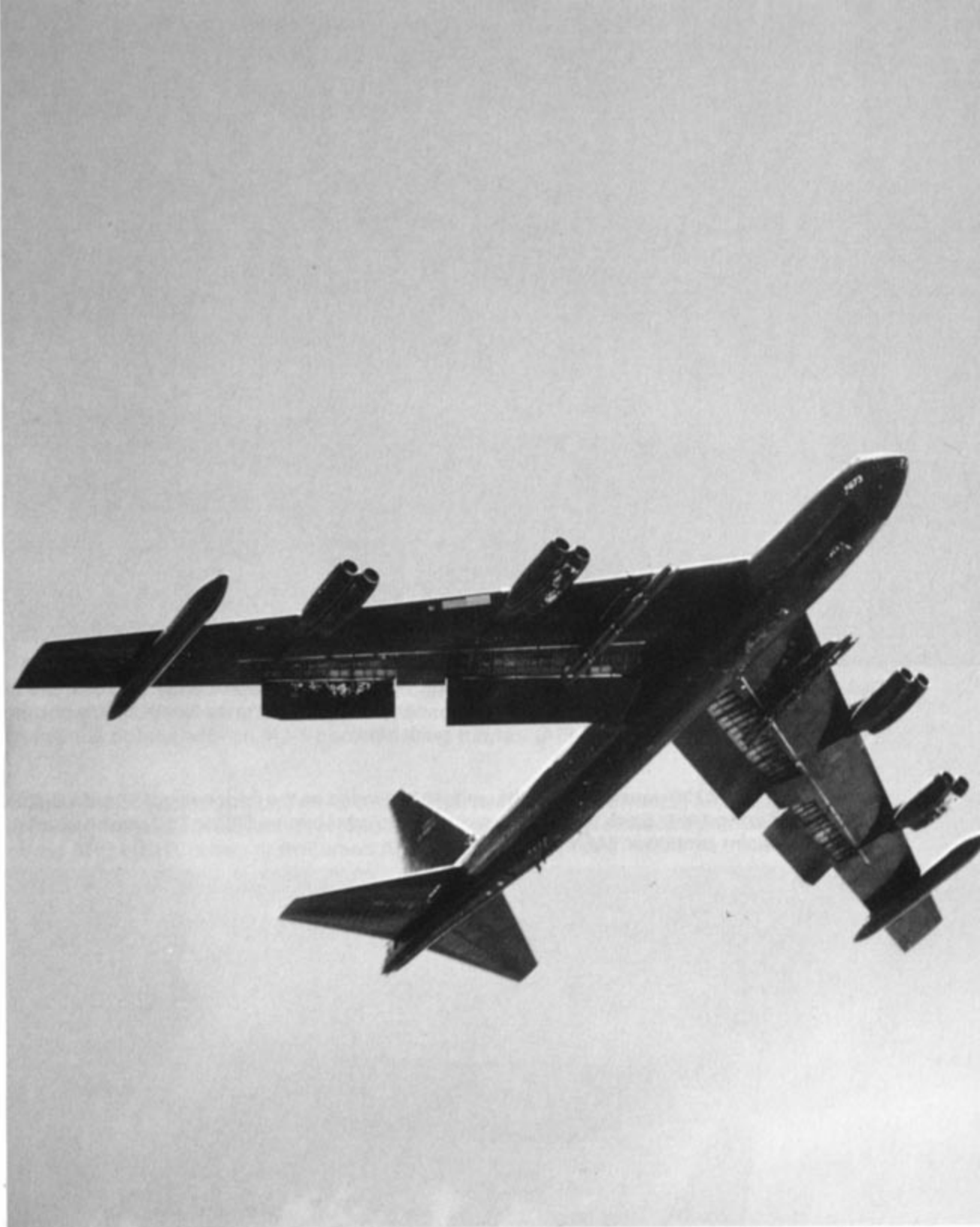
A fully loaded 43rd SW B-52D leaves Andersen AFB enroute to targets in Vietnam during 1970. This mission would involve a 5,400 mile round trip flight. The Black undersurface camouflage shows signs of extreme wear and paint peeling on the engine intakes and control surfaces. (Warren Skonieczny)
