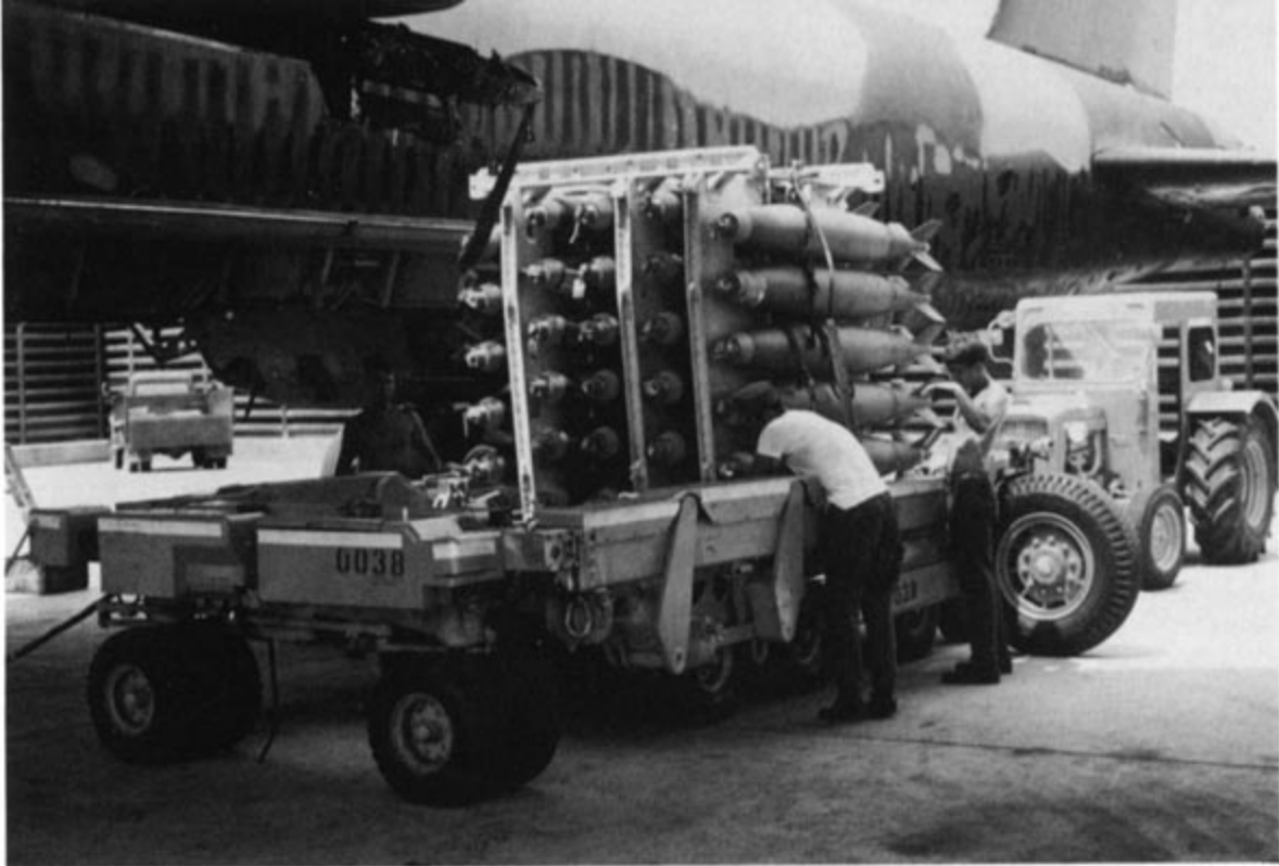
Readying a "clip" of twenty-eight Mk 82 500 pound bombs for installation in a BIG BELLY B-52D Stratofortress. Three of these High Density Bomb Racks, or "clips," can be loaded into the bomb bay. (AFM)
