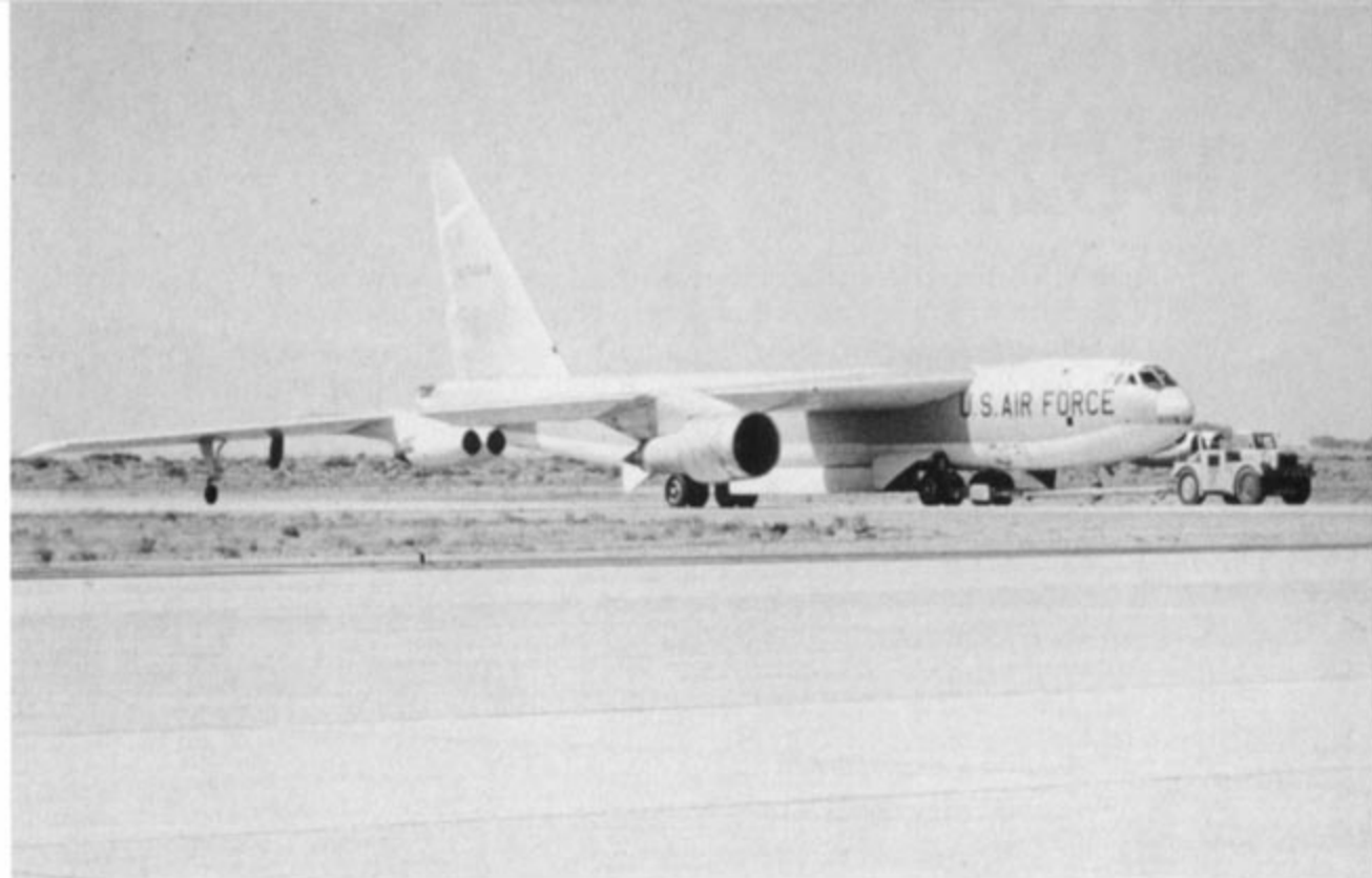
As with other B-52 variants, some of B-52Es were modified to test other equipment and systems. This NB-52E was fitted with a single GE JT-9D turbofan engine which was intended to power the Boeing 747 Jumbo Jet transport. (JEM Aviation Slides)
