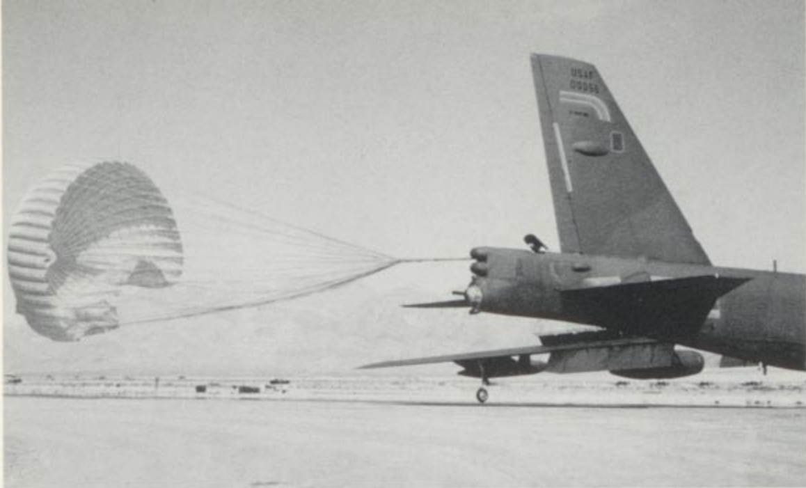
A 410th BW B-52H streams its drag chute and slows to a stop. The B-52H was armed with an M61 Vulcan tail turret and has the Phase VI ECM rear fuselage modification for the AN/ALQ-117 ECM equipment. The bulge on the side of the vertical fin is the AN/ALE-153 RHAW antenna fairing. (Brian Rogers)
