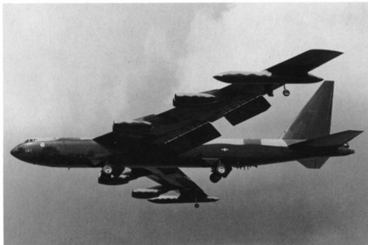
A 7th Bomb Wing BUFF on final approach with the flaps fully extended. By 1980 most of the remaining B-52D fleet had gone through the PACER PLANK program, which literally rebuilt the entire airframe. (Robert F. Dorr)
