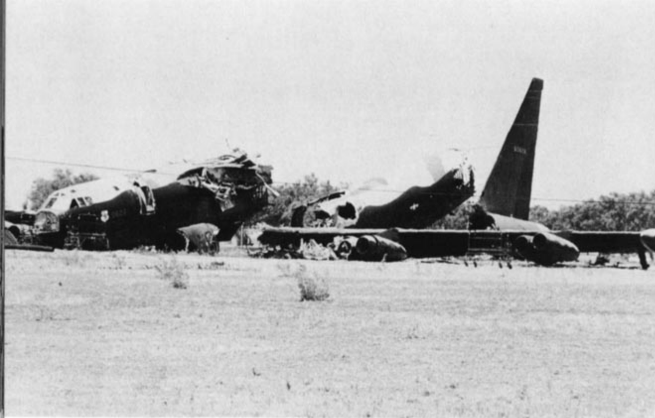
To assure the Soviets that B-52Ds were being destroyed in accordance with the SALT Treaty, many aircraft were destroyed through the use of shaped explosive charges which blew off the wings and cut the fuselage into sections. This B-52D was destroyed at Dyess AFB during the early 1980s. (Joe Bruch)
