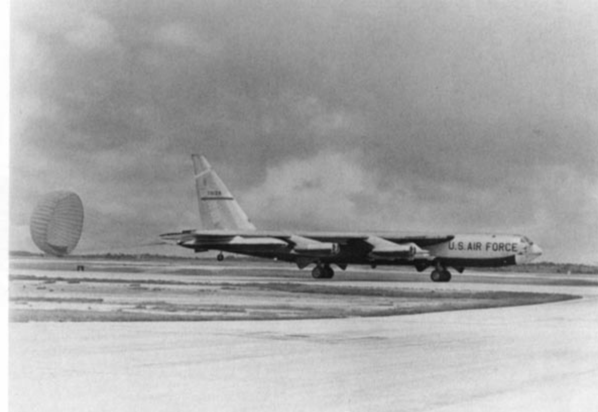
Streaming its drag chute, a 7th Bomb Wing B-52F rolls to a halt at Andersen AFB during early 1966. The Gloss Black undersurface camouflage began to appear on BUFFs in late 1965. The wingtips and outrigger landing gear are not touching the runway, an indication that the fuel tanks were at Bingo fuel (nearly empty). (Joe Bruch)
