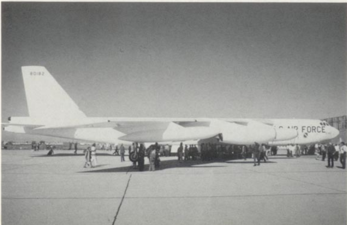
This overall Gloss White B-52G was assigned to the Air Force Flight Test Center at Edwards AFB during the mid-1970s, flying tests for the AGM-86 ALCM cruise missile program. The aircraft carries permanently mounted 700 gallon underwing fuel tanks developed for the B-52G. (LTC Barry Miller)
