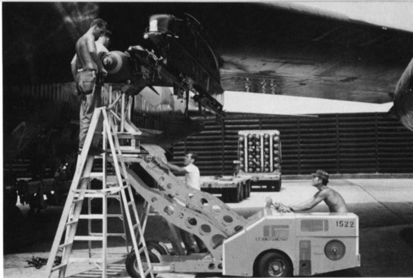
Armament technicians loading M117 750 pound iron bombs on the underwing MER of a B-52D. Although a fully loaded MER could be loaded on the HSAB, the usual practice was to load individual bombs with an MJ-1 bomb loading tractor. (AFM)
