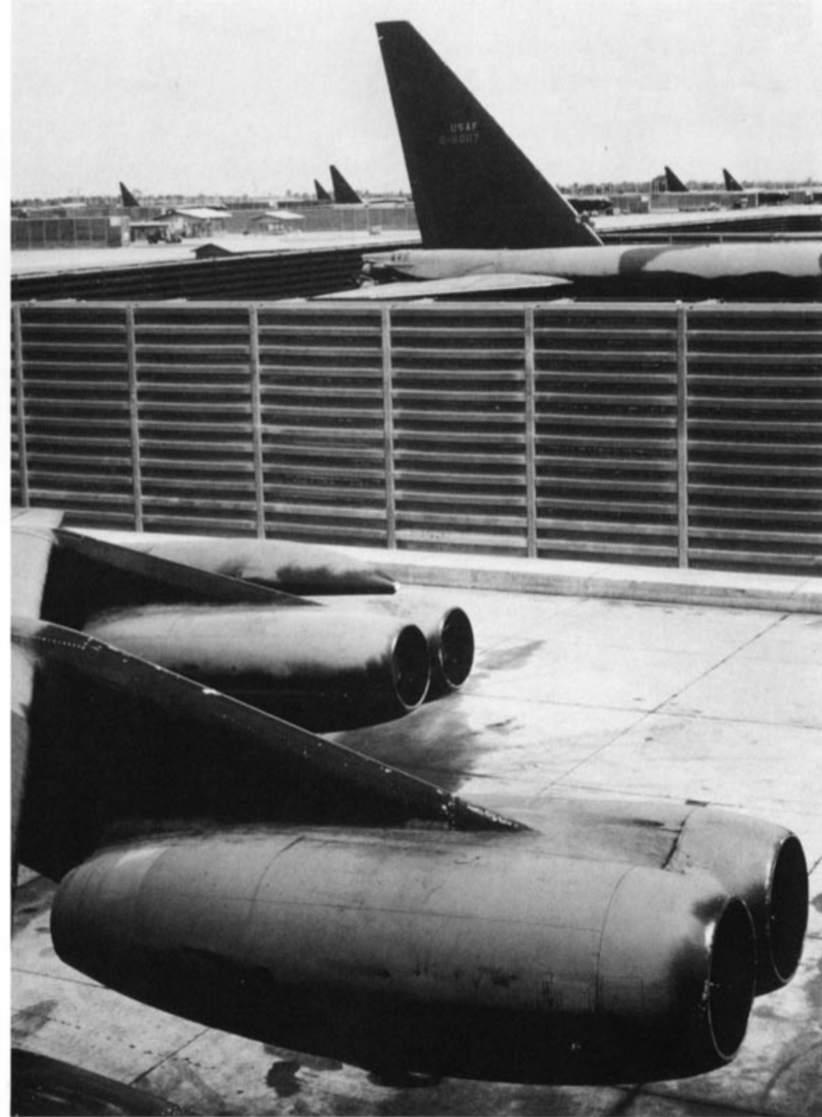
The 4258th SW B-52D revetments at U-Tapao, Thailand during 1970. The revetments only covered to the top of the fuselage, leaving the 48 foot vertical fin exposed. The Black under-surface camouflage was obviously applied without benefit of masking. (AFM)
