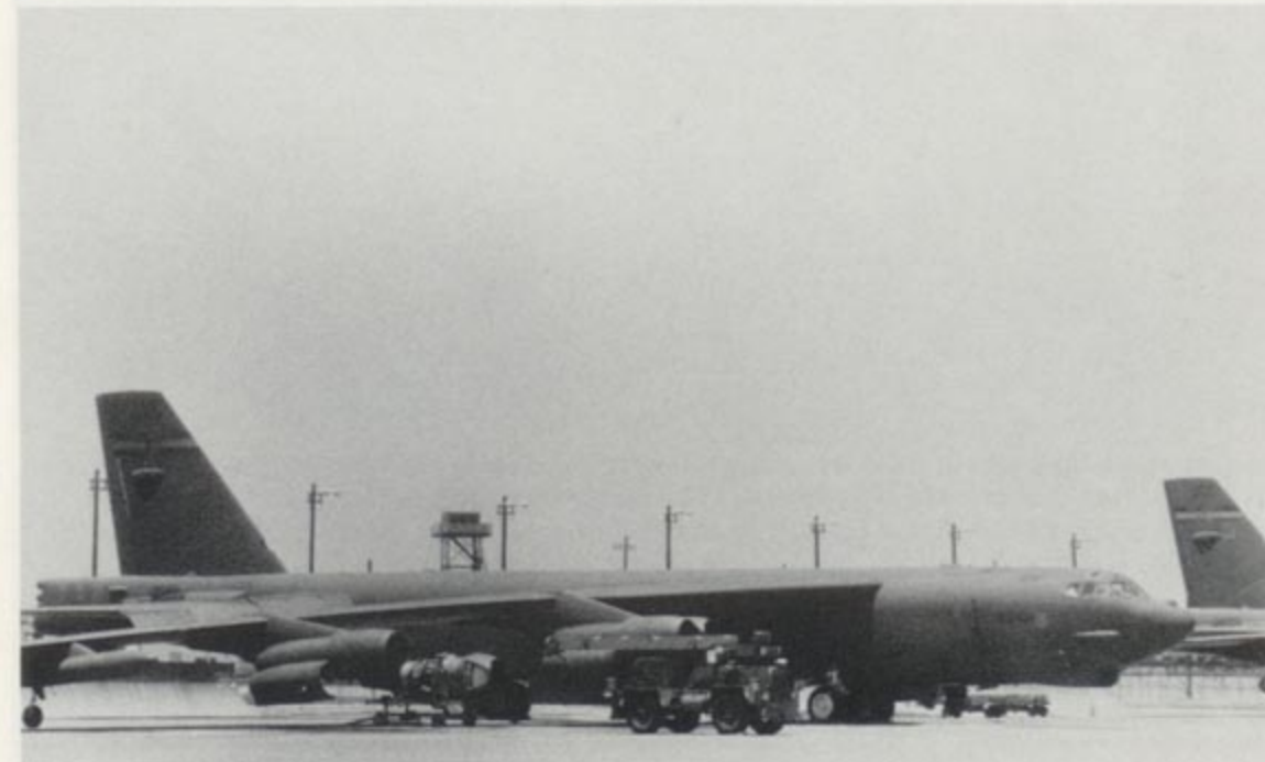
Ground crewmen have removed the outboard engines from this 7th Bomb Wing B-52H. The 7th BW was based at Carswell AFB, Texas until late 1992 when most of its aircraft were transferred to Barksdale AFB. (N. J. Waters III)
