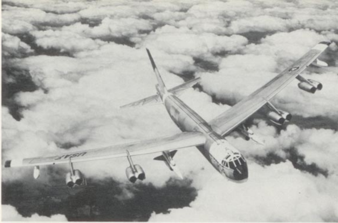
A 2nd Air Force B-52G carries a full compliment of Hound Dog missiles while on airborne alert during the early 1960s. At the height of the Cold War, airborne alert aircraft often remained aloft for 24 hours. The wingtips, nose and tail bands are in Dayglo Orange. (Marty Isham)
