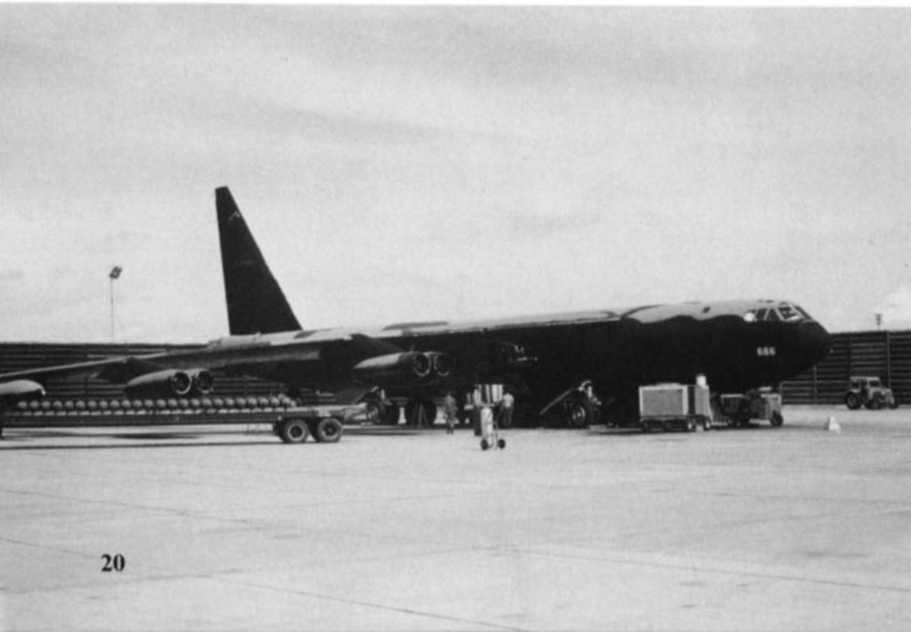
A trailer full of M117 750 pound iron bombs waits to be loaded on the underwing MERs of a B-52D at U-Tapao during 1969. Each underwing pylon could hold twelve 500 or 750 pound bombs, CBUs, or napalm canisters. (AFM)
