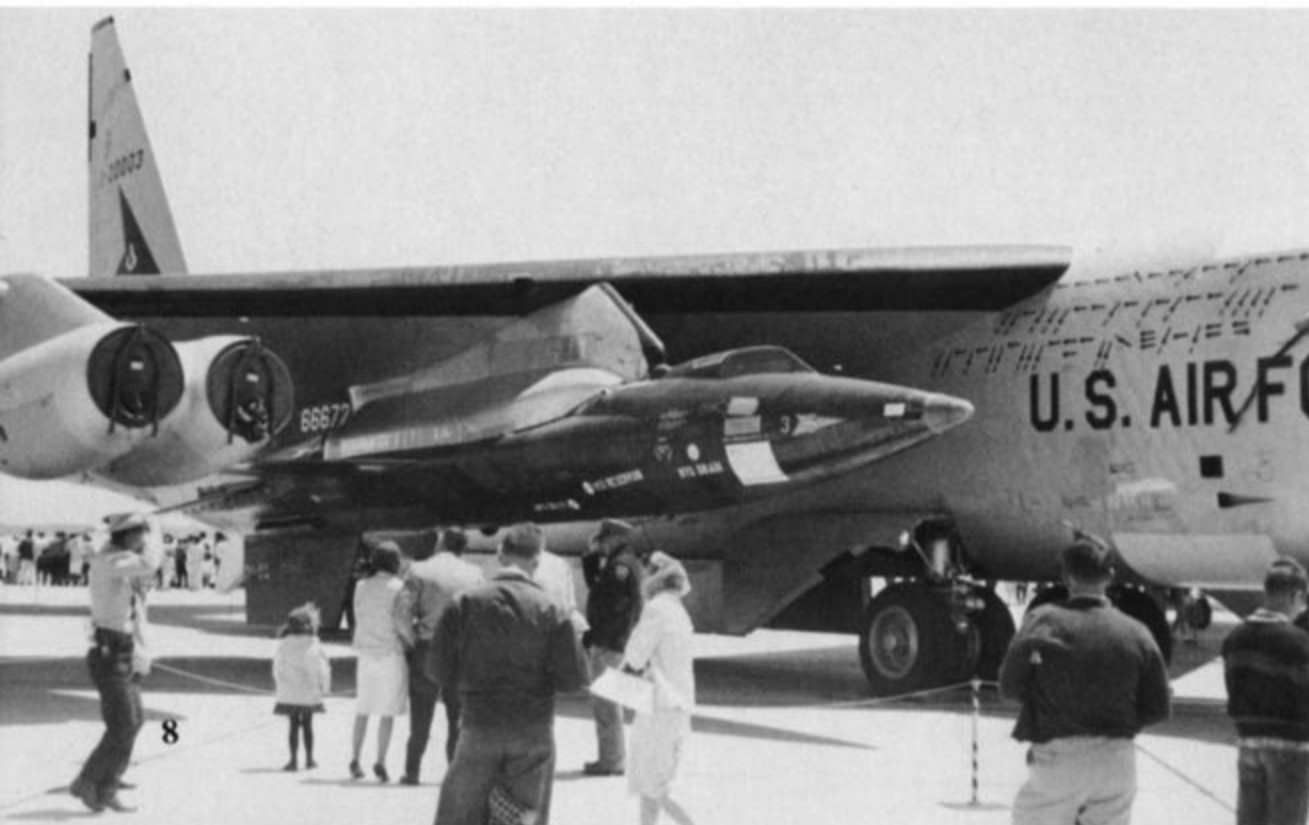
The X-15 was mated to the NB-52A on a specially designed launch cradle/pylon assembly. The mission marks on the fuselage indicate powered and unpowered flights. (Tom Brewer)
