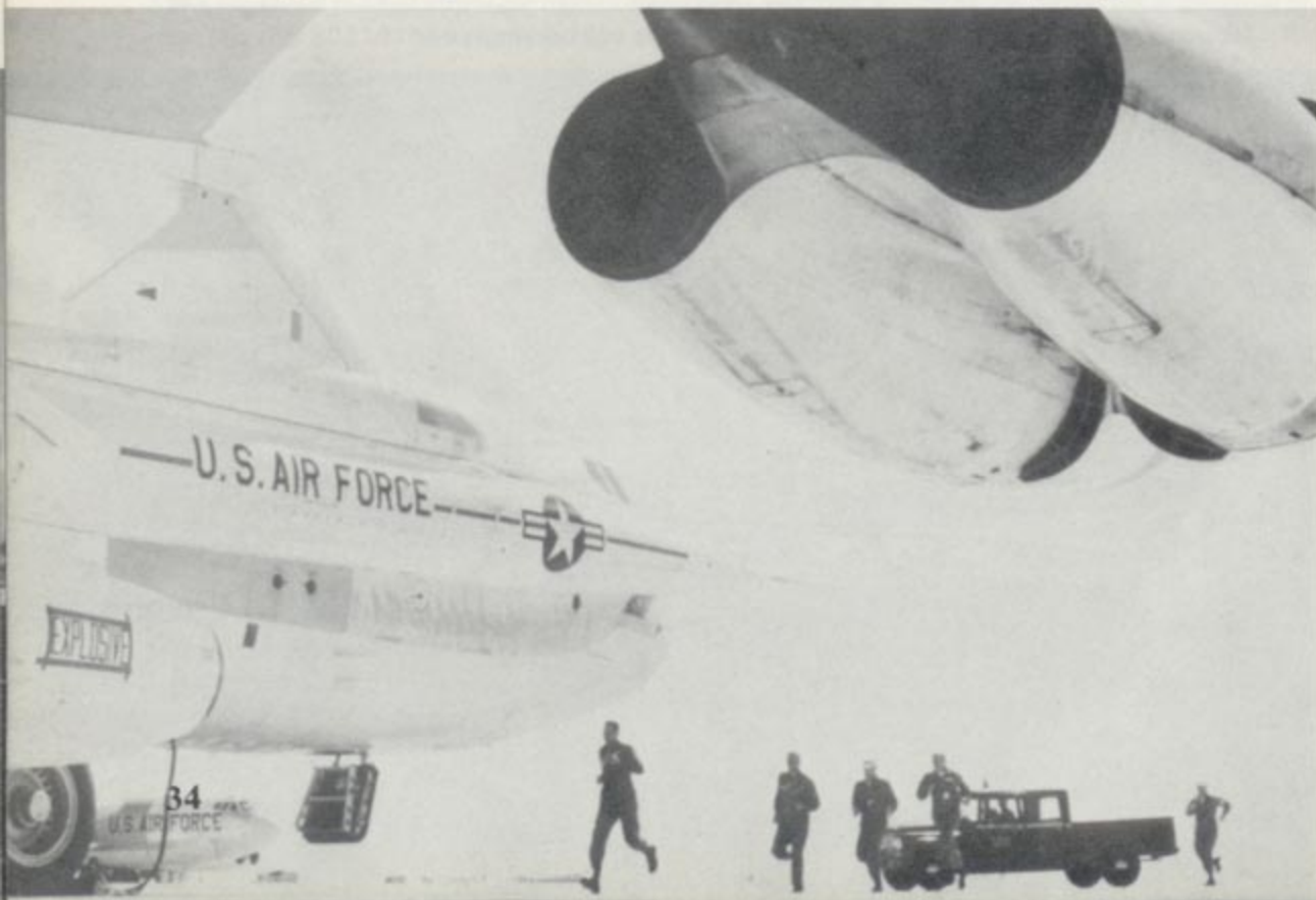
SAC B-52G combat crew racing to their "cocked" alert B-52G. One of the smaller changes on the B-52G was that the crew entry door opened to the rear instead of forward. The sign on the Hound Dog missile engine intake indicated the missile was armed. (USAF)
