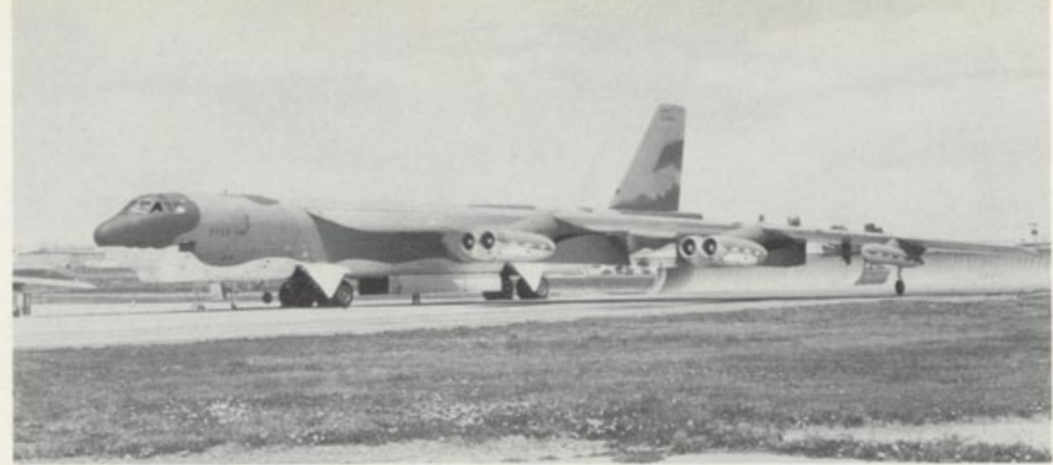
This B-52G from the 28th BW at Ellsworth AFB in 1976 has both EVS turrets closed to protect the system. The strategic camouflage or SIOP pattern is a three tone Green (FS 34201, 34159, and 34079) camouflage, not a Tan and Green pattern. (Brian Rogers)
