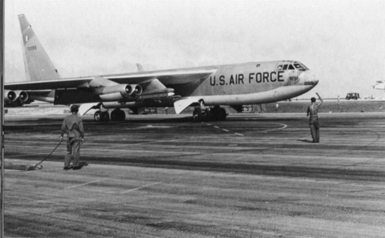
A 320th Bomb Wing B-52F on the ramp at Andersen AFB in the Summer of 1965. At this early date in ARC LIGHT operations, the BUFFs still retained their Gloss White nuclear anti-flash paint and had little in the way of ECM equipment to counter Soviet-built AAA or SAMs. (Joe Bruch)
