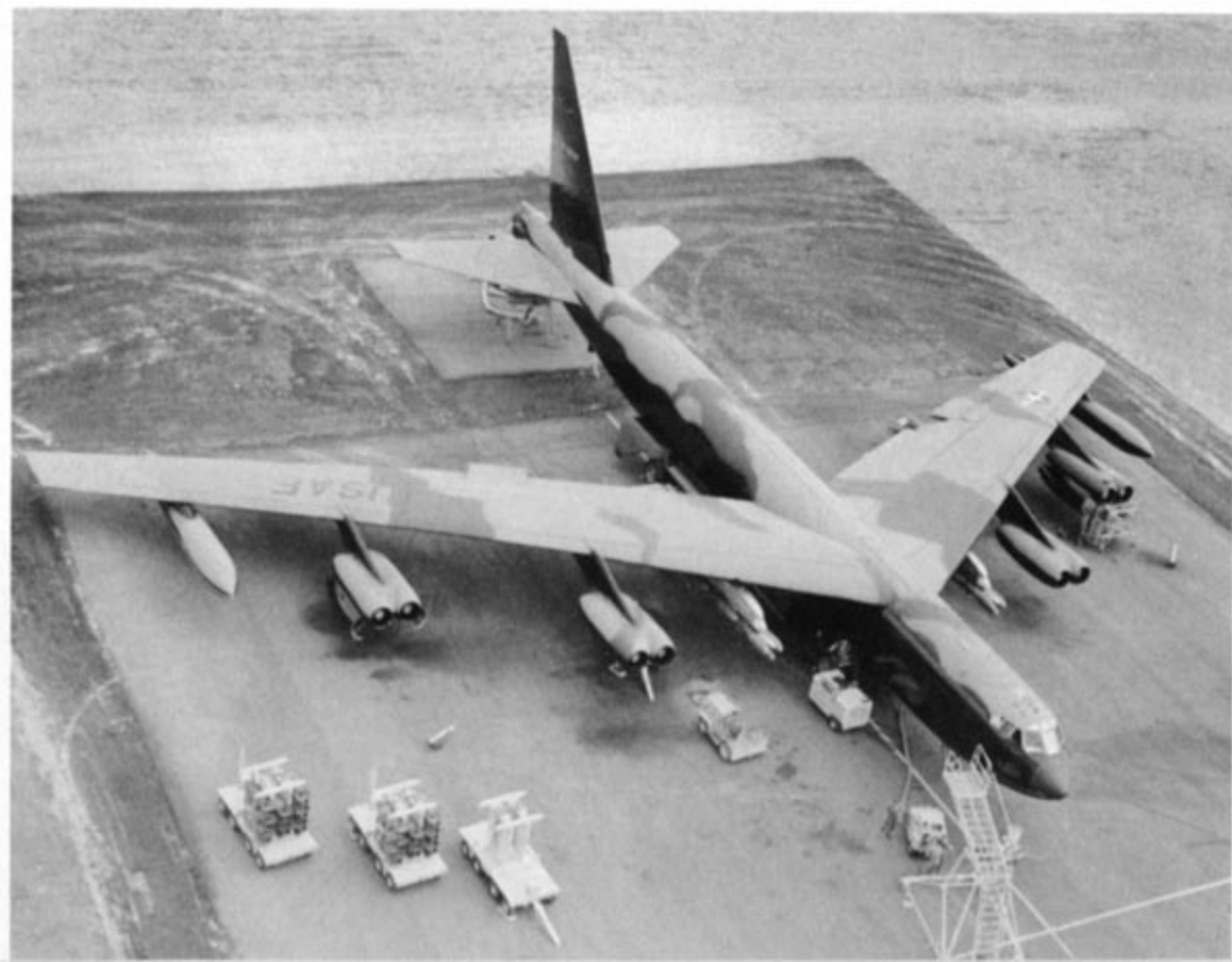
A 4133rd BW (P) B-52D on its parking spot at Andersen AFB, Guam with a full load of Mk 82 bombs on the underwing pylons and "clips" of M117s ready for loading into the bomb bay. With M117 bombs in the "clips," the maximum load was sixty-six bombs. (Robert F. Dorr)
