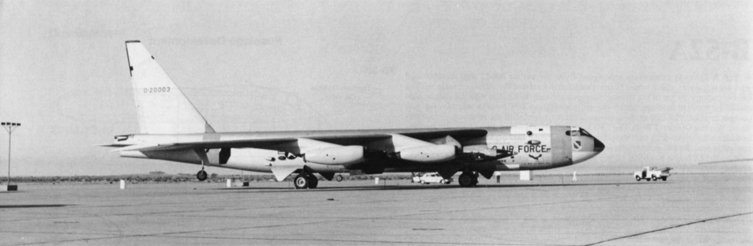
The last of three B-52As (52-003) was modified to carry and launch the North American X-15 rocket-powered research aircraft. Named "The High And Mighty One," the B-52A was modified with sensors, camera stations and visual monitoring ports and redesignated as an NB-52A. (Duane Kasulka)
