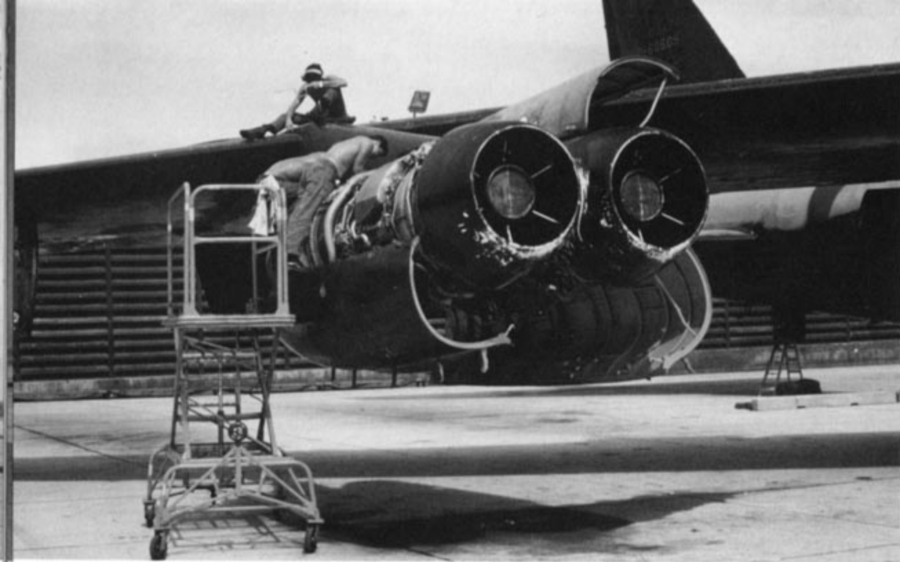
Crew chiefs and maintenance personnel work on the engines of a B-52D of the 4258th SW to make sure it is able to make the next ARC LIGHT mission out of U-Tapao during 1969. The engine hatches are hinged and can be completely removed for easy access to any system. (AFM)
