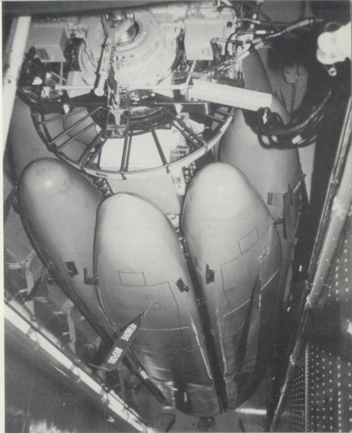
The open bomb bay of a B-52H configured with a Common Strategic Rotary Launcher or CSRL, which can hold up to eight SRAMs or ALCMs, or a mix of the two missiles. The B-52H can carry up to twenty SRAMs or ALCMs when fitted with underwing pylons. (Brian Rogers)
