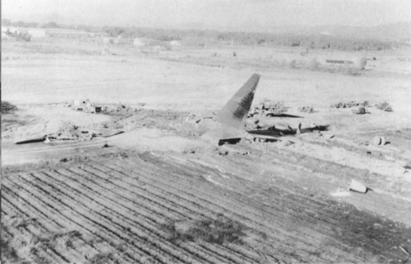
This 4133rd BW B-52D (56-601) suffered a mechanical failure and could not make the long flight back to Andersen AFB. The aircraft landed at Da Nang, lost its brakes and overran the runway. The aircraft ran into the mine field and was totally destroyed. The tail gunner was the only survivor. (Joe Bruch)
