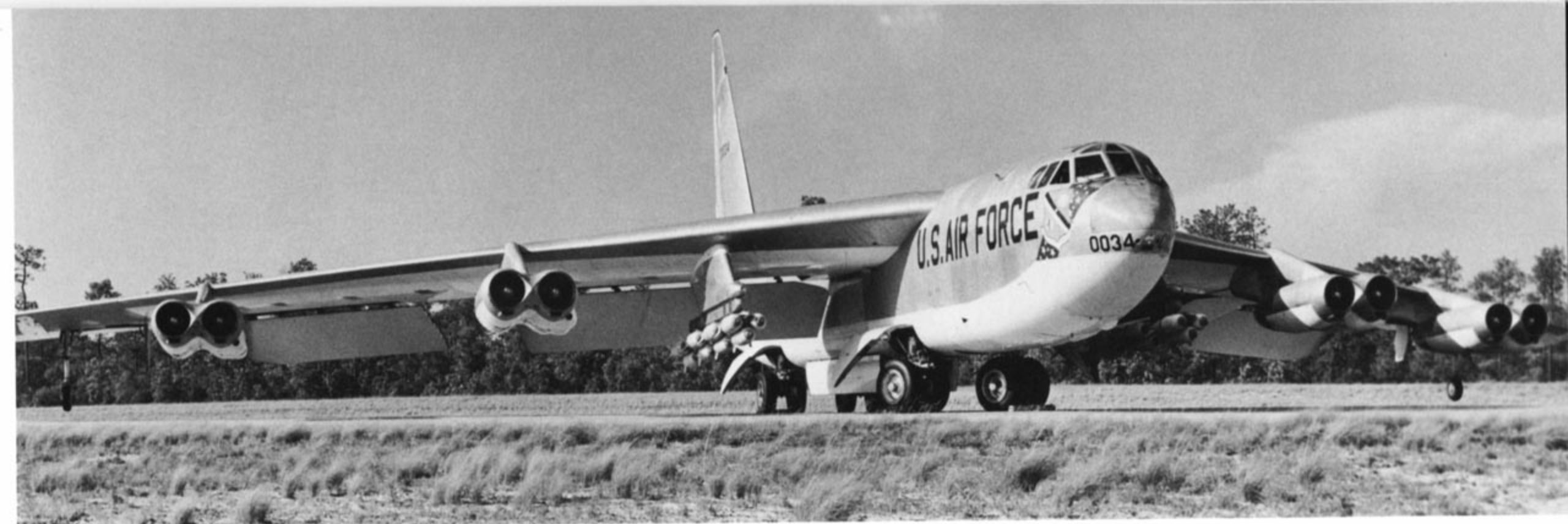
This 93rd BW B-52F is configured with the steel I-beam Heavy Stores Adapter Beam (HSAB) with a pair of Multiple Ejector Racks (MERs) under each wing for carrying conventional munitions during Project SHORT TRIP tests at Eglin AFB in the Summer of 1964. (Joe Bruch)
