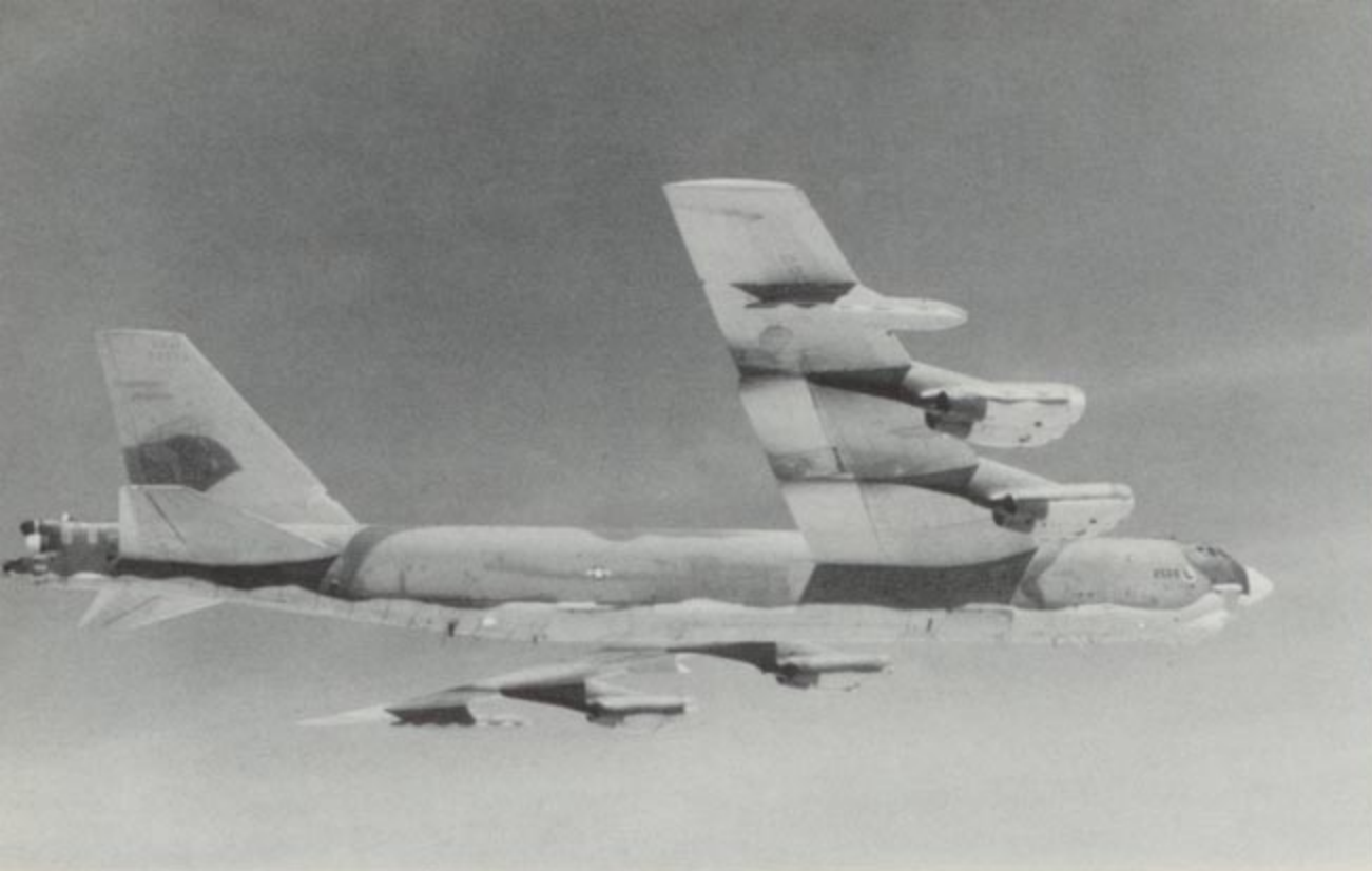
This 92nd BW B-52G in flight over Fairchild AFB in 1977 has the initial Phase VI ECM modifications to the rear fuselage. The fuselage was extended 40 inches between the tail turret and the trailing edge of the stabilizer to house the AN/ALQ-117 ECM system. (Robert F. Dorr)
