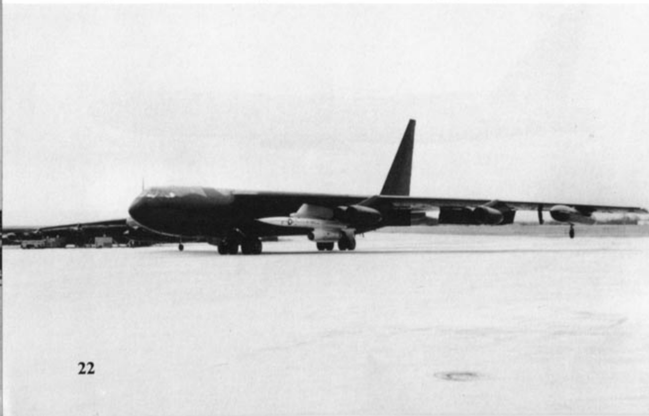
When the American involvement in SEA ended in 1973, most of the B-52D force returned to a normal nuclear alert mission still wearing their SEA camouflage. This B-52D carries uncamouflaged AGM-28 Hound Dog missiles on the underwing pylons. (Joe Bruch)
