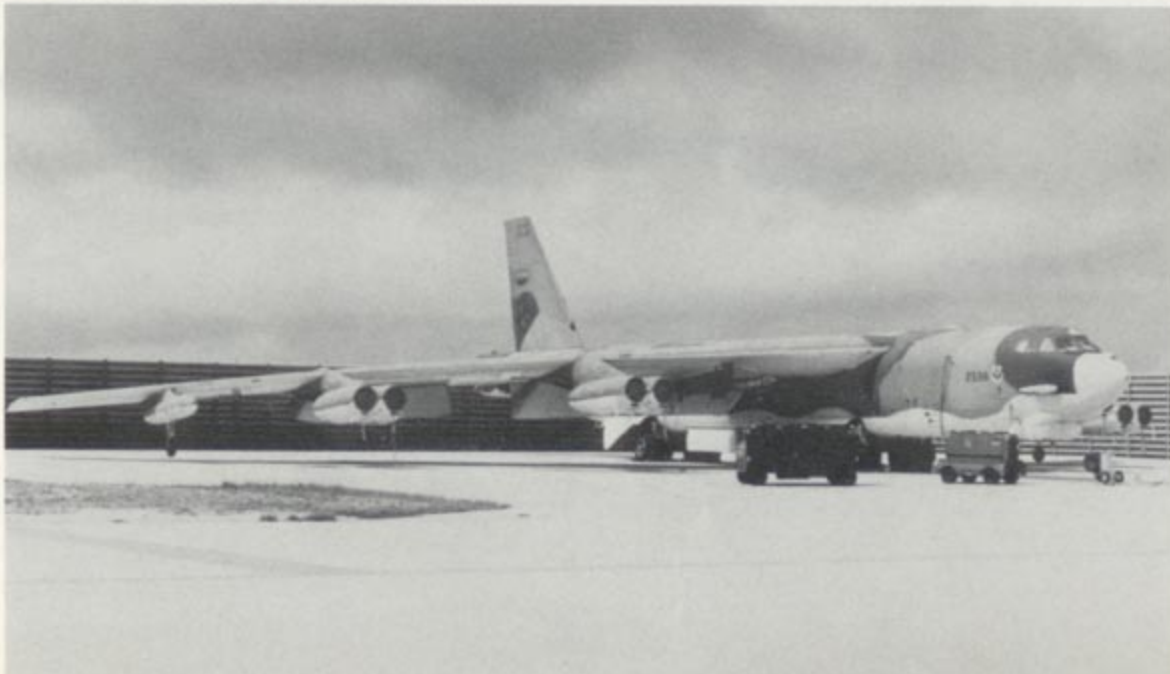
A B-52G of the 43rd SW sits in a revetment at Andersen AFB, Guam during 1985. The aircraft has both the EVS and Phase VI ECM modifications and is fitted with "stub" wing pylons with HSABs mounting MERs. With the phaseout of the B-52D, the conventional munitions mission fell to the B-52G fleet. (Brian Rogers)
