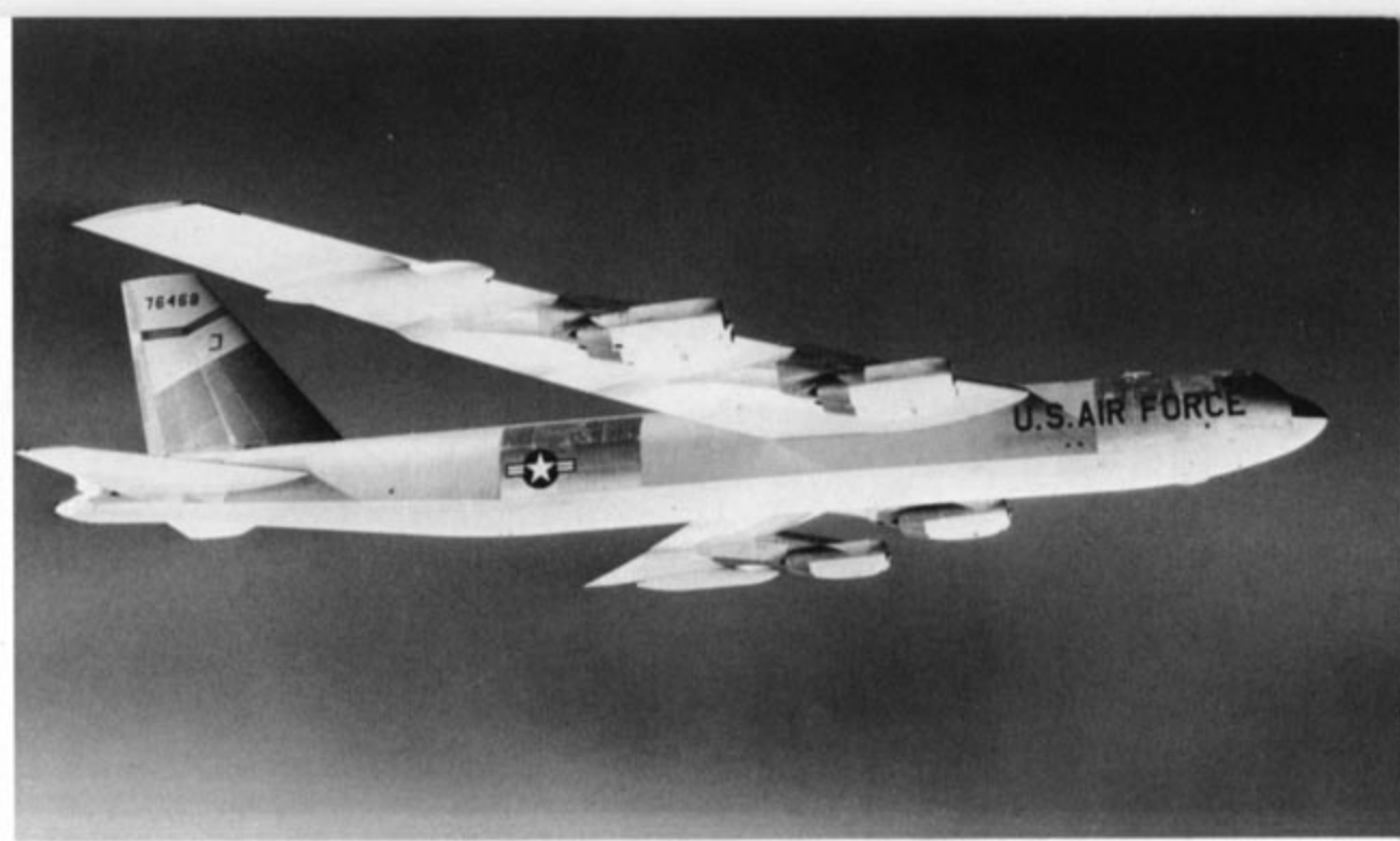
The first B-52G in flight over Wichita during November of 1958. The B-52G introduced the shorter vertical fin, remote-controlled tail turret and was built solely at the Boeing plant in Wichita. (Marty Isham)
