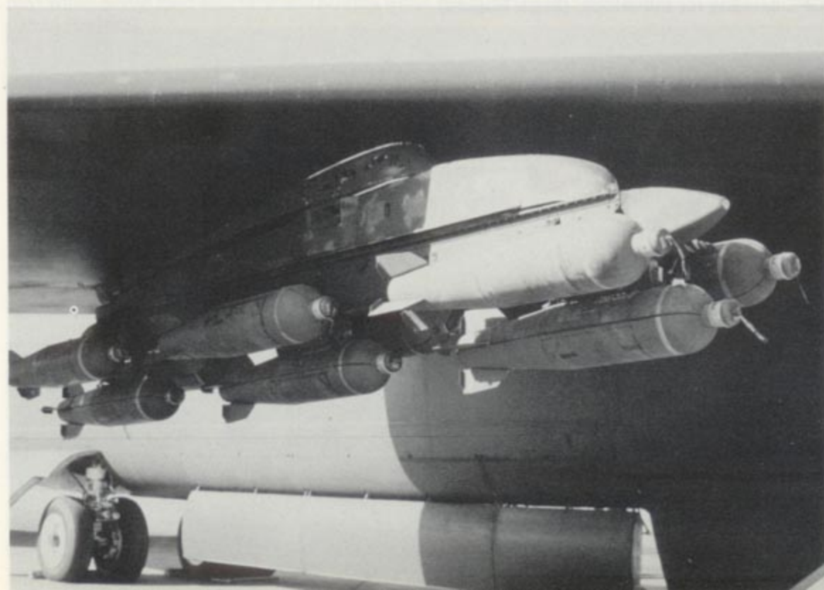
Many B-52G strikes against the Republican Guard positions near Kuwait were flown using CBU-58 cluster bombs, which could penetrate the upper armor of Iraqi tanks. The CBUs were mounted directly to the HSAB without using a MER. (Brian Rogers)
