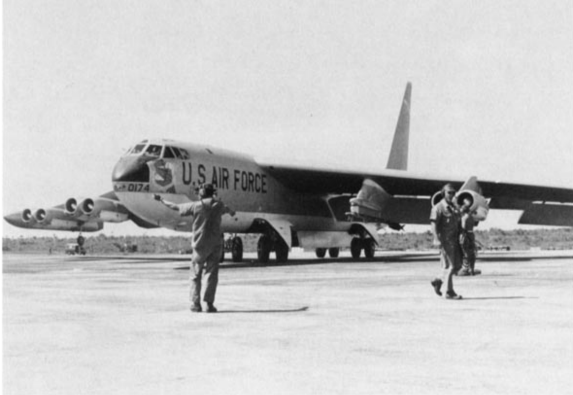
This 320th Bomb Wing B-52F returned to Andersen with a “hung” bomb on the left rear MER. B-52Fs dropped over 100,000 tons of bombs on ARC LIGHT operations between June 1965 and April 1966. The distinctive engine bulges common to the B-52F are visible. (Joe Bruch)
