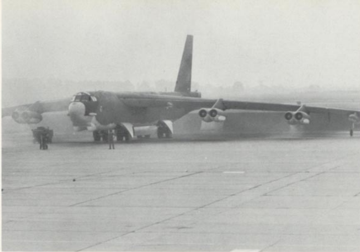
Project QUICK START installed cartridge starters on all eight engines to decrease the time needed to become airborne. The smoke cloud from this 97th BW B-52G is toxic and ground crews have to wear respirators during QUICK START exercises. (Joe Bruch)
