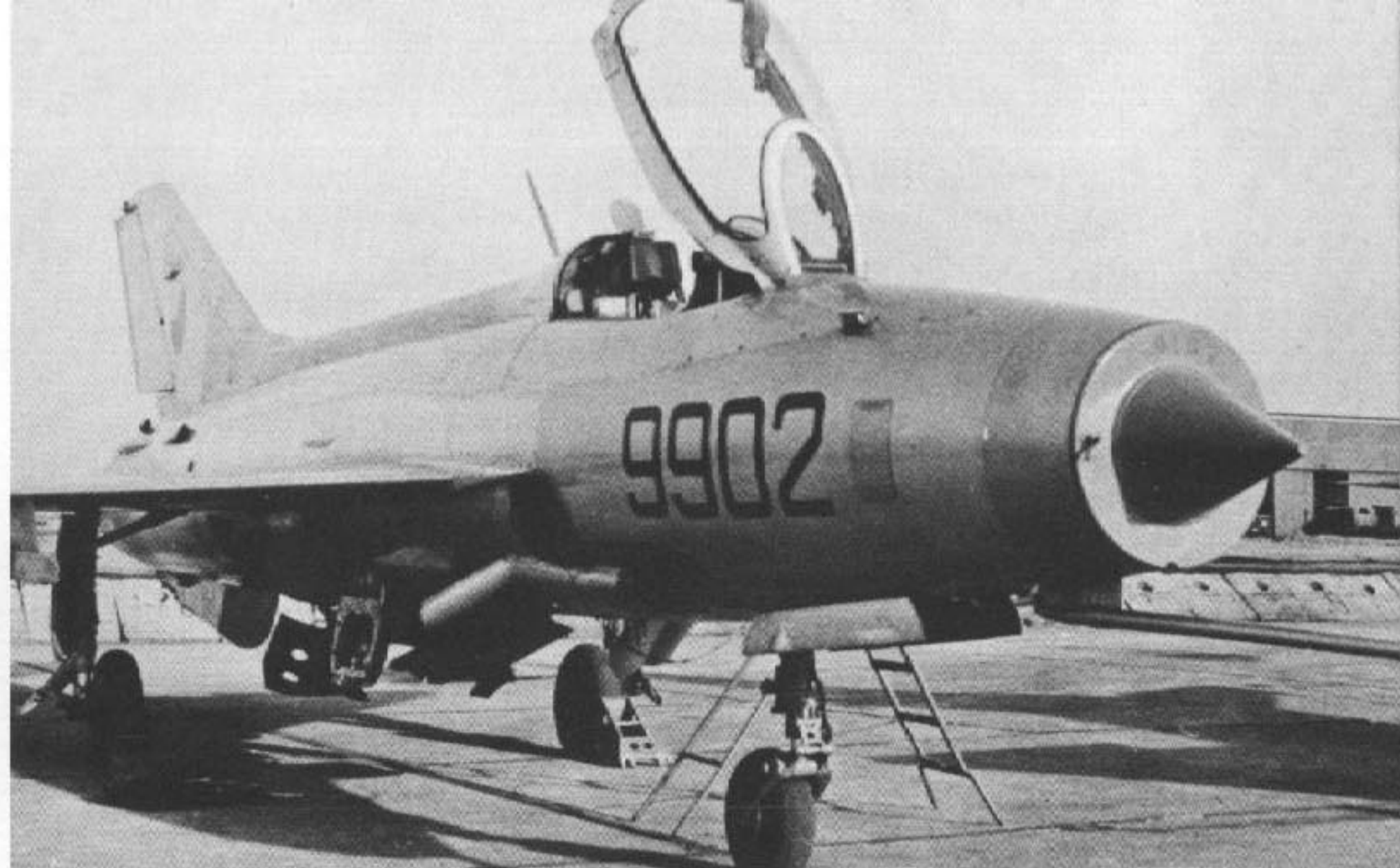
This Czech Air Force MiG-21F-13 Fishbed C, Black 9902, has both the forward and rear speed brakes deployed. The aircraft has Red protective covers over the air intake and the suck-in door on the fuselage side above the NR 30 cannon. (Norm Taylor)
