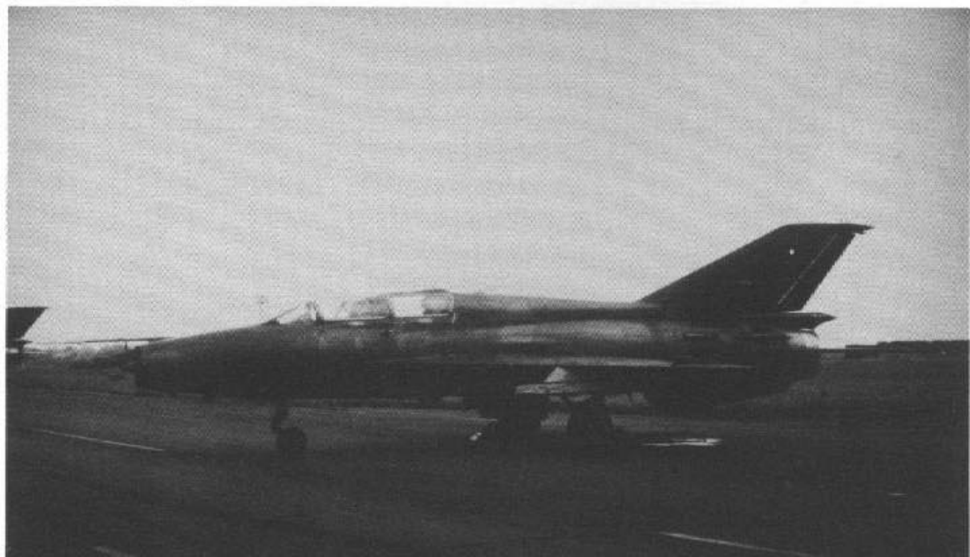
This former East German Air Force MiG-21US Mongol B carries the Federal German registration code 24-12 but lacks full German insignia. The MiG-21US Mongol Bs used by East Germany were delivered in Natural Metal and camouflaged during the mid-1970 in East Germany. (Jens Schymura)
