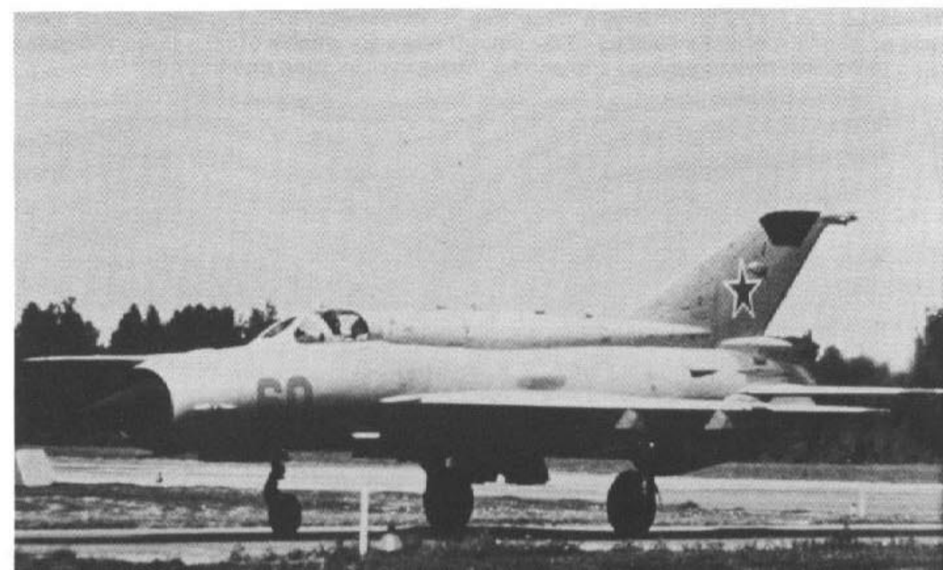
The tactical number on the nose of this overall Air Superiority Gray Soviet Air Force MiG-21bis Fishbed L is Blue with a thin Black outline. The spine of the Fishbed L was faired farther back into the vertical fin than the earlier Fishbed J. (NASM)
