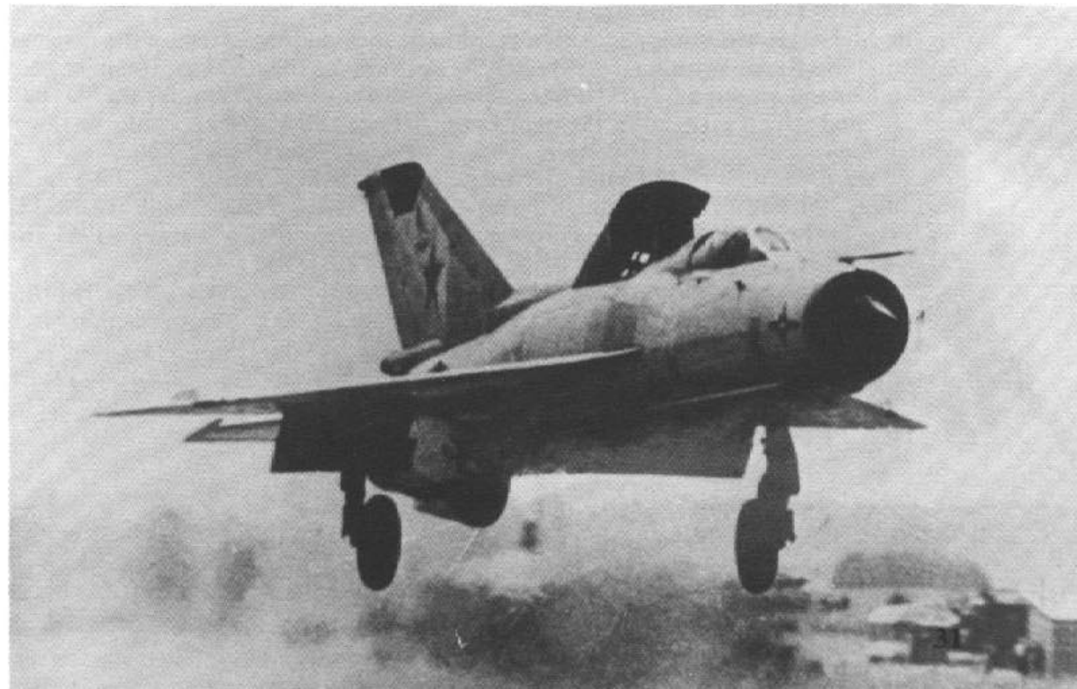
The MiG-21DP was a converted MiG-21PFM with two RD-36-55 lift engines in the fuselage. The STOL version of the Fishbed was demonstrated in the Summer 1967 at the Domodedovo Air Display and it was given the NATO reporting name Fishbed G. (Hans-Heiri Stapfer Collection)
