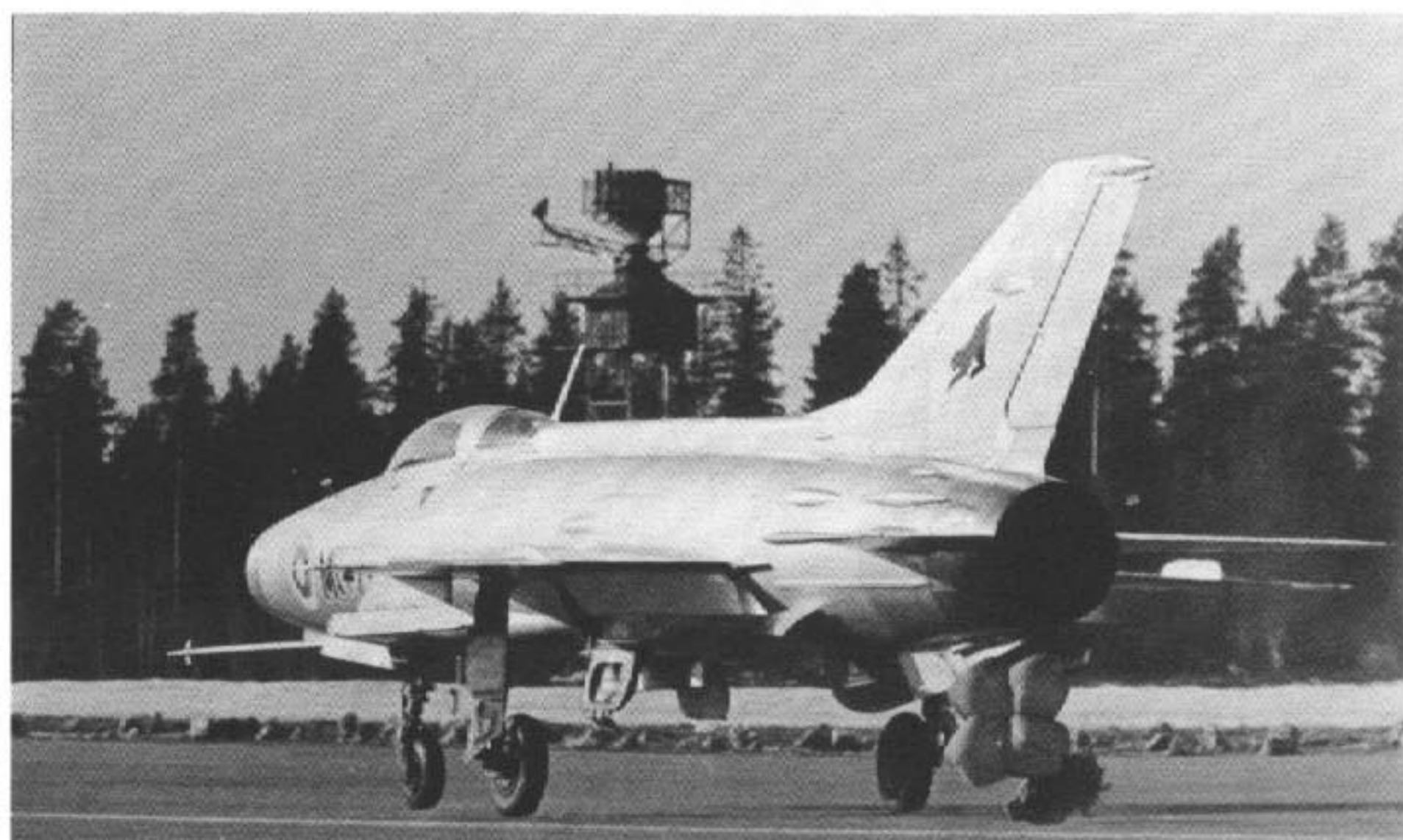
The drag chute is just deploying as this MiG-21F-12 lands at Halli Air Base. The Black Lynx on the tail identifies this Fishbed as being assigned to Havittajalentolaivue 31 (31st Fighter Squadron) of the Ilmavoimat (Finnish Air Force). (Jyrki Laukkanen)
