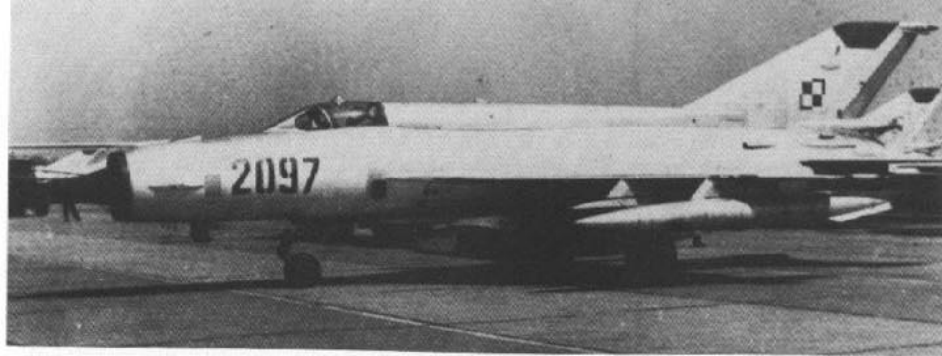
This Polish Air Force MiG-21R Fishbed H, Red 2097, is equipped with a D type reconnaissance pod, 490 liter drop tanks on the outboard wing pylons and a R-60MK (AA-8 Aphid) missile rail on the inboard pylon. (Hans-Heiri Stapfer Collection)
