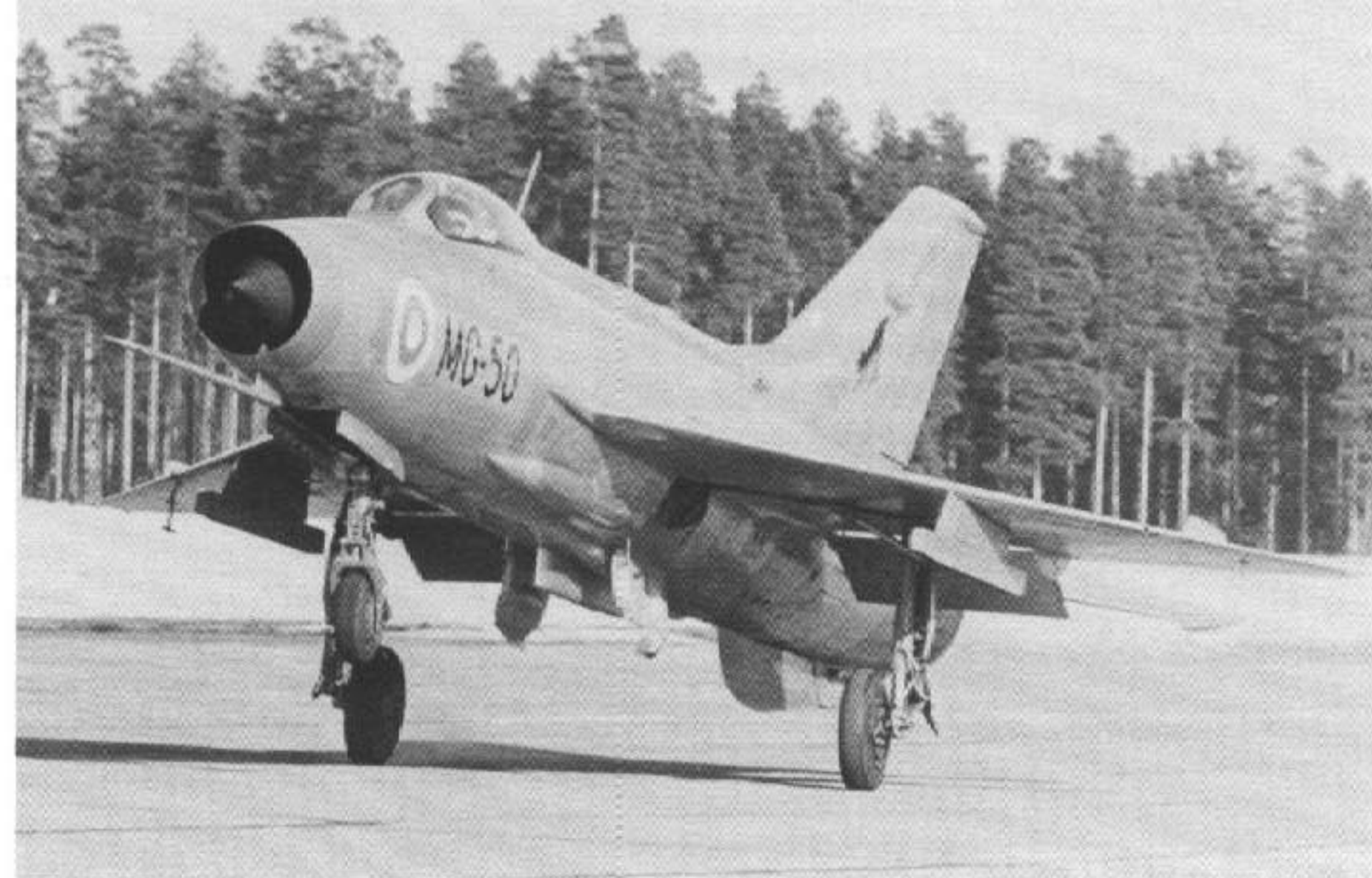
The MiG-21s exported to Finland were given the designation MiG-21F-12, although they were identical to standard Soviet MiG-21F-13 Fishbed C. This Finnish Air Force Fishbed, lifting off from Halli Air Base during May of 1974, is assigned to the 31st Fighter Squadron. (Jyrki Laukkanen)
