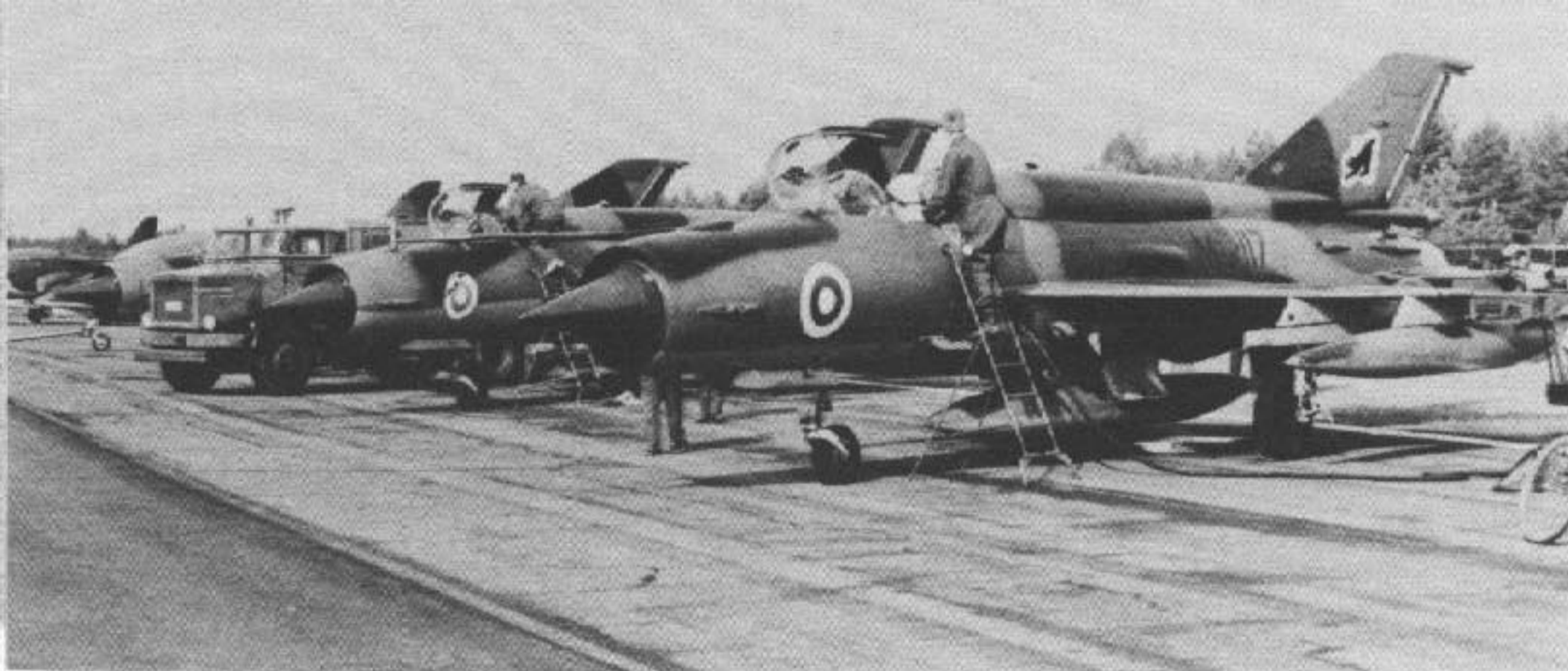
Three Finnish MiG-21bis Fishbed Ls on the ramp at Oulu Air Base during June of 1987 being prepared for a training sortie. Each MiG has three drop tanks, two 290 liter (76.6 gallon) tanks on the outer wing pylons and a 800 liter (211 gallon) tank on the centerline. (Jyrki Laukkanen)
