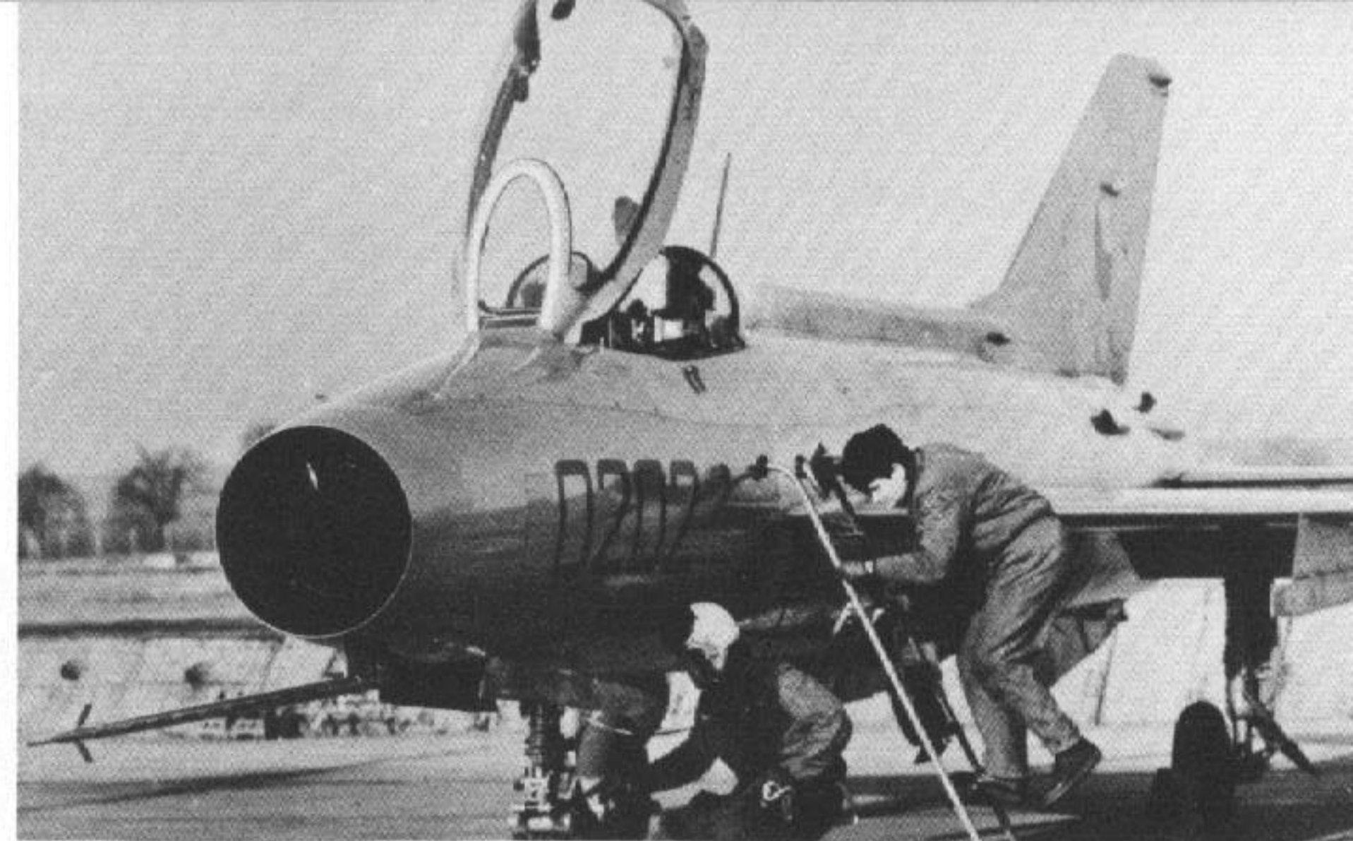
The pilot of this Czech-built MiG-21F-13 inspects the nosewheel during his preflight inspection. The Czech-built MiG-21F-13 differed from the Soviet-built Fishbed C in that the clear panel behind the cockpit was deleted and faired over. (Norm Taylor)
