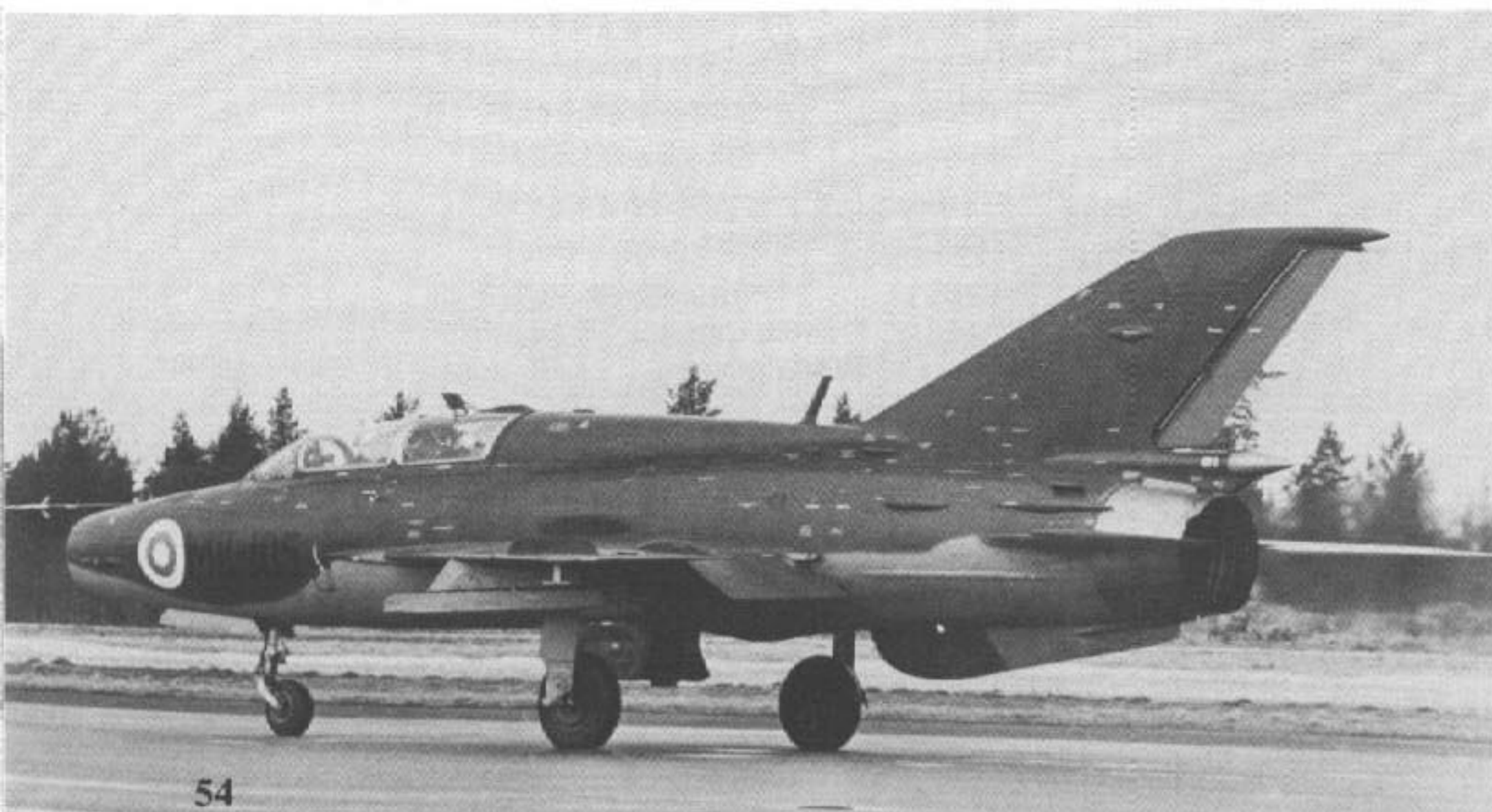
The crew of a Finnish Air Force Mig-21UM Mongol B conducts preflight checks on the runway of a Finnish Air Force base. The rear cockpit of the MiG-21U series was not raised making it necessary to provide the instructor with a periscope to allow him to see anything in front of the aircraft. (Jyrki Laukkanen)
