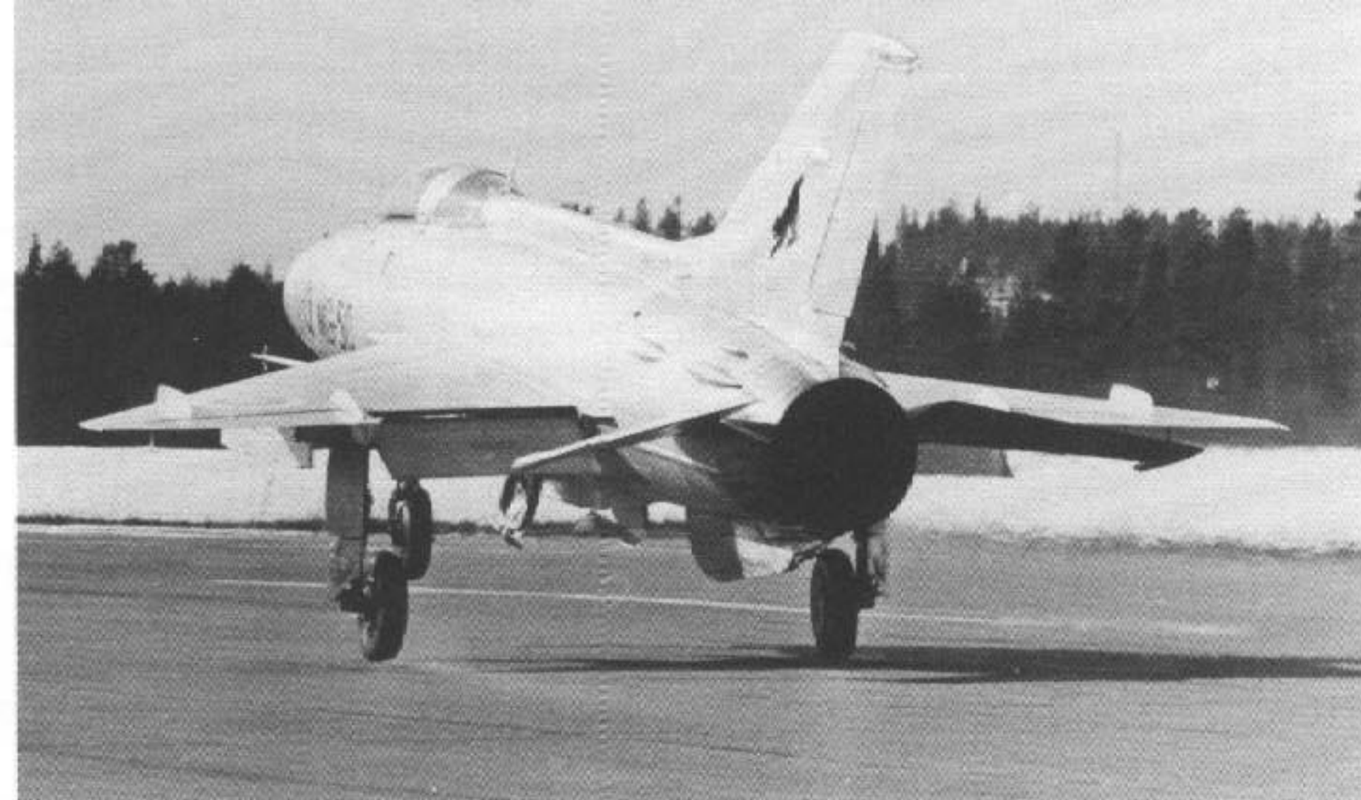
A Finnish Air Force MiG-21F-12 lands at its home base with the trailing edge wing flaps fully deployed. The Finnish national insignia was carried on both the upper wing surfaces just inboard of the wing fence and was repeated on the wing undersurfaces. (Jyrki Laukkanen)
