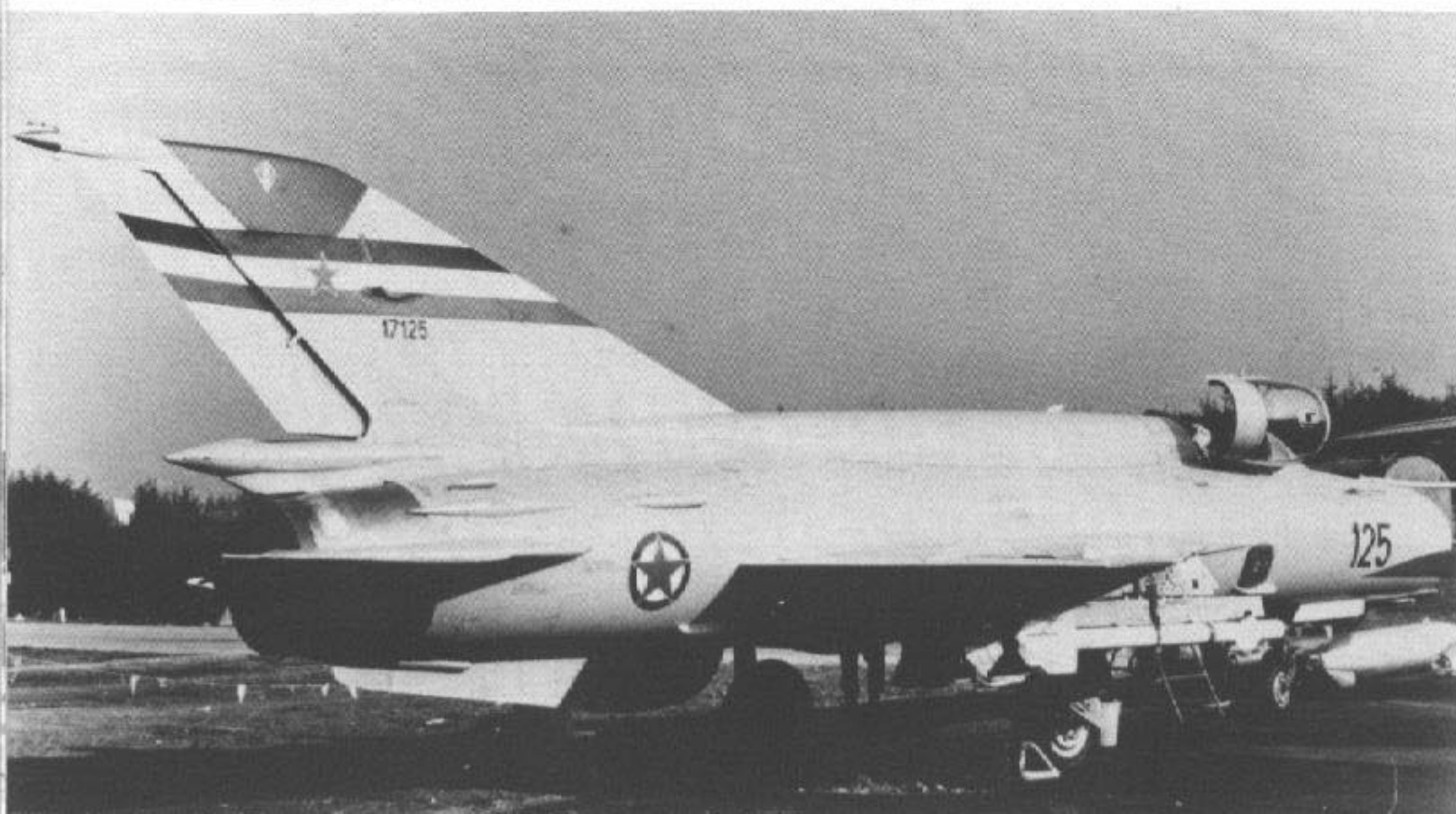
This overall Air Superiority Gray Yugoslav Republic Air Force MiG-21bis-SAU Fishbed N, Black 125, carries a K-13A (AA-2 Atoll) missile on the outboard wing pylon. Since the partitioning of Yugoslavia into separate republics, the national markings have been changed and the Red star is no longer carried. (Don Sperry)
