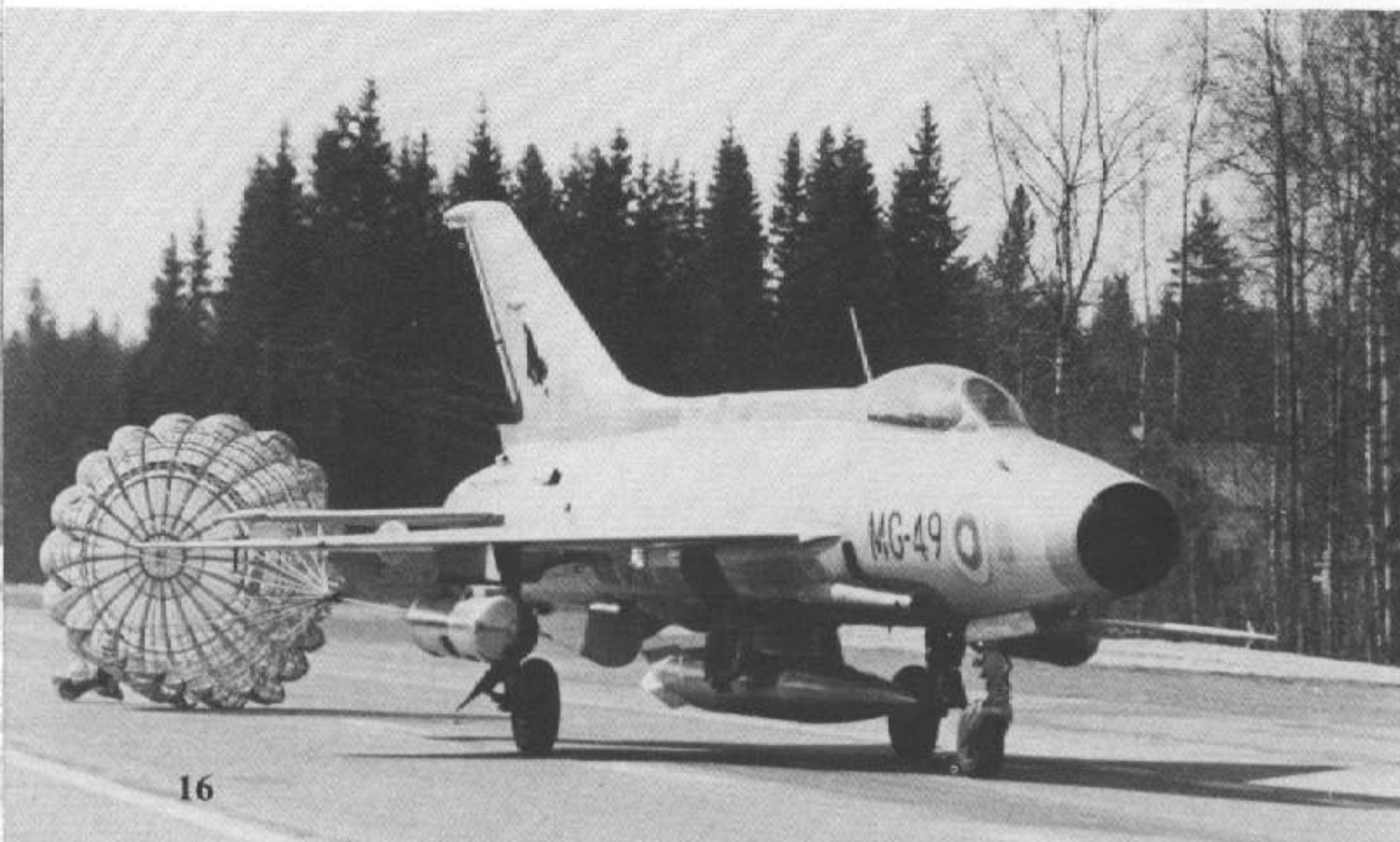
The braking parachute of this MiG-21F-12 is fully deployed as the aircraft rolls out after returning from a search and rescue mission. The Fishbed is carrying a Valmet manufactured rescue pods on the underwing pylon. (Jyrki Laukkanen)
