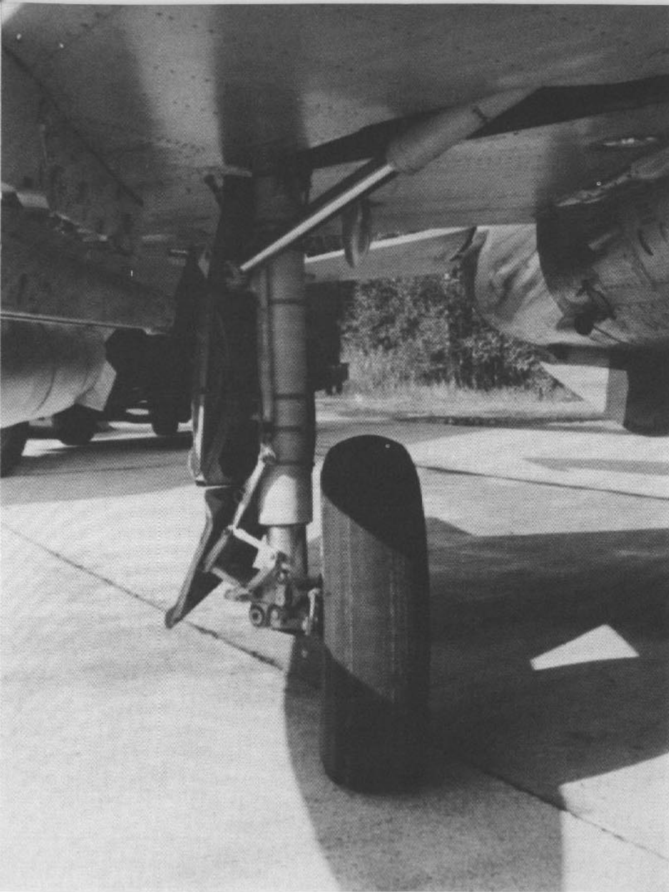
The main landing gear doors are a two part door, with the lower section attached to the main landing gear strut. The door closing piston is mounted in front of the main gear strut. (Jyrki Laukkanen)
