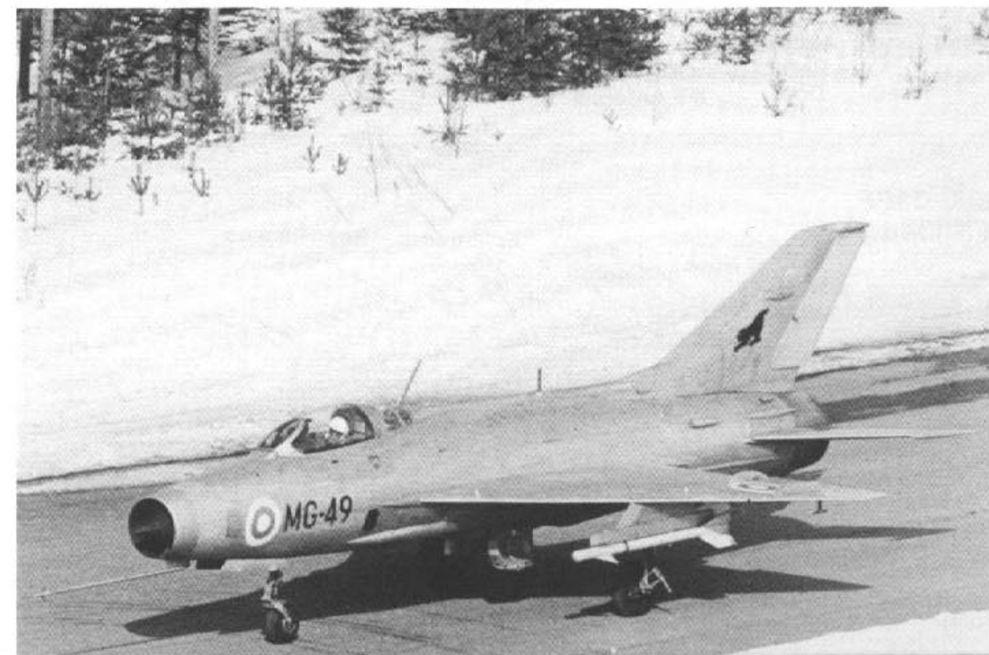
A MiG-21F-12 Fishbed C, armed with a pair of IR homing K-13 (AA-2 Atoll) air-to-air missiles, taxis in after a mission. The MiG-21F's lack of all weather instrumentation seriously restricted its tactical usefulness, especially in the harsh Finnish climate. (Jyrki Laukkanen)
