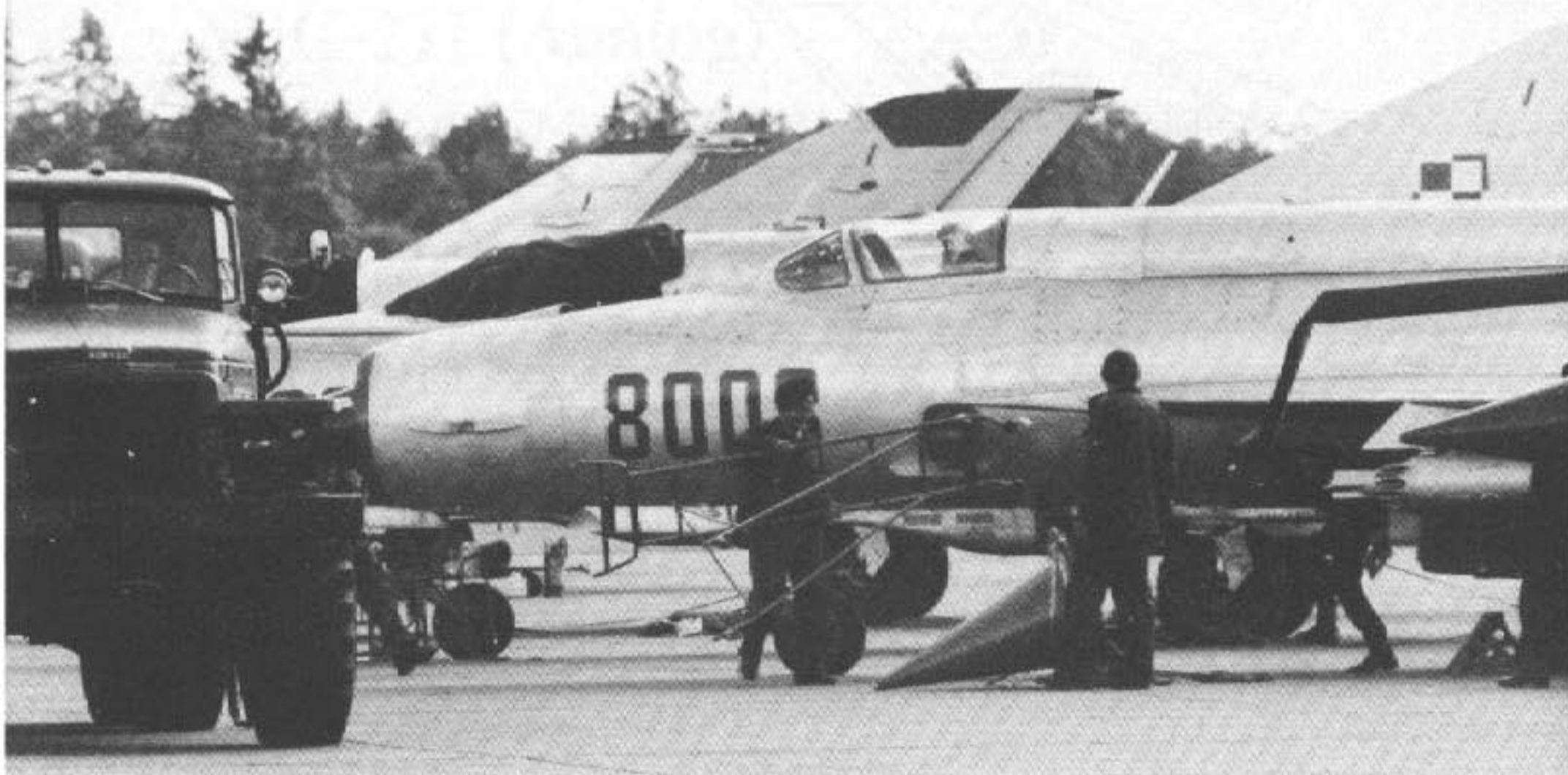
Ground crewmen prepare a Polish Air Force MiG-21MF, Red 8008, for another mission. The aircraft is armed with a UB-16-57U rocket pod on the inboard wing pylon. The aircraft behind it is a MiG-21PFM Fishbed F armed with a GP-9 gun pod which is visible under the Fishbed J in the foreground. (Hans-Heiri Stapfer)
