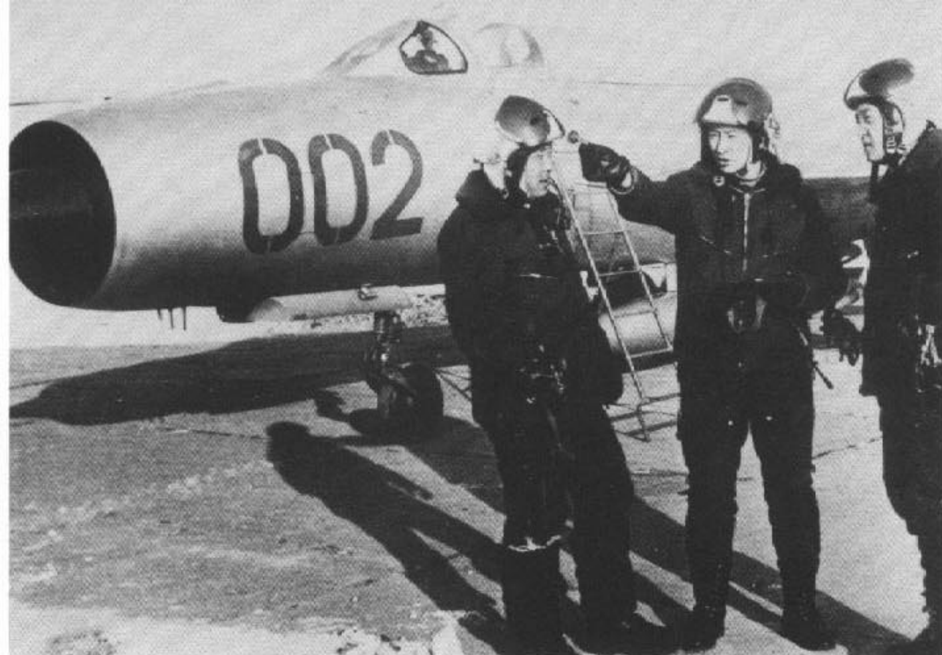
This MiG-21PFM, Red 002, of the Mongolian Air Force has been retrofitted with a rearview mirror on the upper canopy framing. Additionally, a number of Mongolian Fishbed Fs also carry the GP-9 gun pod as standard equipment. (Hans-Heiri Stapfer Collection)
