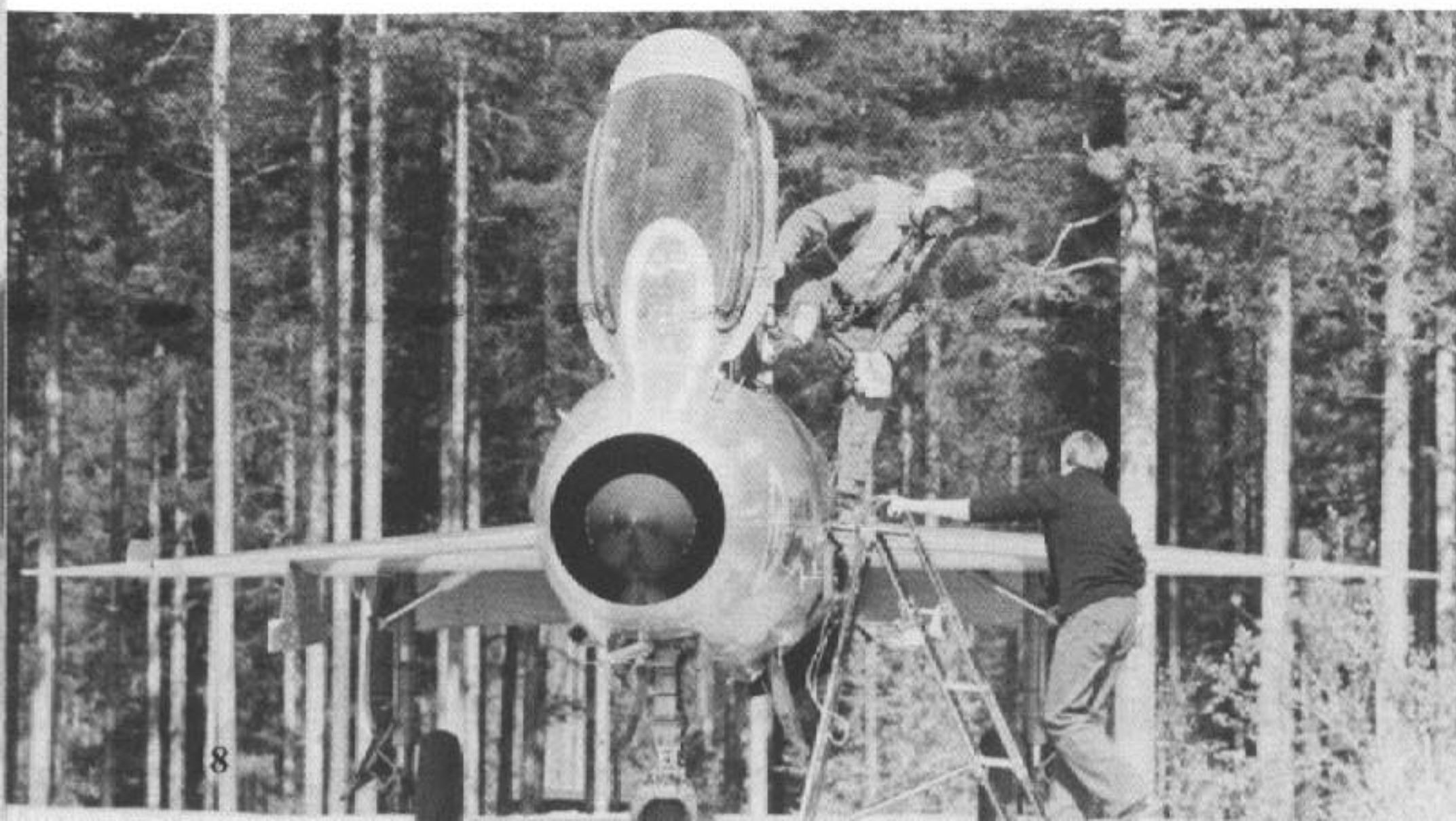
The pilot of this Finnish MiG-21F-12 steps out of the cockpit onto the crew boarding ladder. The nosewheel has a tow bar attached to allow ground crewmen to maneuver the fighter from one parking spot to another. (Jyrki Laukkanen)
