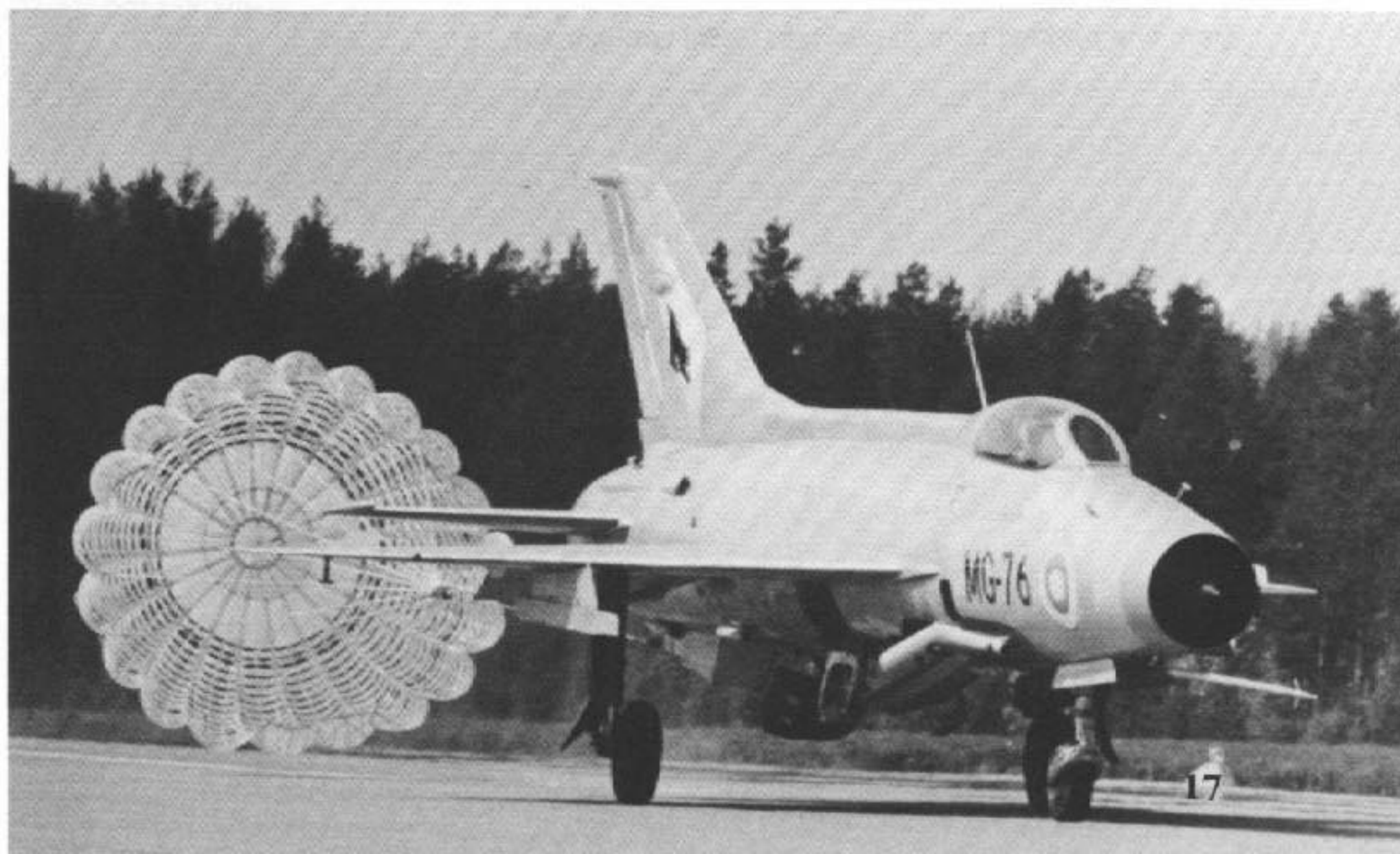
This early MiG-21F-12 Fishbed C, landing at Halli Air Base in southern Finland during 1974, has the braking parachute and both sets of speed brakes fully deployed. The aircraft has missile rails installed on the underwing pylons. (Jyrki Laukkanen)
