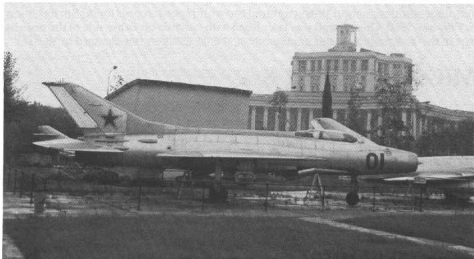
The third Ye-6 prototype was fitted with canard surfaces on the nose under the designation Ye-6T/3. For missile tests the aircraft was also outfitted with a pylon for a single R-13 (AA-2 Atoll) air-to-air missile under each wing. The canards were free-floating at subsonic speeds and locked at supersonic speeds. (Hans-Heiri Stapfer Collection)
