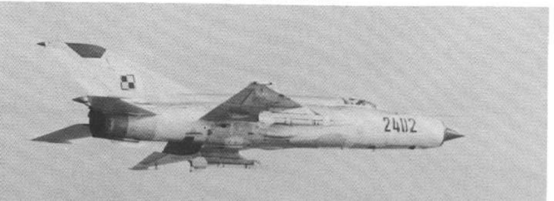
This Polish Air Force MiG-21R Fishbed H does not have a reconnaissance pod installed on the centerline. It is armed with a pair of K-13 (AA-2 Atoll) IR homing air-to-air missiles which are normally carried for self-defense. (Don Spring/AIR)
