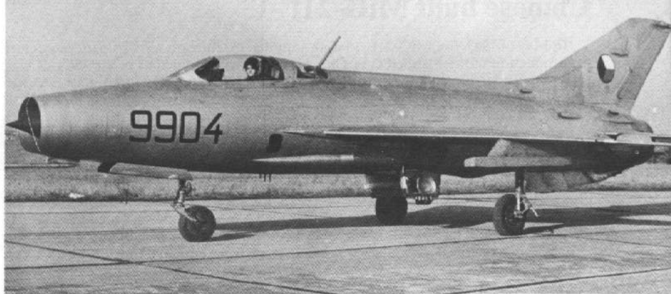
Black 9904, an early Soviet-built Czech Air Force MiG-21F-13, taxis to the run up area for preflight checks. The MiG-21F-13 Fishbed C differed from the MiG-21F Fishbed B in that it had a wider chord fin and rudder. (Norm Taylor)
