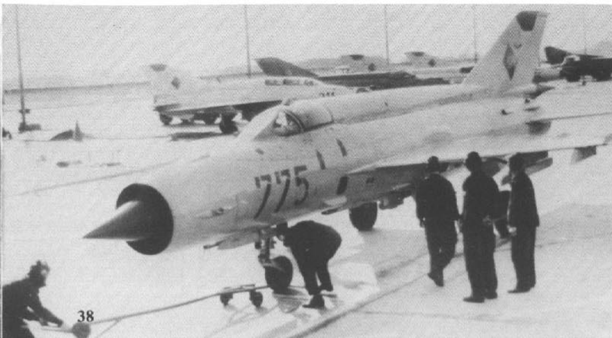
Ground crews attach the nosewheel tow-bar to the nosewheel of an overall Air Superiority Gray MiG-21MF (Red 775) of the East German Air Force. The aircraft in the background are MiG-21UM Mongol B trainers and other camouflaged MiG-21MF Fishbed Js. (Wolfgang Tamme)
