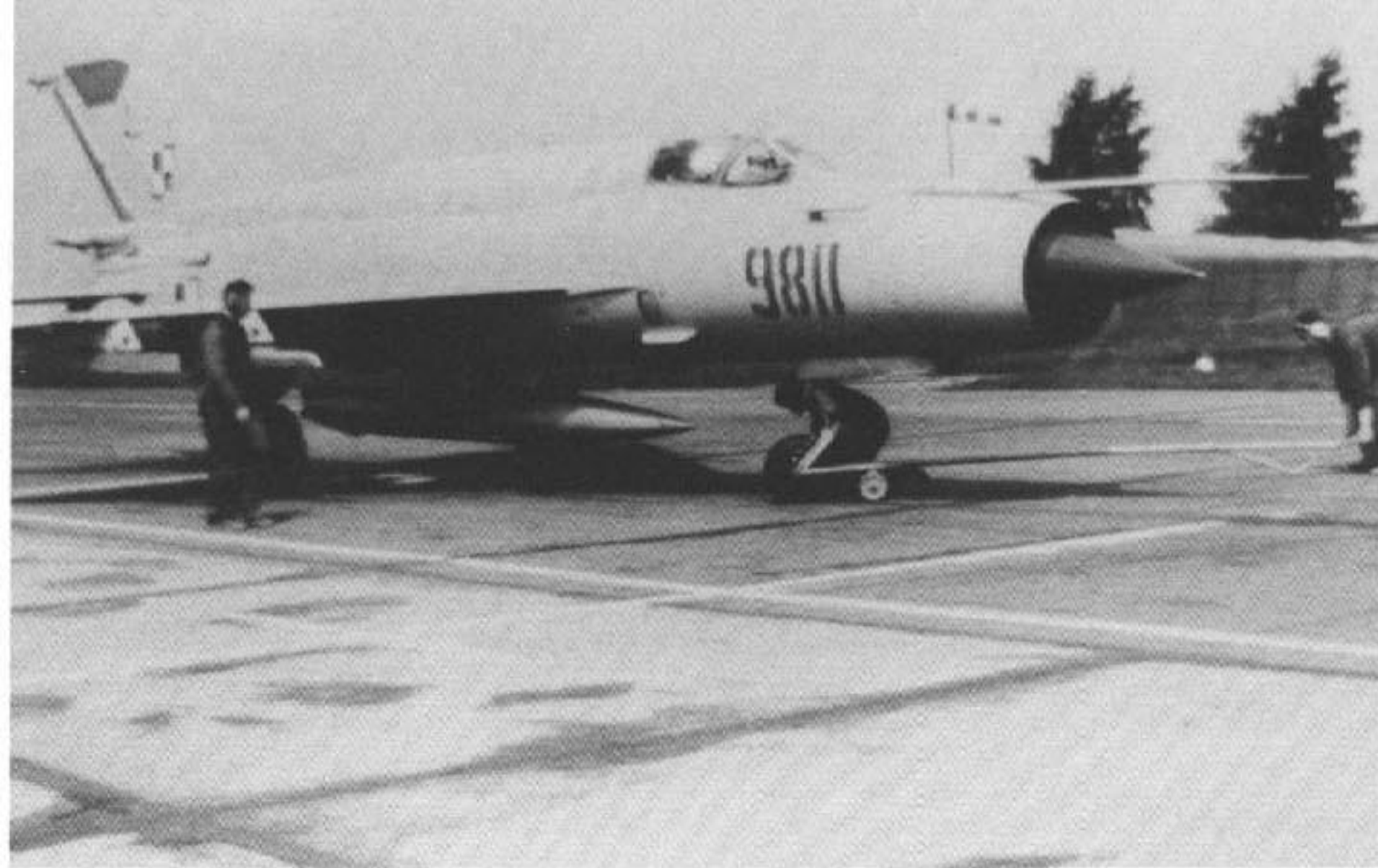
Ground crewmen detach the tow bar from a Polish MiG-21bis, Red 9811, while the pilot performs his preflight checks. There were only a few MiG-21bis Fishbed Ls delivered to Poland, the main variant in service being the MiG-21MF Fishbed J. (Wolfgang Tamme via Hans-Heiri Stapfer)
