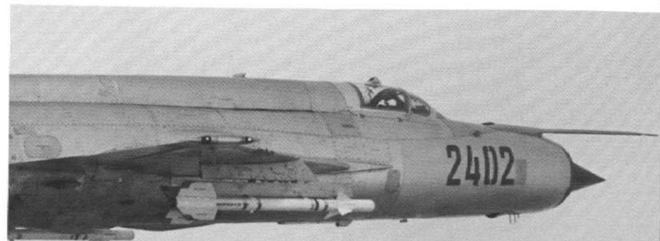
This Polish Air Force MiG-21R Fishbed H does not have a reconnaissance pod installed on the centerline. It is armed with a pair of K-13 (AA-2 Atoll) IR homing air-to-air missiles which are normally carried for self-defense. (Don Spring/AIR)
