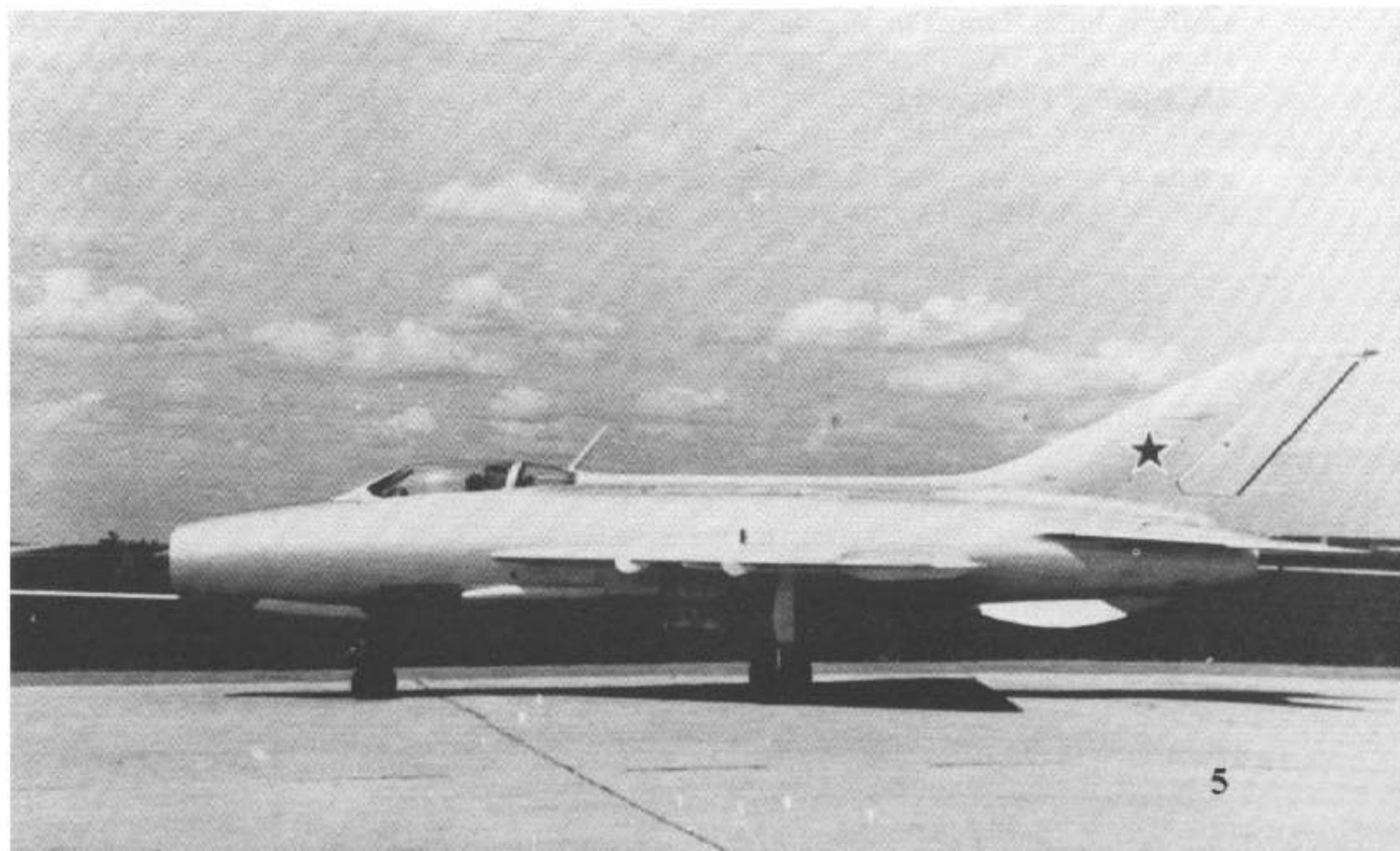
The Ye-5 prototype differed from the Ye-4 in the engine installed. The Ye-5 was powered by 5,098 lbst AM-11 power plant, which boosted the top speed by nearly 700 kph (434.9 mph). The Ye-5 was unveiled on 24 June 1955 and NATO assigned the reporting name Fishbed to the prototype. (Hans-Heiri Stapfer Collection)
