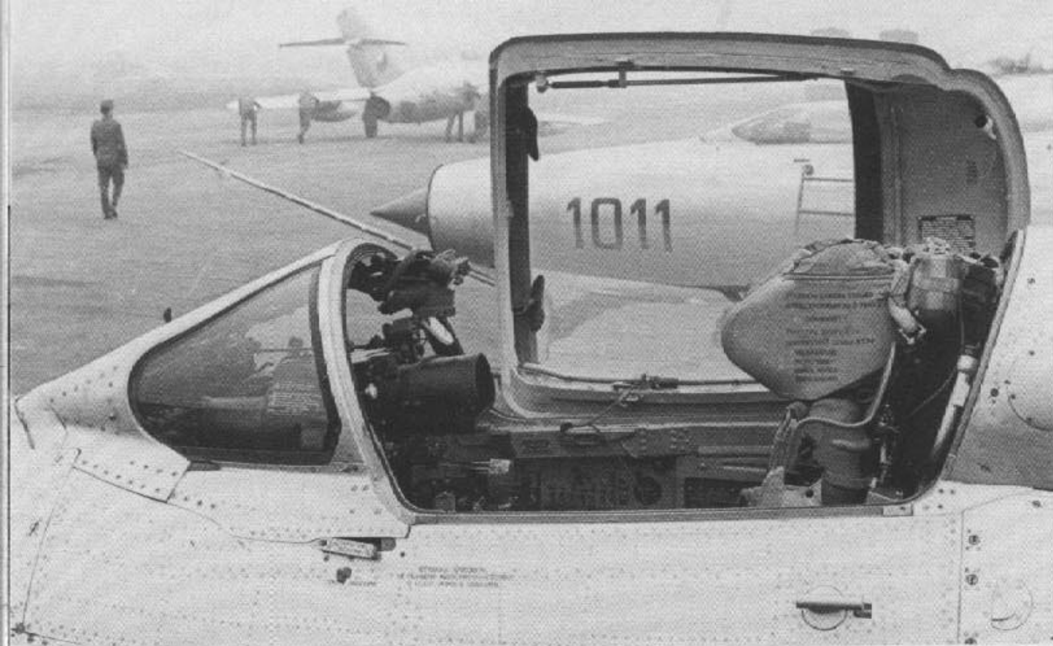
The MiG-21PFM was the first of the Fishbed series to incorporate a side opening canopy. The ejection seat used on the PFM was the KM-1 zero-zero ejection seat. The aircraft in the background are a MiG-21F-13 Fishbed C and a MiG-15 Fagot (left). (Don Spring/AIR)
