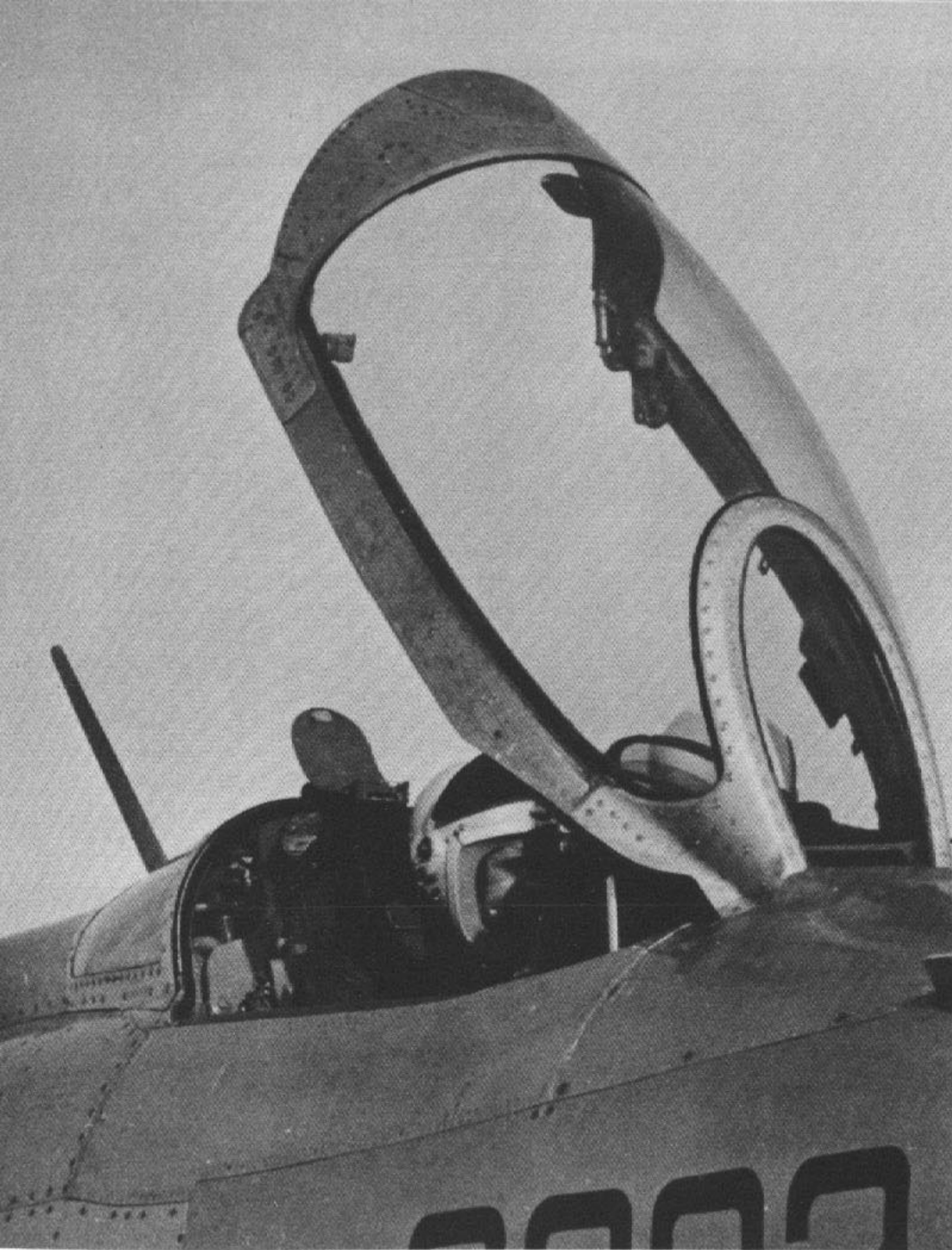
The canopy on the MiG-21 was unique in that it was forward hinged. The plate above the ejection seat was compressed downward when the canopy was closed, arming the ejection seat. (Norm Taylor)
