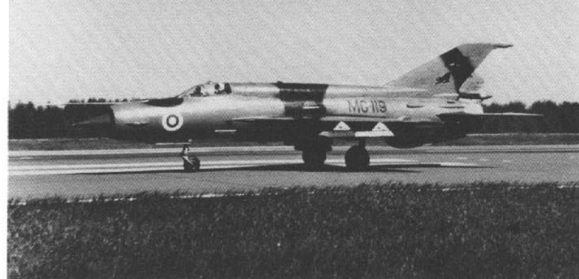
A Finnish Air Force MiG-21bis Fishbed L taxis along the taxiway of its home base. The MiG-21bis Fishbed L has a completely re-engineered fuselage that is lighter, stronger and has more space for internal fuel in the larger fuselage spine. (Jyrki Laukkanen)
