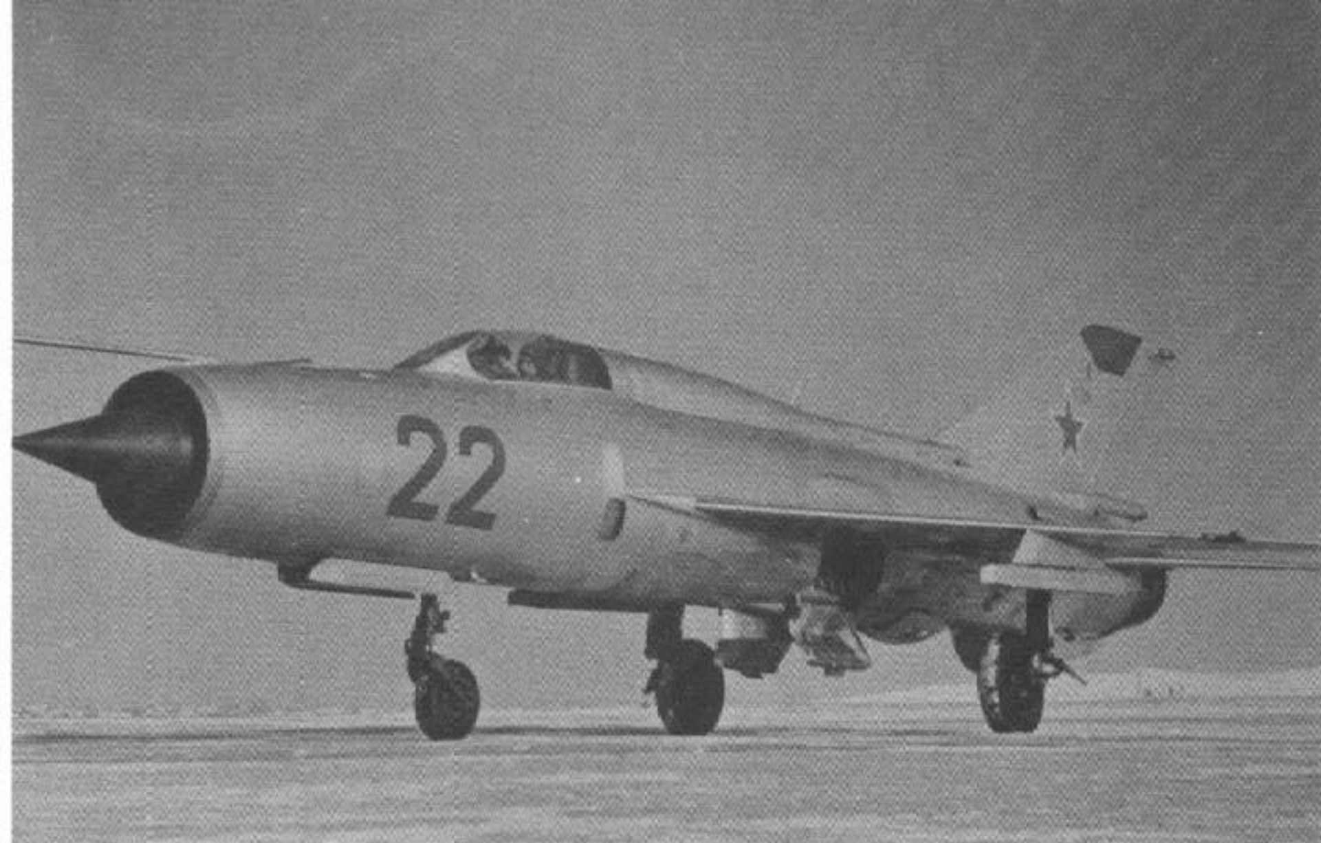
Red 22 was a late production Soviet Air Force MiG-21PF Fishbed D. The Fishbed D had an enlarged spine, larger main wheel doors and a larger main wheel fairing on the fuselage side. (Hans-Heiri Stapfer Collection)
