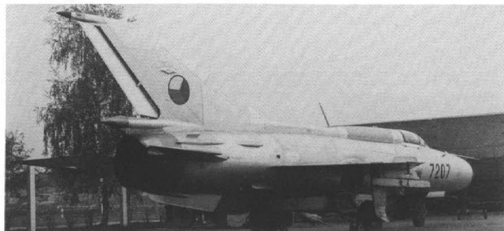
The wide chord fin was incorporated to improve stability and the under fin location of the braking parachute helped keep the aircraft on the runway centerline when landing. (Don Spring/AIR)
