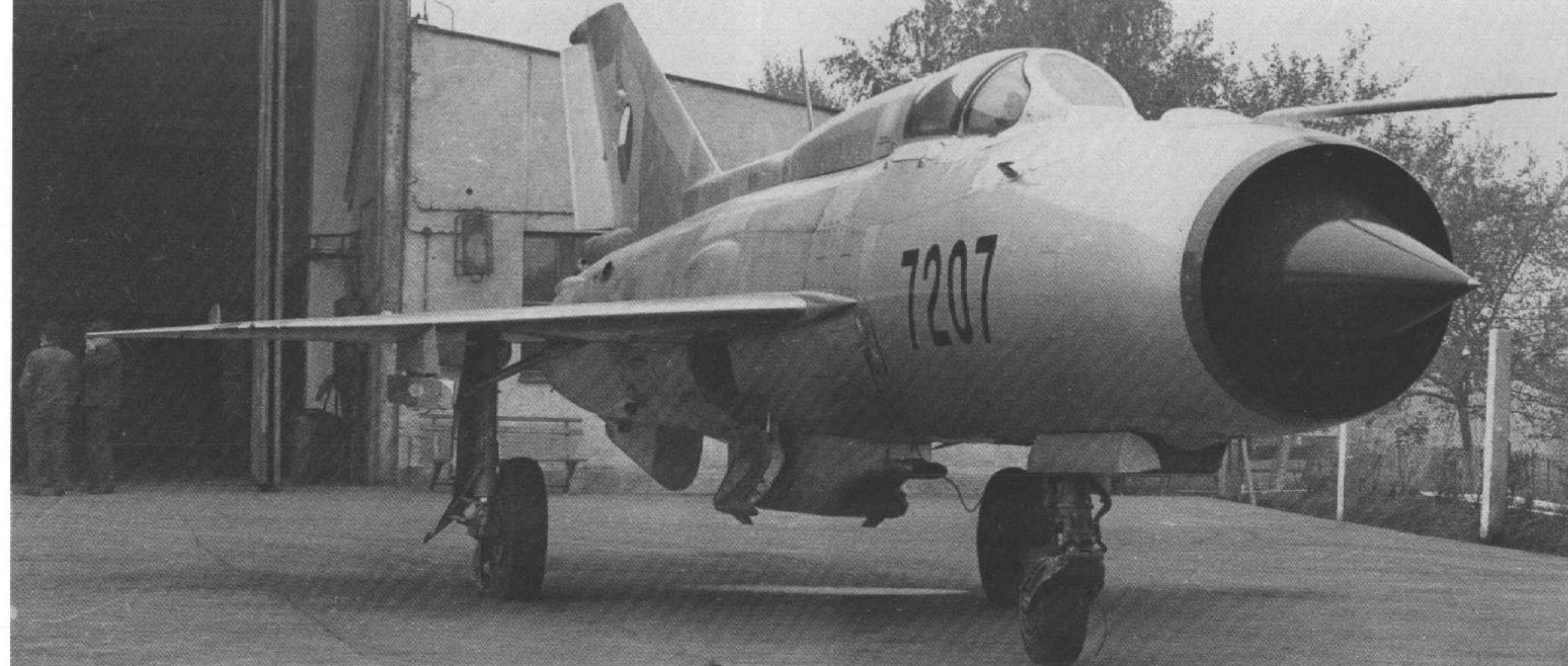
The increased diameter of the air intake is another feature that sets the MiG-21PF/PFM apart from the earlier Fishbed C. The center shock cone also housed the radar antenna for the RP-21 Sapphire air intercept radar. (Don Sperring/AIR)
