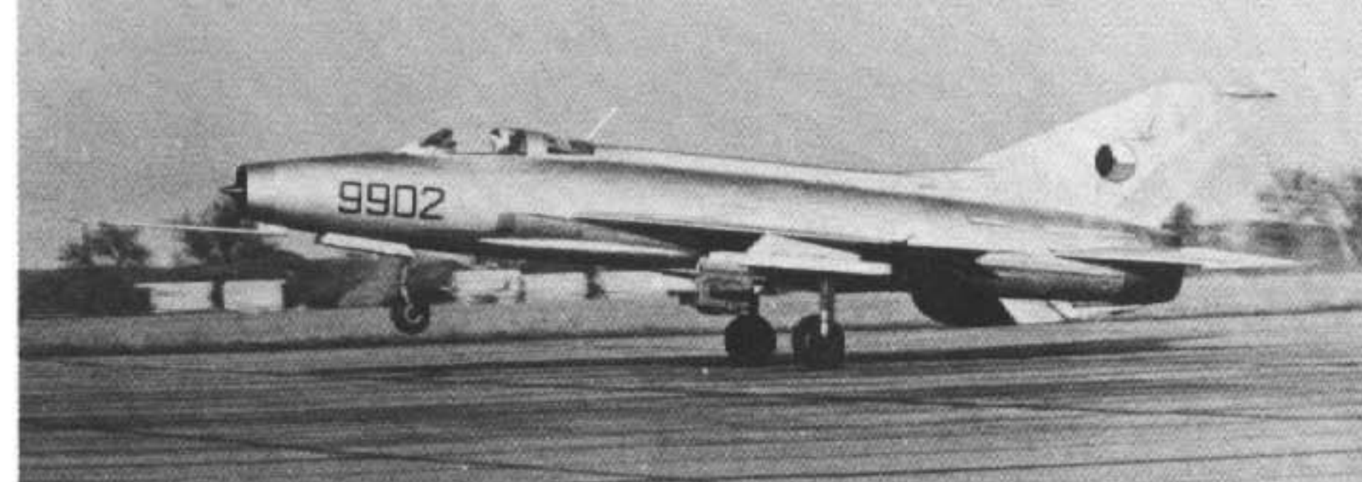
This Czech Air Force MiG-21F-13, Black 9902, takes off for a training sortie. This is a late production aircraft which has the port NR 30 30mm cannon deleted and the cannon port faired over. (Norm Taylor)
