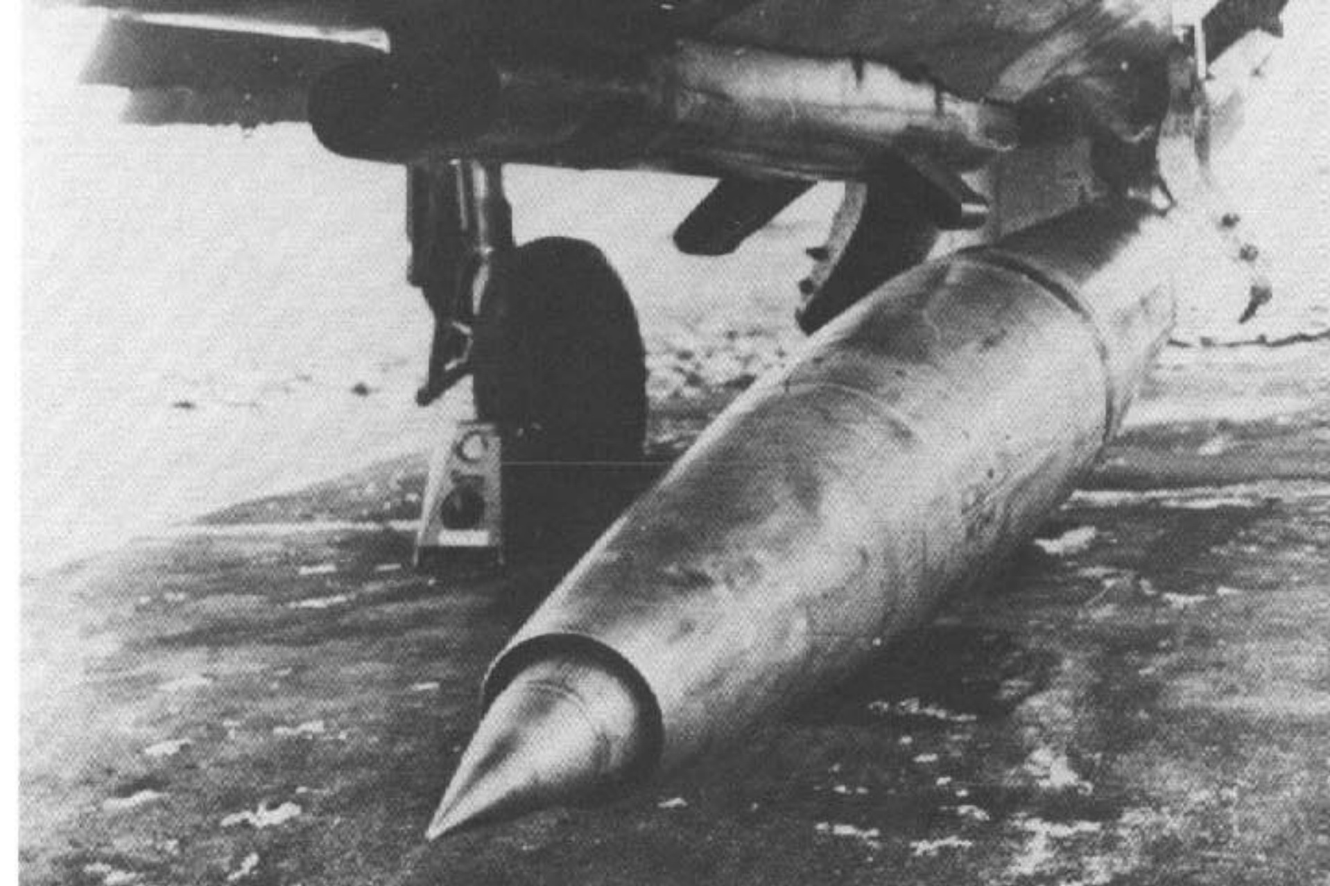
The twin barreled GSh-23L cannon was mounted semi-internal on the fuselage underside ahead of the fuselage pylon. This Soviet Air Force MiG-21MF carries an experimental 490 liter (129.4 gallon) drop tank on the centerline pylon. (Hans-Heiri Stapfer Collection)
