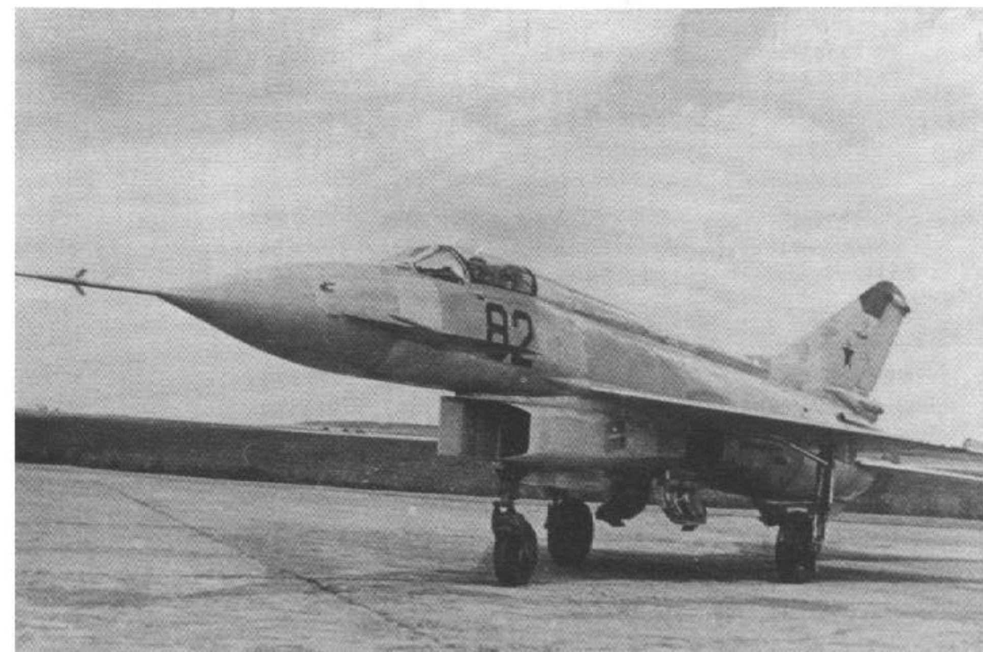
The Ye-8/2 prototype carried the tactical number Red 82 on the nose. The aircraft was developed from the MiG-21PF with a solid radar nose and the air intake moved under the fuselage. The Ye-8/2 flew for the first time on 29 June 1962 and made thirteen test flights before the crash of the first prototype Ye-8/1, Red 81, grounded the aircraft. (Hans-Heiri Stapfer Collection)
