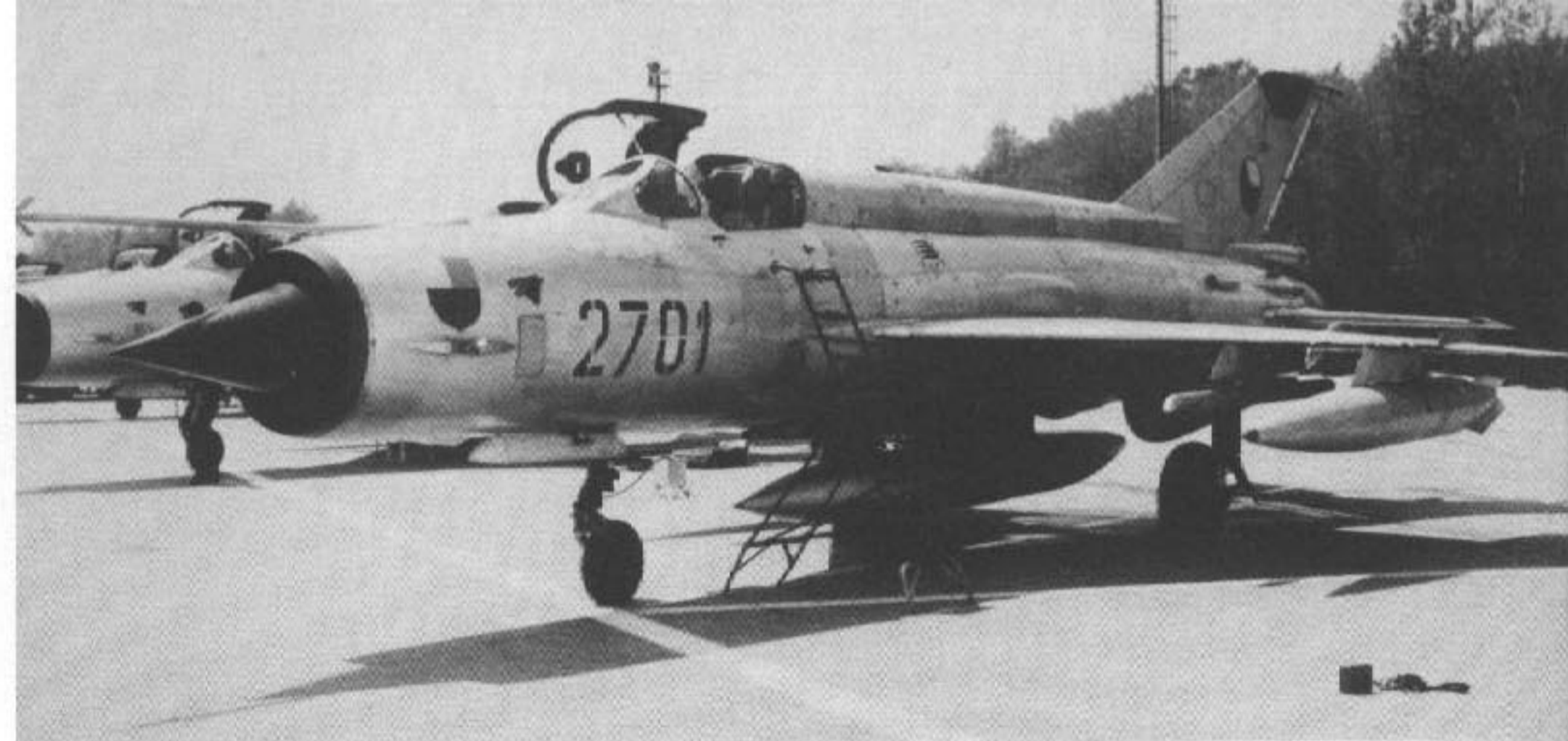
This Czech MiG-21MF Fishbed J carries a squadron insignia on the nose. These insignias were strictly forbidden during the cold war period but are now becoming common on former Warsaw Pact aircraft. The aircraft carries a 790 liter (208 gallon) tank on the centerline and a 490 liter (129 gallon) tank on the outboard wing pylon. (SIGMA via Roman Sekyrka)
