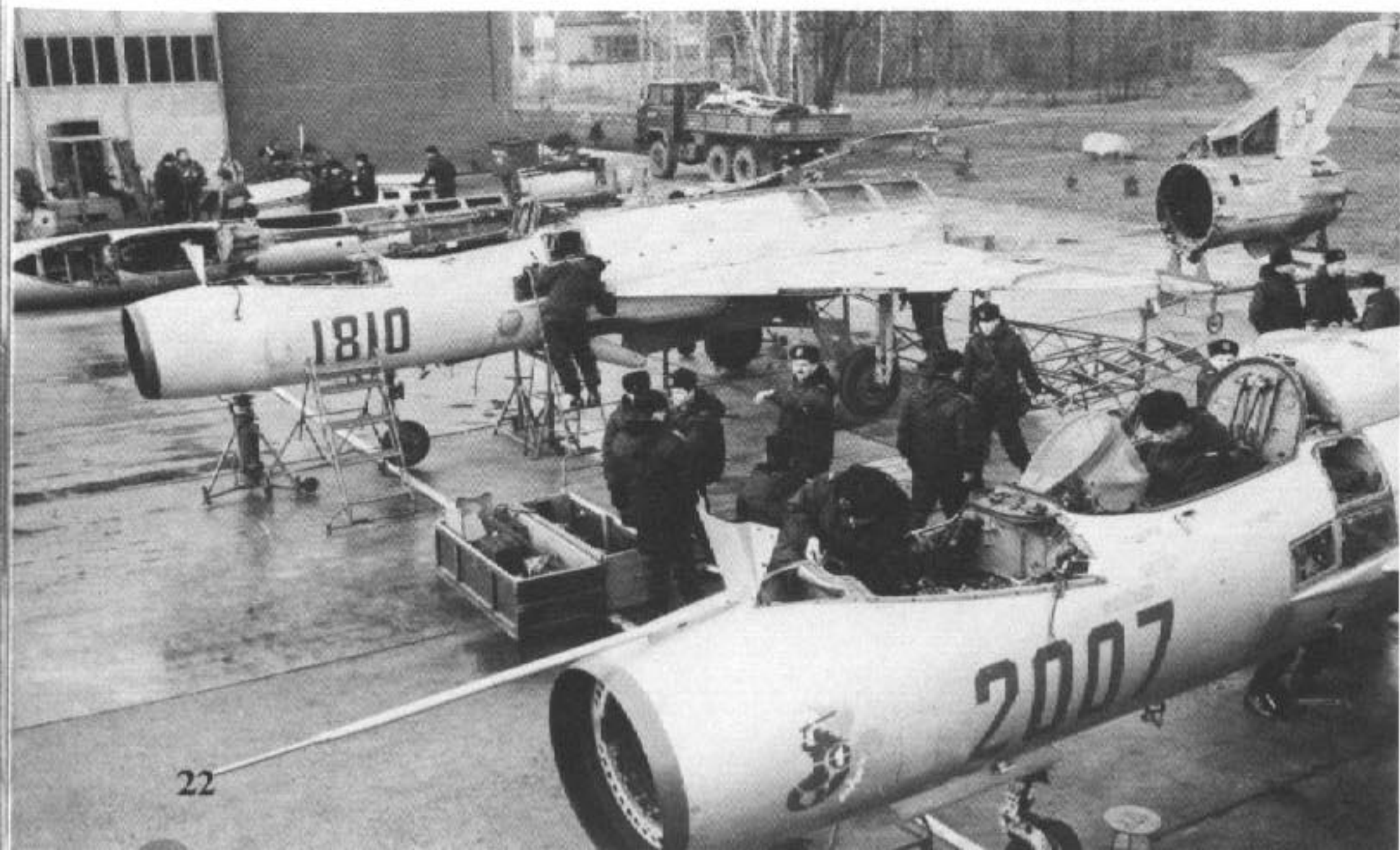
Polish Air Force MiG-21PF/PFM Fishbed Ds being stripped of usable parts before being scrapped. The lead MiG-21 is a PFM variant and carries the unit marking of the 1st Fighter Regiment Warszawa based at Minsk-Mazowiecki (the crest is that of the city of Warsaw). (via Rene van Woezik)
