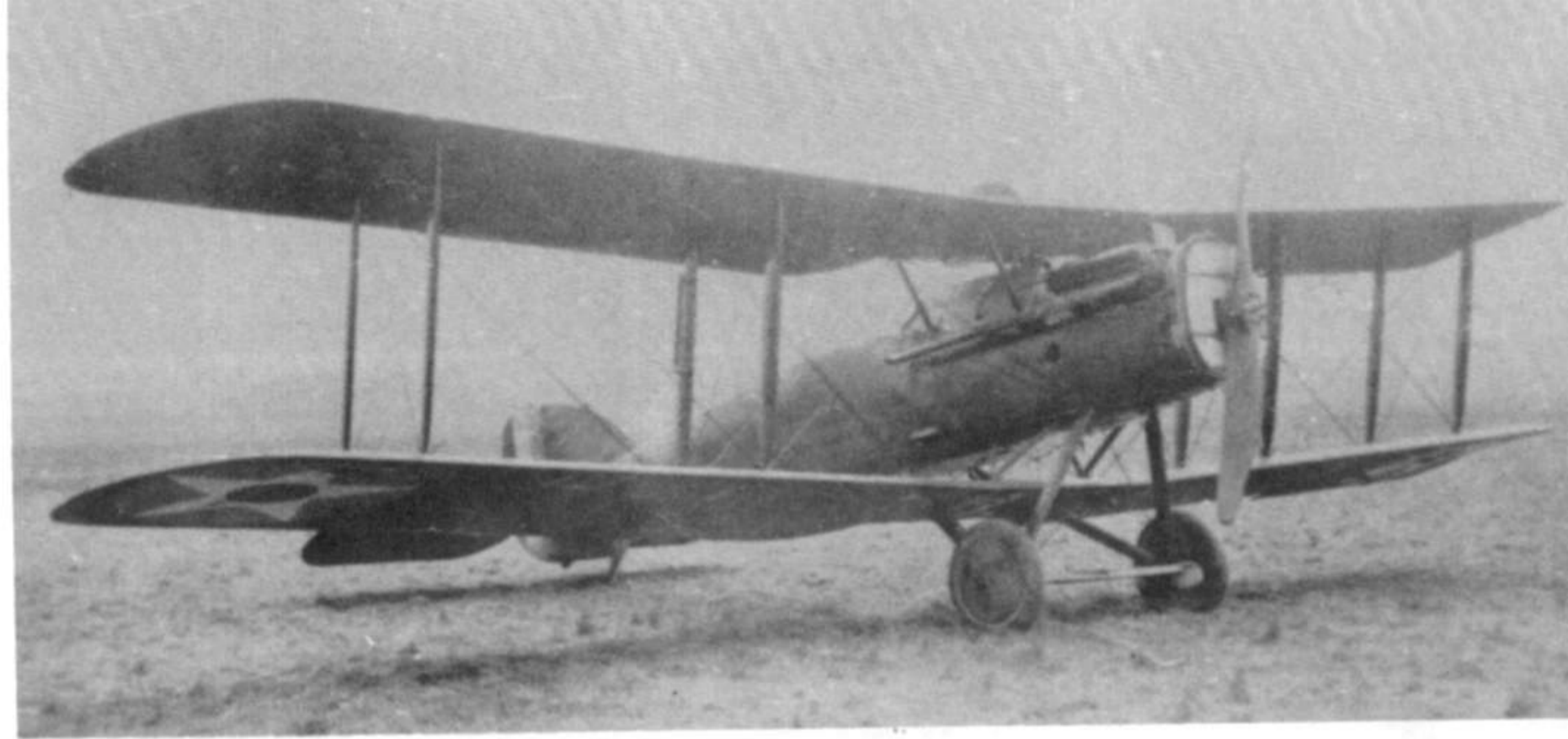
This XB-1A (serial A.S. 64158) was powered by a 300 hp Wright H (license built Hispano) liquid cooled engine and had the contractor number 179.
