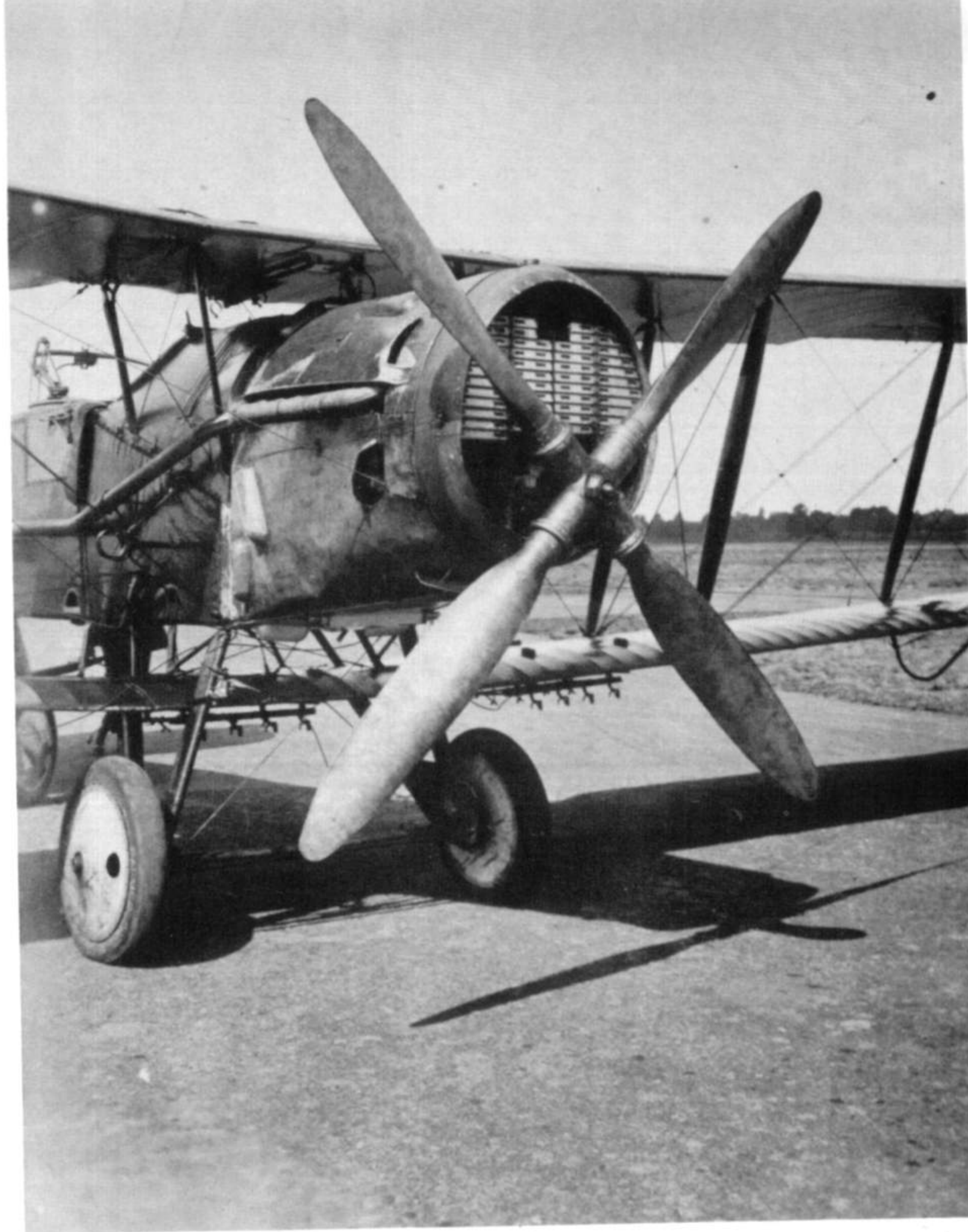
This Falcon III powered F.2B was experimentally fitted with a steel Leitner-Watts four blade propeller in place of the standard two blade wooden unit.
