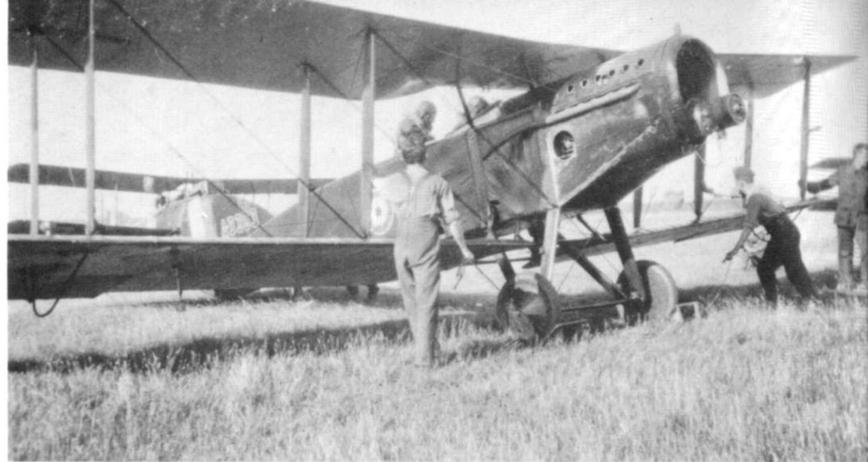
The F.2A prototype (A3303) is prepared for take off at Orfordness. A gun ring mount has been fitted for the observer and the serial number on the fin is outlined in white. The aircraft was used in an attempt to intercept German Gotha raiders on 7 July 1917.
