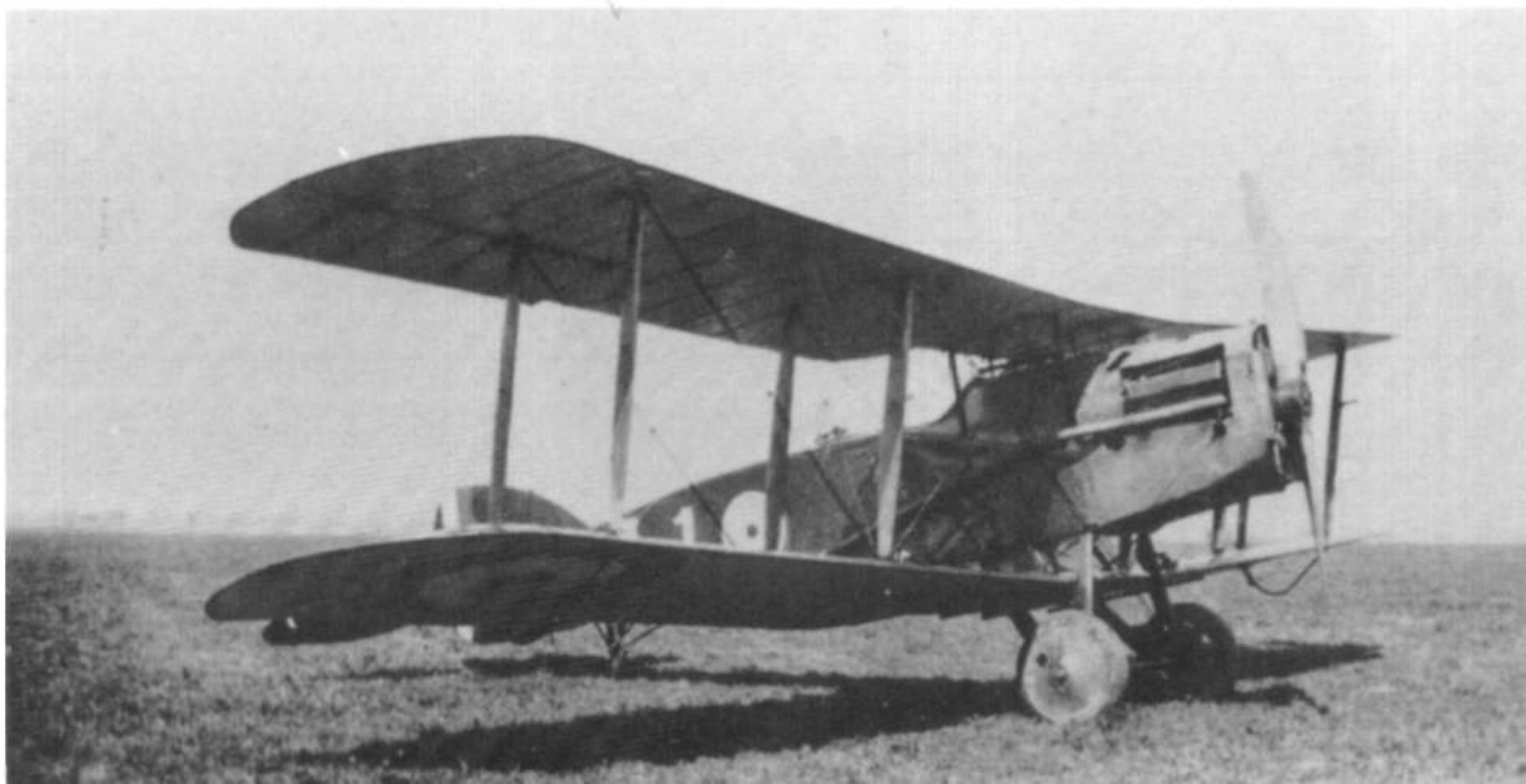
Carrying the individual aircraft number A1 on the fuselage in White, this F.2B was operated by "M" flight of the Long Range Artillery Spotters. The aircraft built by Gloucestershire Aircraft and was powered by a 204 hp Sunbeam Arab engine.
