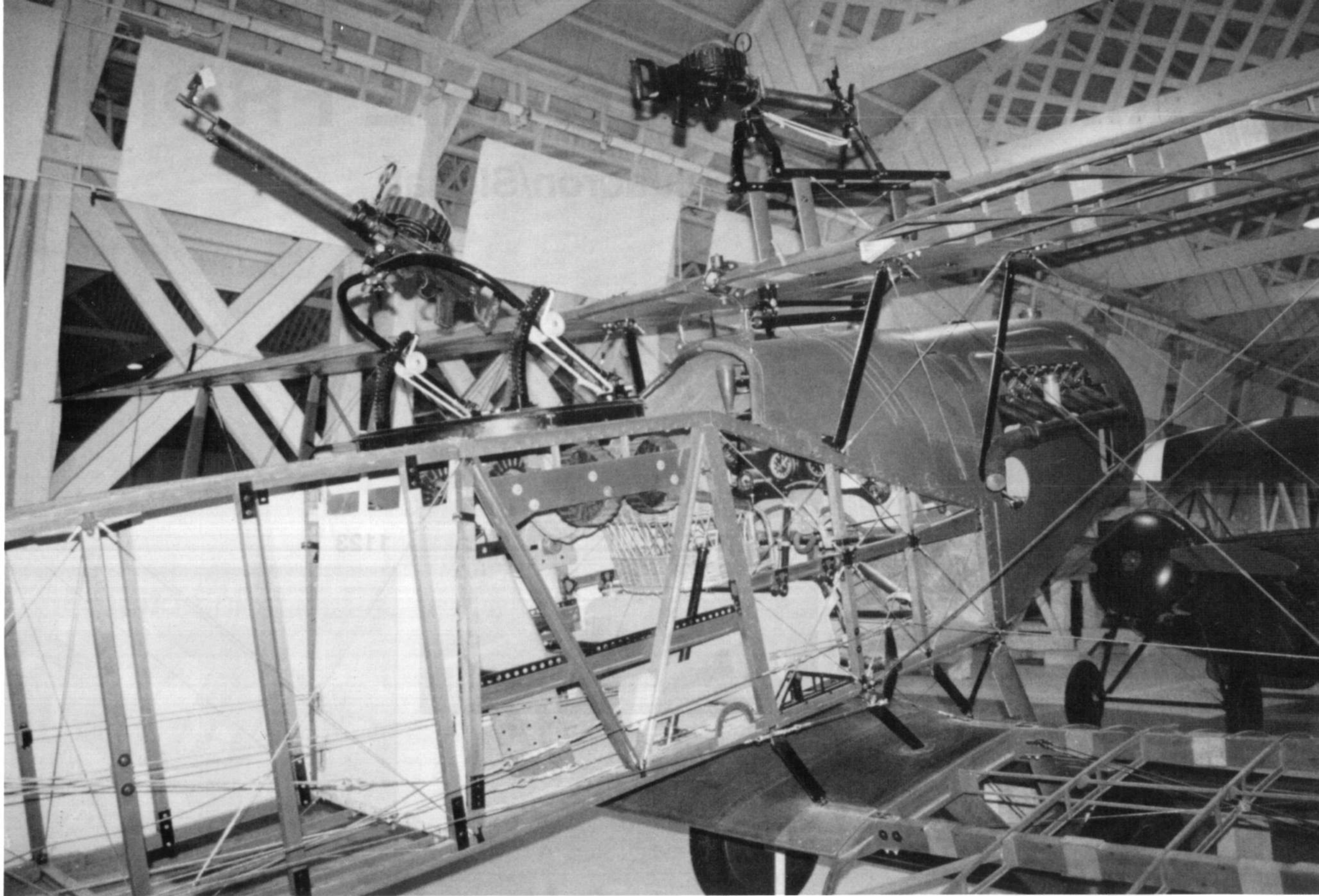
On display at the RAF Museum outside London, this F.2B has the fabric on the fuselage and lower wing removed to show the interior of the aircraft. The guns are .303 inch Lewis machine guns, the one over the wing being a modification done at the squadron.
