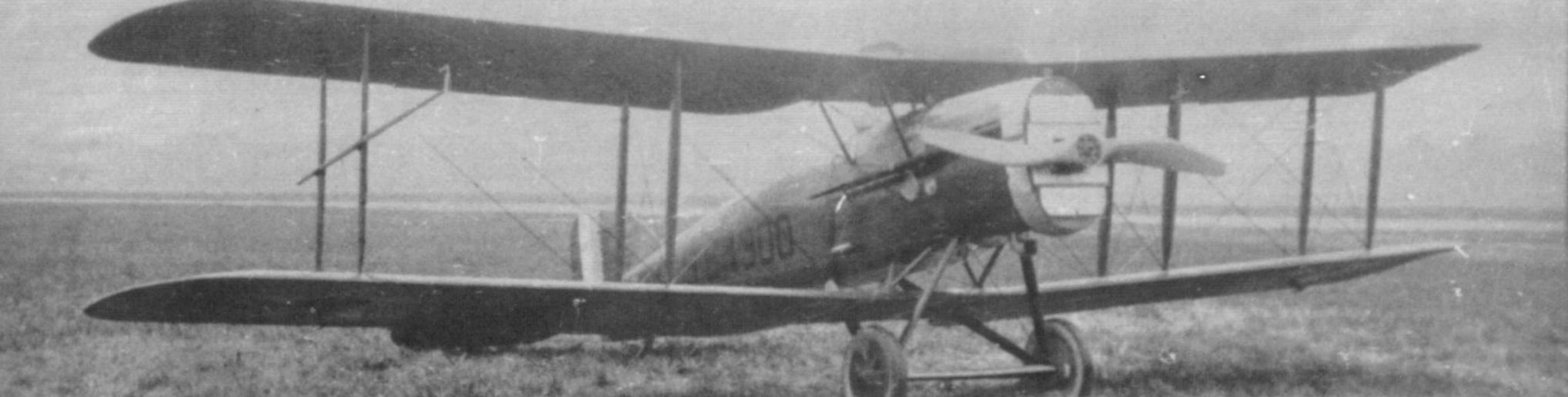
B-1A (A.S. 64156) has the serial number repeated on the rudder in small Black letters across the rudder stripes. The aircraft was fitted with a 420 hp Curtiss D.12 liquid cooled engine.
