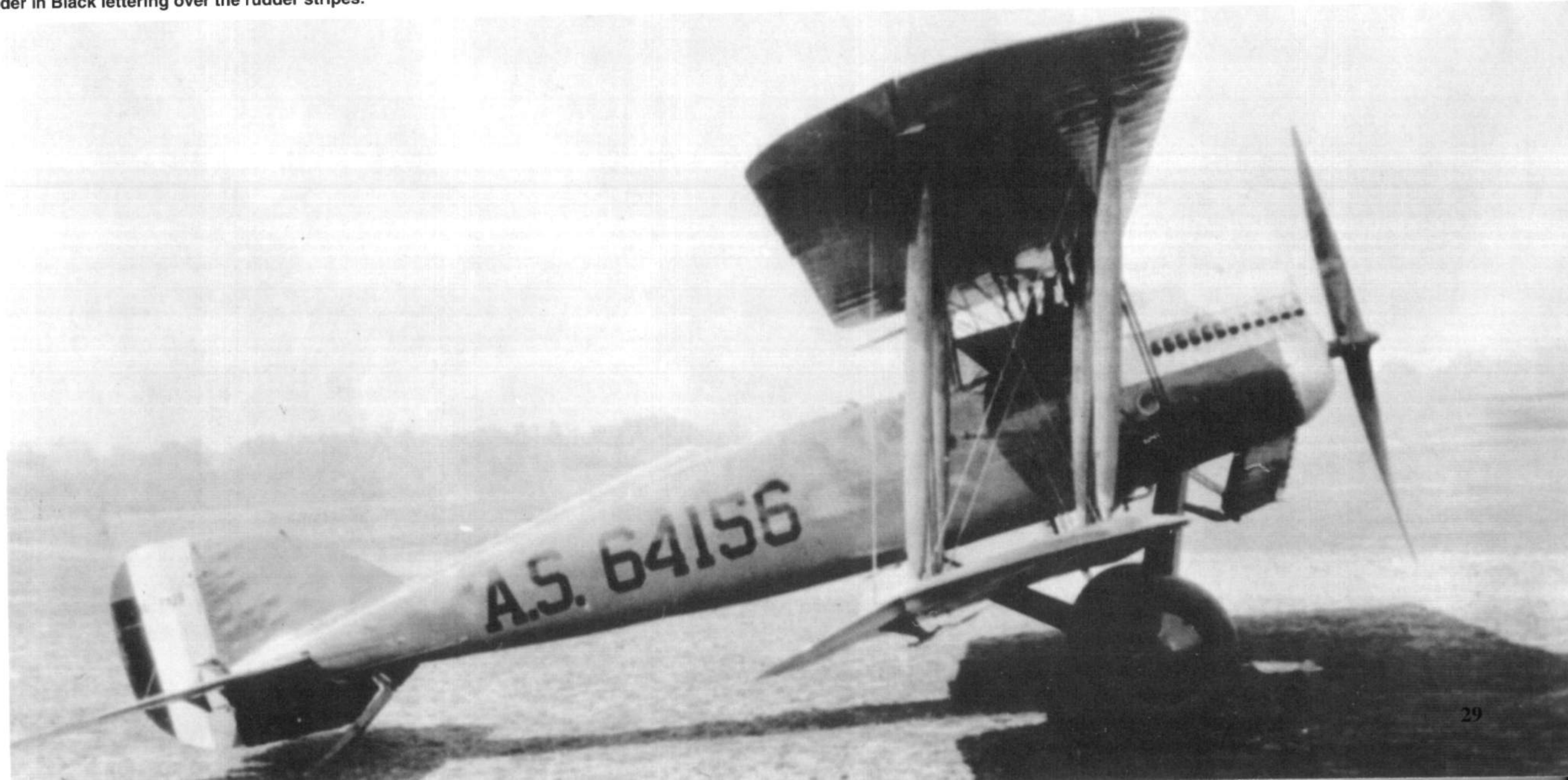
This XB-1A (serial A.S. 64158) was powered by a 300 hp Wright H (license built Hispano) liquid cooled engine and had the contractor number 179.
