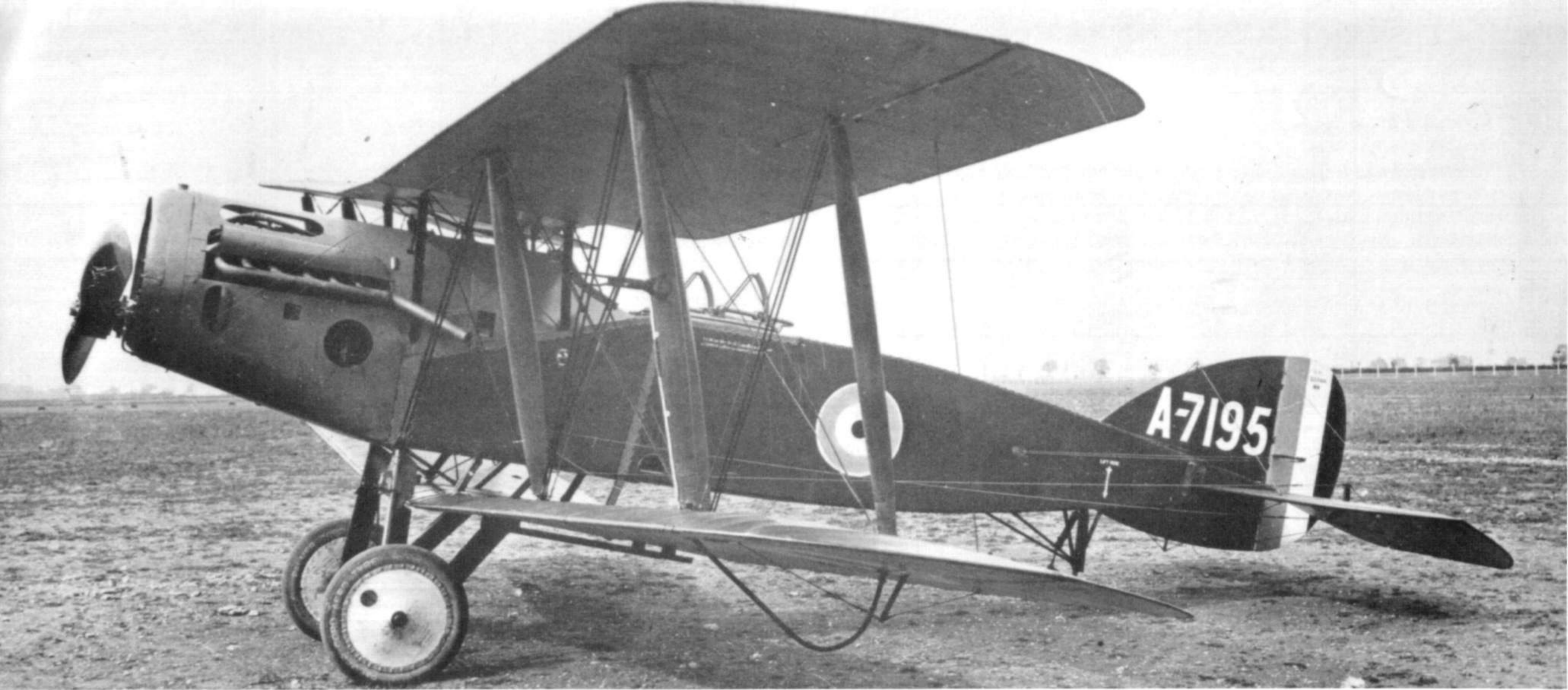
This early production F.2A on the landing ground at Ayr, Scotland during April of 1917 was from the first production batch. It was powered by a 190 hp Falcon I engine. The aircraft was lost in action later this same month.
