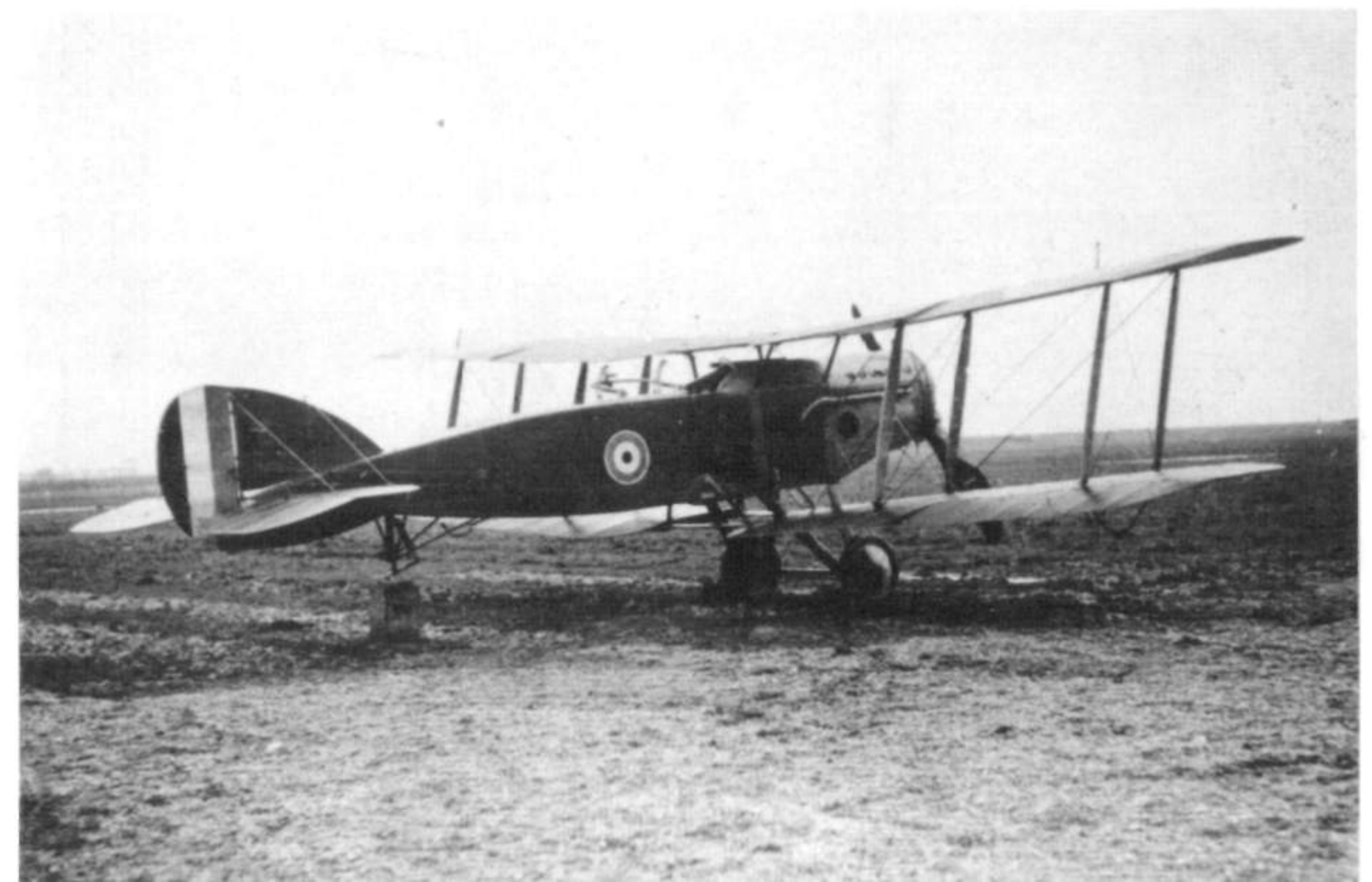
The first F.2A prototype (A3303) at the experimental armament center at Orfordness after it was modified with a frontal radiator. The end plates have been removed from the lower wing roots on the lower center section remains uncovered.
