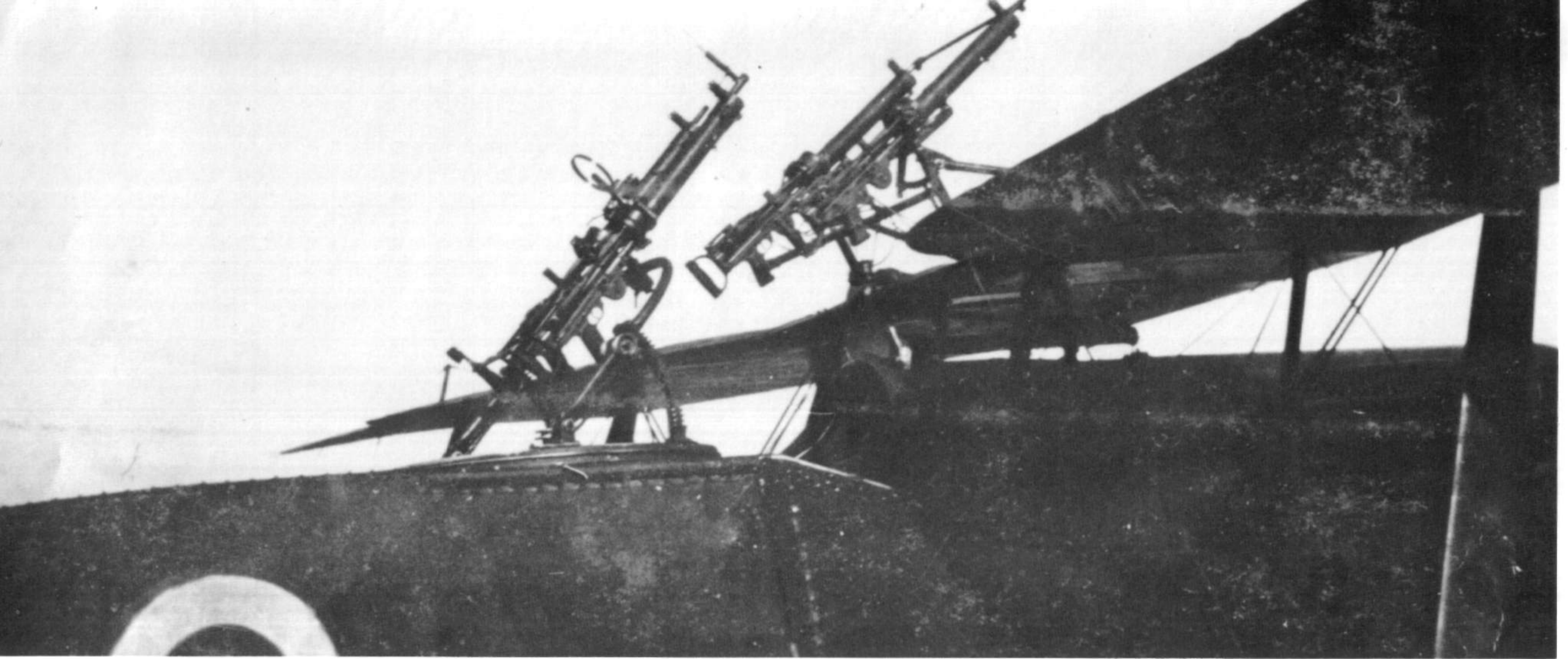
This F.2B has twin .303 inch Lewis machine guns mounted above the upper wing center section and a twin Lewis mount in the observer cockpit. It is believed that this F.2B was a night fighter assigned to No 39 (Home Defense) Squadron.
