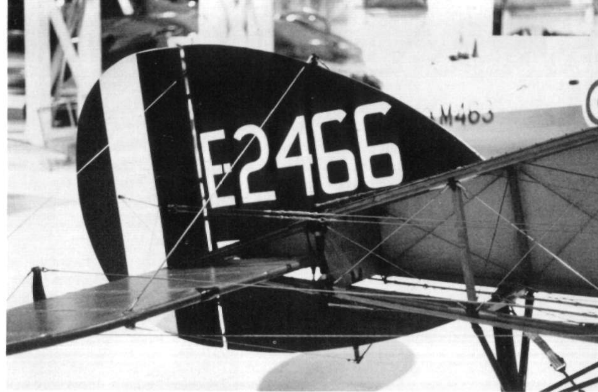
The tail unit of E2466 shows the pushrods and pulleys of the elevator and rudder controls, along with the bracing wires that run from the vertical fin to the horizontal stabilizer. E2466 is on permanent display at the Royal Air Force Museum, Hendon, London.
