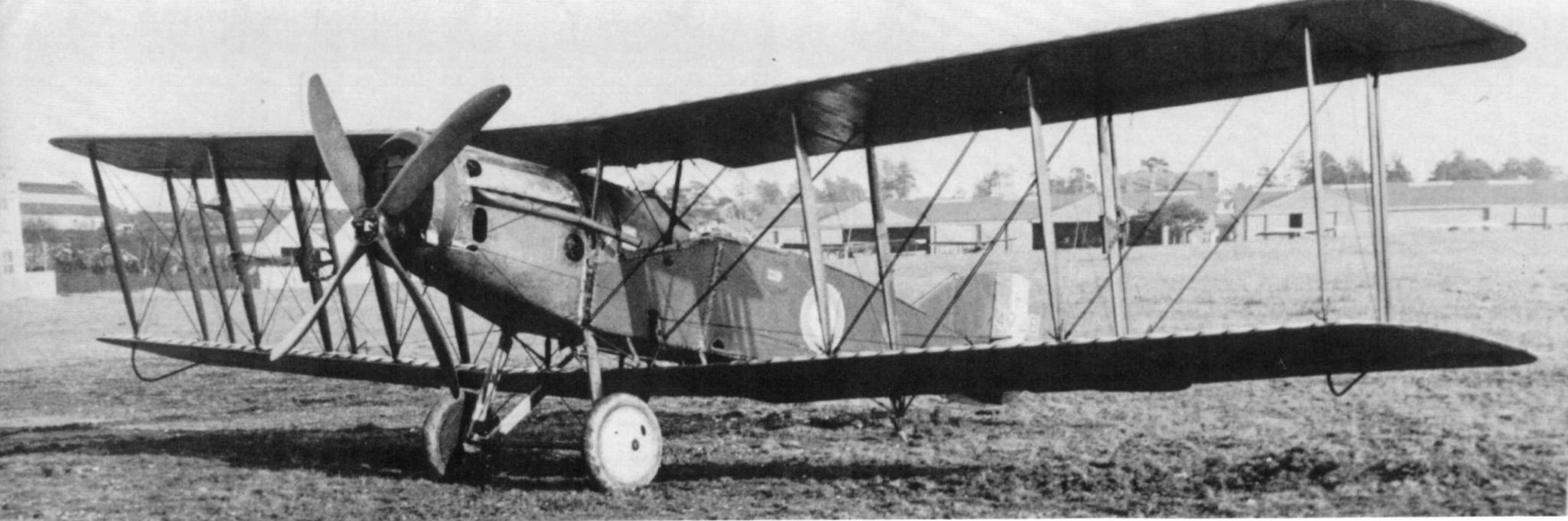
This F.2B was modified with three bay wings and flown at the Experimental Establishment at Farnborough. The aircraft was involved in trials with the three-bay wing which had an aspect ratio of 9.78.
