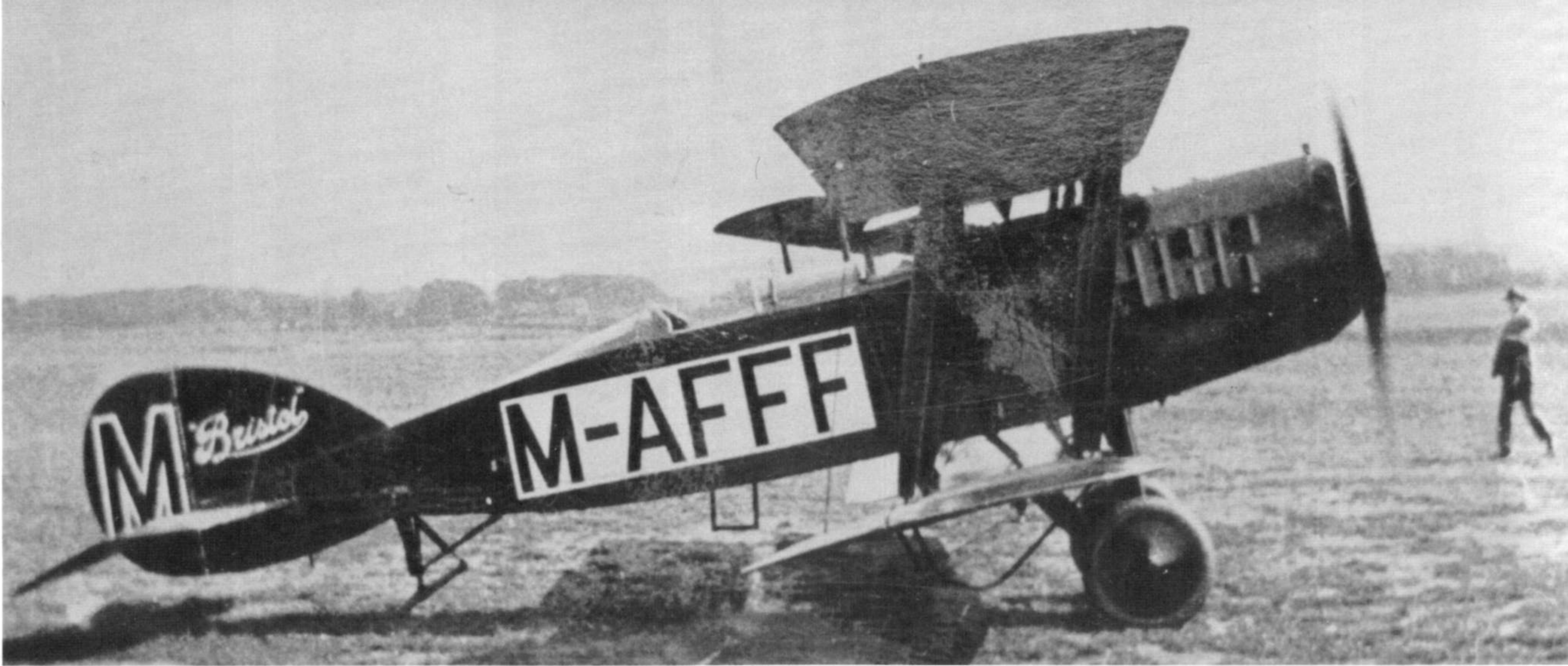
This F.2B at Waddon, Croydon during September of 1921 has been converted to a three seat touring aircraft (c/n6110). The aircraft carries a Spanish civil registration and represents one of several unusual conversions of surplus F.2Bs that were common on the civil market during the immediate post First World War period. The aircraft carries the Bristol company logo on the vertical fin in White. The registration is believed to have been Black against a White background.
