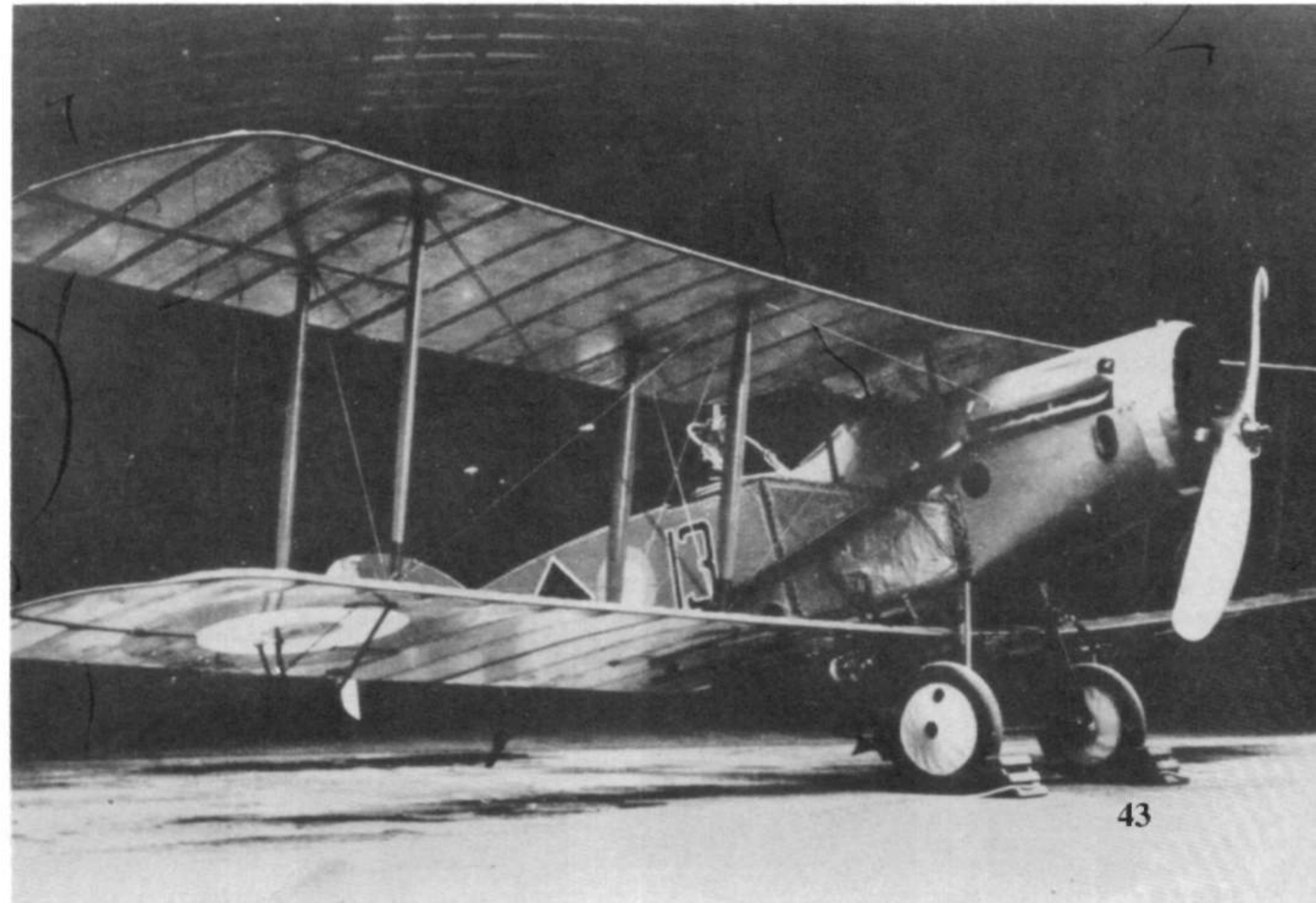
This F.2B at Waddon, Croydon during September of 1921 has been converted to a three seat touring aircraft (c/n6110). The aircraft carries a Spanish civil registration and represents one of several unusual conversions of surplus F.2Bs that were common on the civil market during the immediate post First World War period. The aircraft carries the Bristol company logo on the vertical fin in White. The registration is believed to have been Black against a White background.
