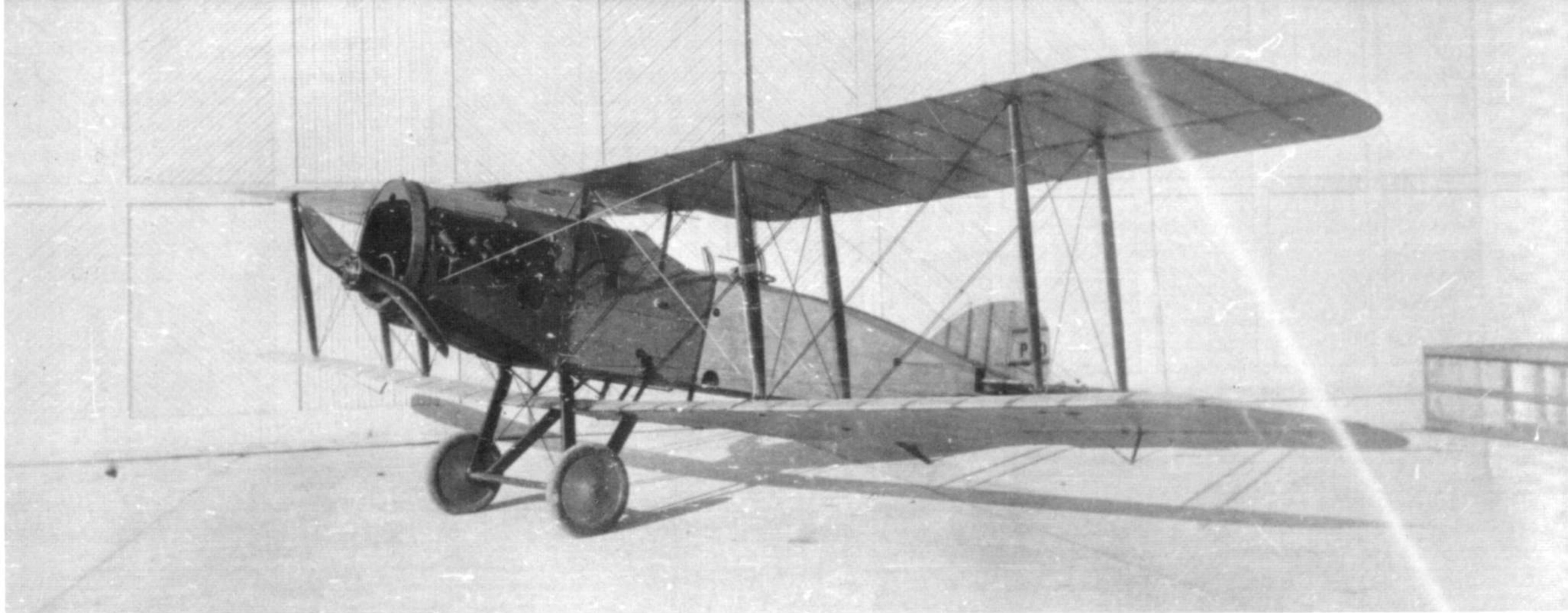
The P-30 was originally an F.2B (serial A7203) which was re-engined with a 300 hp Hispano-Suiza engine. The aircraft set a new altitude record over Dayton, Ohio on 18 November 1918, while based at McCook Field.
