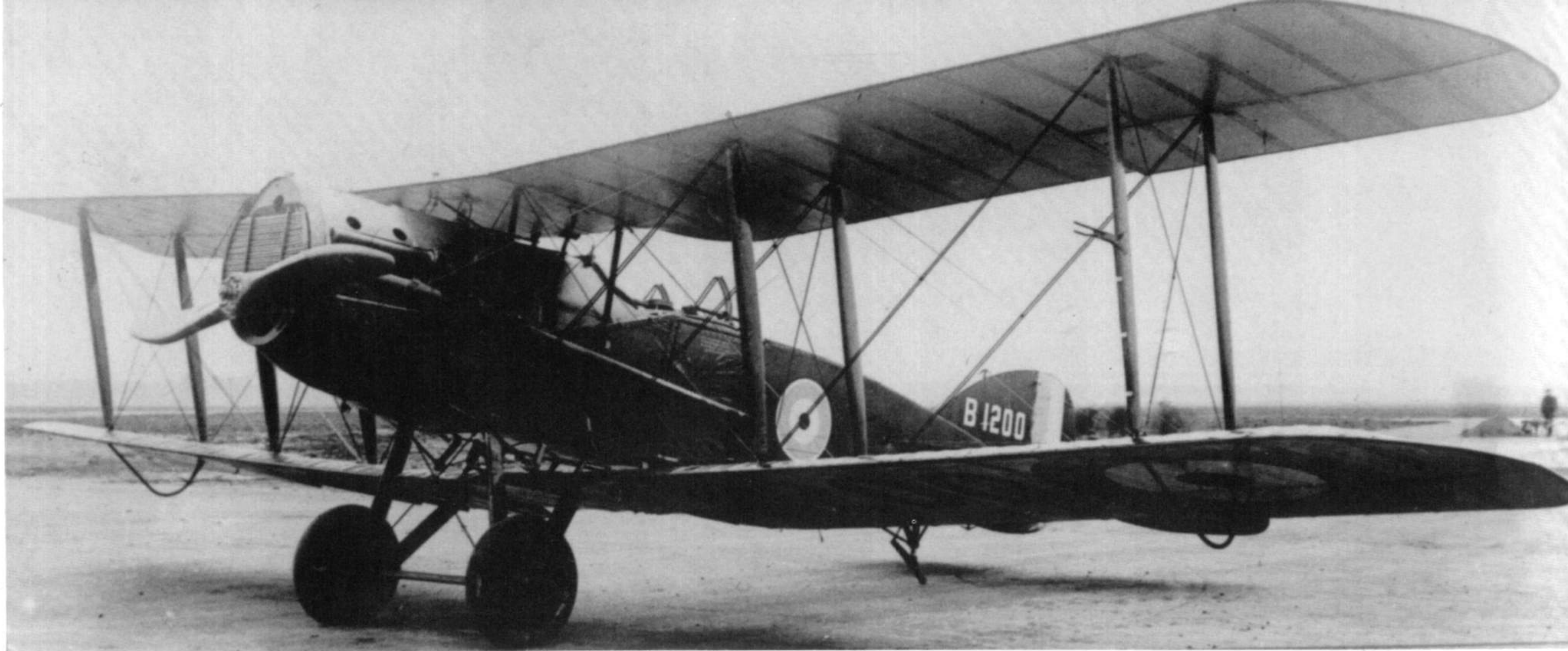
To solve the engine shortage problem, an number of F.2Bs were tested during the war years with different engines. This F.2B (B1200) at the experimental establishment at Marlesham Beath in September of 1918 was powered by a 200 hp Wolsey Viper liquid cooled engine.
