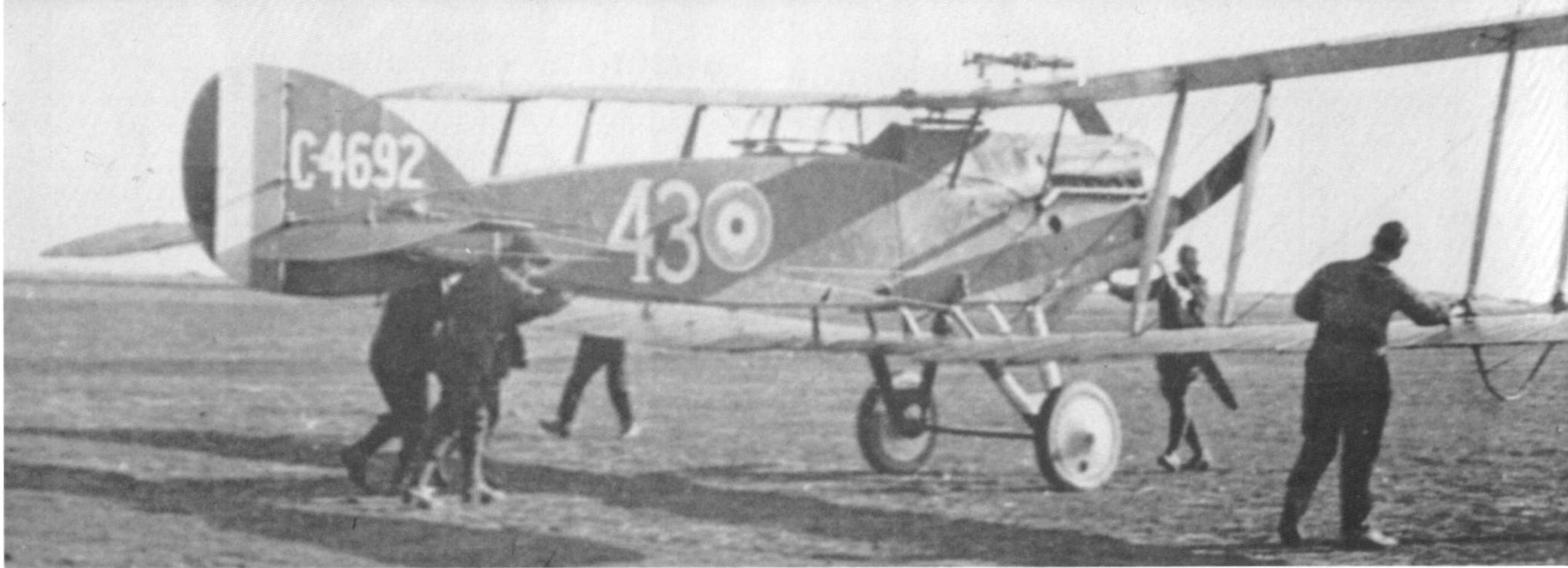
Ground crews reposition this F.2B (C4692) on the landing ground at Marske. The aircraft appears to have a camera-gun mounted above the upper wing center section and is equipped with a four blade propeller.
