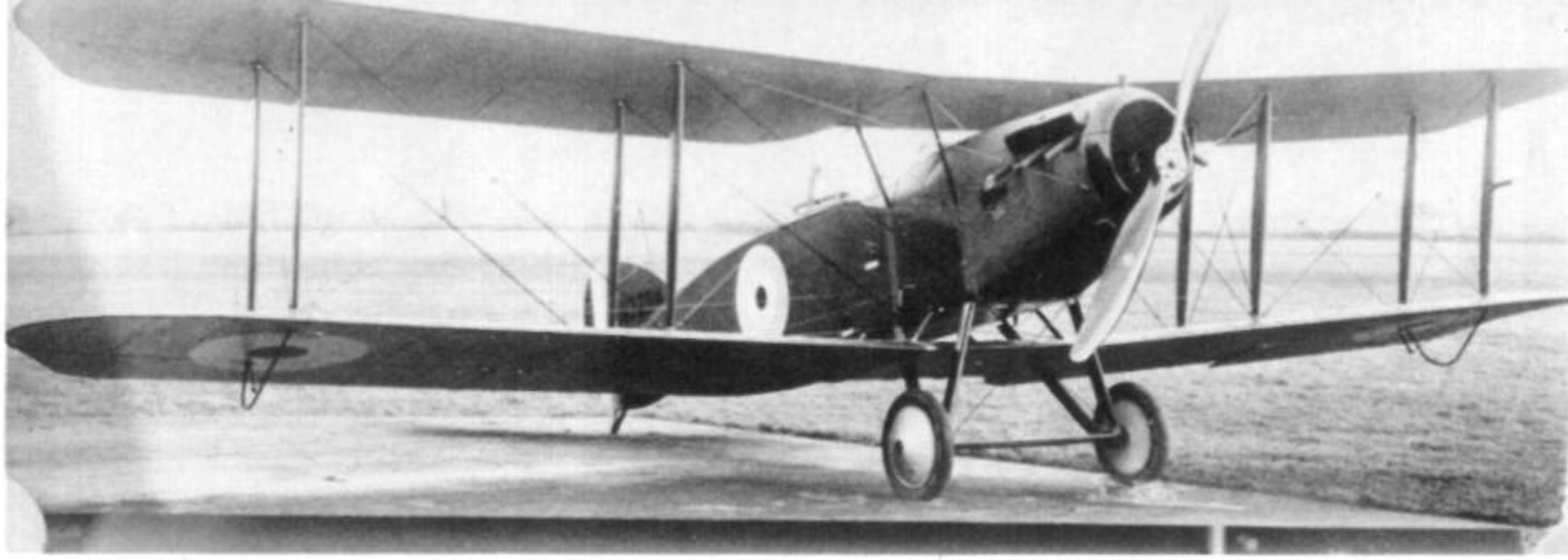
The second F.2A prototype at Filton in December of 1916 has a Scarff ring in the rear cockpit and a circular radiator. The gap in the lower wing center section is covered and the forward fuselage longerons are sloped bringing the aircraft up to F.2B standard.
