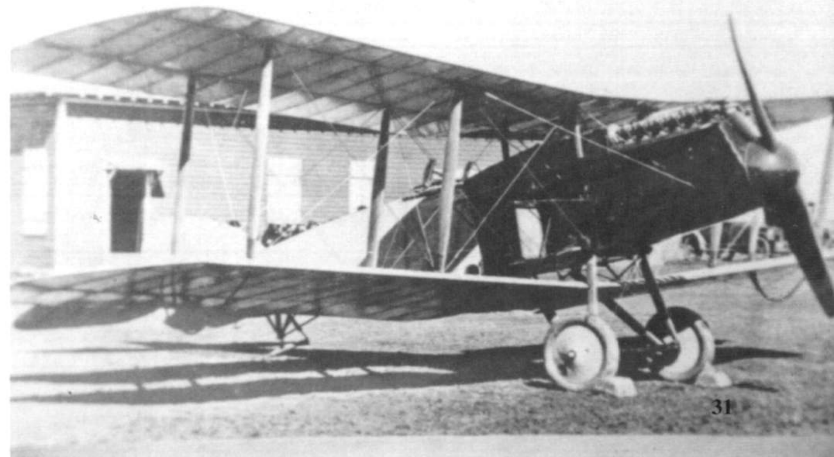
The second F.2B to be sent to the U.S. was re-engined with a 290 hp Liberty 8 engine. The P37 still carried British national markings at McCook Field during the Summer of 1918. The aircraft was destroyed before trials could be carried out.
