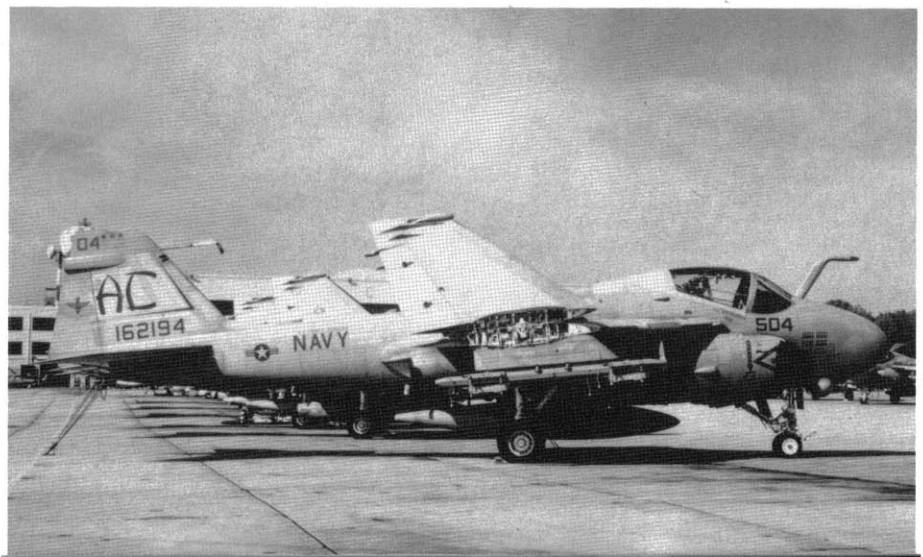
This A-6E TRAM of VA-75 Sunday Punchers off the USS JOHN F. KENNEDY (CV-67) carries thirty-four DESERT STORM mission markings on the nose in Black just in front and below the aircraft side number . The weathering and use of different shades of Gray for touch ups during maintenance makes the aircraft appear very patchy. (Author)
