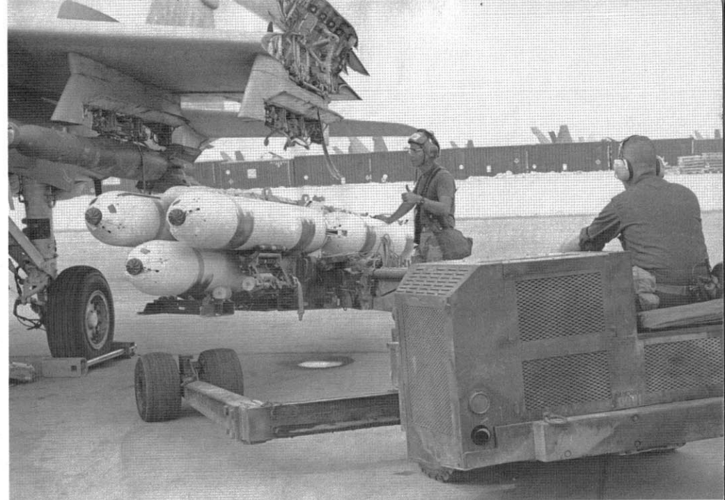
An A-6E TRAM of VMA-224 being loaded for another mission over Kuwait during DESERT STORM. The Marine unit was based in Bahrain and shared this location with FA-18 Hornets (in the background). A load of Rockeye cluster bombs attached to a MER is being loaded on the outboard pylon, while a Laser Guided Bomb (LGB) is already in place on store station 2. (CPL Murray van Pelt USMC)
