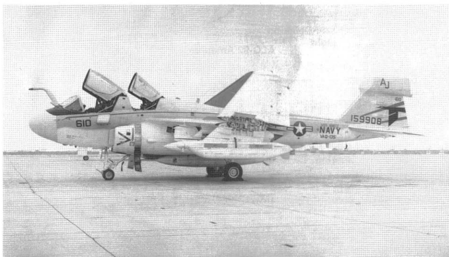
This EA-6B Prowler ICAP I of VAQ-135 Black Ravens assigned to USS NIMITZ. The port boarding platform on the pilot's side is in the open position and both boarding ladders are in the lowered position. The raised canopies have a Goldish tint unlike the windshield, which is clear. (Bruce Trombecky)
