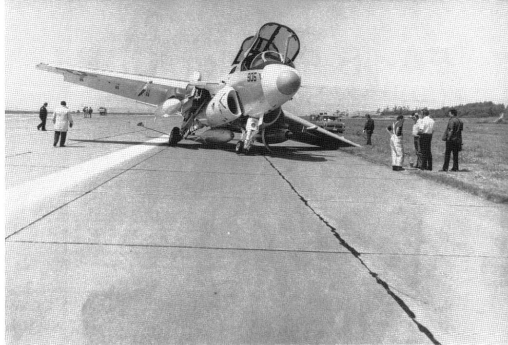
An EA-6B EXCAP Prowler (BuNo 158811) of VAQ-129 comes to rest on its port wingtip after the port main landing gear failed during an arrested landing at Naval Air Station Whidbey Island during July of 1981. The aircraft has four mirrors on the inside of the forward canopy framing. (USN)
