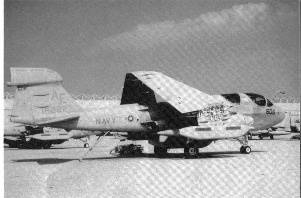
The most recent VAQ squadron is VAQ-142 Grim Watchdogs, which was established as the thirteenth EA-6B Prowler squadron on 1 June 1988. This VAQ-142 aircraft was visiting NAS Cecil Field NAS in August of 1989. The blotchy appearance of the aircraft shows the intense effort of maintenance personnel to control corrosion. (Jim Tunney)
