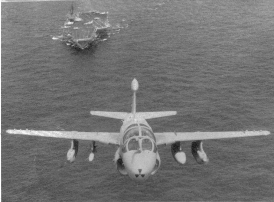
An EA-6B ICAP II Prowler of VAQ-138 Yellow Jackets climbs away from USS CONSTELLATION (CV-64). The aircraft is carrying an AGM-88A High Speed Anti-Radiation (HARM) missile on the starboard inboard pylon. The ICAP II was the first variant of the EA-6B Prowler to be armed. (USN)
