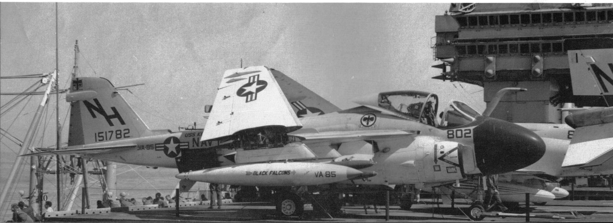
This A-6A of VA-85 was parked next to the deck edge elevator aboard USS KITTY HAWK (CVA 63) during 1965 with the nose wheel tow bar in place. It carried the standard paint scheme of Light Gull Gray (FS 16440) and Insignia White (FS 17875). The Black radome was soon changed to a White neoprene coating (starting with BuNo 155642). (Lionel Paul)
