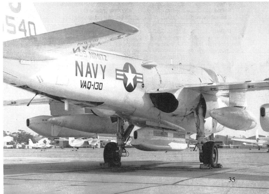
The underside of the centerline station of an EA-6B (looking forward) showing the rear of an early low band AN/ALQ-99 jammer pod which had a wider bottom than the pod now in use. The four curved pipes are engine bay vents. (Bruce Trombecky)
