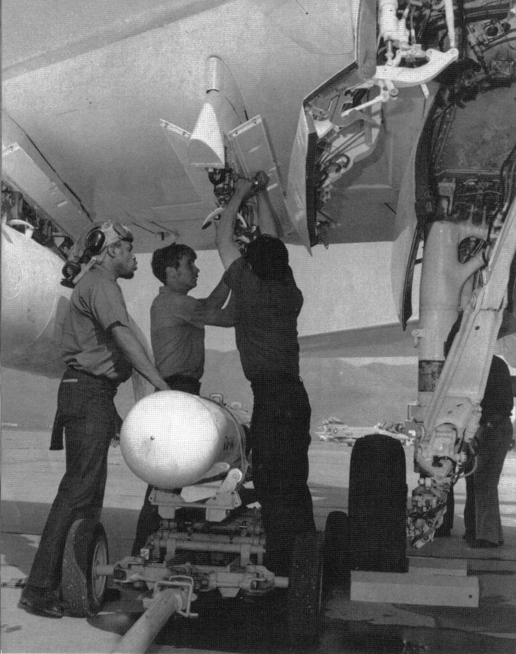
Ordnancemen check the internal bomb locks on the starboard inboard weapons pylon of an A-6E (TRAM) Intruder prior to loading a Harpoon air-to-surface (ASM) missile at the Pacific Missile Test Center (PMTC) which is located at Naval Air Station Point Mugu, California. (PH1 Jerry Jolin USN)
