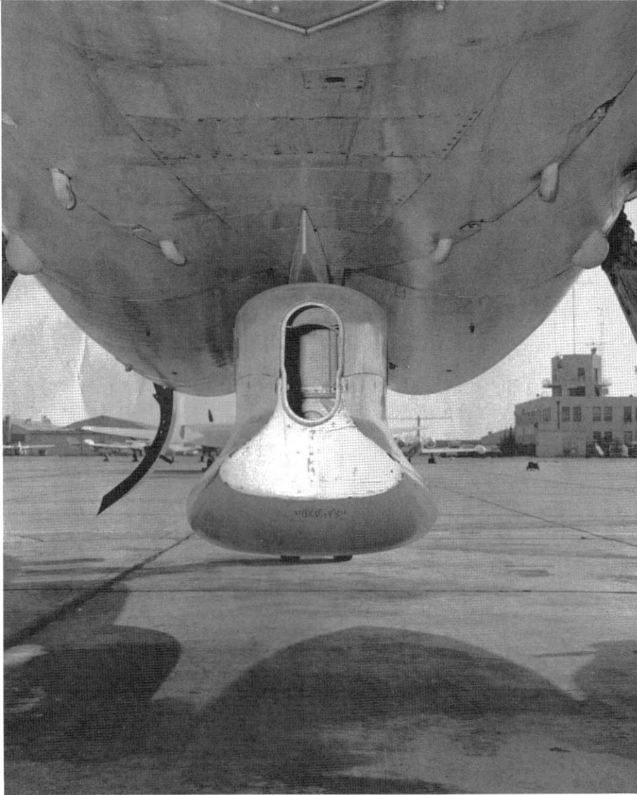
The underside of the centerline station of an EA-6B (looking forward) showing the rear of an early low band AN/ALQ-99 jammer pod which had a wider bottom than the pod now in use. The four curved pipes are engine bay vents. (Bruce Trombecky)
