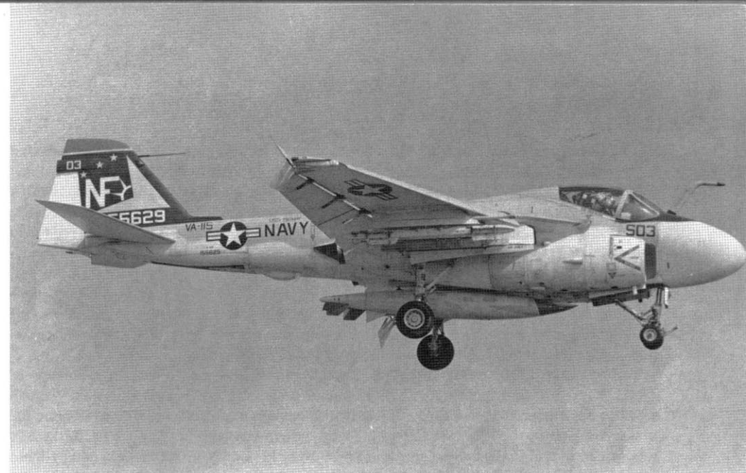
An A-6B (BuNo 155629) PAT/ARM of VA 115 off USS MIDWAY (CVA-41) lands at Atsugi, Japan in October of 1974. This variant of the A-6B did not carry the external blisters and radar receiver button antennas because of an internal modification to the radar system that rendered these unnecessary. (Lionel Paul)
