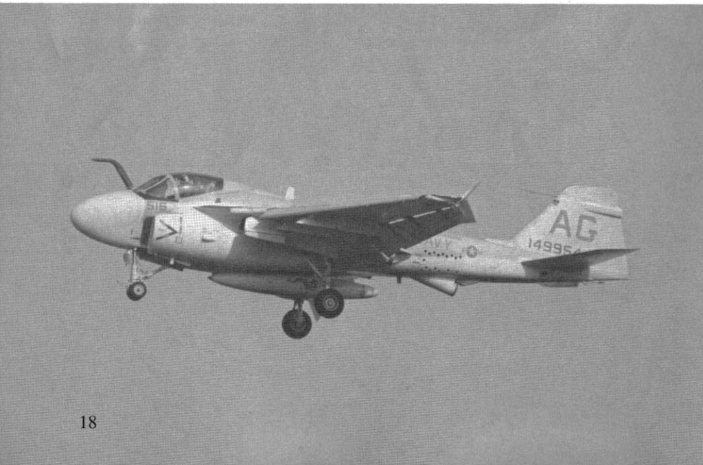
A KA-6D of VA-65, attached to Air Wing Seven deployed aboard USS EISENHOWER (CVN-69) on final approach for landing at NAS Oceana, Virginia. The omega system blade antenna used for navigation is visible just to the rear of the cockpit. (Don Linn)
