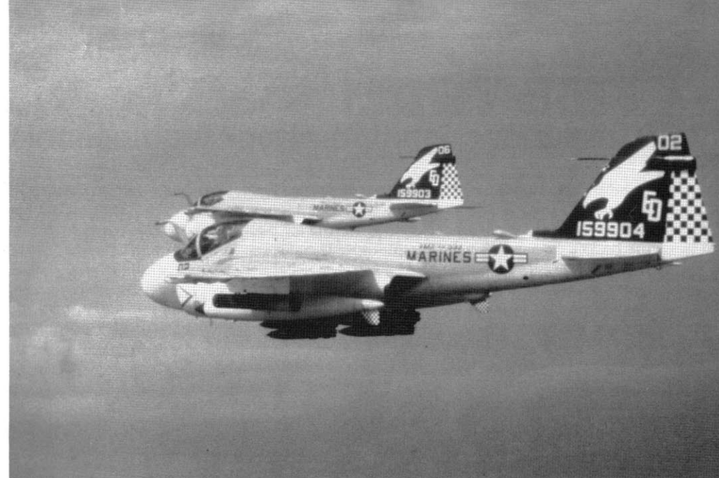
Two Marine A-6Es of VMA(AW)-533 fly formation over the Pacific Ocean in December of 1982 armed with Mk 82 Snakeeye bombs on the centerline station and a LAU-10 rocket launcher pod on the wing station. The LAU-10 has not been fitted with its streamlined nose and back covers. (T. Metler)
