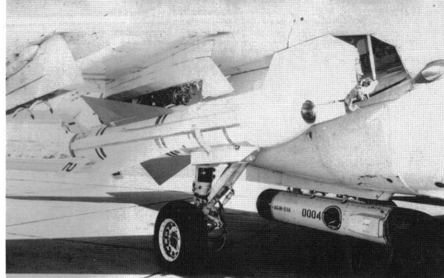
This A-6E is armed with an AGM-53 Condor missile carried on the number 4 stores station (inboard starboard wing pylon) along with a data link electronics pod on station number 3 (fuselage centerline pylon). The missile had alternating Red and White forward fins. (USN)
