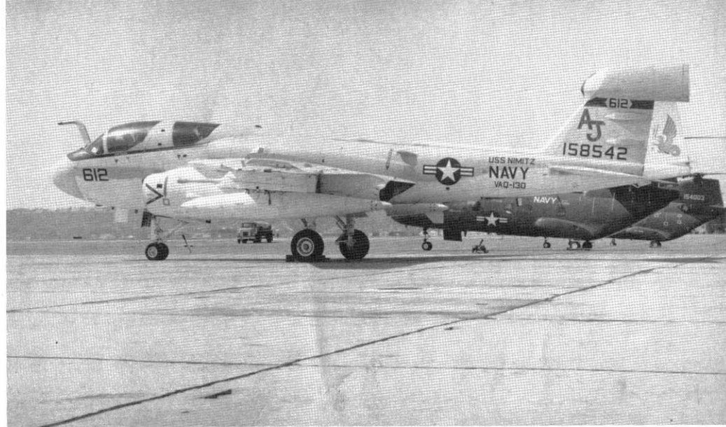
An EA-6B Standard Prowler of VAQ-130 off the USS NIMITZ parked on the transit line at NAS North Island, California. The probe extending from the outboard pylon is the antenna for the AN/ALQ-100 ECM system. (Bruce Trombecky)
