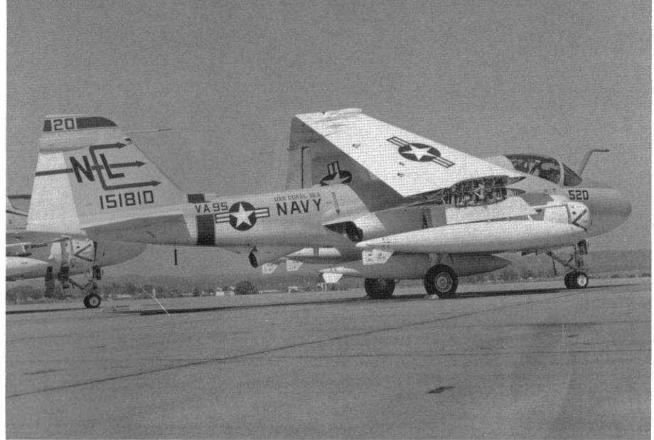
This KA-6D of VA-95 Green Lizards has the camouflage demarcation carried out onto the radome, with a Dark Gull Gray anti-glare panel in front of the canopy. There is a Red Remove Before Flight tag attached to the arresting hook. The trident on the fin and fuselage band are in Green. (Lionel Paul)
