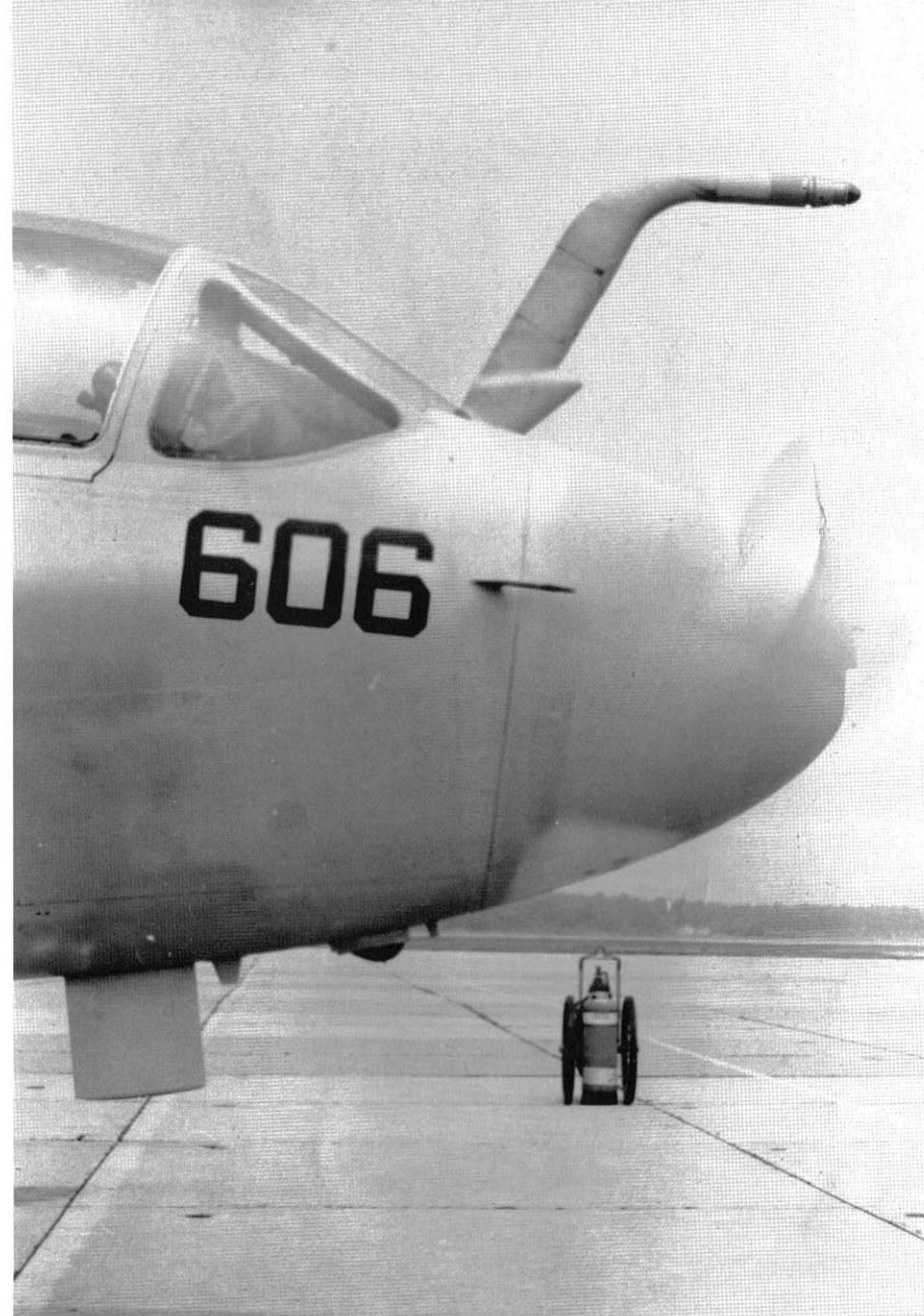
The EA-6B ICAP Prowler featured a modified refueling probe that housed an AN/ALQ 126 ECM antenna in the "sawtooth" housing at the base of the probe. The small object just in front of the side number is the starboard pitot tube and the bulge under the fuselage just behind the radome is the Red anti-collision light. (Author)
