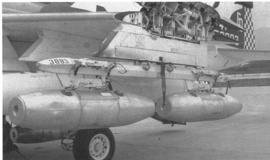
This Marine Corps A-6E is carrying a Multiple Ejector Rack (MER) with BLU-27 fire bombs on the center rack. The overall Natural Metal bombs have not been fitted with their nose caps and the rear fin assemblies. The fuel caps have Red seals. (T. Metler)
