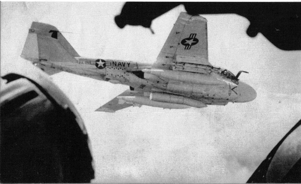
This A-6E of VA-85 is carrying a Ford Aerospace AN/AVQ-10 Pave Knife laser designator pod attached to the number 3 stores station (fuselage centerline pylon). Normally in this configuration, the Intruder would be acting as the designator aircraft for other Intruders armed with Laser Guided Bombs (LGBs). (Don Linn)
