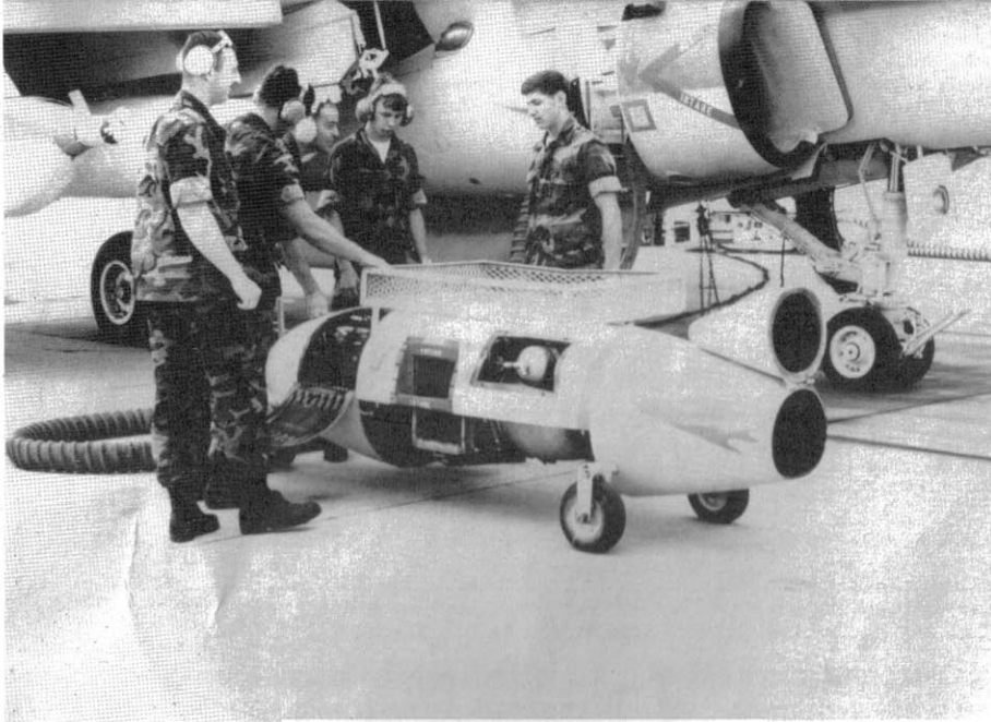
A group of Marine ground crewmen receive on-the-job-training (OJT) from an expert on the proper way to use a small start unit to start an EA-6B. The starter unit is overall Yellow with Red warning markings. The hose is attached to the Prowler in the starting receptacle which is located just to the rear of the boarding ladder. (Author)
