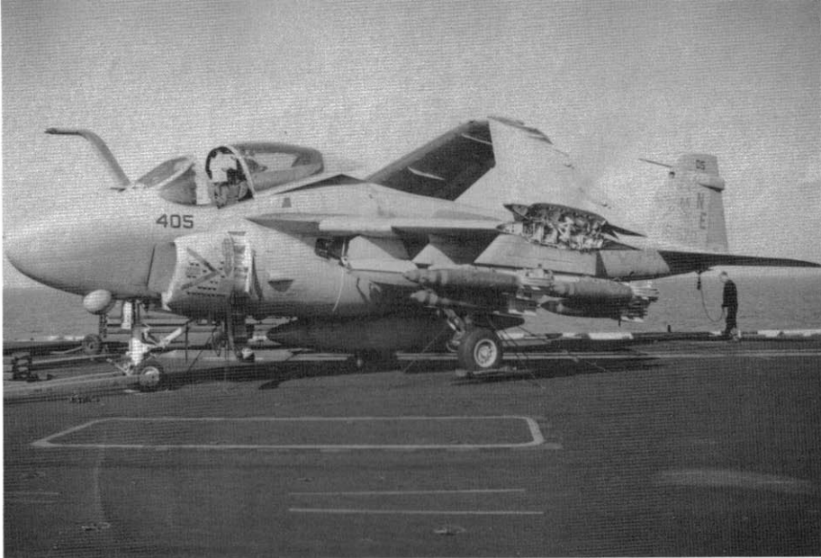
This A-6E TRAM of VA-155 aboard USS RANGER (CV-61) is armed with twelve Mk 82 500 pound low drag bombs. The aircraft carries twenty-two camel shaped mission markings on the engine nacelle in Black. (LT Doug Stevens via LT Richard Dann)
