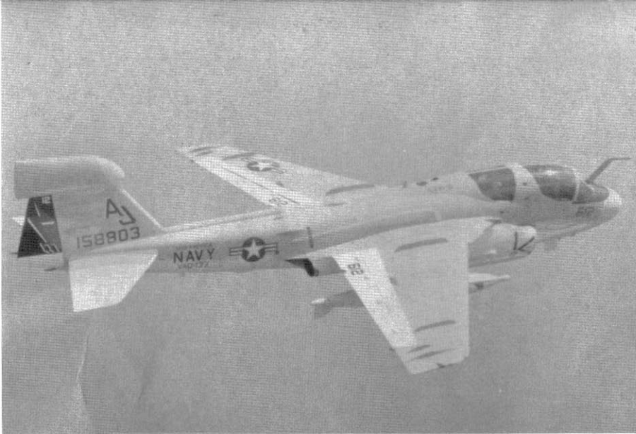
This VAQ-133 Wizards EA-6B EXCAP carries the standard Gloss Gull Gray and White scheme. The EA-6B has only two wing fences while the earlier EA-6A carried three fences. The fairings on the wingtip are the hinges and actuator for the wingtip speed brake. (Bruce Trombecky)
