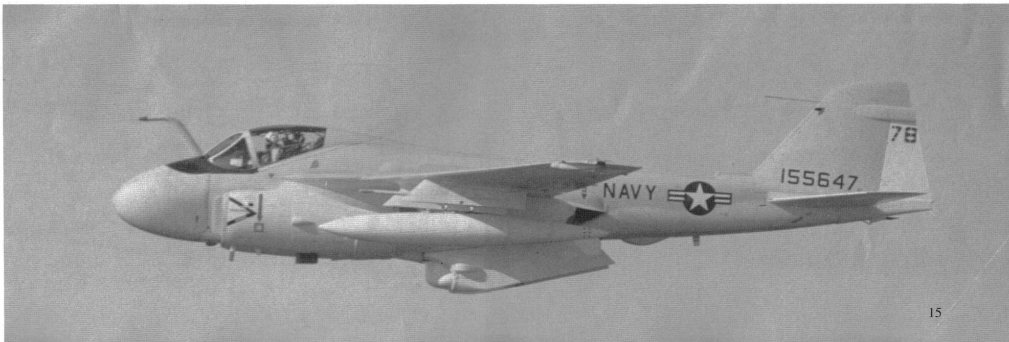
The first A-6C was converted from a standard production A-6A. The aircraft had the fuselage speed brakes faired over and had the ventral TRIM pod faired in to the underside of the fuselage. This particular aircraft was lost in combat on 8 January 1971 while assigned to VA-145 aboard USS RANGER (CVA-61). (Grumman)
