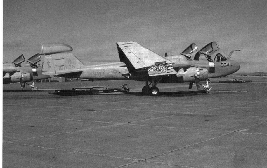
The first EA-6B ICAP II Prowler (BuNo 161776) on the ramp at Naval Air Station Whidbey Island NAS during August of 1985. The aircraft was assigned to VAQ-133 aboard the USS ENTERPRISE and carried the dull but highly effective tactical low visibility Gray paint scheme. (Bruce Trombecky)
