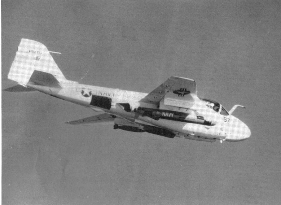
This A-6E of The Pacific Missile Test Center at NAS Point Mugu, California is carrying a Tomahawk cruise missile on the wing pylon and its guidance system electronics pod on the centerline station. The missile is a Reddish-Orange color with NAVY in White. The Intruder is also carrying a 1,000 pound bomb on the opposite wing as a counterweight. (USN)
