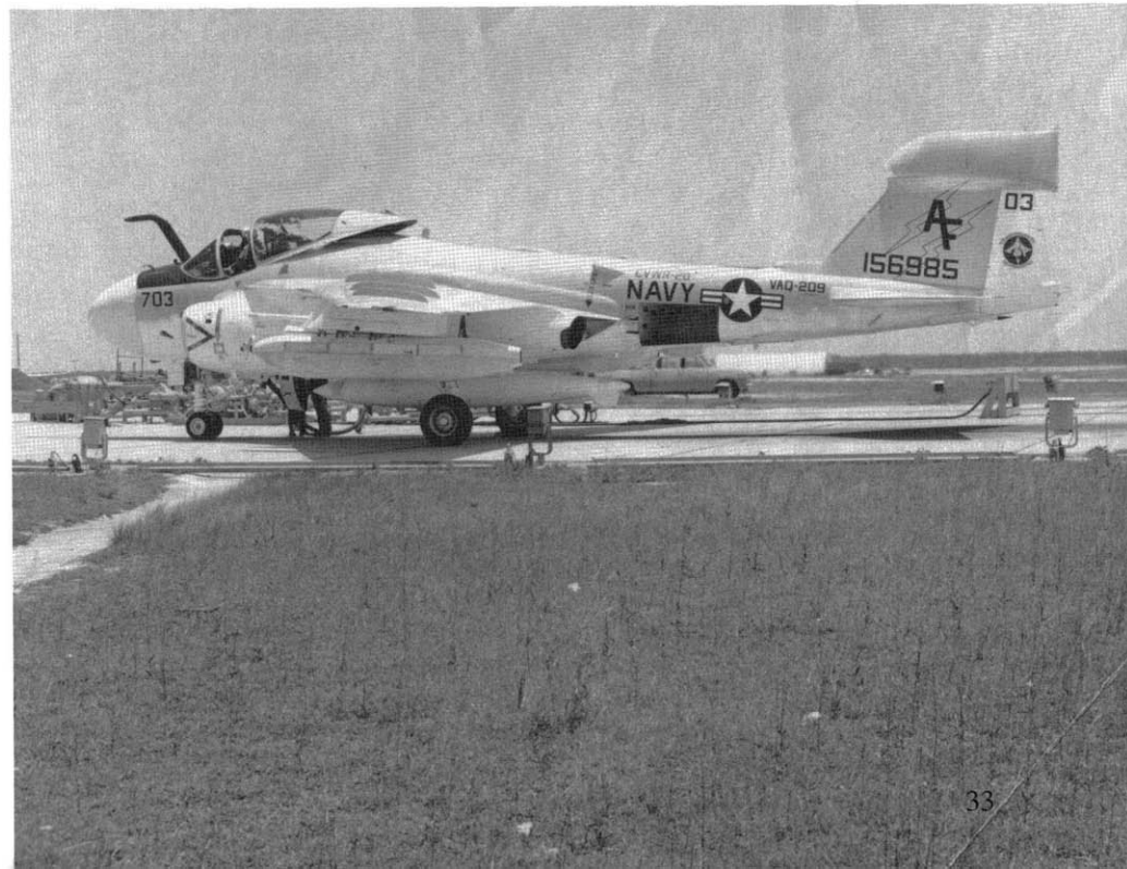
A (RECAP) EA-6A Intruder of VMAQ-4 on the ramp at NAS Cecil Field during February of 1989. The small "beer can" antenna fairing on the lower portion of the tail cap radome and the "sawtooth" at the base of the air refueling probe indicate that this aircraft has had the AN/ALQ 41 and AN/ALQ/100 ECM systems replaced by AN/ALQ 125 and 126B ECM systems. This aircraft also had the Doppler navigation radar system replaced (J. Tunney)
