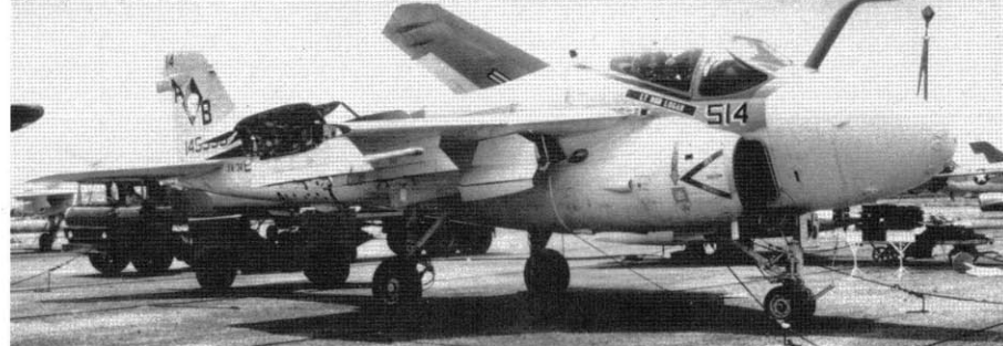
An A-6B TIAS-MOD 1 (BuNo 149955) Iron Hand Intruder of VA-34 Blue Blasters on the ramp at the NAS Norfolk, Virginia, Naval Air Rework Facility awaiting its turn to be reconfigured to A-6E standard as part of the Conversion in Lieu of Procurement (CILOP) program. (Author)
