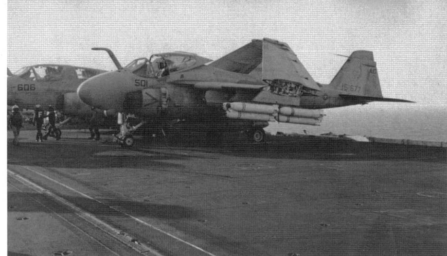
This A-6E TRAM of VA-34, parked on the deck edge of USS DWIGHT D. EISENHOWER (CVN-69) in the northern Red Sea on 18 August 1990, is armed with twelve Mk 24 Rockeye II cluster bombs, six on each outer wing pylon. (USN)
