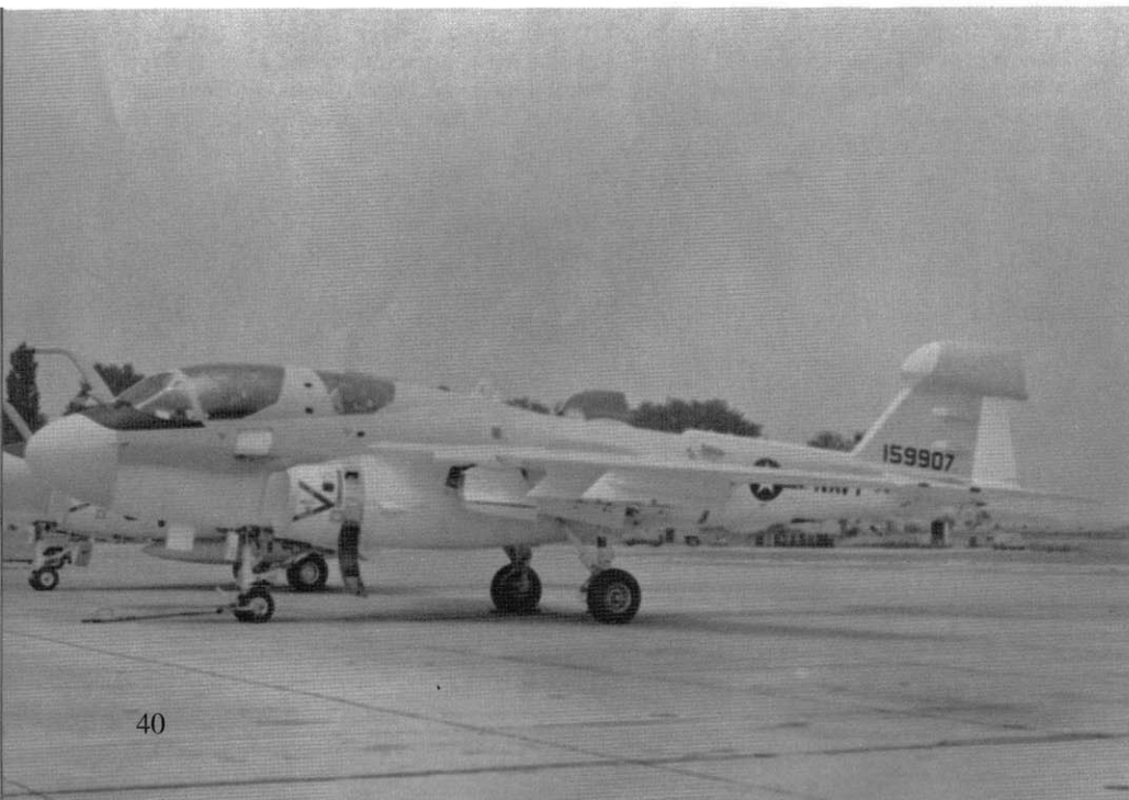
The EA-6B ICAP Prowler featured a modified refueling probe that housed an AN/ALQ 126 ECM antenna in the "sawtooth" housing at the base of the probe. The small object just in front of the side number is the starboard pitot tube and the bulge under the fuselage just behind the radome is the Red anti-collision light. (Author)
