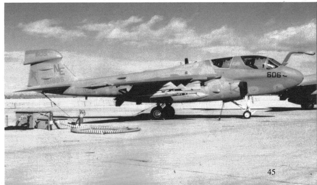
A VAQ-131 EA-6B ICAP II Prowler at Naval Air Station Fallon, home of the Navy's Strike school. This squadron had the distinction of being the first to operate the first four variants of the EA-6B. The aircraft is fitted with a Tactical Air Combat Training System (TACTS) pod on the outboard pylon. The pod is an overall Reddish Orange with a Black section just to the rear of the nose probe. (Bruce Trombecky)
