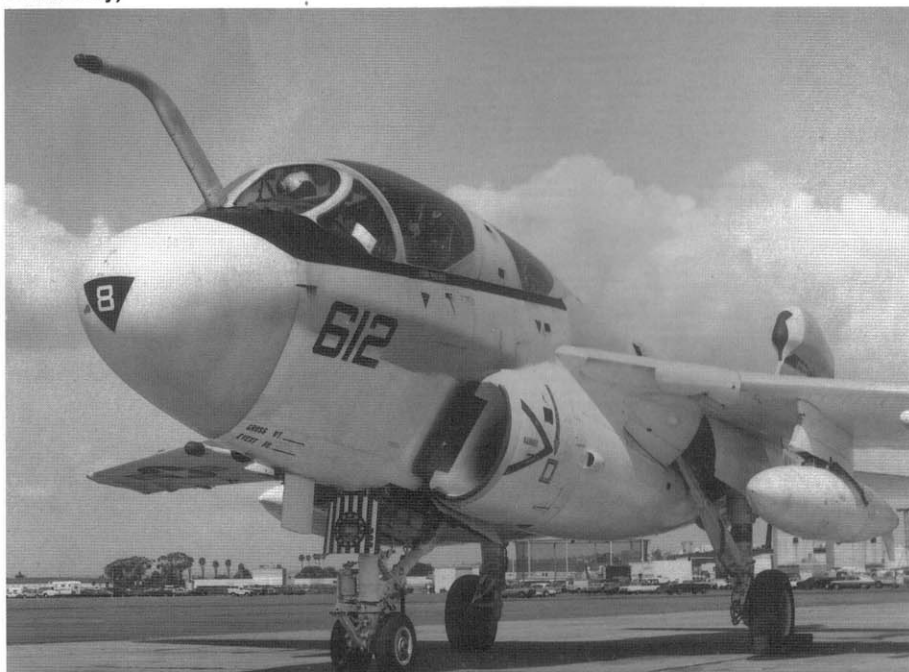
An EA-6B Standard (BuNo 158542) of VAQ-130 carries a Black triangle with a White number 8 in the center, identifying this Prowler as being assigned to Carrier Air Wing Eight. This marking on the center of the nose is used by the Landing Signal Officer (LSO) to help him distinguish the Prowlers from Intruders on final approach to the carrier. (Bruce Trombecky)
