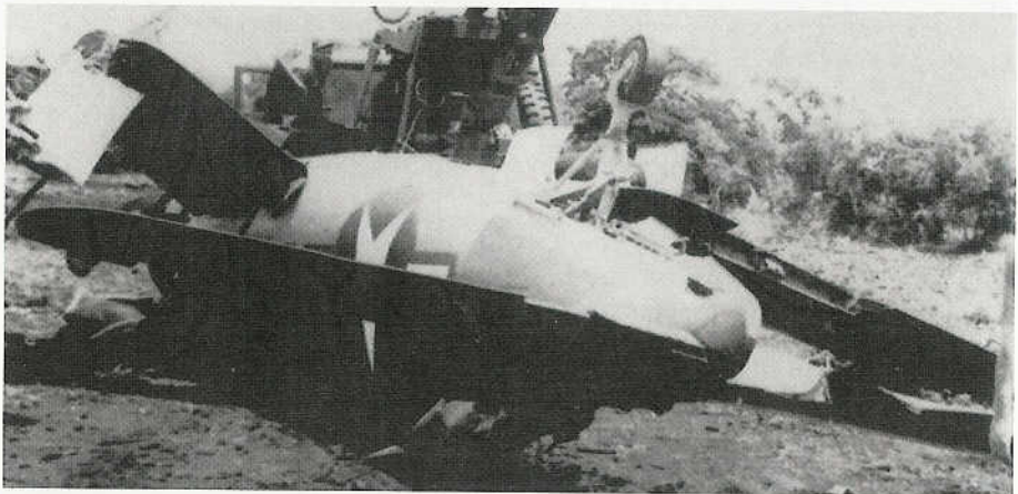
Returning from a night bombing raid on Japanese installations during August of 1944, Lieutenant Ed Sovik's F4U-2, side number 204, was hit by anti-aircraft fire and suffered hydraulic line damage. As Sovik attempted to land on Saipan only one main landing gear came down and, in the resulting crash landing, the Corsair came to rest on its back. The F4U-2 was destroyed but Sovik suffered only minor injuries. (W.F. Gemeinhardt Collection)
