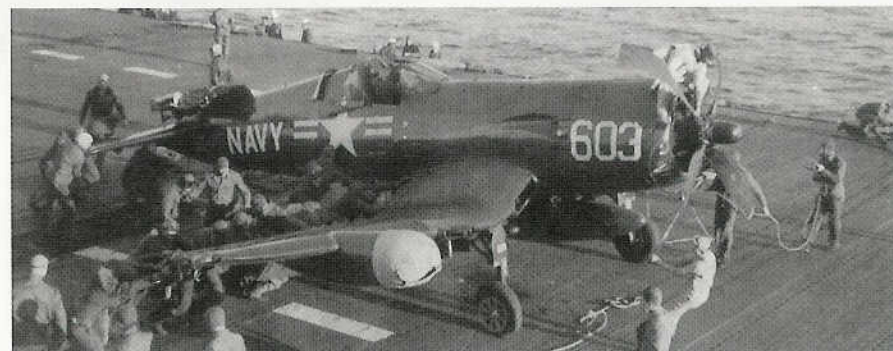
This F4U-5N (BuNo 124691) of VC-4 suffered extensive damage after engaging the barrier while coming aboard USS LEYTE off Korea on 3 November 1951. The Corsair had flipped over on its back, destroying the vertical fin. Deck crews are in the process of hoisting the aircraft back on its landing gear. (Robert Mathers)
