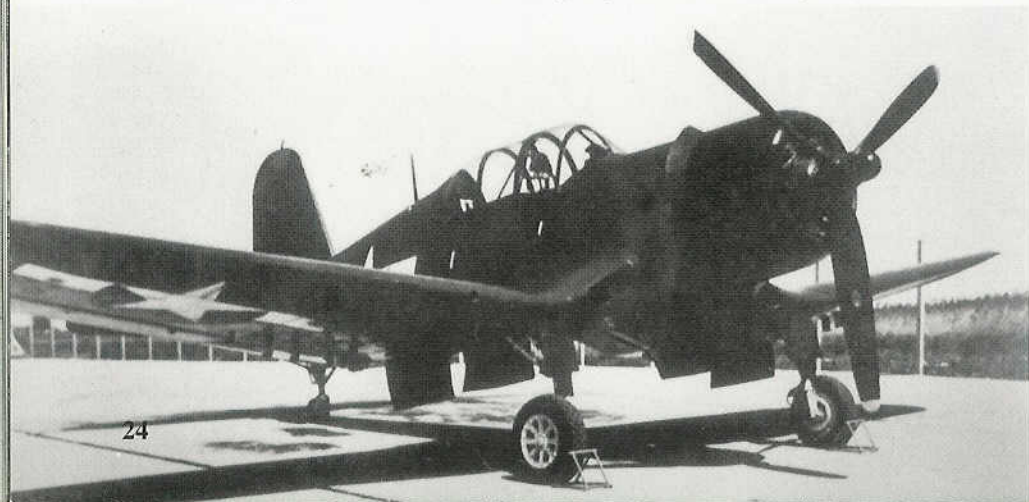
This F4U-1D Corsair airframe was modified by Vought to a two seat configuration during 1945. Arriving too late to be of any practical value to the war effort, the modification never went into production or service use. (Vought via Art Schoeni)
