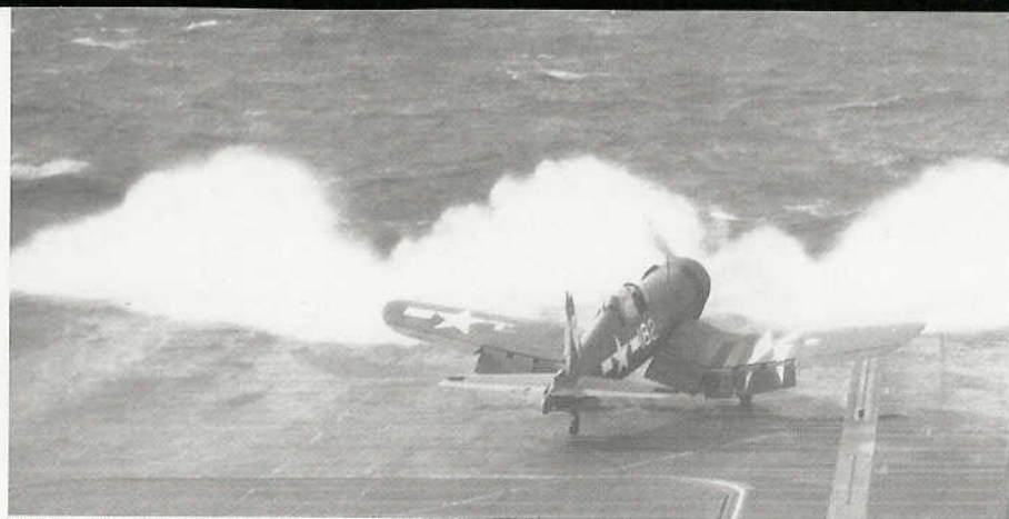
A F4U-1D, side number 182, of VBF-83 plows through heavy ocean spray while taking off from USS ESSEX during rough weather. The pilot was holding right rudder to counteract the torque of the 2,000 hp P&W R-2800-18W engine and successfully flew off the deck. (Paul Madden/USS ESSEX CV-9)
