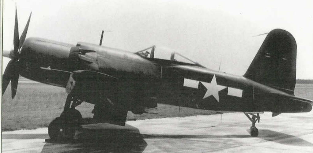
XF2G-1 (BuNo 14692) on the ramp at NATC Patuxent River, Maryland during flight testing. This Corsair variant had a top speed of 450 mph and was armed with six .50 caliber machine guns. The bubble style canopy on the XF2G-1 gave the best pilot visibility of all the variants. (National Archives via Hal Andrews)
