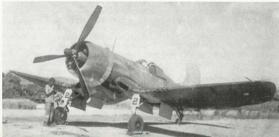
The F4U-1 was equipped with a thirteen foot Hamilton Standard three-blade propeller, the largest prop used on any Second World War fighter. This F4U-1 was assigned to VMF-124 on Guadalcanal during March of 1943. (Bob Esposito)
