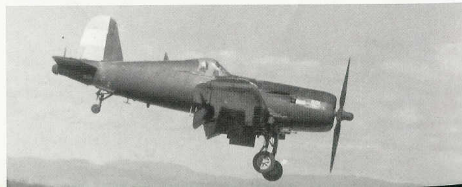
A F4U-5N, serial 601, of the Honduran Air Force on final approach for landing at Toncontin Airport, on 21 March 1976. The Corsair carried Medium Blue and White national markings on the tail with Blue/White stripes on the wingtips. The original starboard wing mounted radome and related night fighter equipment had been deleted. (F. Ariza via Carlos Planas)
