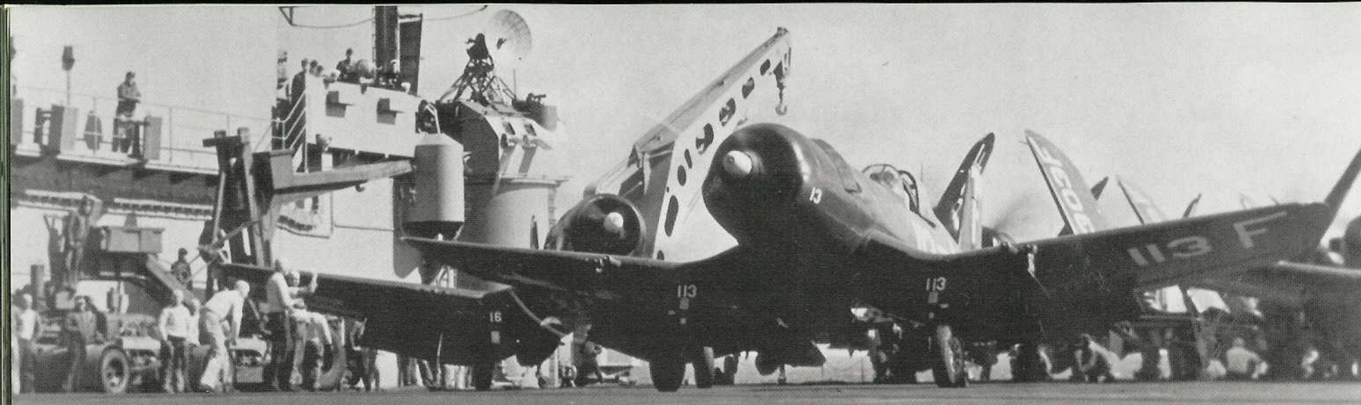
A F4U-5, side number 113, of VF-41 rolls down the flight deck of USS MIDWAY for a deck run takeoff. The propeller hub and tip of the fin was trimmed in White. The Pratt & Whitney R-2800-32W engine produced 2,300 hp and the F4U-5 could reach a top speed of 470 mph. (U.S. Navy)
