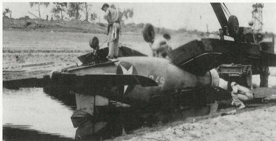
The F4U-1 was equipped with a thirteen foot Hamilton Standard three-blade propeller, the largest prop used on any Second World War fighter. This F4U-1 was assigned to VMF-124 on Guadalcanal during March of 1943. (Bob Esposito)
