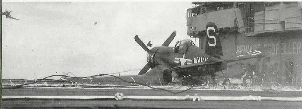
Shedding parts of Corsair and chewing up the flight deck with its thirteen foot propeller, this F4U-4B (BuNo 62952) of VF-53 Blue Knights came to a grinding stop beside the island of USS ESSEX ON 23 JULY 1951. The pilot was uninjured and the Corsair was later repaired and continued in the Korean air war. (U.S. Navy via Art Schoeni)
