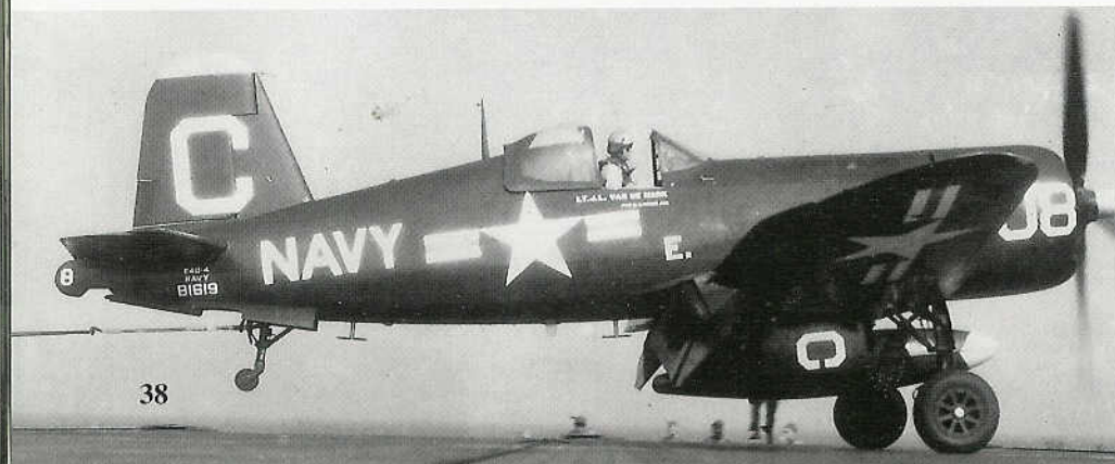
A F4U-4 (BuNo 81619) of VF-41 Black Aces catches a wire aboard USS MIDWAY during August of 1952 and comes to a sudden halt. This Corsair carried the battle efficiency "E" marking low on the fuselage beneath the cockpit. (Bob Esposito Collection)
