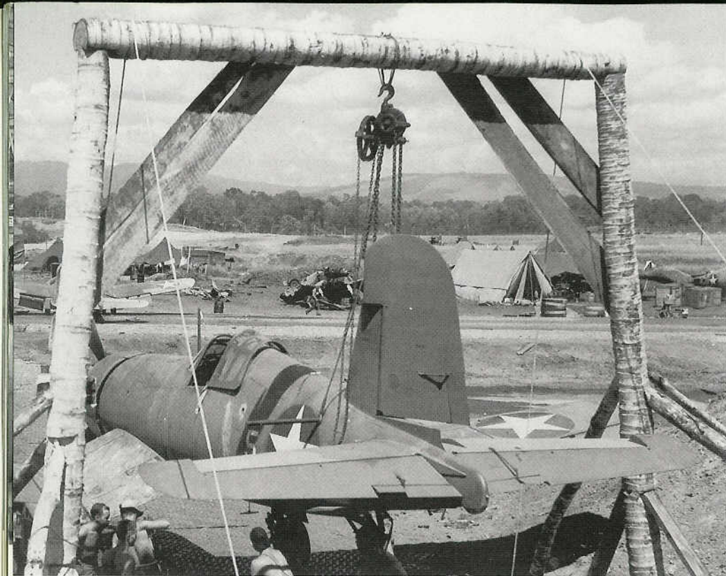
This Marine F4U-1 Corsair is having its six .50 caliber machine guns bore sighted on Guadalcanal during June of 1943. The lifting cradle was built of local coconut tree logs. The aircraft carried the side number five on the fuselage in White in front of the national insignia. (USMC)
