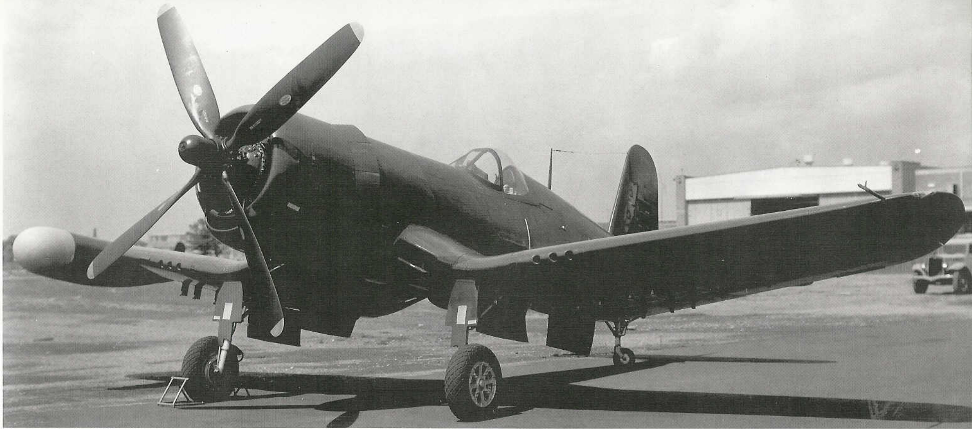
The one-of-a-kind F4U-4N (BuNo 97361) parked on the ramp at the Vought facility on 29 August 1946, was equipped with AN/APS-6 radar in a large radome mounted on the starboard wing. This night fighter was to be used for air-to-air night intercept missions. (Vought)
