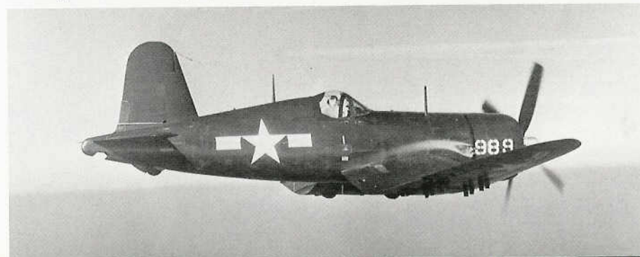
An F4U-4 (BuNo 80989) of AES-12 high over the Virginia countryside near Marine Corps Air Station Quantico, Virginia. The F4U-4 was powered by the Pratt & Whitney R-2800-18W engine and had a top speed of 414 mph. (Colonel Rhinehardt Lieu)
