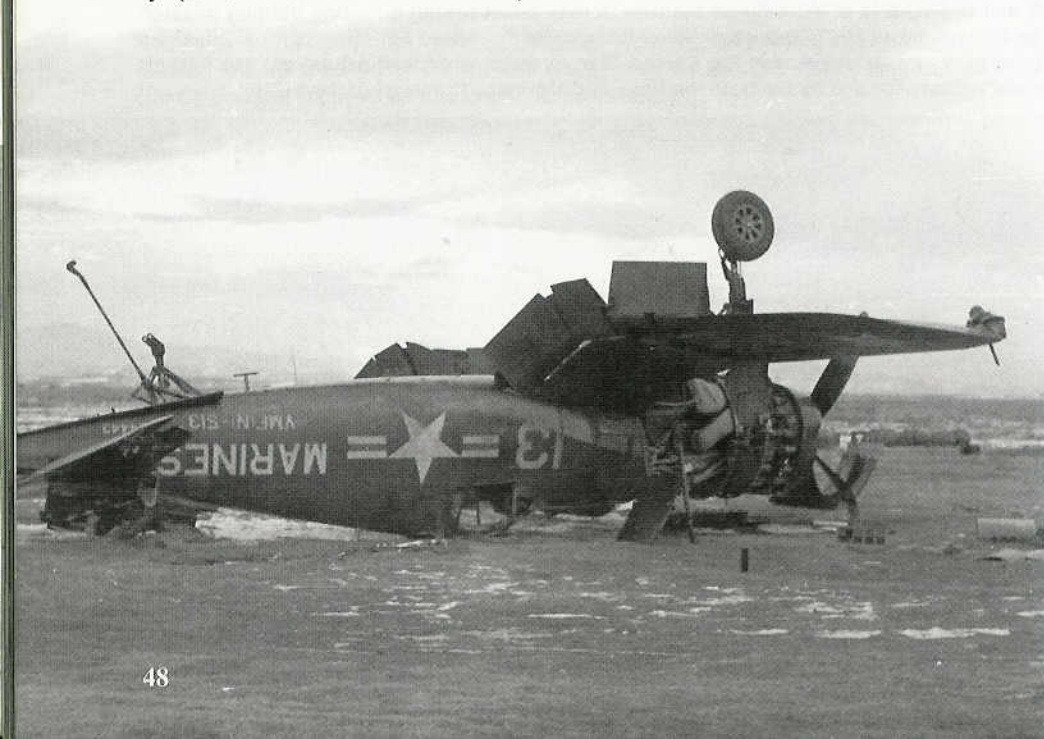
This F4U-5N (BuNo 124443) rested upside down at Kimpo Airfield (K-16), Korea after suffering strike damage when it nosed over on landing on 3 December 1950. The white markings on this Corsair have been muted by overspraying with Blue to lower its visibility. (LT J.A. Buebe via Robert F. Dorr)
