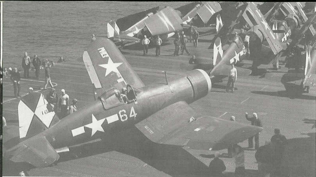
After landing, a F4U-1D of VBF-83 folds its wings and taxis forward to join other AG-83 Corsairs and Hellcats aboard USS ESSEX during the Spring of 1945. CV-9 was the first fast carrier to deploy the Corsair with three squadrons of F4U-1D/FG-1D aircraft assigned to VBF-83, VMF-124 and VMF-213. (Paul Madden/USS ESSEX CV-9)
