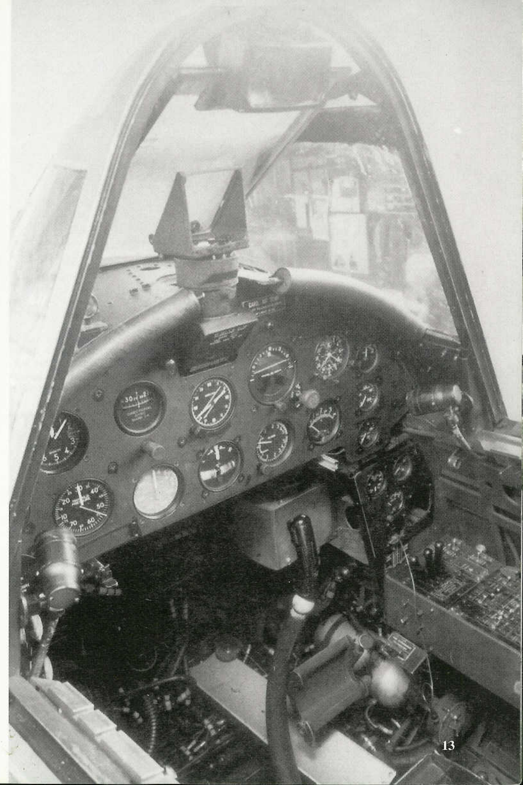
The F4U-1 port console showing cockpit controls, throttle, propeller controls, fuel mixture. The open area at left is the radio compartment. (Vought)
