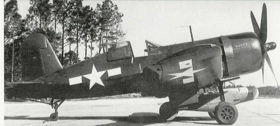
This F4U-4 (BuNo 80779) was equipped with a BAT missile on an underfuselage launch rail during October of 1946. The missile launch tests were successful; however, the missile never became operational with F4U squadrons. (U.S. Navy via Hal Andrews)
