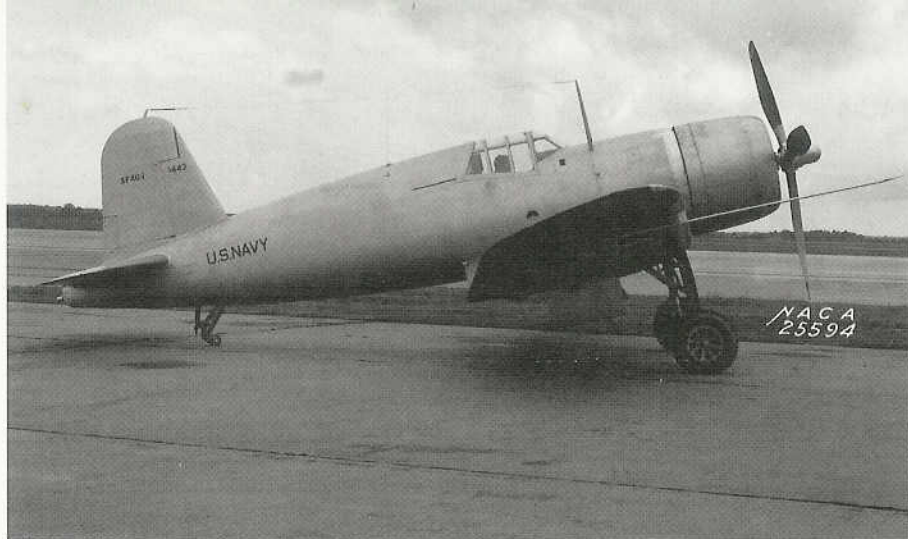
The XF4U (BuNo 1443) arrived at Langley Field, Virginia for drag reduction tests in the full scale thirty foot by sixty foot wind tunnel during the Fall of 1941. Testing was carried out by the National Advisory Committee for Aeronautics (NACA) the forerunner of today's National Aeronautics and Space Administration (NASA). (NASA via Mark Chambers)
