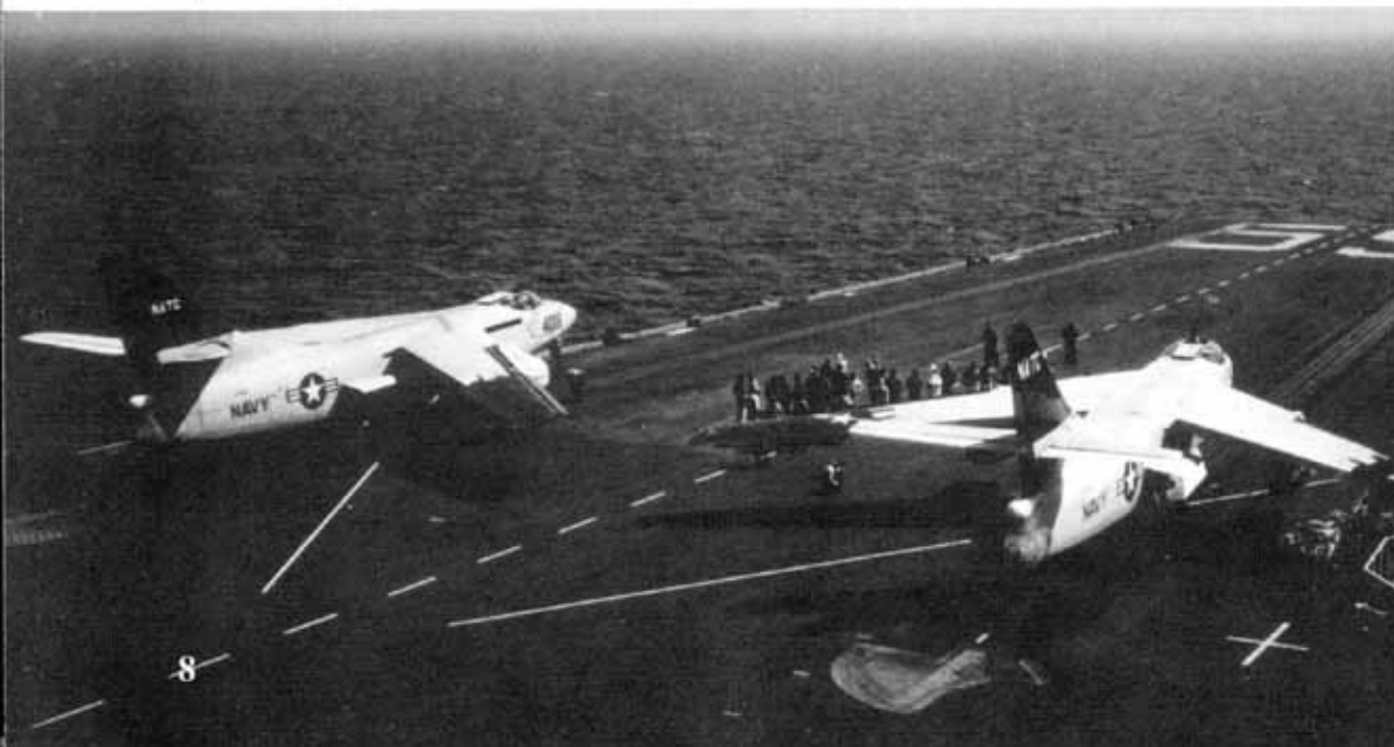
The Skywarrior had hydraulic folding outer wing panels and a folding vertical fin. These aircraft are assigned to the NATC for flight test and evaluation and both have the 20mm cannon turret installed. (Douglas via Jim Mesko)
