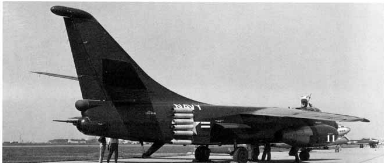
This A3D-1 (BuNo 130356) had JATO rockets installed on the fuselage stations and still had the twin 20MM tail cannon installed. The aircraft was on display during the Dayton, Ohio airshow on 7 October 1954. The aircraft also carried the early production fin mounted electronics antenna fairing. (Gordy via Pete Bowers)
