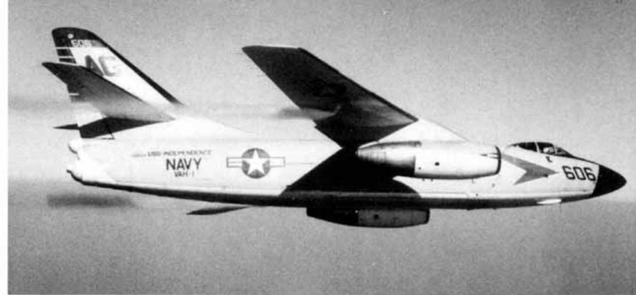
Dumping fuel from its underwing vents to get down to proper landing weight, this A3D-2 (BuNo 138933) of VAH-1 is preparing to land aboard USS INDEPENDENCE. This Skywarrior was assigned to Carrier Air Group Seven during 1961. (USN via Harold Andrews)
