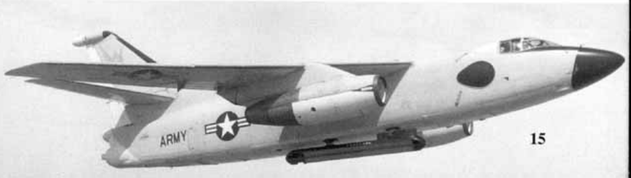
This A3D-1Q (BuNo 130361) was the third airframe converted to the electronic reconnaissance role. The Skywarrior was on loan to Westinghouse and the Army for testing their SLAR (Side Looking Airborne Radar) pod (similar to the one later installed on the OV-1 Mohawk) during 1966. (Dave Lucabaugh Collection)
