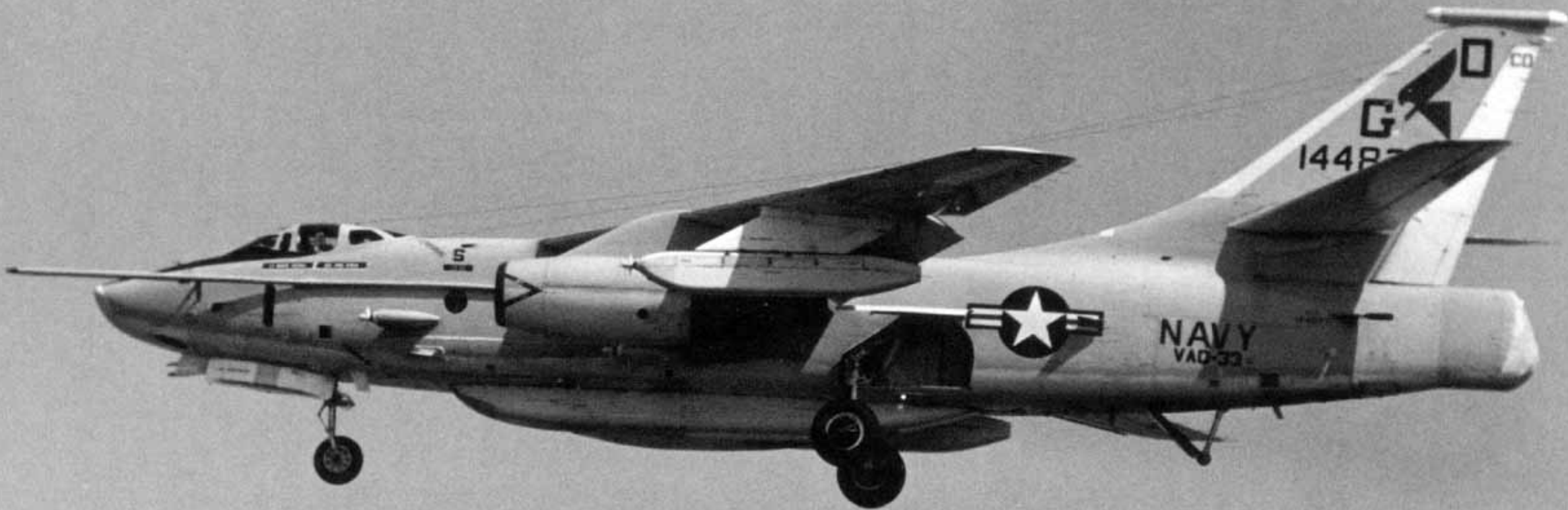
This ERA-3B (BuNo 144827) of VAQ-33 was lined up for final approach at NAS Oceana, Virginia, on 11 May 1978. The Skywarrior carried an ECM pod on its underwing pylon outboard of the engine nacelle. (Jim Sullivan)
