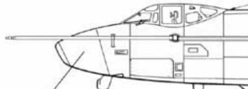
"Flat Nosed" Radome
