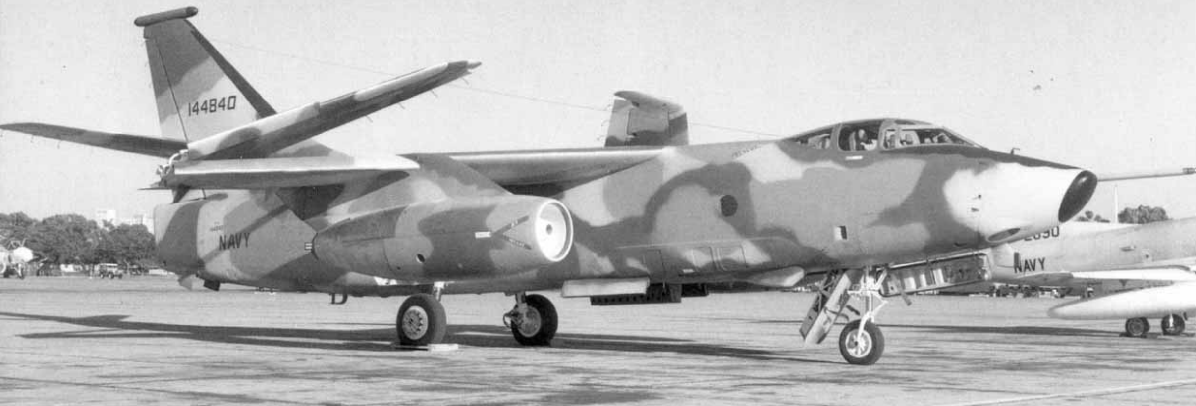
(Above) This RA-3B (BuNo 144840) Skywarrior of VAP-61 carried an unusual Gray and Blue camouflage for missions over North Vietnam. The aircraft was at NAS North Island, California on 26 November 1968. This Whale was modified in 1974 to become a NRA-3B and worked with missile systems and special programs. (Clay Jansson)
