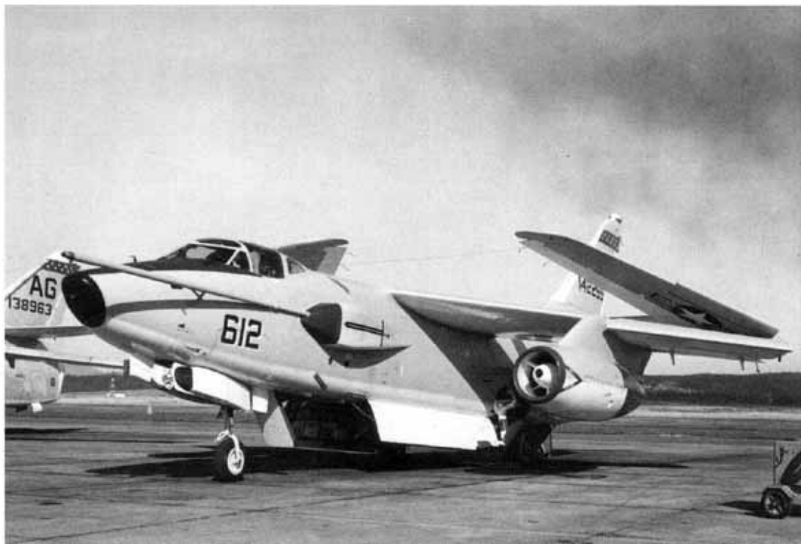
An EKA-3B (BuNo 142255) of VAH-130 on the ramp at its home station, NAS Whidbey Island, Washington during 1967. The fairing on the nosewheel door housed an ECM antenna. (USN via Thomas Gates)
