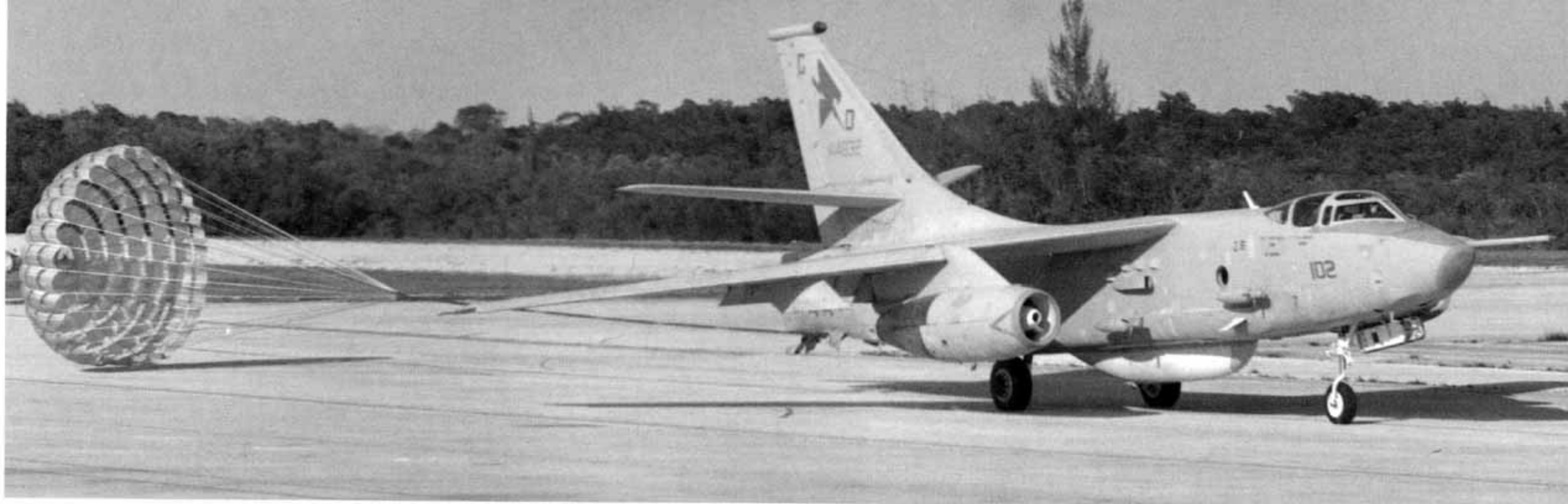
This ERA-3B (BuNo 144832) of VAQ-33 carries a low-vis overall Gray paint scheme. This version of the Whale represented the ultimate modification of the 1959 vintage airframe. Its twenty-four foot drag chute billowing out behind it, this Skywarrior was one of the last few still flying in April of 1991 and was soon retired from service. (Don Spring/A.I.R.)
