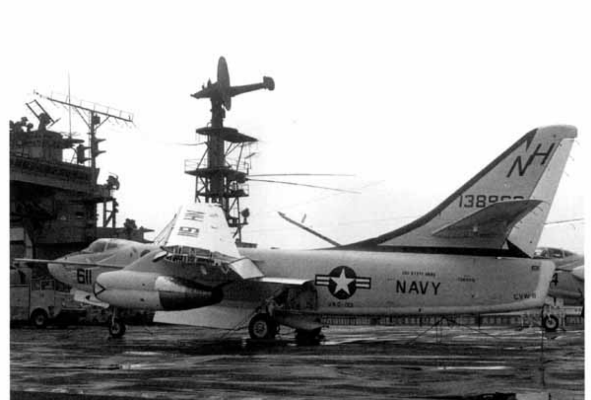
A KA-3B (BuNo 138966) of VAQ-133 on the flight deck of USS KITTY HAWK pier side at NAS North Island, California on 3 October 1970. The squadron was attached to Carrier Air Wing Eleven. The squadron modex and aircraft number were carried on the underside of the port wing and the trim on the fin was in Red. (Clay Jansson)
