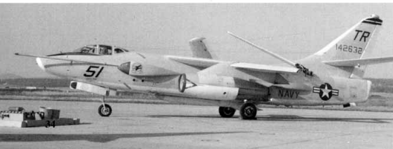
A Black Ravens EKA-3B (BuNo 142632) on the ramp at NAS Whidbey Island, Washington during 1969. Skywarriors of VAQ-135 carried the "TR" modex on the fin. The large fuselage blisters housed ECM equipment and were unique to the EKA-3B. (Pete Bowers)
