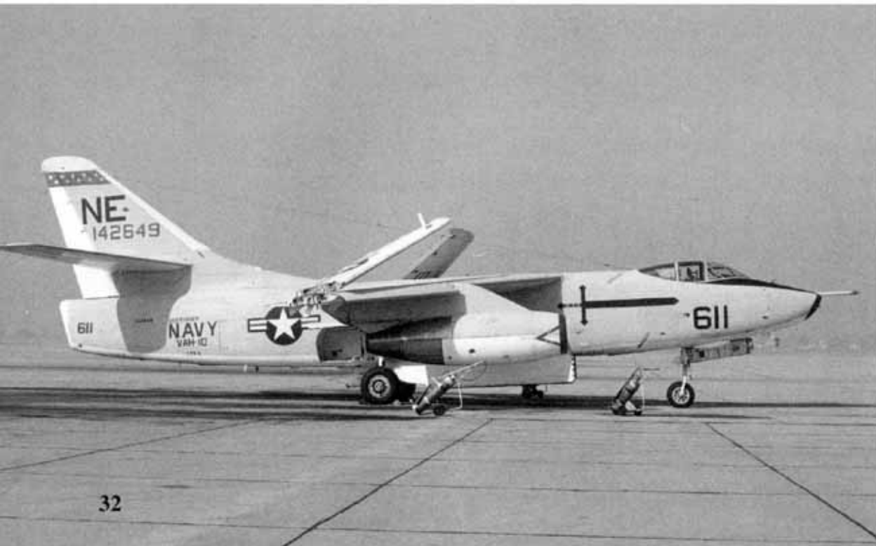
This KA-3B (BuNo 142649) of VAH-10 was assigned to USS RANGER when not ashore at NAS North Island, California. The bomb bay doors on the Skywarrior tanker could only be opened while the Whale was on the ground. The stylized Viking sword was displayed on both sides of the fuselage. (Clay Jansson)
