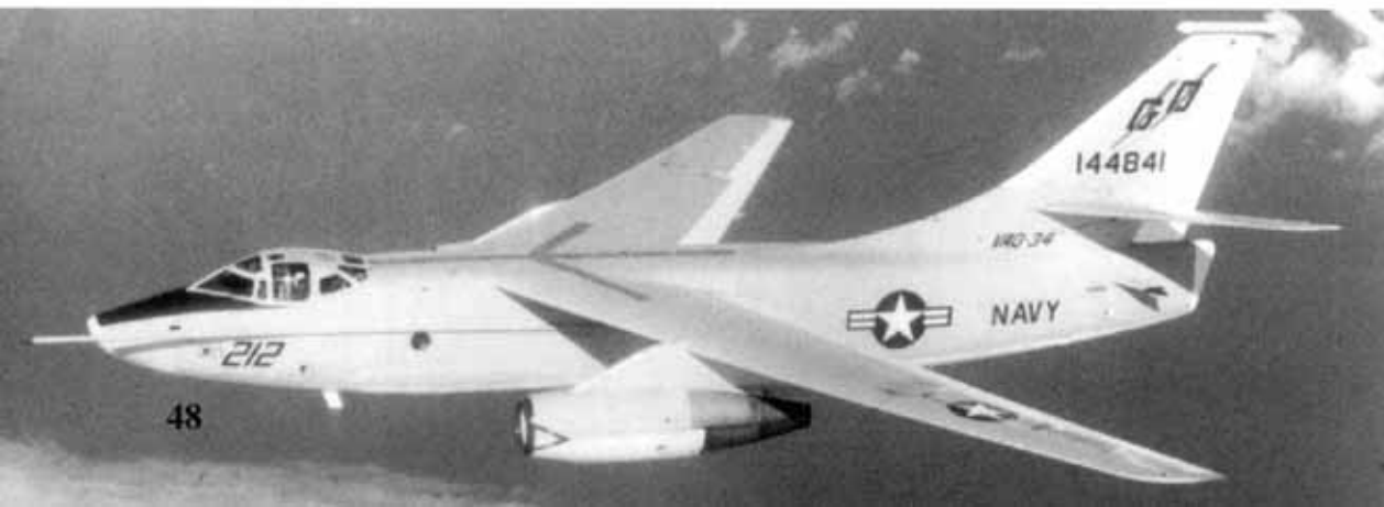
An ERA-3B (BuNo 144841) of VAQ-34 in flight over the Pacific off the California coast during October of 1983. This Skywarrior had the earlier dove-tail faring installation, but has chaff dispensers on the fuselage sides. GD-212 was flying from NAS Miramar, California. (Bruce Trombecky)
