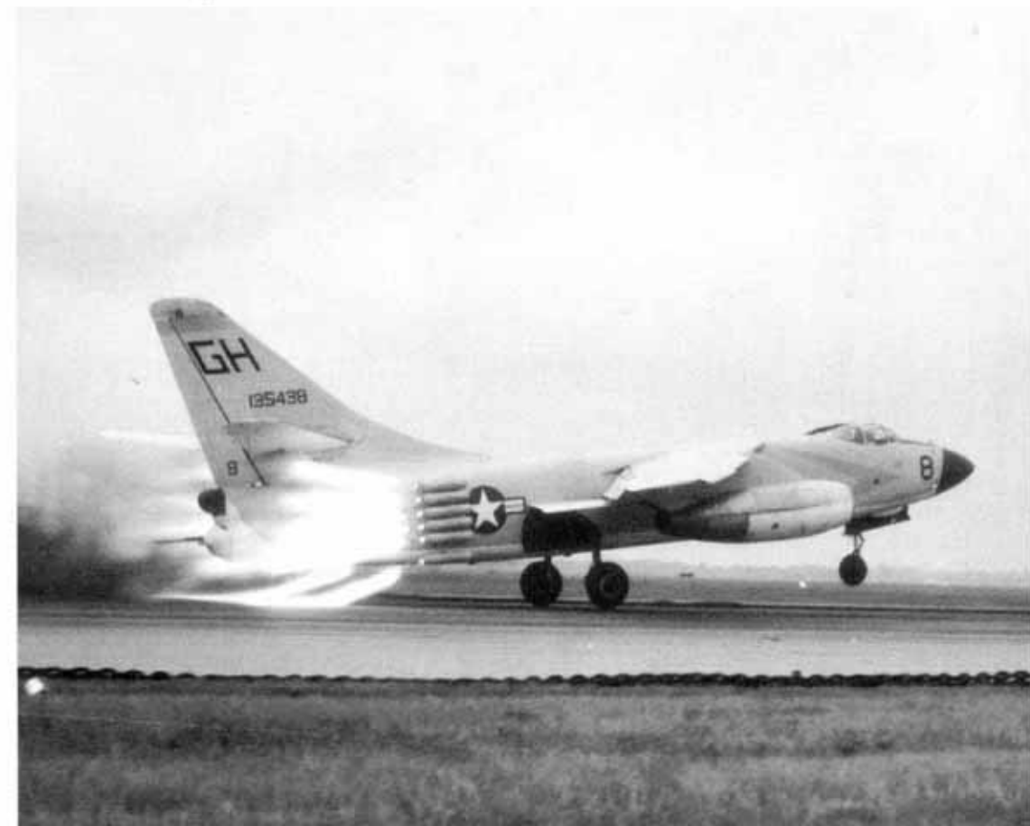
This A3D-1 (BuNo 135438) of VAH-1 used twelve JATO bottles to dramatically shorten its take off run from NAS Jacksonville during 1957. With JATO assistance, the thirty-five ton bomber could lift off in four seconds in less than the length of a football field. (USN via Harold Andrews)
