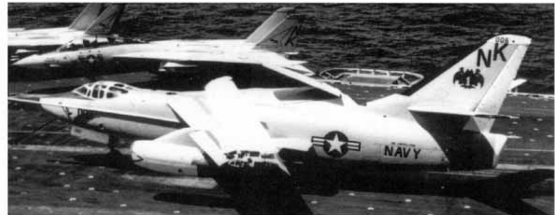
Having recovered safely aboard the USS KITTY HAWK during operations in the South China Sea in 1973, this EA-3B, side number 7, of VQ-1 folded its wings and headed for the deck edge elevator. (Lionel Paul)
