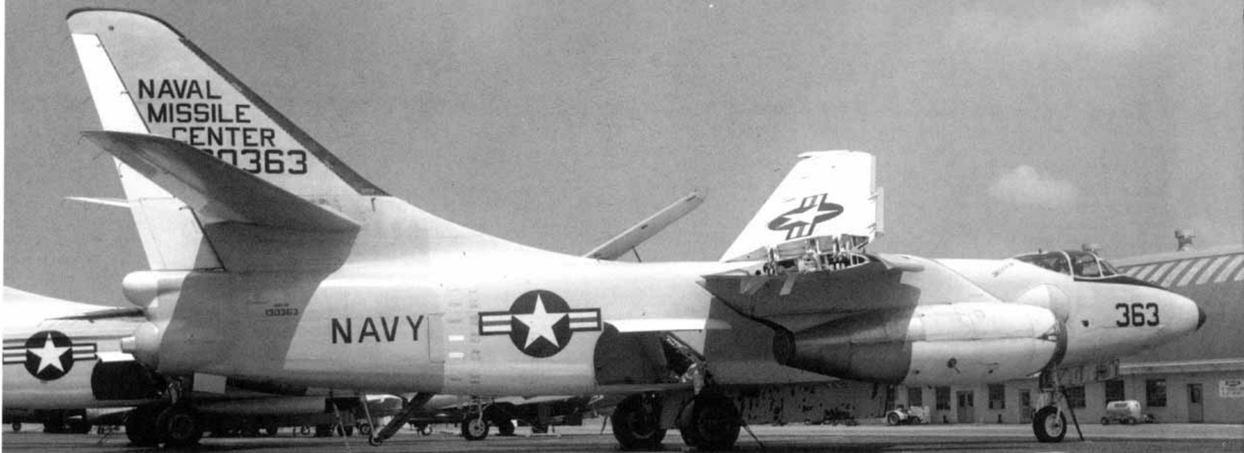
This A3D-1Q (BuNo 130363) was the last of a batch of five standard bombers converted to the electronic reconnaissance role. This Skywarrior, parked on the ramp at the Naval Missile Center, Point Mugu, California on 19 May 1962, carried a crew of seven, adding four ECM operators to the standard flight crew. The tear drop shaped fuselage blister below and to the rear of the cockpit helped identify the A3D-1Q. (Doug Olson via Clay Jansson)
