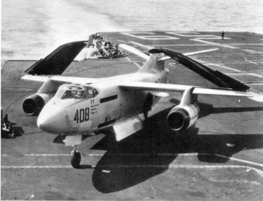
This A3D-1 is being positioned on the deck edge elevator for a trip down to the hangar deck aboard USS FORRESTAL on 5 April 1956. This A3D-1 Skywarrior was the thirteenth aircraft off the production line. (USN via Jim Mesko)
