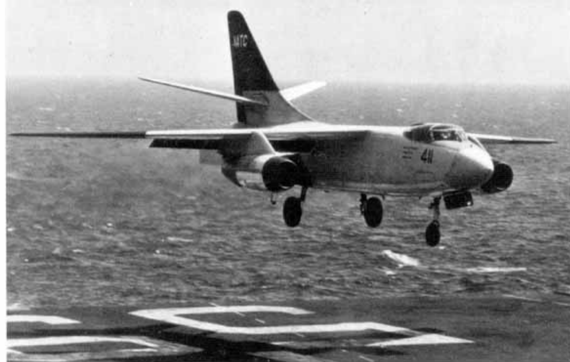
An A3D-1 comes over the ramp aboard USS FORRESTAL during the carrier suitability trials on 4 April 1956. The A3D was sometimes referred to as the "Aluminum Overcast" because it was the largest aircraft aboard the carrier. (Douglas via Jim Mesko)
