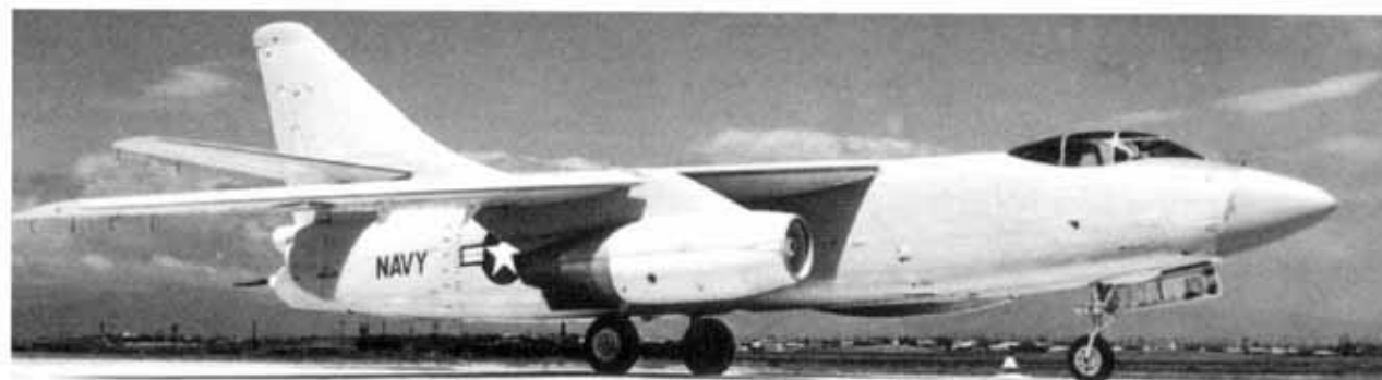
This A3D-1 (BuNo 130356) had JATO rockets installed on the fuselage stations and still had the twin 20MM tail cannon installed. The aircraft was on display during the Dayton, Ohio airshow on 7 October 1954. The aircraft also carried the early production fin mounted electronics antenna fairing. (Gordy via Pete Bowers)
