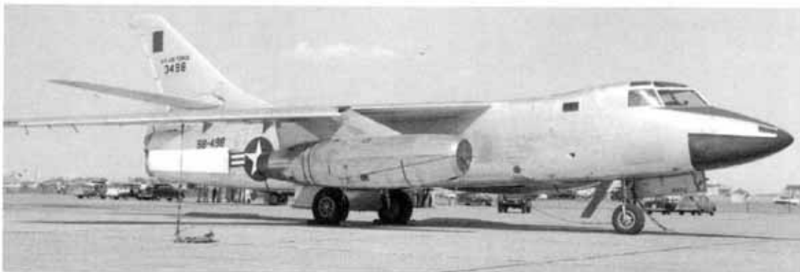
(Above and below) Douglas produced a close cousin to the Navy Skywarrior for the USAF under the designation B-66 Destroyer. There were 294 Destroyers manufactured and externally they strongly resembled the big Navy jet. The B-66 served several roles with the Air Force from 1953 to 1974 when they were retired. (Peter Bowers Collection)
