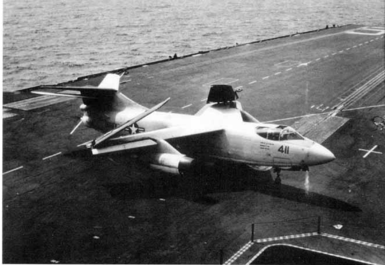
A Flight Test A3D-1 moves toward the forward deck edge elevator aboard USS FORRESTAL during the aircraft's carrier suitability trials. To fit on the hangar deck, the wings and fin had to be folded. (USN via Harry Andrews)
