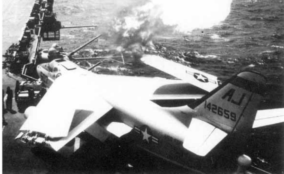
This A3D-2 (BuNo 142659) of VAH-5 Savage Sons (based at NAS Sanford) was spotted just forward of the island during a gunnery exercise aboard USS FORRESTAL in the Spring of 1962. The aircraft's folding wings saved precious deck space. (USN via Fred Carment)
