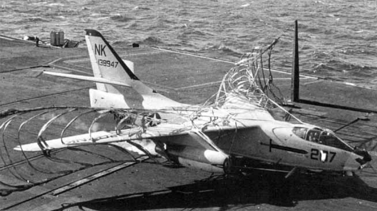
This A-3B (BuNo 138947) of VAH-10 came to a halt after engaging the barrier aboard the USS CONSTELLATION ON 6 August 1962. This Skywarrior suffered minimum damage and was quickly returned to flying status. Unfortunately, it was lost three years later during an operational accident in Tonkin Gulf. (USN via Peter Mersky)
