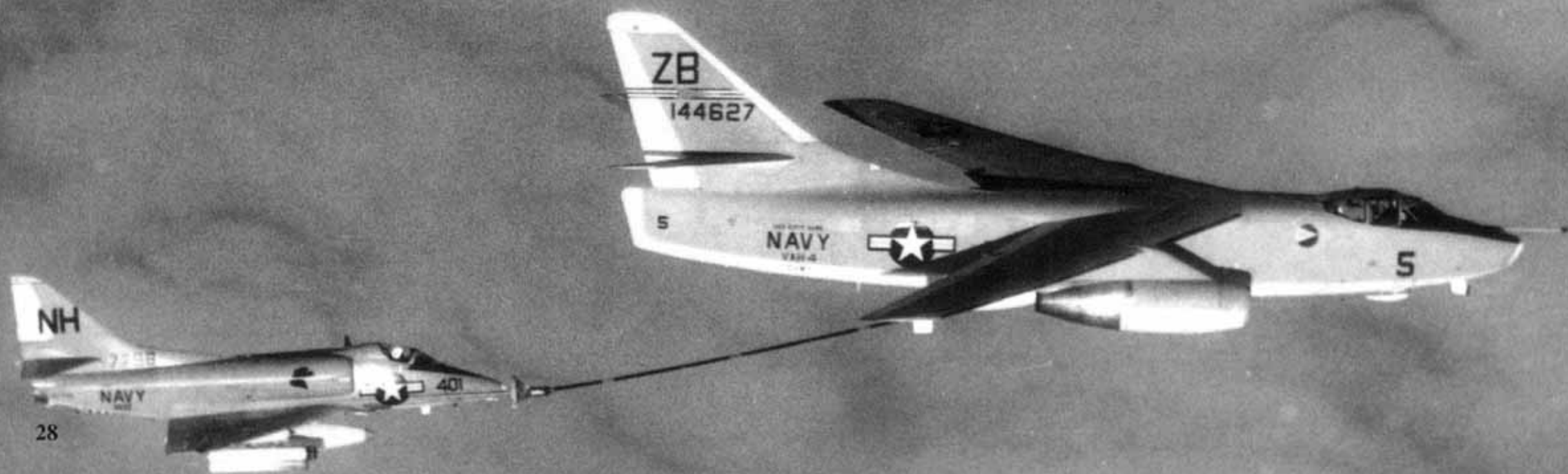
A KA-3B (BuNo 144627) of VAH-4 refuels an A-4C (BuNo 147798) Skyhawk of VA-113. Heavily loaded with ordnance, attack aircraft often departed the carrier with minimum fuel and once airborne they hooked up with a tanker, refueled and headed for the target. Both jets were from Carrier Air Wing Eleven aboard the USS KITTY HAWK during 1967. (Lionel Paul)
