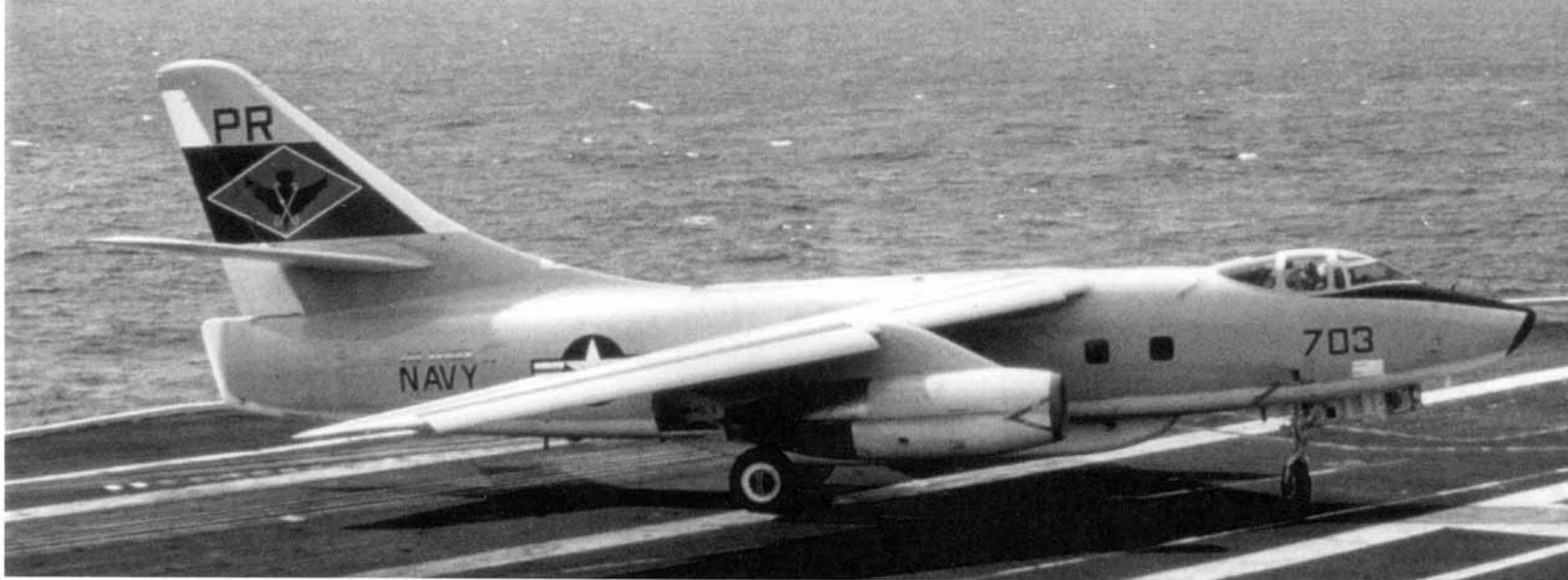
An EA-3B of VQ-1 heads toward the deck edge elevator after trapping aboard the USS RANGER during November of 1974. This version of the Whale was used for ECM/reconnaissance missions and carried a crew of seven. (Bruce Trombecky)
