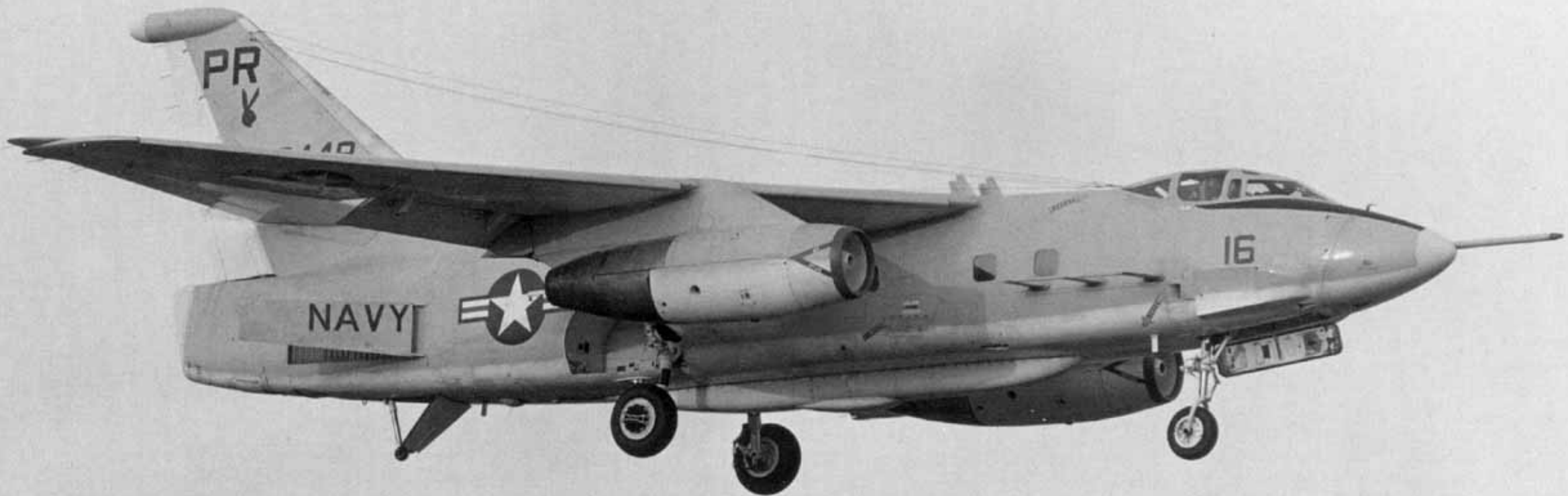
An EA-3B (BuNo 146449) of VQ-1 displayed "the rapid-rabbit" Playboy bunny insignia on its vertical fin during July of 1974. The aircraft was on final approach for landing at NAF Atsugi, Japan. This Skywarrior was equipped with an array of three blade antennas low on the forward fuselage side and the speed brakes were extended. (Hideki Nagakubo)
