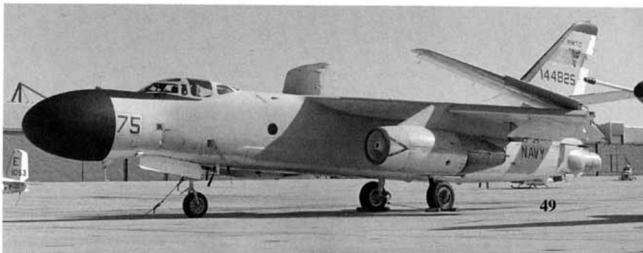
This NRA-3B (BuNo 144825) on the ramp at NAF Washington, DC on 6 November 1982, was a one-of-a-kind modification. This large nose radome was installed by Grumman for use in testing missile systems. More non-standard modifications were installed on the aft end of the fuselage. (Don Linn)
