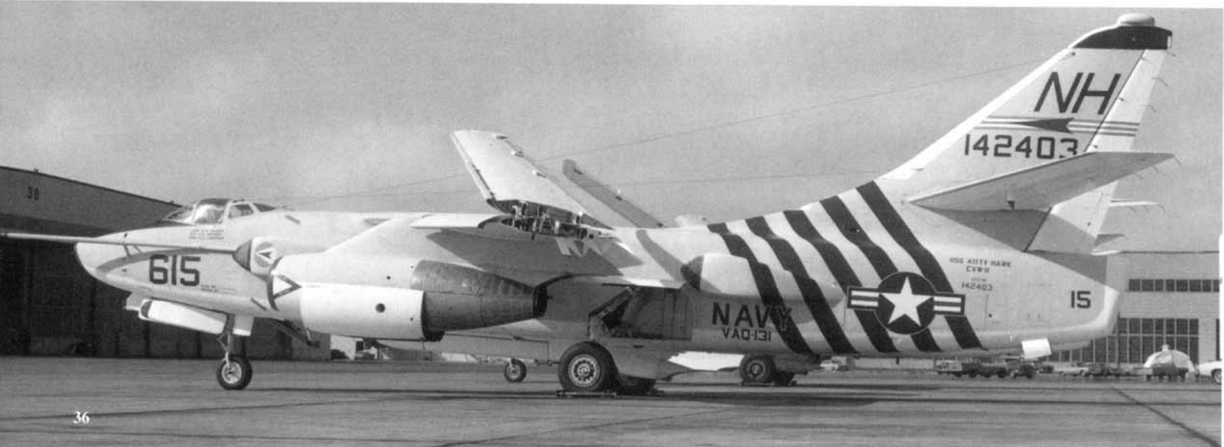
This EKA-3B (142403) of VAQ-131 had just returned to NAS Alameda, California on 13 September 1969 after seeing action in Vietnam as part of Carrier Air Wing Eleven aboard USS KITTY HAWK. The Lancers squadron emblem was displayed forward on the ECM blister beneath the cockpit. The port engine nacelle lower access panels were partially open. (Clay Jansson)
