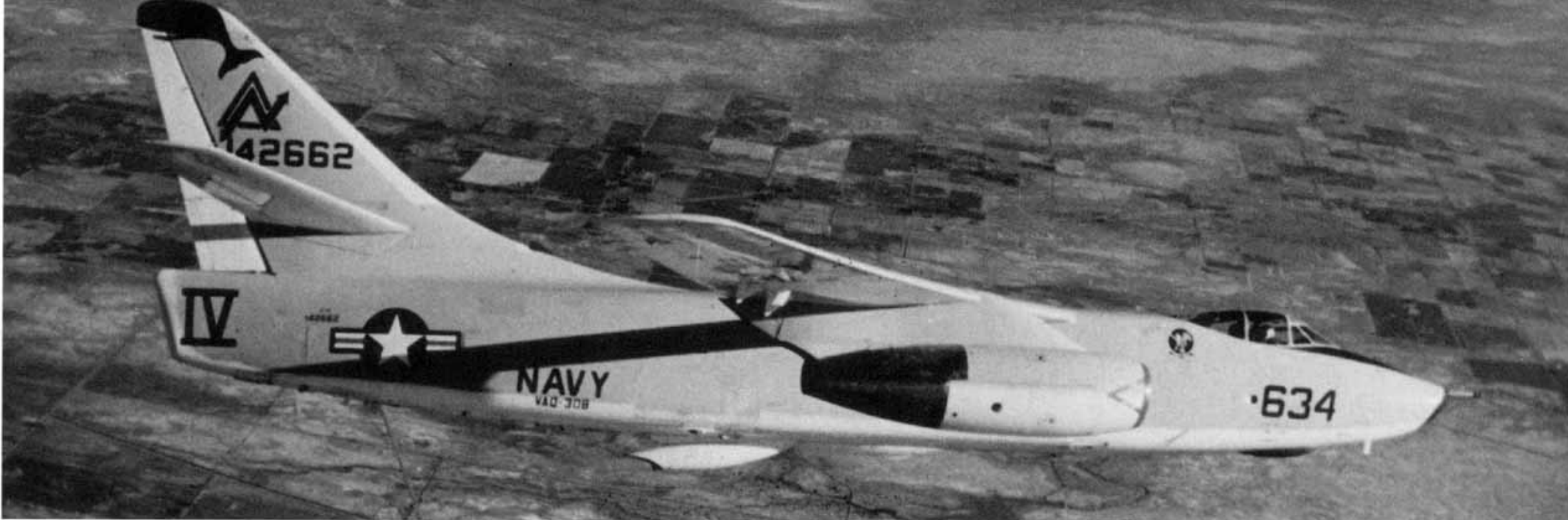
Tanker Four, a KA-3B (BuNo 142662) of VAQ-308, begins its letdown over the California countryside during 1978, while enroute to its home base at NAS Alameda, California. The national insignia was carried well to the rear on the fuselage side, followed by the large Roman numeral IV. This marking was carried to make the tanker highly visible. (USN via Peter Mersky)
