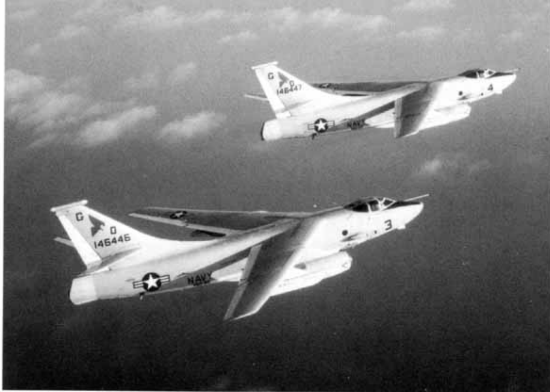
A pair of ERA-3Bs (BuNos 146446 and 146447) of VAQ-33 Firebirds fly high over the Pacific off the California coast during May of 1983. Both Skywarriors were equipped with a chaff-dispensing installation in the elongated tail section. The flight originated at NAS Miramar, California. (Bruce Trombecky)
