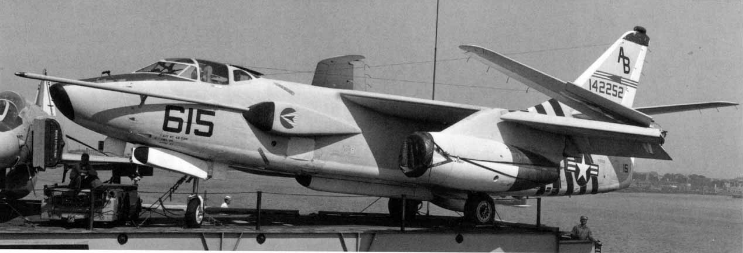
This EKA-3B (142403) of VAQ-131 had just returned to NAS Alameda, California on 13 September 1969 after seeing action in Vietnam as part of Carrier Air Wing Eleven aboard USS KITTY HAWK. The Lancers squadron emblem was displayed forward on the ECM blister beneath the cockpit. The port engine nacelle lower access panels were partially open. (Clay Jansson)
