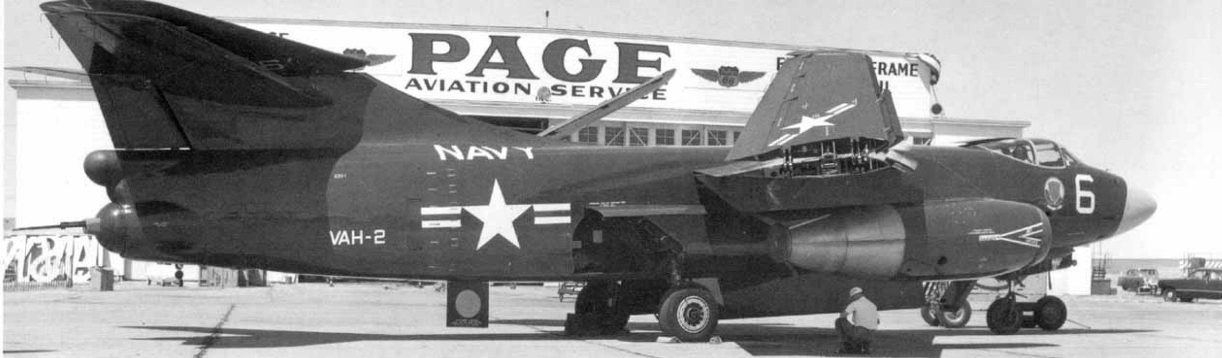
An overall Glossy Sea Blue Heavy Two (VAH-2), Royal Rampants, A3D-1 Skywarrior parked on the ramp with its wings and tail folded during 1956. The aircraft still had the 20MM tail-mounted cannon in place. All lettering was in White and the nose radome was left unpainted. (Pete Bowers)
