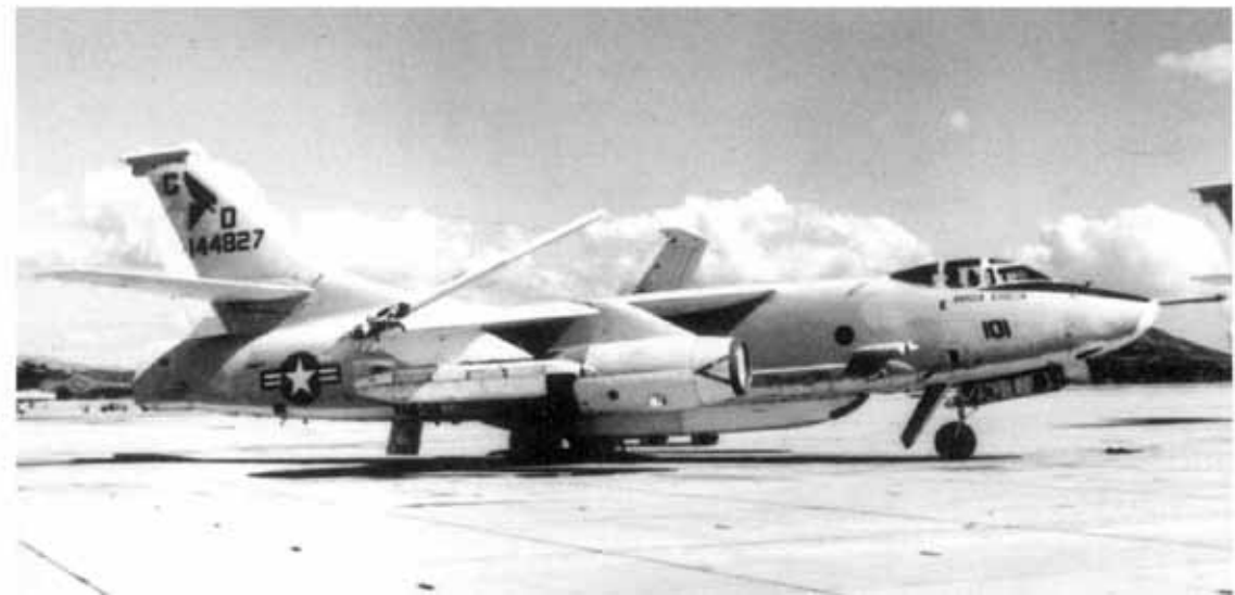
An ERA-3B (BuNo 144827) of VAQ-33 on the flight line at NAS Miramar, California during October of 1983. This Skywarrior carried a yellow "Pacman" design on the flat nose radome. The RAT (Ram Air Turbine) installation was low on the fuselage beneath the circular window. (Bruce Trombecky)
