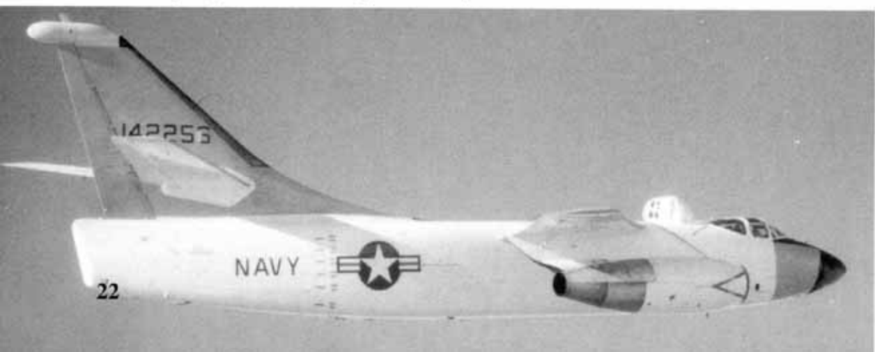
Highly modified and redesignated as a NA-3B, this Skywarrior (BuNo 142256) was bailed to Westinghouse for research work tracking re-entry vehicles during February of 1964. Special optical equipment was installed in the made-to-fit B-50 turret located just behind the cockpit. (Bruce Trombecky Collection)
