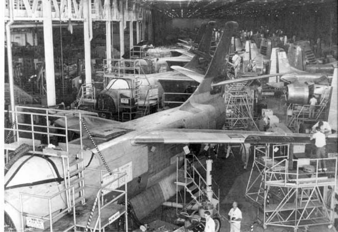
A3D-1 Skywarriors on the final assembly line at the Douglas El Segundo factory during 1955. These very early production A3D-1s had the fin cap antenna fairing. The aircraft in the background are AD-5W Skyraiders. (Douglas via Harry Gann)
