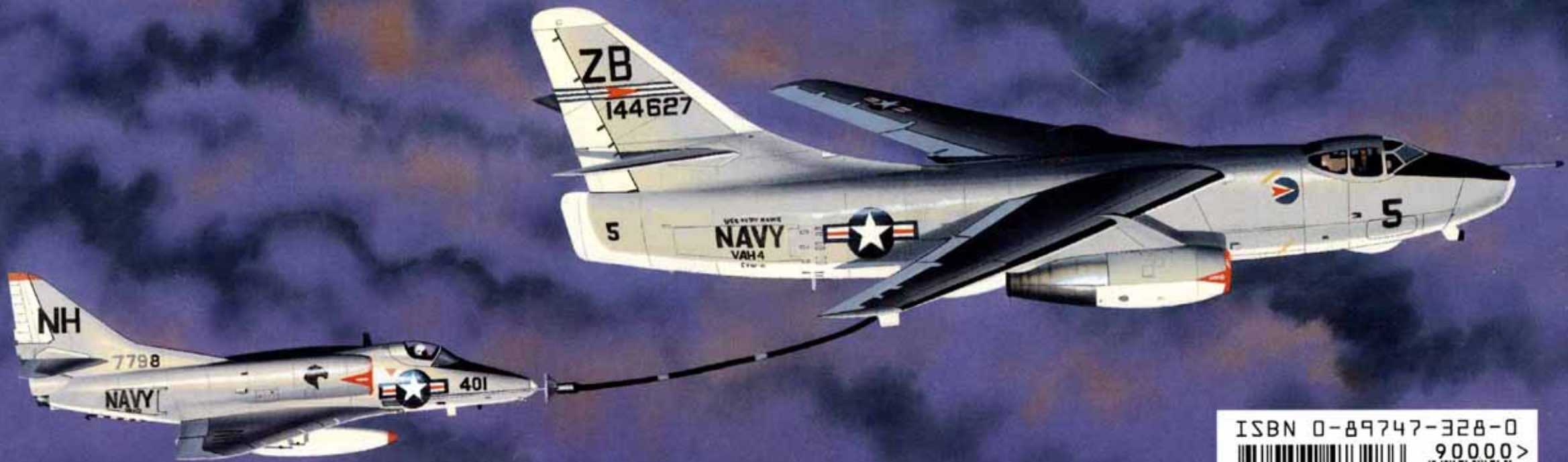
A KA-3B tanker of VAH-4 refuels an A-4C Skyhawk of VA-112 off the coast of Vietnam during 1967. KA-3Bs were the primary tanker asset for the Navy during the Vietnam war.
