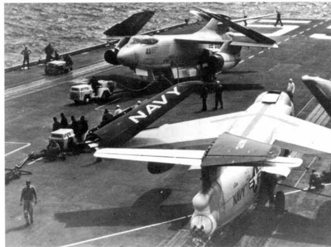
The Skywarrior had hydraulic folding outer wing panels and a folding vertical fin. These aircraft are assigned to the NATC for flight test and evaluation and both have the 20mm cannon turret installed. (Douglas via Jim Mesko)
