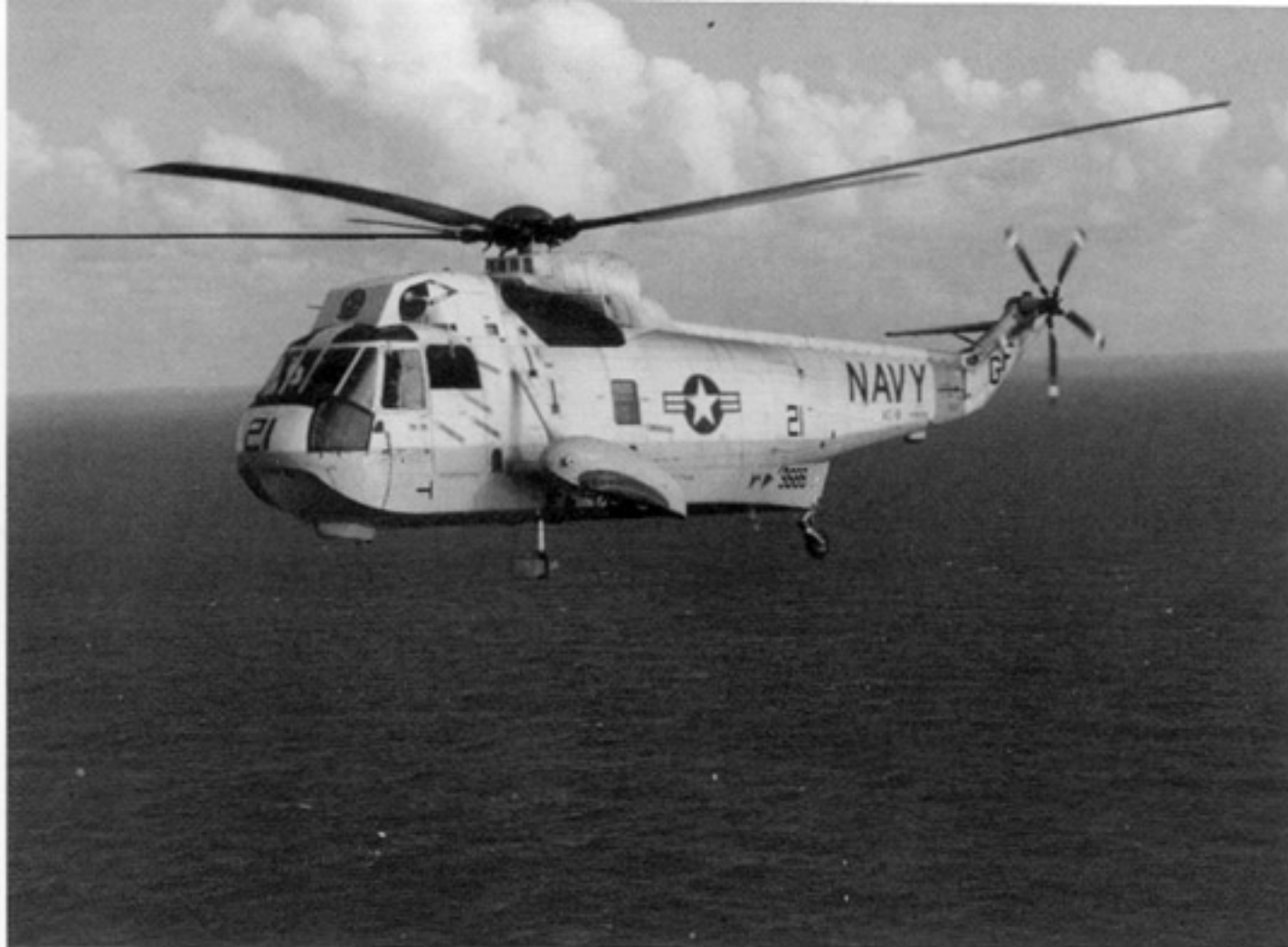
A SH-3G of VC-8 flies near NAS Roosevelt Roads, Puerto Rico during 1983. The aircraft carries a Pacific Missile Test Center (PMTTC) blocking system antenna under the forward fuselage. The antenna is used for locating downed practice air-to-air missiles. (Navy)
