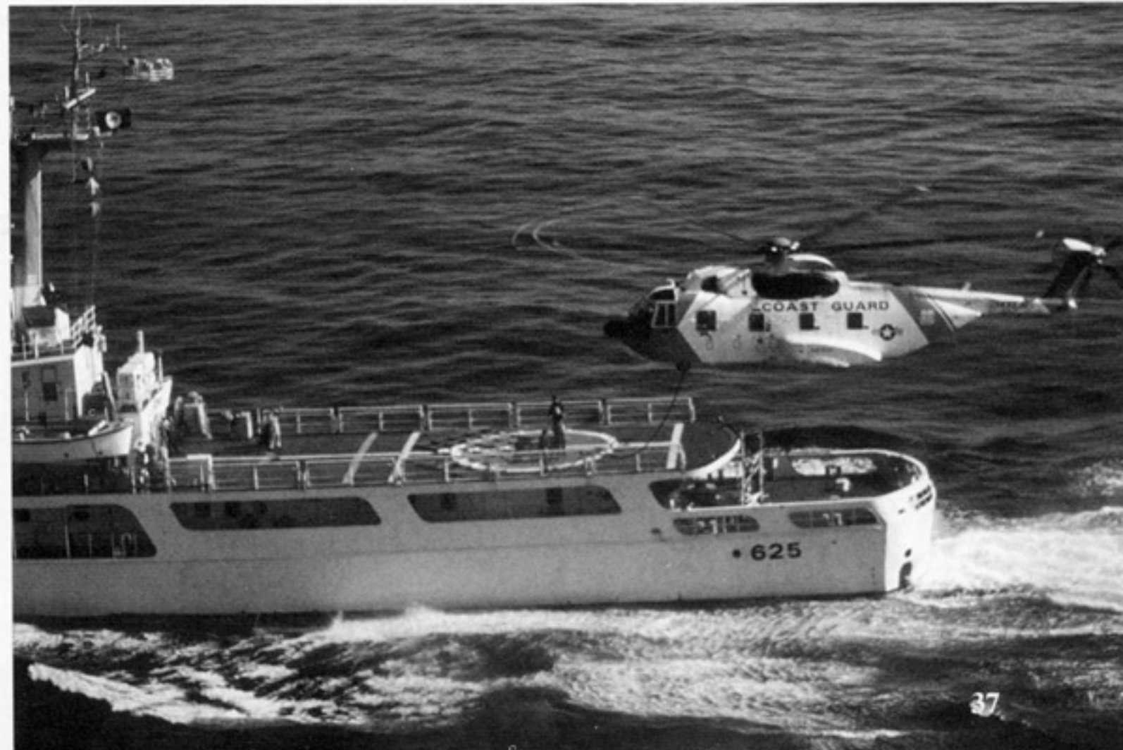
A HH-3F conducts a Hover in Flight and Refuel (HFIR) operation over the USCG Cutter VENTUROS (WMEC 625). By the use of the HFIR technique, the range of the HH-3F is limited to available ships and crew endurance. This HH-3F was stationed at USC Air Station San Diego, California. (USCG)
