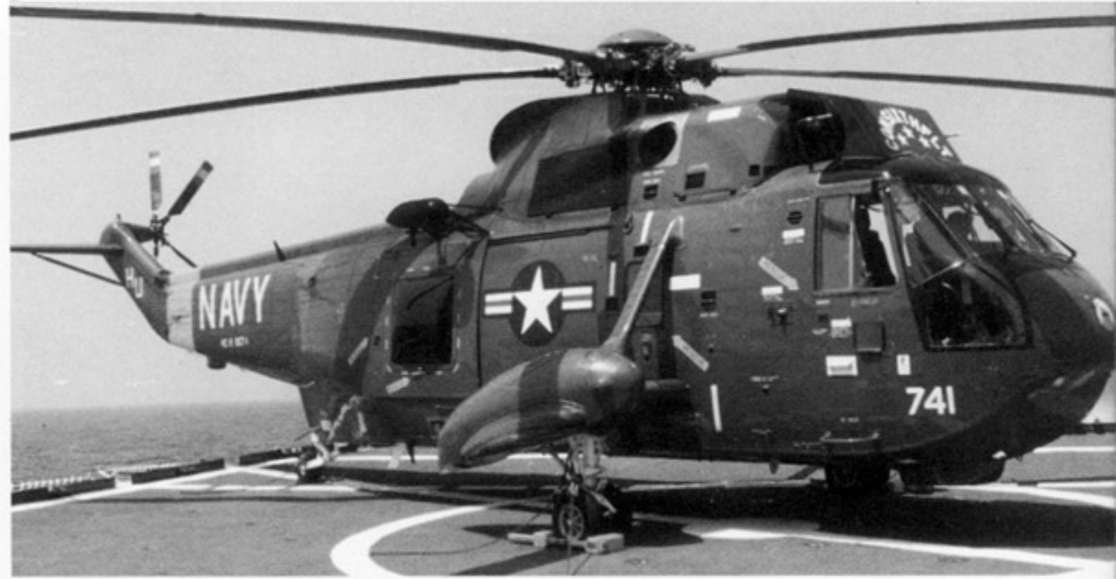
Ghostrider 741 is tied down to the helo deck of USS BELKNAP (CG-26) during June of 1992. The aircraft serves with HC-2 Det One as the personal transport for the Commander of the Sixth Fleet (COMSIXTHFLT) in the Mediterranean Sea. The aircraft was modified with an enlarged window in the cargo door. (Stu Jones)
