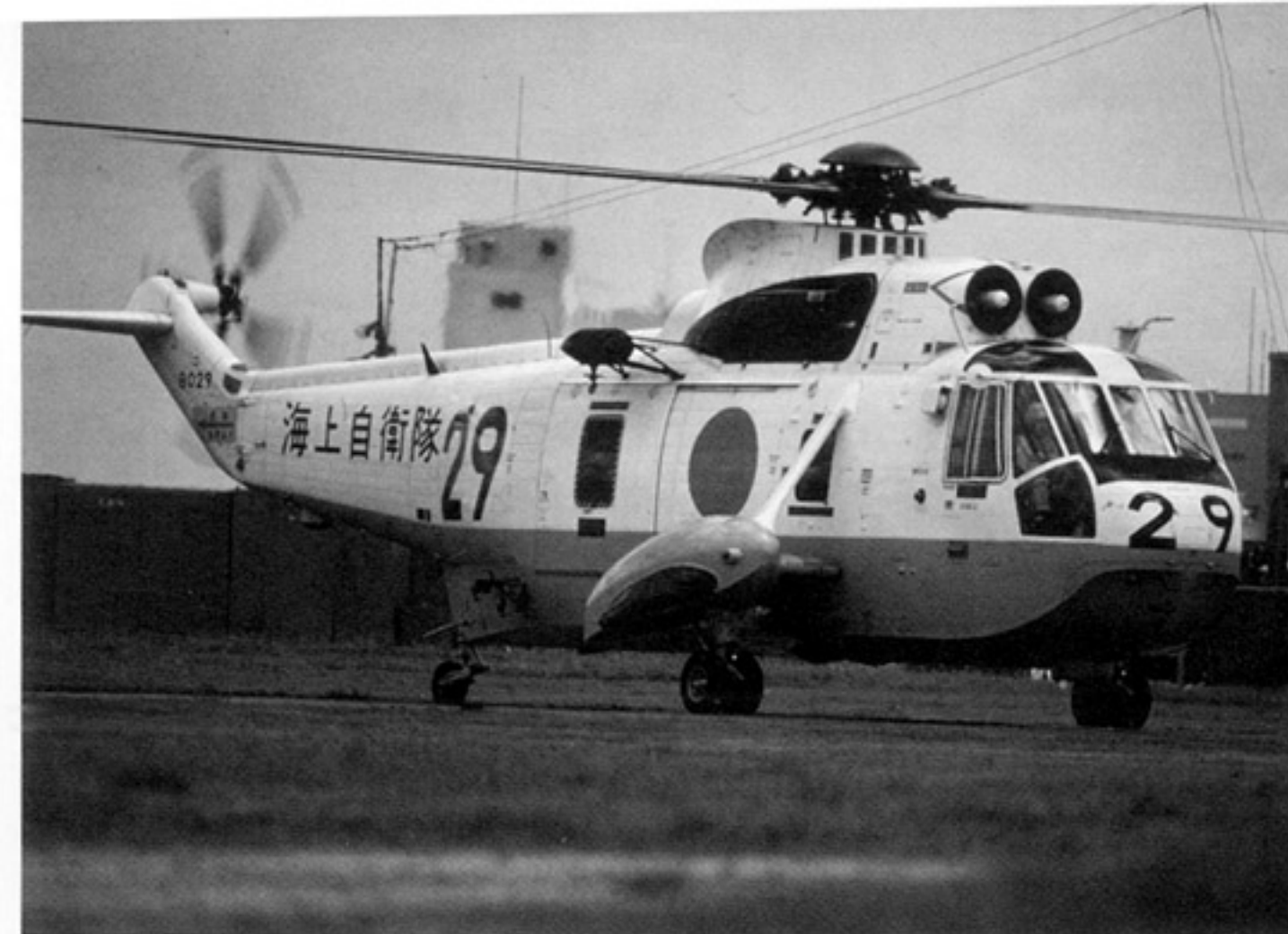
Mitsubishi of Japan obtained a license to produce the SH-3A under the designation HSS-2. The first three were assembled in the U.S. with the remaining aircraft being assembled in Japan. The aircraft carried a Gloss White over Gray color scheme. (Terry Love)
