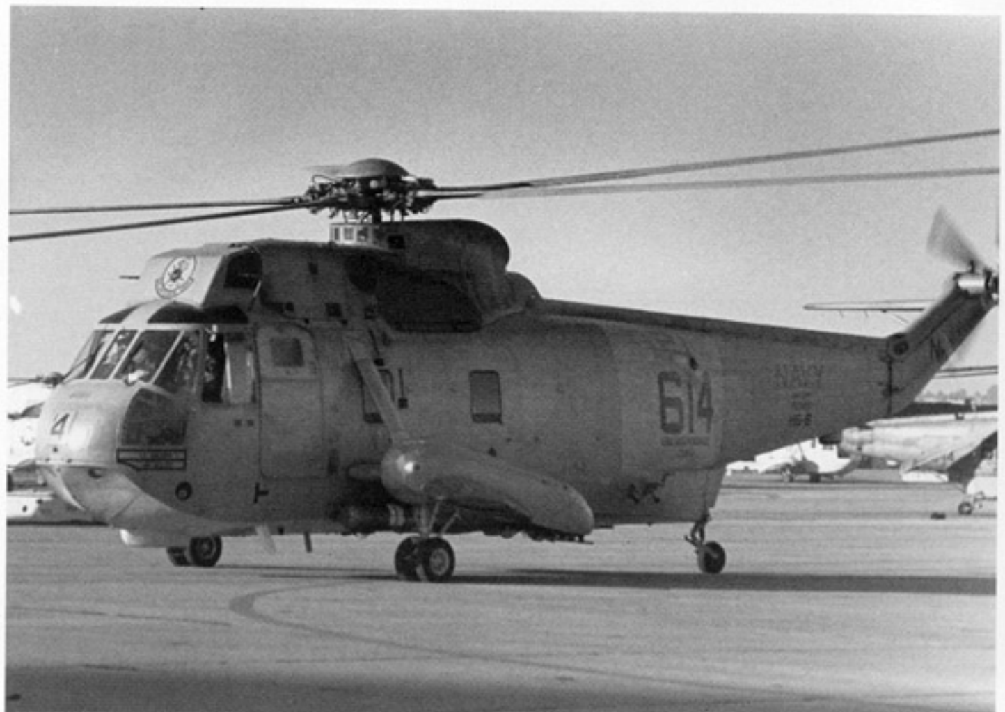
This SH-3H is carrying a torpedo on the sponson weapons station as it taxis on the ramp of NAS North Island, California during 1990. HS-8 would soon deploy aboard USS INDEPENDENCE (CV-62) for duty in Operation DESERT SHIELD. (HS-8, Navy)
