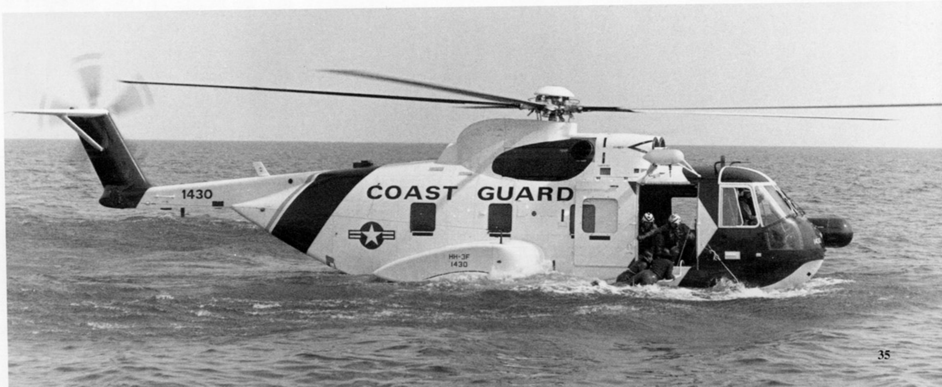
The prototype HH-3F (1430) during a test flight from the Sikorsky plant. The HH-3F was based on the HH-3E without armor, armament, self-sealing fuel tanks and in-flight refueling. The aircraft was also equipped with a nose mounted weather/search radar. (USCG)
