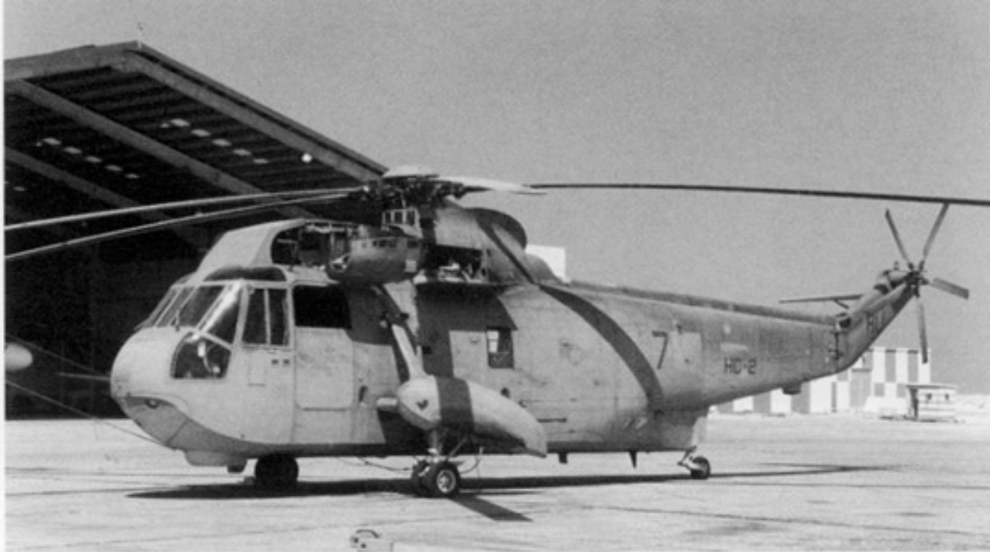
A SH-3G sets on the ramp at Bahrain with the engine panels open. These panels also serve as work stands for maintenance personnel. The aircraft is in the process of having its individual aircraft number changed and has the last two digits painted out. It was later number 741. (Stu Jones)
