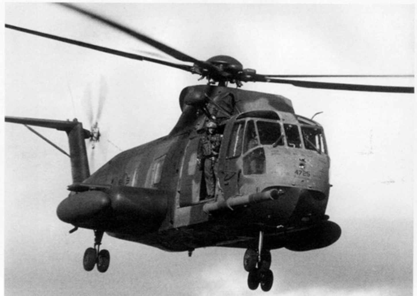
An aircrewman stands in the door of this HH-3E of the 129th AARS Jolly Greens from NAS Moffett Field, California. The aircraft is in the wraparound "Lizard" camouflage. (via Michael R. Hursh)
