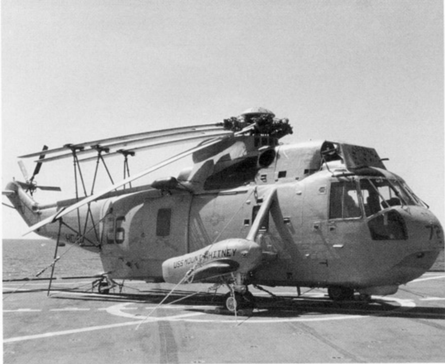
A SH-3H of HC-2 Detachment 4 tied down on the deck of USS MOUNT WHITNEY. The rotors are folded back and tied down to keep them from flapping in the wind. (Stu Jones)
