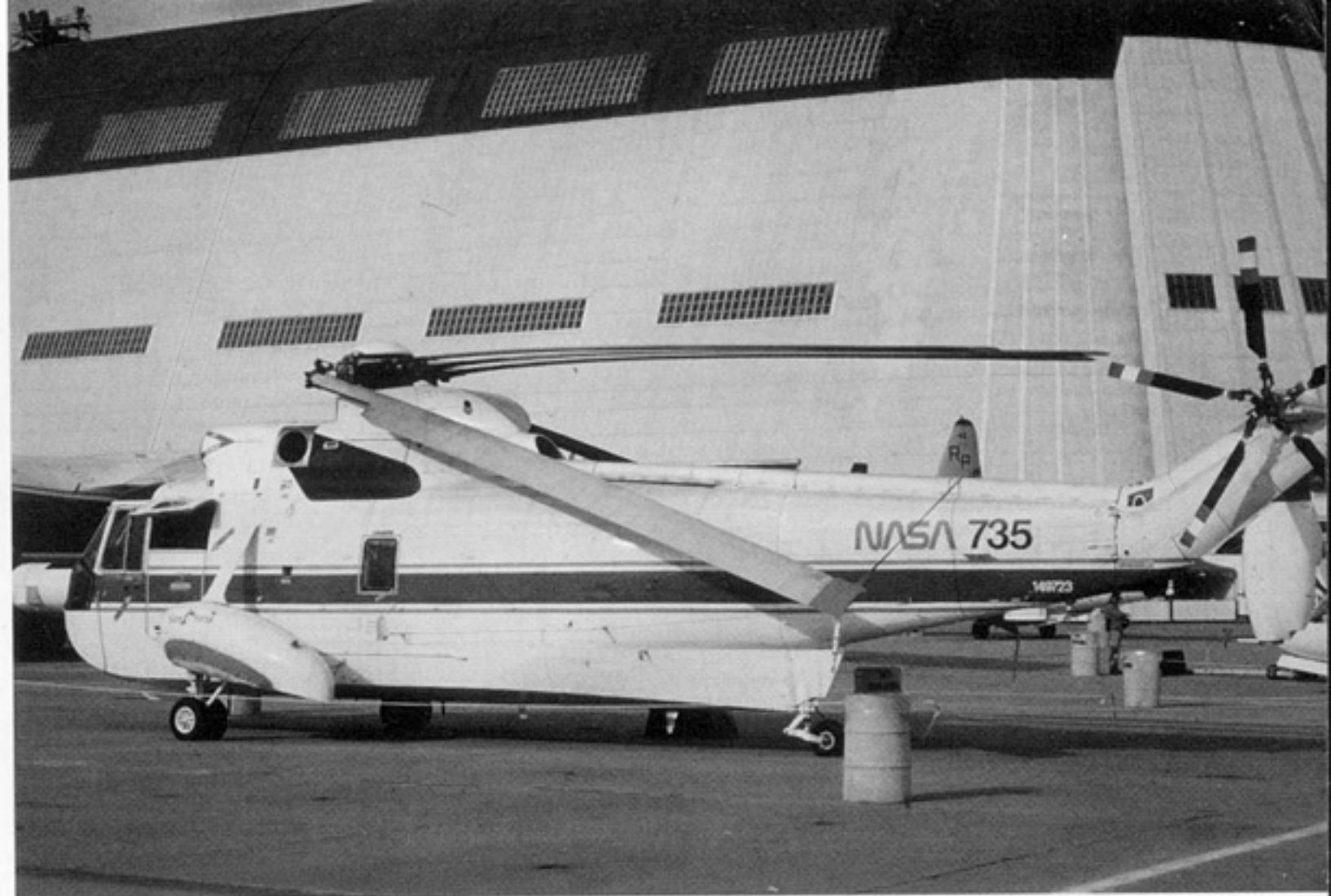
NASA used this SH-3A (BuNo 149723) to flight test the nose mounted APN 215 search radar that would later become a standard feature on Coast Guard HH-3F Pelican SAR helicopters. The aircraft was in overall Gloss White with Blue stripping. It carried the legend Sea King on the sponson in Red. (Terry Love)
