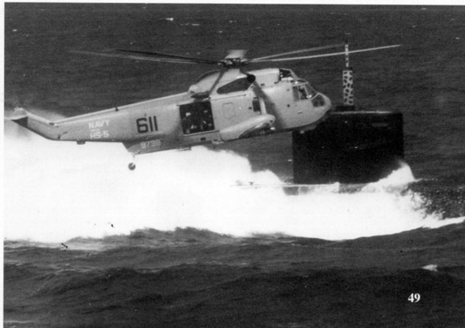
This SH-3H (BuNo 152124) of HS-6 Indians is towing its AN/AQS-81 MAD towed body. The Sea King is over a Navy Frigate in the Pacific. Smoke markers are carried under the sponson for target marking. (Navy)
