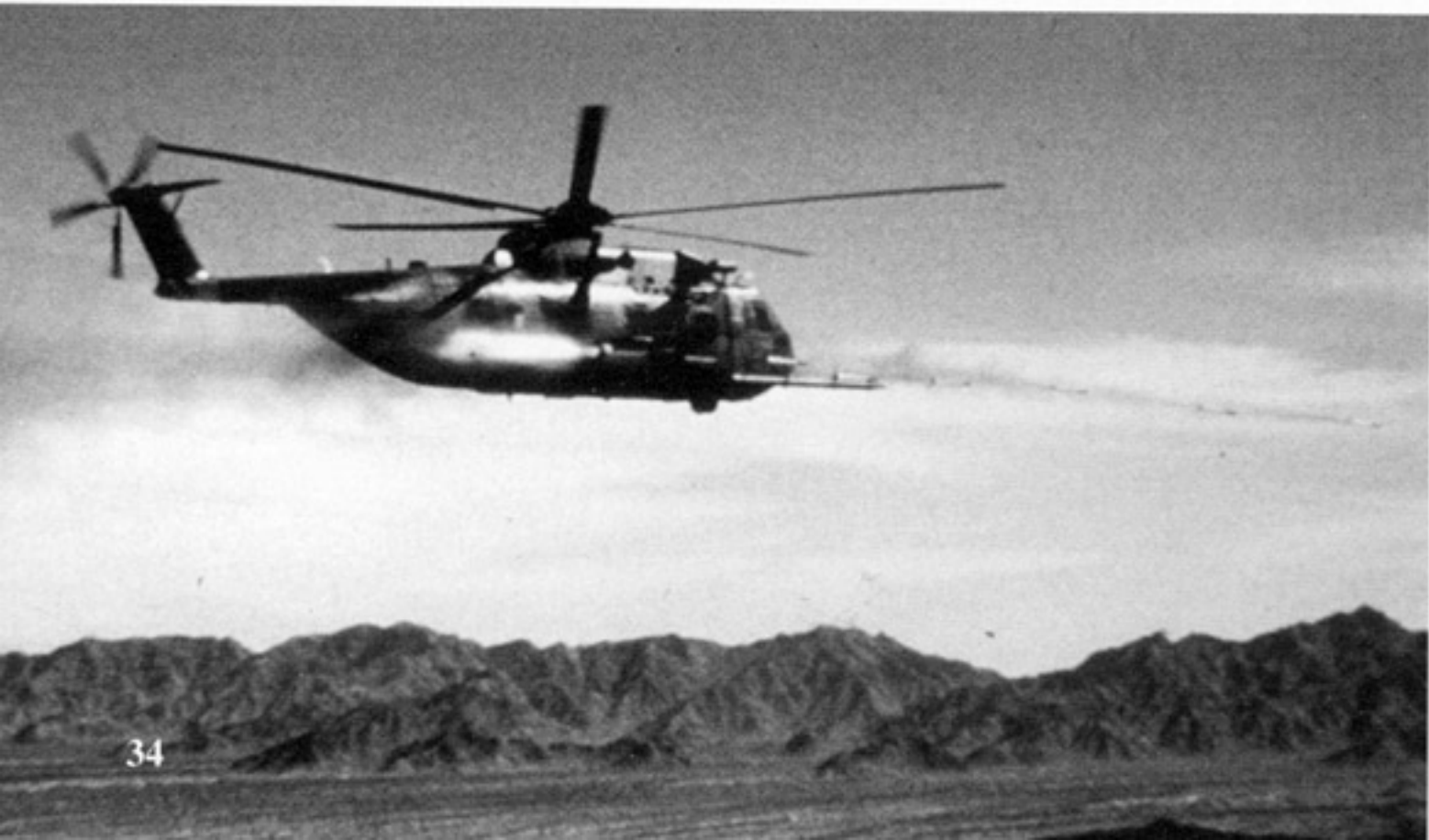
A HH-3E of the 71st Special Operations Squadron, Davis-Monthan AFB, Arizona fires a volley of 2.75 inch rockets during tests at the Goldwater North tactical range at Gila Bend. Although successful, it was decided not to arm the HH-3Es with rockets. (Major Michael G. Shook, USAF)
