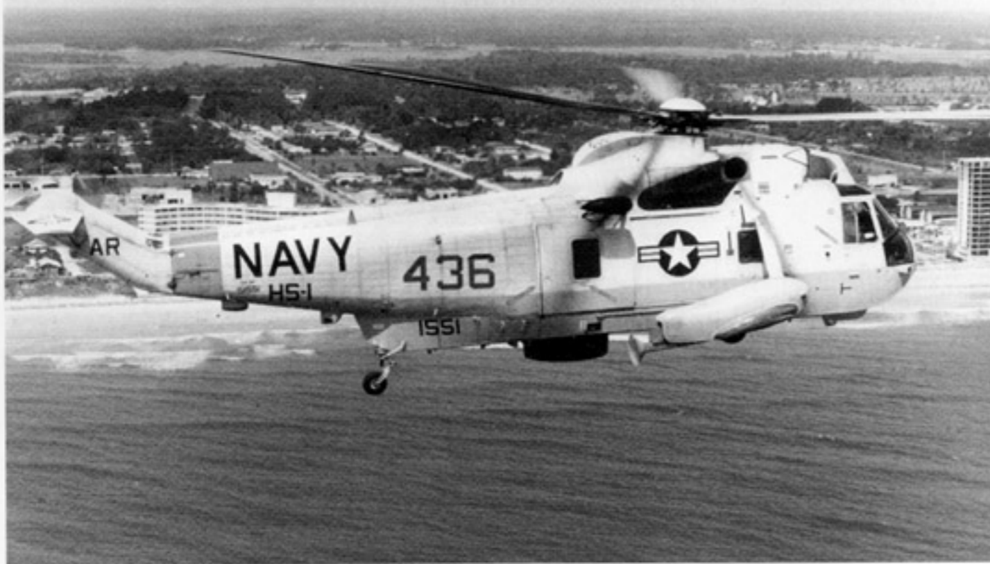
An early SH-3H (BuNo 151551) of HS-1 Seahorses flies over the beach near NAS Jacksonville, Florida. HS-1 is the Atlantic Fleet training squadron for the SH-3. This SH-3H carries the surface search radar under the fuselage. (Navy via Ron Williamson)
