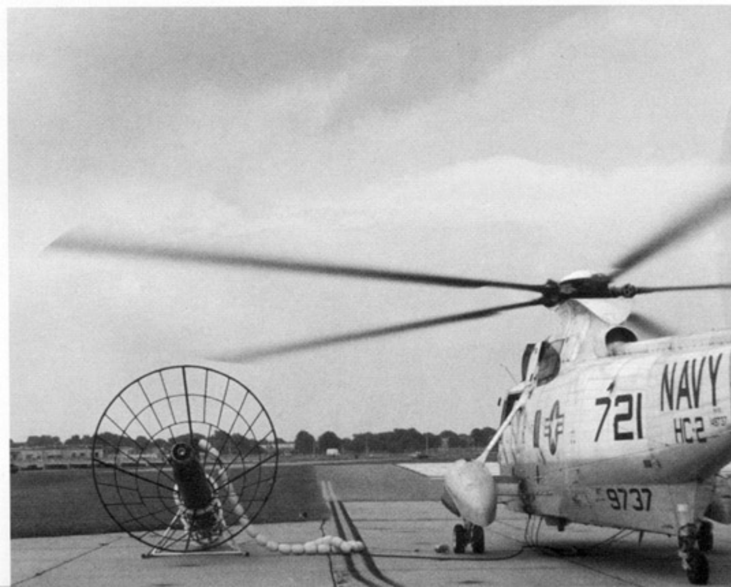
A SH-3G (BuNo 149737) lands at NAS Norfolk, Virginia with a Mk 48 training torpedo in the recovery cage. HC-2 supports the Atlantic fleet in the utility and transportation roles. (Stu Jones)
