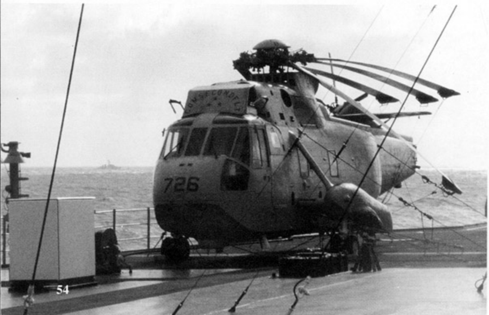
This SH-3H is assigned to the Commander Second Fleet aboard USS MOUNT WHITNEY (LCC-20). The aircraft is secured by chains to the metal tie-downs in the ship's deck to prevent it from rolling about in heavy seas. (Stu Jones)
