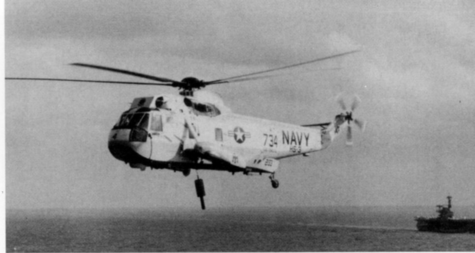
A Sea King of HS-3 Tridents deploys its AQS-13 dipping sonar. The aircraft was assigned to USS FORRESTAL (CV-59) and was a SH-3A that was converted to SH-3H standards. The squadron recently re-equipped with the SH-60F Seahawk. (Navy via Ron Williamson)
