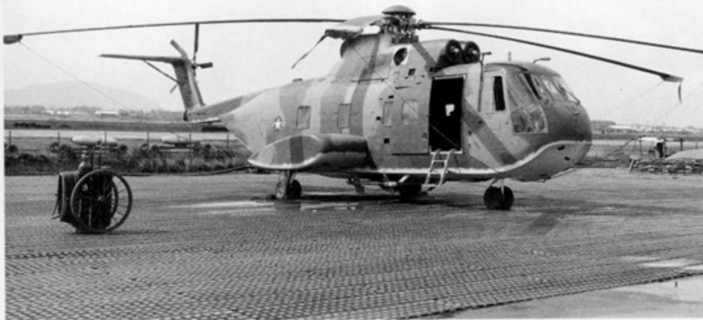
A CH-3C of the 37th Air Rescue Squadron on the ramp at Danang Air Base, South Vietnam. The 37th ARS was activated at Danang to operate in I and II Corps of South Vietnam as well in North Vietnam. The CH-3C had a top speed of 180 mph and could carry up to twenty-six troops. (USAF)
