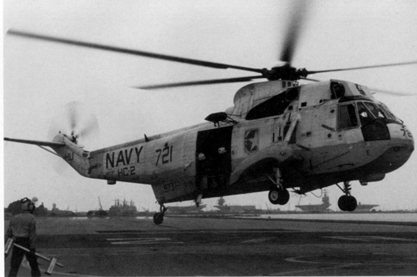
A ground crewman holds the wheel chocks for this SH-3G (BuNo 149773) of HC-2 as it lands at NAS Norfolk, Virginia during 1991. The aircraft carries the squadron insignia on the ice/FOD deflector in front of the engine air intakes. (Stu Jones)
