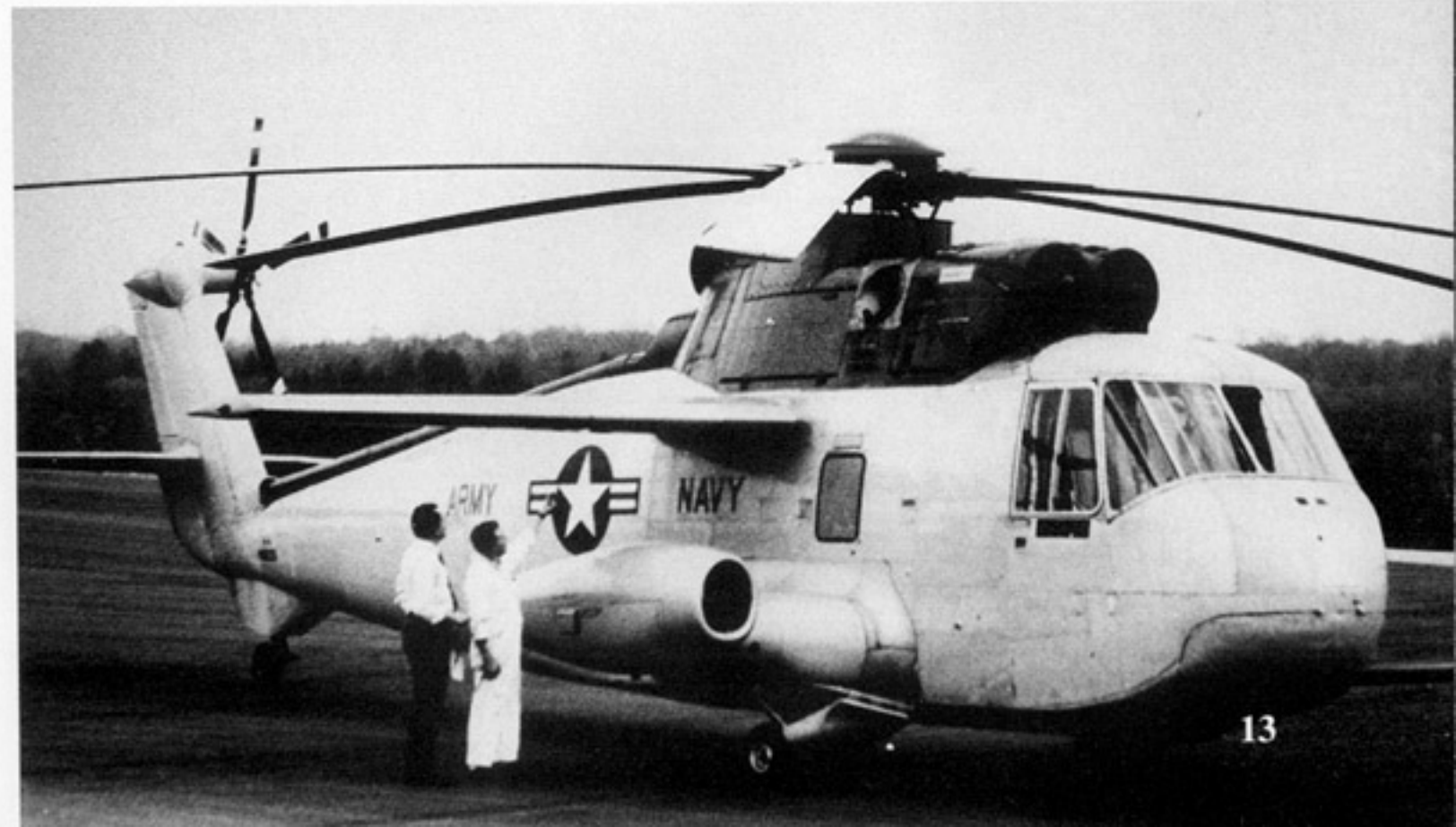
The NH-3A (BuNo 148033) was an experimental airframe used by a joint Army/Navy team to explore the merits of compound helicopter technology and flight characteristics. The Sea King was modified with the addition of thirty-two foot wings, and two Pratt & Whitney 3,000 lbst turbojets. (via Paul Novak)
