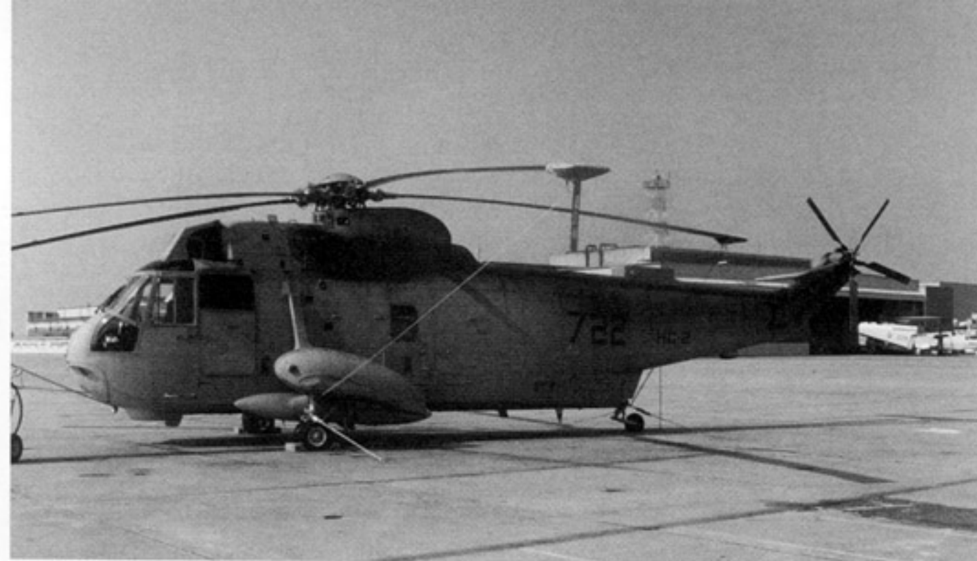
HU 722, a SH-3G of HC-2 parked on the ramp at Bahrain during 1991. During Operation DESERT STORM, the aircraft was kept on alert with external fuel tanks for SAR missions. The Sea King was finished in overall Medium Gull Gray with Dark Gray lettering. (Stu Jones)
