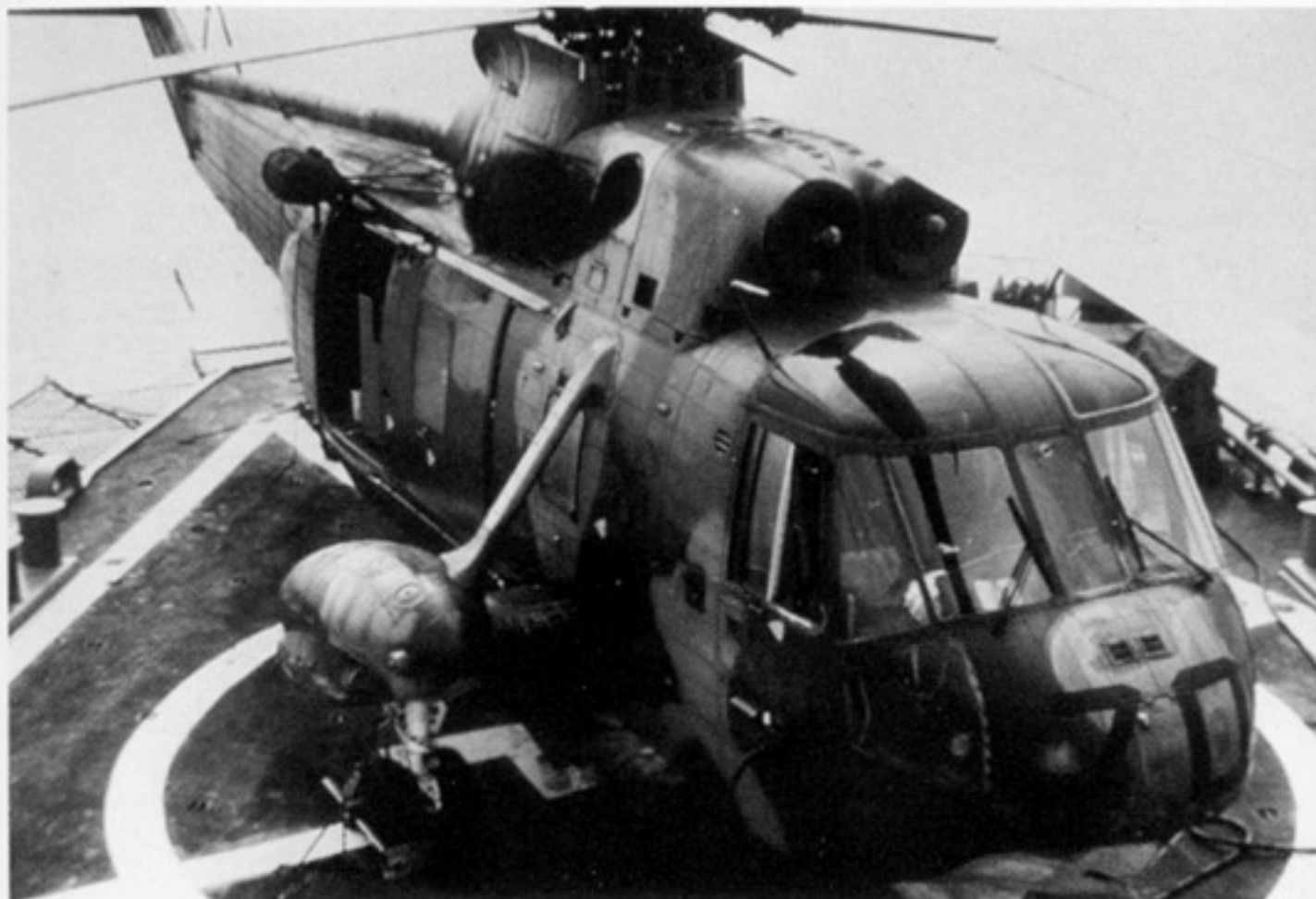
This SH-3A of HS-2 Golden Falcons operated off USS MAHAN (DLG-11) as a Search and Rescue (SAR) detachment. The Sea King was camouflaged in Dark Green, Tan and Gray and was armed with two GAU-23 Miniguns in the port and starboard doors. (Captain Steve Millikin, USN, Ret.)
