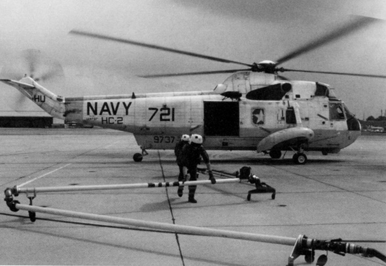
These crewmen have just completed refueling their SH-3G and are moving the hard hose back out of the way prior to take off from NAS Norfolk, Virginia during 1991. (Stu Jones)
