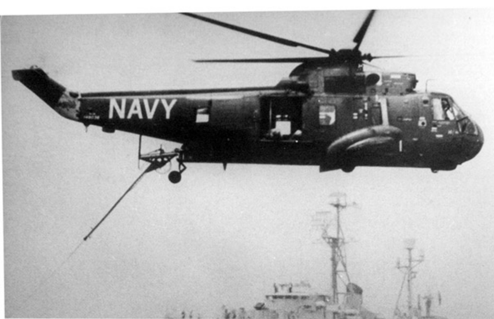
Sikorsky modified nine SH-3As with mine clearing equipment under the designation RH-3A. RH-3As were used aboard mine-countermeasures ships to extend the range of mine sweeping operations. This RH-3A served aboard USS THOMAS J. GRAY (DER-326). (via Paul Novak)
