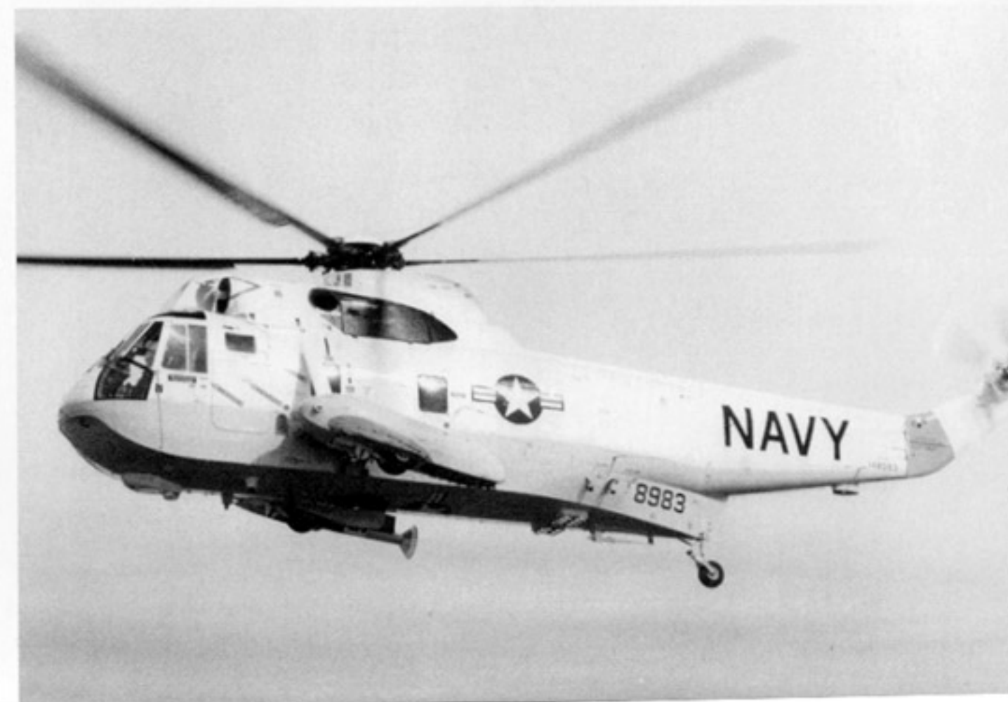
A late SH-3H (BuNo 148983) without the underfuselage radar antenna. Sonabouy launchers and a sonabouy data link antenna are under the rear fuselage just below the weapons racks. The MAD towed body is visible on the opposite sponson. (United Technologies via Ron Williamson)
