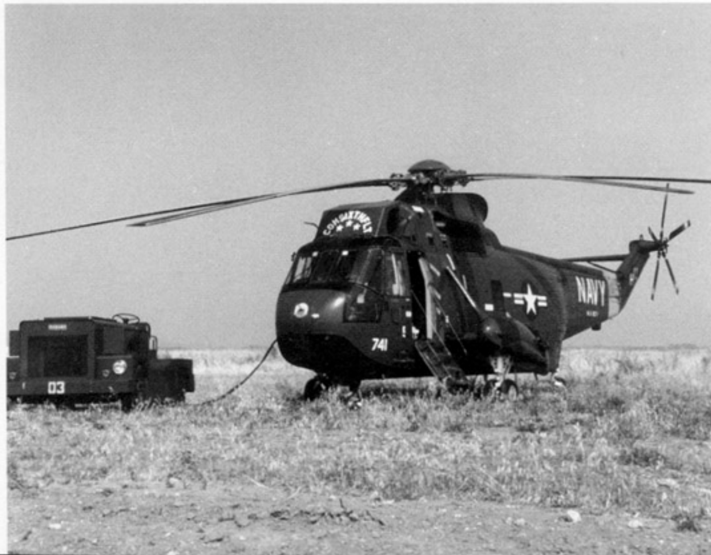
This SH-3G (BuNo 151527) is parked on the dirt ramp at Naval Air Facility, Naples, Italy during 1992. The aircraft is hooked up to an Italian power unit for preflighting. HC-2 keeps a detachment at Naples to support the Sixth Fleet. (Stu Jones)
