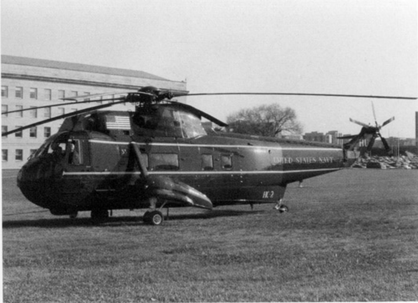
A VH-3A (BuNo 150613) of HC-2 rests on the grass pad at the Pentagon awaiting its VIP passengers. HC-2 flies high ranking officials around the Washington area. Their Sea Kings are painted Gloss Olive Drab with White stripping. (Stu Jones)
