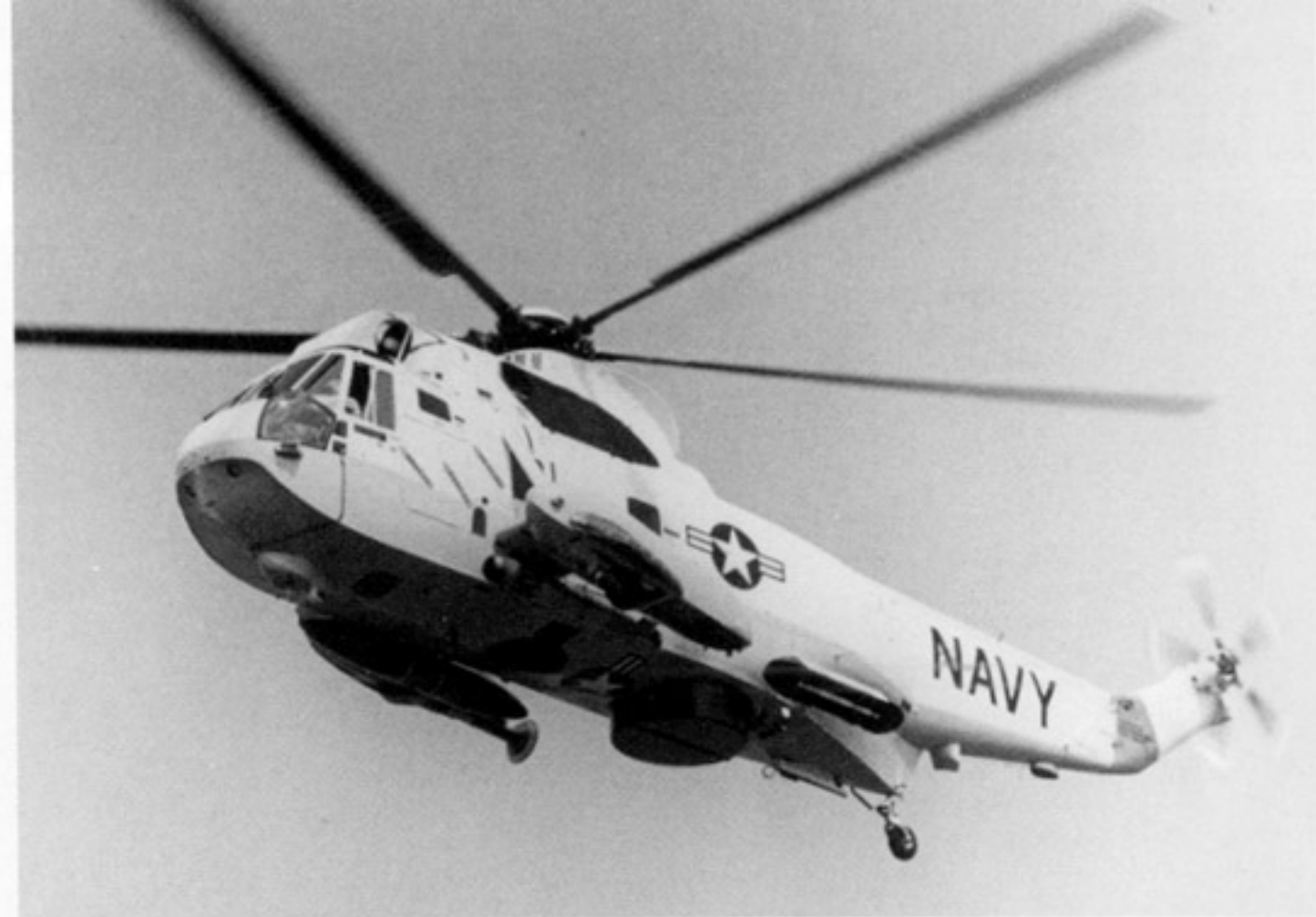
This newly converted SH-3H (BuNo 149927, ex-SH-3A) is equipped with a Canadian-Marconi radar under the fuselage, an under sponson fuel tank and a MK 48 torpedo under the port sponson. The object on the rear fuselage station is a chaff/flare dispenser. (Navy via Jim Presley)
