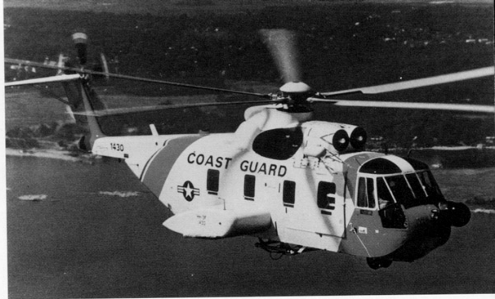
The prototype HH-3F (1430) during a test flight from the Sikorsky plant. The HH-3F was based on the HH-3E without armor, armament, self-sealing fuel tanks and in-flight refueling. The aircraft was also equipped with a nose mounted weather/search radar. (USCG)
