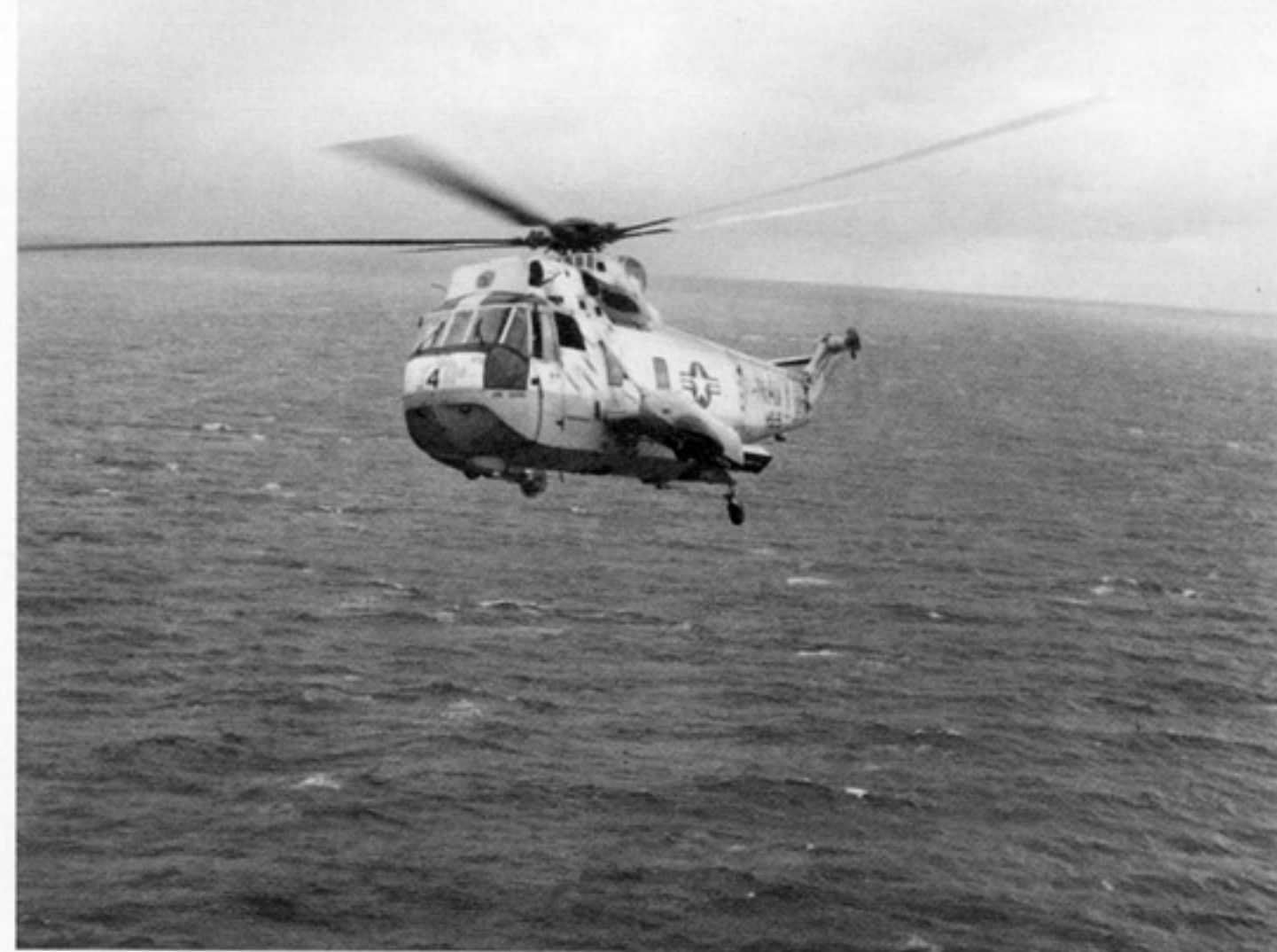
A SH-3H of HS 9 Sea Griffins flies low over the Bermuda operating area during 1986. The aircraft carries a chaff/flare dispenser on the port rear weapons station. (Navy)
