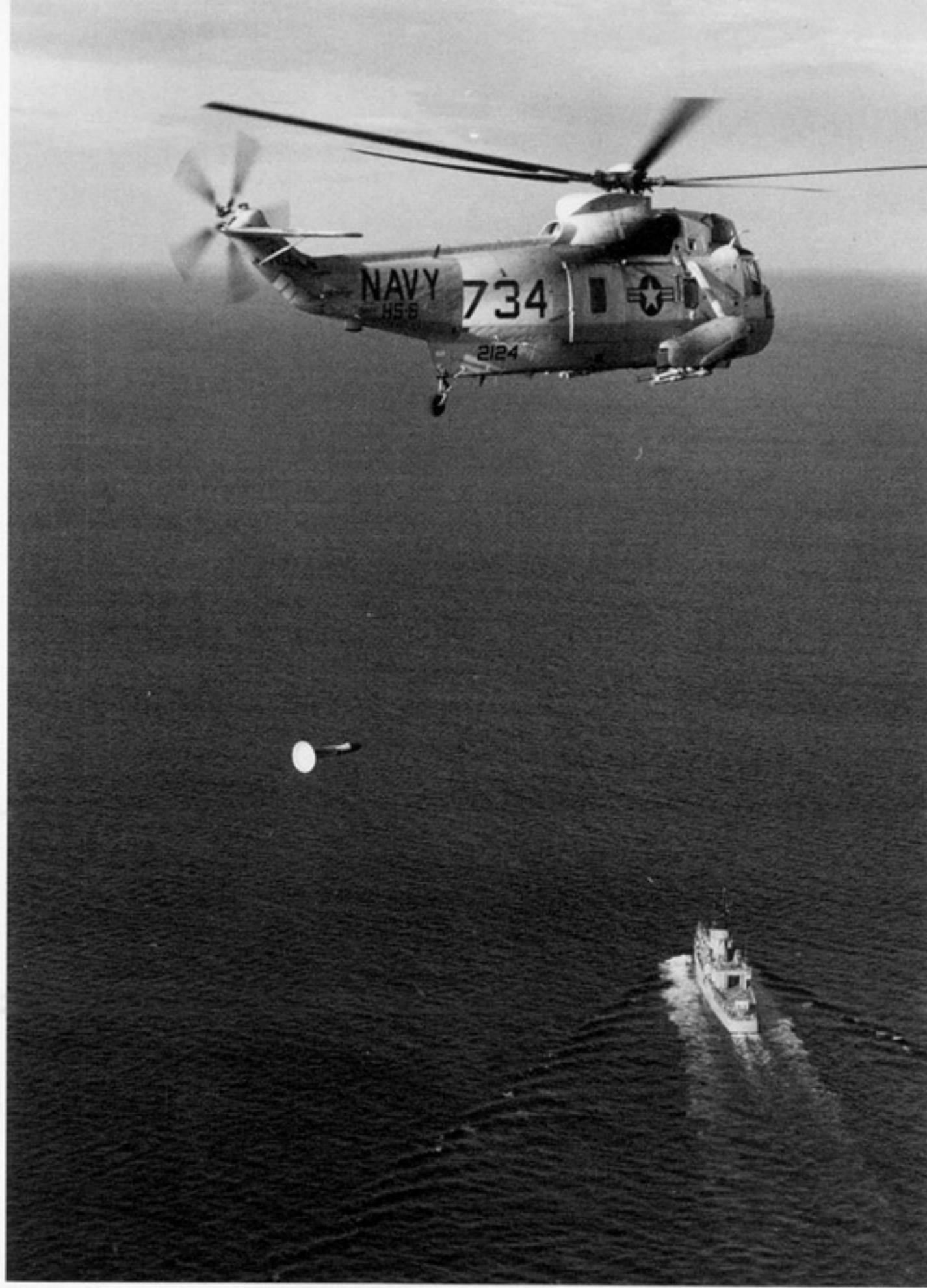
This SH-3H (BuNo 152124) of HS-6 Indians is towing its AN/AQS-81 MAD towed body. The Sea King is over a Navy Frigate in the Pacific. Smoke markers are carried under the sponson for target marking. (Navy)
