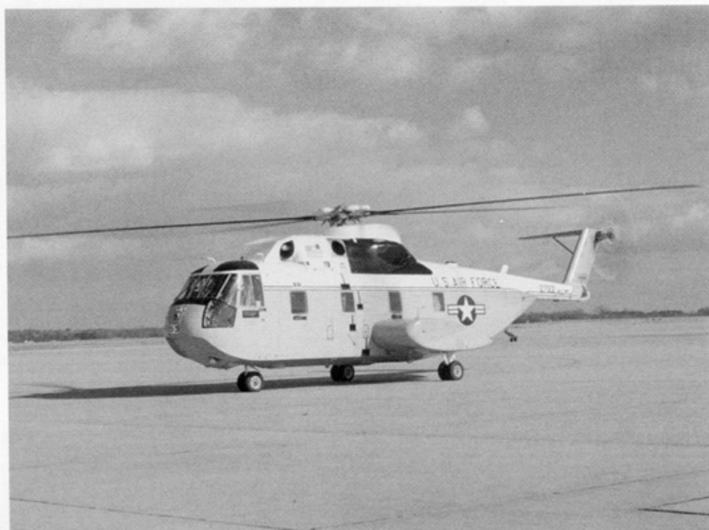
A CH-3E of the 1st Helicopter Squadron, 89th Military Airlift Wing, at Andrews AFB, Maryland taxis out to the active runway. The aircraft was White over Light Gray with a Red/White/Blue cheat line. This aircraft was one of nine that were transferred to the USCG and rebuilt to HH-3F standards. (USAF)
