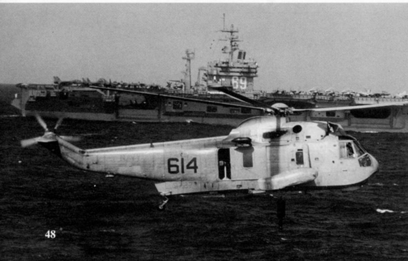
This SH-3H of HS-5 Night Dippers is lowering its dipping sonar to begin a sweep for submarines in the Mediterranean Sea during 1988. At the time the aircraft was flying from USS DWIGHT D. EISENHOWER. (CVN-69) (Navy)
