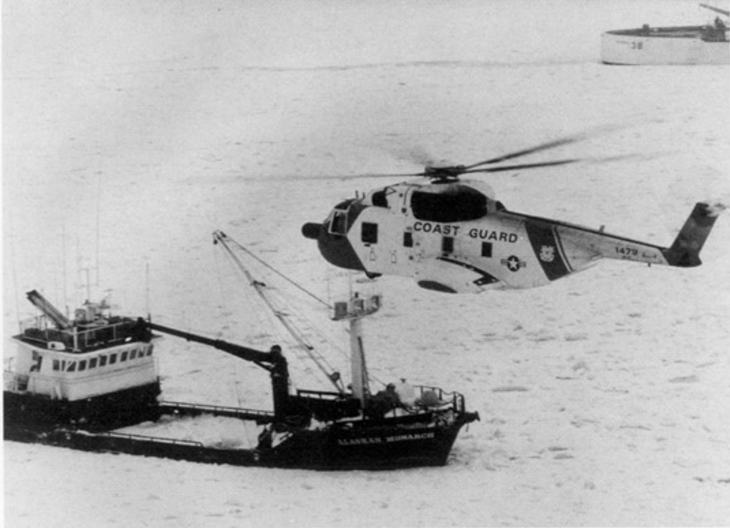
A HH-3F (1479) from Sitka flies over the ALASKAN MONARCH to check to see if there are any crewmen still aboard the ice bound ship. The HH-3F has a range of over 500 miles. The Orange nose and fuselage bands are very useful under Alaskan conditions. (USCG)
