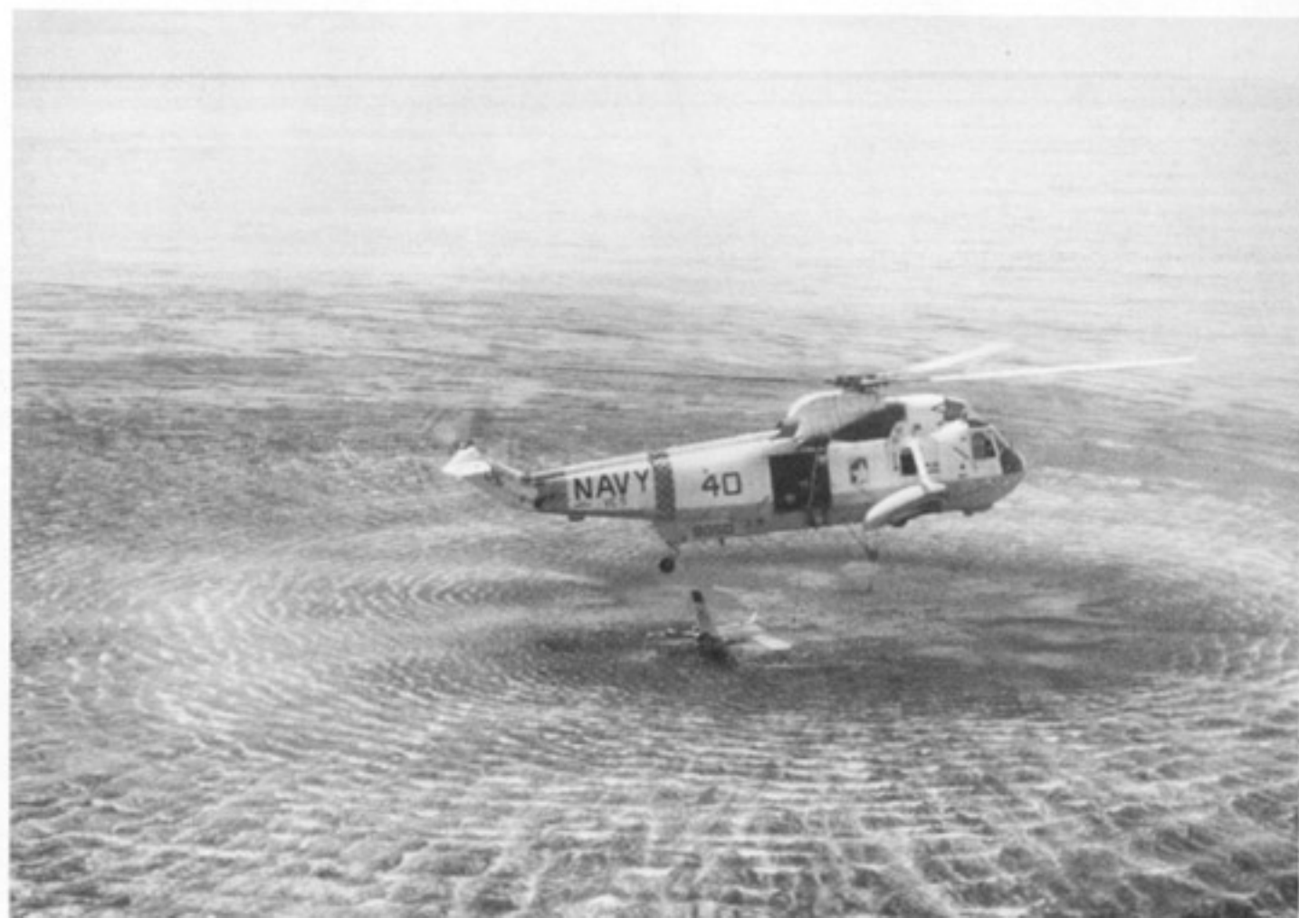
A SH-3G of Fleet Composite Squadron Five Checkertails recovers a Ryan BQM-34-S Firebee drone from the waters off Cubi Point, The Philippines during 1981. The cabin crewmen are using the rescue hoist to snag the drone before attaching it to the under-fuselage sling load hook. (Navy)
