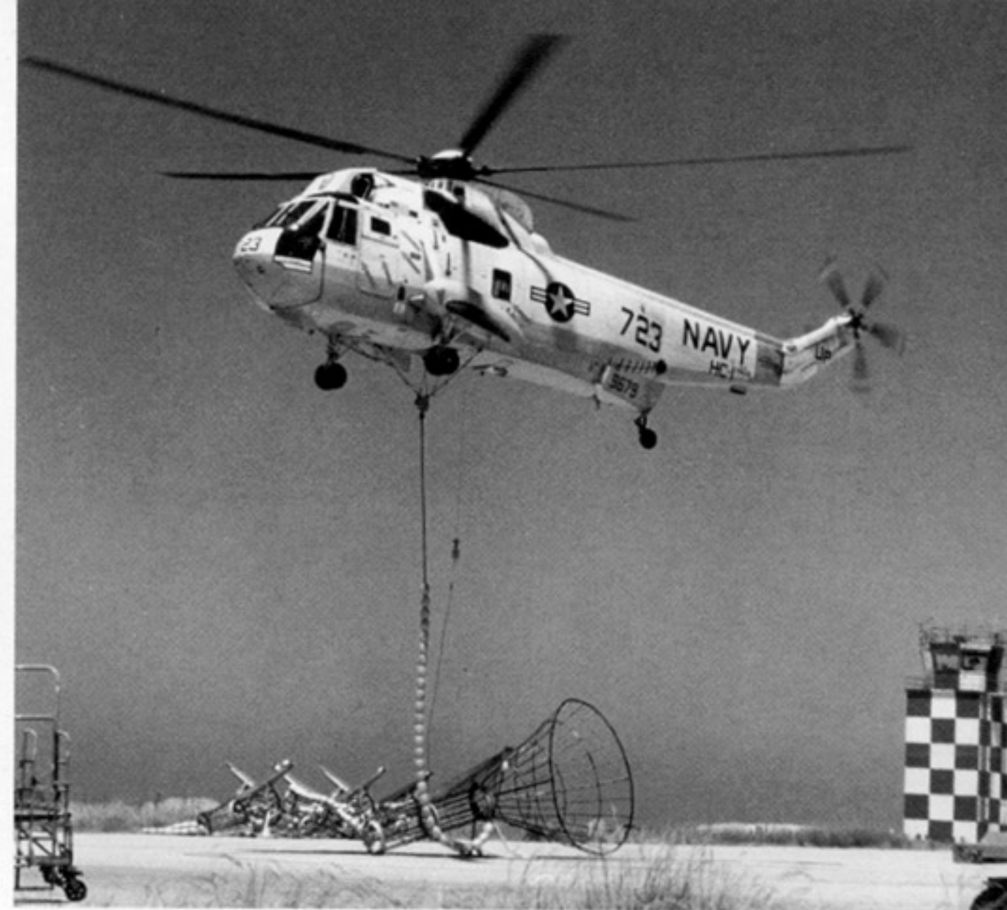
A SH-3G (BuNo 149679) of HC-1 lifts a Mk 2 Mod 0 torpedo recovery cage at NAS North Island, San Diego, California during 1991. UP 723 is fitted with an auxiliary antenna on the rear fuselage to aid in locating the training torpedoes for recovery. (Donn Keels via Stu Jones)
