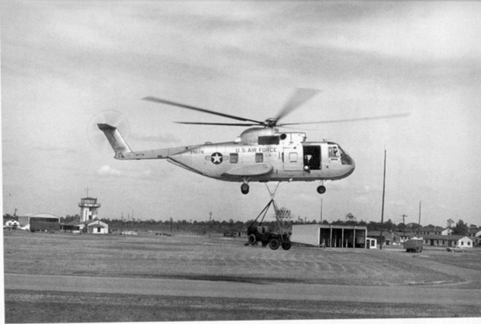
A CH-3C (63-9678) lifts a sling loaded Jeep at Eglin Air Force Base, Florida during early 1963. The CH-3C could lift up to 8,000 pounds on its external cargo hook. The loadmaster/crew chief keeps an eye on the load and if it were to become unstable he could jettison the entire load with the push of a button. (USAF via Rodney Bankston)
