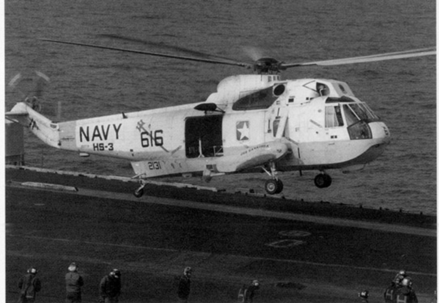
A SH-3H (BuNo 152131) of HS-3 lands aboard USS SARATOGA (CV-60) during the ship's Med cruise of 1966. The aircraft carries a M-60 machine gun mount in the open doorway, although no gun is fitted. AA 616 carries an "E" ribbon award on the fuselage under the pilots window. (HS-3, Navy)
