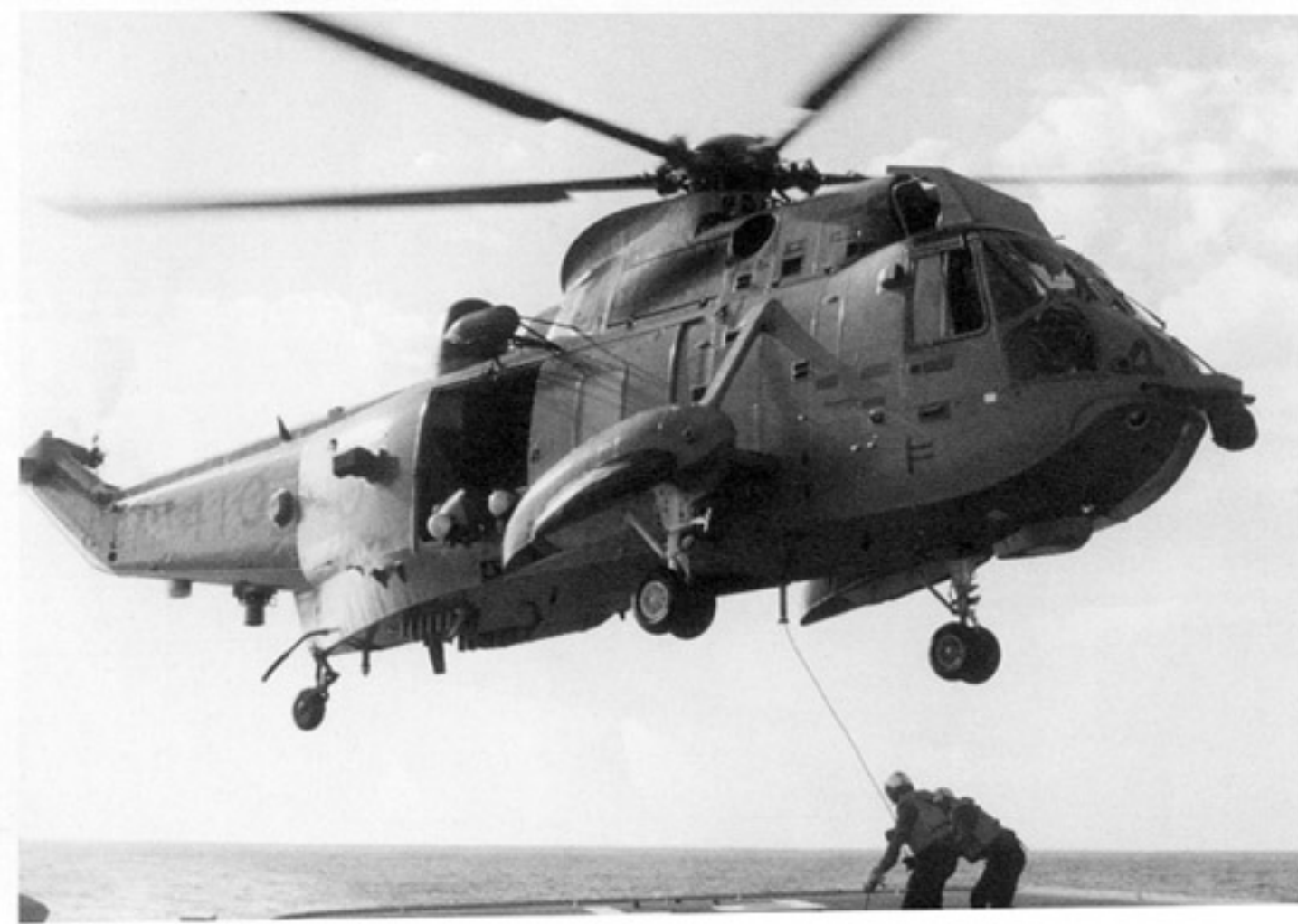
In August of 1990 Canada modified their CH-124s with a nose mounted Forward Looking Infrared (FLIR), chaff and flare dispensers and other sensors. These aircraft were deployed to the Persian Gulf as part of Operation FRICTION, the Canadian version of Operation DESERT SHIELD. (Canadian Armed Forces)
