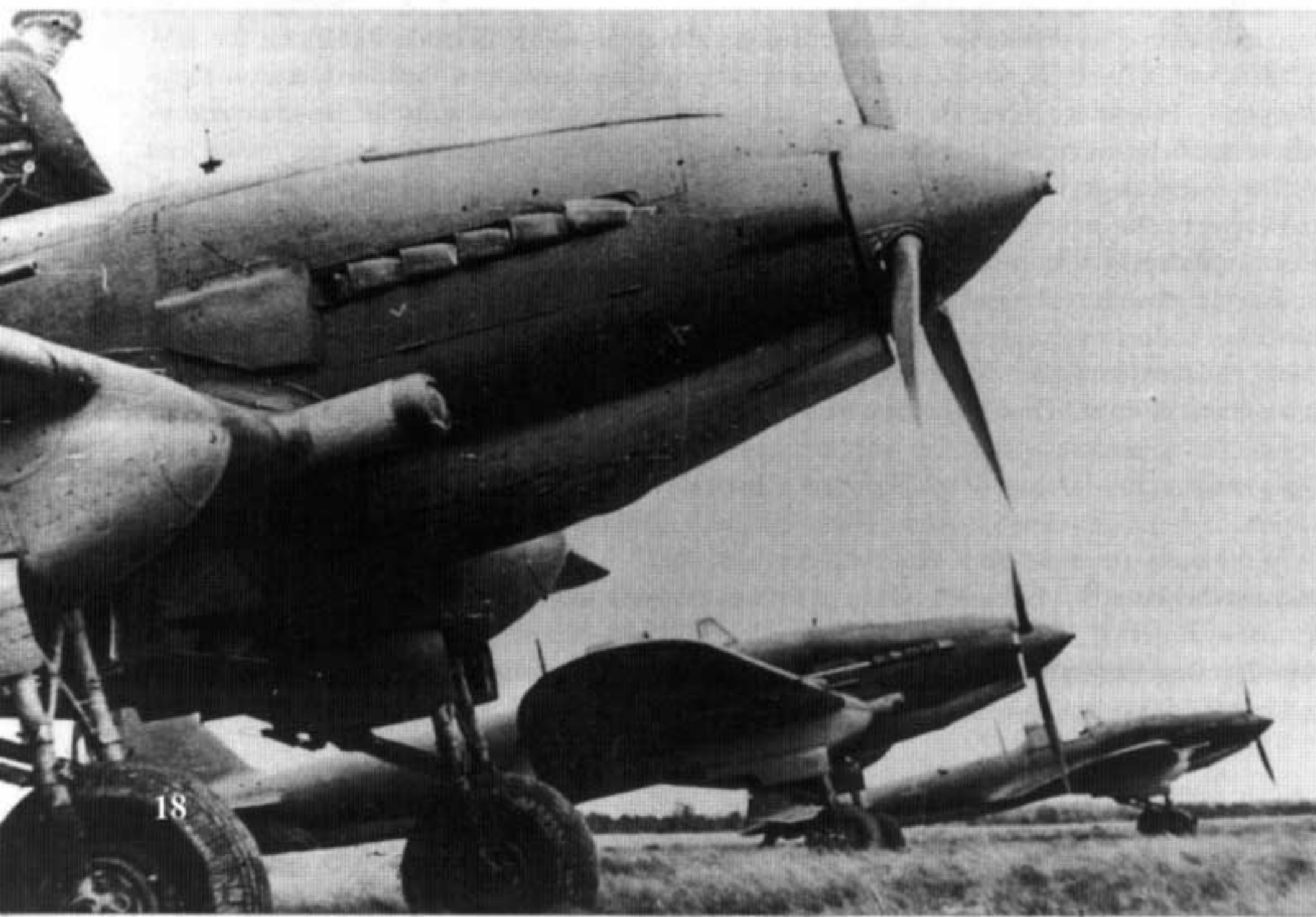
A line-up of three late production single seat Il-2s. Some late production single seat Il-2s were fitted with a sand filter mounted on the starboard wing root. This filter was not fitted to most single seaters, but became standard on all two seat Stormoviks. Late production Il-2s also had the aileron mass balance weight deleted. (G.F. Petrov)
