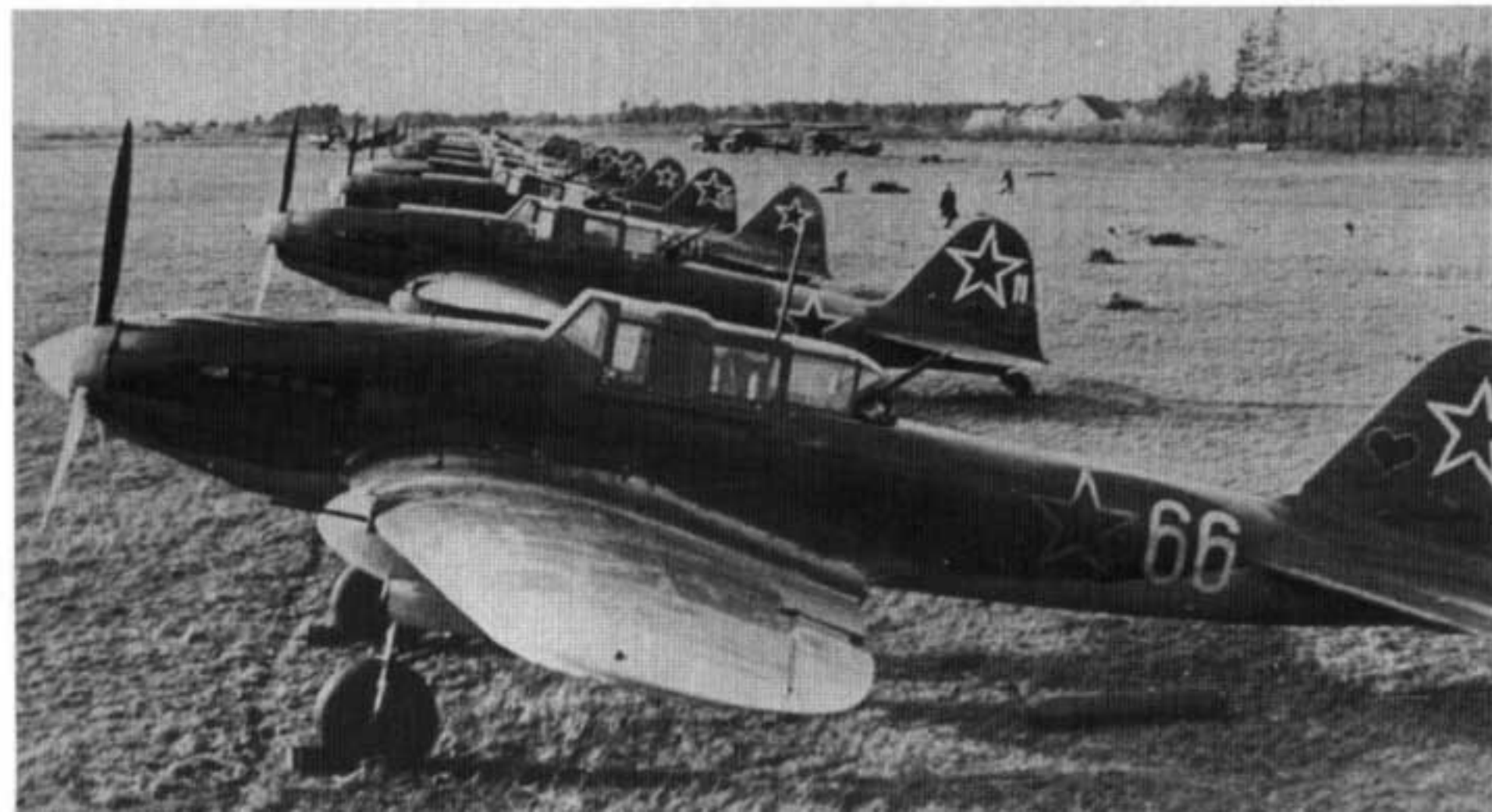
A line-up of Il-2 Type 3s of the 281st Assault Aviation Division, 14th Air Army. The aircraft in the foreground, has the tactical number, White 17, on the tail and the number, White 66, on the rear fuselage. The aircraft carries a Red heart on the fin with a thin White outline. This aircraft lacks the ventilation hatch on the rear canopy which was standard on most Il-2 Type 3s with this canopy configuration. (Klaus Niska via Carl-Fredrik Geust)
