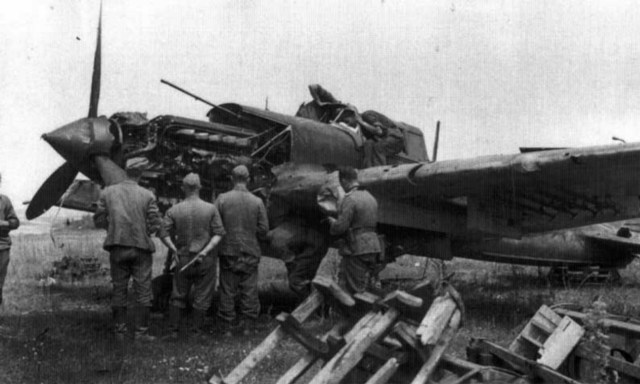
Luftwaffe personnel examine a late production Il-2 fitted with a VV-1 gun sight and four reinforcing ribs on the rear fuselage. The aircraft has had its armament stripped from the wings and has had the cowling panels removed so that Luftwaffe personnel can study the engine. (Manfred Griehl)
