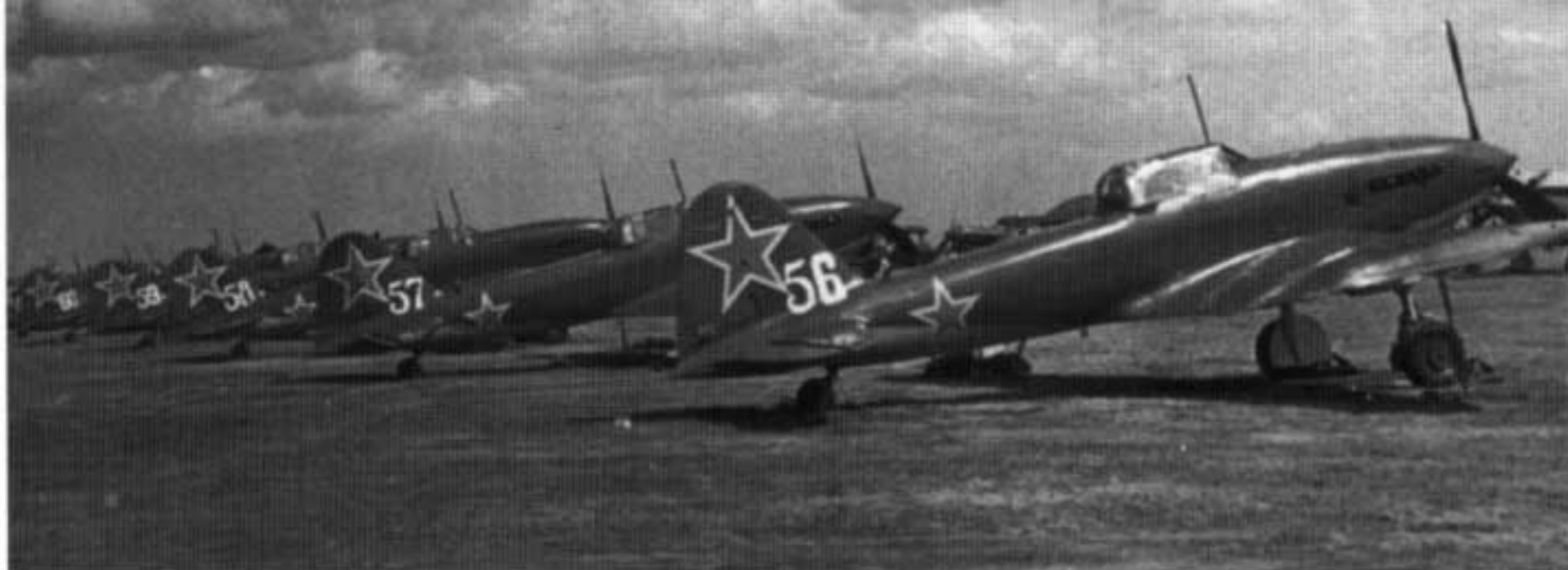
A line-up of Il-10s on an airfield in the Eastern Zone of Occupied Germany during the late 1940s. These aircraft carried their tactical markings in White at the base of the vertical fin. All are equipped with a direction finder antenna on the fuselage spine in front of the fin. (Carl-Fredrik Geust)
