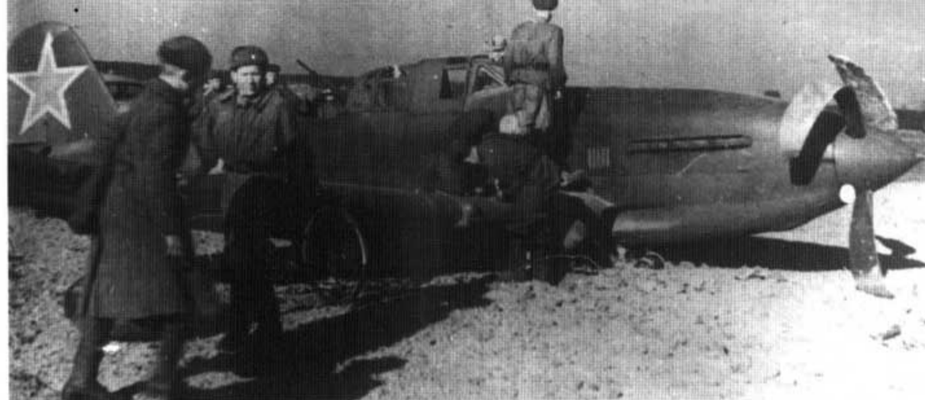
This Il-10 of the 571st Assault Aviation Regiment made a belly landing during a mission over occupied East Germany on 15 April 1945. The bent propeller blades indicate that the AM-42 engine was running at when the aircraft touched down. (Ivan Ivanov)
