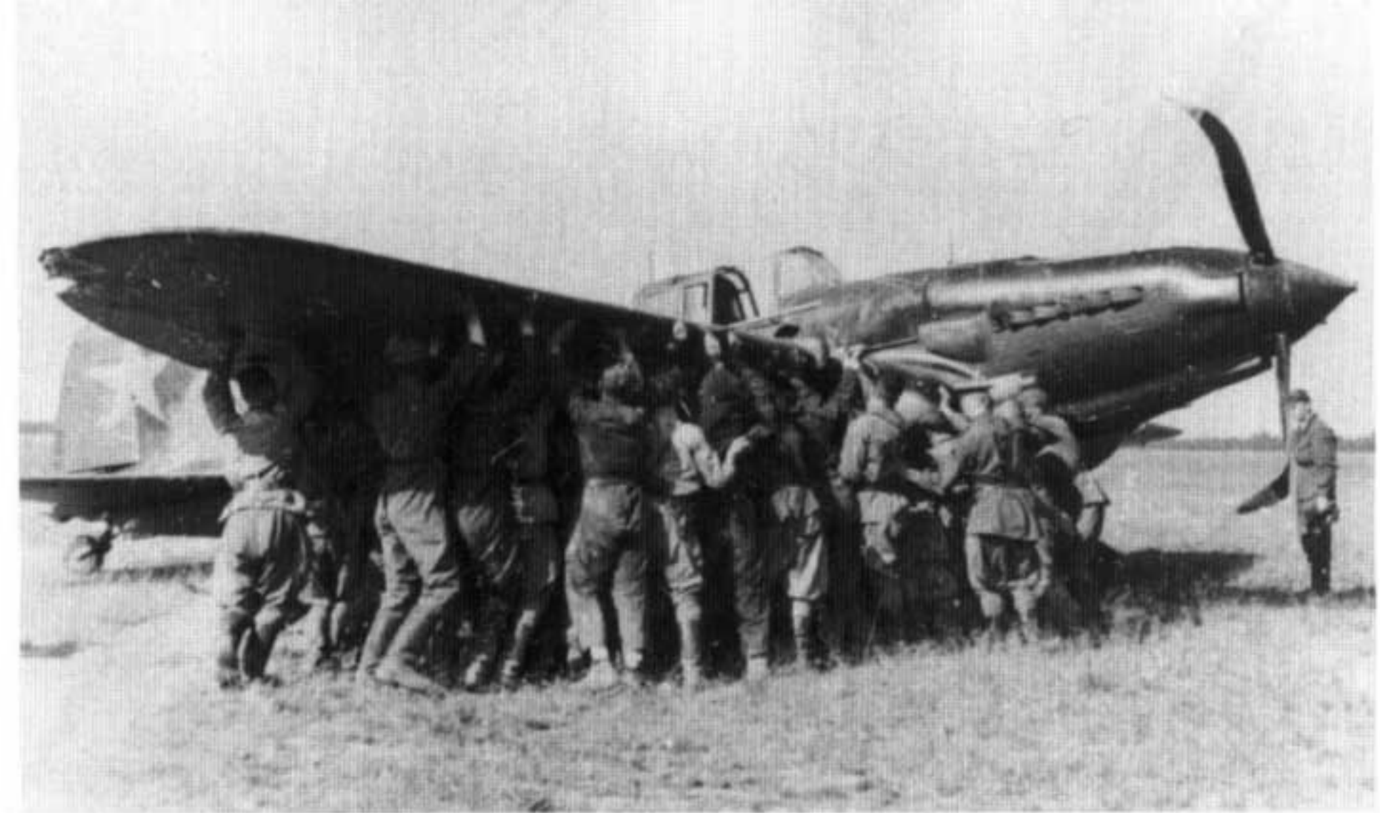
This Black-Green and Olive Drab Il-2M was lifted by ground crews so that the starboard landing gear could be lowered and locked down. The only visible damage was a bent wing tip and bent back propeller blades indicating that the engine was still running when the landing gear failed. (G. F. Petrov)
