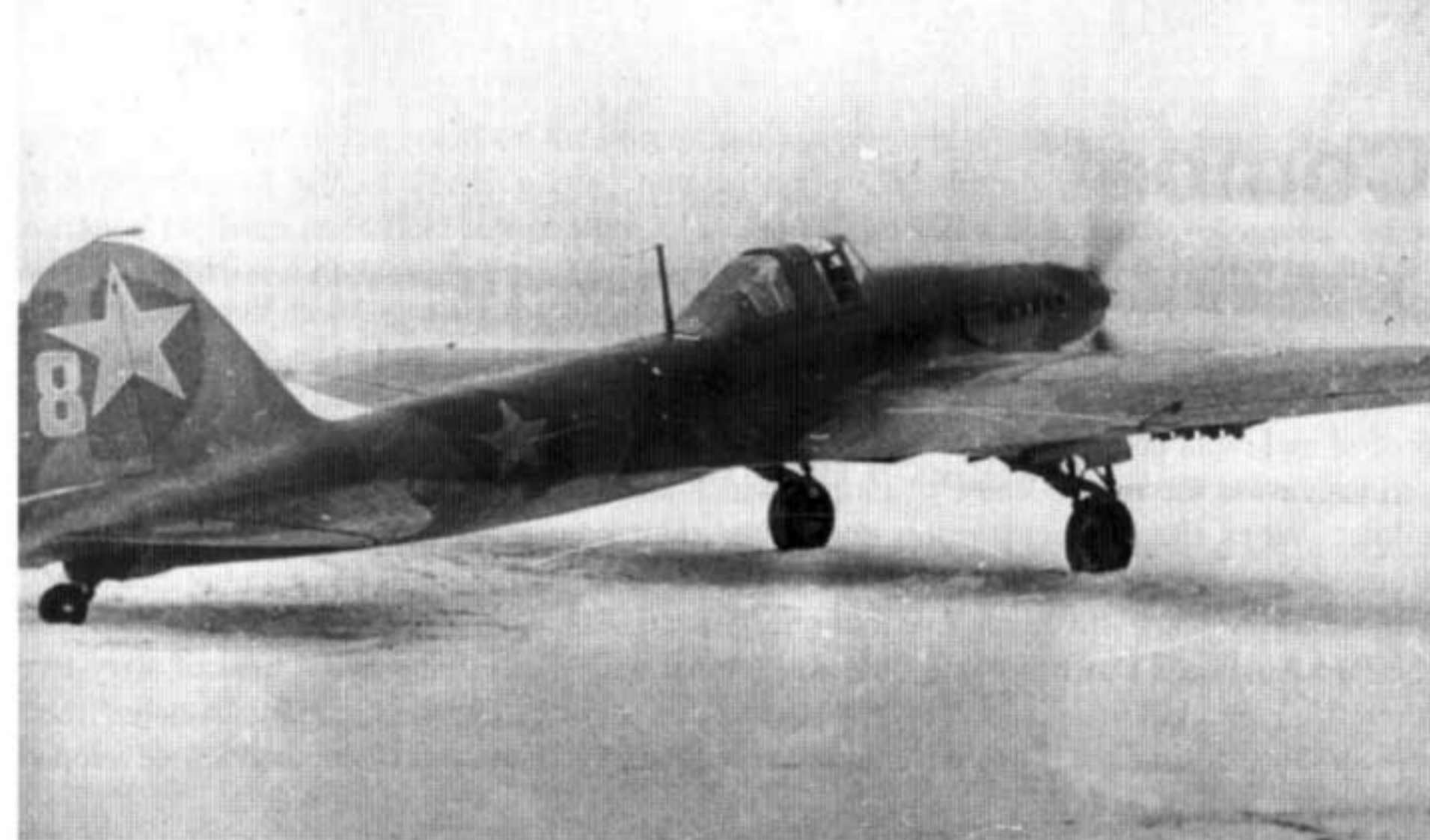
This Il-2, Red 8, of the 174th ShAP has a modified rear canopy section that has been fitted with extra armor. In addition, an armor plate was fitted to the top of the canopy frame. These features were introduced to enhance the survivability of the Il-2, since it had become clear that the single seat Il-2 was extremely vulnerable to fighter attacks from the rear. (G.F. Petrov)
