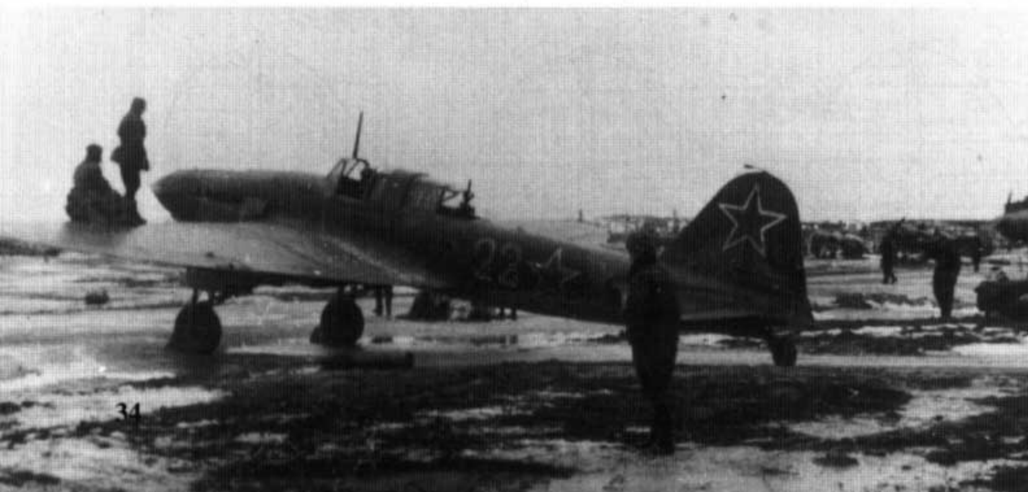
A few late production Il-2 Type 3s had the antenna mast fitted on the front cockpit canopy frame. This Il-2 Type 3, Yellow 22, shares a muddy airfield with some Lavochkin La-5FN fighters which served as the Stormovik's escort. (SHAA/B79 2254)
