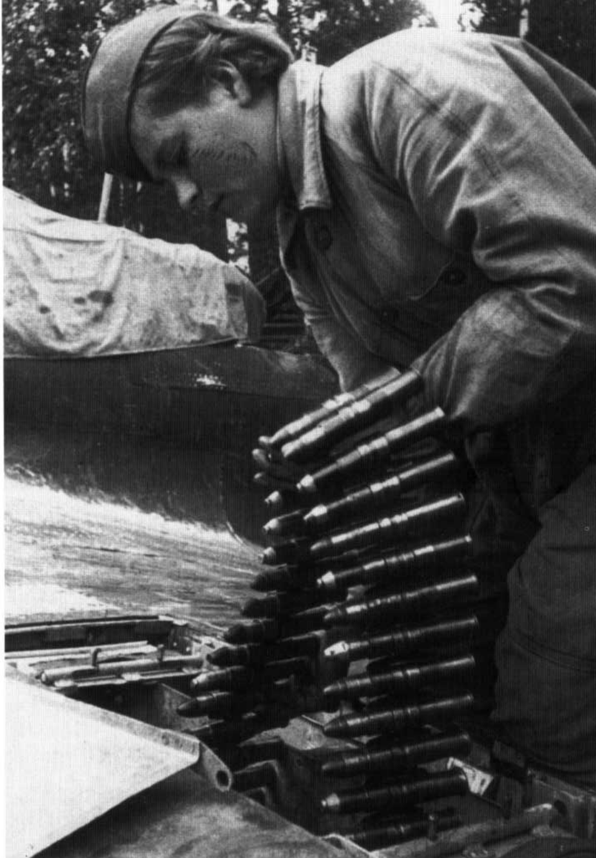
Private Klavdiya Yefimovna Danilova of the 3rd Squadron, 6th Guards Assault Aviation Regiment, loads 23mm rounds into the ammunition bay of the VYa-23 23mm cannon of an early Il-2 Type 3 on 24 July 1943. These rounds could penetrate armor up to 25mm thick at distances up to 1,300 feet (400 meters). Each ammunition bay could hold up to 300 rounds. (Ivan Ivanov)
