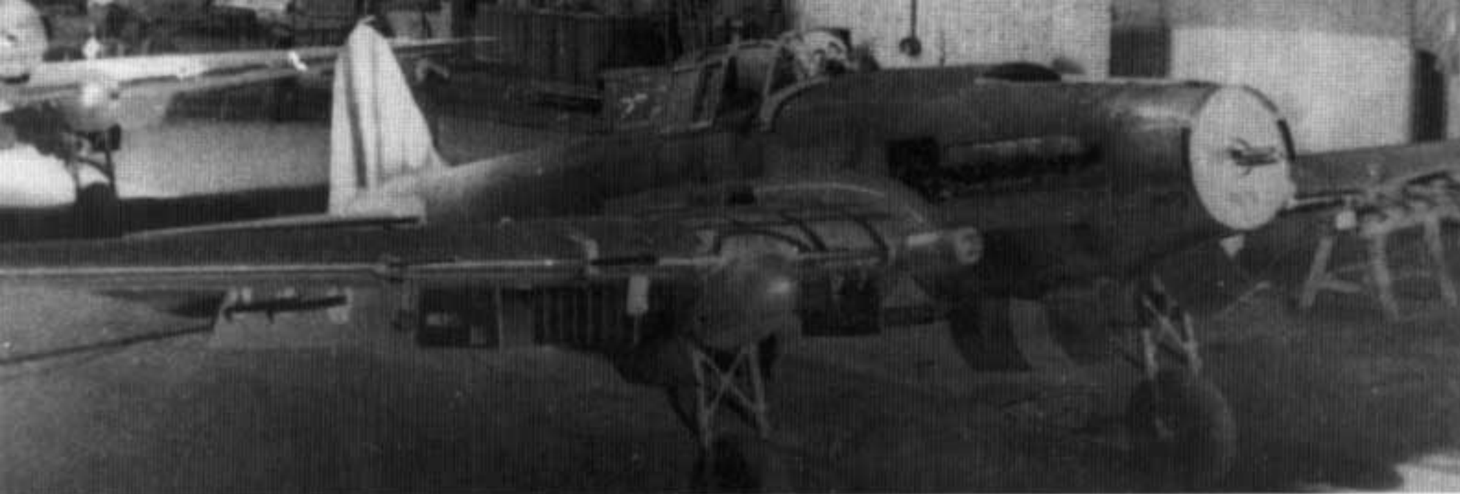
Early production Il-2 Type 3s undergo final assembly at State Aircraft Factory 18 at Kuibyshev during early 1943. This nearly completed Il-2 Type 3 has two rocket rails under the wing instead of the four carried by the single seat Il-2. The open doors under the wings are the bomb bay doors for the wing bomb bays. (G. F. Petrov)
