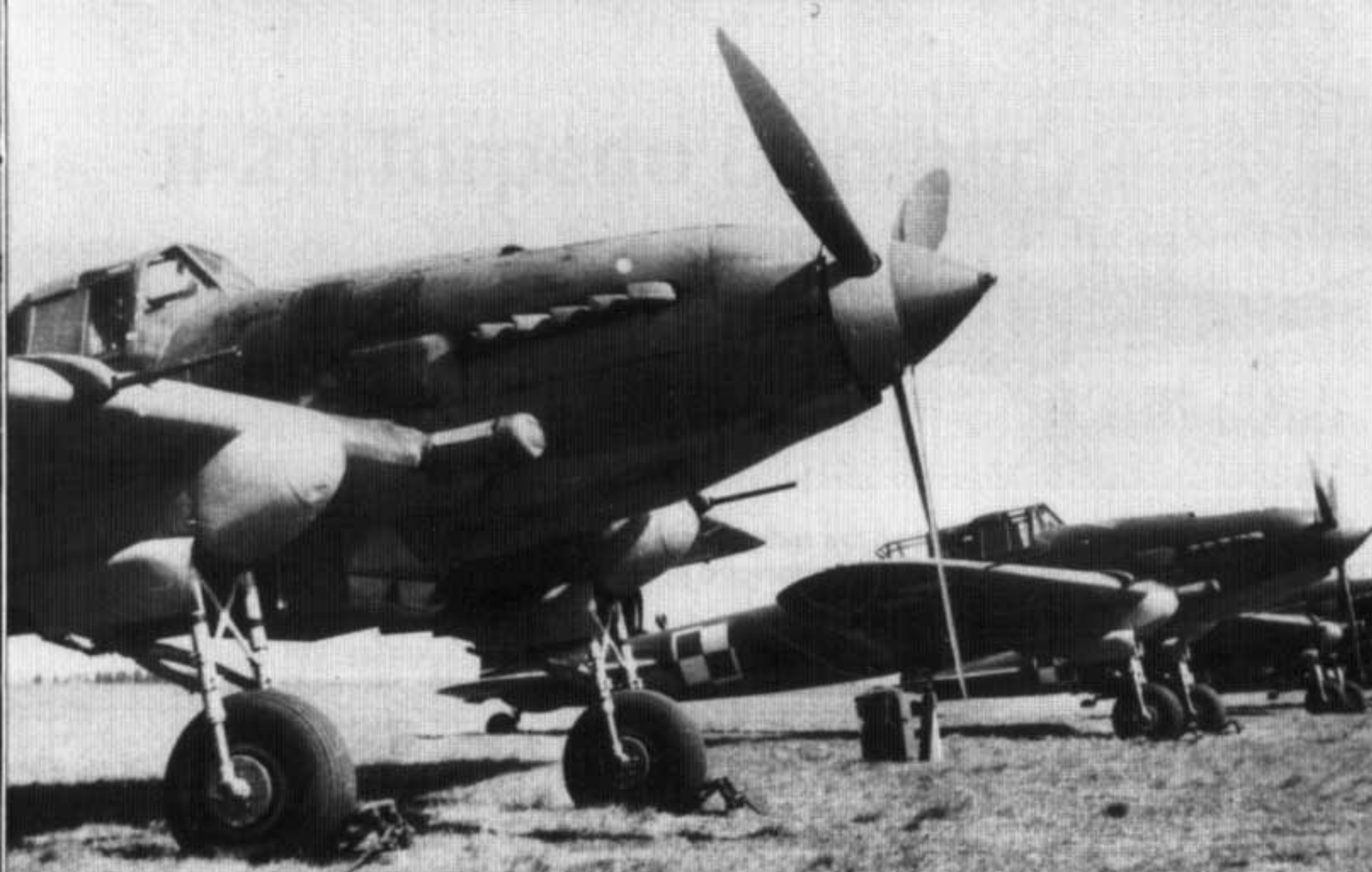
A line up of Polish Air Force Il-2 Type 3s. All of the aircraft have the late style cannon fairing. The second aircraft in the row is equipped with a direction finder loop antenna for a RPK-10 radio compass. (Andrzej Morgala)
