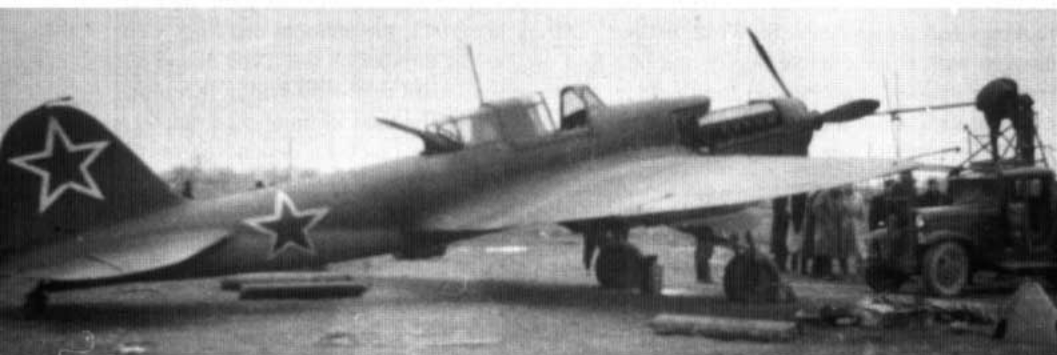
A few late production Il-2 Type 3s had the antenna mast fitted on the front cockpit canopy frame. This Il-2 Type 3, Yellow 22, shares a muddy airfield with some Lavochkin La-5FN fighters which served as the Stormovik's escort. (SHAA/B79 2254)
