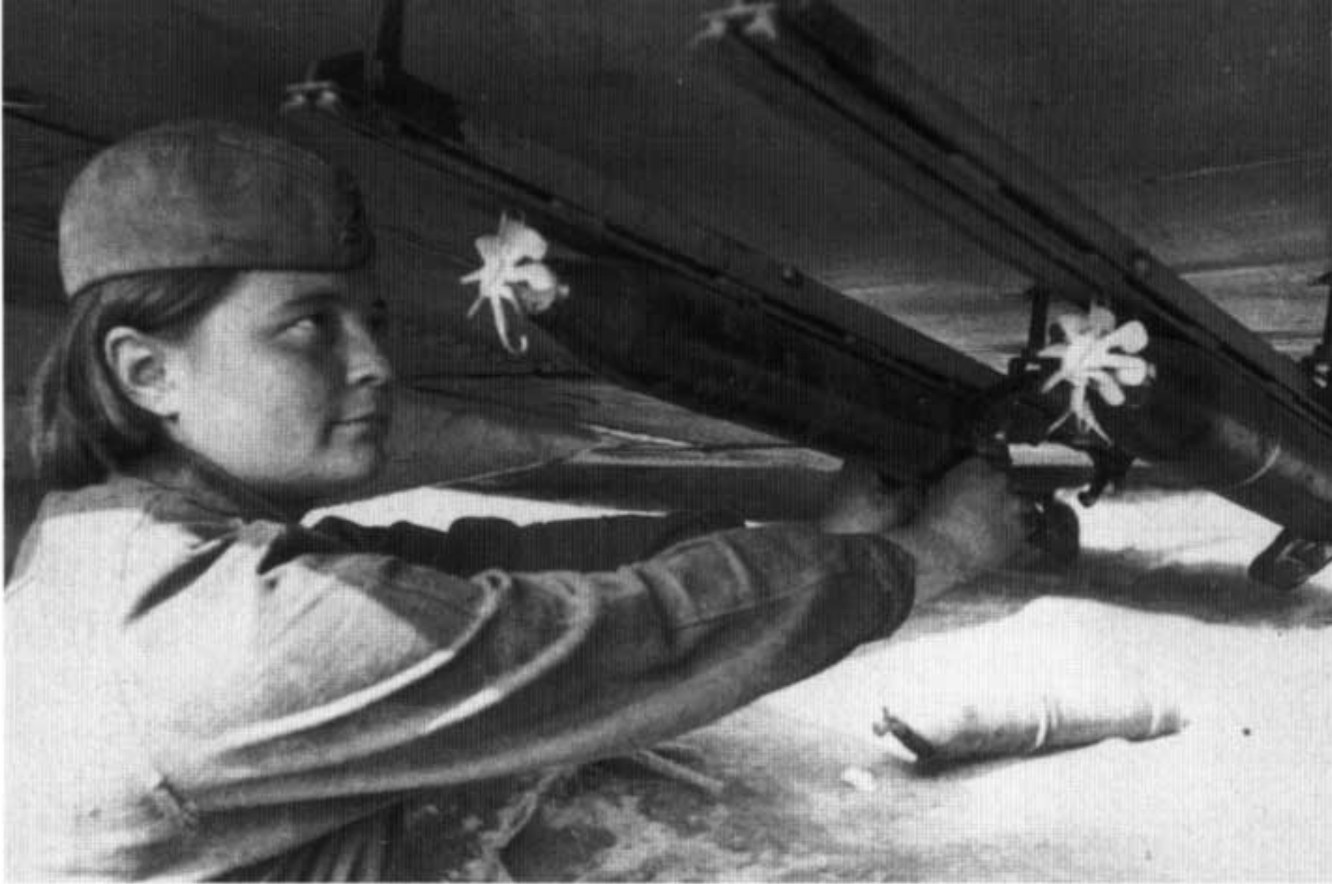
Private Yekaterina P. Butorina, of the 6th Assault Aviation Regiment, loads RS-82 rockets onto the Type RO underwing rocket rails of a Il-2 Type 3 during August of 1943. The unfaired rocket rails identify this as an early production Type 3. (Ivan Ivanov)
