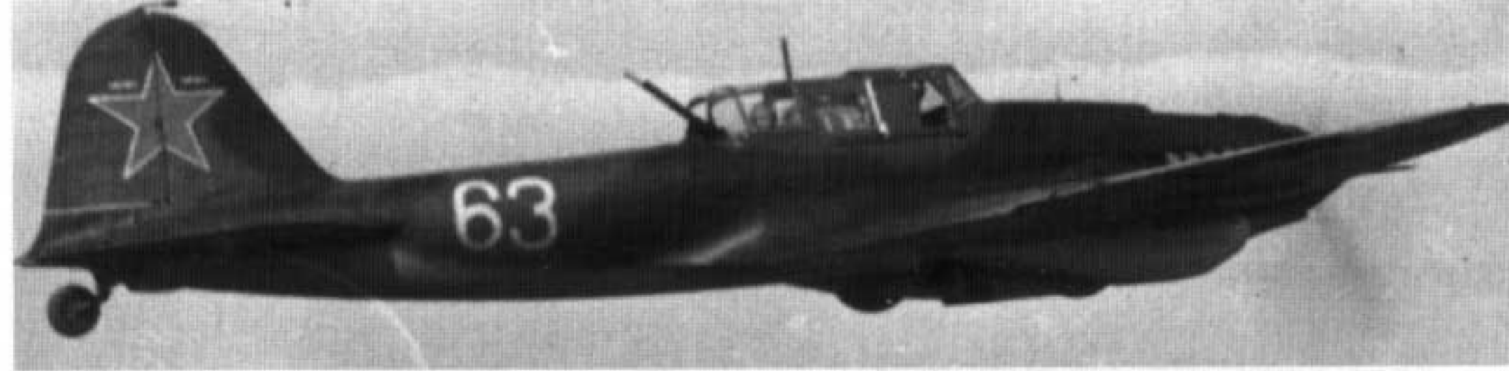
This Il-2 Type 3, White 63, is camouflaged in Black-Green and Olive Drab. The national marking is carried on the fin, but not on the rear fuselage. The White lettering above the star on the fin are the aircraft's serial numbers. (Carl-Fredrik Geust)
