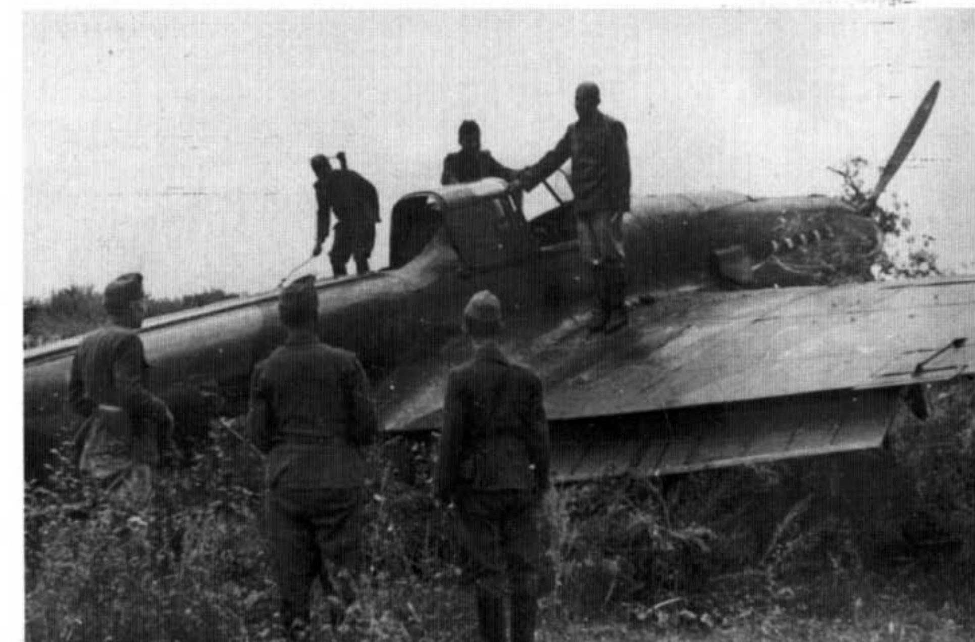
This Soviet pilot surrendered to Hungarian troops after coming down in the southern sector near Kharkov in the Summer of 1941. His Il-2 had the external reinforcing ribs on the rear fuselage first introduced as a field modification. The Red star on the fuselage had a thin Black outline. (George Punka)
