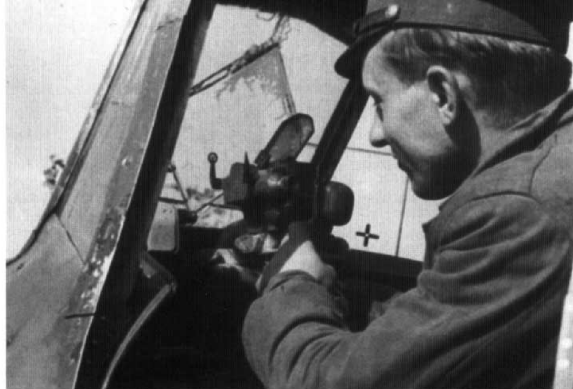
The VV-1 gun sight on some Polish Il-2 Type 3s was replaced by the more advanced PBP-1B gun sight, which was also used on the Yak-9D and Il-10. (Andrzej Morgala)
