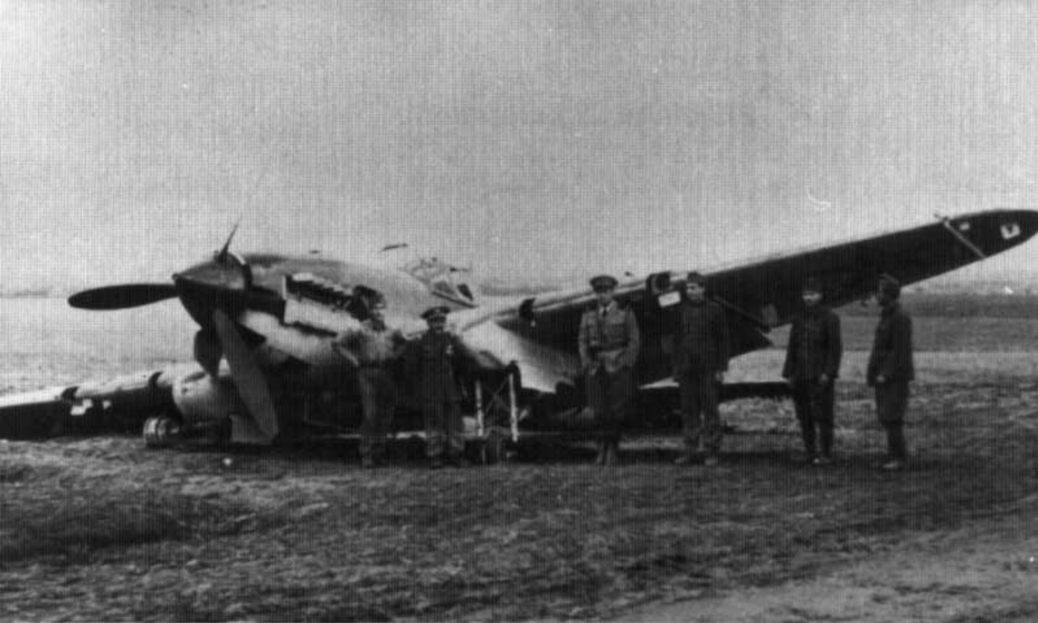
This pre-war production Il-2 was captured by Hungarian troops at Skala-Kurilovcze on 5 August 1941 during their rapid advance into the Ukraine. All the armament, the landing light and pitot tube were removed. The spinner and propeller were painted Black. (Attila Bonhardt)
