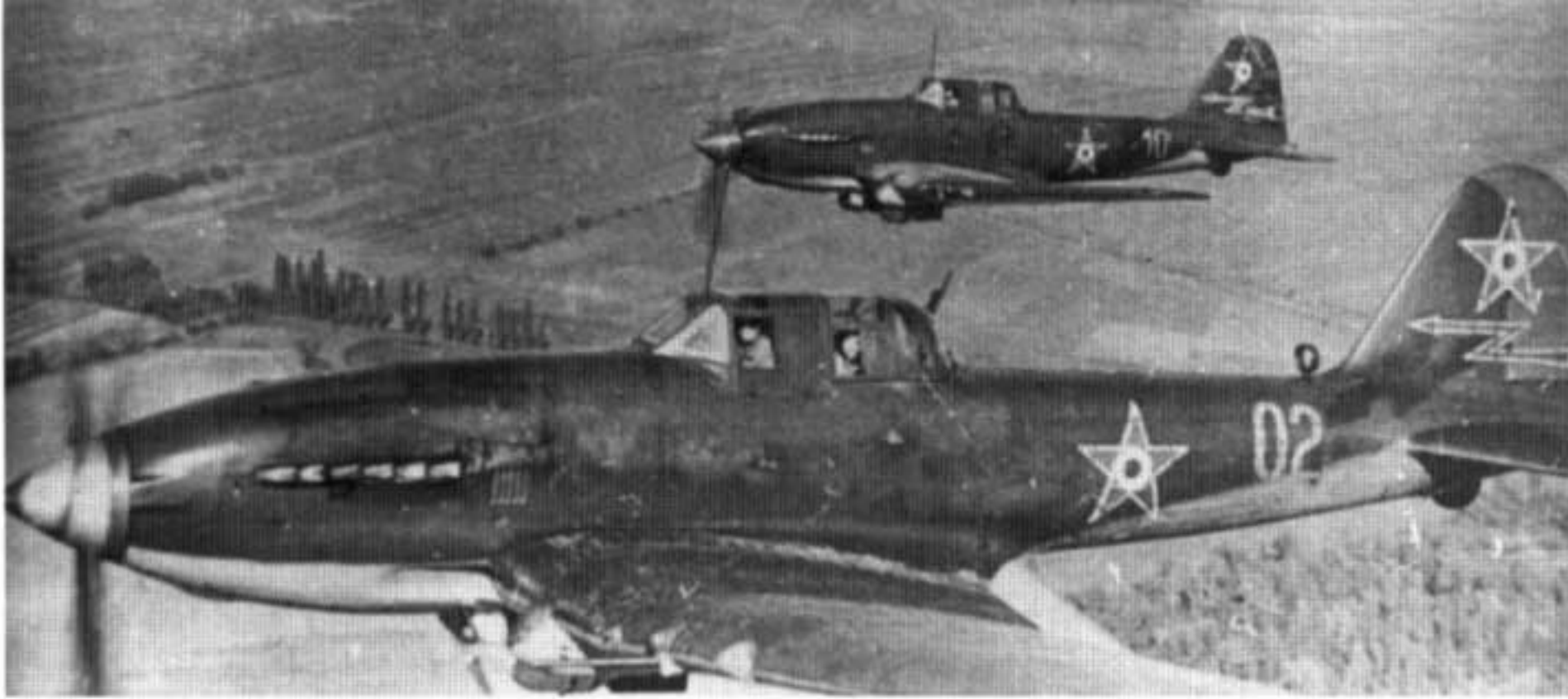
A pair Szekesfehervar-Tac based Il-10 Parduc (Panther) armed with FAB-100 bombs on their external bomb racks. The Red arrow on the fin had a thin White outline. The aircraft in the foreground had a Light Blue spinner while the aircraft in the background had an Olive-Green spinner. (George Punka)
