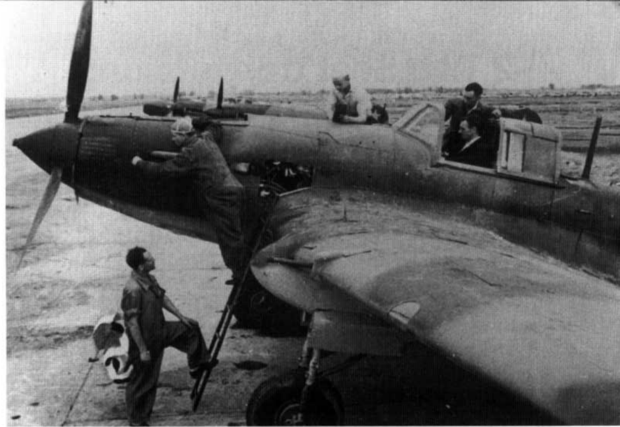
Il-2s, fresh off the assembly line, receive final checks at State Aircraft Factory 18 at Kuibyshev. The landing light on production Il-2s was mounted on the starboard wing only. (G.F. Petrov)
