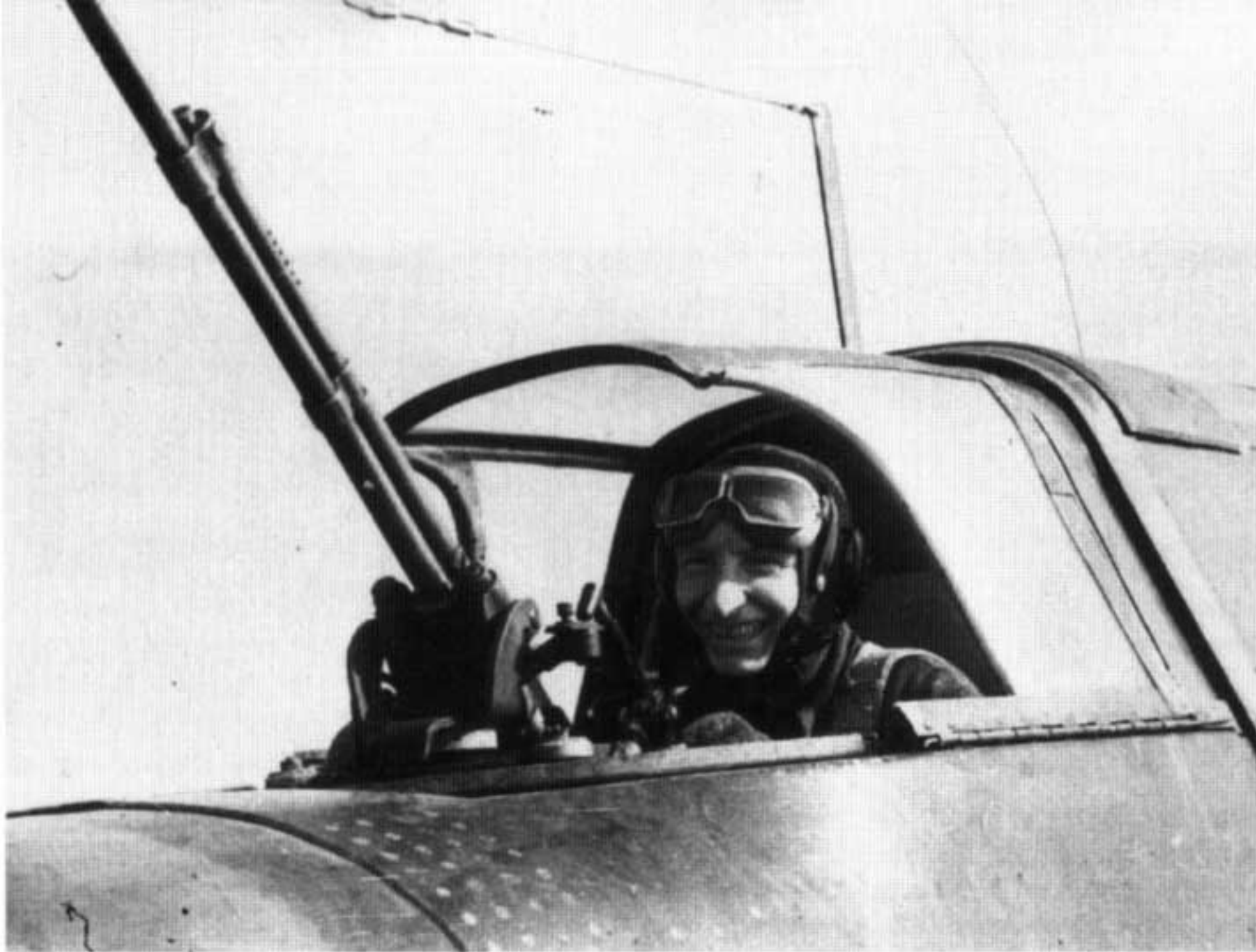
Some late production Il-2Ms, as well as early production Il-2 Type 3s had a portion of the rear canopy glazing cut back in order to improve the gunner's view. Such field modifications were common among Assault Aviation Regiments, as crews sought to improve their aircraft. (Ivan Ivanov)
