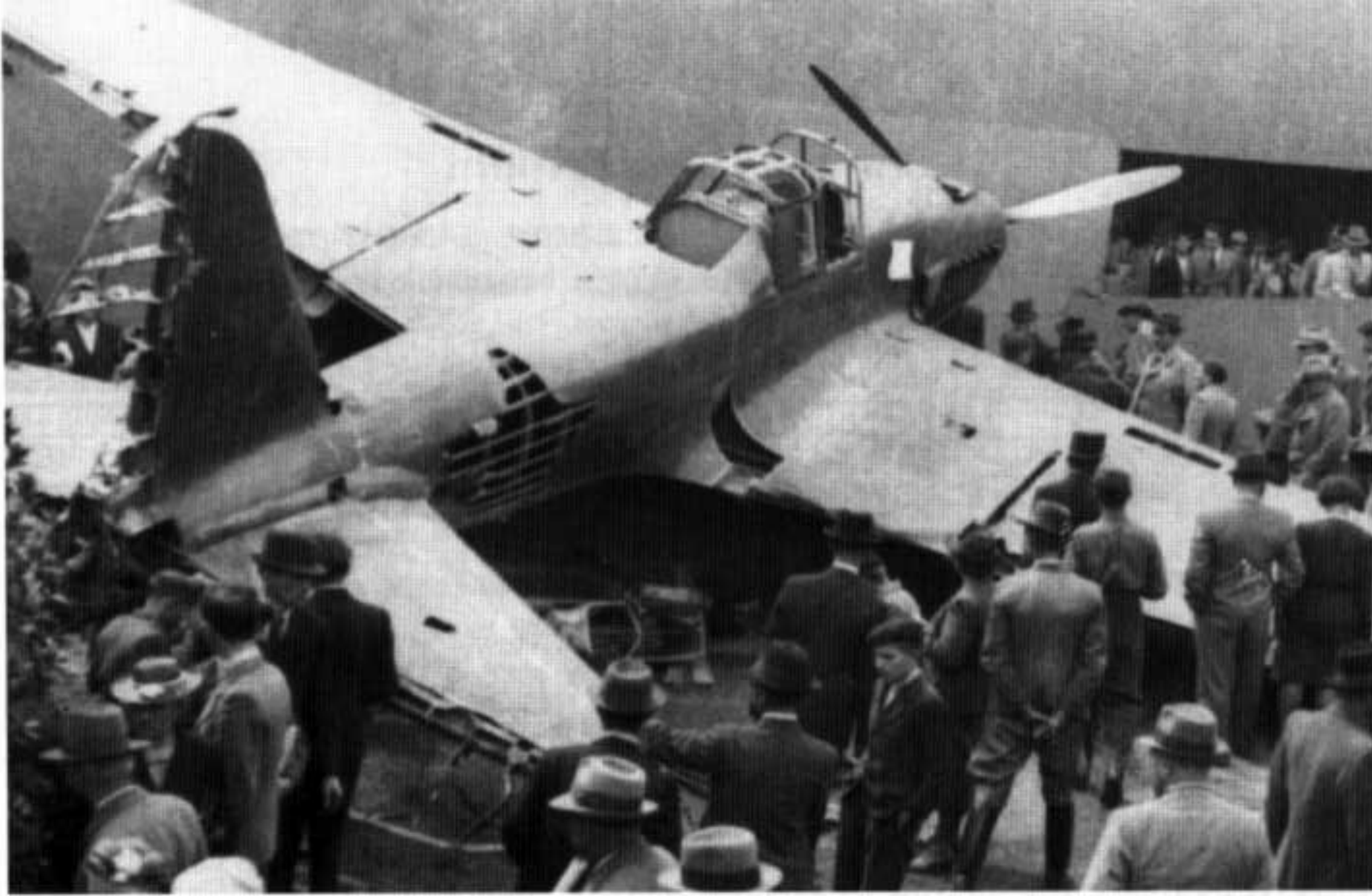
This Il-2 was part of an exhibition of war booty held in Budapest, Hungary during May of 1942. The national markings had been cut off from the fuselage and the fabric covering was gone from the control surfaces. The glazed rear canopy section and lack of an armor on the canopy top were typical of early production Il-2s. (O. Horvath)
