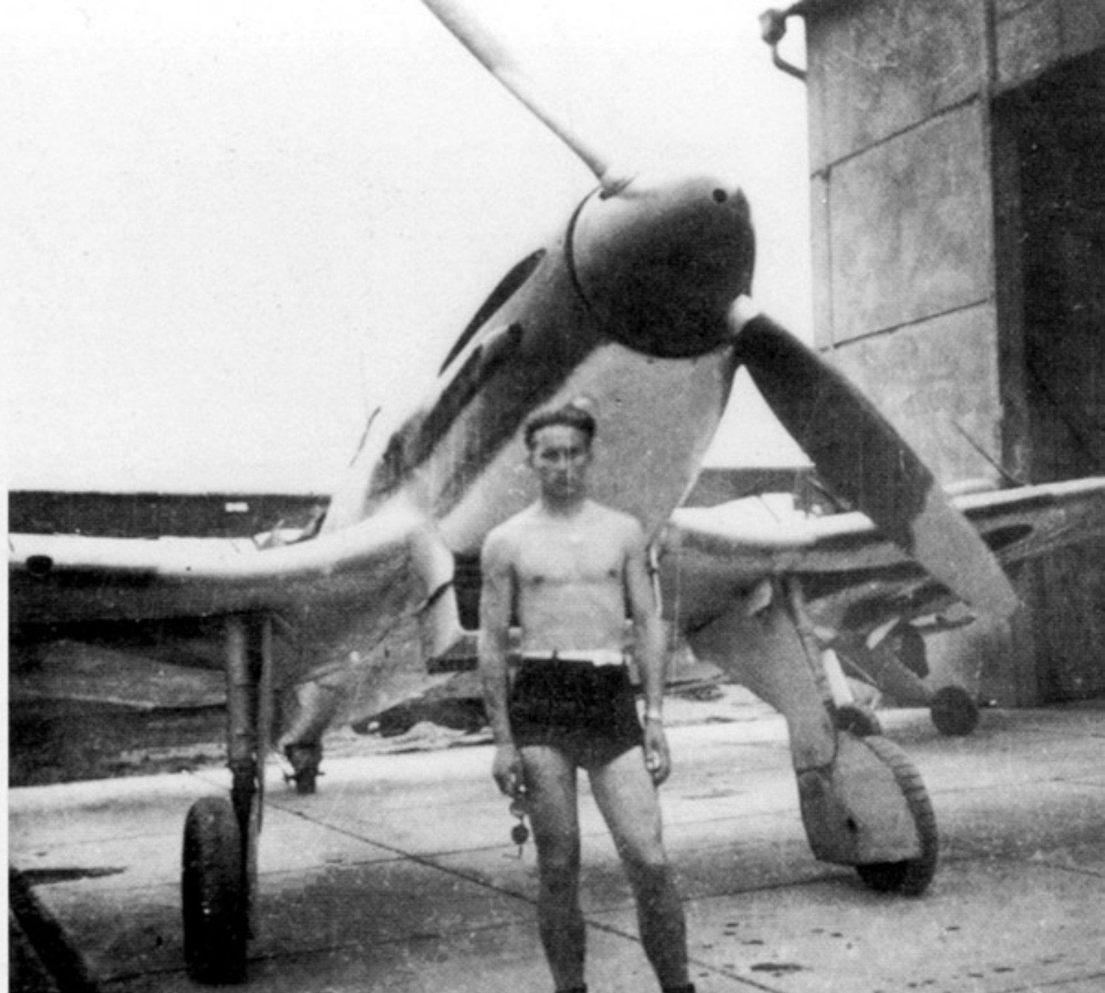
The propeller blades of this Hungarian He 112B were camouflaged. The aircraft in the background is a Bücker Bü 131 Jungmann trainer. (Jávor via Mujzer)
