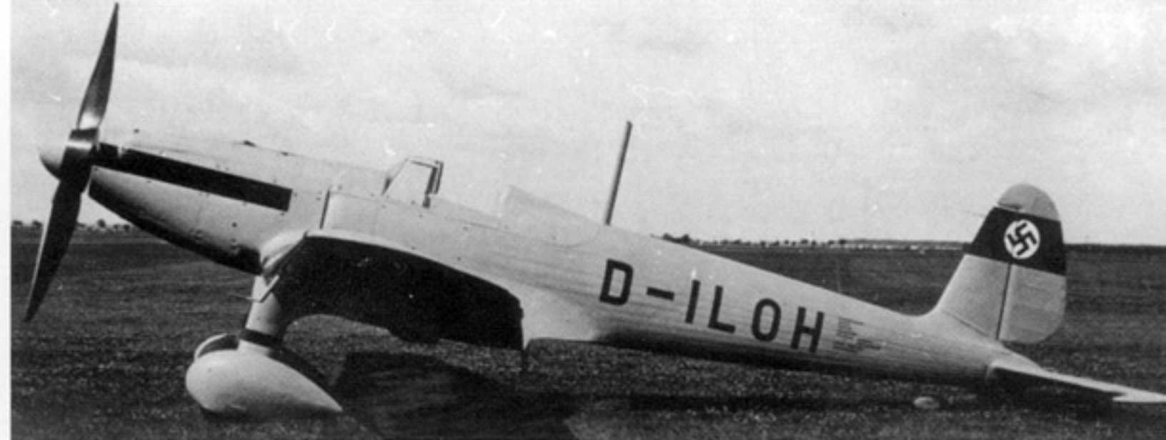
The Ar 80 V2 (D-ILOH) was of mixed wood and metal construction, with a fixed undercarriage. Equipped with a Rolls-Royce Kestrel V engine, it was considered an outsider from the very beginning. (Petrick)
