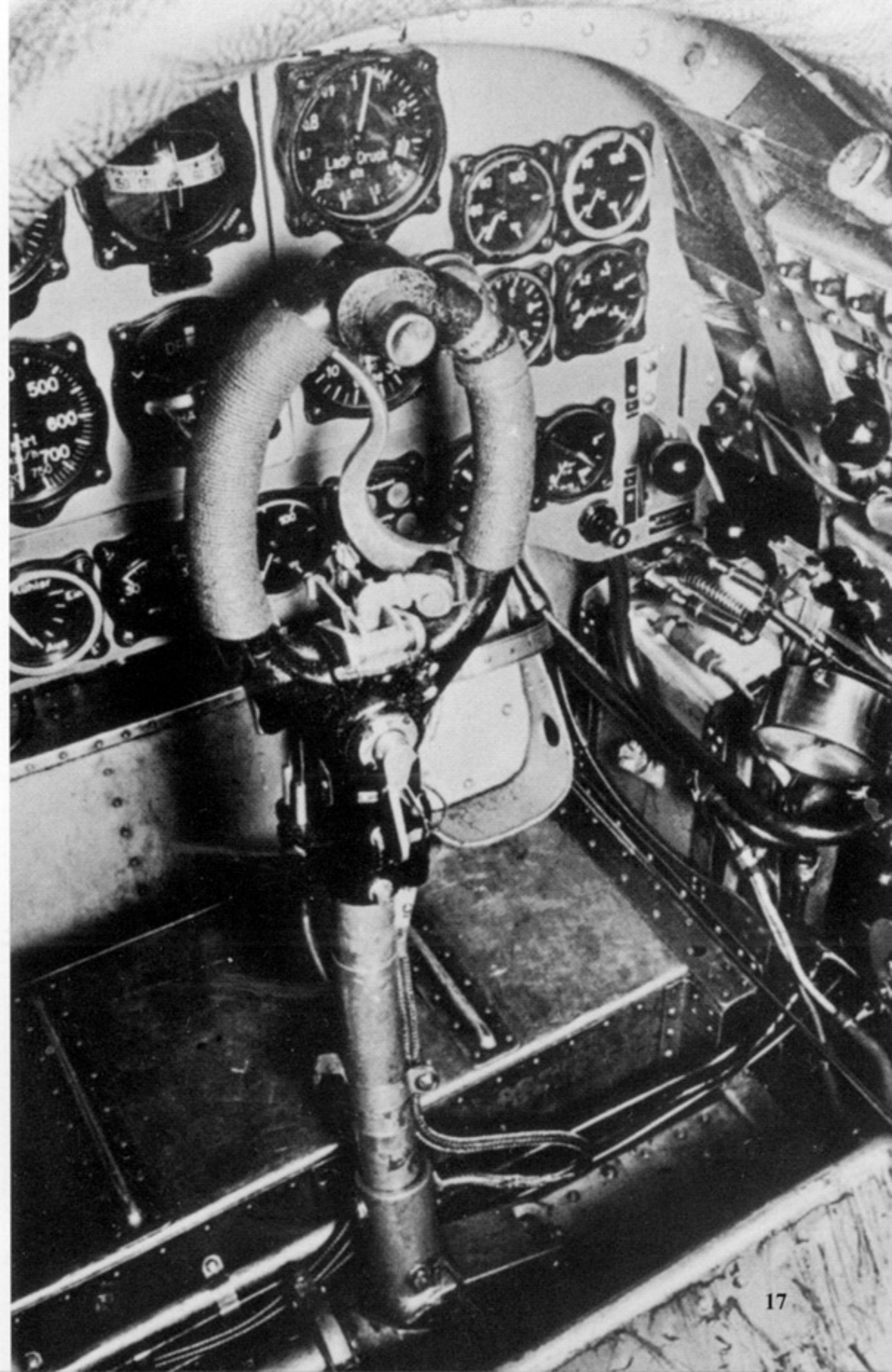
The right side of the He 112B cockpit. One of the rudder peddals is visible at left. On the cockpit sidewall are mounted various electrical boxes and switch panels. (Valtonen)
