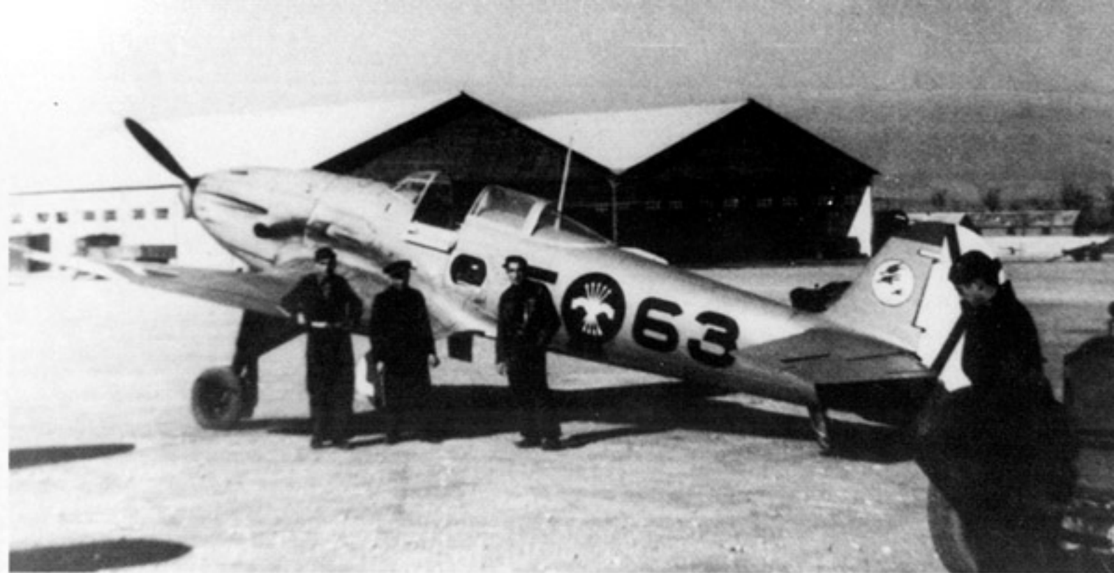
5•63 of 1ª Escuadrilla was probably an He 112B-2 with the fuel-injected Jumo 210Ga engine. The aircraft carries the insignia of 7ª Escuadra de Caza (7th Fighter Regiment) on the fin. The insignia consisted of three Blue aggressive birds on a White circle. (Desrousseau)
