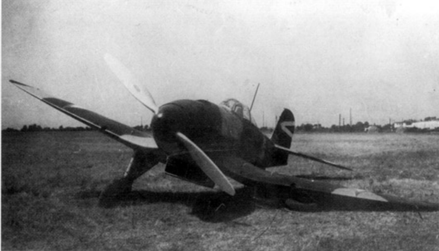
This Hungarian He 112B-1, V.303, had the port landing gear fail on landing during the late Summer of 1941. The two-blade all metal propeller on this He 112 was left unpainted. (Kovács)
