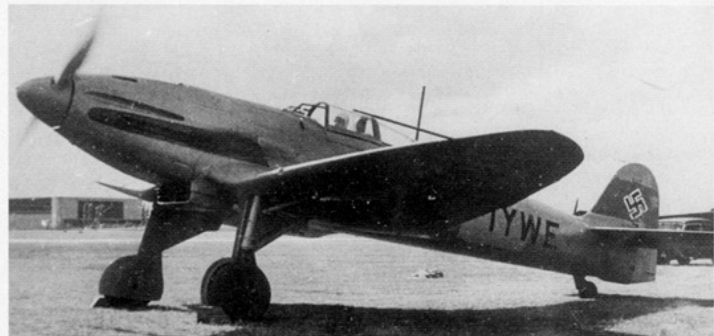
A subtle maneuver of the German propaganda machine. A picture of the original He 112A-01, D-ISJY was heavily retouched to represent a completely different aircraft with a "new" fuselage, tail and fitted with an enclosed cockpit. Additionally, the radiator bath and engine cowling were also redrawn. The pictures were largely publicized during the war in various aeronautical revues. (de Celis Borrell)
