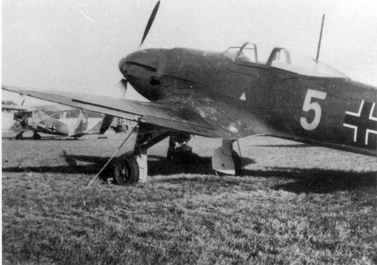
A He 112B-1, Yellow 5, at Karlsbad during October of 1938. The aircraft in the background is an Arado Ar 68E-1, White 8, of III./JG 132. The Yellow triangle beneath the cockpit indicates the location of the fuel filler cap and the fuel octane number. (Matthiesen)
