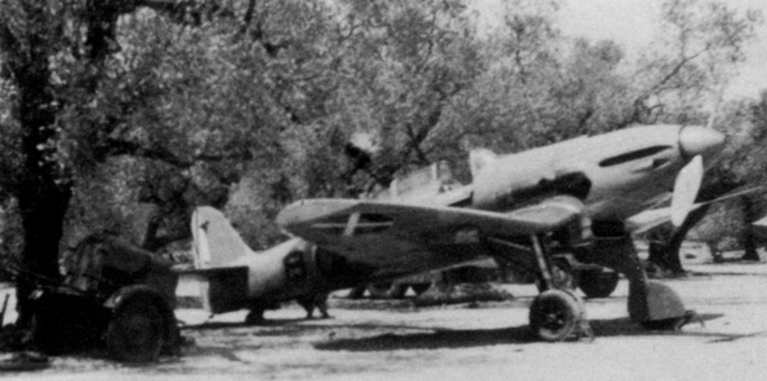
The He 112 V9 on the edge of a front-line airfield during the Summer of 1938. By this time the Hakenkreuz in the fuselage roundel had been deleted. The small wheel well doors were removed during field service. A Messerschmitt Bf 109 Bipalas is visible in the background hidden under the trees. (Petrick)
