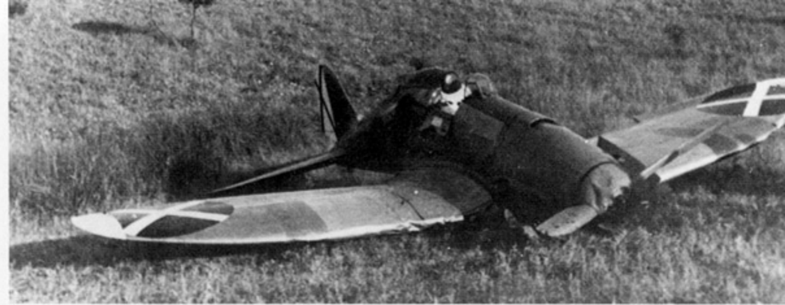
The Kanonenvogel lies in a field with its back broken. The He 112 V6 met its fate following a crash landing at Escalona del Prado (Toledo) on 19 July 1937. Before landing the engine was shut down and only one of the two propeller blades was bent. The aircraft carries unusually large Nationalist markings applied on the wing upper surfaces. (EA-IHCA, via Borrell)
