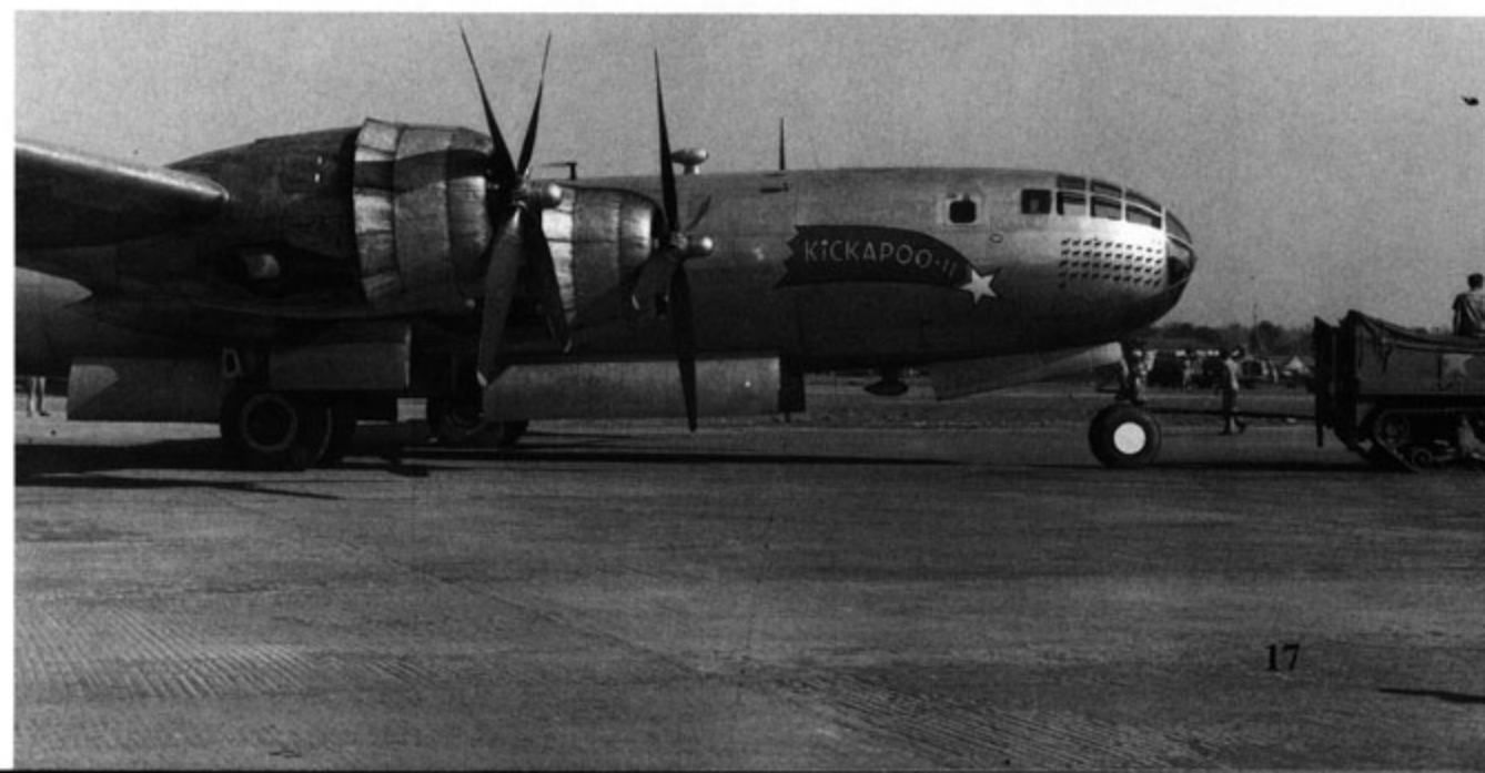
KICKAPOO-II, a 468th BG B-29 tanker with 41 missions over The Hump, is pulled to its parking spot by an Army M3 halftrack. B-29 tankers were devoid of all armament except tail guns. (Dave Lucabaugh)
