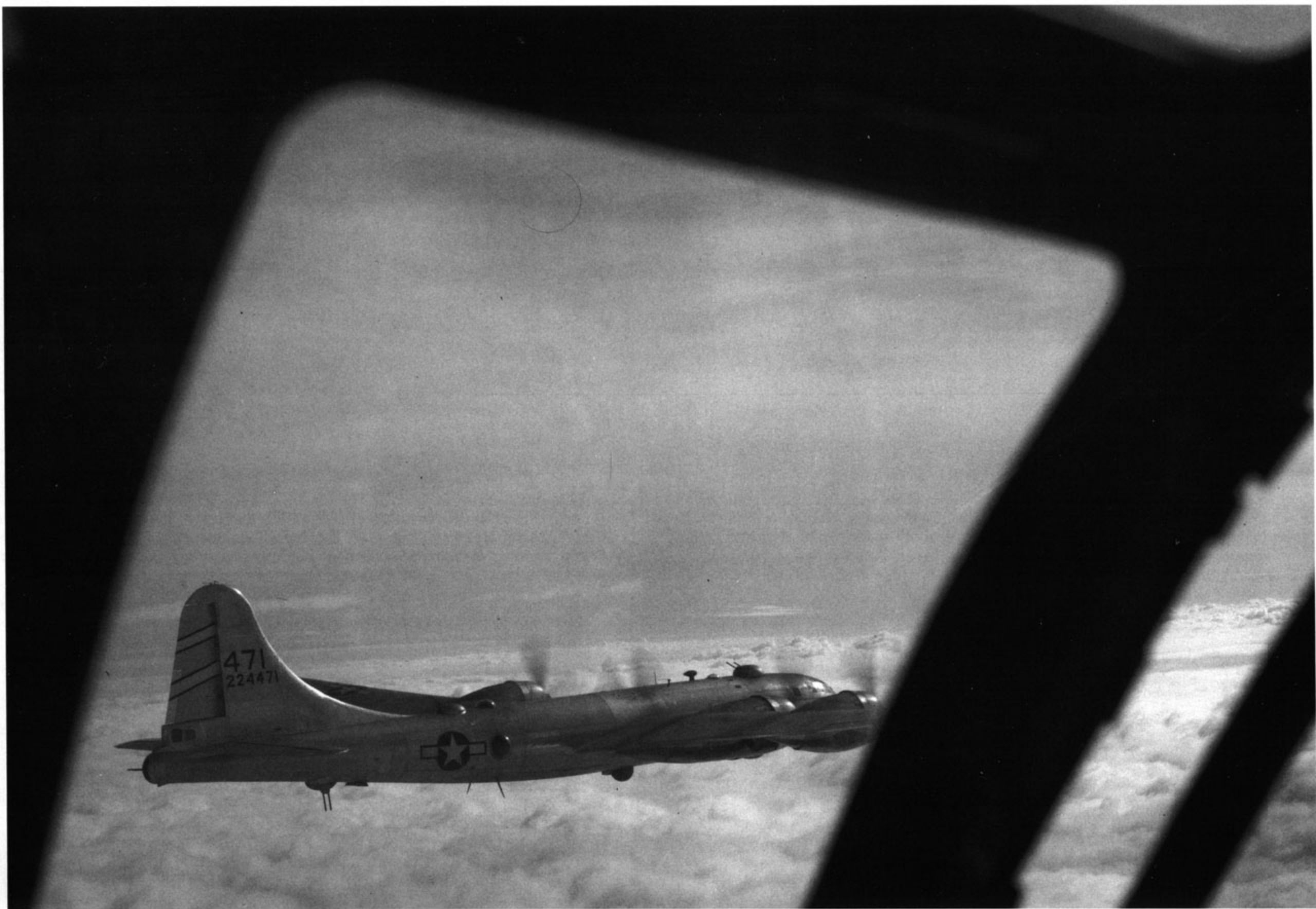
Looking through the pilots side window at another 468th Bomb Group Superfortress enroute to Anshan, Manchuria on 8 September 1944. The APQ-13 thirty inch radome is extended from the bottom of the fuselage. (Dave Lucabaugh)
