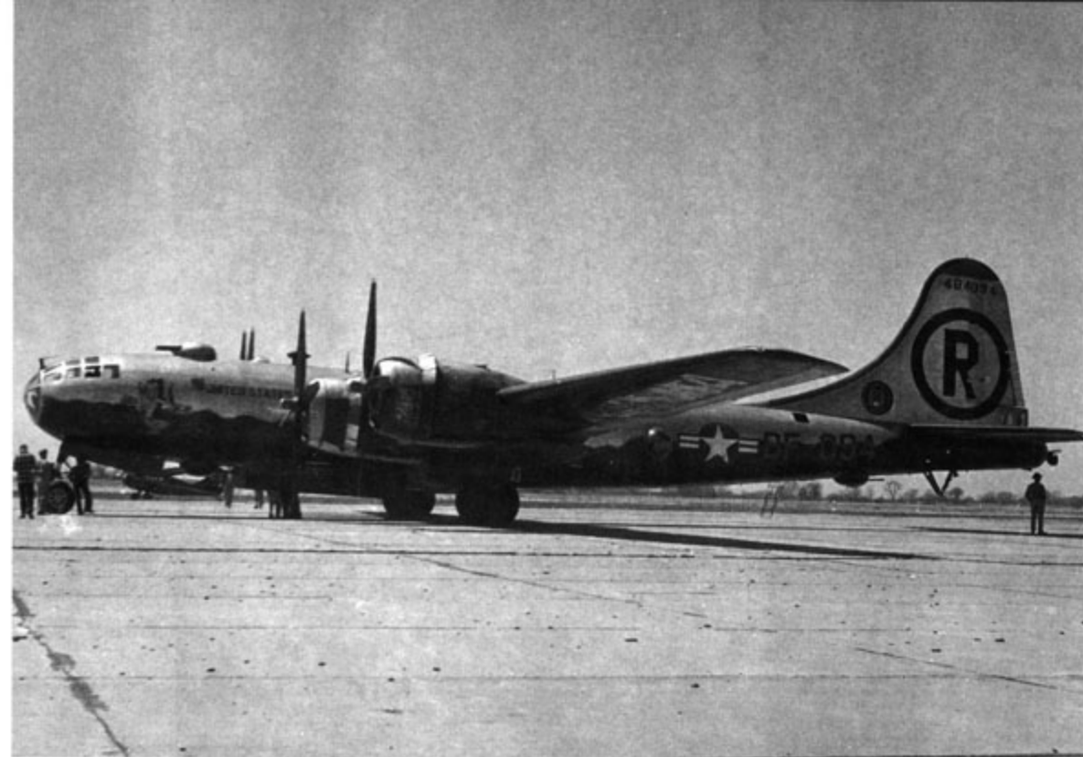
Pistol Packin' Mama, a B-29B assigned to the 28th BG of the 15th Air Force at Rapid City, SD, has its buzz number in Red over the Black camouflage. The APQ-15 gun laying radar can be seen silhouetted at the tail turret. (Robert Mikesh)
