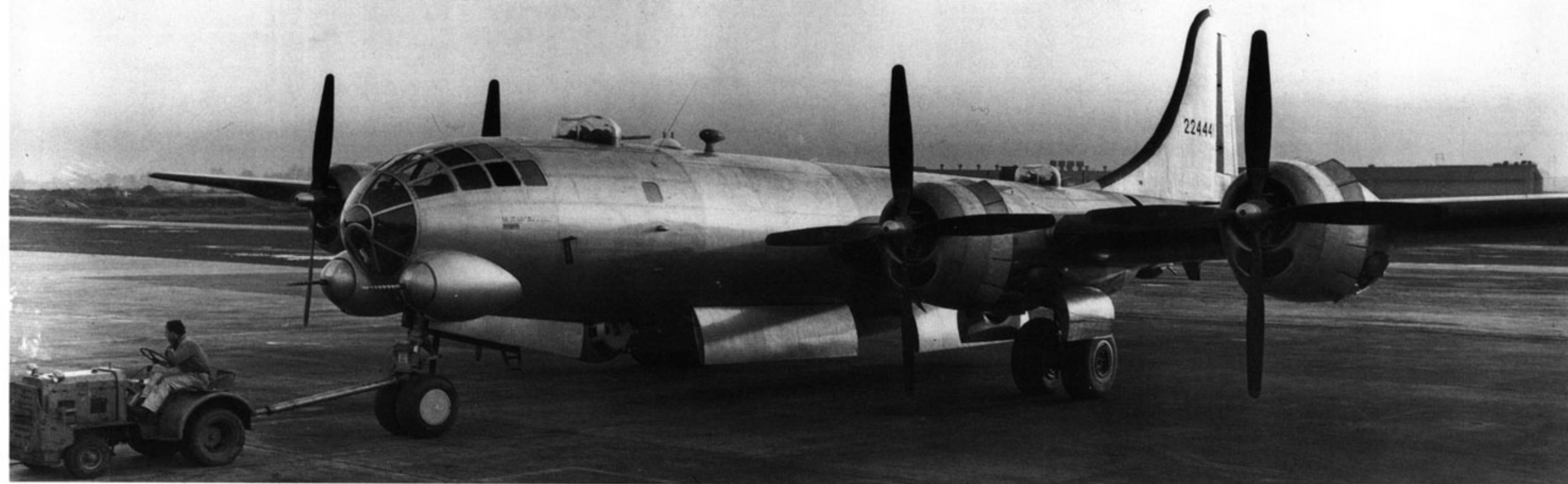
Many different armament variations were developed and tested for the B-29. This Superfortress has manned B-17 upper turrets, with manned ball turrets under the fuse-
