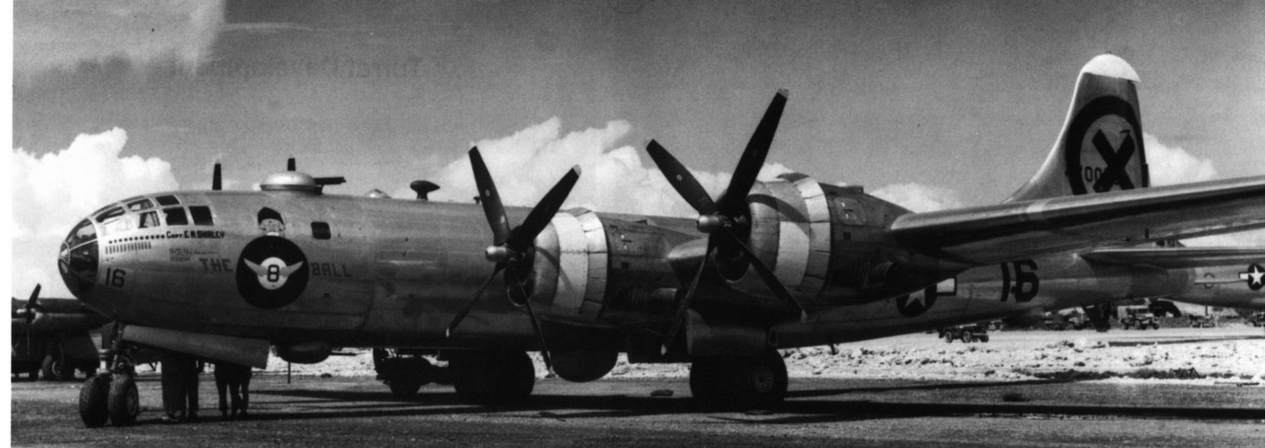
(Below) This 19th BG B-29 carries only the twin .50 caliber machine guns common to 21st Bomber Command aircraft. (Ron Witt)
