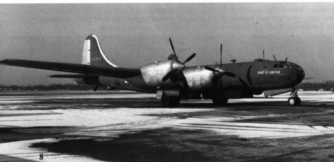
(Below) The first YB-29 was modified by General Motors with the installation of Allison V-3420-11, twenty-four cylinder liquid cooled engines and re-designated the XB-39-GM. A V-3420 engine was two 12 cylinder V-1710 engines mated together. (David Menard)
