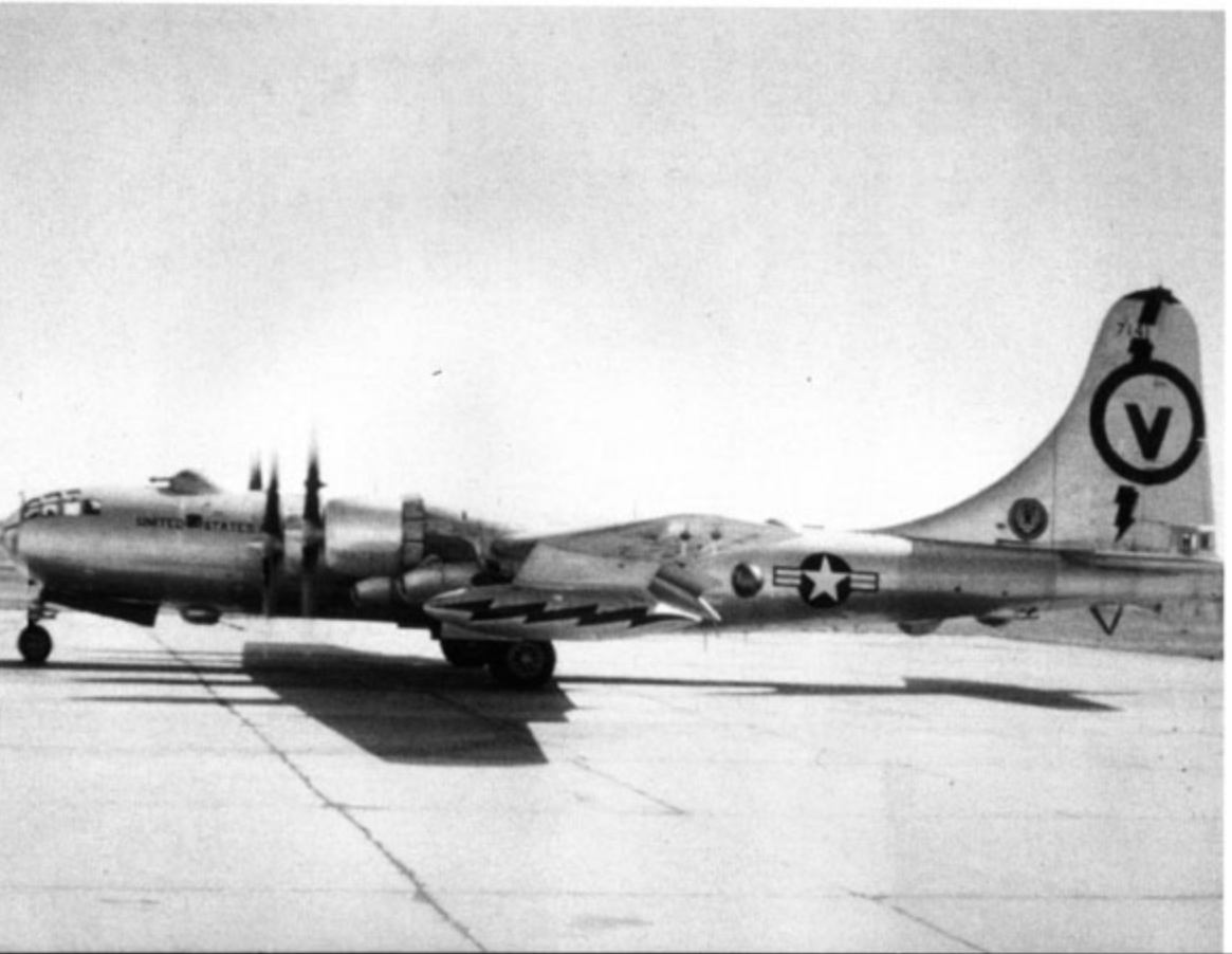
An RB-50F from the 55th Strategic Reconnaissance Wing based at Forbes AFB, Kansas in 1953. The RB-50F had additional ELINT antennas, including a large radome under the rear fuselage. (Andy Meyers)
