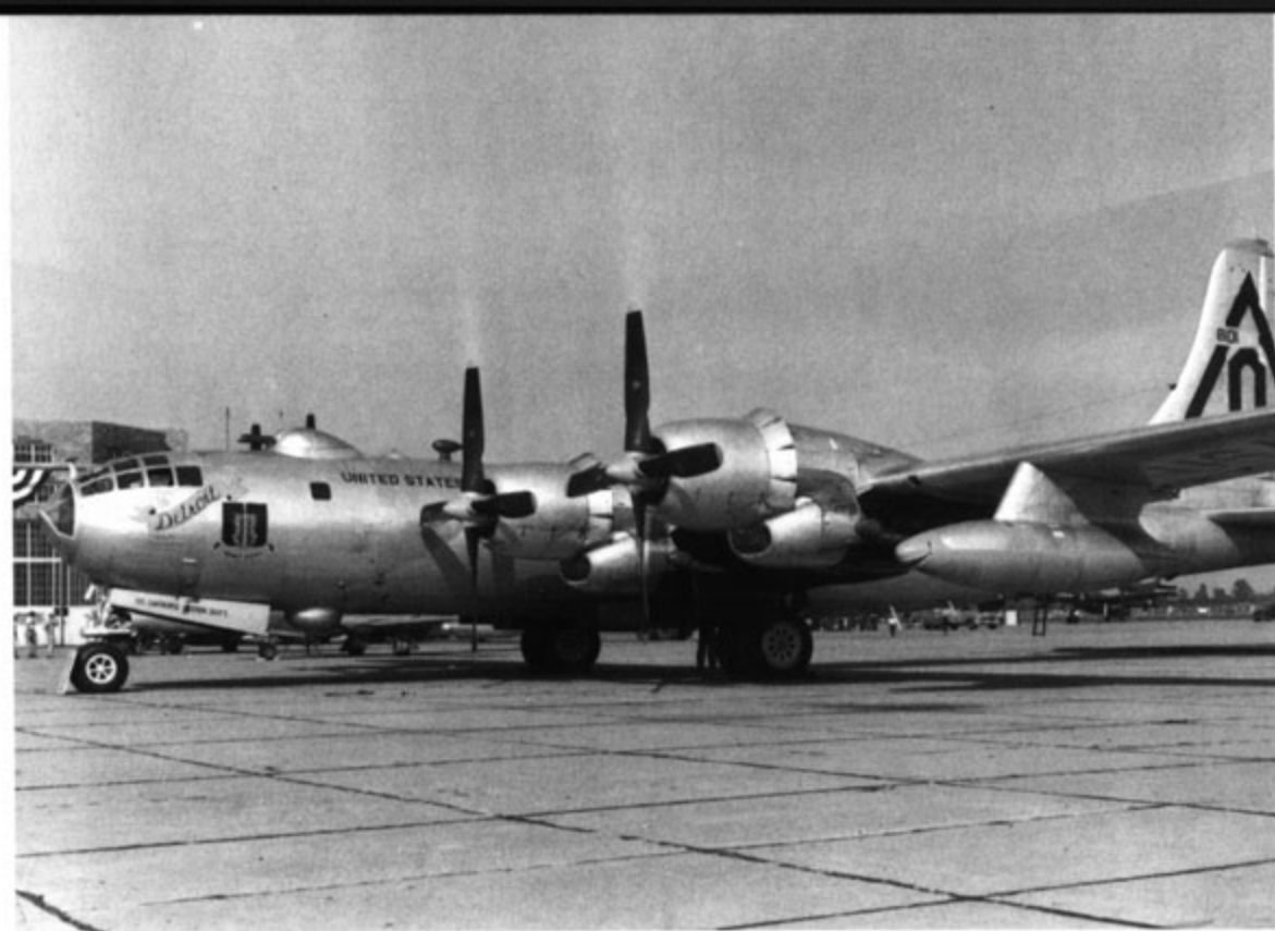
Detroit , a B-50D from the 97th Bomb Wing at Biggs AFB, TX. The B-50D featured the one piece bombardier nose perspex, and an In Flight Refueling receptacle behind the canopy to connect with the Boeing Flying Boom. A shark mouth has been painted on the wing tank. (Peter Bowers)
