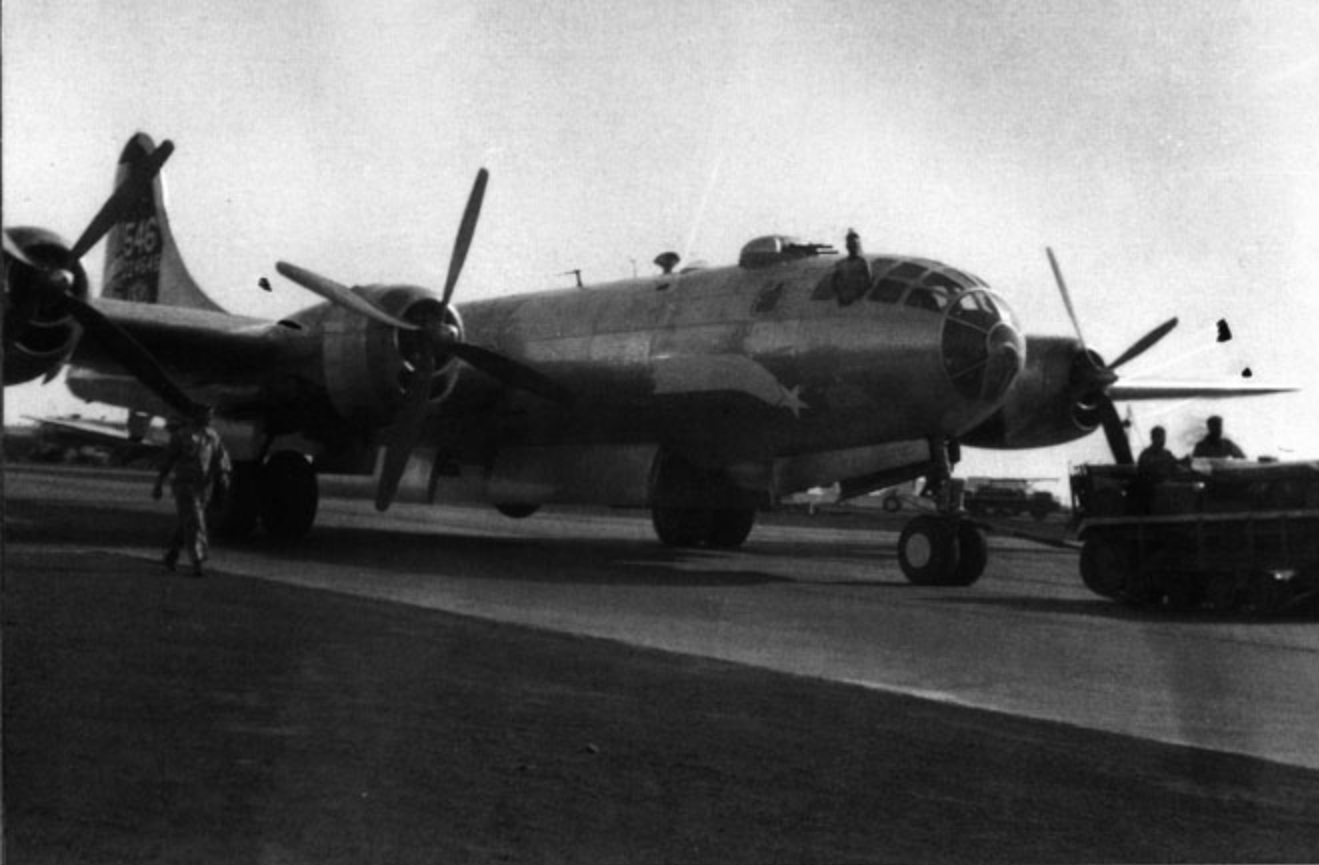
A B-29 from the 468th Bomb Group is pulled to its parking spot by a tow tractor at Kharagpur, India. All aircraft from B-29-5 onward were delivered in Natural Metal. The unit marking on the nose of the aircraft is unfinished. (James Eckert)
