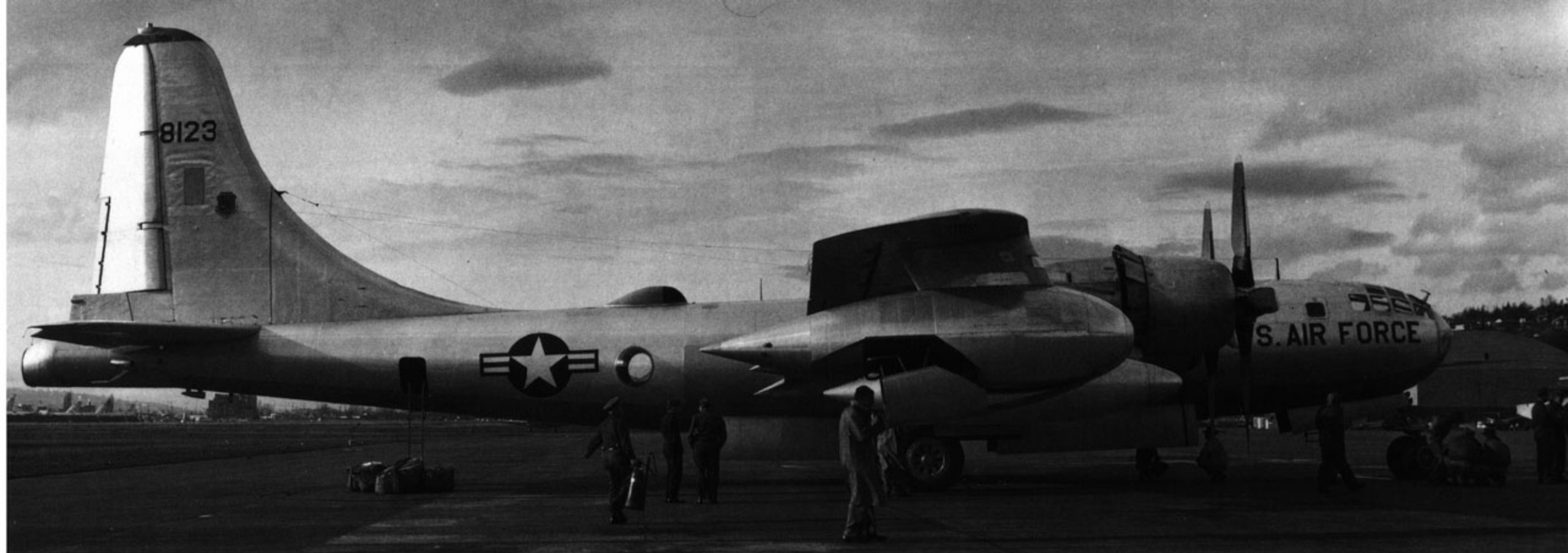
(Above) The KB-50J tanker had three inflight refueling systems — one in the rear fuselage, and one in each wing tip tank assembly. KB-50Js were delivered to Tactical Air Command beginning in 1958. (Peter Bowers)
