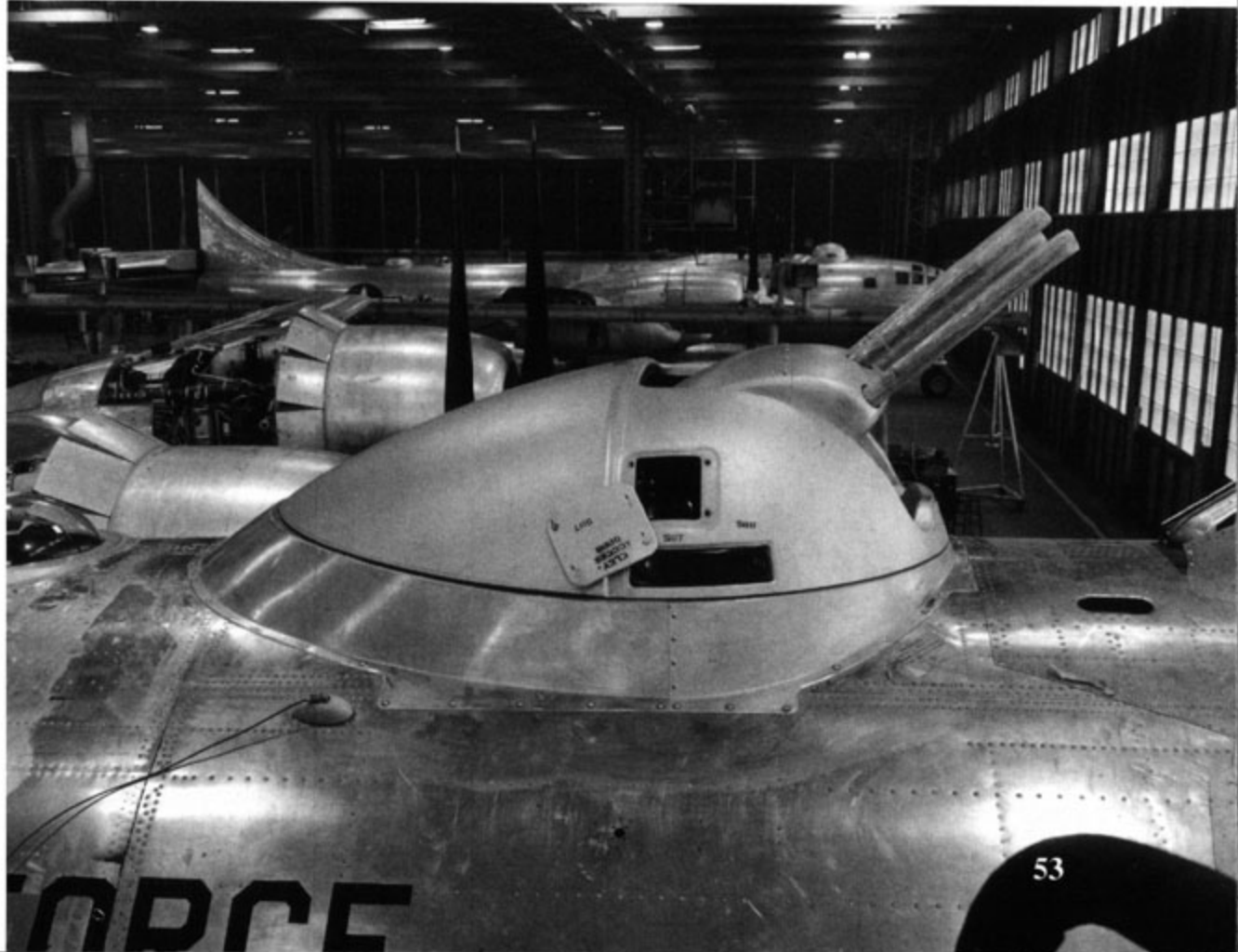
(Below) The streamlined four gun top turret was adopted for the late production B-29A and all variants of the B-50. The open inflight refueling door can almost be seen in front of the turret. (Peter Bowers)
