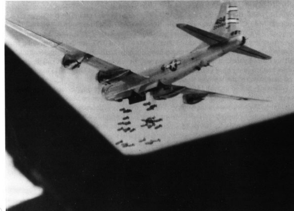
"MARY ANN", a 468th Bomb Group B-29 Superfortress unloads 500 pound bombs on Haito, Formosa on 16 October 1944. The B-29 had a maximum capacity of 10,000 pounds of bombs, the largest bomb load carried by any American aircraft in World War Two. (Ernie McDowell)
