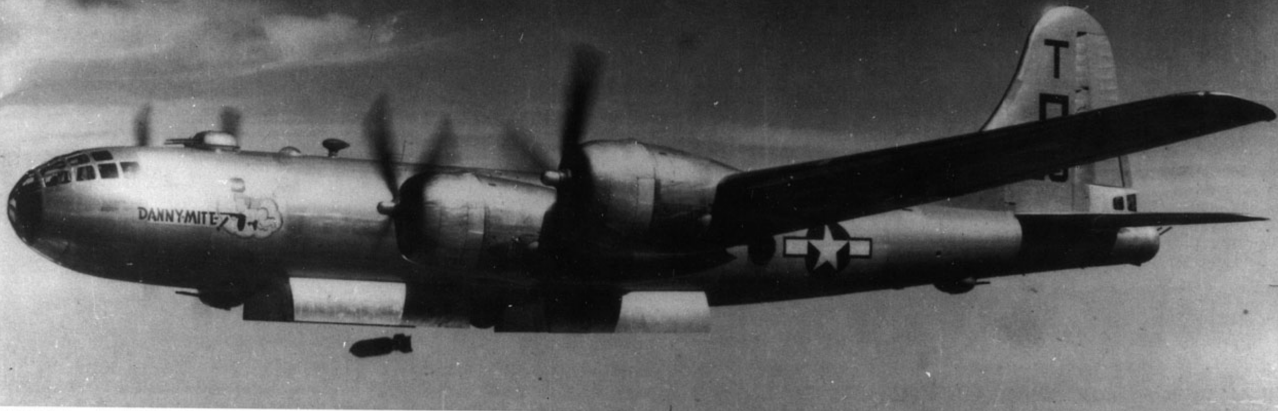
DANNY MITE , a 498th BG B-29 (44-69777), unloads 500 pound HE bombs. An intervalometer alternated the bomb drops from both bomb bays to keep the aircraft's center of gravity balanced. (USAAF)
