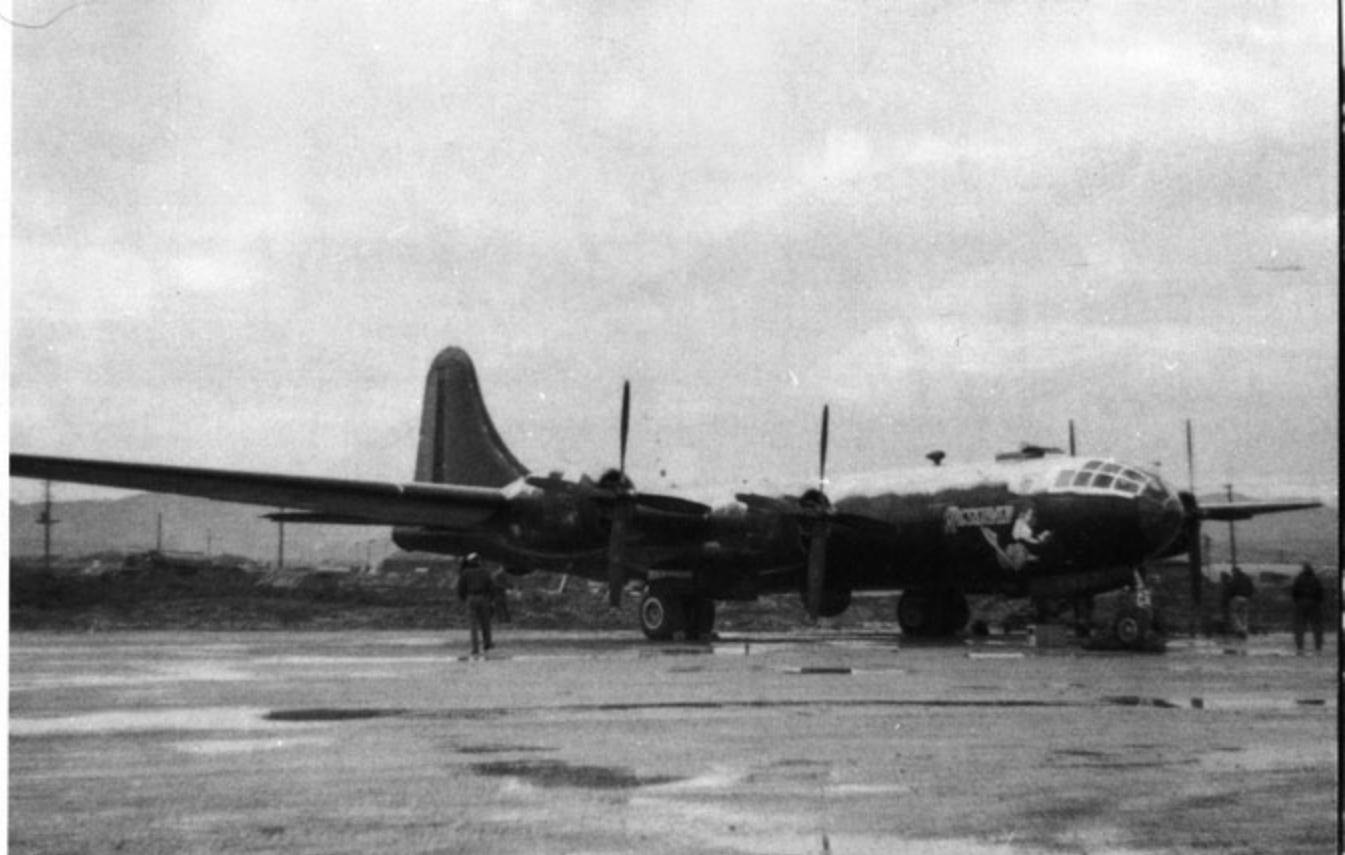
RESERVED , a 98th BG B-29 based at Yokota AB, Japan in late 1951, wears the Gloss Black camouflage after MiG attacks forced FEAF Bomber Command to fly night missions. (M.H. Havelaar)
