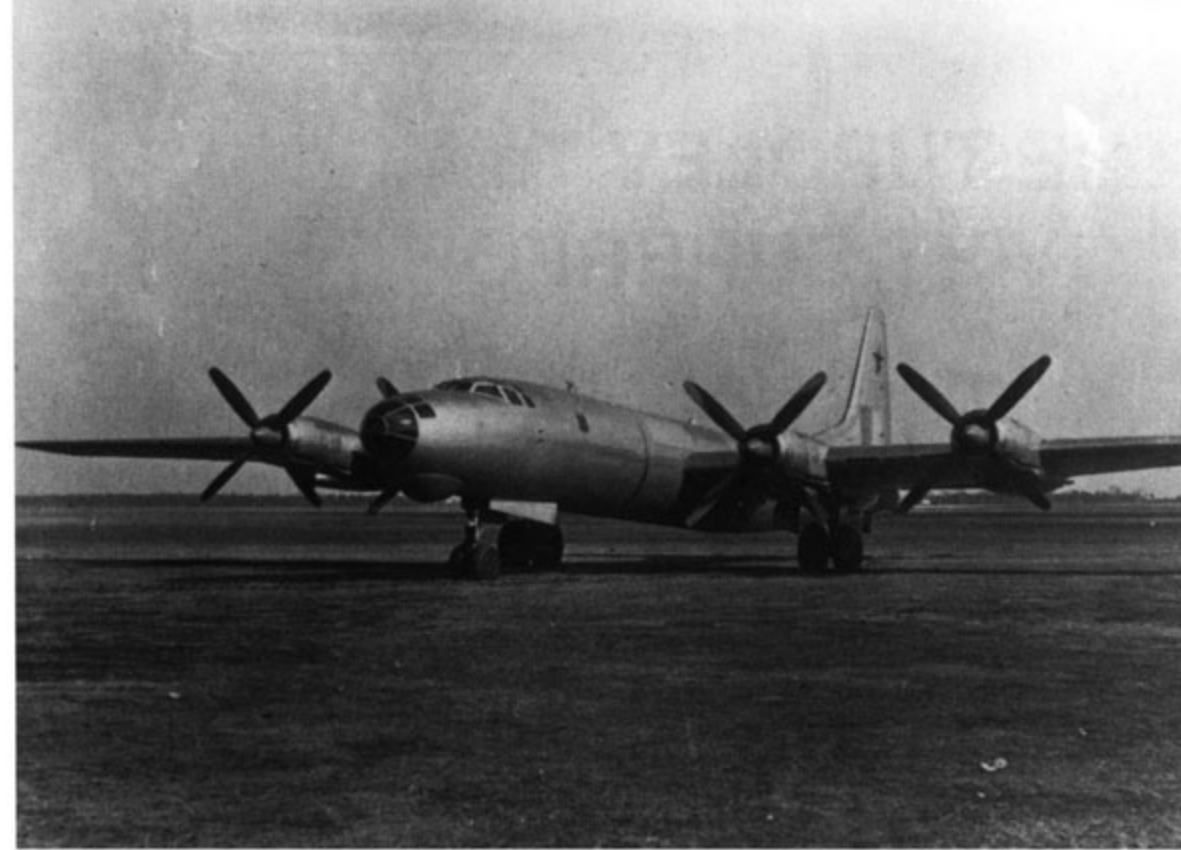
The Tu-80, the successor to the Tu-4 strategic bomber, with a stepped nose and wings moved to the middle of the fuselage is beginning to take on a definite Tupolev look. (Hans-Heiri Stapfer)
