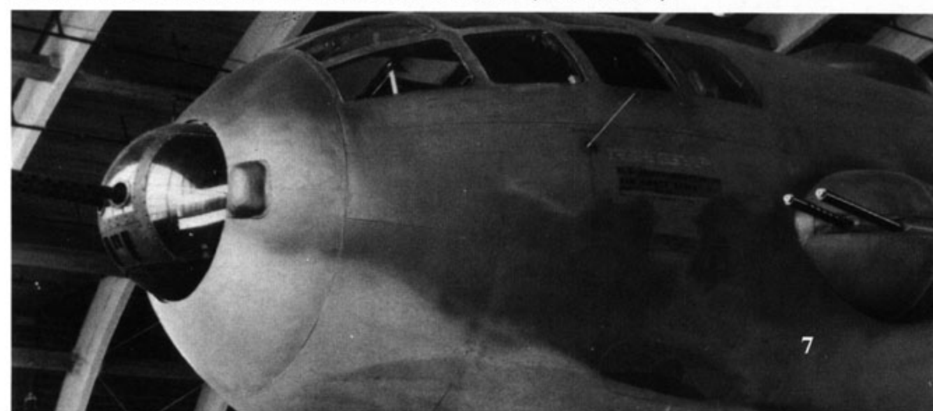
(Above / Below) The seventh YB-29 was experimentally fitted with an ERCO ball turret in the nose, and twin gun turrets on the fuselage sides that had originally been developed for the Convair PB4Y-2 Privateer and B-32A Dominator. (Peter Bowers)
