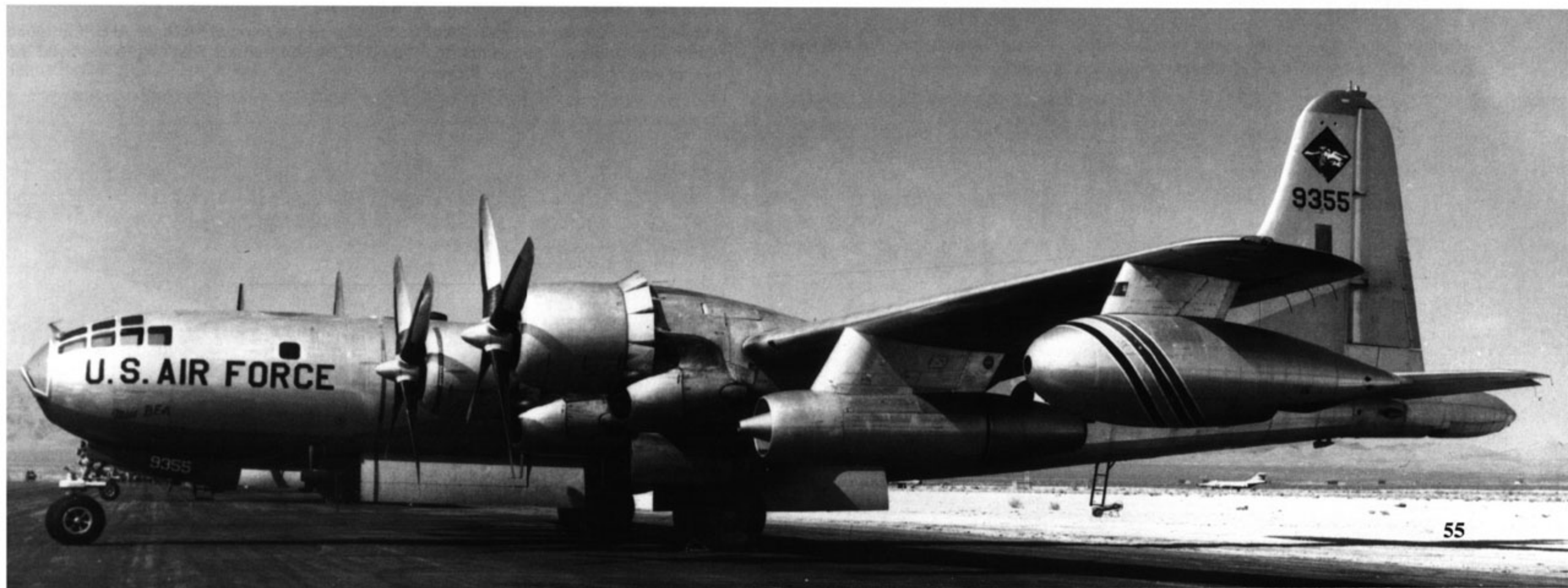
(Below) Miss BEA was a KB-50J assigned to the 421st Air Refueling Squadron in 1964. Many KB-50Js had General Electric J47 jet engines installed on the out board wings in order to increase their speed, making them more compatible with the TAC jet fighters they had to refuel. (E.M. Sommerich)
