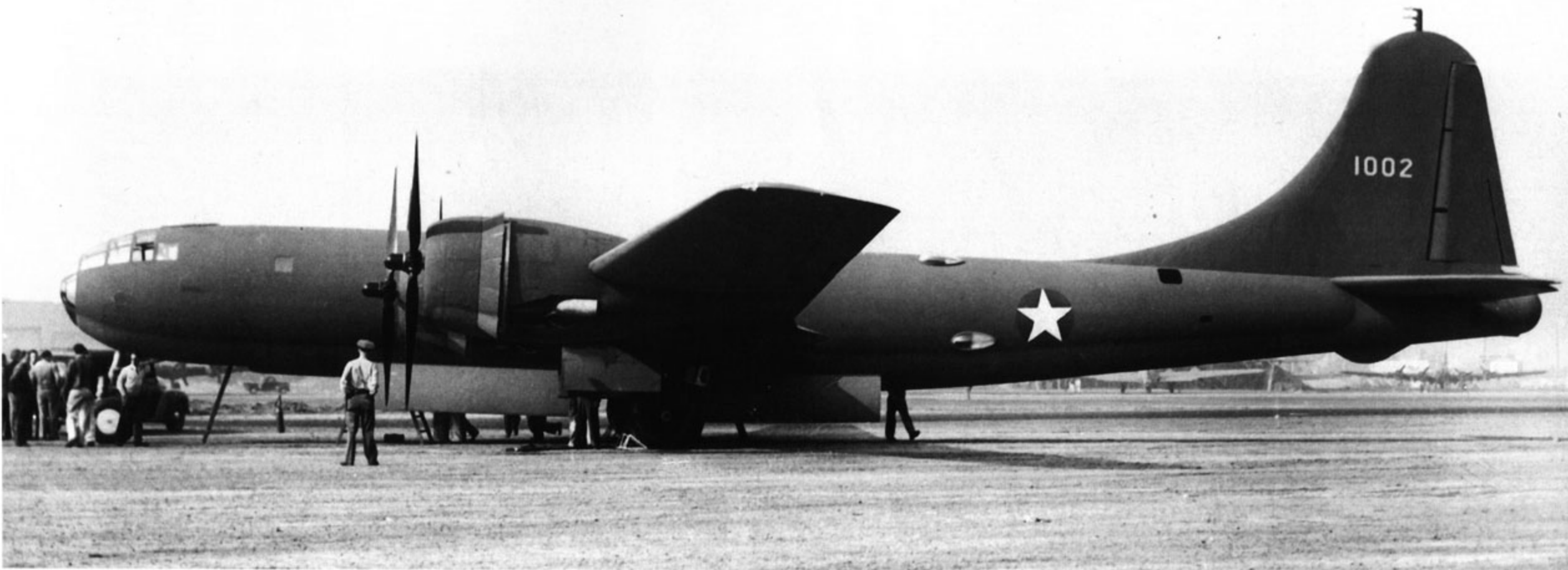
Rollout of the XB-29 came during early September of 1942. The tail bumper, small tail gunners windows, and larger rudder were found only on the XB-29s (Peter Bowers)
