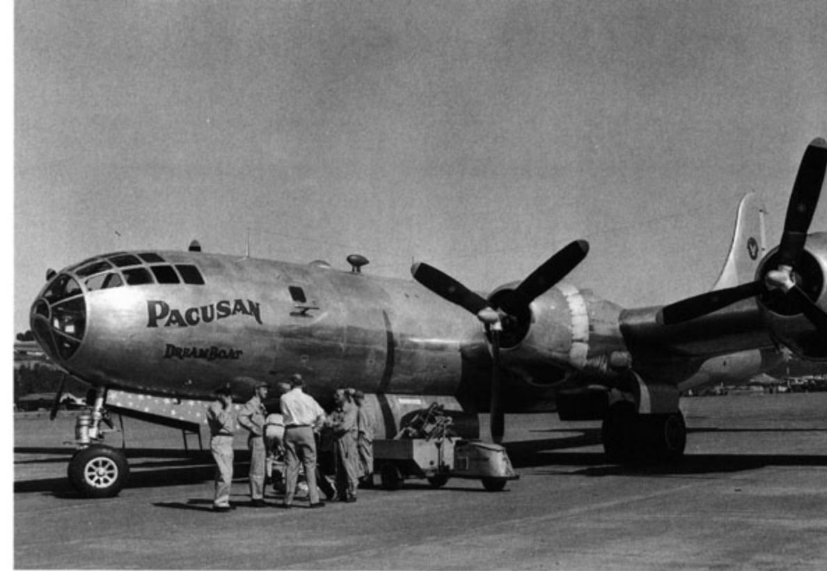
PACUSAN DREAMBOAT flew 8,198 miles non-stop from Guam to Washington, D.C., DREAMBOAT had the so-called 'Andy Gump' engine nacelles installed which were slated for production on the B-29. The SAC 'Milky Way' has been painted on the nose gear doors. (David Menard)
