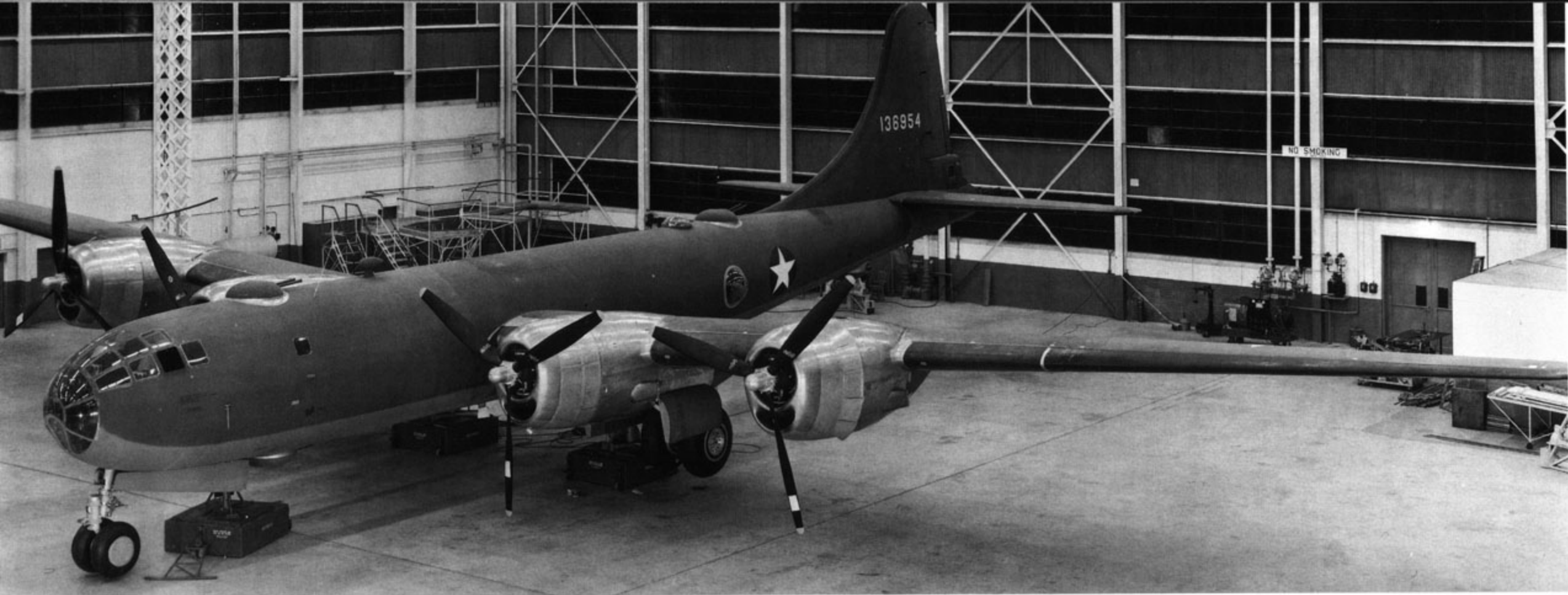
(Above) The first XB-29 on the portable scales at Boeing during June of 1943. The General Electric remote gun turrets have been installed, as well as new engine cowlings for the Wright R3350-13 engines. (Peter Bowers)
