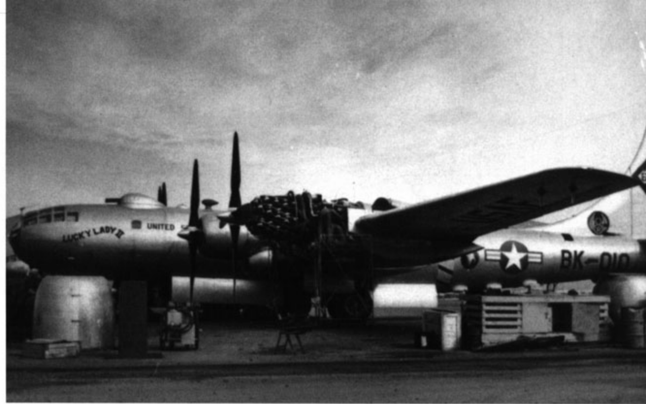
LUCKY LADY II (46-10), a B-50A of the 43rd Bomb Wing, using inflight refueling flew non-stop around the world between 26 February and 2 March 1949, flying 23,452 miles in 94 hours. The distinctive 'corn-cob' cylinder configuration of the P&W R-4360 engines is obvious when the cowling is removed for maintenance. (USAF)
