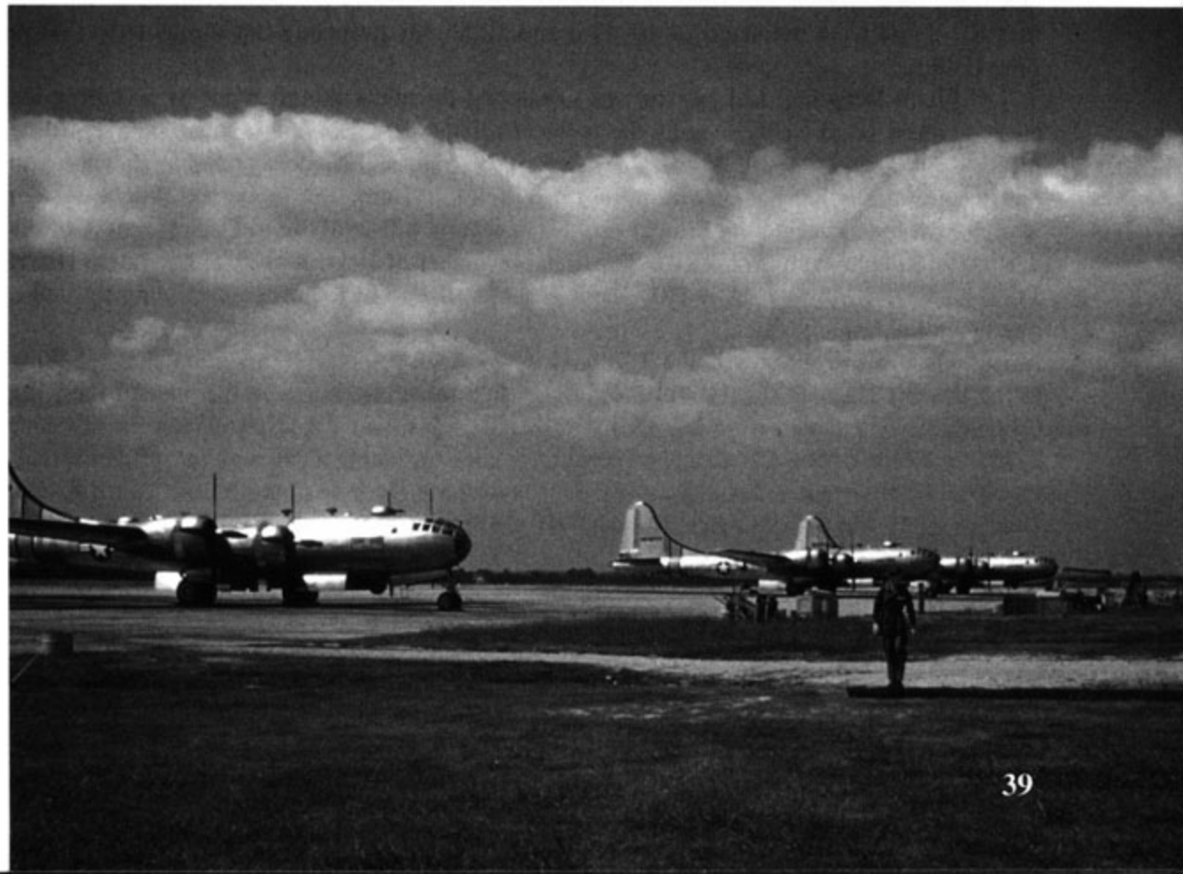
(Below) A trio of Air Rescue Service SB-29s at Maxwell AFB, AL in 1951. When a lifeboat is not being carried the bomb bay doors can be opened. Additional fuel and rescue supplies were carried in the bomb bays. (Robert Mikesh)
