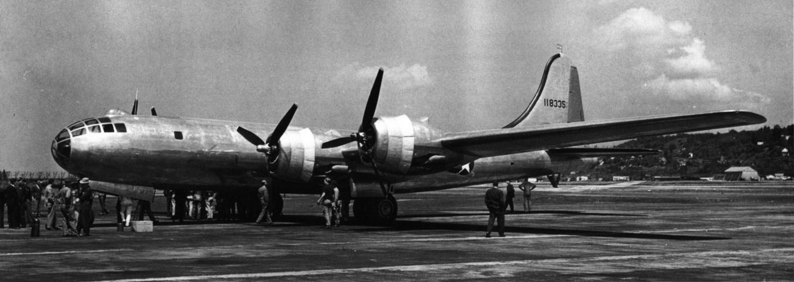
The 3rd XB-29 on the ramp at Boeing Field in of June 1943, showing the teardrop-shaped astrodome above the canopy. The three blade propellers were common to all three XB-29s. (Peter Bowers)
