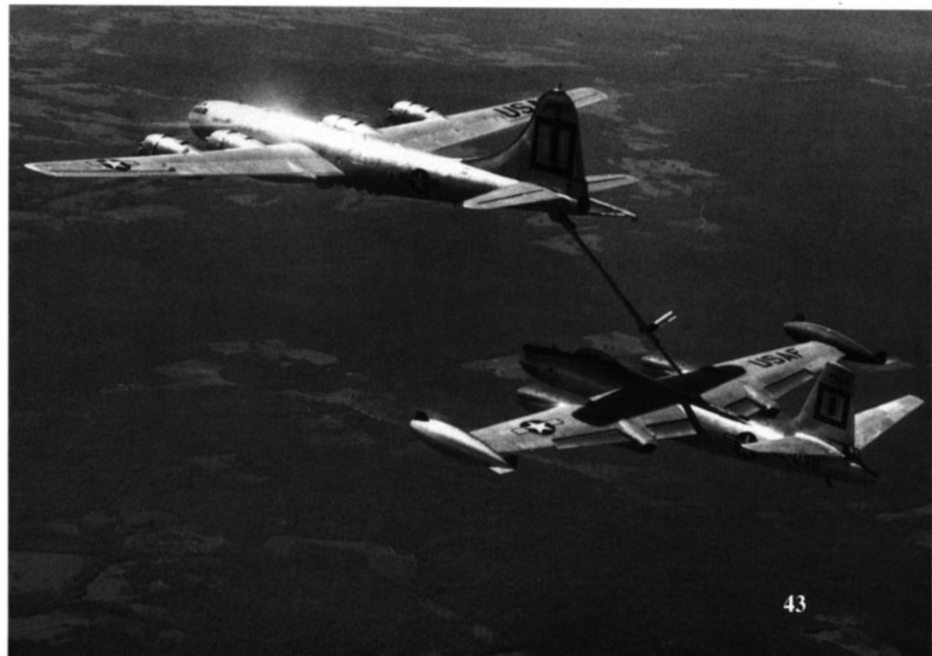
(Below) An RB-45C from the 91st Strategic Reconnaissance Squadron hooks up to a 91st ARefS KB-29P over Japan during the Korean War. The RB-45C needed inflight refueling to reach its assigned target areas on or above the Yalu River. (USAF)
