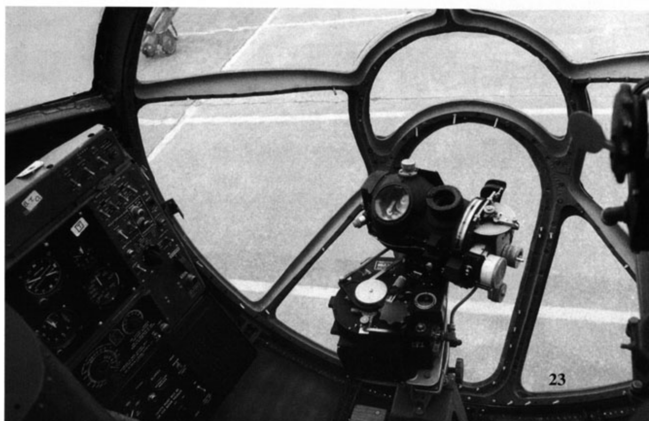
The most classified instrument in the Army Air Force was the famous Norden bomb sight, rarely seen in any photographs. (Larry Sutherland)
