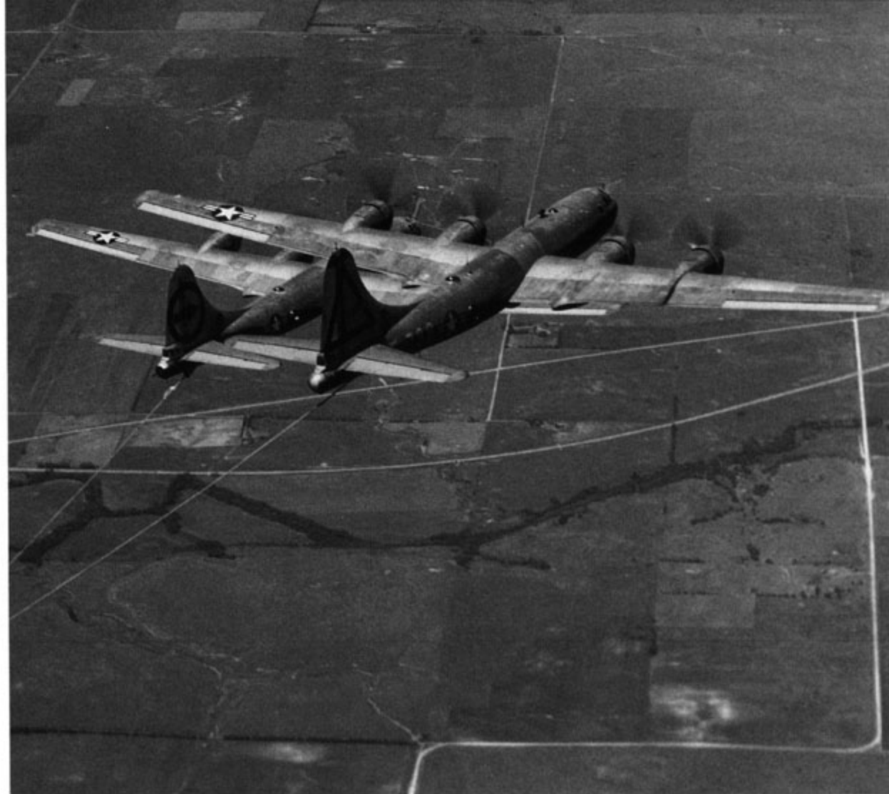
The upper aircraft is a KB29M tanker of the 509th Air Refueling Squadron that has deployed the fueling hose and made contact with, and is refueling a B-29MR of the 509th Bomb Group. The hose was snagged in mid-air by the B-29MR crew and dragged inside where it was plugged into the refueling receptacle. (Peter Bowers)
