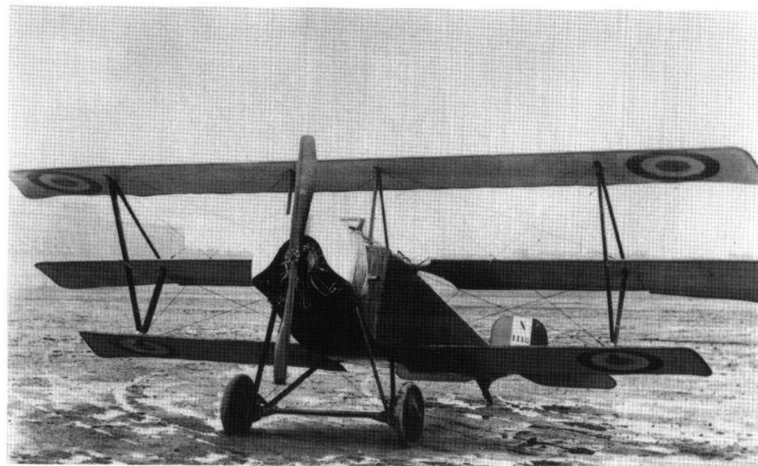
This triplane wearing French national markings and the number 1448 on the rudder appears to have been based on an Nie.11 fuselage and differs from others in having a positive stagger to the wings.
