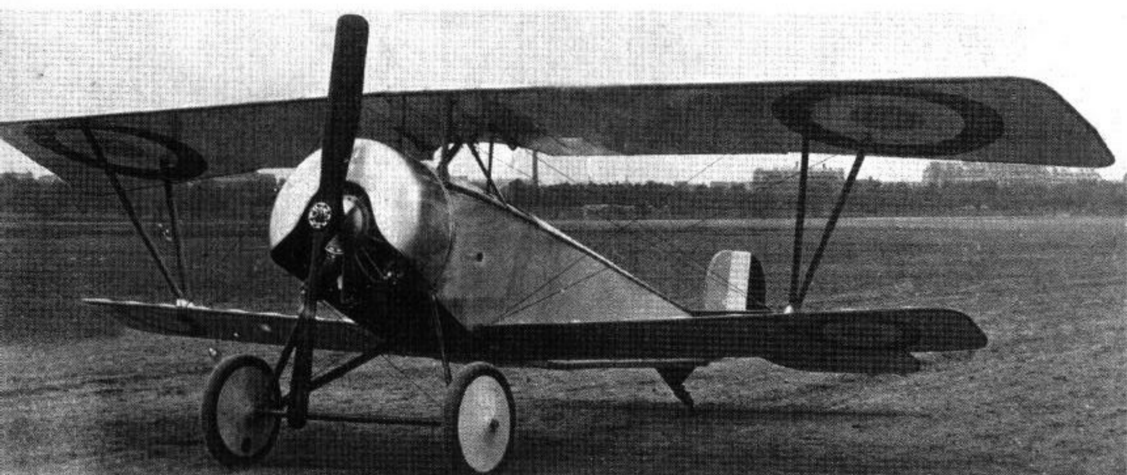
This French Nie.11 appears to have a revised, non-standard wing bracing system.
