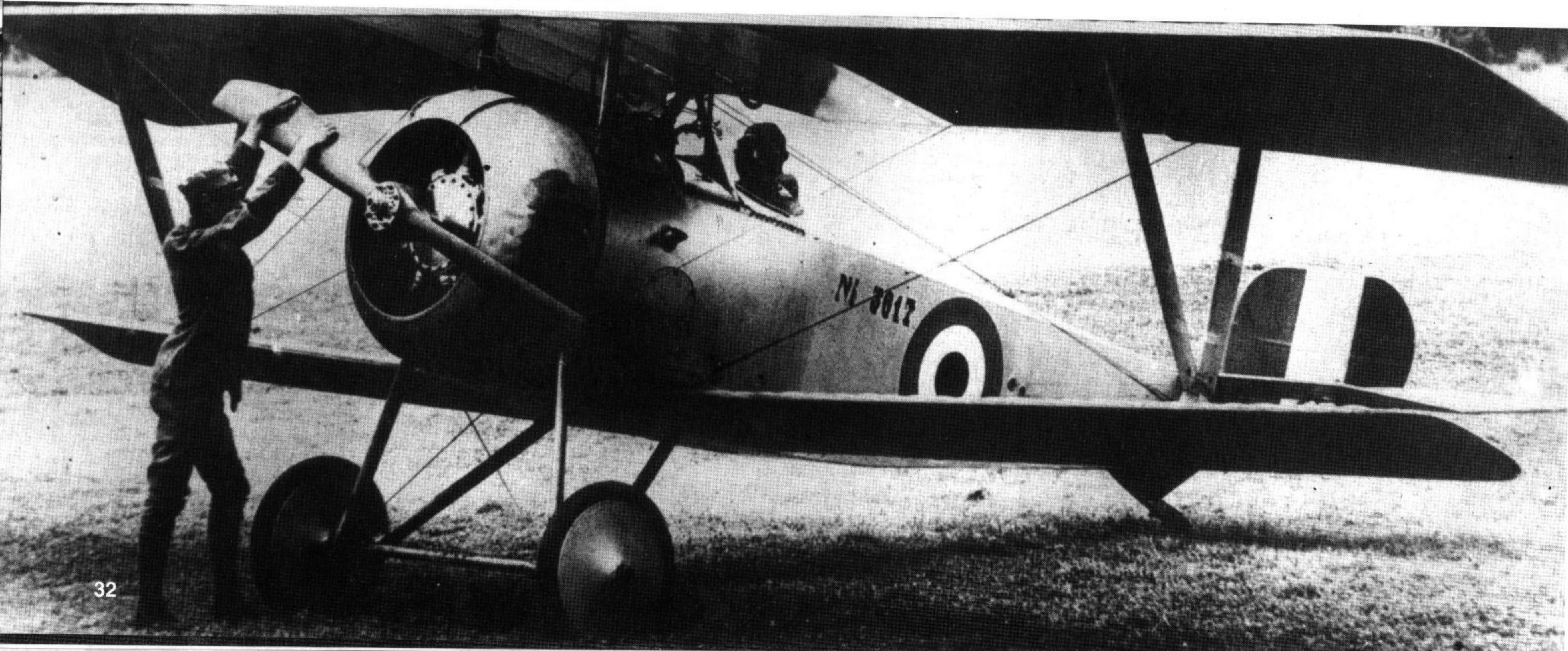
An Italian machine marked Ni 3817; the location of the number and their shaded presentation were features of Macchi built Nieuports. Roundel proportions differ from those of France or Britain.
