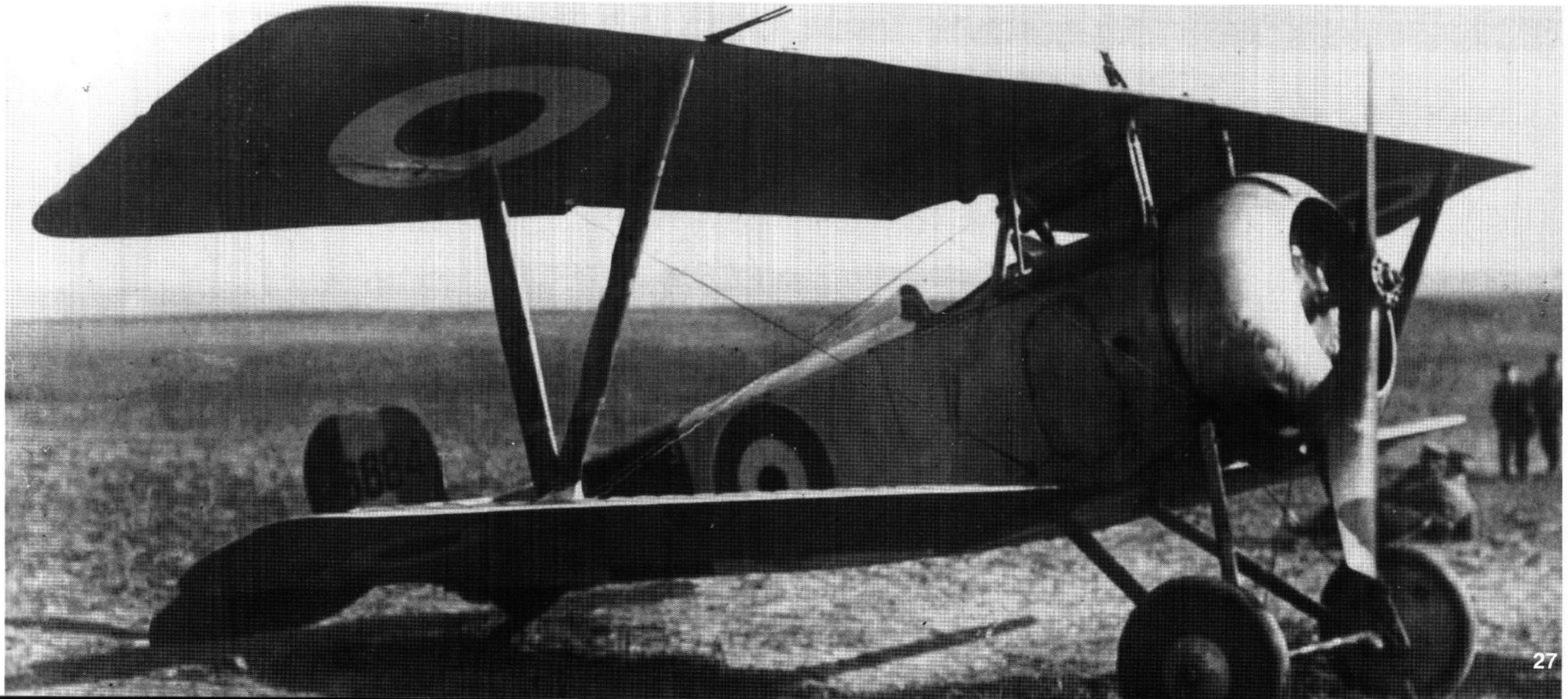
An Nie.17 believed to be of No.1 Squadron RFC, the first RFC unit to be fully equipped with the type, January 1917. With its Lewis gun on a mounting resembling those found on French examples, this aircraft carries a prominent Aldis sight.
