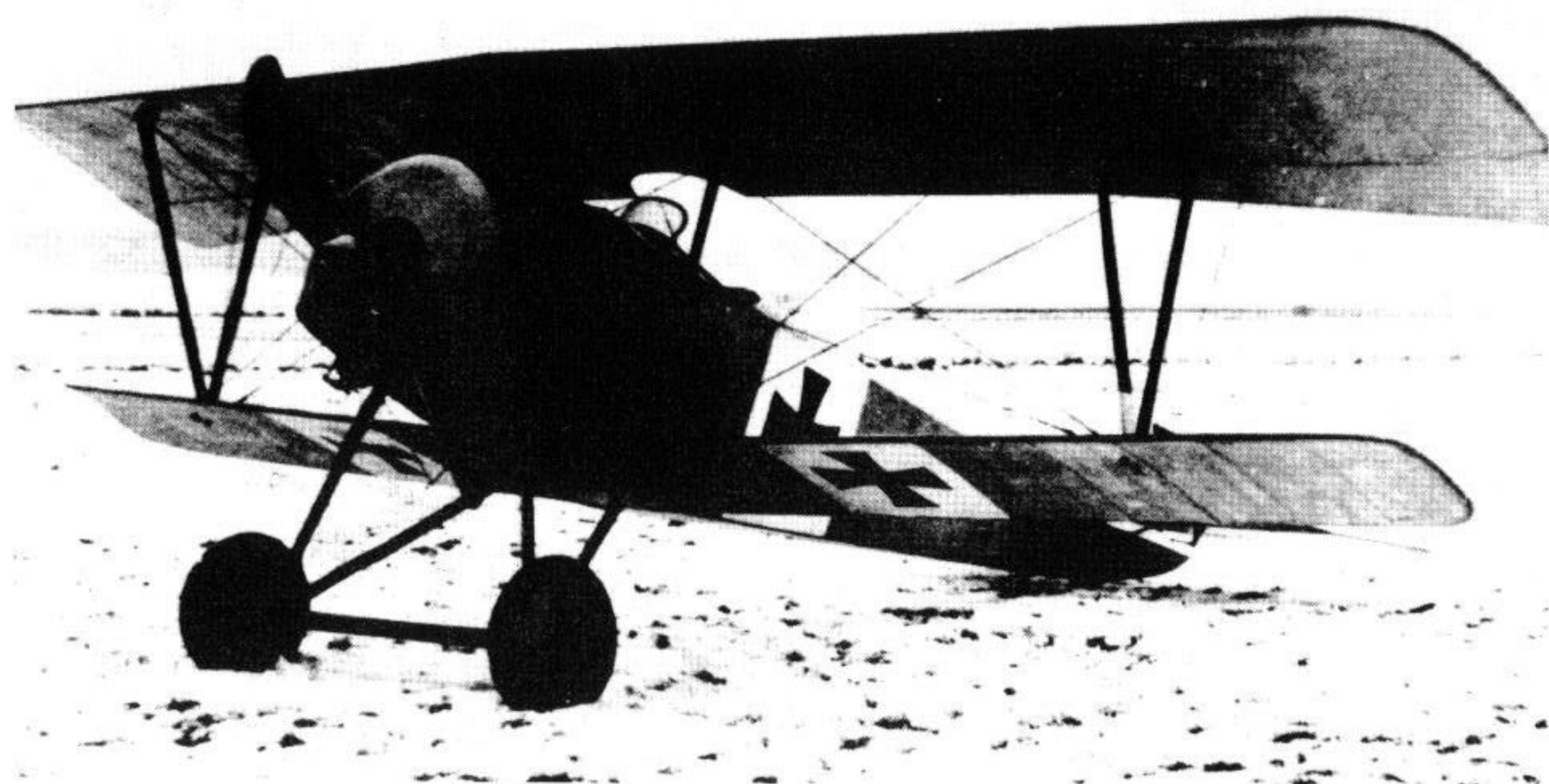
One of several Nie.11s that fell into German hands and were test flown. The armament has been removed and a small cone de penetration has been added to the airscrew boss. The extreme inboard position of the national markings under the lower wing is unusual.
