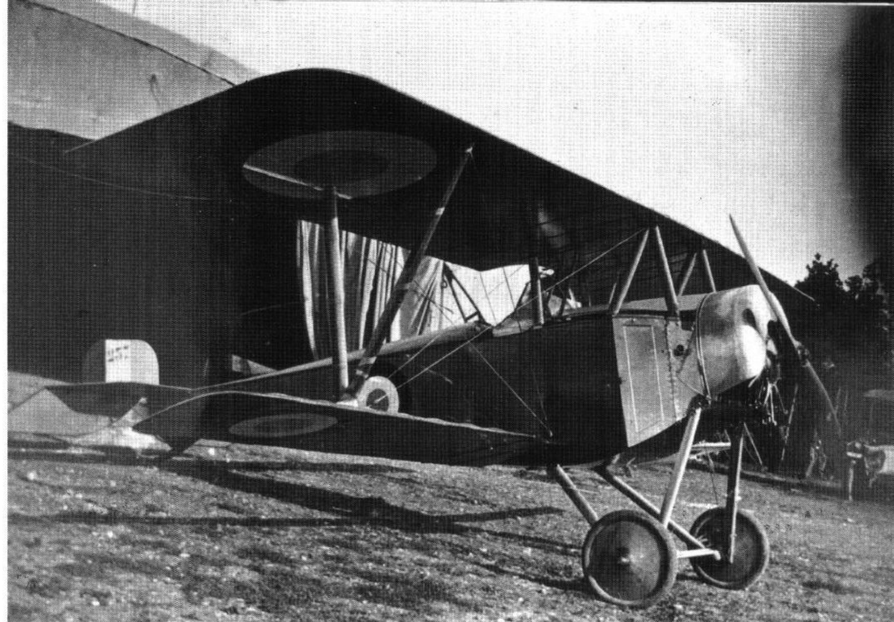
This Nieuport 10 single seater, wearing French colors, carries the number 237 on the rudder. The V struts can be seen between the upper and lower wing. Armament is a single, centrally mounted, overwing Lewis gun.
