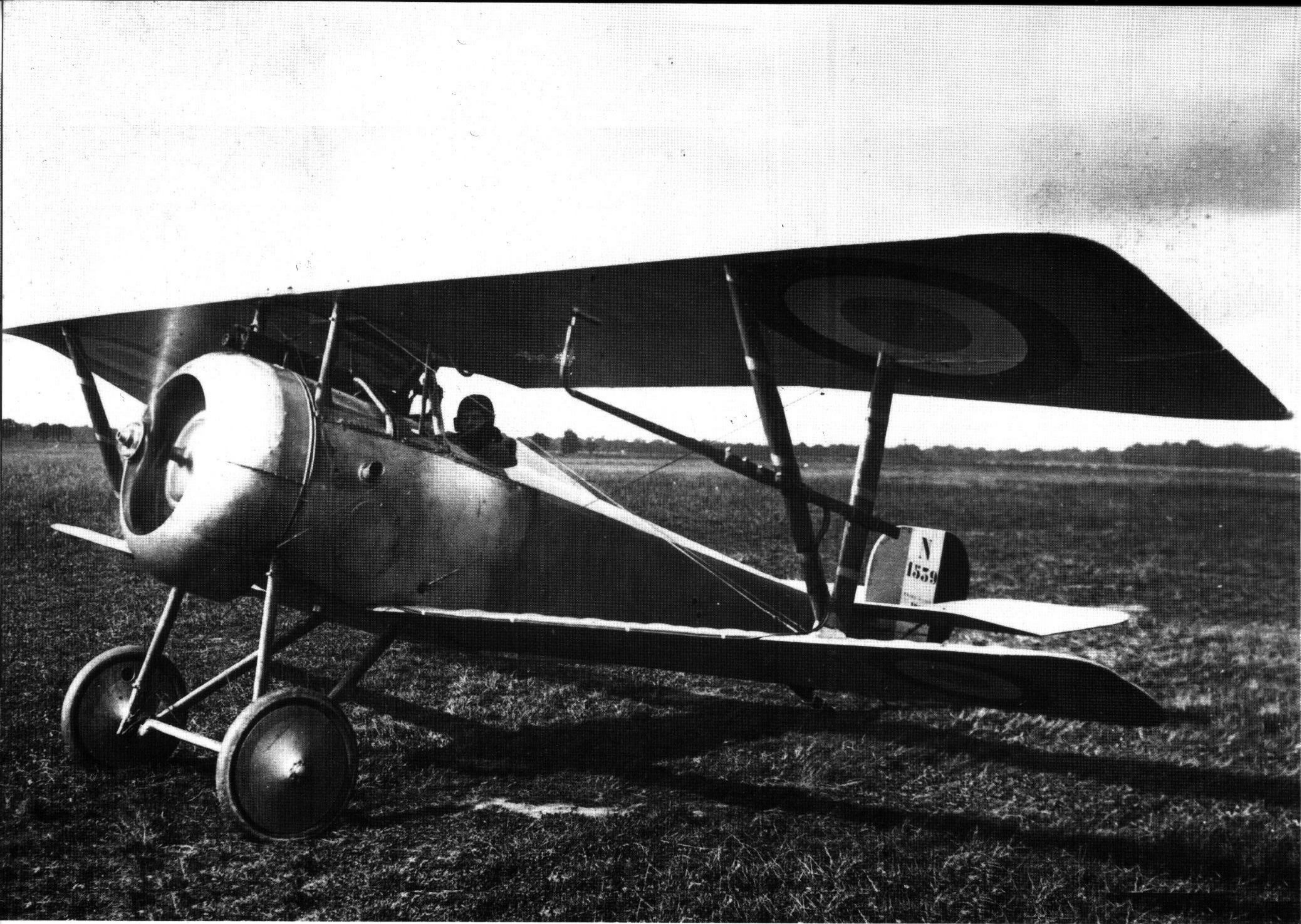
A French Nie.17 numbered N1539 with a fuselage mounted Vickers gun and an experimental venturi tube on the port wing struts.
