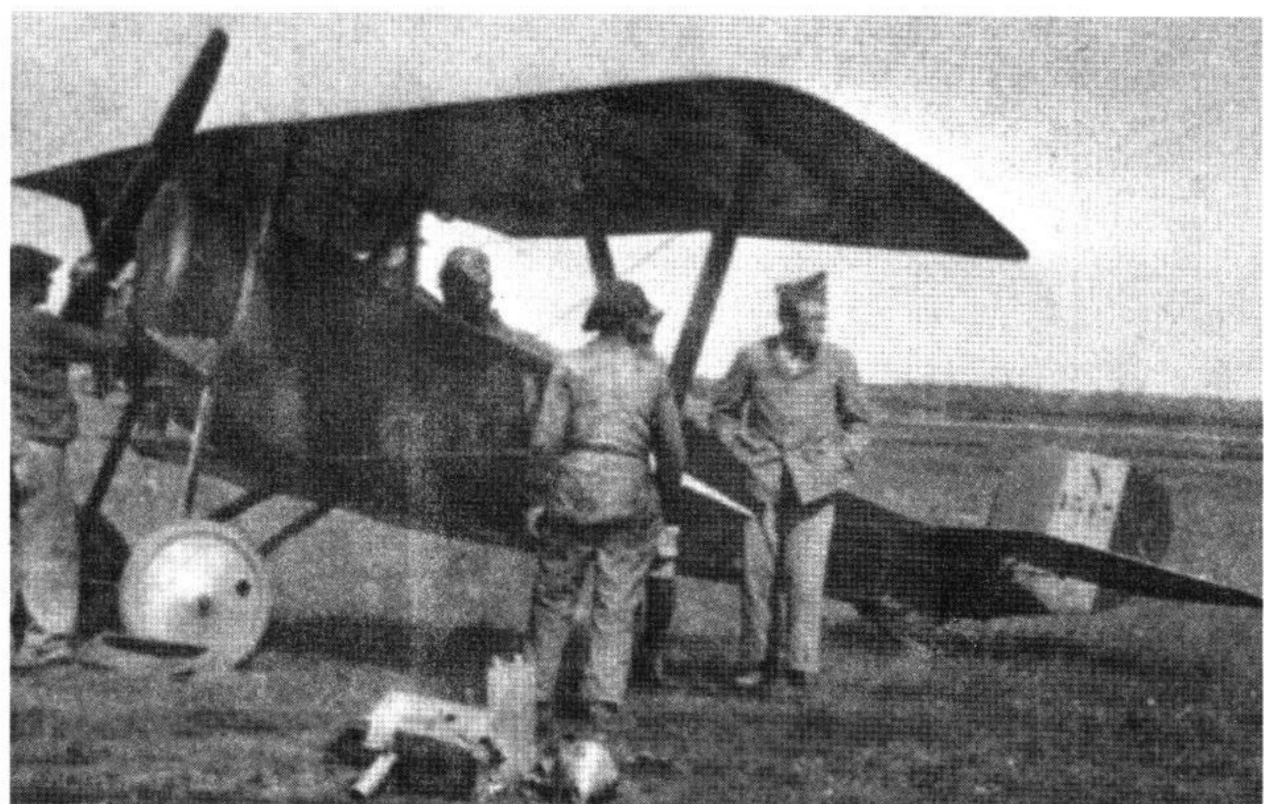
This Nie.11 (N1374), operating with a French unit in the Dardanelles, is having its 80-hp Le Rhone rotary engine serviced.
