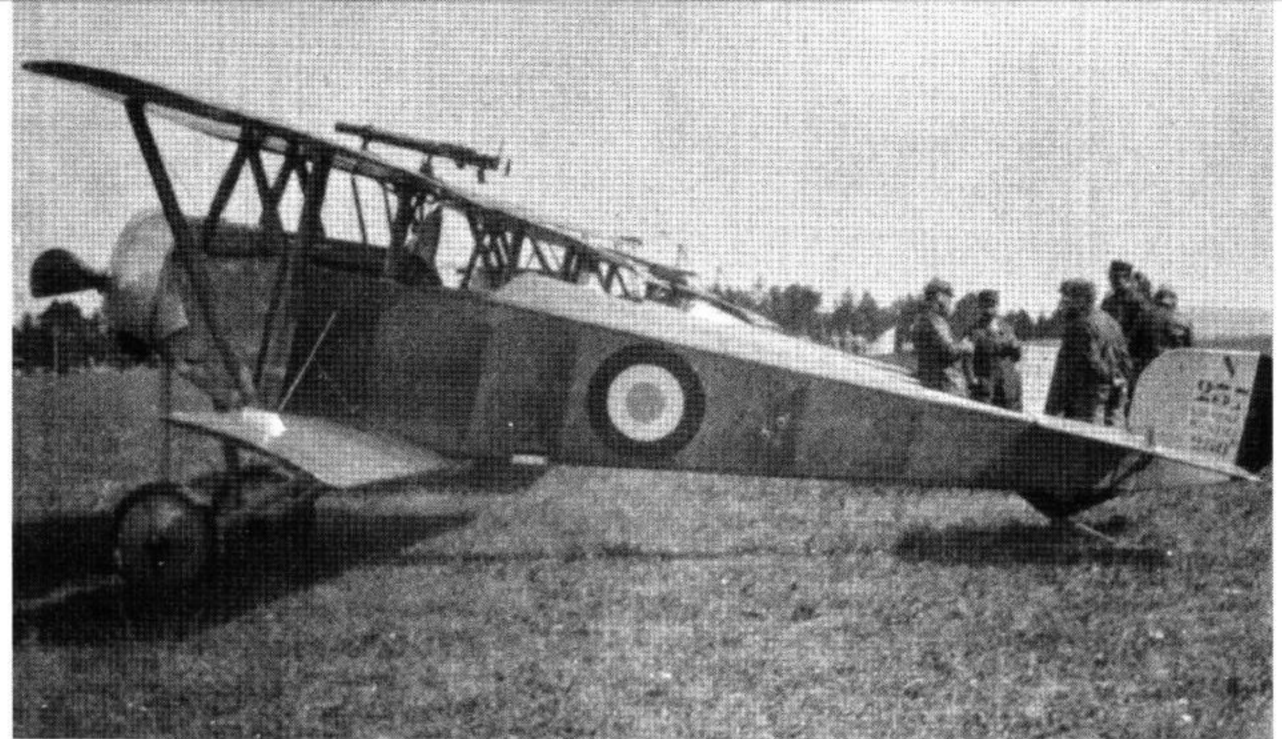
(Above) A carry over from the days of the two seater, the Nieuport 10 has the characteristic look of an elongated two seater fuselage.
