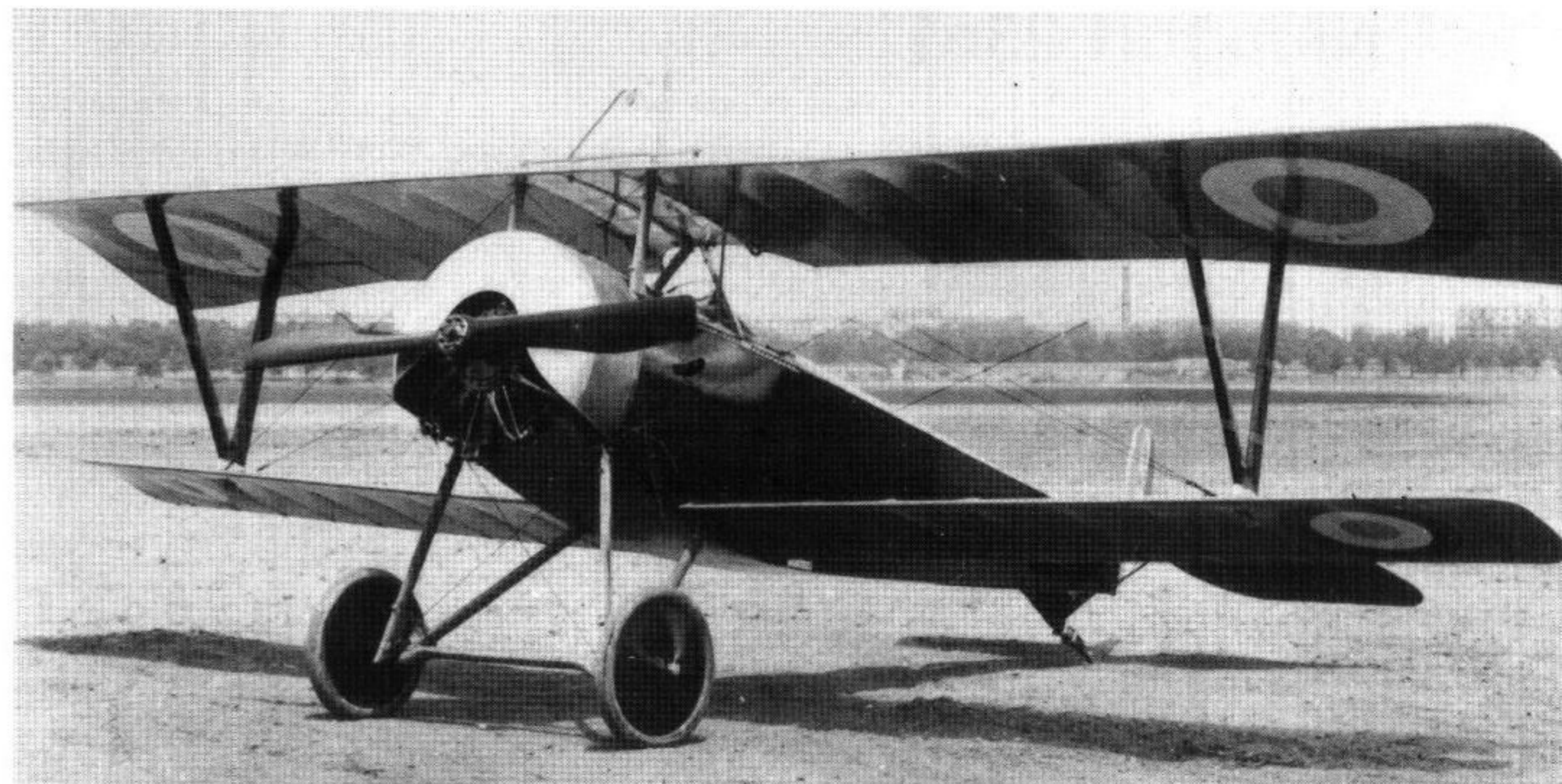
(Above) A newly completed Nie.21 ready for allocation to an escadrille. It has an over wing mounting for the armament and transparent panels in the center of the upper wing.
