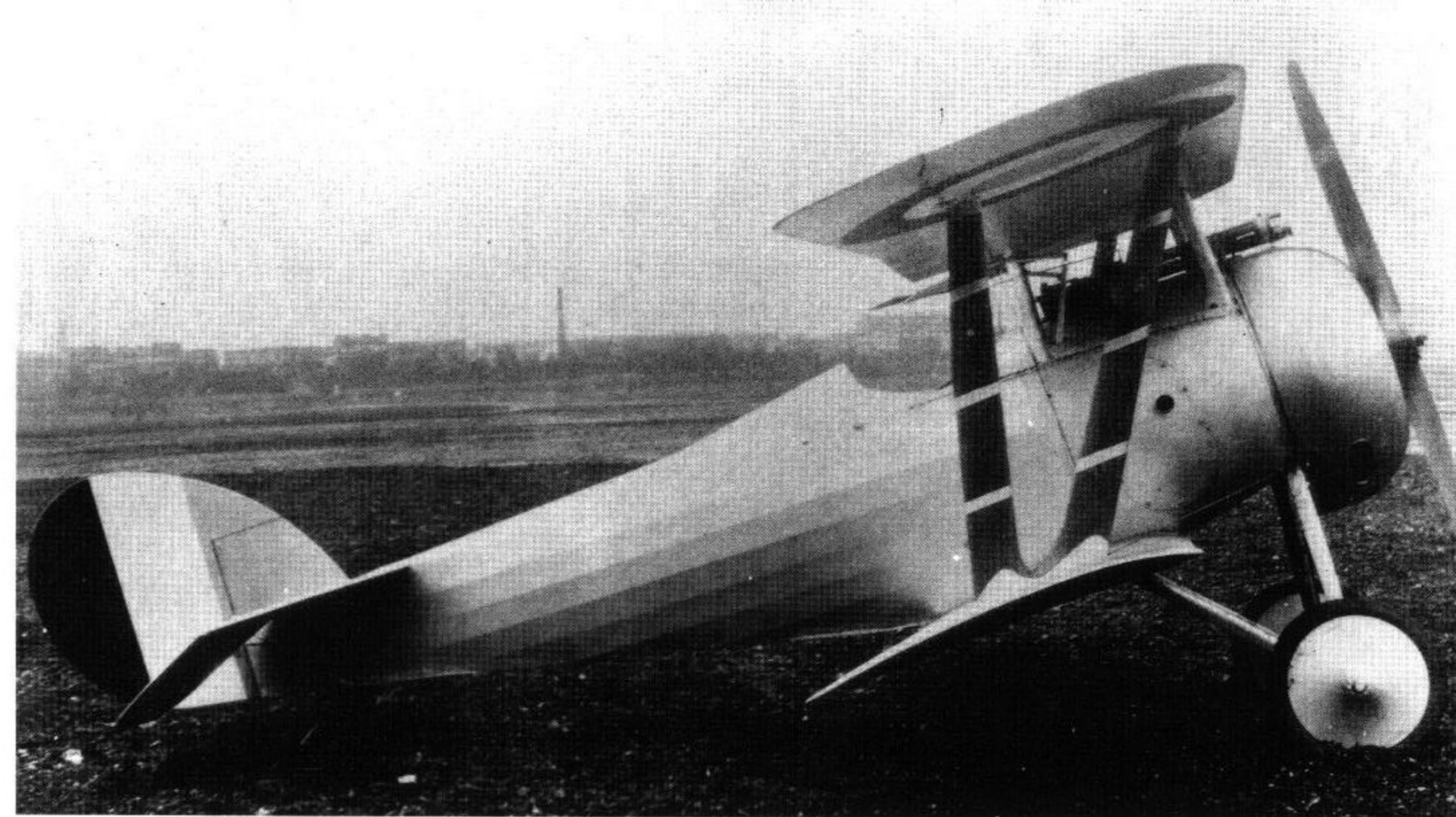
An unnumbered prototype with wings of an increased chord on the airframe of an Nie.27. This attempt to direct design trends in a fresh direction contributed much to the evolution of the Nie.28.
