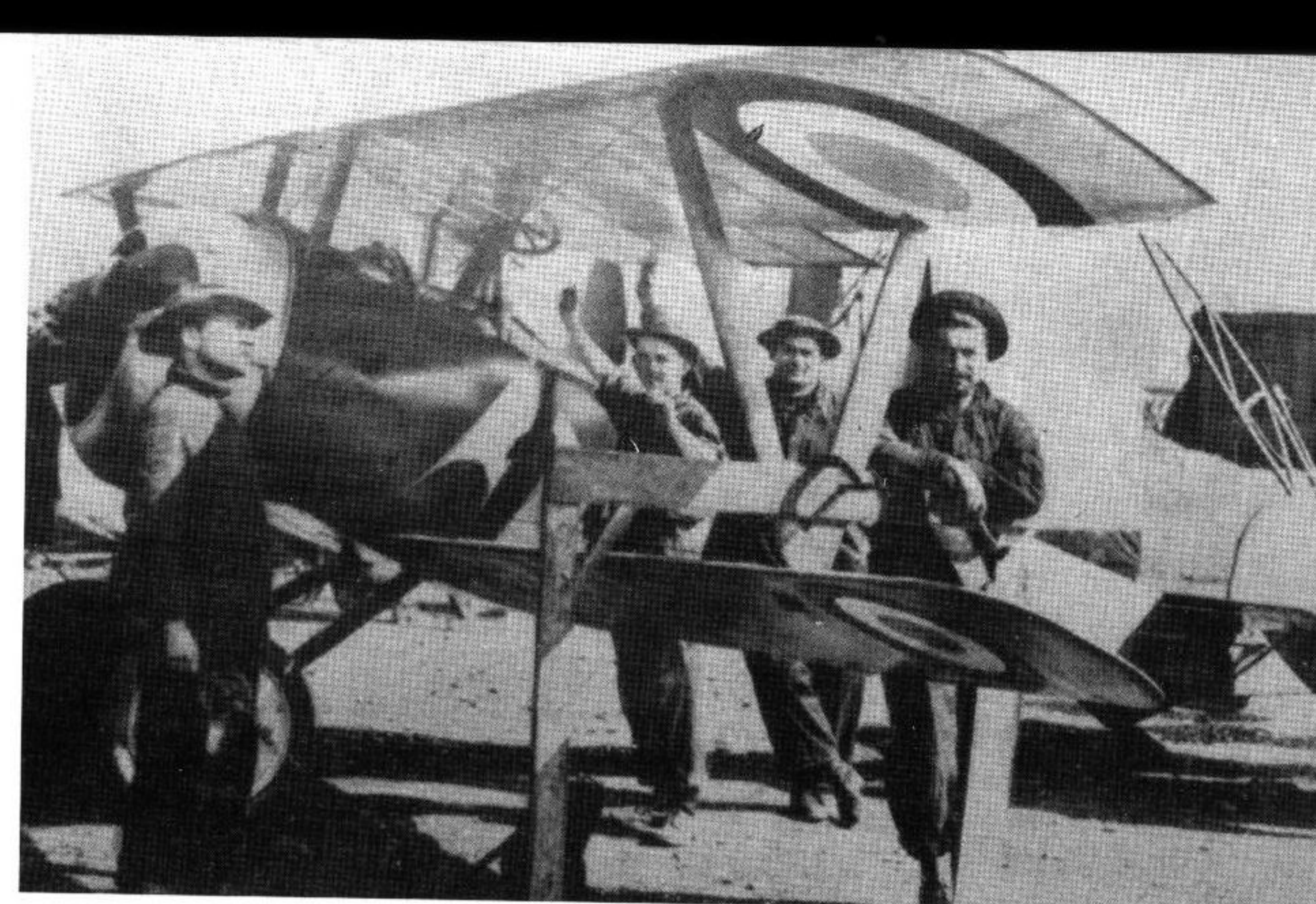
An Nie.17 under repair at the American Aviation School on Field No.2, Isseudon in France during May 1918. The diagonal girder to the right supports a Bessoneau canvas hangar.
